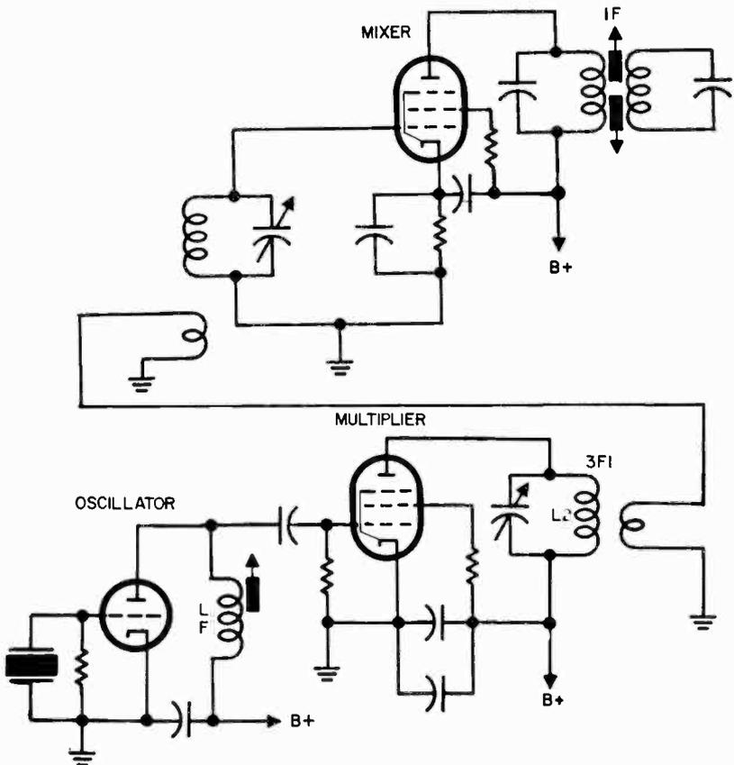
Fig. 1114. Local oscillator, multiplier and mixer circuits. Only one multiplier is shown. Some receivers use several frequency multipliers.
