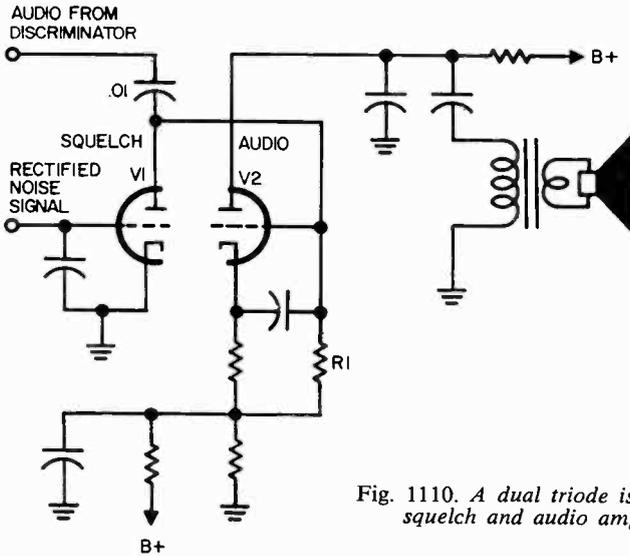
Fig. 1110. A dual triode is used as a squelch and audio amplifier.
