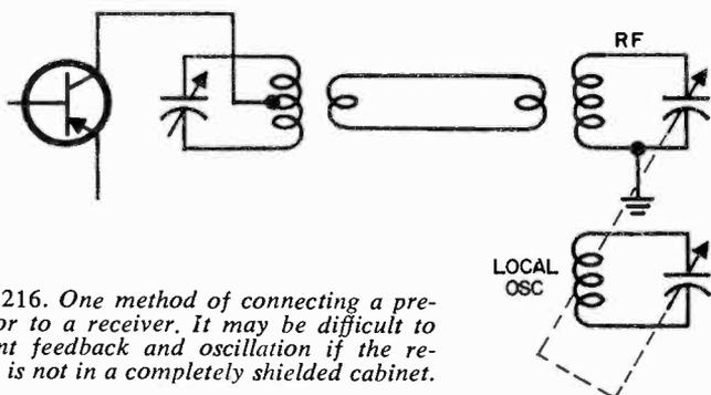
Fig. 1216. One method of connecting a preselector to a receiver. It may be difficult to prevent feedback and oscillation if the receiver is not in a completely shielded cabinet.
