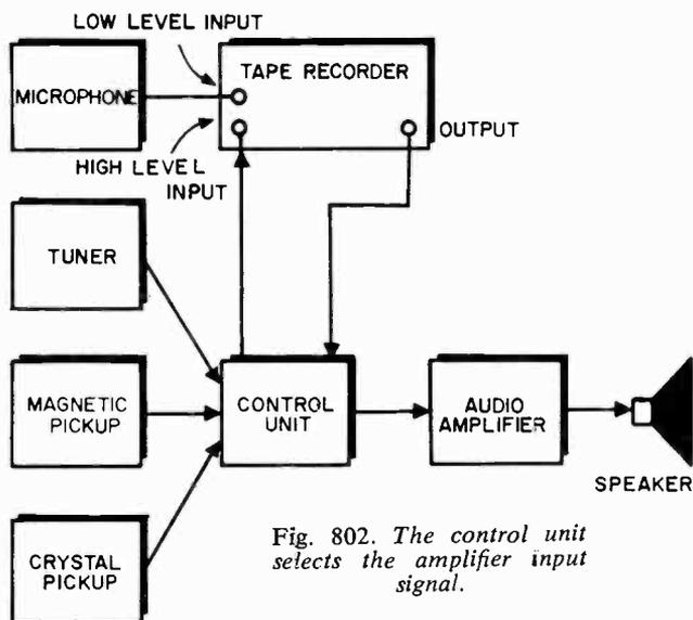
Fig. 802. The control unit selects the amplifier input signal.
