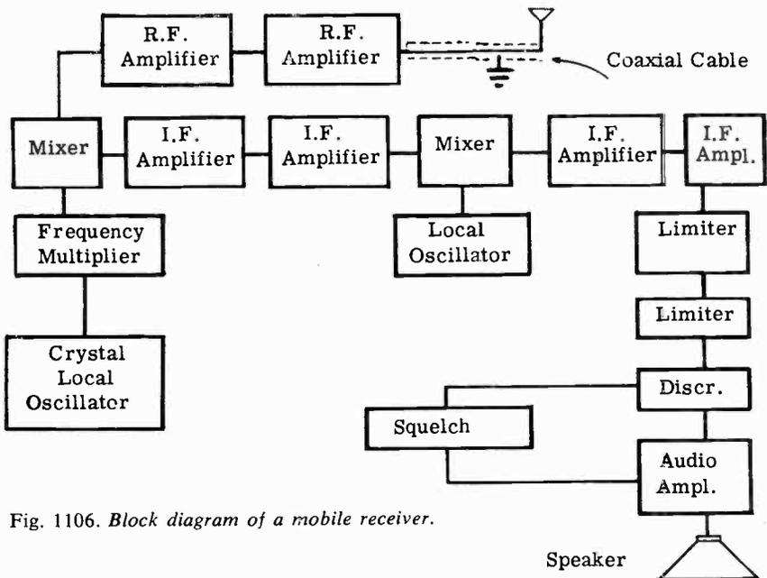
Fig. 1106. Block diagram of a mobile receiver.
