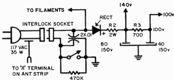
Fig. 609. Semiconductor units are often used in place of rectifier tubes.
