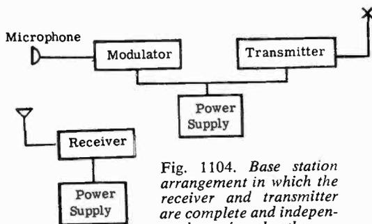
Fig. 1104. Base station arrangement in which the receiver and transmitter are complete and independent of each other.
