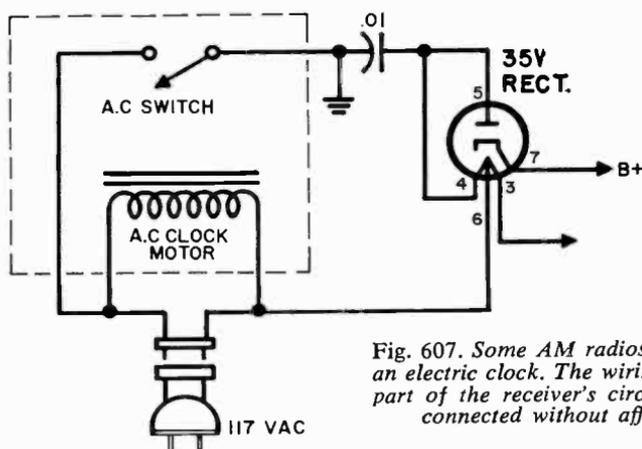
Fig. 607. Some AM radios come equipped with an electric clock. The wiring of the clock is not part of the receiver's circuits and can be disconnected without affecting the radio.
