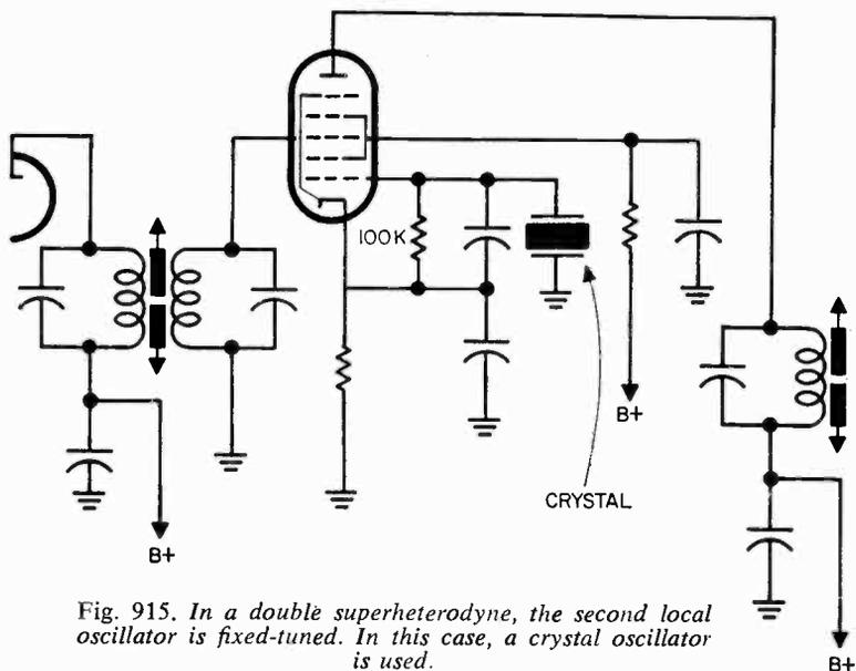
Fig. 915. In a double superheterodyne, the second local oscillator is fixed-tuned. In this case, a crystal oscillator is used.
