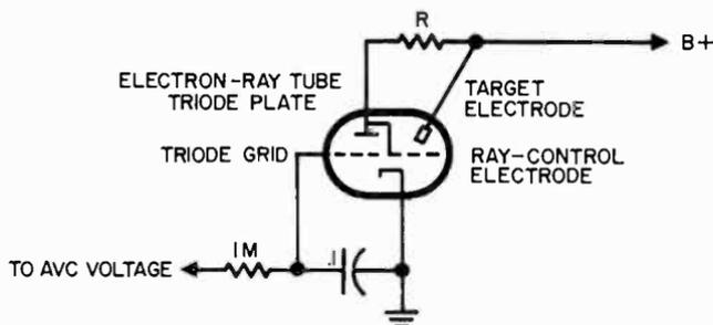
Fig. 820. *Indicator-tube circuit. Indicator tubes are often used with FM receivers or tuners.*
