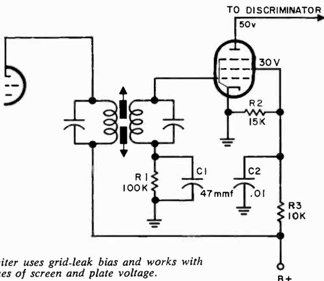
Fig. 717. The limiter uses grid-leak bias and works with low values of screen and plate voltage.
