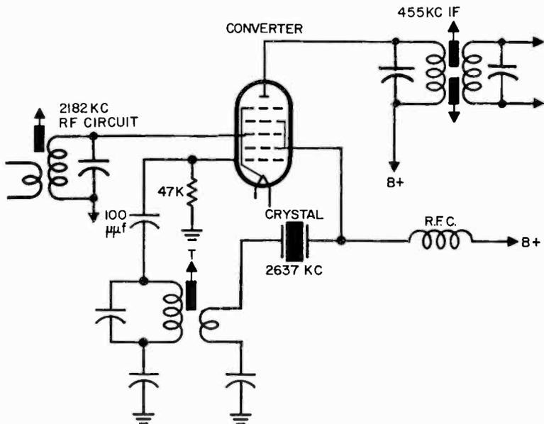
Fig. 1015. Crystal control of the local-oscillator circuit.
