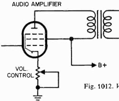
Fig. 1012. Volume control in the cathode circuit.
