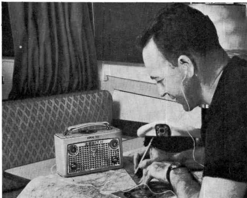
Fig. 1002. Two-band transistor portable covers the standard AM broadcast band and the radio-beacon band. (Zenith Radio Corp.)
