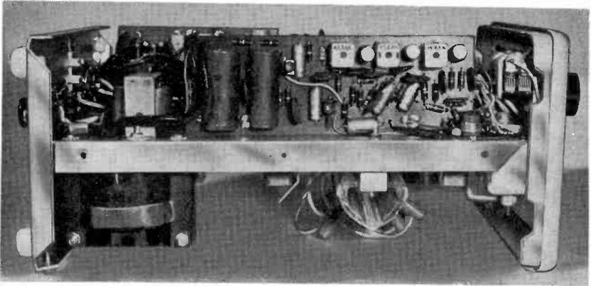
Fig. 1017. Side view of transistorized receiver.
