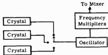
a doubler. This multiplies the frequency by 2, giving us 72 mc. By using another doubler circuit, we manage to get our local oscillator up to 144 mc.
