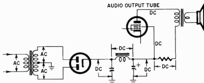
Fig. 703. *Ac and dc voltage points in a power supply. All voltages, starting at the cathode of the rectifier, are dc. All voltages, starting at the rectifier plates and going back to the power line, are ac. The voltage drops across the filter capacitors, the filter choke and the filter resistor are dc. All tube voltages (no signal input) are dc.*
