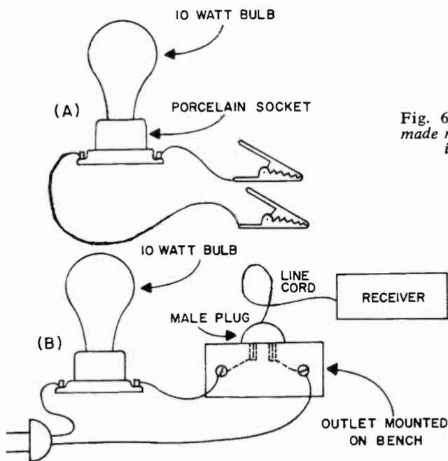
Fig. 604. Some home-made methods for checking filaments.
