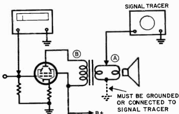
Fig. 617. Signal-tracing the audio power amplifier stage.
