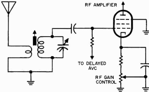
Fig. 919. *Rf gain-control circuit.*
