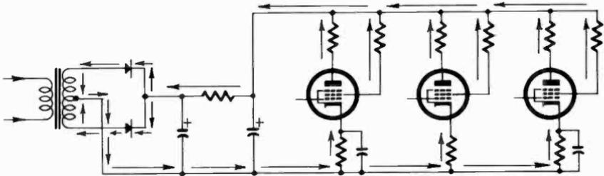
Fig. 705. The tubes in most circuits are connected in parallel. The current that flows through the tubes must also pass through the rectifier. The more tubes, the heavier the load (that is, the greater the amount of current). As you remove tubes, less current will pass through the rectifier. The arrows show the direction of electron current flow.
