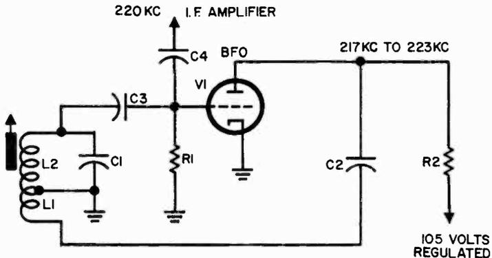
Fig. 905. This bfo is a Hartley oscillator.
