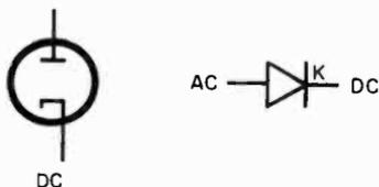
Fig. 704. Symbols for rectifiers used in power supplies. Up to and including the anode we have ac. From the cathode and beyond it we have dc.
