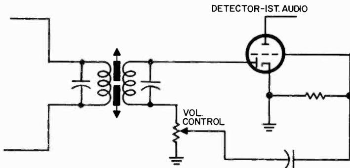
Fig. 1011. Volume control works as the diode load.
