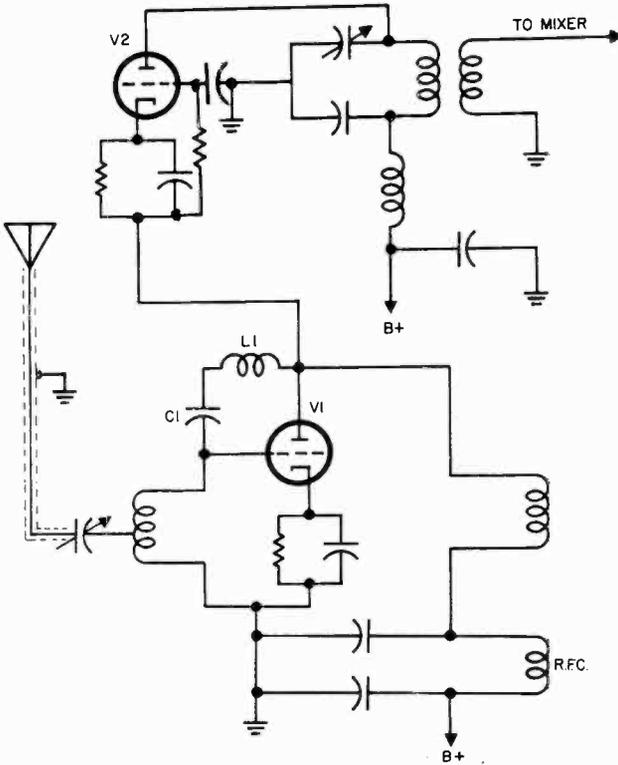
Fig. 1116. The cascode circuit is a voltage divider.
