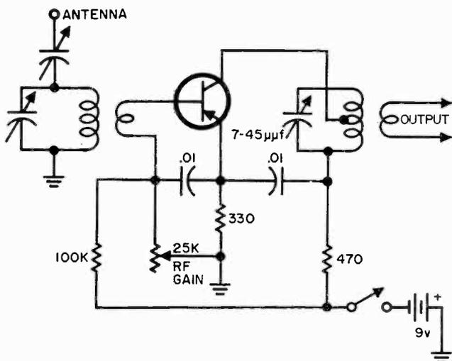
Fig. 1215. Preselector circuit is a tuned radio-frequency amplifier.
