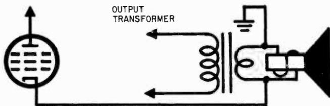
Fig. 615. Sometimes the voice coil is part of a negative feedback system. Transposing the ground connection on the voice coil to the wrong side will cause the audio amplifier to oscillate.
