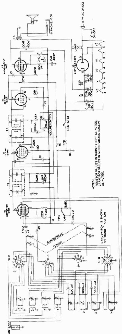
Fig. 908. Simple type of communications receiver. Rotary wafers switches are used to select any one of four different bands. The set has bandspread tuning. Regeneration is used in the first if for CW signals. (National Radio Co., Inc.)
