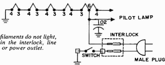
Fig. 605. If the tube filaments do not light, the trouble can be in the interlock, line cord, male plug or power outlet.
