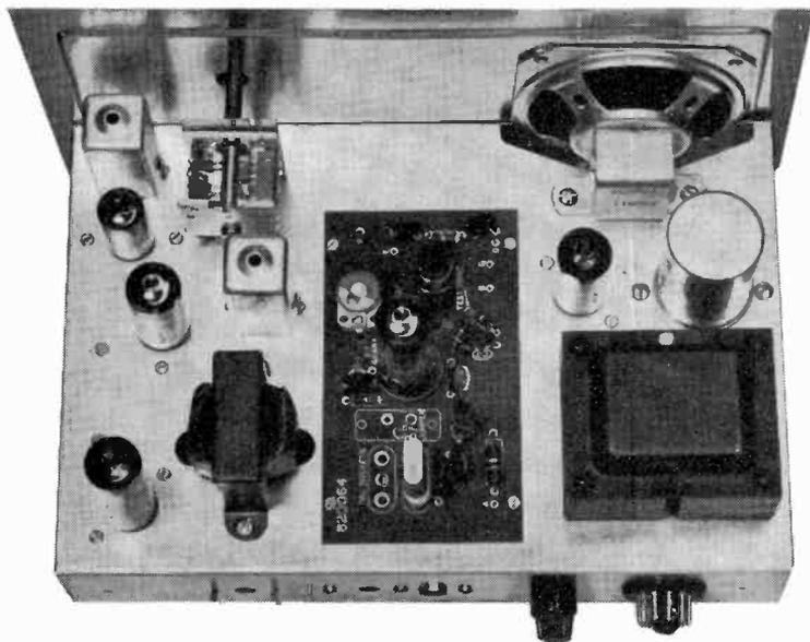
Fig. 1213. *Inside view of Citizens-band transceiver. The printed-circuit board is mounted on a chassis cutout. (Allied Radio Corp.)*
