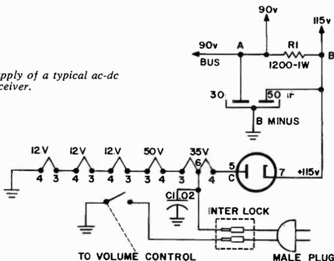
Fig. 606. Power supply of a typical ac-dc receiver.
