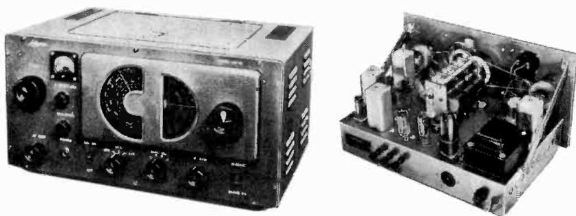
Fig. 910. *With 9 tubes and 10 controls this communications receiver chassis is not crowded. Speaker is in separate cabinet.*
