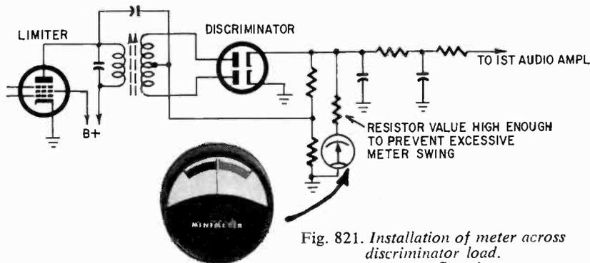
Fig. 821. Installation of meter across discriminator load.
