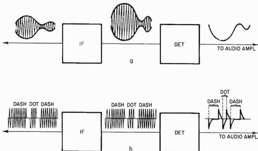
Fig. 903. Audio modulation on the rf/ca if signal (a) easily passes into audio amplifier. Code transmission (b) has no audio and only start and stop edges of the code characters are passed on to the audio amplifier.
