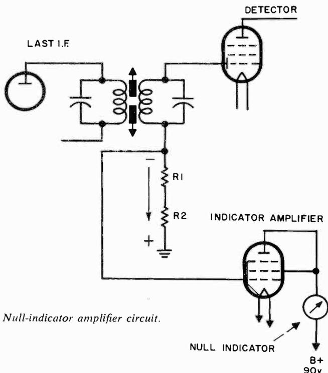
Fig. 1009. Null-indicator amplifier circuit.
