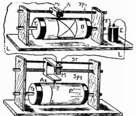
Fig. 5. The type of apparatus shown above operates by a positive action of the receiving stylus, the latter making a mark on the receiver drum when the transmitter current is interrupted by lines of the drawing.
