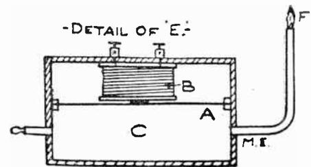
Fig. 13. Here is the light changing device indicated by a box in the previous figure. When diaphragm A moves, flame flickers.
