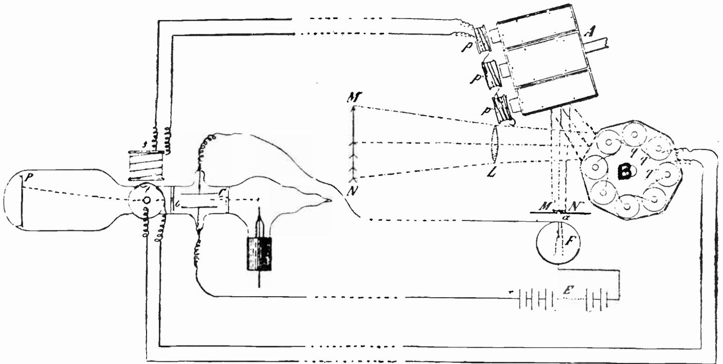
Fig. 17 Here is an ingenious television scheme which has not as yet been fully developed, to a state of practicability. It makes use of the Braun cathode ray tube.
