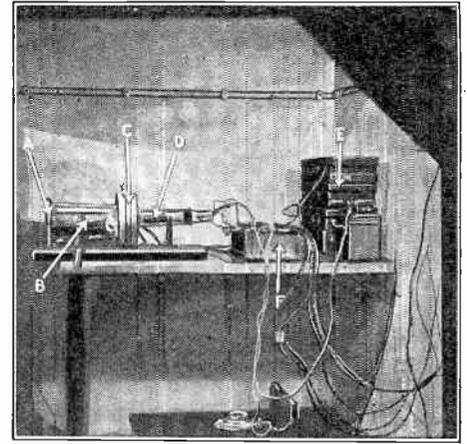
Fig. 82. Receiving apparatus: A, fluorescent screen; B, calcium tube for producing a vacuum in the oscillograph; C, concentrating coil; D, cathodic oscillograph; E, plate batteries, 300 volts; F, potentiometer box.
