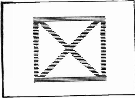
Fig. 6. A "positive" reproduction received on the apparatus shown in Fig. 5 is illustrated above. This is an exact duplicate of the transmitted drawing.
