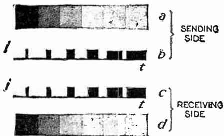
(a) Tinted row of surfaces to be transmitted. (b) Telegraph signal by which tone values are indicated. (c) Received impulses. (d) Reproduced tone picture at receiver.
