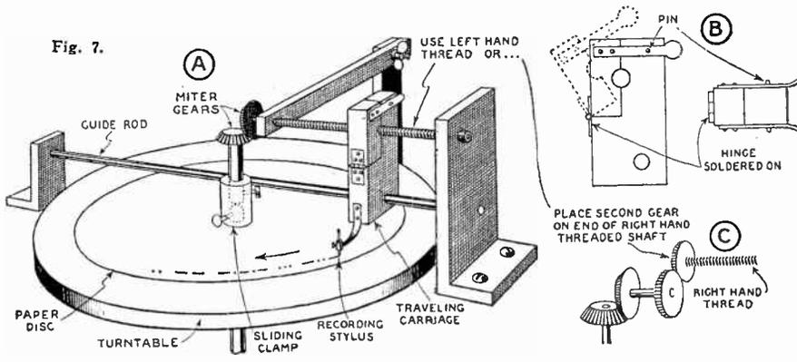
By means of the attachments shown above, and which can readily be fitted to any disc type phonograph, it is possible to transmit and reproduce a larger image than with the arrangement described and illustrated previously, wherein the regular tone arm of the phonograph is used to traverse a recording pen across a small disc.
