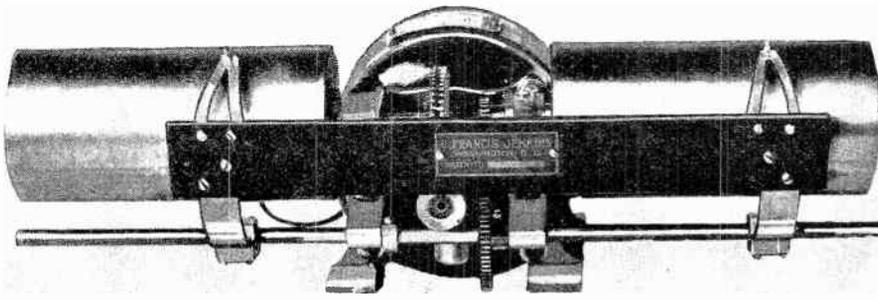
Another form of the device employs a small motor for turning over the cylinders which carry the "pens" and the chemically treated paper.
