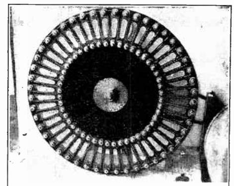
Fig. 37. Front view of the receiver disc showing how the lens prisms are mounted.
