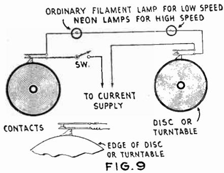
Simple synchronism indicator utilizing ordinary filament lamps for low speeds, and neon lamps for higher speeds. Whenever the transmitting and receiving discs are rotating in step or in synchronism, both lamps will light.
