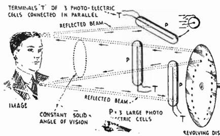
Fig. 95. How the extreme positions of the succeeding pencils of light exploring the object at the transmitter are enabled to pick up the whole image. The solid angle of vision is made up of rapidly moving beams of light.
