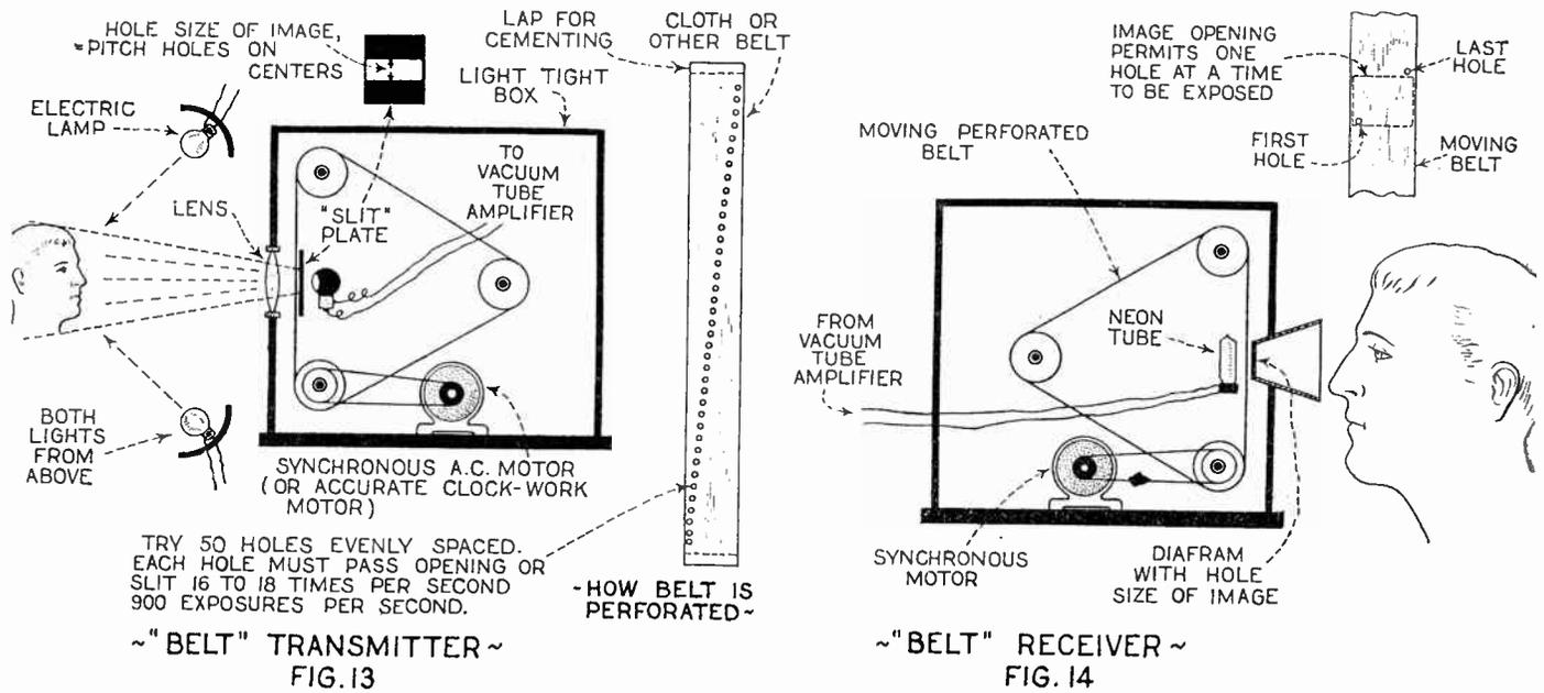
The experimental television machine shown at Fig. 13 and 14 above, has been tried out successfully by its inventor, Mr. L. J. Schramek. The perforated belt represents one way of causing the light ray to progressively traverse the image at the transmitter, and also to build up the image from the successive light pulses in the neon tube at the receiver.
