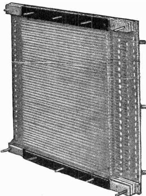
Fig. 92. The large 24 by 36-inch glass tube screen on which the television image was reproduced at the demonstration in the Bell Telephone Laboratories in New York City.
