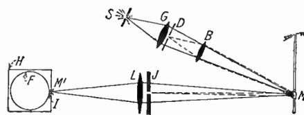
Fig. 27. The receiving plant of the Belin apparatus, illustrated diagrammatically. The reflected light acts upon a photographic film and reproduces the picture.
