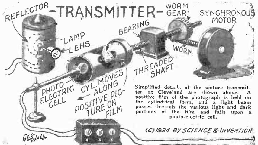
Simplified details of the picture transmitter at Cleveland are shown above. A positive film of the photograph is held on the cylindrical form, and a light beam passes through the various light and dark portions of the film and falls upon a photo-electric cell.
