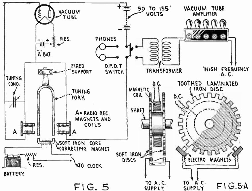
Fig. 5 above shows how a vacuum tube may be utilized in connection with a tuning fork and a pair of radio receivers, so as to produce a suitable current for operating a 500 or higher cycle A. C. motor. Fig. 5A shows simple synchronous motors.
