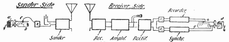
These sketches show the system of picture transmission by radio and line telegraphy. It was developed during the war for the needs of the German army
