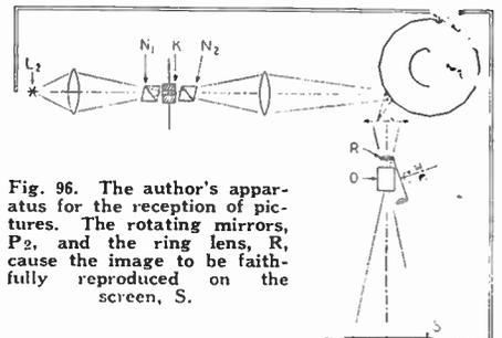
Fig. 96. The author's apparatus for the reception of pictures. The rotating mirrors,  $P_2$ , and the ring lens, R, cause the image to be faithfully reproduced on the screen, S.
