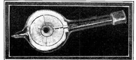
Fig. 103. The photo-electric cell invented by Dr. Schroter. Note the potassium cathode on the inner glass surface, the grid-anode and the hole in the center of the ring.
