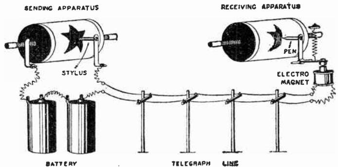
Fig. 19: Line transmission of a star illustrated in diagram, showing the system by which the Nile boat had its picture transmitted.
