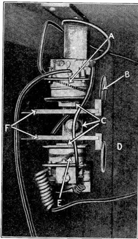
Fig. 81. A, coil producing alternating current of ten cycles; B, mirror; C, permanent magnetic circuit; D, frame; E, receiving coil of the tuning fork connected to the triode tubes; F, legs of the tuning fork (oscillating armature of the alternator).
