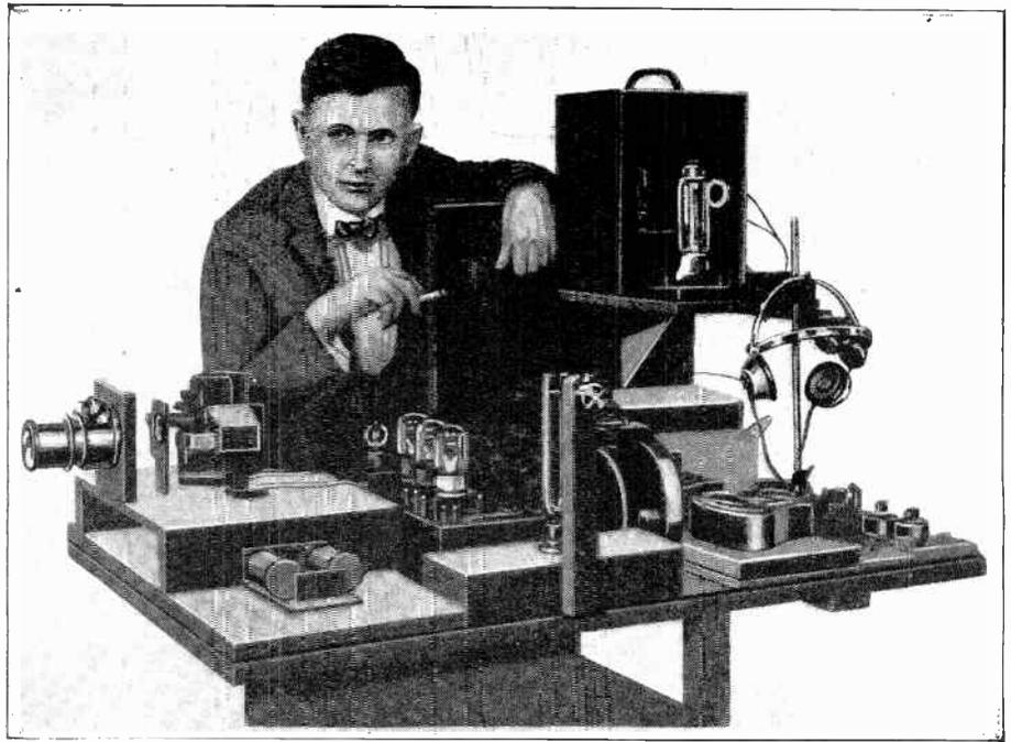
Fig. 44. Another view of the telehor machine with its inventor, Mr. Dionys Mihaly. The numbers refer to 1 tuning fork interrupter, 2 selenium cell, 3 mirror of oscillograph, 4 lenses, 5 phonic drum, 6 armature, 7 electromagnet of phonic drum, 8 diaphragm, 9 oscillograph.
