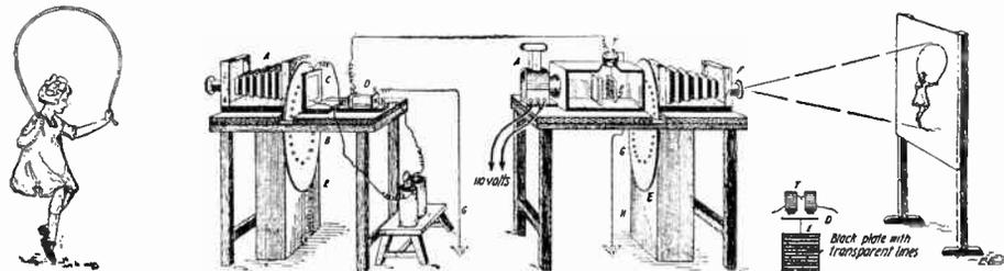
Fig. 22. The Dussaud Telephot uses two perforated discs B revolving synchronously. The holes are arranged helically; thus every point of the picture is covered during one revolution of the disc. Selenium cell C transmits impulses to receiver T, which vibrates plate E. The latter only passes parallel rays of light. With this machine it is—*theoretically*—possible to transmit objects in motion, electrically.
