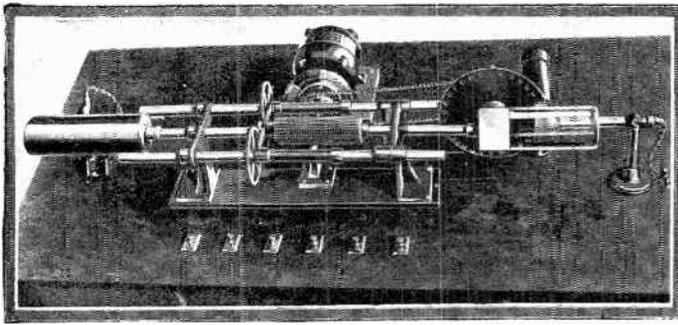
The machine for sending radio-photo messages and for receiving at the same time. For such a complicated performance the machine is unusually simple in its makeup.
