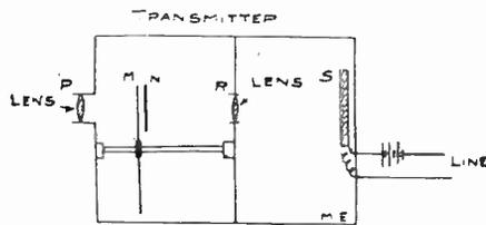
Fig. 11. This is the transmitter of the De Vendenil system in which the image is projected upon a single cell through a revolving shutter.
