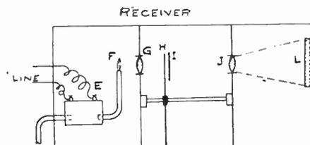
Fig. 12 shows the receiver in which the image is reconstructed; note box leading to flame F.
