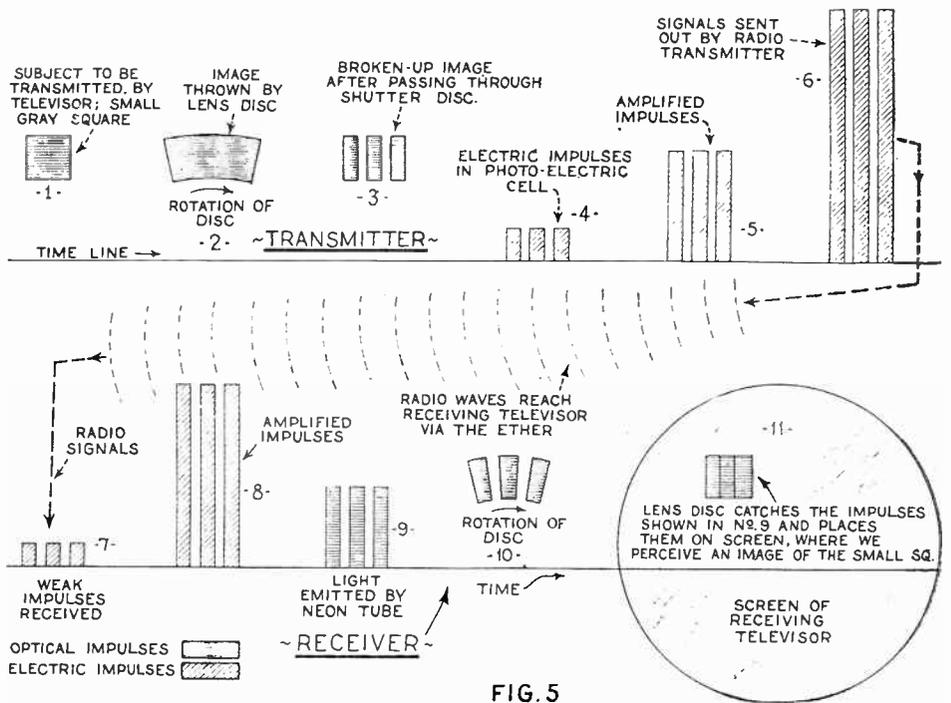
The diagram above shows progressively the stages gone through in transmitting and reproducing an image by the Baird television system, of the type employing revolving lens discs at both transmitter and receiver. The subject being transmitted in this case is a small gray square at 1, and we see how it is reproduced finally at 11.
