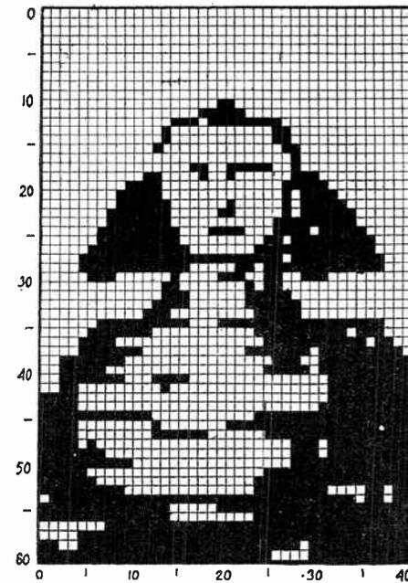
Fig. 15. The Sphinx sent by the code system. Here it will be seen that a very exhaustive specification would be required for transmission.
