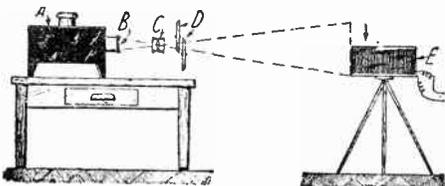
Left: Picture Broadcasting station. A—Magic Lantern. B—Picture. C—Lens. D—Rotating Prismatic rings. E—Light-sensitive cell box. Right: Receiver. Q—Fluctuating light. R—Camera lens. S—Prismatic rings. T—Camera plate holder.
