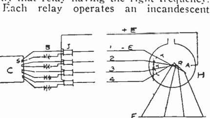
Fig. 2. Light entering camera, C actuates selenium cells S, closes circuit to spark coils J, and produces rays in X-Ray tube H.
