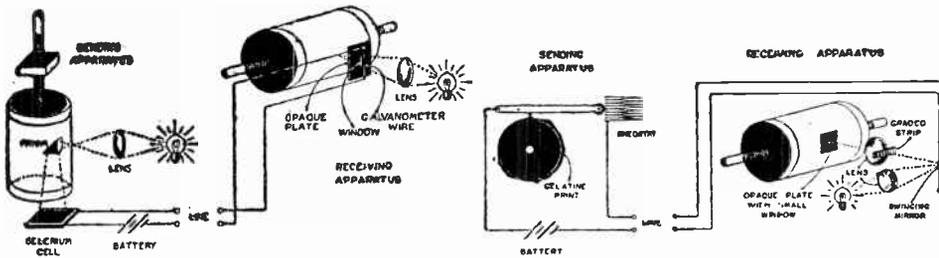
Fig. 20. Selenium cell apparatus for sending moving pictures; they are received photographically upon a film wound upon a rotating cylinder. Sending and receiving apparatus, also operated photographically, that allow for use of an oscillating mirror.
