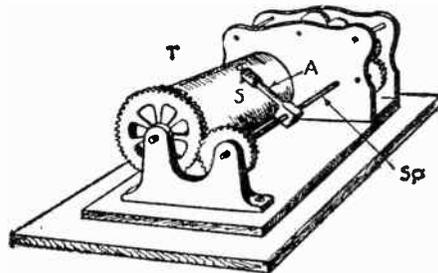
Fig. 3. The early form of the "telephotographic" device was driven by a clock spring. The stylus is moved transversely by a threaded rod or lead-screw geared to the drum shaft.
