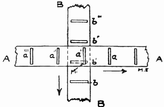
Fig. 16. Right. Here is a detailed view of the shutter arrangement. The arrows indicate the direction of movement and the small letters a, and b, represent the slots in the endless bands.
