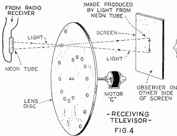
The diagram at the left shows arrangement of the revolving lens disc together with neon tube and translucent screen, such as ground glass, on which the image is built up. The man at the right is observing the image of the arrow as reproduced on the translucent screen, the image being built up by the rapidly changing spots of light thrown on a screen, due to the joint action of the light pulses from the neon tube and the revolving lenses on the whirling disc.
