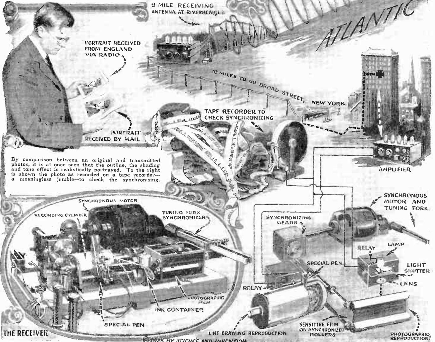
By comparison between an original and transmitted photos, it is at once seen that the outline, the shading and tone effect is realistically portrayed. To the right is shown the photo as recorded on a tape recorder—a meaningless jumble—to check the synchronizing.
