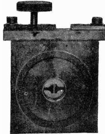
Fig. 101. The Karolus-cell. Note the two condenser-electrodes inside the glass cell and the terminals for connection to the receiver. The handle allows adjustment of the electrodes.
