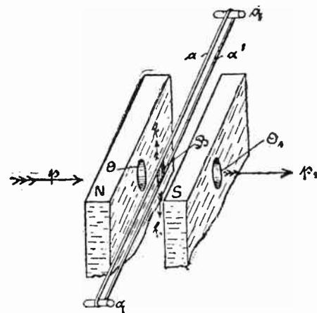
Fig. 5. The light relay described in this article.
