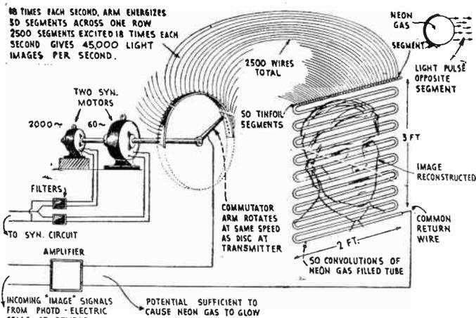
Fig. 100. The large exhibition screen, built up of a continuous length of glass tubing, along the rear walls of which are cemented 2,500 tin-foil segments. The tube is filled with neon gas; light spots appear opposite each segment when electrically energized.
