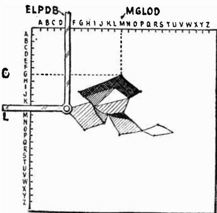
Fig. 12. At the receiving end the various letter combinations are potted by the operator and filled in by the artist.
