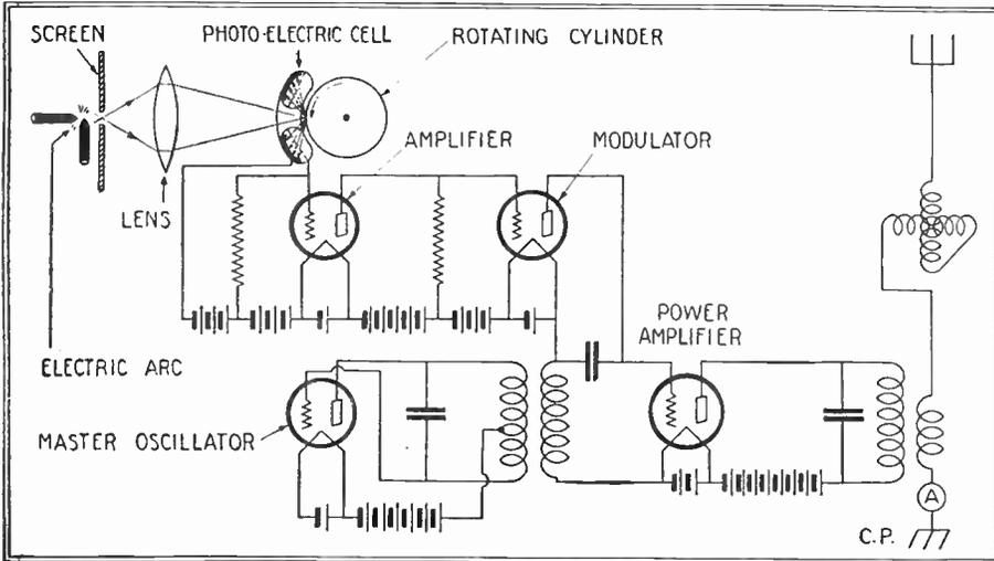
Fig. 100. Above is shown the circuit employed in the transmission of pictures by radio. Notice the peculiar construction of the photoelectric cell and its connections.
