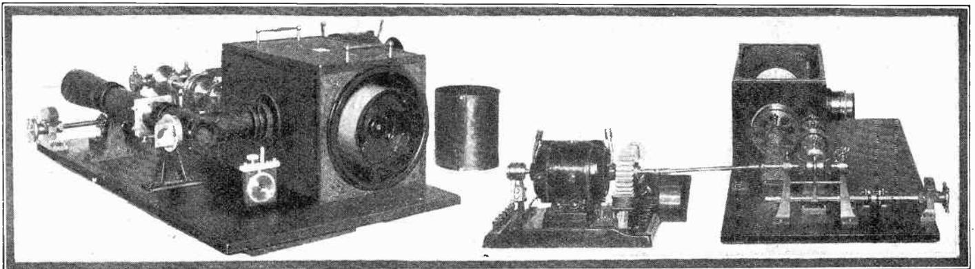
Fig. 102. The Telefunken-Karolus receiver system showing at the right a cylinder on which the unexposed negative film is mounted. One Karolus-cell may be seen in position in the center of the optical device and one standing in front of the receiving cylinder case.
