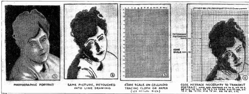
Fig. 1. The above pictures show successive stages in a new method evolved for the transmission of photographs or other pictures by code, over telegraph or telephone circuits, as well as by radio or cable. The original photograph at left was first retouched or redrawn so as to resemble a line-cut, as shown at No. 2. A transparent code scale (3) is then placed over the line cut as at 4, and the black and white portions of the picture coded by noting the lines which the black portions intersect.
