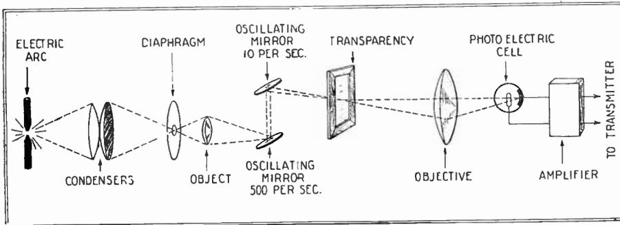
Fig. 68. After the light from the arc has been concentrated by the condenser lenses it is caused to pass in a wavy line over the transparency (See Fig. 69) and the variations of the transmitted light are registered on the cell.
