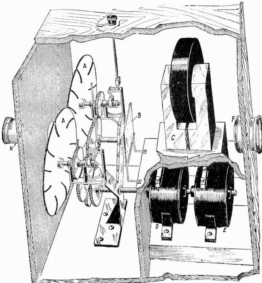
Fig. 49. The reproducing apparatus which recreates the image transmitted to it by the sender.
