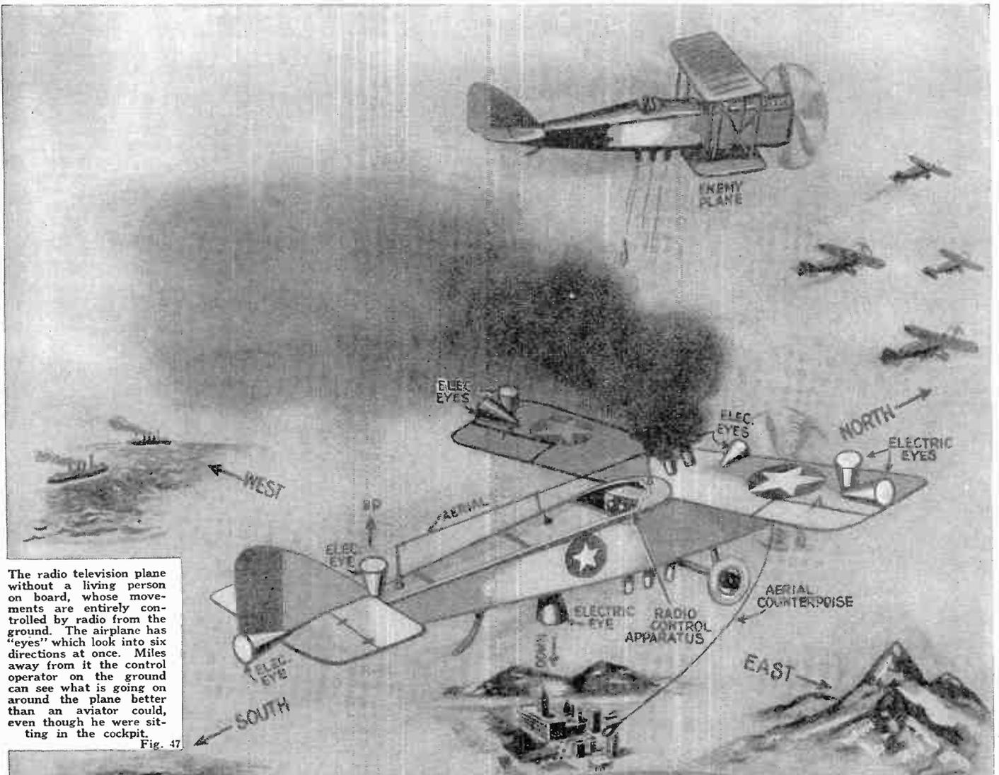
The radio television plane without a living person on board, whose movements are entirely controlled by radio from the ground. The airplane has "eyes" which look into six directions at once. Miles away from it the control operator on the ground can see what is going on around the plane better than an aviator could, even though he were sitting in the cockpit.
