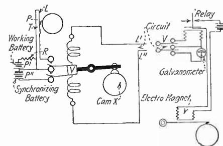
Fig. 26. Diagram of the transmitting end of the Belin apparatus for transmitting pictures by telegraph or telephone line.
