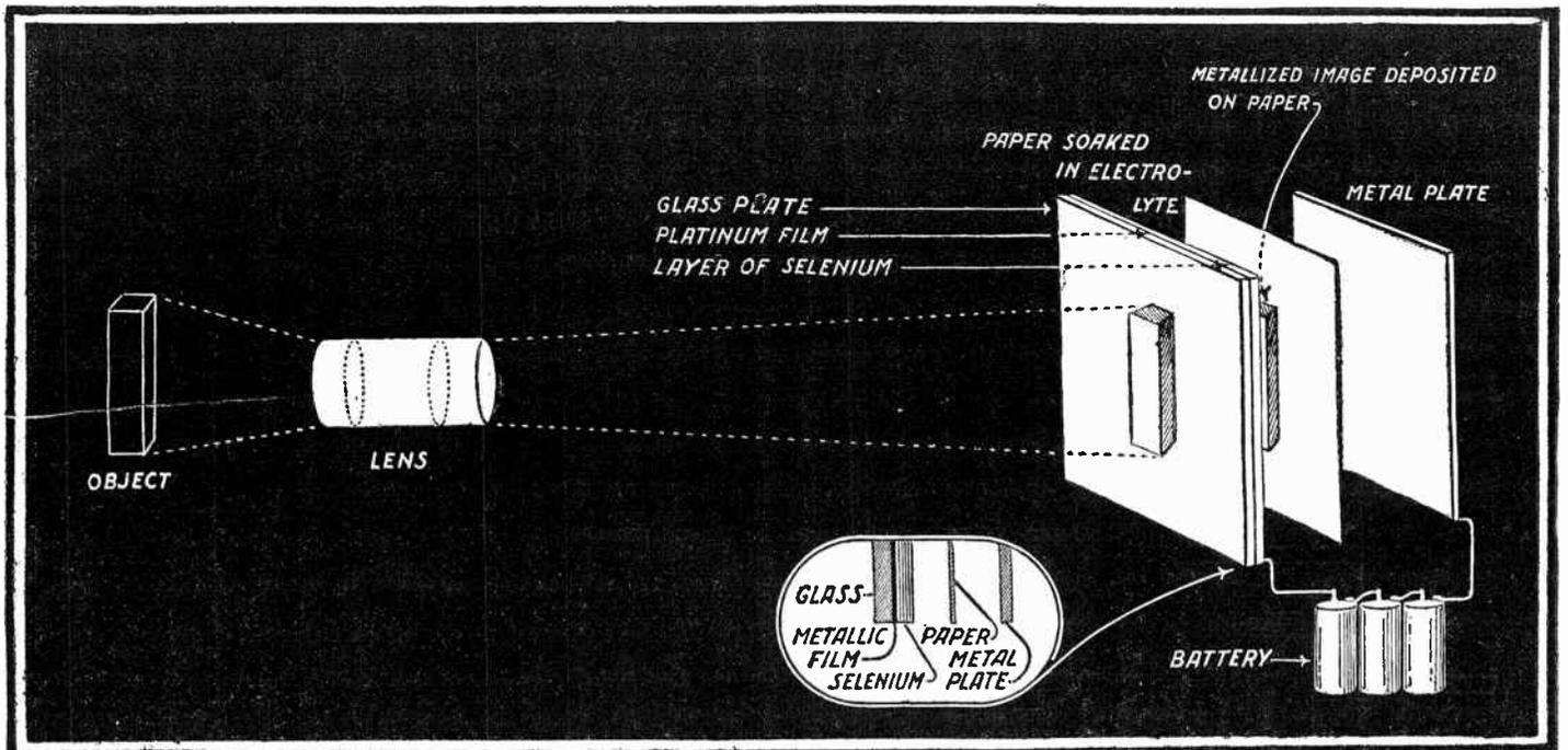
Through the agency of selenium which is sensitive to light, a German scientist, Mr. K. Wilcke, has just evolved a method for taking photographs by placing a thin sheet of this metal upon a metallic film, usually of gold or platinum, and placing the whole against a piece of paper. An electric current is then passed from the selenium to the metal plate and the whole exposed to light. Where strong light falls on the selenium its conductivity
