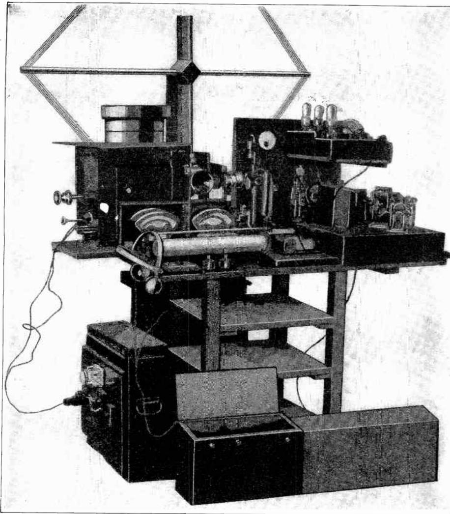
Fig. 43. The Mihaly Telehor machine. 1 is the arc lamp, 2 the light relay oscillograph, 3 the tuning fork, 4 the screen, 5 the diaphragm, 6 the oscillograph, 7 electro-magnet of phonic drum, and 8 the brush.
