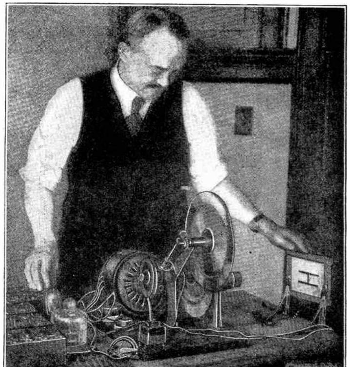
Fig. 31. Mr. C. F. Jenkins, original inventor of the motion picture machine, is here shown at work in his laboratory, together with the apparatus which transmits stationary or moving pictures via radio or wire, as desired. The underlying principles are fully explained in the accompanying text. Note the two prismatic glass discs rotated by the motor.
