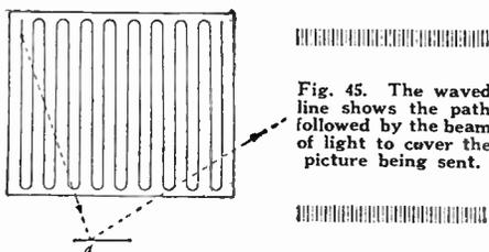
Fig. 45. The waved line shows the path followed by the beam of light to cover the picture being sent.
