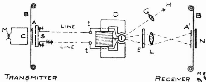
Fig. 15. Here is a schematic representation of the television method outlined in the accompanying article. Both transmitter and receiver are illustrated. A and B show the two shutters operating at right angles to each other.
