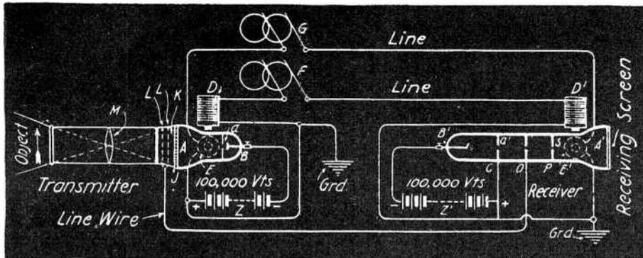
Fig. 18a. Diagram of Proposed "Television" Scheme.
