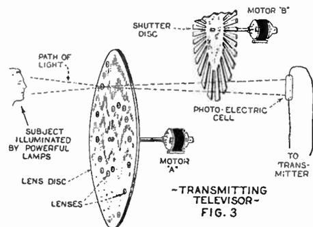
The diagram above shows arrangement of shutter disc together with lens disc and photo-electric cell in one of the television machines devised by Mr. J. L. Baird.
