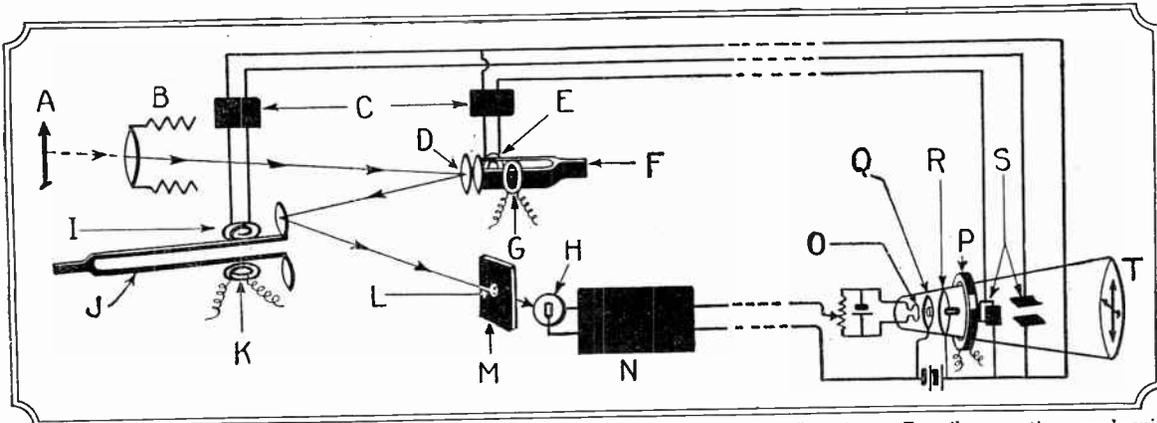
Fig. 84. Diagram of the Dauvillier apparatus: A, object; B, objective; C, amplifier; D, mirror; E, coil generating synchronic currents; F, 800 cycle tuning fork; G, exciting current; H, photo-electric cell; I, coil generating synchronous currents; J, 800 cycle tuning fork; K, hole determining the point of the image; L, hole; M, optical screen; N, amplifier; O, filament; P, concentrating coil; Q, grid; R, plate; S, condensers producing electrostatic fields; T, fluorescent screen.
