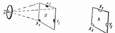
Fig. 46. By means of three dots placed at some point on the screen the synchronism between the transmitter and receiver may be checked.
