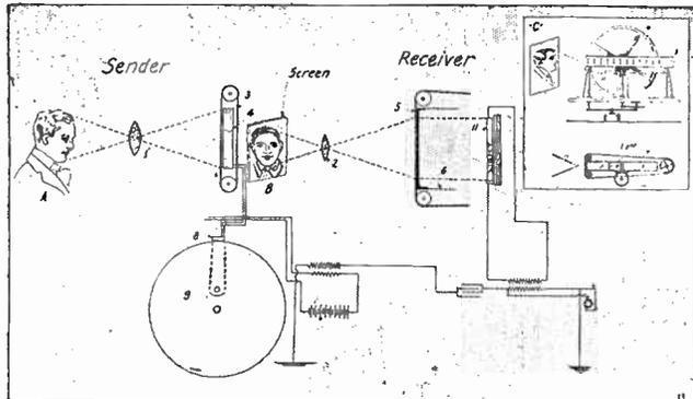
Fig. 23. This is the Rothschild telephot scheme which cuts up the light impulses by means of a slotted revolving belt 3 at the sender. Passing rapidly before the selenium cell 4 the impulses are sent over the line and influence a source of light 11 at the receiver where a similar revolving belt scheme reconstructs a picture as shown at E.
