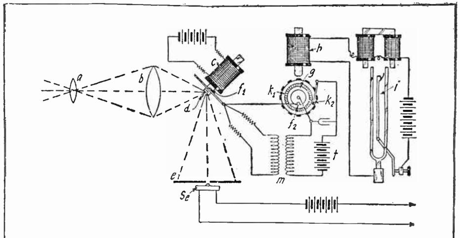
Fig. 41. The transmitting apparatus of the telehor. The object to be seen at the receiver is placed in front of the lens.
