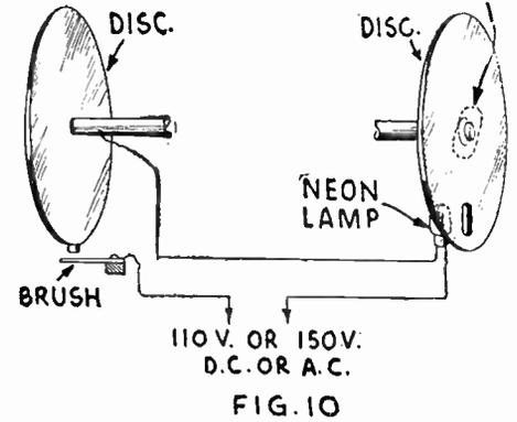
Simple synchronizing scheme which will cause the neon lamp to be lighted each time the brush and segment or tooth on the transmitting disc makes contact, the light pulsations being visible only when the slot in the receiving disc is opposite the neon lamp.
