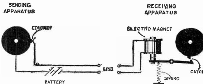
Fig. 21. Very simple arrangement by which perpetual synchronism between two rows of rotating cylinders at distant stations is obtained. This is used on the Belin apparatus.
