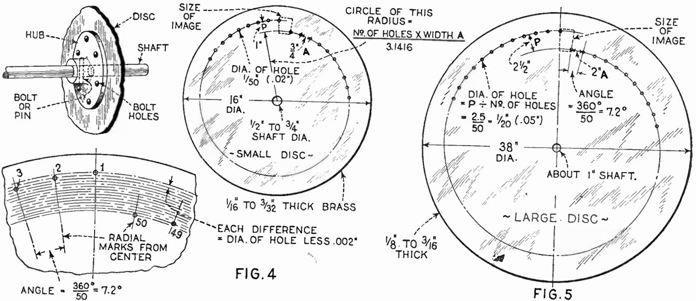
The method of laying out the holes in the disc used in the Bell television apparatus is shown in the drawing above.
