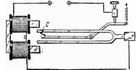
Fig. 39. The tuning fork interrupter which is kept vibrating with an electro magnet.
