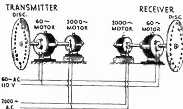
FIG. 4 This diagram shows a simplified form of dual motor drive for television disc.
