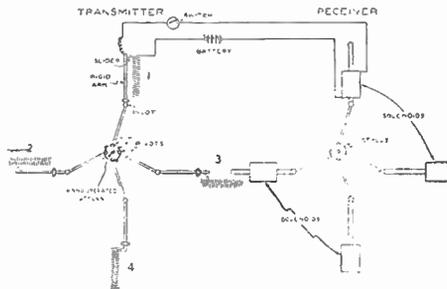
Simplest form of electric writing machine or Telautograph, utilizing four variable resistances and four electro-magnets or solenoids. Fig. 8-A
