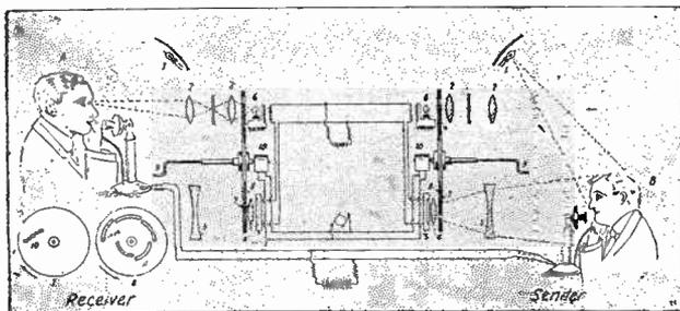
is a metal disc *B* perforated with certain holes. The disc is driven by clockwork contained in the case *E*. The ingenious part of this arrangement is that the disc *B* is perforated in a curious manner, the holes being disposed in the form of a helix or involute spiral. In other words, when the disc rotates the perforations cut off successive points of the picture formed in the camera *A*. Thus at each fraction of a sec-
