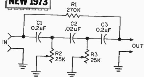
storer should be assembled in a metal cabinet to prevent hum pickup. Connect the output of your phonograph to the restorer input. Connect the output of the restorer to your tape recorder. Set potentiometer R2 to maximum resistance and adjust potentiometer R3 for the most pleasing sound. If R3's adjustment is too little, or too much as evidenced by a "hole" in the sound quality, trim the restorer with R2 until you get the optimum equalization.
