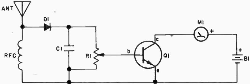
A kilowatt transmitter may pin the needle of regular FSMs (field strength meters), but you need high sensitivity to get readings from low-power oscillators, flea power transmitters and CB walkie-talkies. This simple, amplified FSM has a sensitivity of 150 to 300 times that of ordinary models. It indicates full scale when other meters can't budge off the pin.
