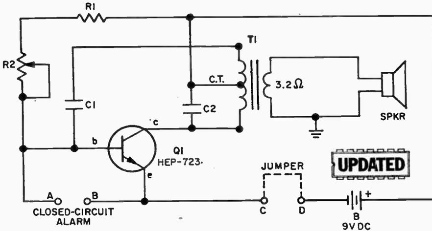
jumper across C and D and connect a series wire circuit across A and B, which disables the oscillator though power is applied. An intruder breaking the series circuit, or a normally closed magnetic switch, causes the alarm to sound off.
