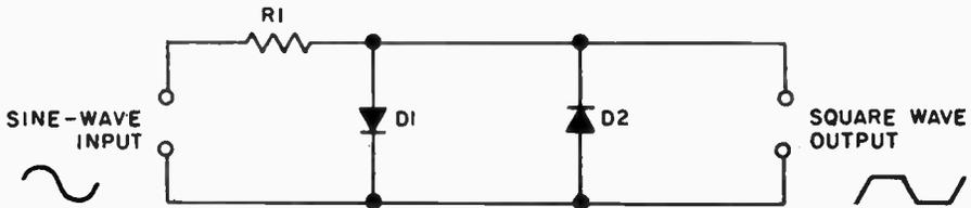
Two reverse-parallel diodes of the germanium type provide an emergency square wave generator. Since a germanium diode has an approximate 0.2 V breakover, any sine wave applied to the diodes will be clipped at 0.2 V. It provides a 0.4 peak-to-peak square wave. It's not perfect since the "rise" of the original sine-wave is still present, as shown in the waveform.
