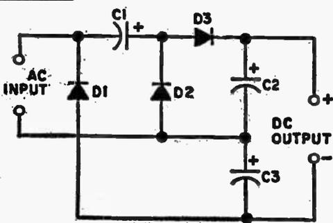
100  $\mu$ F at 300VDC. The larger the value for C2 and C3, the better the filtering. On the negative half-cycle, C1 charges through diode D2, while C3 charges through D1. On the positive-half cycle, C1's charge, plus the line voltage, charges C2 through D3. The output is the voltage across C2, which is the line voltage plus the charge from C1, plus the added voltage of C3. The total is almost three times the line voltage.
