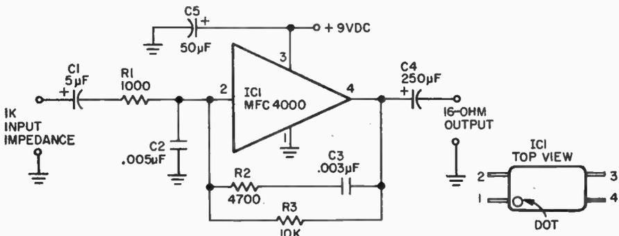
Using an IC no larger than a fly, Spy-Size Amplifier delivers almost 250 mW into a
