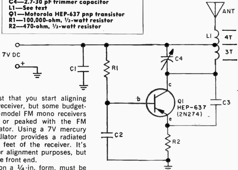
We don't suggest that you start aligning your stereo FM receiver, but some budget-priced and early-model FM mono receivers can be aligned or peaked with the FM Alignment Oscillator. Using a 7V mercury battery, the oscillator provides a radiated signal within 10 feet of the receiver. It's strong enough for alignment purposes, but won't overload the front end.
