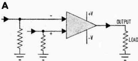
Fig. 3A. Open-loop gain results when amplifier is connected as shown and its maximum gain available. Fig. 3B. Closed-loop gain is device's gain after feedback has been applied; it's equal to  $R_f/R_{b1}$ .
