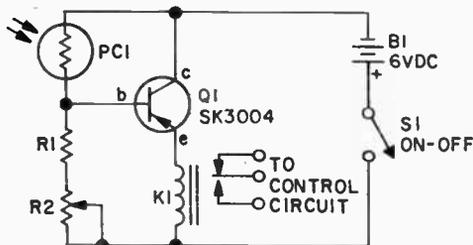
set so that with normal illumination falling on PC1 the base bias current (through PC1) is just below the value needed to generate the collector-emitter current required to activate relay K1. When additional light falls on PC1, photocell resistance decreases, thereby increasing the base bias, which causes greater collector current to flow and the relay closes.
