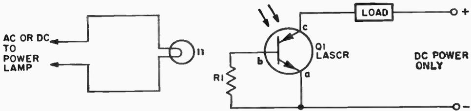
The triplamp can be any ordinary flashlight bulb powered by two D cells. When the lamp is turned on the LASCRLAMP gate is closed, causing current to flow through the load and the LASCRLAMP anode (a) cathode (c) circuit.
