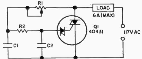
Old universal appliance motors and shaded-pole induction motors salvaged from inexpensive turntables can be easily converted to slow-speed hobby drills, chemical stirrers, vari-speed turntables movable display drives, etc. It's done with a full-wave Triac speed controller.
