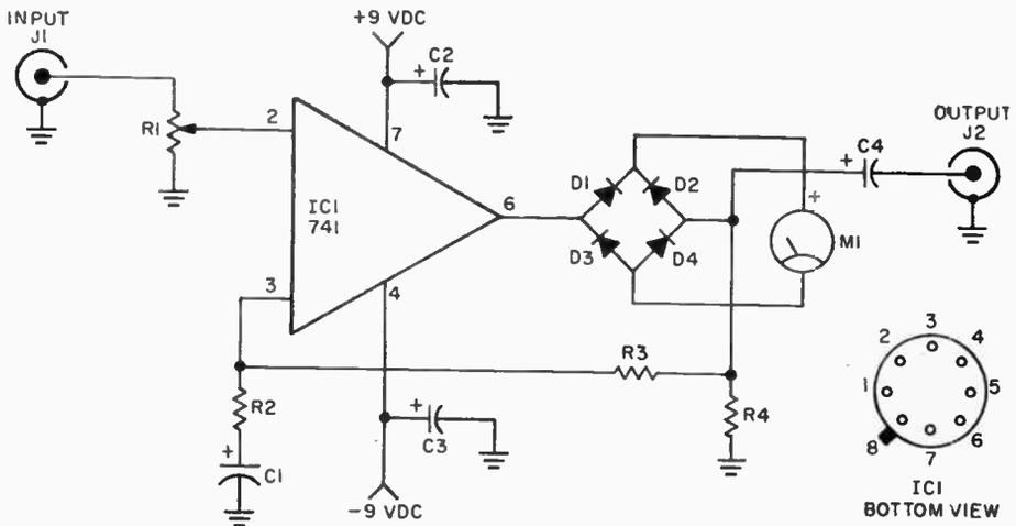
internal rectifier has been removed (open the case and unsolder the rectifier). Total current drain is less than 5 mA
