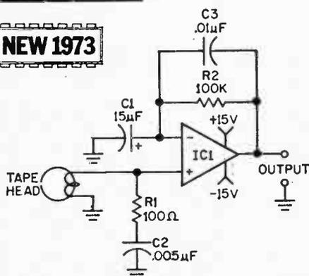
Is it worth about \$20 to have another tape or cassette player? From time to time surplus dealers offer complete tape or cassette mechanisms—everything ready-to-go except for the electronics, and at rock-bottom prices of \$10, \$15 or \$20. All the mechanism needs is this equalized tape head pre-amplifier. Though the power supply is rated at  $\pm 15$  VDC, almost optimum results will be obtained with supply
