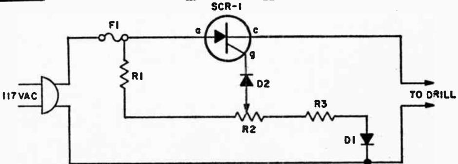
As the speed of an electric drill is decreased by loading, its torque also drops. A compensating speed control like this one puts the oomph back into the motor.
