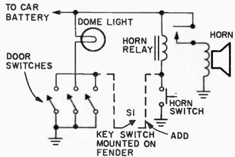
to frighten off a potential burglar. If all the car doors are not equipped with switches you can easily install them; switches are available from local auto supply stores.
