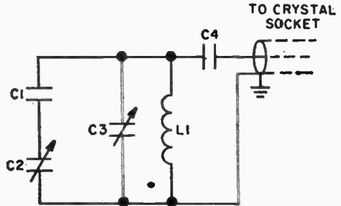
adjust C2 until channel 1 is received. Depending on the IF frequency, C3 might tune slightly more or less than the full band. If so, change C1's value very slightly to obtain only 23-channel coverage with C3. Making C1 smaller narrows the tuning range.
