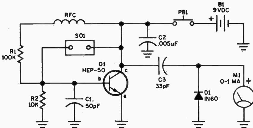
A fast way to see if the crystal from your transmitter or receiver is properly "active" is to compare its output against that of a
