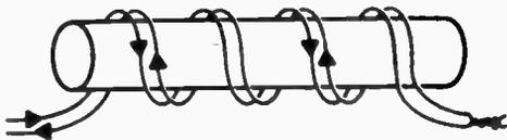
as the current tends to form a magnetic field in one direction, its return path, which is in the opposite direction, generates an equal and opposing magnetic field. Hence, no traceable inductance. However, the more turns you make on the wood form, the more capacitance. You can't win!
