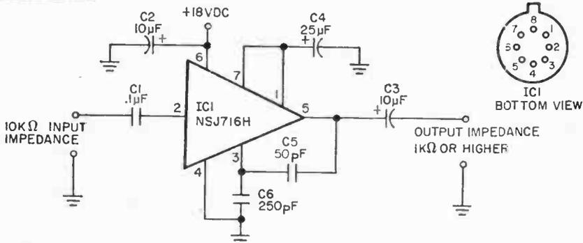
Gabber Grabber works best with the 10,000 ohm microphones and telephone pickup coils supplied with most solid-state recorders. It provides 26dB gain, and is ideal when a single microphone is used for conference recording or when remote telephone monitoring through a pickup coil is desired. The 18V power supply can be two series-connected 9V transistor radio batteries. Since the IC is a high frequency device, its leads should be kept as short as possible. A socket holding the IC is sug-
