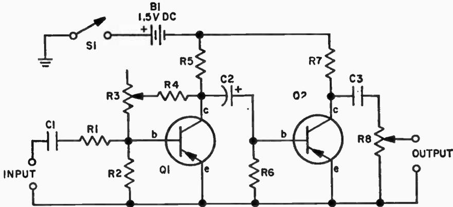
Add that 'way-out fuzz sound to any electric guitar by connecting the Fuzzbox between your guitar and amplifier. Potentiometer R3 sets the degree of fuzz, R8 the output level.
