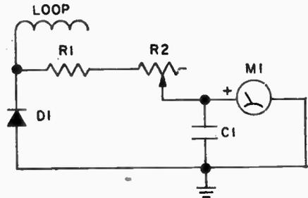
be as short as possible. The loop consists of four or five turns of insulated, solid hook-up wire wrapped around an exposed part of the output coax cable. Remove a part of the
