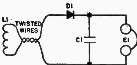
This simple modulation monitor for AM ham transmitters requires no connection to the transmitter. Just position the loop near the final tank or antenna matching coil un-
