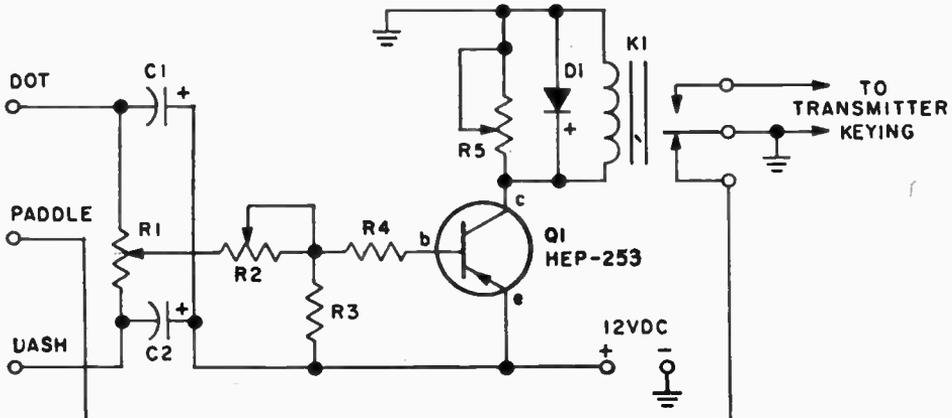
dot terminal, C1 starts to charge. When C1's voltage causes Q1 to conduct, collector current pulls in relay K1, thereby keying the transmitter. When K1 grounds the paddle terminal, C1 discharges, causing Q1 to stop conducting and dropping out the relay. When K1's paddle connection is restored to ground the cycle repeats until the paddle is released.
