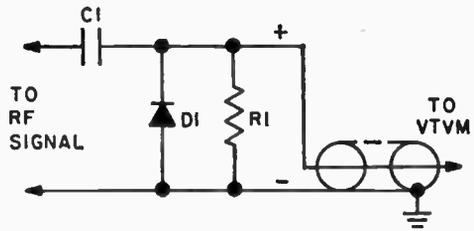
higher voltage small signal detector diode.
