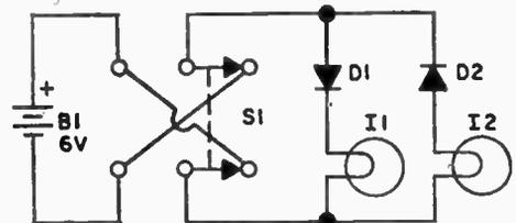
Using diode switching, a single pair of wires controls two circuits that normally require four wires. Though illustrated here with
