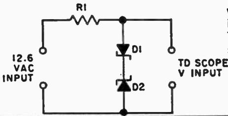
positive. The reverse action takes place when the top of D1 goes negative, providing an output waveform of 5 V negative. The total result is a 10 V peak-to-peak square wave to calibrate the scope face.
