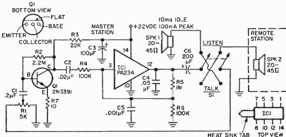
station always monitoring the Remote. The speakers can be any "intercom type" rated from 20 to 45 ohms. Though miniature 16 ohm speakers can be used, they do not have the power handling capacity of the "intercom" speaker. If there appears to be some high frequency instability, use a shielded wire between S1 and R1; make a
