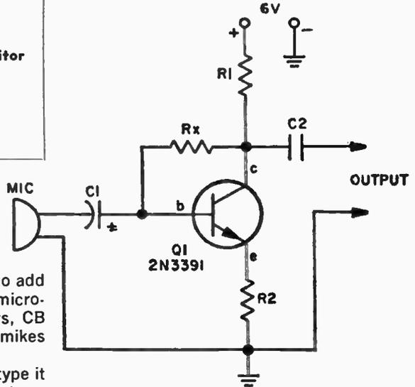
Just a handful of parts is all it takes to add up to 30 db gain for low-impedance microphone inputs found on tape recorders, CB rigs, etc. The circuit is suitable for mikes in the 50- to 1000-ohm range.
