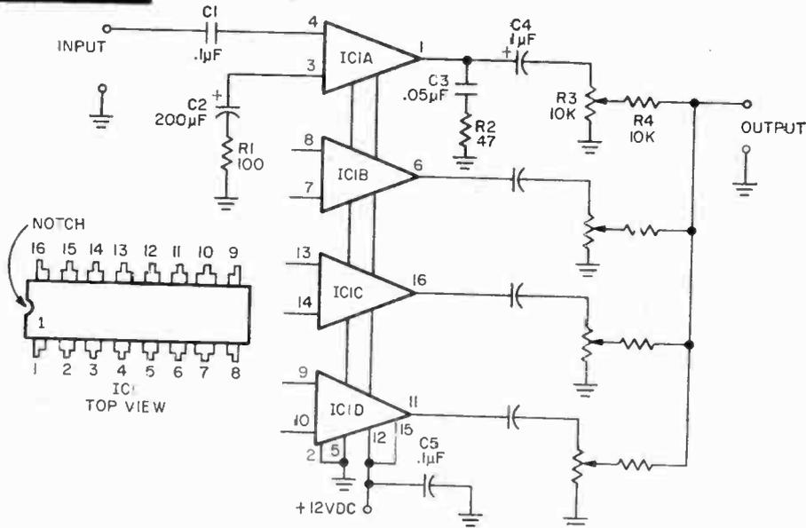
Best signal to noise ratio in a microphone mixer is always obtained if amplification is provided ahead of the loss in the mixer network. You can easily put this idea to work with our Pro-Mix—a full-fidelity, professional-grade microphone mixer that contains four independent amplifiers within the integrated circuit.
