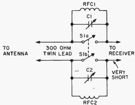
tion. If your antenna's downlead is coaxial cable, only one filter is installed—in series with the center (hot) conductor. To adjust, tune in the offending station and use an insulated alignment screwdriver to adjust trimmer capacitors C1 and C2 for *minimum* signal strength.
