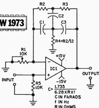
Ever hear a telephone voice on radio or TV. The effect is usually created by passing the signal from a high quality microphone through a bandpass amplifier—a device that attenuates the frequencies on both sides of a selected frequency. Bandpass amplifiers are also effective at providing mid frequency boost—presence, as it's called in hi-fi terms.
