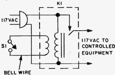
coil so the relay contacts stay open. When S1 closes the loop on the hysteresis coil, the impedance of the main coil drops. Current flows and the contacts close.
