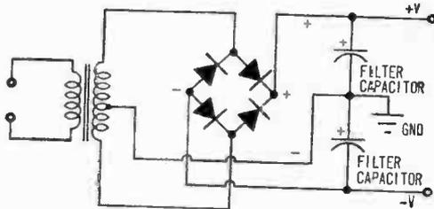
Fig. 8. Even cheaper way to achieve bi-polar output is to combine bridge rectifier with center-tapped power transformer. Full-wave output is easy to filter, ideal for most OpAmp circuits.
