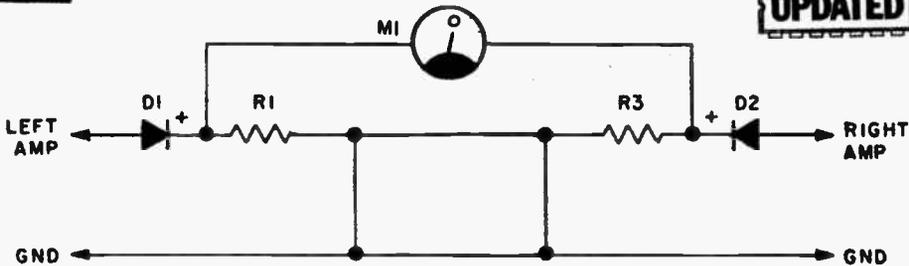
It looks ridiculously simple, but this instrument will give you precise volume and tone control balance between left and right stereo amplifiers.
