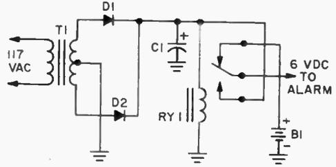
Both home-brew and battery operated burglar alarm kits are made fail-safe with this automatic AC power supply. Normally, power
