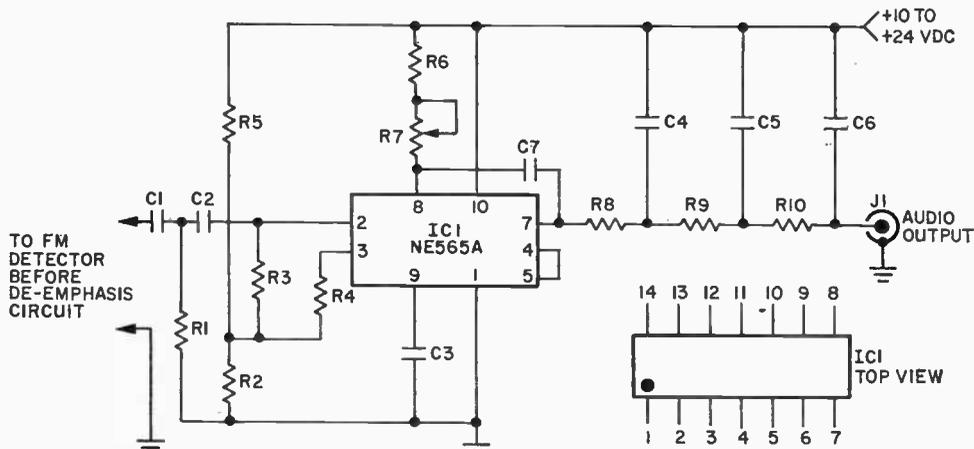
R7 for a clean SCA audio output. Potentiometer R7's adjustment is not critical—the subcarrier is pulled in when R7's adjustment is near the correct setting. A metal cabinet is suggested. If
