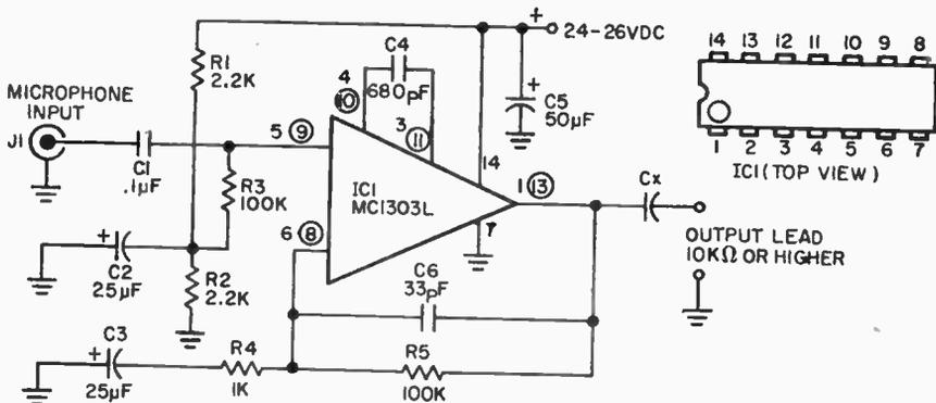
With resistors R1 and R2 providing a center-tap for the power supply, the IC can be powered from a standard single-ended power supply, or series connected batteries. Be very careful to observe the correct polarity for capacitors C2 and C3. In the event the unit motorboats (low frequency oscillation), install a 0.1 uF capacitor from pin 14 to ground. The connections for one of the two amplifiers is shown circled; the connections for the second
