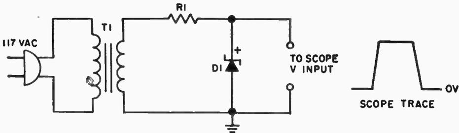
You can make accurate voltage measurements with your oscilloscope if you calibrate the vertical input with a Scope Calibrator.
