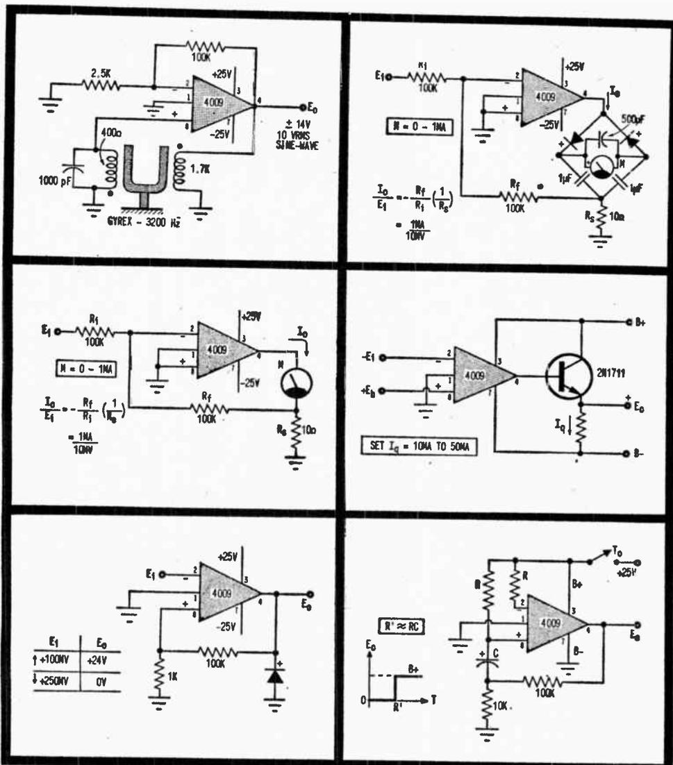
Fig. 5. Six circuits using 4009 OpAmp, available from OpAmp Labs, 172 S. Alta Vista Blvd., Los Angeles, Calif. 90036 for \$10.00 ea., postpaid. Circuits, from left to right, are 1) tuning fork oscillator, 2) AC millivoltmeter, 3) DC millivoltmeter, 4) DC medium-power amplifier, 5) Schmitt trigger, 6) fast turn-on timer.
