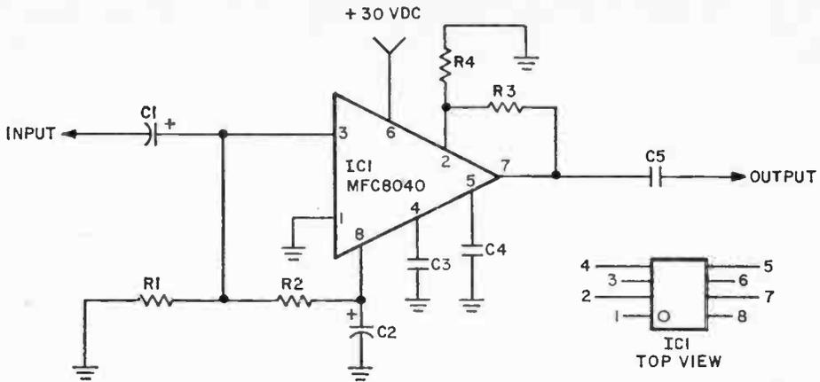
theless is almost dead quiet. The input impedance is about 75,000-ohms; output impedance about 100-ohms. Actual maximum output voltage depends upon the load resistance, ranging from 7 volts output into a 10,000-ohm load to 4 volts output into a 1000-ohm load. Parts layout is not critical and any type of assembly can be used. The power supply current is typically 8 mA, with a maximum of 12 mA.
