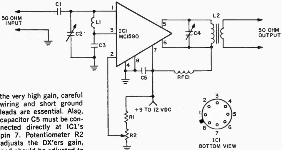
the very high gain, careful wiring and short ground leads are essential. Also, capacitor C5 must be connected directly at IC1's pin 7. Potentiometer R2 adjusts the DX'er's gain, and should be adjusted to just below the point where the DX'er overloads. To align, tune in a signal in the center of the desired frequency coverage and adjust trimmer capacitors C2 and C4 for maximum signal strength.
