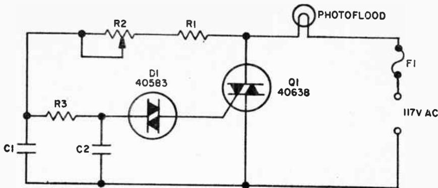
surge current when 500-watt photo lamps burn out will instantly destroy Q1. Connect an 8AG (fast-action) 5-ampere fuse in series with the lamp or any other fuse of
