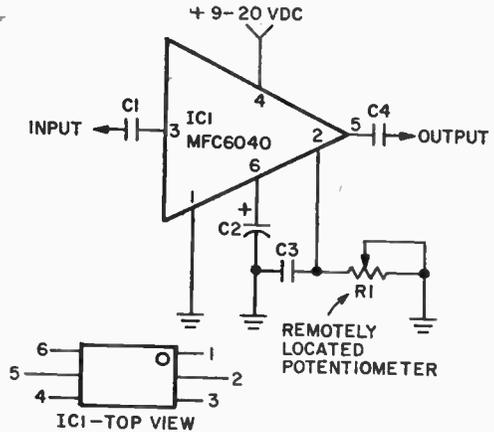
potentiometer R1 and applying 3.5 to 6 volts DC directly to pin 2. With 3.5 VDC the amplifier works at full gain. The attenuation increases to a maximum of 90 dB as the control voltage is increased to 6 VDC.
