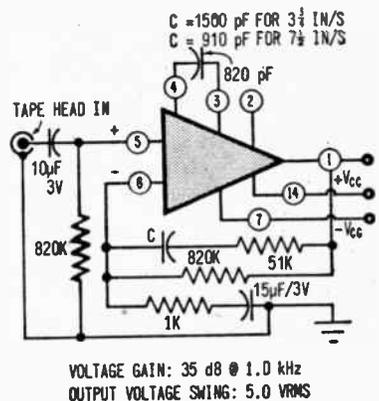
VOLTAGE GAIN: 35 dB @ 1.0 kHz
