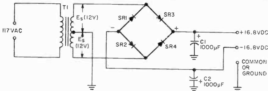
Filter capacitors C1 and C2 should be at least 1000  $\mu$ F (2000  $\mu$ F preferred) at a voltage rating at least equal to the supply's output voltage.
