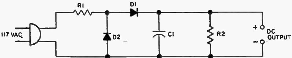
Just a handful of components are needed for a line-powered low-voltage low-current supply for powering audio preamplifiers.
