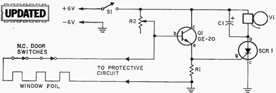
is an AC powered 6 VDC source or a lantern battery; standby current is about 100  $\mu$ A. To adjust, connect a voltmeter (10 VDC range) across resistor R1, open the protective circuit and adjust potentiometer R2 so the meter indicates a voltage rising towards 1 volt. The alarm bell should ring before 1 volt is reached on the meter. If it does not, there is a wiring error. Finally, set R2 for the 1 volt meter reading, remove the meter and restore the protective circuit.
