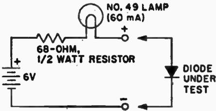
Low voltage signal diodes are easily tested with this "go/no-go" checker. The only re-
