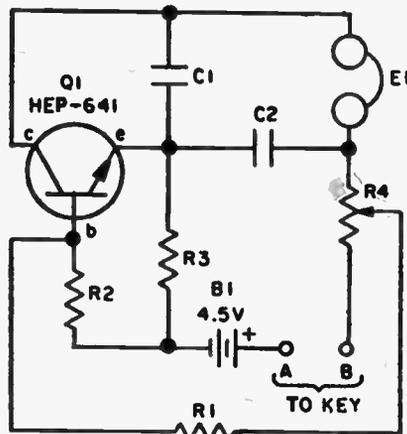
than C1. Battery current drain is only about 1 milliampere.
