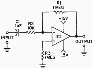
This general purpose amplifier features a power gain of 100 (20dB) and can be used as a preamplifier for a microphone, receiver, signal tracer, etc. The IC is internally compensated, providing stable performance with a flat frequency response to about 10 kHz with a gradual roll-off to 20 kHz. The overall gain can be reduced to 10 by
