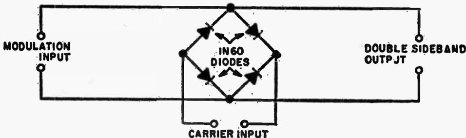
Feed audio modulation to one input, a carrier to another and the output of this sideband generator will be upper and lower sideband with suppressed carrier. Where is
