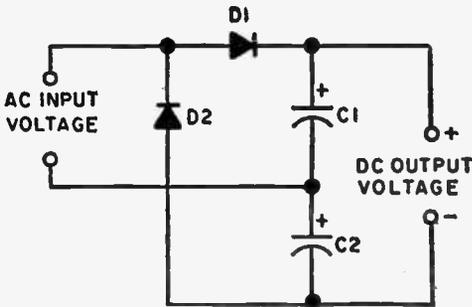
Found in many CB transceivers, the full-wave voltage doubler provides reasonably good regulation with DC output voltage twice the AC input. Capacitors C1 and C2
