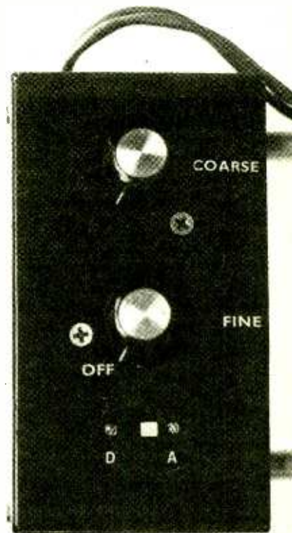
Hounddog's control head is laid out simply; there's an SPDT switch and two adjustments.
