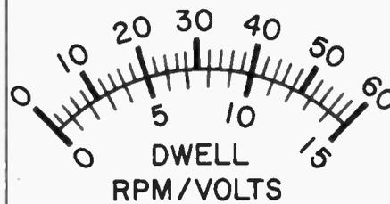
Fig. 3. This is a full-scale template for use on the meter face. It is designed to be used with the GC Electronics movement described in the parts list, but will likely fit other meter faces just as well.
