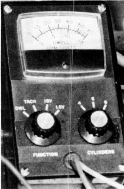
**O**UTSIDE OF A GOOD SET of wrenches, the most commonly called for automotive tool is the dwell/tachometer. When tuning up an engine, there's no substitute for the kind of accuracy a dwell/tach can bring to your engine adjustments. A commercial version of this apparatus might run as high as \$25.00. With some judicious parts buy-
