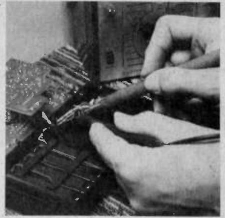
A voltmeter is vital for checking out the electrical continuity, finding shorts and tracing through the circuitry. Pocket calculators very often show signs of abuse.
