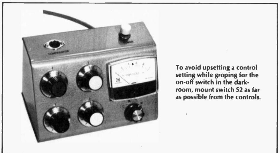
To avoid upsetting a control setting while groping for the on-off switch in the dark-room, mount switch S2 as far as possible from the controls.
