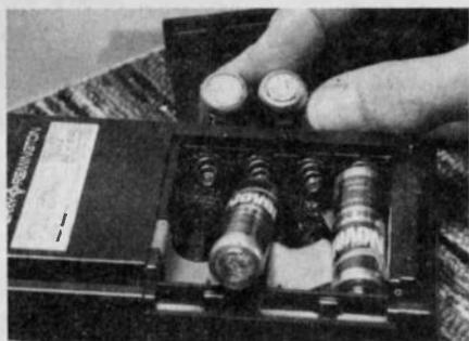
**Corroded Battery Terminals.** When batteries are left unused for a long period of time, they begin to leak and corrode around the battery terminals. Try to keep fresh batteries in the calculator to prevent corroded terminals. Replacement with leak-proof and long life batteries helps, but after a long time it takes only a very small amount of corrosion to prevent juice from getting to the calculator's circuitry. A light going over with alcohol very often does the trick.
