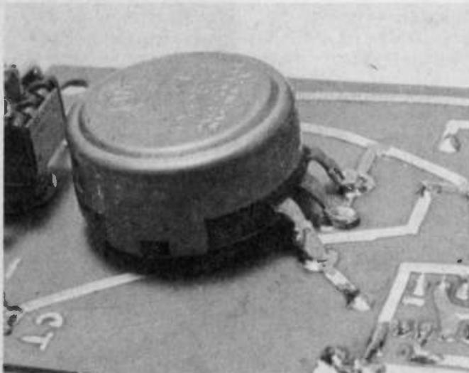
To prevent a shock hazard caused by the pins sticking up on the top side of the printed circuit board, R1's terminals are tack-soldered to the pads on the etched side of the board. A strong physical connection is assured by through-the-board mounting of R1's shaft.
