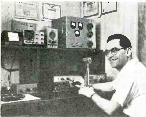
Bernie Ostrofsky, W9HTF, Gary, Ind., divides his time between CW and SSB, rag-chewing or DX chasing. His Drake TR-3 transceiver drives a high-power, home-built final amplifier, and he has a multi-trap dipole and a 3-element tri-band beam.
