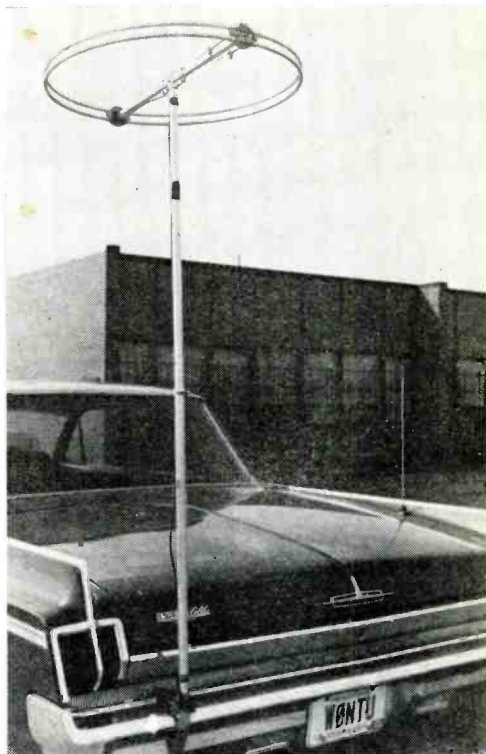
About 15 years ago hams on 6 meters switched from vertical to horizontal antenna polarization, which complicated matters for mobile stations—since verticals are naturals on cars. One solution was the development of the halo. This is a Hy-Gain HH6BA.
