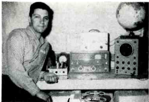
John Casazza, Staten Island, N.Y., used the modest equipment shown to track ham satellite OSCAR III. The receiver is a National NC-140 fed by a Tecraft converter tuned to the 2-meter band. Signals were recorded on a Wollensack tape recorder.
