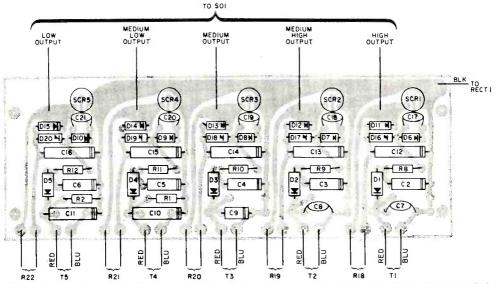
Fig. 5. When mounting parts on the printed circuit board, be sure to position the diodes with the polarity markings as shown. Also, make all input and output connections from terminal pins on the circuit board.
