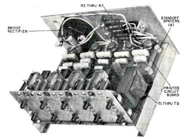
Fig. 8. This fully assembled unit shows printed circuit board mounted on four standoff spacers. Run all pointto-point wiring to the controls and pilot lamps before installing the transformers.
