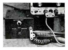
(1) Set selector switch to SQUAREand connect a jumper between Q3's base and ground to disable the multivibrator.
