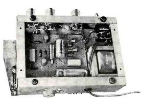
Interior view showing components mounted on perforated phenolic board, suspended on standoff screws. Transistor Q3 is mounted on the chassis back panel while transformer T1 is on the inside of the right panel, directly behind the on/off switch.
