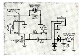
Fig. 2. Modulation indicator tells how much a.c. signal is present with respect to unmodulated d.c., to provide a percent modulation figure. Distortion indicator 11 lights up in the presence of harmonic frequencies which are generated by overmodulation.
