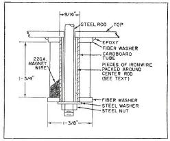
Fig. 4. Construct coil forms as shown. Each coil takes about 80 feet of No. 22 enamel-coated wire. A  $\frac{1}{2}$ -pound spool should be enough for both coils.
