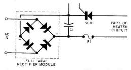
Fig. 5. A full-wave bridge rectifier in the line circuit causes the SCR to conduct on both half cycles, resulting in a doubling of the heater power.
