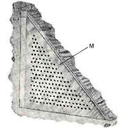
Cage side cover is held in place by  $2\frac{1}{2}$ "-long screws fed into front and bottom of cabinet from outside, and by  $1\frac{1}{4}$ " screws through piece L.
