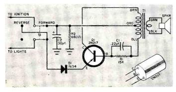
er shown is easily adapted to a positive ground system, with only three minor but very important—differences in the wiring: (1) a 2N647 *npn* transistor is used for Q1; (2) the positive side of electrolytic capacitor C2 is connected to the ground lug of the terminal strip; and (3) the anode of diode D1 is connected to the emitter of Q1, and the cathode goes to S1. The instrument can be operated in either 6- or 12-volt systems without any circuit changes.
