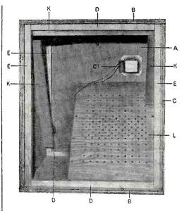
Location of tweeter is not critical. If you want to dispense with testing procedure, drill 80  $\frac{1}{4}$ "-diameter holes (8 rows of 10) in woofer compartment.
