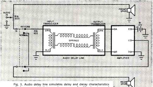
Fig. 1. Audio delay line simulates delay and decay characteristics of a large concert hall, in your home or car. Amplifier boosts sound just enough to compensate for insertion loss of the delay line.
