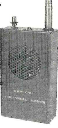
**B**UILD a portable time-signal receiver and you can tune in on standard time broadcasts from your living room, picnic table, boat, car, or even from a private plane. This miniature receiver is a complete superhet circuit with crystalcontrolled local oscillator, prepackaged pretuned i.f. module, and *transformerless* audio amplifier. A printed circuit board makes it easy to build and only a screwdriver (no test equipment) is needed for alignment!
