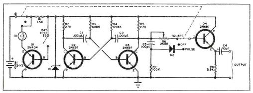
Fig. 1. Essentially a square-wave generator, the scope calibrator also produces a positive-going pulse for test purposes. The battery condition is monitored by means of the test lamp (I1) in Q1's circuit.
