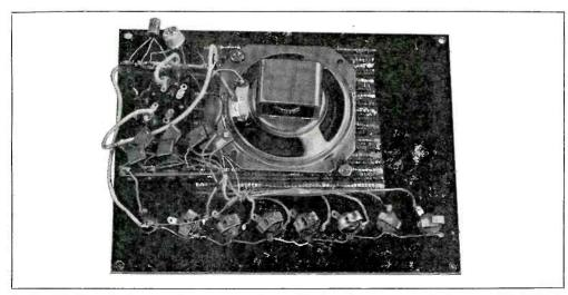
Fig. 2. This photograph shows the rear panel of the author's prototype organ which was later rewired to improve lead dress. Parts are mounted on terminal strips, and the battery is strapped down in the case.
