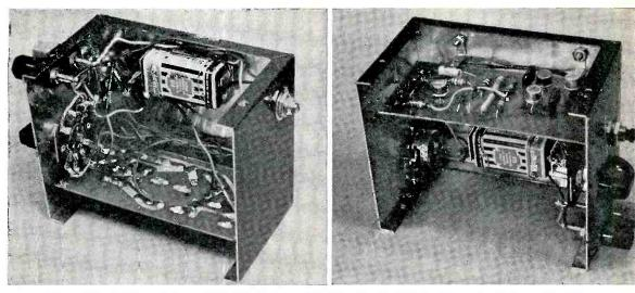
Fig. 3. The bottom cover has been removed to show how printed circuit board is mounted in the cabinet. In view at left, the unit is on its left side. In view at right, the unit is turned on its right side.
