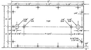
Fig. 2. Drill a  $7'' \ge 12'' \ge 3/16''$  Masonite panel to hold the soft iron loop and the pilot lamp sockets. Position of mounting screw holes is not critical.
