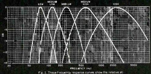
tenuation of each band of frequencies in the audio spectrum.
