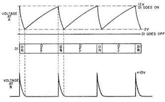
As battery current through R1 in this circuit is held to 0.5 ma. or less, it cannot hold the diode on; the capacitor recharges, and repeats the cycle.
