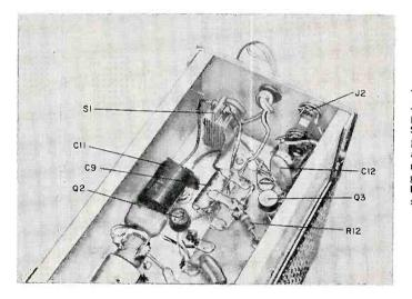
This view is toward the rear of the chassis. Jack J1 is under J2—one jack being regular phone size, the other a miniature. Switch S1 controls the time constant of the output circuit so that a chart recorder can read a rough average of the background noise not individual noise bursts. Circuit values given are suitable for use with a Rustrak low-cost chart recorder such as the one shown on the cover.
