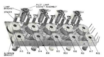
Fig. 6. The pilot lamps and controls are first preassembled on the aluminum bracket which is then mounted  $5/16^{\prime\prime}$  behind the front panel.
