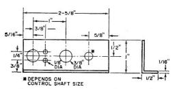
Fig. 2. Mounting bracket is made from 1/16''-thick aluminum plate cut to dimensions given. It acts as a heat sink for SCR1 and as a support for R3.
