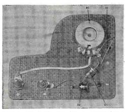
All parts, including banana plugs, are mounted on a piece of fiberboard shaped to conform to the meter.
