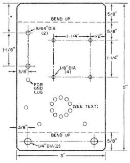
Fig. 2. The complete IC, including the battery supply, can be mounted on a small  $(3'' \times 5'')$  aluminum plate, drilled and bent to form a chassis support.
