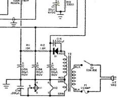
R9 thru R4-C5 before it is applied to V2. Switch S1 selects the coils for the desired band while R8 varies the regenera-
