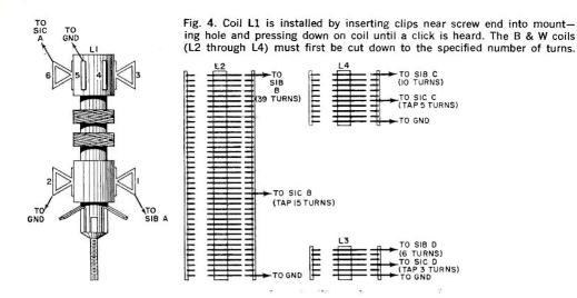
ponents and circuit wiring. Be sure to dress the 6.3-volt filament wires close to the chassis while keeping them away from the coils. Keep all wiring as direct and as short as possible.
