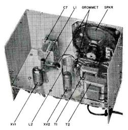
Fig. 3. Assemble major components on the chassis at the locations shown. Be sure to use four 3/8"long spacers between capacitor C7 and front panel.
