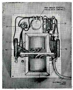
The author made a simple aluminum bracket to mount the two transformers back to back. Remainder of internal wiring is obvious from this rear view.
