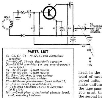
**Construction.** The preamplifier can be assembled on a  $2'' \ge 3''$  piece of perforated phenolic board, using push-in Vector terminals for the connections. If there is a space problem, you can use a smaller board and simply utilize both sides of the board. Mount the assembled board in any convenient spot in the recorder using stand-off spacers or two rightangle brackets which you can make from a thin piece of aluminum cut to the proper size.
