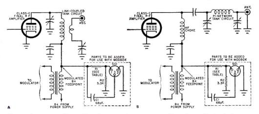
Fig. 1. Voltage divider R1 and R2, and harmonic frequency coupler C1 are installed in the final r.f. amplifier to obtain a sampling of harmonics and B-plus voltage without upsetting transmitter operation.
