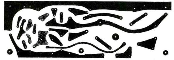
Fig. 6. Foil side of board is shown actual size to help you make your own; however, wiring isn't critical. 1967 Spring Edition
