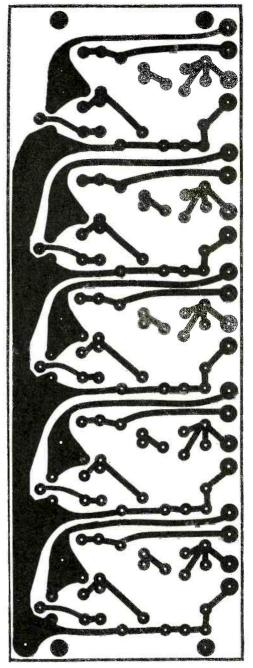
Fig. 11. Actual-size illustration of printed circuit board. For hole drill sizes, refer to Fig. 4.
