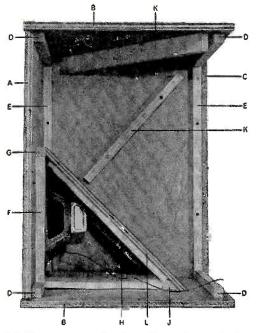
Except for the front, all inside surfaces of the woofer cage are covered with foam plastic. Loosely pack the woofer cage with a sheet of fiberglass.
