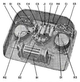
Only electrical connection to the chassis is at J1. The unused side of S2 conveniently serves as a terminal strip for the common capacitor leads.
