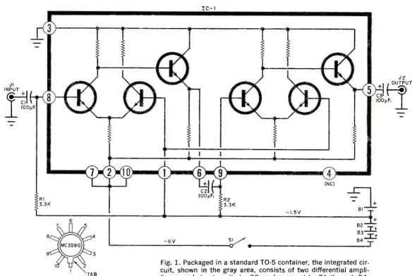
fiers coupled externally by C2, and powered by B1 through B4.
