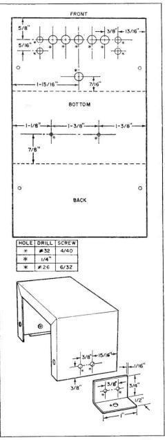
Location and size of holes may vary for different style of terminal strip. It's a good idea to lay out all parts before drilling any holes in the box.
