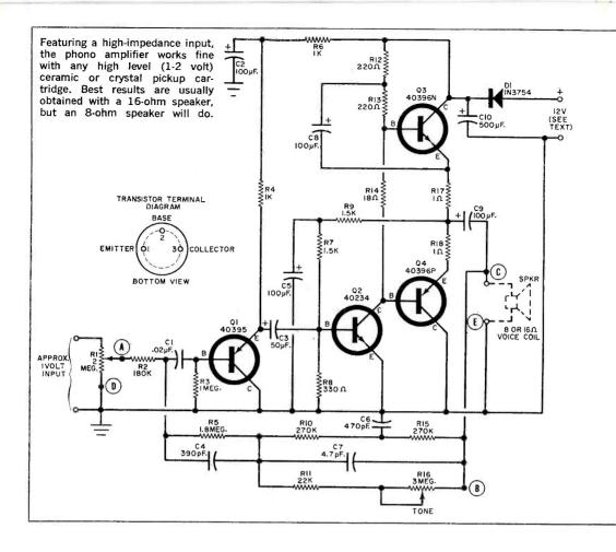
How it Works. The amplifier input from a phono cartridge is applied to the base of emitter follower QI (as shown in the schematic diagram, above) through volume control R1, limiter resistor R2, and coupling capacitor C1. With QI serving as an impedance-matching device, this transistor provides a high input impedance to the source and a low output impedance to driver Q2.
