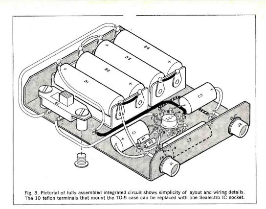
**Construction.** The circuit is easily assembled on an improvised aluminum plate laid out and drilled as shown in Fig. 2. The IC socket used by the author is made up of 10 teflon press-fit standoff terminals inserted into appropriate-sized holes drilled in the plate. Then the leads from the IC case are fanned out and each soldered to a standoff.
