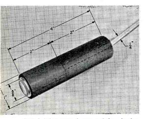
Fig. 3. Switches mounted on one end of wooden dowels make suitable hand-held responders. Any normally open push-to-close type of switch can be used.
