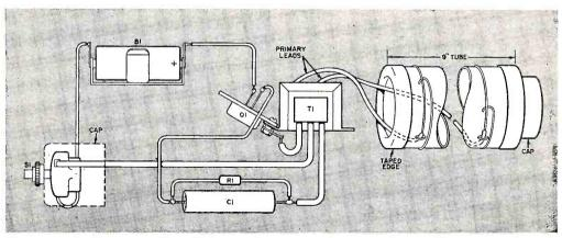
All components, including battery, fit into cardboard tube. Primary leads from T1 pass through inside of tube to the outside, and are covered with foil. About 1" of space separates the 4"-wide electrodes.
