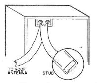
length of lead-in wire across the set's antenna terminals, letting the free end hang loosely toward the floor. Check to see if there's an
