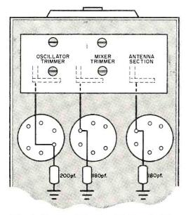
This combination wiring/pictorial diagram shows the exact wiring position of the three silver mica fixed capacitors. Placing these capacitors in the circuit bandspreads the receiver's tuning range.
