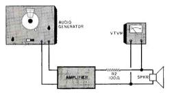
Typical test setup required to determine speaker and enclosure resonant frequencies if you use a different speaker or change cabinet dimensions.
