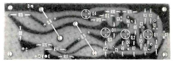
Fig. 3. Non-conductive paint is used on component side of printed circuit board to show location of parts. 10 ELECTRONIC EXPERIMENTER'S HANDBOOK
