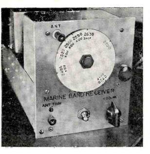
ANY small boat owner or SWL can change a BC-454/ARC-5 receiver into a bandspread 2.5-MHz marine band receiver. The BC-454 24-volt unit is easily modified for 117-volt a.c. operation (see "Converting Your First Command Receiver," POPULAR ELECTRONICS, June, 1963). To confine the original
