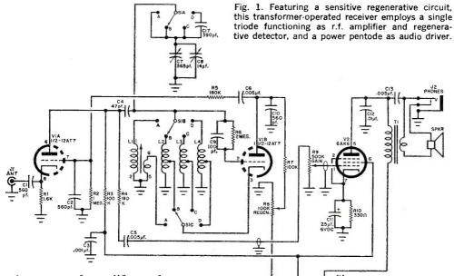
erates as an r.f. amplifier and regenerative detector. A power pentode (6AK6) drives the speaker or headphones through output transformer T1. Transformer T2, silicon diode D1 and a filter consisting of C15, R11 and R12 provide B+ power.
