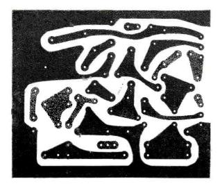
Actual size photos show foil side (left) and component side (below) of printed circuit board that can be used instead of point-to-point wiring. A packaged kit is also available (see Parts List).
