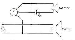
Low and high audio frequencies are separated by C1 and kept in balance by L-pad R1. For best results, the tweeter and woofer must be wired in phase.
