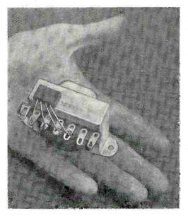
TINY MODULAR RECTIFIER CIRCUITS SIMPLIFY CONSTRUCTION OF A.C.-OPERATED D.C. POWER SUPPLIES
