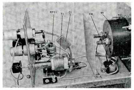
Note the aluminum shield that the author found necessary to add above the chassis to prevent feedback from the meter to the input circuitry surrounding Q1. Coupling capacitor C6 is mounted in a rubber or plastic grommet so that one lead is above the chassis, the other lead below it. Leads to the meter pass through another grommet.
