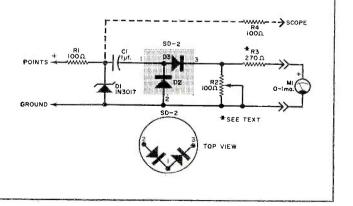
3.5 ma. would indicate 3500 rpm.) When other commercial rpm meters are used, R3 may have to be jumped, as some of them incorporate 0-2 ma. movements. Regardless of scale markings or meter movements used, you should calibrate the tach before you install it in your car.
