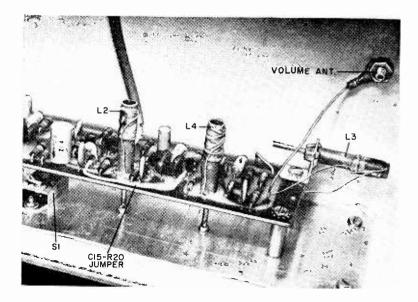
circuit consisting of L4 and C22. The r.f. signal across this second tuned circuit is rectified by diode D1 and applied to the base of d.c. amplifter Q5. Thus, the d.c. voltage level present at the collector of Q5 is a function of the amount of r.f. present on L4-C22. This level is at its maximum when the L4-C22 tuned circuit is at the same frequency as the Q4 collector tuned circuit.
