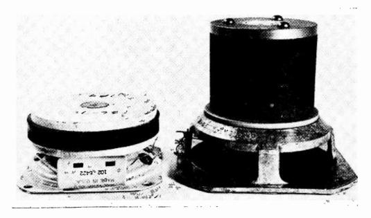
Massive magnet size of both tweeter (left) and woofer are apparent in this photo. Although low cost, these speakers are of modern design and capable of very good sound. fiberglass. And, finally, the back can be installed; a gasket of thin cork, felt, or caulking compound around the rear cleats is desirable to eliminate air leaks.
