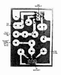
Although the author used this PC board layout, you could build the FET calibrator on a sturdy perforated board.
