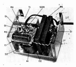
Fig. 3. The perforated circuit board is secured to the side of the chassis with a small L-bracket. Resistor R1 is mounted directly on bulb 11's socket.
