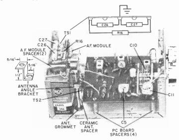
Fig. 5. Shown at left are construction details for the antenna mounting bracket and the parts arrangement on terminal strip TS1. Battery is held in place by a metal clamp. each screw from inside the cabinet, placing each lug so that it bears against the mounting lip of the speaker. Fasten the lugs in this position with two 4-40 nuts, so that the speaker and grille are securely held against the cabinet.
