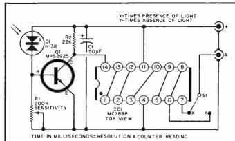
Fig. 11. This high-speed photo pickoff employing a silicon photo-diode is extremely useful in timing fast camera shutters, dragsters, or any high-speed phenomena where a beam of light can be interrupted. The switch permits operation either with presence or absence of light. A similar technique can be used to verify flash synchronization.
