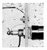
is cut, secure it to the panel with the hex nuts as shown in the photo. Solder hookup wire directly to the pipe, or to a solder lug placed under the hex nut. Now bend a 3/8" wide by 2"-long (approx.) piece of springy brass strip as shown, and
