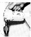
be used with  $\frac{1}{4}$ " drills is the most convenient and inexpensive type. Many hardware stores sell imported chucks for about 98 cents. The mixer-cum-drill can then be used to drill holes in metal chassis or woodwork. You can also take advantage of the variable speeds available on this type of mixer. —Art Trauffer
