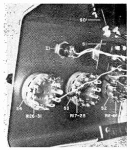
Timing resistors R8 through R31 are soldered to the terminals of rotary switches S2, S3, and S4. If you use 5% resistors, cut the wire leads short, but use a minimum amount of heat to make connections.
