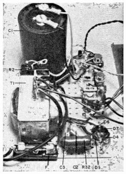
Any layout plan convenient to the builder can be used to duplicate construction of the Stopclock. The author used perforated phenolic board because the circuit was totally enclosed in a metal cabinet.
