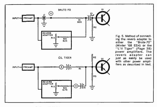
either the "Brute 70" or "L'il Tiger." The value of R12 shown in Fig. 1 is correct for use with power supplies between 40 and 50 volts. For higher voltage sources, such as are found in vacuum-tube equipment, the value of R12 will have to be increased to a value that delivers the approximately 30 volts required by the reverb adapter, as shown in Fig. 6.
