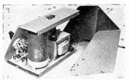
The author managed to squeeze everything in a Bud sloping panel aluminum box (Type AC-1612). A phenolic board bearing most of the wiring is supported away from the metal bottom of the box with short insulating spacers. Size of the box used will be determined by the physical size of charging capacitor C1. A smaller and cheaper capacitor can be used at C1. Investigate the Sprague 36D or 39D series electrolytics stocked by some industrial parts suppliers.
