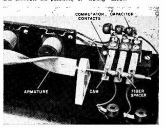
The armature is fabricated from a  $\frac{5}{8}$ "-wide x 6"-long strip of  $\frac{1}{8}$ "-thick soft iron twisted as shown in Fig. 4; aluminum or other non-ferrous metal *cannot* be used. You can start with a strip about 2' long. Put one end in a vise and attach a long wrench on the other end. Twist the strip until you wind up with 1 complete revolution (360°) within a 6" length. Mark this piece off and use a hacksaw to cut away the unused portions. Cut a notch on each end as shown.
