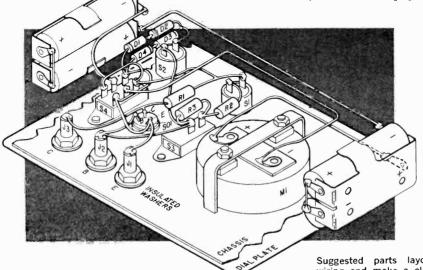
Suggested parts layout to simplify wiring and make a clean-looking unit.
