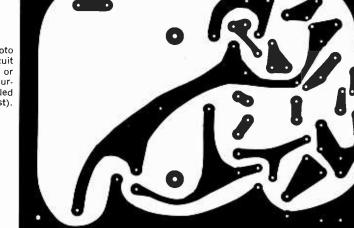
Fig. 5. Actual-size photo of amplifier printed circuit board can be copied or the board can be purchased etched and drilled (see note in Parts List).
