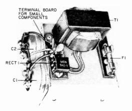
Fig. 6. The power supply is built on a 3" x 3" piece of heavy-gauge aluminum with a  $1\frac{1}{2}$ " mounting lip.
