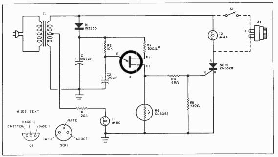
Fig. 1. When R6 is shielded from the light by an opaque card, the unijunction SCR-bulb I2 circuit operates once per second. Without a message in the slot, the circuit shuts itself off and remains on standby.
