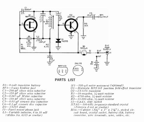
Circuit of the FET calibrator is designed around commonly available solid-state components. A phono jack on the front panel permits operation of the calibrator from an external power source.
