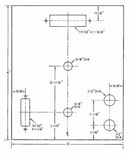
Fig. 2. Front panel cutout and drilling information. The author used a standard size aluminum utility box and discarded the mating section. A new section was bent from perforated aluminum. The new section provides ventilation and eliminates the shock hazard of accidentally touching components.
