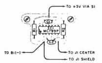
Fig. 5. Component layout. Note that the IC carries both a coding dot and notch for proper positioning.
