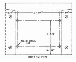
Fig. 6. If you obtain the LMB box used by the author, these rear, front and bottom view drawings will guide you in drilling necessary control holes.
