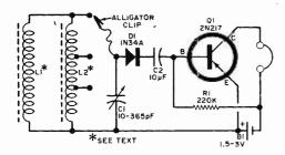
Stacked ferrite core antennas (L1 and L2) provide an AM radio with increased sensitivity to incoming signals. Since the antennas also form part of a tunable tank circuit, they must be specially wound.
