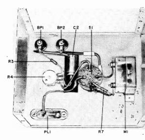
Fig. 3. In this rear view of the front panel, the location of those components attached to the panel can be seen. All of these components should be attached after the front panel has been lettered.
