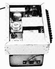
In this underchassis view, PC board has been put in place and leads brought out to a 12-tag strip.
