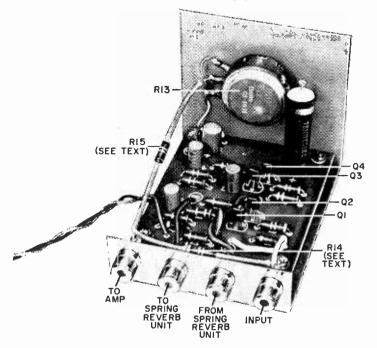
Fig. 4. The finished board can be mounted on a metal chassis with the external connections completed as shown here. Short spacers isolate board from chassis.
