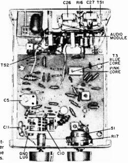
the signal, applying it to the primary of ratio detector transformer T3 through "swamping" resistor R12. The effect of strong signals on the high primary inductance of T3 is limited by R12, preventing "ringing" and oscillation in the circuit. The i.f. signal applied to the tuned primary of T3 is induced into the tuned secondary through mutual coupling. Both the primary and secondary windings are resonant at 10.7 MHz, being tuned by C18 and C19 respectively.
