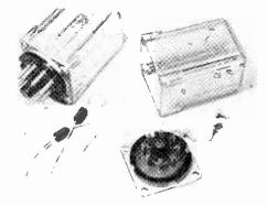
against high voltage hazards. After removing the plastic case from the octal base as shown in the photo, solder the silicon rectifiers to the correct base pins. Then drill a few small holes in the plastic cover to allow for heat dissipation when the rectifiers are in operation, and replace the cover. This same type of dust cover can be used for housing small projects and other circuit modifications not associated with power supplies. —*Fred H. Horan*
