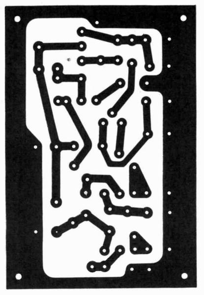
Fig. 3. Construction of COMPLY is greatly simplified through use of a printed circuit board. You can make your own board if you follow this twice-size board pattern. An etched and drilled board is available to readers at a very low cost.
