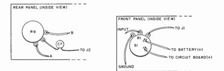
Fig. 7. Before mounting the COMPLY printed circuit board, attach the two controls, R1 and R9, to the front and rear panels, respectively. Capacitor C7 is then soldered in place from R9 to J2.
