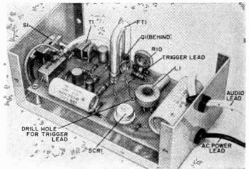
Fig. 4. The finished strobe before the top cover and reflector are assembled. Note that a hole must be drilled in the PC board to accommodate the lamp trigger. Be especially careful when installing the strobe tube as it is fragile and it cannot withstand mechanical shock. The flashtube is polarized. The end of the tube with the mesh attached to the wire inside the tube must be connected to the ground side of circuit.
