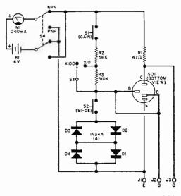
Note that there are two base contacts on SO1 to accommodate both the TO-5 triangular lead configuration and the older in-line arrangement.
