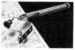
up things. To use the "pencil," simply depress the plunger at the top, and when the gripper jaws extend, clamp them over the part to be heat-sinked or picked up. Then release the plunger. After the work is done, depress the plunger again to release the jaws. You'll find that this "tool" is a real time-saver when you're working on circuits that look like they
