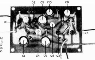
Fig. 5. The printed circuit board should look something like this just before it is mounted in the cabinet. Capacitor C7 is not on the board—this capacitor is connected directly between R9 and J2.
