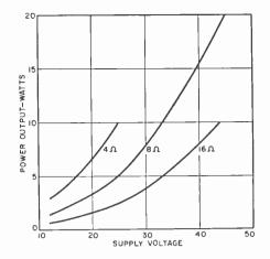
Fig. 3. If you know supply voltage and speaker impedance, amplifier power output can be determined.
