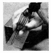
"Stake" the edges of the screw hole with a broad-bladed screwdriver or small dull chisel. All it takes is a few light taps with a hammer. -Henry R. Rosenblatt
