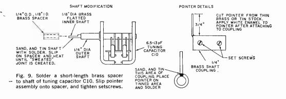
o.d. x  $\frac{1}{8}$ "-i.d. brass spacer to the existing shaft. Lightly sand the shaft and apply a thin coat of solder. Now slip the brass spacer onto the tinned shaft, heat the spacer until the solder on the shaft flows and allow the spacer-and-shaftjoint to cool.
