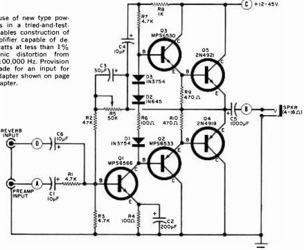
Another solution to the problem has been to use one silicon and one germanium power transistor in the output stage. This combination can lead to thermal (heat) compensation problems, and the transistors are usually far from complementary in their characteristics. Again, lots of negative feedback can produce a pretty good amplifier, but feedback is used to correct for circuit nonlinearities, rather than the circuit being inherently linear with feedback used only to make it better.
