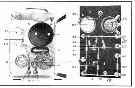
The completely assembled DCEV (left, above) is made up of the front-panel assembly (center), and the insulated board assembly (above, right). Battery is clamped to bottom of case as shown. Note that R20 is mounted on the transistor side of the board (see text).
