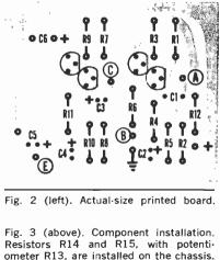
of these two resistors. With transistor audio equipment, resistors R14 and R15will be in the range from 1000 to 4700 ohms, again with the best value determined by experimentation. A good compromise is 2200 ohms.
