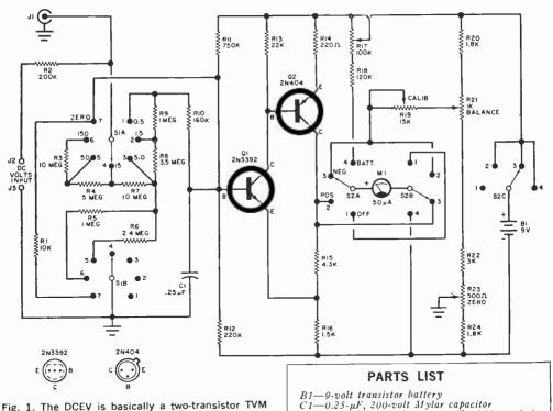
Fig. 1. The DCEV is basically a two-transistor TVM (transistor voltmeter) having the very high input impedance of the VTVM and the portability of a VOM. Unlike most VOM's, the DCEV has a 0 to 0.5 volt full-scale lower range, making it ideal for use with any type of semiconductor circuit including IC's.
