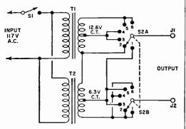
T1 and T2 are improperly phased. For correct phasing, simply reverse the primary connections of only one of the transformers. When d.c. voltages are required, the output at J1and J2 can be connected to a rectifier and d.c. filter network. —*Frank H. Tooker*
