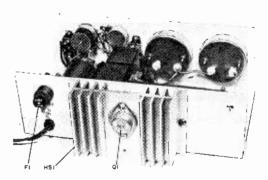
Fig. 5. Rear view of power supply chassis. Transistor Q1 is thermally (not electrically) connected to heat sink HS1. The heat sink is mounted to the rear apron of the chassis, as is the line fuse.
