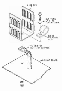
Fig. 7. Method of installing each power transistor, heat sink, and diode mounting clamp. The cupshaped lock washer is necessary to prevent cracking the power transistor when it gets hot after long use.
