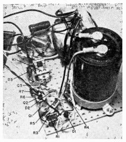
Parts placement is not critical in circuits like the Stopclock. Point-to-point wiring using small terminals and transistor sockets proved convenient for the author. As mentioned in the caption to the photo above, the size of C1 is larger than need be for this project. Use any metal enclosure to house your duplication of this unusual timer project.
