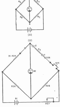
Fig. 2. The classical Wheatstone bridge is illustrated at A, while B shows how it is created in the bridge-substitution box project.
