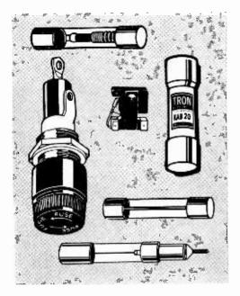
FROM a strictly mechanical point of view, fuses may be placed into two general categories. The first category is the "clipin" fuse, which must be placed into some kind of fuseholder or a pair of clips to perform its normal function. The other category includes those fuses that have leads soldered to the end-caps and are generally referred to as "pigtail" fuses. Pigtail fuses can be soldered directly into an electronic circuit or printed circuit board, without a fuse-holding device.
