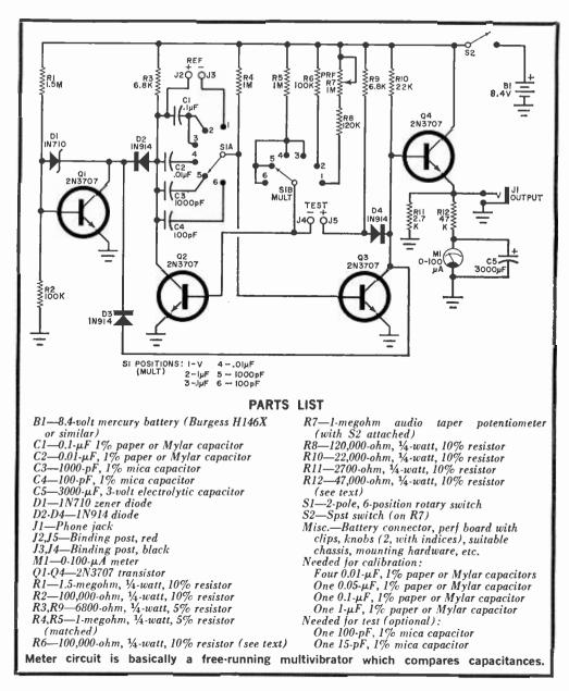
charging time is reduced tenfold when S1B switches from R5 to R6, the latter being selected during calibration.
