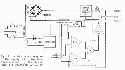
to transformer TI, one of whose secondaries supplies bridge rectifier RECTI and filter C3 to provide unregulated dc for the overall regulator. The other secondary supplies rectifier DI and filter CI to create the dc power required by the reference voltage regulator in ICI.
