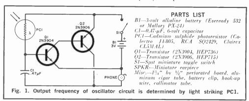
light striking the sensitive surface of a photoresistor (PC1). The prototype has a frequency range of up to  $5500~{\rm Hz}$ , depending on the amount of light striking PC1.
