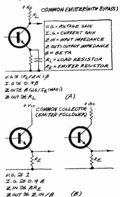
than unity, the common-collector approach can't be used. The common emitter (Fig. 4A) looks good except that the desired input impedance is higher than that normally associated with a common-emitter circuit. So we have to add another stage (emitter follower) to raise the input impedance (Fig. 4B).
