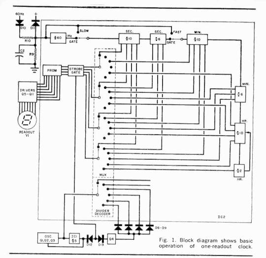
er. An output and reset are incorporated to return these counters to zero on the next pulse after counting to 59 seconds. This output line also provides a one-pulse-per-minute signal for the minutes counter.
