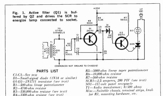
Circuit Design. Almost any npn transistor can be used for Q1 and Q2 as long as the one for Q1 has a minimum beta of 50 and for Q2 a minimum beta of 100. The SCR should have sufficient power rating to operate the lamps to be used. If lamps with voltage ratings other than line voltage are used, the rating of the SCR may have to be changed. For very large loads, transistor Q2 should have a high output and R6 and R7 may have to be decreased in value to provide the extra drive.
