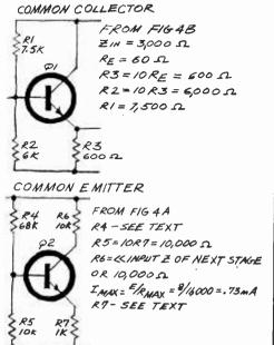
this time, R6 would be considered in regard to the desired voltage gain. A quick check shows that the 10,000-ohm value provides a gain of over 20.
