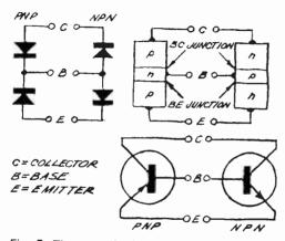
Fig. 5. Three methods of drawing transistor.
