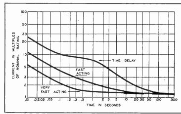
Fig. 1. Operating characteristics of three fuse types described in text.
