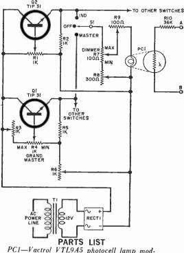
PC1—Vactrol VTL9A5 photocell lamp module (do not substitute)\*
