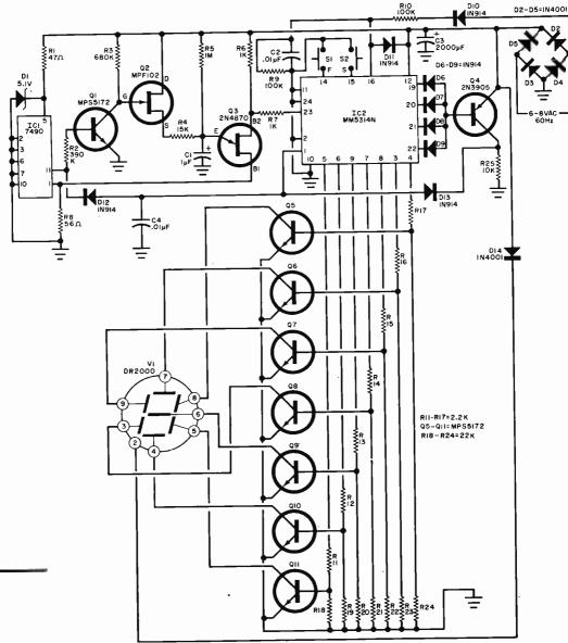
Q3—Unijunction transistor (2N4870, 2N4871) or MU10)
