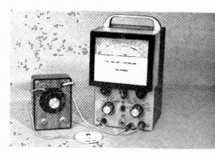
Photosensitive resistor *PC1* is mounted between two small pieces of insulating material such as plastic or insulation board with the sensitive surface exposed through a hole. After connecting the cable to *PC1*, and closing the "sandwich," paint the enclosure (not the sensitive *PC1* surface) white.
