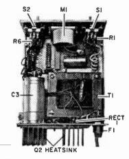
This shows completed supply except that the small board is not plugged into edge connector so that it doesn't hide other parts.
