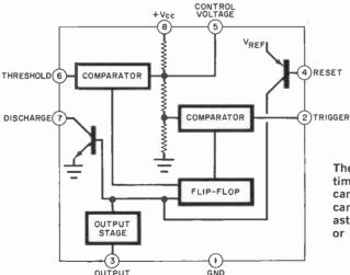
The internal circuitry of the 555 timer IC. Besides timing, the IC can be used as an oscillator and can operate in both monostable and astable modes. The output can sink or source 200 mA or drive TTL.
