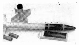
One of the most spectacular developments in model rocketry is the Cineroc movie camera shown here. Constructed of sturdy black plastic, camera has enough 8-mm color film to record over 20 seconds of high-speed rocket flight. Camera shown here is mounted on a carrier rocket. The stubby, four-finned section to the rear is rocket's first stage booster. In front are two engines and plastic encased film holder.
