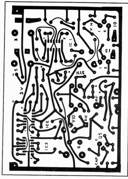
wire (close-wound, with one turn touching the other). Then carefully spread the coil until the ends are %-inch apart. Bend the end leads to the proper angle and remove the resistor before mounting the coil. Before the coil is soldered to the board, solder one lead of C18 to the coil, four turns from the end connected to the collector of Q5. Note that this lead of C18 does not go through the board, but directly to the coil.
