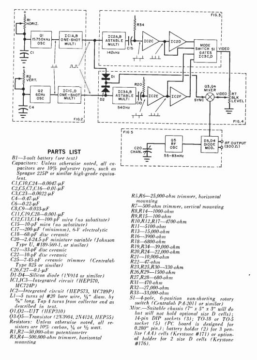
Fig. 1. This is the logic flow diagram of the convergence generator. The boxes in dashed lines show the four major sections: at left, the sync oscillators; upper right, horizontal drive; below that, the vertical drive; and, lower right, the r-f section. Some typical waveshapes are also shown to indicate circuit operation.
