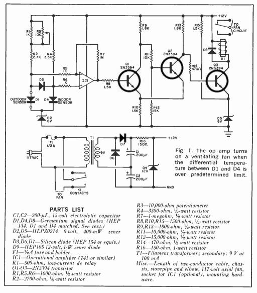
working margin is included by using the trigger to drive a biased power stage, Q3, which has the relay in its collector circuit. The emitter of Q3 is biased by R15 and zener diode D5, so that Q3 is either on or off. When the positive-going signal from Q2 occurs on the base of Q3, it turns on very fast, energizing the relay.
