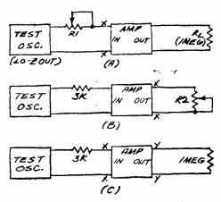
Fig. 9. Testing input/output impedances.
