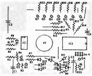
"Hurry-up" logic is built into the circuit to speed up the counting process when it is necessary to set the time. An externally operated switch (S2) bypasses the first divide-by-60 divider, increasing the count speed by a factor of 60. Another switch (S1) bypasses the first three dividers, increasing the count speed by a factor of 3600. These two switches are used to set the clock.
