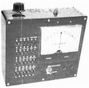
Any size zero-center microammeter may be used and the meter scale may be left "as is," or marked as "over" and "under" on the right and left sides. The meter scale divisions are not used.
