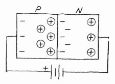
Fig. 2. Pn junction is shown forward-biased.
