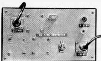
A front panel mounted crystal socket permits moderate shifting of the received frequency without internal retuning. If you use an external 6-volt supply, be sure to remove the dry cell.
