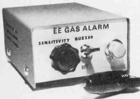
Author's model for portable use. A remote location for both the semiconductor "nose" and Sonalert alarm is an option to consider.
