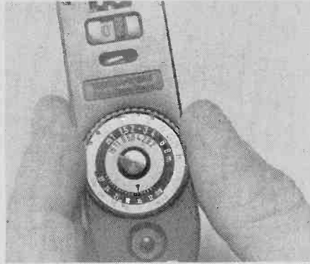
To calibrate Flash-Mate you will need an accurate electronic flash with an f-stop computer disc. Calibration can be done either for ambient light or bounce flash.
