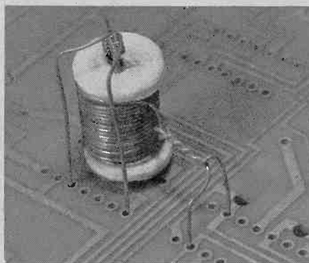
Because of their compactness, these home brew relays are easy to mount on a PC board. This particular double pole relay uses two switches within one coil.
