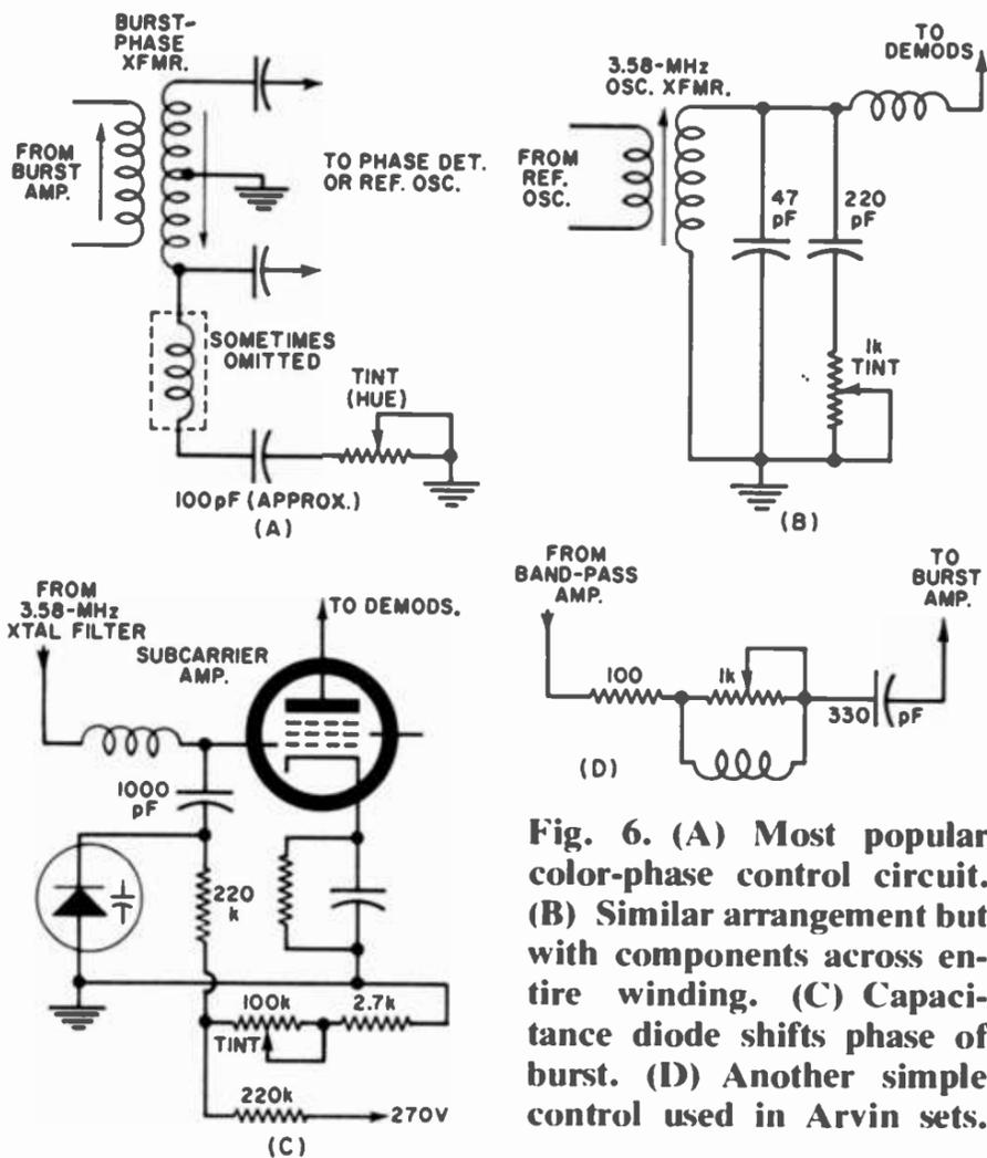
**Fig. 6.** (A) Most popular color-phase control circuit. (B) Similar arrangement but with components across entire winding. (C) Capacitance diode shifts phase of burst. (D) Another simple control used in Arvin sets.
