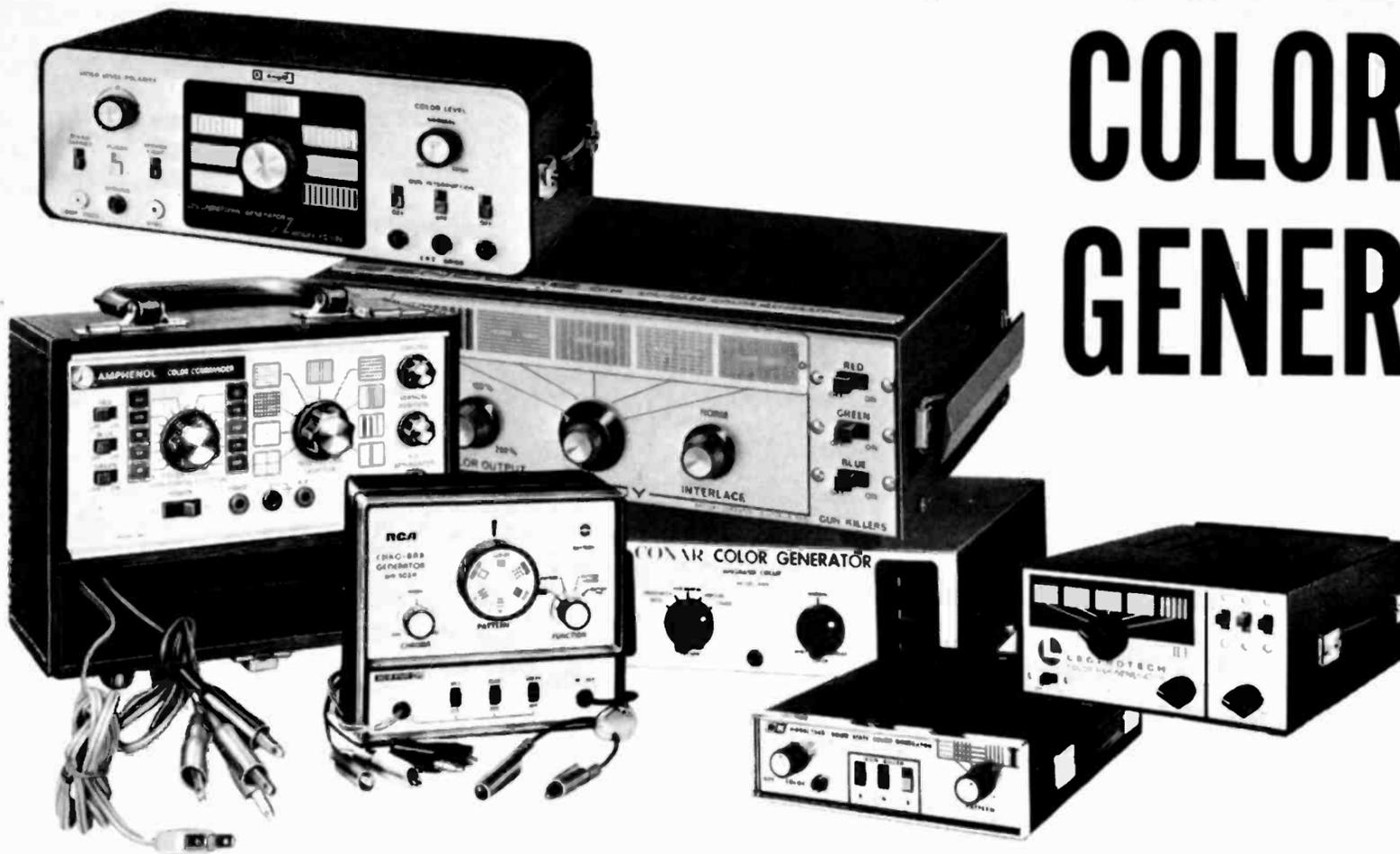
*Improved stability, more reliability, longer life, cooler operation, light weight, and portability are the direct result of using transistors and IC's in a new generation of color-bar generators. Here is a complete directory of what's available, along with how the various units operate and compare.*
