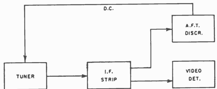
Fig. 4. Closed loop forms automatic fine-tuning system.
