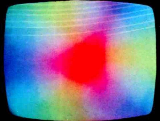
**RED FIELD PURITY** Set up screen for purity adjustments while operating red gun only with yoke pulled back. Off-centered red spot (top), is centered (above) by adjusting red purity magnet.
