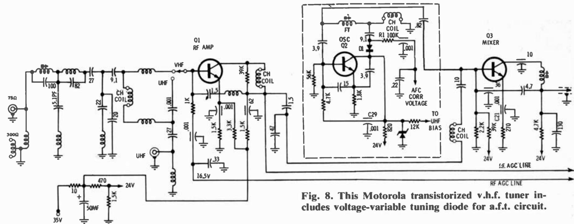
Fig. 8. This Motorola transistorized v.h.f. tuner includes voltage-variable tuning diode for a.f.t. circuit.
