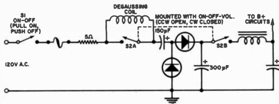
**Fig. 6.** Manual degaussing system used in a Philco.
