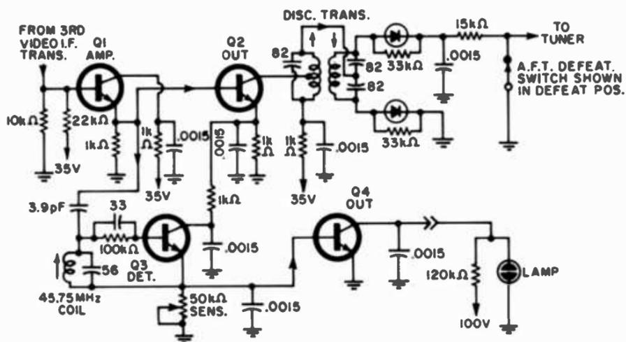
Fig. 9. Motorola's a.f.t. system, "Fine Tuning Lock."
