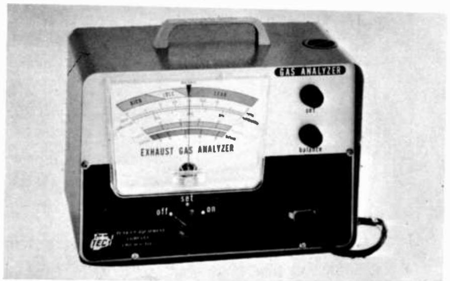
**To analyze the exhaust gas from your car's muffler, a gas analyzer, such as Tune-Up's EGA-100, may be used.**
