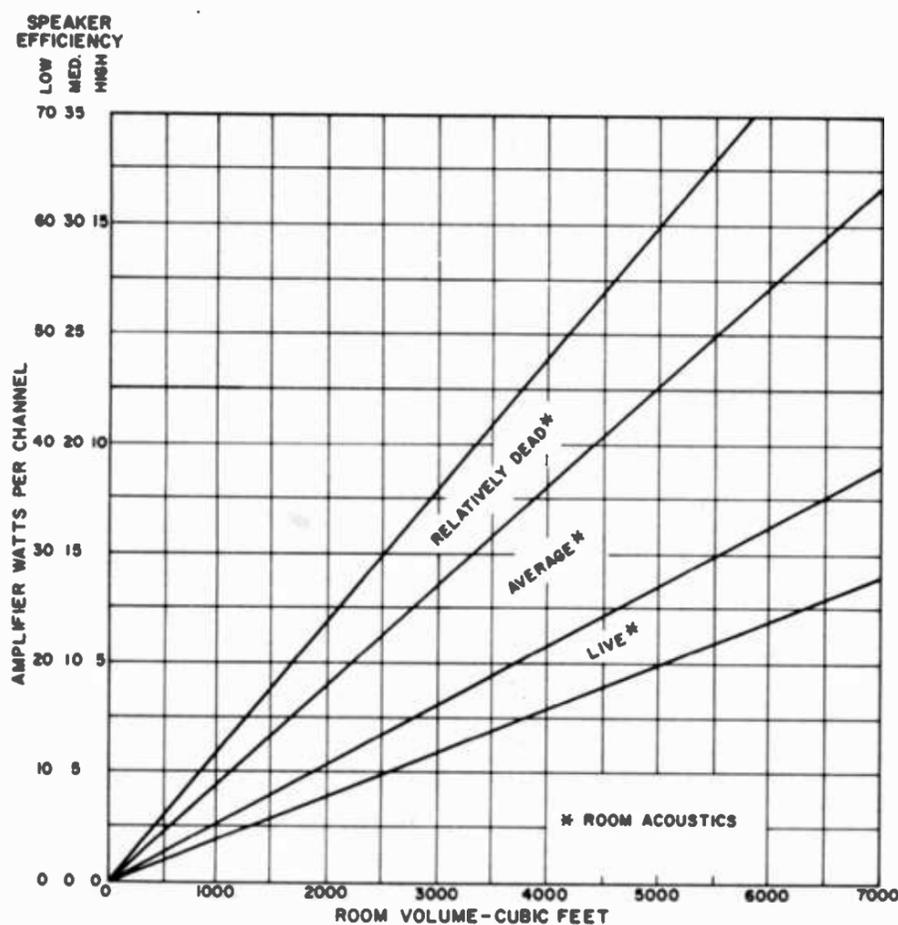
**Fig. 1. Continuous power requirements for various room sizes and acoustics, for speaker systems of different efficiencies. In general, completely closed acoustic-suspension systems are fairly low in efficiency while closed and ported enclosures using efficient speakers are fairly high in efficiency. If most listening is at very high levels, somewhat more power is needed, at low levels, less power is needed.**
