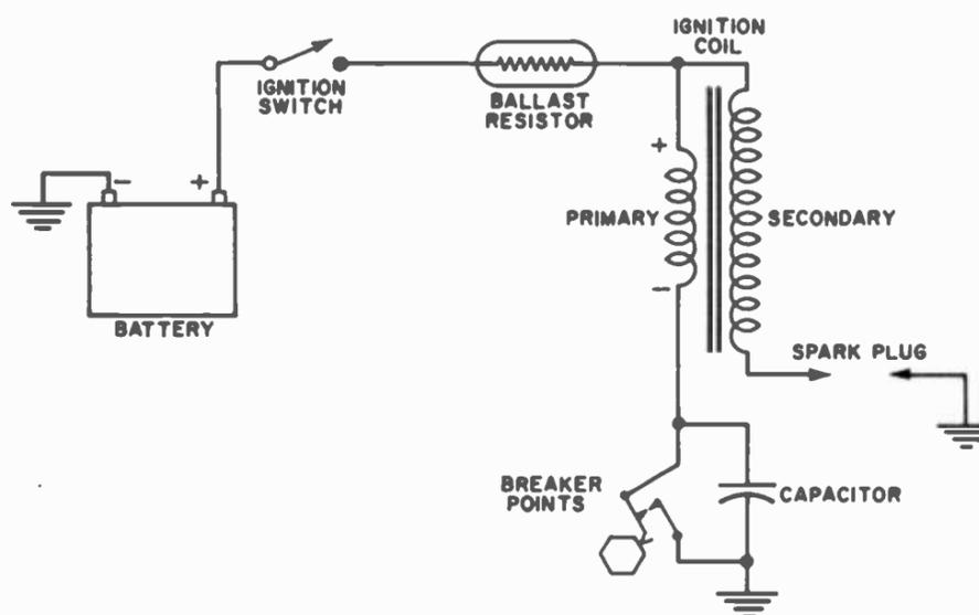
an open circuit between the "+" terminal of the ignition coil and ground. This could be caused by a bad ignition coil, improperly set or dirty points, or an open wiring connection. The source of trouble can usually be isolated by checking continuity with an ohmmeter, or by trial and error substitution of components.
