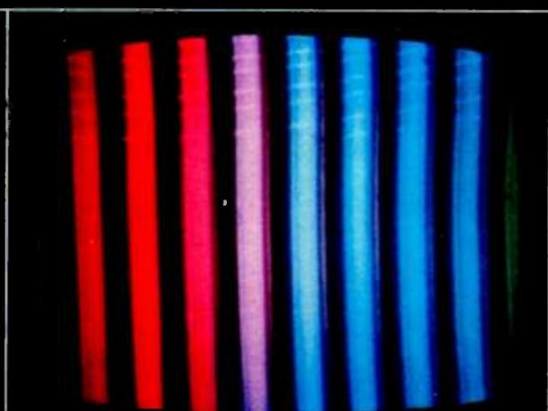
**COLOR BAR PATTERN** Normal display is indication of proper operation of phase, matrix, and other circuits.
