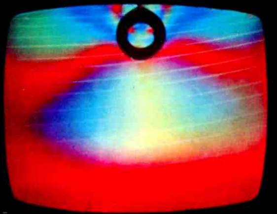
**WEIRD COLORS** Distortion caused by magnet held close to screen. Use degaussing coil to demagnetize tube and set before adjusting convergence.
