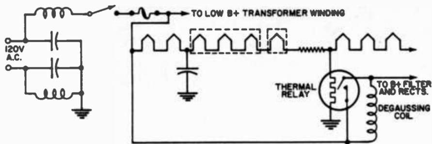
**Fig. 5.** Some sets use thermal relay to cut off degaussing action before receiver raster comes on. Action of large B+ filter capacitor causes current to taper off gradually in degaussing coil before it is shorted.
