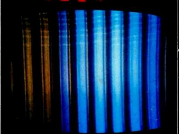
**DEMODULATORS INOPERATIVE** Defective Z (or B-Y) demodulator shows up mostly as loss of blues (top); predominant loss of reds (above) can be traced to troublesome X (or R-Y) demodulator. Absence of the red or blue colors also causes a loss of the green.
