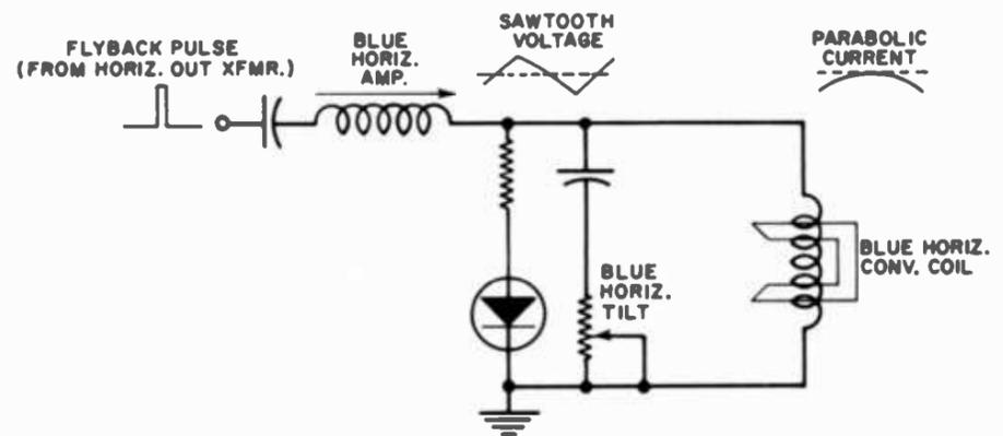
**Fig. 8. Blue dynamic horizontal convergence circuit.**
