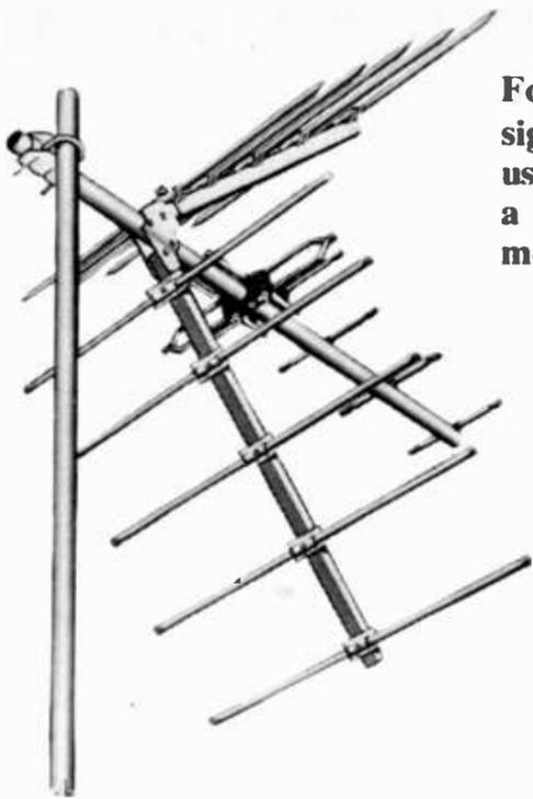
For long-distance reception of u.h.f.-only signals, an antenna of this type may be used. The RCA 10B715 shown, combines a yagi antenna with folded-dipole driver mounted with corner-reflector assembly.
