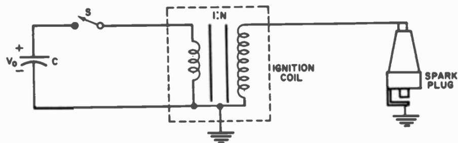
Fig. 6. A simple capacitor discharge circuit and coil.
