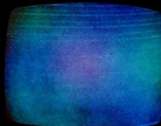
**POOR FIELD UNIFORMITY** With only the blue gun operating, discolorations due to poor purity adjustments show.
