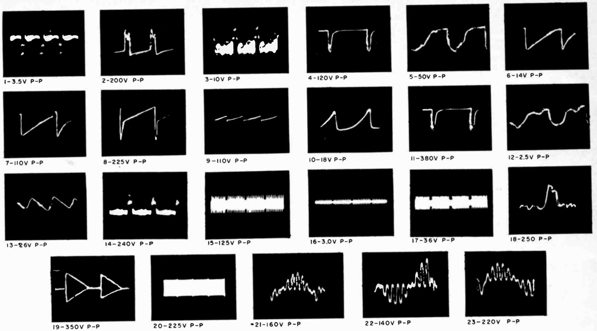
The troubleshooting waveforms shown above have been keyed, by means of numbers, to test points shown circled on schematic. For chroma waveforms, use color-bar generator, wide-band scope with low-capacitance probe.
