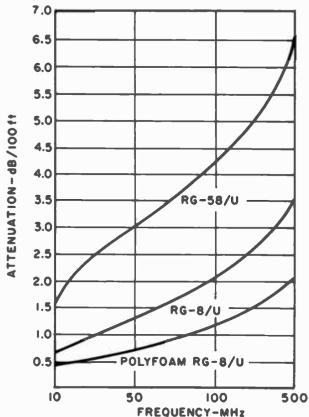
Fig. 3. Attenuation of common coaxial feedline cables.
