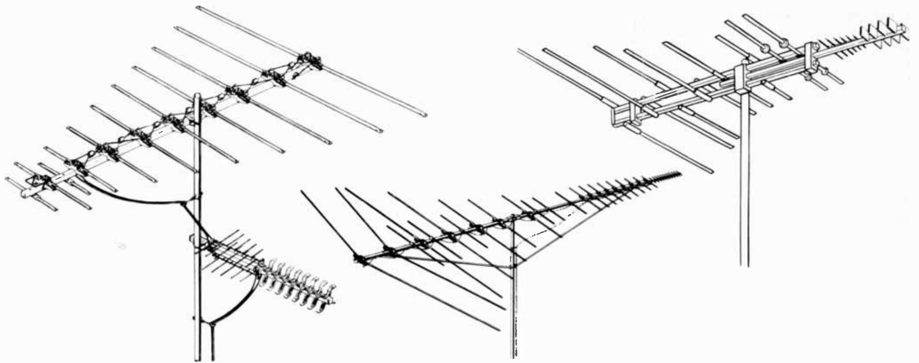
(Left) When u.h.f. stations are located in a different direction from v.h.f. stations and a rotator is not a part of the antenna installation, then separate u.h.f. and v.h.f. antennas may be used. In the example shown here, a Lancer Model LC882 antenna is connected to a Model LU820, from which a single downlead is run to the television receiver. Another alternative is to use a combination antenna with separately orientable sections.
