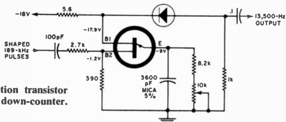
**Fig. 5. The unijunction transistor as a color-generator down-counter.**
