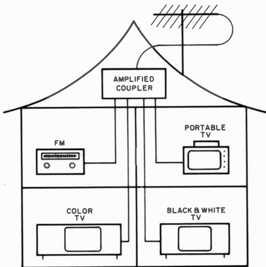
Fig. 5. An amplified coupler feeding four receivers.
