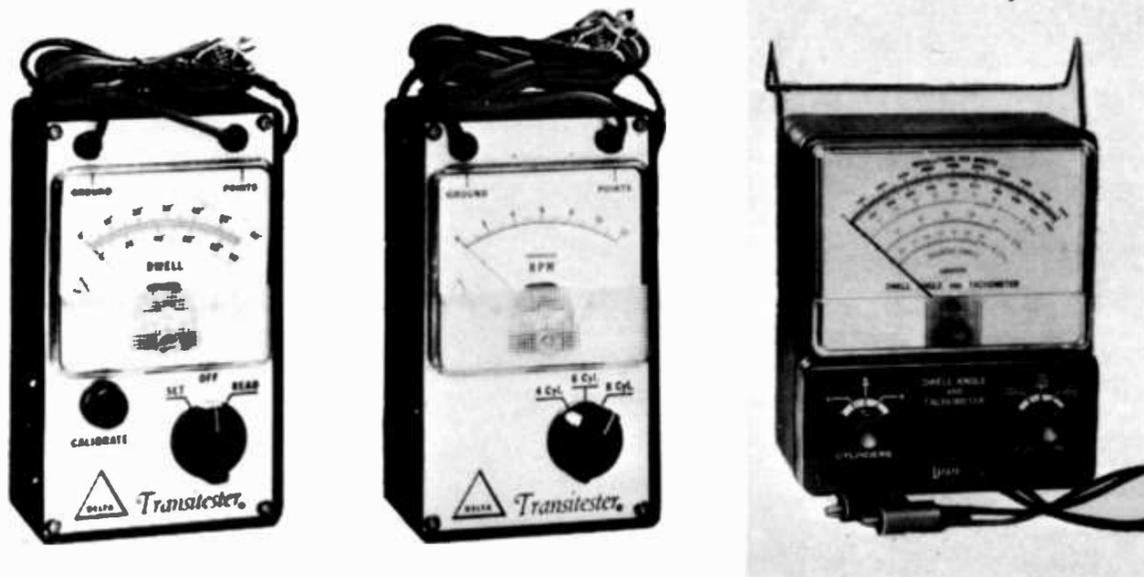
Examples of typical dwell meter (far left) and tachometer (center) are these Delta D-1000 and T-1000. Such units show how long breaker points stay closed, and speed of engine. A combination automotive dwell meter and tachometer (right) is this Lafayette No. 11-0101 unit.
