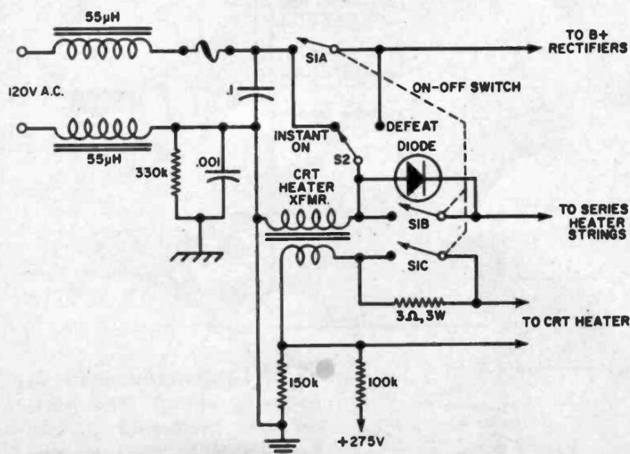
to all tube heaters at all times, even though the set switch is "off." Turning on the switch causes full voltage to be applied to the tubes and also activates the "B+" supply. The entire set comes on almost instantly—within about 8 seconds in the slowest set. Sound is usually a little faster, sometimes preceding the picture by about 5 or 6 seconds.
