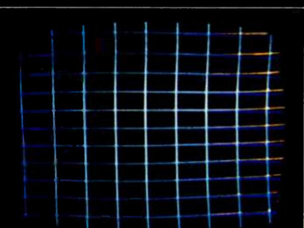
**BLUE HORIZONTAL LINES** Straighten the blue horizontal center lines to correct droop and misconvergence.
