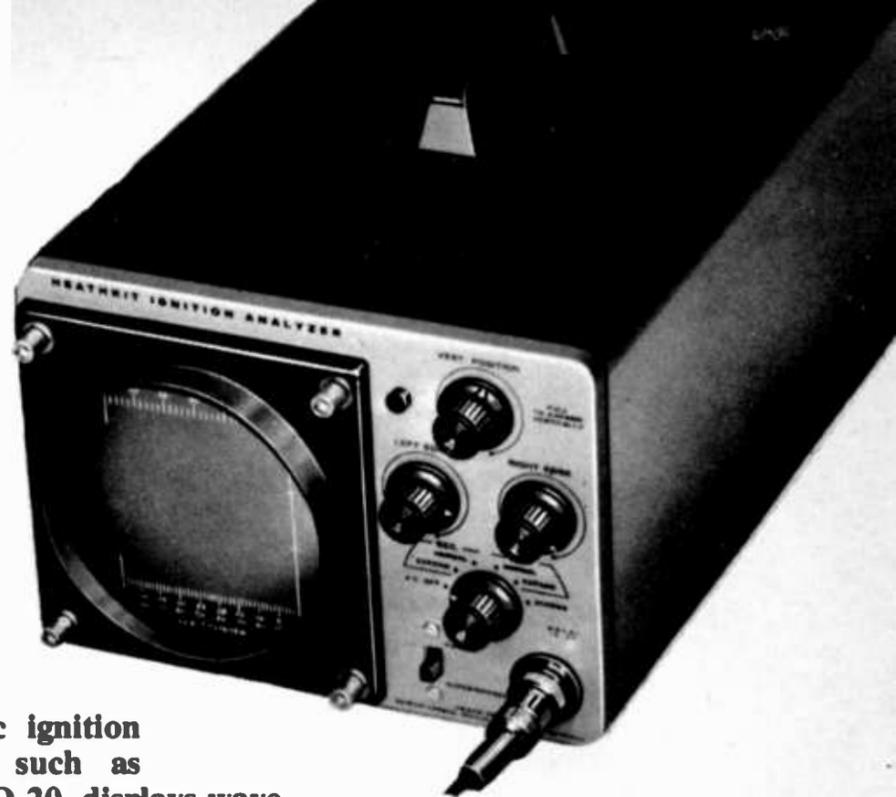
Electronic ignition analyzer, such as Heath's IO-20, displays waveforms (Fig. 1) that will show operating condition of an automobile's ignition system.
