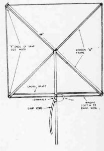
**Extra-large** loop antenna and capacitor C1 form a tuned circuit covering the very low frequency band. The antenna should be positioned for best sensitivity and least noise.
