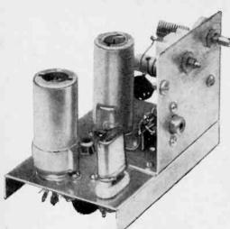
Transmitter subassembly at left is available prewired or as a kit. Construction from scratch is not recommended because of critical wiring and parts mounting.
