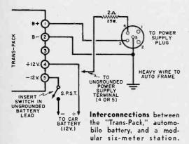
mounting plate. The 5-screw terminal strip is mounted on the *outside* of the chassis lip to minimize the possibility of shorts.
