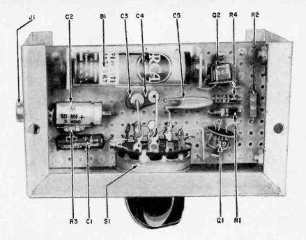
charge and allow the generator to operate. Vary the potentiometer resistance until the square waves are symmetrical. Shut off the generator, disconnect the potentiometer without disturbing its setting, and measure its resistance. Then select a resistor of the same value and wire it in place.
