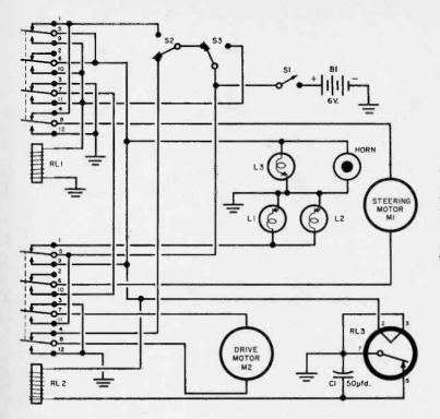
The coding of brain relays RLI and RL2 correspond to the relay contact pictorial shown on next page. Note that RL3 may not operate unless batteries are at full charge.
