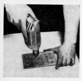
**Template** for making the fixed plate of the tweeter. Use a  $\frac{1}{4}$ " bit to drill the  $\frac{1}{8}$ " steel plate. Two holes must be countersunk for heads of bolts to fit flush.
