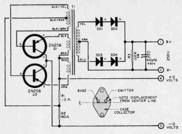
Special circuit of the "Trans-Pack" is made possible by transformer TI which was developed for transistor oscillator power supply applications.
