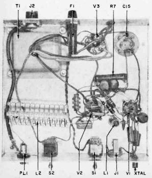
**Pictorial diagram** above details the connections to tube sockets VI and V2. The leads need not be as long as this but should connect to points indicated.
