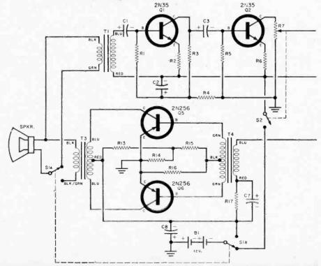
compact, the unit presented here combines a ten-watt power trumpet with a second high-gain amplifier that can convert the sound of an approaching automobile into that of a roaring avalanche. It's completely transistorized and, except for the flaring horn and the telephone handset, is contained complete with batteries in a 5" x 6" x 7" aluminum cabinet.
