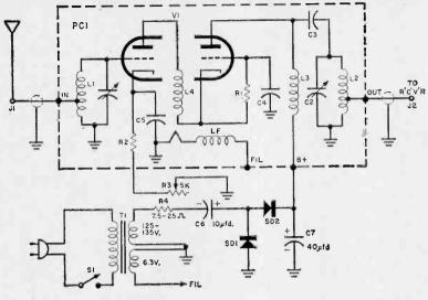
Schematic diagram of cascode r.f. unit. Part of schematic shown in dotted lines is printed-circuit board.
