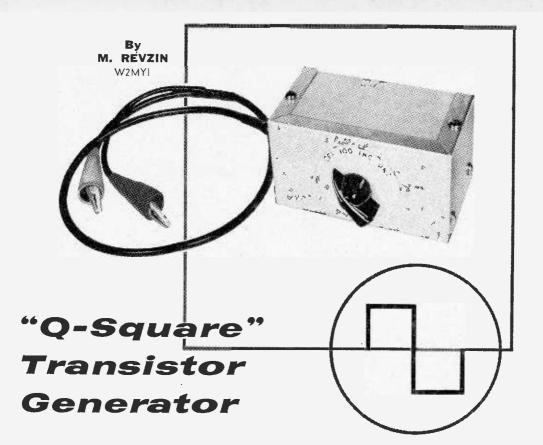
We have all read of the advantages of using square waves to test our hi-fi equipment, only to be scared off by the cost and complexity of the generator. The rise-time requirements are strict, or interpretation of the results is very difficult. However, low-cost transistors are available which make possible a simple unit with rise-times as good as 2.5 *microseconds*.
