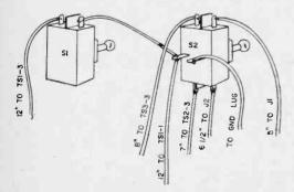
Fig. 6. Wiring details of toggle switches SI (on-off) and S2 (transmit-receive). Leads to J1 and J2 should connect to the normally grounded lugs (J1 and J2 are insulated from the metal chasis by  $1/2^{\prime\prime\prime}$  rubber grommets).
