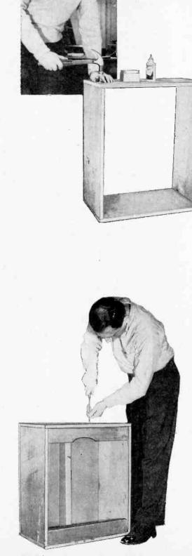
Sides, top and bottom of enclosure are assembled using a good wood glue and 8d (penny) finishing nails. All joints are butted with five or six nails per joint. Design of cabinet makes use of cleats unnecessary.
