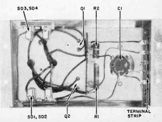
Parts arrangement beneath the chassis is non-critical. Holders for the silicon rectifiers may be fuse clips or special diode clips. Make sure that all components are properly insulated and polarized,
