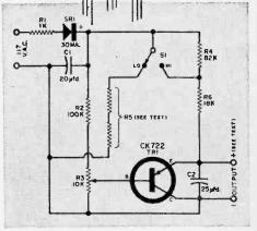
This circuit can be constructed on any type of chassis. Built-in current limiting factor prevents transistor burn out. CI is a 150-volt unit; C2, 25 volts.
