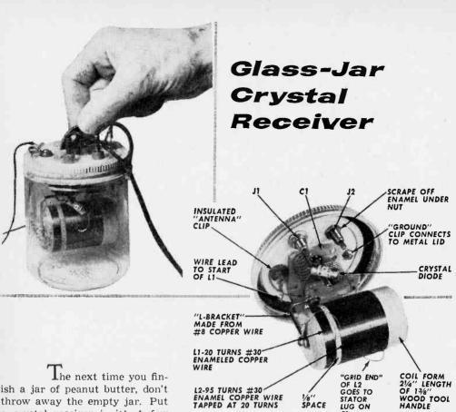
ish a jar of peanut butter, don't throw away the empty jar. Put a crystal receiver in it! A few inexpensive parts will transform that old dispenser of sandwich filling into a dispenser of local radio broadcasts.
