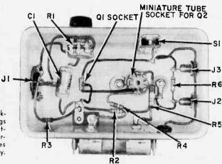
Use a 7-pin or 9-pin sock-3 Use a /-pin of /-pin et to connect to prongs on Q2. Do not solder directly to prongs. After soldering all components and wires in place, check for accuracy.
