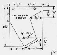
Fig. 1. Caster sides and top should be screwed together. Resultant caster assembly should be rigged.
