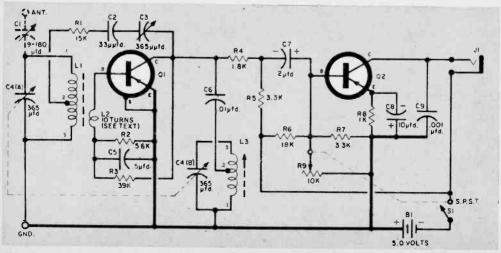
Major parts placement is shown in bottom and rear views of chassis. Phone jack JI should be insulated if metal chassis is used. Note use of two-gang tuning capacitor (C4) and one-gang regeneration control (C3).
