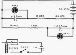
The high-value resistors can be made up from several series-connected resistors of lower value. Since current demands are low, the blinker battery may be a weak unit salvaged from your junk box.
