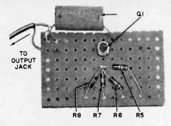
Phenolic board with QI, CI and series resistors ready for installation in cabinet.
