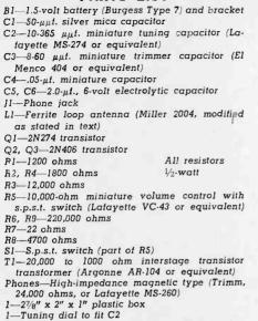
1—3%" o.d. x 5/32" i.d. shouldered fiber washer Misc. screws, washers, nuts, wire, rosin-core solder the other components) can be assembled on the plastic terminal strip before being mounted in the case. Most of the detector can also be preassembled.
