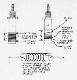
The coil forms used for L1 and L2 are Cambridge Thermionic 3%" ceramic slug-tuned units (Type LS-3).
