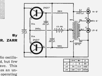
Many transistorized audio oscillators have been built and described, but few can boast a really pure sine wave. This Hartley oscillator circuit generates an undistorted 2-kc. signal suitable for operating bridges, hi-fi testing, filter experiments, etc. The push-pull feature eliminates even harmonics, increases the output to 5 mw., and reduces distortion. A choice of three distinct output impedances and voltages are available.
