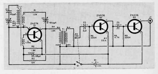
type phono jack, but it could be one of the miniature phone jacks. A thin strip of plastic is mounted on the solder lug of J1 for use as a tie strip for the audio amplifier section.
