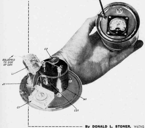
You can squeeze the last drop of power from your transmitter and antenna system with the help of this Citizens Band Class C and D field strength meter. By "peaking-up" the transmitter adjustments for the highest field strength meter reading, you can be sure that your Citizens Band station is working at top efficiency. The antenna length of the transceiver, which is usually critical, can be "trimmed" for the strongest signal.
