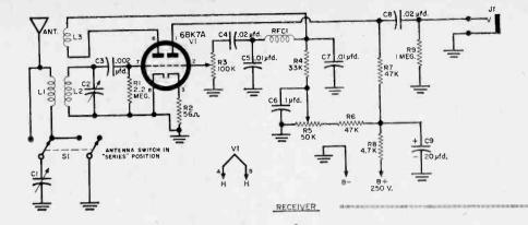
power can be tapped from the amplifier. If a separate power supply is preferred, the one shown works well and decoupling filter C9 and R8 may be omitted in the receiver proper. Neither side of the tube filament is grounded at the receiver chassis. Ground is made at the amplifier or power supply used with the receiver.
