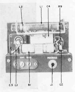
to and as far as possible from L1. Place L3 so that you will have easy access to its adjustment screw. Other than this, parts layout is not critical.
