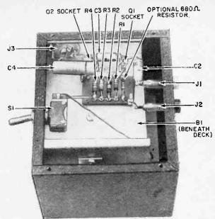
Bottom view of black box with cover removed. The two transistors and the battery are on the other side of the deck. A 680-ohm resistor can be wired across JI and J2 to widen bandwidth, but sensitivity will be lost.
