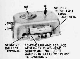
Rear view of completed chas-4 **4** sis. Insulated phone tip jacks are used for J2 and J3. The battery holder terminals are connected so the two cells are in series with the positive end grounded.
