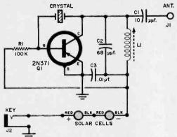
**Carefully check** the solar cell connections with the diagram after wiring the transmitter.
