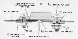
Prior to mounting power transistor Q2, cement two 1/2" fiber washers to the chassis as shown. If done correctly, the mounting screws and lugs of Q2 will be insulated from chassis ground.
