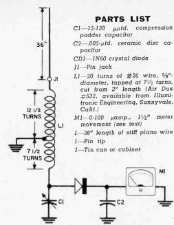
C1. Connect the banded end of CD1 to the plus terminal of M1. Then connect the .005-µfd. capacitor (C2) across the meter terminals, and wire last connections.
