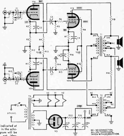
Voltages indicated at VI's socket in the schematic diagram will be close but not identical to those of V2.
