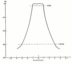
Fig. 1. Bandwidth of 2 kc. at 6 db expands slowly to 6 kc. at 60 db. Steep skirt characteristic makes it possible to separate closely spaced stations.
