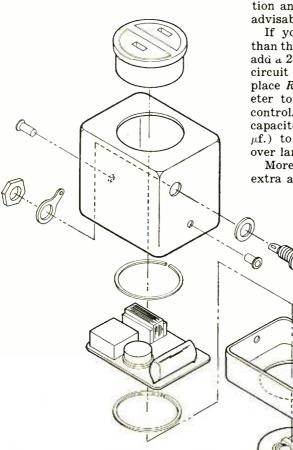
Fig. 4. Octal base shield houses all components. If desired, silicon rubber can be poured into the case to keep the printed circuit board in place. jack. Screws or rivets can be used to fasten the two parts of the case.
