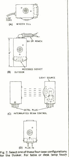
for the Dusker. For table or desk lamp touch control applications, the outer casing is not used.
