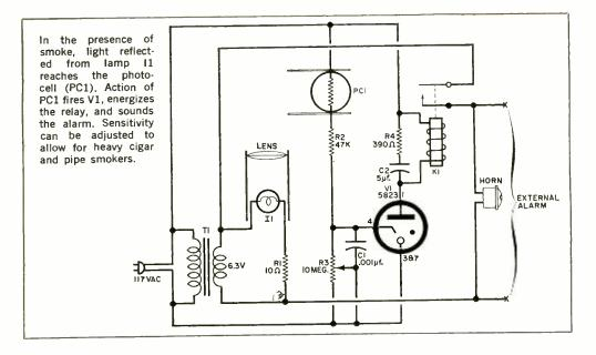
on the ceiling and build down. A room almost filled with smoke may have an area close to the floor that will allow a safe crawl space for escape. By the same token, if a smoke alarm were located near the ceiling, it would sound an alert long before a dangerous concentration of smoke accumulated. Here's a smoke detector you can construct complete with a built-in alarm for about \$10.00.
