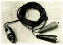
Simple gadget for turning over engine consists of two clip leads connected to normally-open push-button switch. Leads are connected to starter control terminals of starter solenoid.
