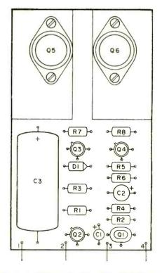
Fig. 2. Carefully locate and solder all of the components onto the printed circuit board as shown.
