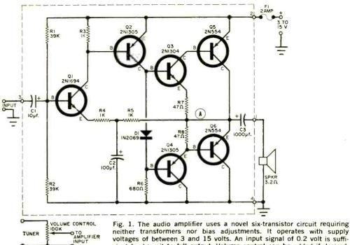
neither transformers nor bias adjustments. It operates with supply voltages of between 3 and 15 volts. An input signal of 0.2 volt is sufficient to drive it to full output. Volume control can be added if desired.
