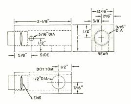
Light-source barrel is made from a block of wood. Size of lens opening can be varied to accommodate your lens. Use a cardboard tube as an extension.
