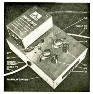
Fig. 2. Large chassis allows plenty of room for mounting the power pack. Use mounting kit for Q2 and Q4, and be sure to mount Q1 and Q3 on sockets. Cables at sides of chassis go to speed controllers.
