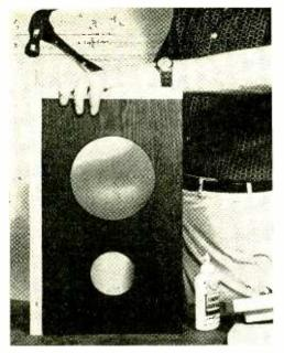
Nail side to bottom and front of the enclosure. Good fit and a liberal use of glue are important.
