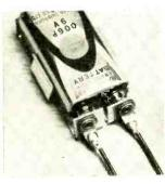
grip on the battery. When inserting the battery in the holder, be careful not to short the terminals against the frame of Art Trauffer the holder.
