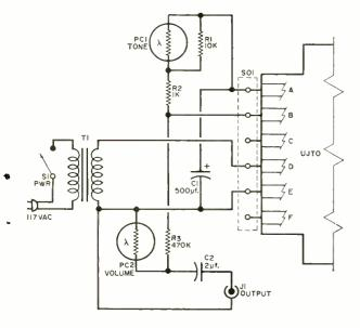
Fig. 2. Diagram of power supply and timing network shows wiring connections to UJTO plug-in module.
