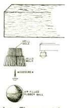
place on a side of the base. Then cement the rubber ball in place inside the mold. If the sides of the base are too thin to hold the screws, you can build up the cabinet with a block of wood.  $-Harry\ Goldman$
