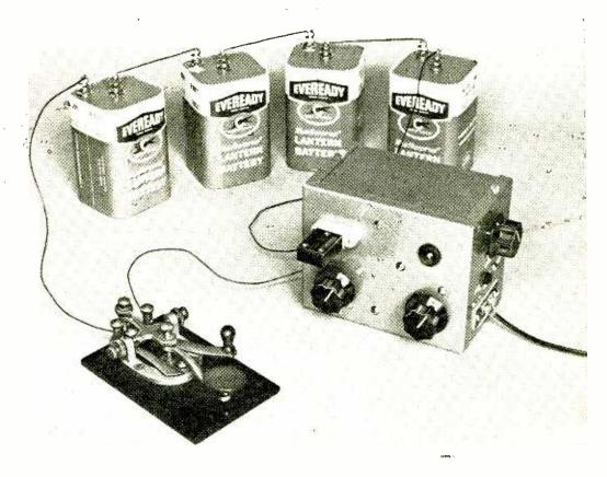
How It Works. Resistors R1 and R2 form a voltage divider to provide a small amount of forward bias for the base of Q1. Current flows in the emitter-collector circuit and through L1 when the key is closed. The application of power causes the crystal to vibrate at its resonant frequency and varies the emitter bias at an r.f. rate. If L1 and C1 are now resonated near the crystal frequency and Q1 amplifies sufficiently to overcome circuit losses, the stage will go into sustained oscillation.
