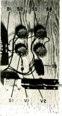
Fig. 3. Align barrel bolt with solenoid to obtain smooth action without bolt rotation. Battery and switches can be mounted in any convenient position.
