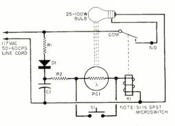
Fig. 7. This low-cost touch control circuit can easily be wired to any desk or table lamp by adding a microswitch across PC1. To turn on lamp, touch S1 gently. To turn off lamp, bring hand near PC1, shielding it from light. For proper operation, PC1 must be shielded from other strong light sources.
