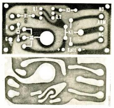
bias circuit) and low-resistance types are placed between terminals I and Gwith a jumper from terminals I and B, as shown in Fig. 2. Actually, the resistive devices are made to function like a voltage source, since terminal B has sufficient voltage of proper polarity to forward-bias the transistors.
