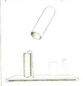
to bend the lead parallel to the component and mount the c o m p o n e n t standing erect. A real spaces a v e r—b u t that long lead is a potential troublemaker! One neat way of preventing a short is to cov-
