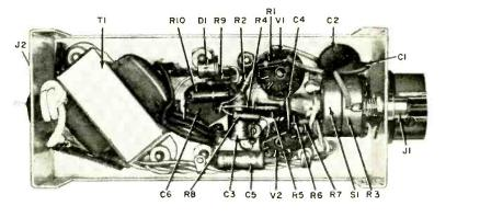
Locate T1 as close to the back of box as possible; note location of tube sockets, and mounting hole for C6. Jack J2 (for strobe connection) is hidden at rear of box.
