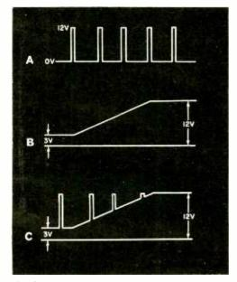
Fig. 4. Pulses rise to maximum as soon as power is turned on (a), providing immediate train start. Crawl knob adjusts pulse width for varying train loads and desired crawl speeds. Throttle adjusts d.c. at emitter of Q8 (b) to run train at desired speeds. With throttle turned down (c), pulses appear prominently, then fade away as d.c. is turned up.
