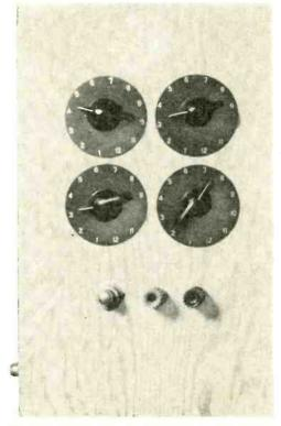
External battery can be connected to the banana jacks to overcome a weak internal battery. However, the lock cannot be opened without the combination.
