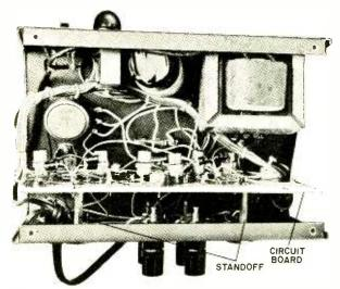
With bottom plate removed, laced wiring harness can be tucked away to one side during repair or maintenance of the unit. The component circuit board is supported with metallic or insulated standoffs. To install the line cord, thread free end through grommet at rear of cabinet. Separate ends of cord back 12 inches and tie into a knot to take up any strain on cord.
