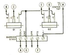
Fig. 4. Wiring details of transistors and barrier strip connections for positive ground ignition system. Terminal marked A-- connects to ignition switch. the ambient temperature under the hood, and, besides, the metal box acts as a heat sink.
