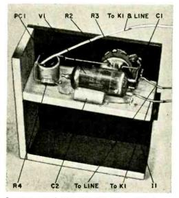
Remove unused tube pins and use a drop of cement to hold the tube in place. Lamp 11 is inside the barrel. A cardboard tube holds the photocell (PC1).
