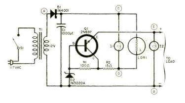
An overload indicator quickly alerts you to operating conditions. Here's what happens. Under normal load conditions the indicator light 11, protruding through the top of the cabinet, is off and the output voltage is correct. Under excessive load conditions, 11 glows and the output voltage is down sharply. When you remove the excess load, 11 will stop glowing and the output voltage will come up to normal almost instantly.
