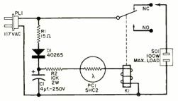
Fig. 1. For dusk-to-dawn control, connect load circuit to the NC relay contacts; for photocell relay application, connect load to the NO contacts.
