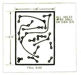
Fig. 2. Printed circuit board is shown actual size to help you make your own. However, almost any suitable chassis or breadboard arrangement can be used.
