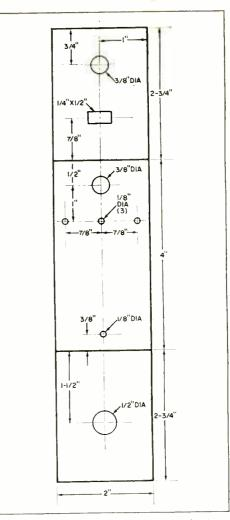
Drill holes in the outer portion of the aluminum box as shown. The size of the rectangular opening can be modified to accommodate any s.p.s.t. switch.
