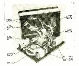
Parts layout and box dimensions are not critical. Paint the outside fireman's red and use large bold letters. Battery mounting brackets are optional.
