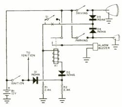
Should you forget to turn off your lights when you turn off the ignition switch, the alarm will sound-unless you install a disabling switch (S1).
