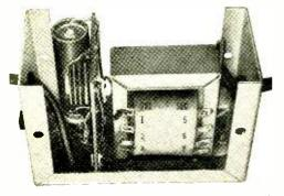
Preassemble the circuit board and install after S1, 11, and T1 (in that order) are mounted. Connect all leads and check the circuit before closing box.
