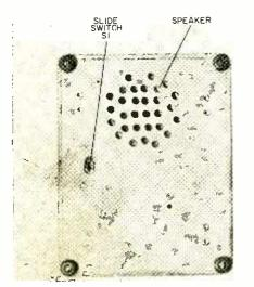
Speaker and "hidden switch" are mounted on back of box. Better chain the box in place lest your victim heave it out the window when the alarm sounds off.
