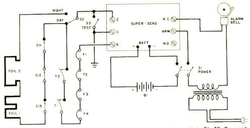
Fig. 5. Fire alarm circuit has fusible links F1 to F4, and thermostatic contacts T1, T2. Door and window contacts C1 to C3 and foil patterns make up burglar alarm. Place sensors in strategic locations.
