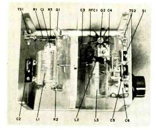
R2—5600-ohm,  $\frac{1}{2}$ -watt resistor R3—150-ohm,  $\frac{1}{2}$ -watt resistor RFC1—2.5-mh. r.f. choke RFC1-2.5-mn.r.j.cnore S1-S.p.s.t. slide switch TS1, TS2-Two-screw terminal strip REV-Telegraph key XTAL-3.5- to 3.8-mc. quartz transmitting crystal 1-5" x 4" x 3" Minibox (Bud CU-2105-A, or equivalent)
