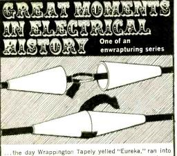
his work shop, slid a cone-shaped Mueller flexible clip insulator over each end of two wires, before splicing, then slid the insulators back together just before wrapping with tape. The high dielectric insulators not only improved insulation at the splice, but made it very easy to remove and replace the covering for inspection of the joint. What new things have you found to do, with Mueller Clips and Insulators? At Jobbers everywhere.
