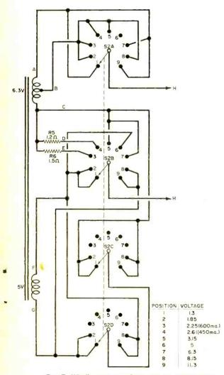
Fig. 7. Windings are made to aid or oppose each other to obtain six more filament voltage levels.
