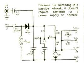
cial attention. One of these is silicon diode D1, which must be suitable for detector operation up through 30 mc. Capacitor C3 must be of the low-leakage variety (Mylar-type) and must have a capacity of at least 1.0  $\mu$ f. The voltage rating of C3 is not important.
