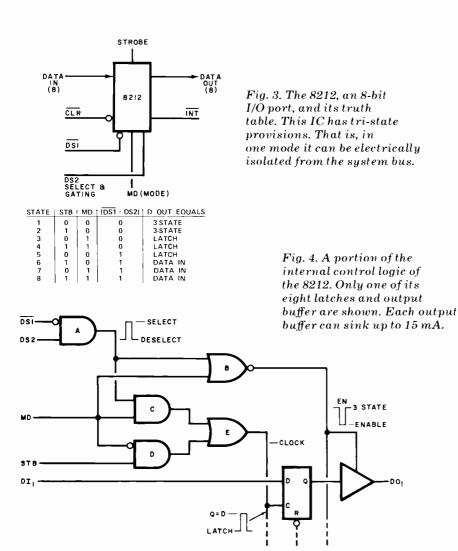
through buffer, to name just a few of its applications. This high-speed Schottky TTL device includes eight data latches and output buffers that can be tri-stated (switched to high impedance). Each buffer can sink up to 15 mA.
