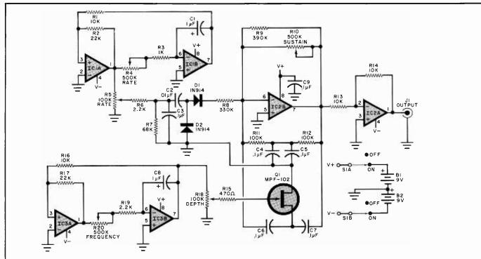
Fig. 1. The circuit around IC2B is the tone-generating section. The five controls react with each other to provide various sound effects.
