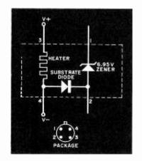
Fig. 4. The LM199 temperaturestabilized zener diode uses an on-chip heater.
