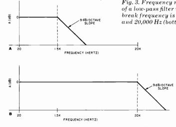
Fig. 3. Frequency response of a low-pass filter when its break frequency is 1500 Hz (top) and 20,000 Hz (bottom).
