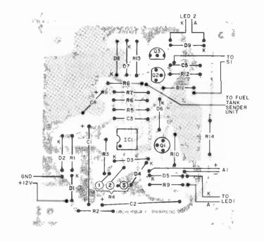
Fig. 3. Actual-size etching and drilling guide is shown at left. Component placement guide is above.
