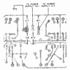
Fig. 11. Special wiring of the main pc board for use with an ac power supply.
