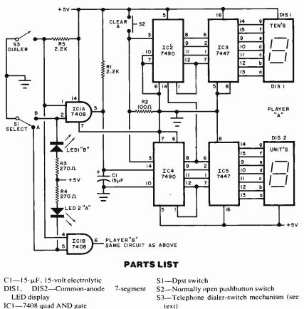
text) Misc.—Duplicate circuit for player B; regulated 5-volt, 1-ampere dc power supply; perforated or printed-circuit board and hardware; suitable enclosure; sockets for ICs (optional); machine hardware; hookup wire; solder; dry-transfer lettering kit; etc.
