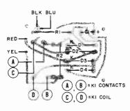
Fig. 2. Actual-size etching and drilling guide, right; component placement above.
