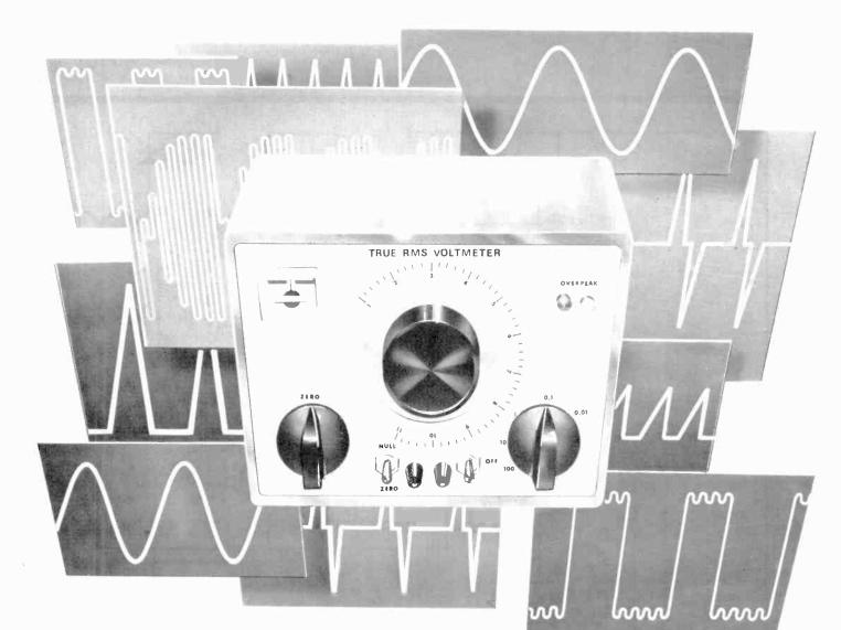
**E** VENTUALLY, most serious electronics experimenters find a need to measure the power content of an odd-shaped waveform. This might occur in measuring the output of a class-C amplifier, audio, video or noise signals; power supply inverter waveforms; or just plain power supply ripple.
