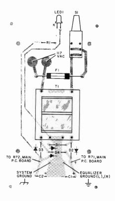
Fig. 9. Component placement for the ac power supply.
