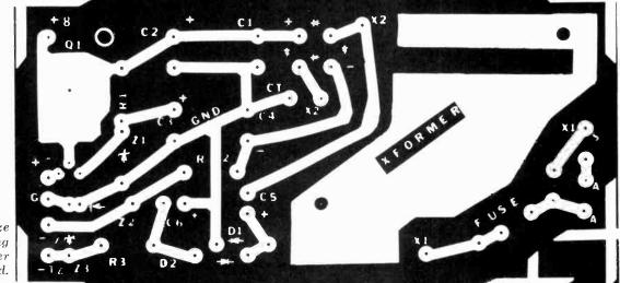
Fig. 9. Actual-size etching and drilling guide for the power supply board.
