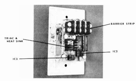
Fig. 4. Photo of the back of the Smart Switch shows how pc board is mounted on a standard plastic cover plate.
