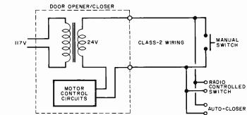
Fig. 2. Class 2 wiring of a typical garage door opener.
