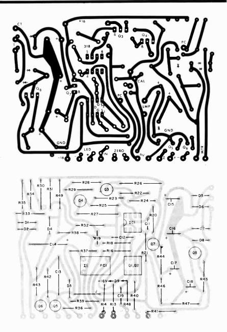
Fig. 2. Actual-size foil pattern for main pc board is at top, component installation immediately above.
