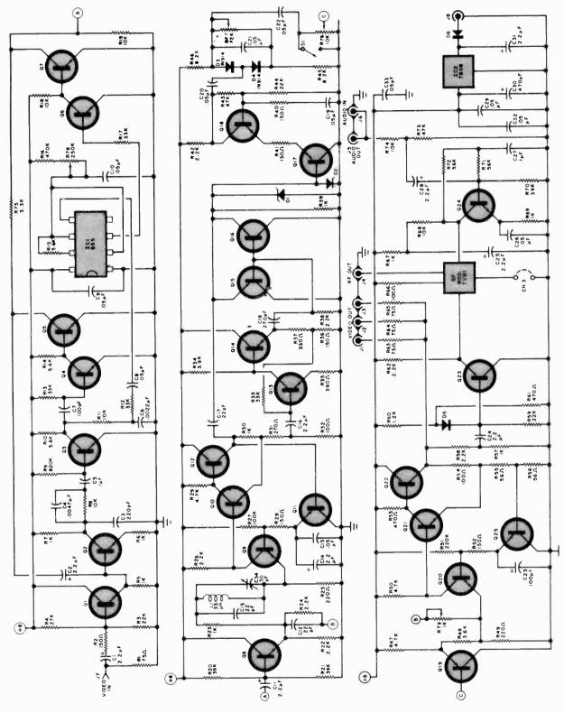
C1,C2,C11,C14,C16,C24,C25,C28,C31-2.2- $\mu$ F, 50-volt electrolytic capacitor C3-220-pF, 50-volt disc capacitor C4-0.0047- $\mu$ F, 100-volt Mylar capacitor C5,C27-0.1- $\mu$ F, disc capacitor C6-0.0022- $\mu$ F Mylar capacitor C7-100-pF disc capacitor
