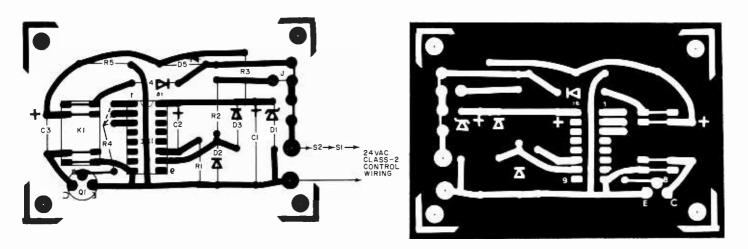
Fig. 3. Etching and drilling and parts placement guides for a suitable pc board.
