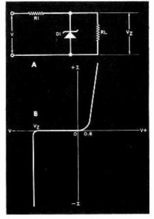
Fig. 1. Zener-diode reference supply. The circuit is shown at A, while the characteristic curve is below at B. The fact that the zener voltage is dependent on temperature must be kept in mind in circuit design.
