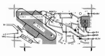
Fig. 10. Component placement for the power supply board shown above.
