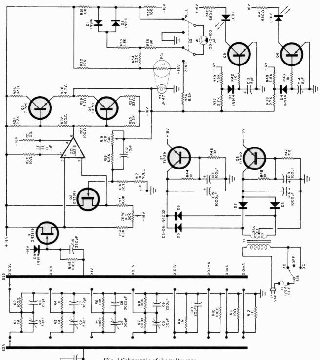
Fig. 1 Schematic of the voltmeter. The amplified input signal illuminates I1, which causes the resistance of PC1 to change. This brings about imbalance in the bridge circuit and meter goes off null.
