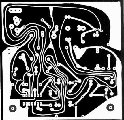
Fig. 3. Actual-size etching and drilling guide for a printed-circuit board for the controller is shown above. Component layout is at top. Note that there are sevral different options regarding components and construction, as outlined in text and Parts List.
