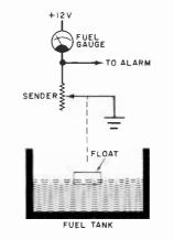
Fig. 1. Typical fuel-gauge circuit.
