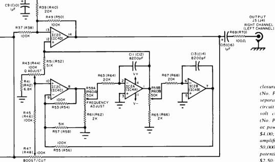
Fig. 2. The complete circuit for a two-channel equalizer. Part numbers not in parentheses are for right channel of a stereo system, others are for left channel. For components with asterisks, see Figs. 3 and 4.
