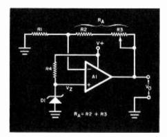
Fig. 3. By adjusting the gain of the op amp (by varying R3), the output voltage can be trimmed to a precise value.
