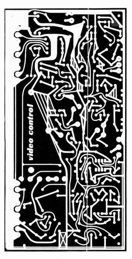
Fig. 7A. Actual-size etching and drilling guide for enhancer project.
