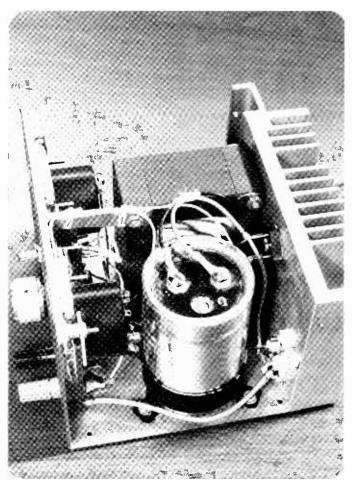
Fig. 5. Interior view of the author's prototype. Heat sink must limit IC temperature to 75°C above ambient.
