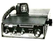
a.n.l.; switchable noise blanker; squelch; external speaker jack; S/RF meter; comes with PTT mike, d.c. power cable, mobile mounting bracket, mike clip; 11.5-14.5 V d.c. switchable negative/positive ground; 101/4" D × 73/4" W × 25%" H ............. \$249.00
