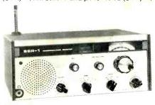
synthesized; selectable sidebands; preselector, clarifier; built-in speaker; S meter; headphone jack; telescoping antenna; coarse and fine tuning controls; built-in 117/234 V a.c. power supply; automatically switches to internal battery pack if a.c. power fails; on-off pushbutton for reduced current drain on d.c. operation; 5¾" H × 13" W × 10½" D.
