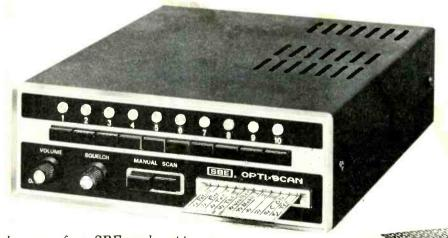
This 10-channel scanner from SBE can be set to any ten of some 16,000 channels in the 30-50 Mhz, 150-170 MHz, and 49-510 MHz bands. Channels to be scanned are selected with a do-it-yourself programmed card. Other channels can be scanned by inserting a different card into receptacle on front panel.
