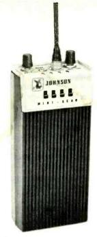
E.F. Johnson's four-channel portable scanning receiver.
