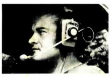
headset combines dynamic receiver with ceramic boom mike; talk-switch, and FET battery-powered amplifier (separate long-life battery); adjustable mike boom rotates 310 degrees to move out of way when not transmitting; talk switch; unterminated headset cord so jacks can be installed to match rig.
