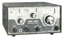
supplied by manufacturer); duaf-conversion; direct frequency readout; three built-in bandwidths, corresponding to mode of reception; 400 Hz for CW, 2400 Hz for SSB, and 4800 Hz for AM; built-in speaker; notch filter; 100-kHz calibrator and i.f.-type noise blanker available as optional extras; S meter;
