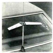
aluminum construction; mounts on trunk without cutting or drilling; overall height 16-in plus 8-in telescoping for fine tuning; capacitive top-loading and a grooved-core coil provide performance equal to 42-48-in center and base-loaded antennas .. \$39.95
