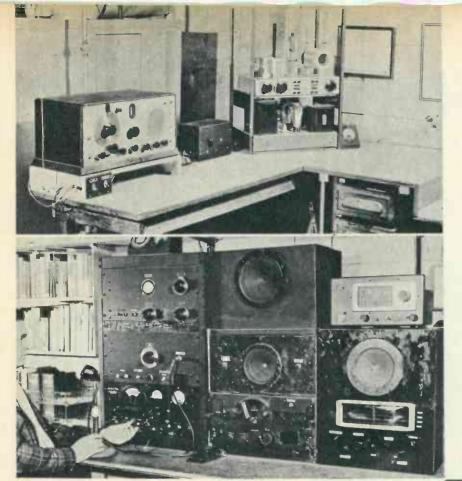
Receiver of this snug, modest ham shack is raised 3 inches above table, and the space beneath it provides convenient storage. Switches on dark panel, lower left, control transmitter. Latter, at right, is built up of uniform-sized aluminum chassis, supported on an open frame of angle iron. Parts are readily accessible.
