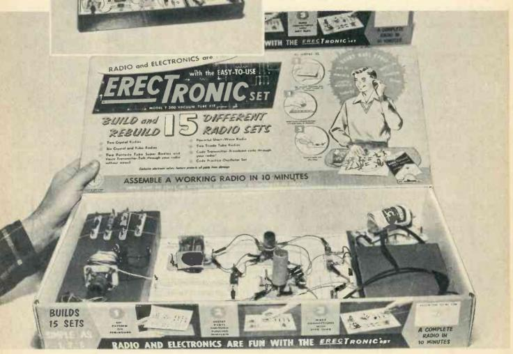
SSEMBLE AND WIRE a complete one-tube radio receiver that really works . . . in ten minutes. A codepractice oscillator or half a dozen other practical electronic units ... in four to seven minutes. And all without tools, absolutely none, not even a screwdriver.
