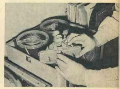
The cut end of the tape is pulled past the playback head slowly, to spot the next cutting point; work carefully.
