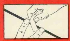
Smooth out the air bubbles after applying cellulose tape; do not use metal.
