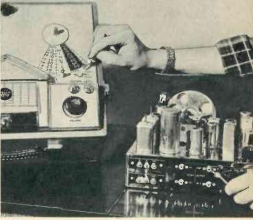
To record directly from turntable to tape, phono cable on turntable is connected to a low gain input on tape recorder.
