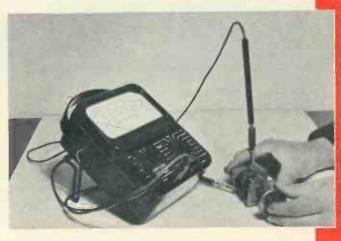
NOISY RECEIVER? If radio receiver is unaccountably noisy when dial is turned, check variable tuning capacitor. Remove from chassis, connect circuit tester, turn shaft, test for short as shown in photo.
