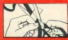
After tape is joined properly, trim and undercut it slightly to avoid sticking.
