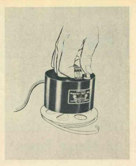
These bulk tape erasers will erase even the most powerful signals from a recorded tape in a few moments; these devices clean the entire tape at once.
