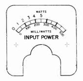
Fig. 6—Meter is calibrated in milliamperes, but if you paste this scale over its scale, you'll be able to read the rig's input power directly.
