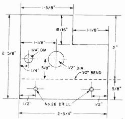
Fig. 2—Shield plate. Nuvistor socket is mounted in ½-in.-dia. hole; resistor R3 fits in grommet in ¼-in.-dia. hole. Bend the bottom toward you.
