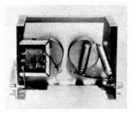
Parts are mounted in main section of  $3 \times 4 \times 5$ in. Minibox. R1 is mounted at left, R2 is mounted at right. Output jack is at left, input jack is at right.
