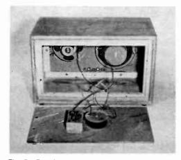
Fig. 7—Completed cabinet ready for stuffing with fiberglass blocks. Mount choke with 2½-in.-long machine screw. Cement electrolytics with epoxy.
