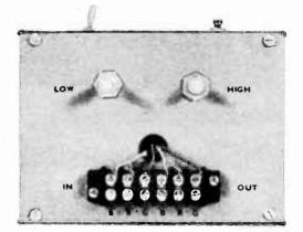
DRY TRANSFER lettering readily identifies parts and terminal lettering on rear of meter case. S1 is at top left: S2 is at right.
