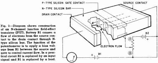
of an N-channel junction field-effect transistor (JFET). Battery B1 causes a flow of electrons from the source contact to the drain contact through Ntype silicon bar. The function of the potentiometer is to apply a bias voltage from B2 between the source and gate to control current flow. In a practical circuit B2 is replaced by an input signal and B1 is replaced by a load.
