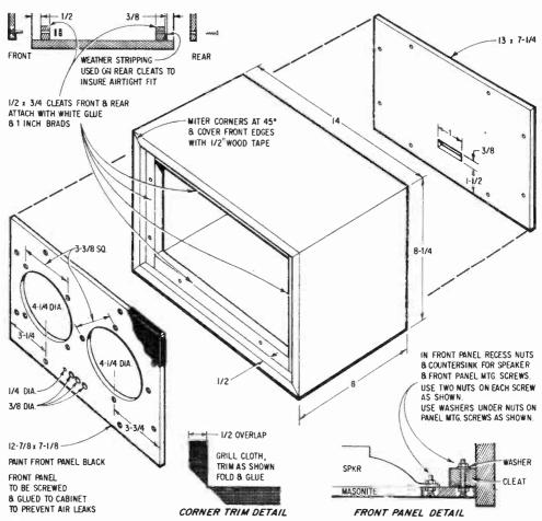
NOTES - MATERIAL: CABINET-1/2 BIRCH PLYWOOD; FRONT & REAR PANELS-1/4 MASONITE - ALL DIMENSIONS ARE IN INCHES
