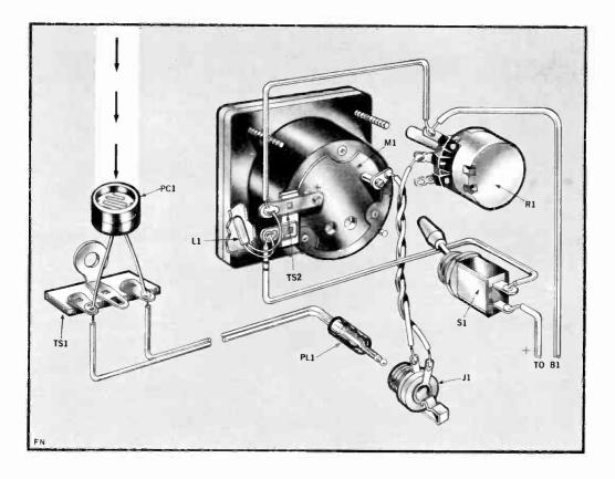
or metal enclosure. You can use a  $\frac{1}{2}$ in.-dia. hole and silicone adhesive. Glue or fasten two-lug terminal strip TS1 adjacent to PC1's mounting hole.
