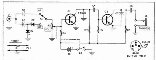
Fig. 2—When S1 is set to AF, audio signals go via C1, S1 and R2 to base of input transistor Q1. To trace RF signals, set S1 to RF. Audio output of D1,D2 detector circuit then is fed via R2 to Q1. R1 is used in probe to prevent the tracer from loading the circuit to which it is connected. First try probe without resistor. If it loads down circuit, use up to a 1-meg. resistor in the probe.
