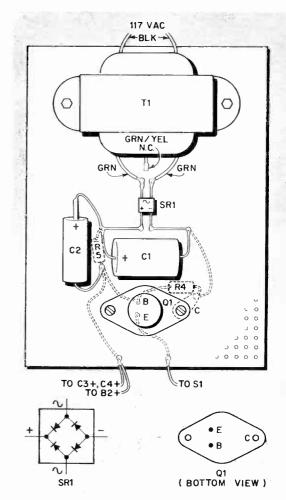
tie points. Do not substitute a different transistor for the type specified.
