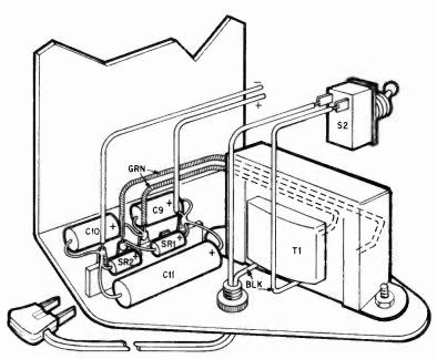
Fig. 3—Power supply is a simple affair that can be built on side of U-section of cabinet. Mount diodes and capacitors on 6-lug terminal strip and make sure ground lug is not used for a the point. AC power switch S2 gets mounted in the main section of meter cabinet.
