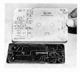
To mount circuit-board parts, you first stick Conar's overlay on reverse side of board. Parts leads are pushed through holes in the template.
