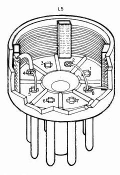
Fig. 4—Pictorial of 20-meter coil. The three diagrams at the right of the schematic in Fig. 2 show pin connections of coils and the jumpers.
