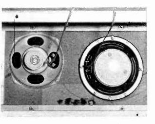
Fig. 4—Rear of front panel after being attached to cabinet. Tweeter is at the left, woofer is at right. Port holes were plugged during tuning.
