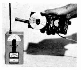
Fig. 6—Easiest way to calibrate the FSM is with α GDO. But be careful you don't overload the FSM. If the FSM's meter pins, move GDO farther away.
