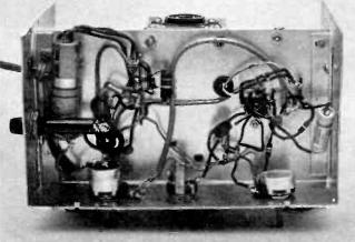
Fig. 1—There is very little under the chassis; therefore, you should have no problems fitting everything in place. Keep all leads to and around V1 short and direct. Note how the chassis is installed in the main section of the Minibox with home-brew brackets. Our chassis was installed 2<sup>1</sup>/<sub>4</sub> in. above the bottom of the cabinet. Heavy wire from volume control R4 to pin 7 on V1 is shielded.
