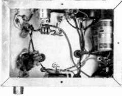
Fig. 1—Underside of transmitter. To layout your chassis, take dimensions from pictorial and multiply by about 2. Arrangement of parts in RF section of transmitter is important; therefore, duplicate our layout as closely as possible. The lugs at the left side of switch S2 are S2A.
