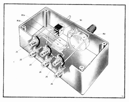
LAYOUT of synthesizer can be anything you want. Our arrangement makes for neat project, however. Ventilation holes are needed between jacks.
