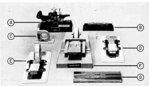
Tapes splicers come in all shapes and sizes. Represented here are (A) Alonge professional splicer, a heavy-duty, relatively expensive unit; (B) Low-cost editing block equipped with hold-down arms to keep tape ends in place; (C) Gibson Girl at its simplest—SP-4 block and cutter; (D) Gibson Girl TS-4J, a stripped-down version of (E) Gibson Girl TS-4S, with splicing tape holder; (F) TS-8D, fanciest of the Gibson Girl sisters; (G) Robins Cut-N-Splice editing block.
