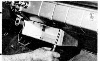
Adjustable wirewound resistor and fuse holder should be mounted on back of chassis. Because resistor will be difficult to get to after unit is mounted, measure the dropped voltage with recorder operating before installing chassis under the dash. Fuse should be a .15 A type 3AG.
