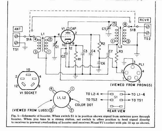
not look exactly the same even though they have the same part number. The windings may be close together or separated slightly. It doesn't matter which design you get as long as the part number is correct. You identify the coil lugs with respect to the color dot on the form as shown in Fig. 5. One final reminder—keep all leads short.
