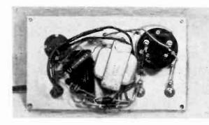
All parts mount on rear of panel. Rectifier diodes are at bottom. Filter capacitors are at left between voltage-adjust pot and the transformer.
