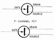
Fig. 5—Standard symbols for FETs. Arrow points toward vertical bar in N-channel FET. Arrow points away from vertical bar in a P-channel FET.
