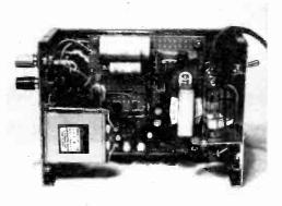
Fig. 6—Completed Tele-Spy. Final assembly results in tight quarters. To avoid burning wires when soldering, follow assembly steps in the text.
