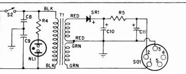
Fig. 6—Power supply schematic and layout. Line cord and socket SO1 are mounted at left. Rectifier SR1 and R5 (we paralleled three 22,000ohm,  $\frac{1}{2}$ -watt resistors) are mounted on terminal strip above electrolytics. Power switch and neon lamp are at the right side of the cabinet.
