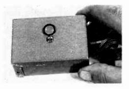
ALUMINUM box houses photocell and terminal strip. Turn photocell away from enlarger light to protect it when the meter is not used.
