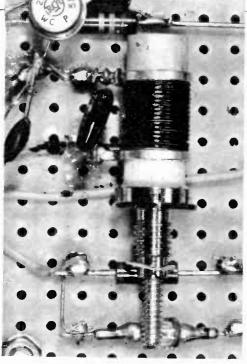
Be sure D1 is under L1's slug against the board, not up in the air. If L1 is wound correctly its terminals should line up with two flea clips spaced two holes apart. Solder L1 directly to clips.
