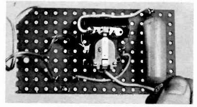
tronics is, say, 12 V the resistor will have to drop the extra 6 V. To compute the resistor's value, use Ohm's Law: R = E/I. E is the voltage to be dropped (6 V). I is the current in amperes drawn by the relay (0.018A). Therefore R = 6/0.018, which equals 330 ohms. A 1-watt resistor will handle the power.
