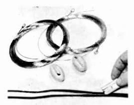
Fig. 3—This is all the material required for antenna: 150 ft. No. 14-18 copper wire and porcelain strain insulators. Slit 2 ft. of twinlead. ter's dimensions are enclosed in parentheses).
