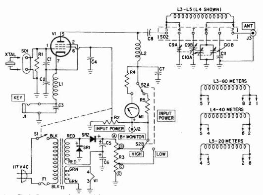
Fig. 2—Transmitter schematic. S2 determines input power. When it's set to "high" (shown), high B+ is supplied to V1 from tap "B" on R3. When S2 is set to "low," lower B+ is supplied to V1 from tap "C." R2, which establishes V1's screen voltage, is used to vary the input power continuously in both ranges. 80-meter coil, L3, is 33 turns. 40-meter coil, L4, is  $17\frac{1}{2}$  turns. 20-meter coil, L5, is  $8\frac{1}{2}$  turns. (See Fig. 4.)
