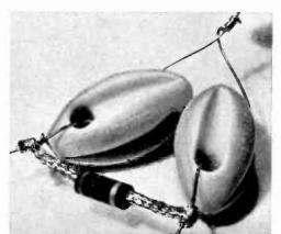
Fig. 5—When legs are longer than signal's wavelength, lobes (pickup pattern) overlap, add signals along axis, Re-STATION sistor absorbs energy after it has traveled through antenna to prevent it from reflecting back and changing pattern of the lobes.
