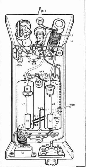
The underside of the cabinet is not particularly crowded. The two filter capacitors (C3,C4) take up most of the space. They are supported by two terminal strips which they fit between. Rectifiers SR1 and SR2 and current-limiting resistors R2 and R3 go on top of the capacitors. Be sure to use spaghetti on bare leads in the power supply. Note the location of the ground lug on the coil form.
