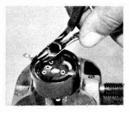
To add off position to R2, cut wire where it connects to left lug. Then remove a few turns so wiper doesn't touch wire when turned all way to left.
