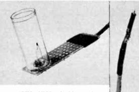
PILL VIAL shields outdoor thermistor from wind, rain. Heat-shrink tubing covers wires of indoor thermistor.
