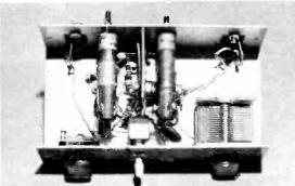
Fig. 4—Top view of completed booster. Although the coils may not look exactly alike, they're electrically identical since the part numbers are the same. Mount L1 (left) so its color dot faces down. Mount L2 (right) so its color dot faces to the right. If you mount coils some other way, improper placement of leads to them may cause oscillation. Be sure to remove the trimmer capacitor mounted on C5's side.
