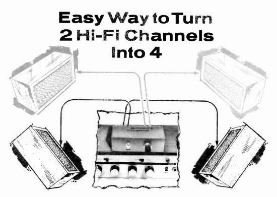
MAGIC BOX—Our easily-built 4-channel synthesizer sits on amplifier, as here, drives front speakers (black) plus two new speakers in rear (color).
