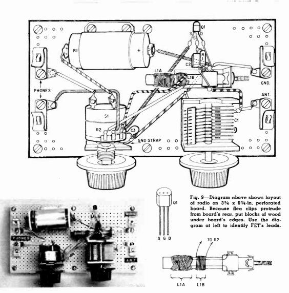
Fig. 8—Our radio was breadboarded on piece of perforated board to make it easy to experiment with circuit. Receiver can be put in small box.
