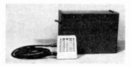
Fig. 1—Tele-Spy control box doesn't have to be near phone; it can be connected to line anywhere. Mike can be hidden as amplifier's gain is high.
