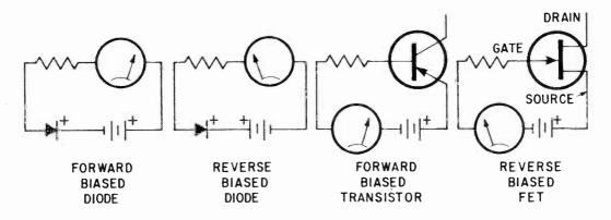
Fig. 1—Heavy current flows in forward-biased diode, meaning circuit resistance is low. Reverse-biased diode current is low so circuit resistance is high. Large current in transistor's forward-biased emitter-base junction means low impedance. Reverse-biased gate-source junction of FET means high input impedance.
