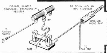
Mount resistor to drop voltage to 6 V on back of chassis. As recorder draws 100 ma, value should be 60 ohms. Use 100-ohm adjustable type and adjust slider with recorder operating to set voltage. Positive lead goes to the sleeve in plug.
