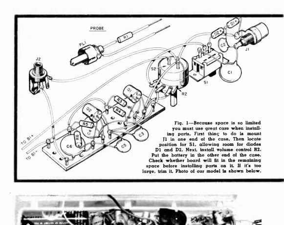
be made with a single-edge razor blade. Cut the front of the case's cover so it fits snugly around J1. Position J2 in the cover in such a way that it will not touch components on the board when the cover is closed.
