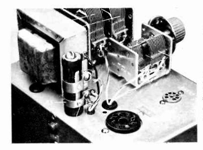
Fig. 3-Closeup of top of chassis shows mounting of B+ voltage-divider power resistor R3. Mount R3 with  $\alpha$  <sup>1</sup>/<sub>4</sub>-20 x 2<sup>1</sup>/<sub>2</sub>-in. screw. Slider contact "C" is home brew since only one slider is supplied. Make a cover of perforated aluminum to fit over R3 so you don't touch it. If you did you'd get a nasty shock and burn. Both sections of C10 (top) are connected in parallel. C9A is the smaller section of C9.
