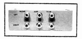
HOOKUP on back of synthesizer. Amplifier plugs in at center, speakers on the outside.
