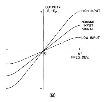
Figure 13. Basic Circuit of a Balanced Discriminator: the output characteristic in (B) shows the dependence of the output on the input signal amplitude
