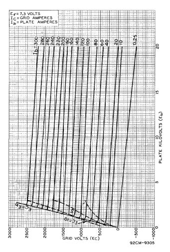
Figure 34. Constant-Current Curves for 6949 Shielded-Grid Beam Triode
