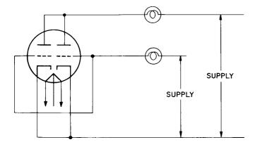
Figure 9. Two-Lamp Twin-Triode Aging Circuit
