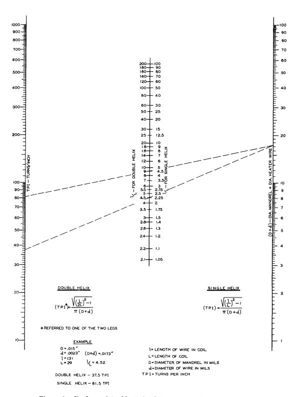
Figure 3. Single- and Double-Helical Heaters: winding characteristics
