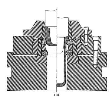
Figure 9. Extruding Dies: (A) backward, (B) forward
