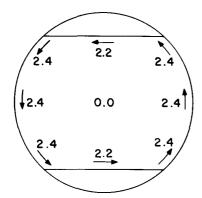
MISREGISTER (IN MILS) DUE TO AN AXIAL FIELD OF O.22 GAUSS-TUBE FACING NORTH
