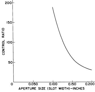
Figure 42. Control Ratio vs. Aperture (Slot) Size
