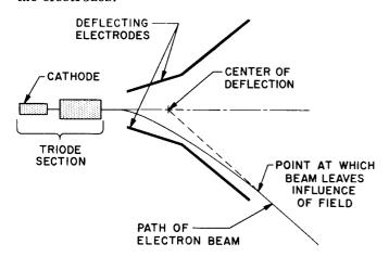
Figure 3. Center of Deflection of a Pair of Deflecting Electrodes
