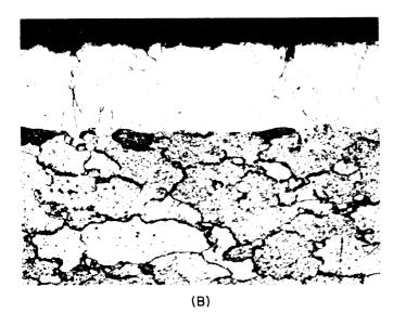
Figure 4. Cross Sections of Carburized Thoriated-Tungsten Filaments: (A) preferred type of laminar carbide (272X); (B) undesirable massive type of carbide (272X)
