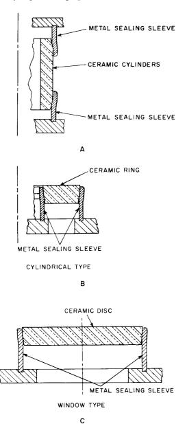
Figure 36. Typical Compression-Seal Configurations
