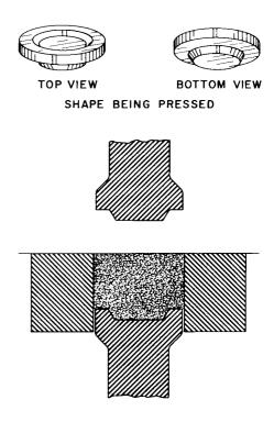
Figure 4. Die for Forming Disk With Shadow Grooves
