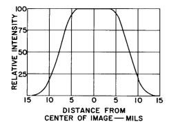
Figure 8. Light Distribution Across an Aperture Image
