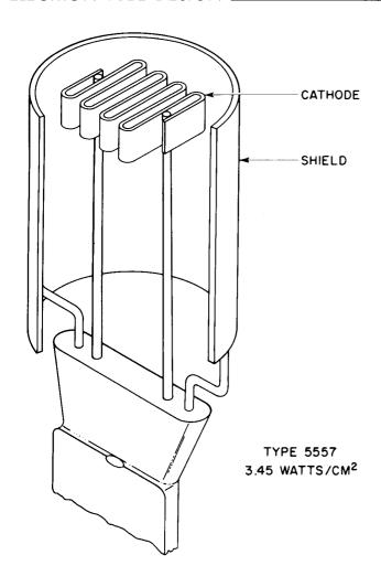
Figure 17. Directly Heated Cathode Structure of Type 5557
