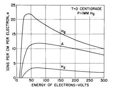
Figure 6. Probability of Ionization
