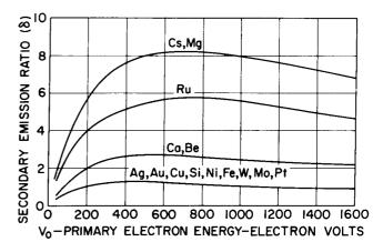
Figure 18. Secondary-Emission Yield vs. Primary-Electron Energy (The curves are approximate and are intended to show only the general behavior and magnitude of the yield of the metals listed)
