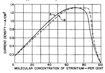
Figure 2. Dependence of Emission on Proportions of Barium Oxide and Strontium Oxide. Curve A: carbonate content before heat treatment; curve B, oxide content after activation 14
