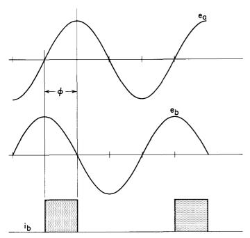
Figure 16. Principle of Operation of Phase-Variation Detection of Frequency-Modulated Signals. Plate current flows only when both  $e_a$  and  $e_b$  are positive. Phase angle between signals  $e_a$  and  $e_b$  is 90 degrees at center signal frequency, but changes as frequency is modulated.
