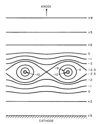
Figure 17. Potential Field of Triode with Grid at Space Potential (V negative)
