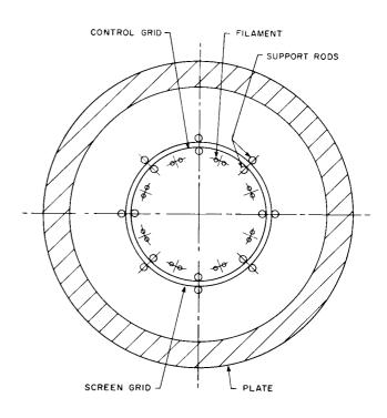
Figure 23. "Squirrel-Cage" Grid Construction Used in Conventional Large-Power Tetrodes
