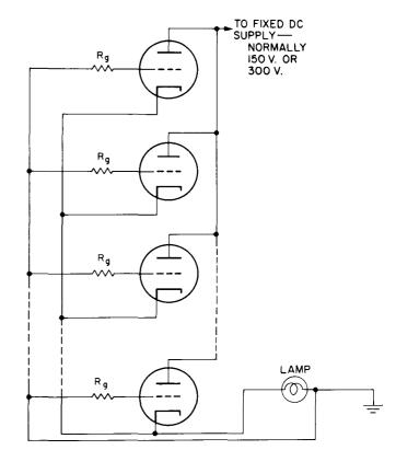
Figure 15. Ten-Tube Stabilization Circuit Showing Lamp Bias
