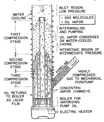
Figure 11. VMF Type Oil Pump
