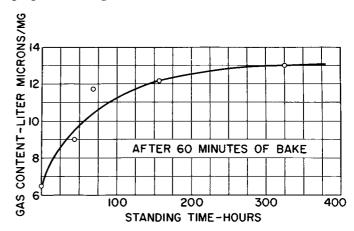
Figure 2. Gas Content of Graphite Coating on Standing
