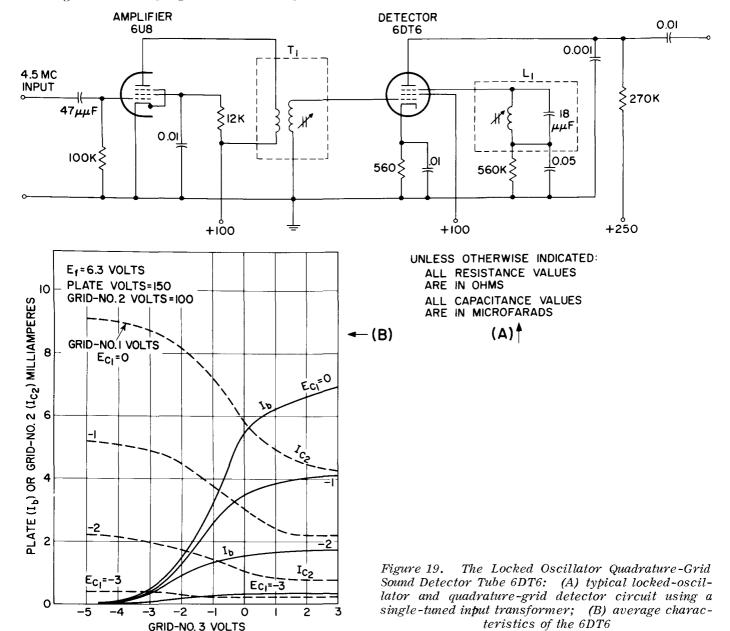
the space current through grid No. 2 becomes large enough to produce a virtual cathode between grids No. 2 and No. 3.
