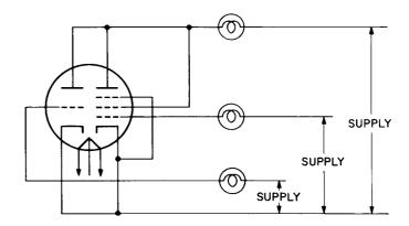
Figure 11. Three-Lamp Triode-Pentode Aging Circuit
