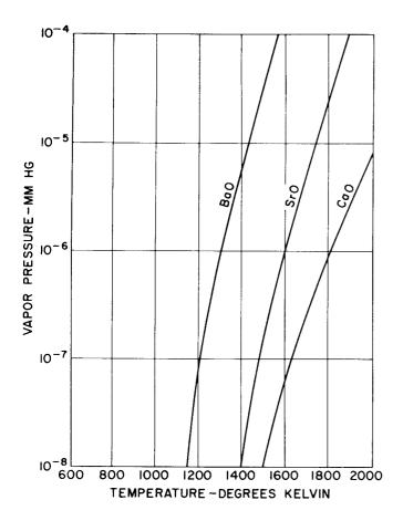
Figure 14. Vapor Pressure of Alkaline-Earth Oxides 51
