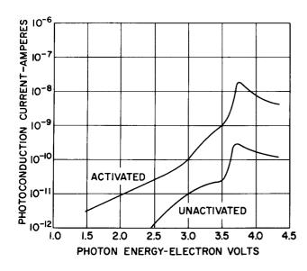
Figure 16. The Photoconduction Current vs. Photon Energy for Activated and Unactivated Ba0
