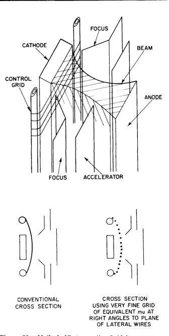
Figure 39. Method of Representing Grid for Field Plot
