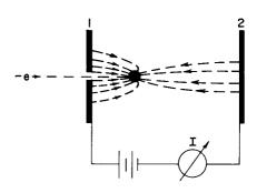
Figure 11. Electron-Induced Current in a Two-Electrode System
