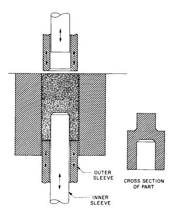
Figure 5. Die With Concentric Sleeves
