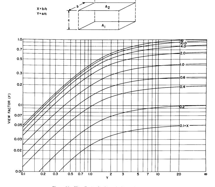
Figure 10. View Factor for Directly Opposed Parallel Planes
