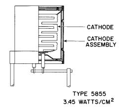
Figure 19. Directly Heated Cathode Structure of Type 5855
