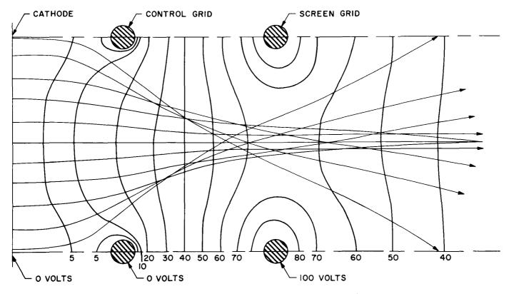
Figure 8. Electron Trajectories for a Developmental Tube
