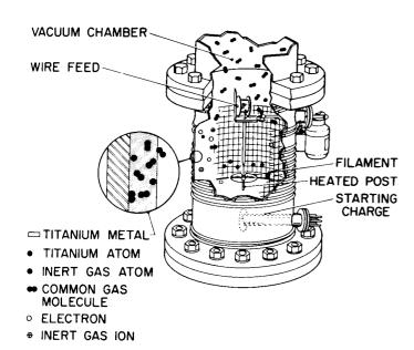
Figure 20. Evapor-Ion Pump
