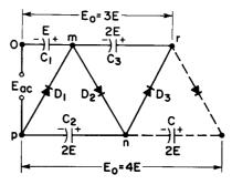
Figure 41. Half-Wave Voltage-Tripler (and half-wave voltage-quadrupler, by addition of dotted section)
