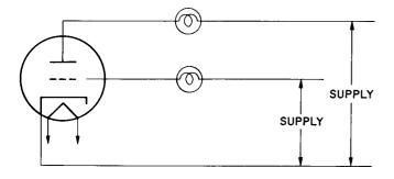
Figure 3. Triode Aging Circuit
