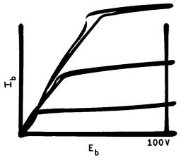
Figure 12. Horizontal-Deflection-Tube Plate Characteristic at Zero-Bias Voltage
