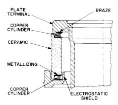
Figure 3. Improved Seal Using Contoured Ceramic
