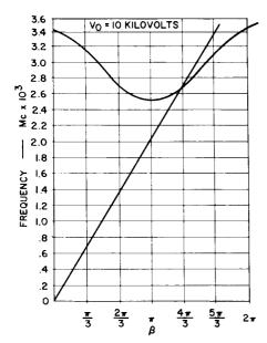
$\omega$  -  $\beta$  Diagram for the Figure 23. Folded-Waveguide Structure Shown in Fig. 22
