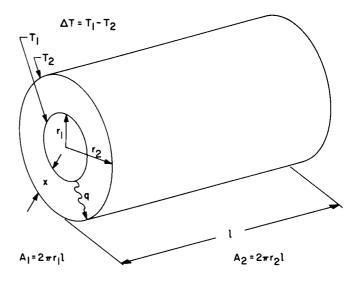
Figure 2. Dimensions of a Cylinder
