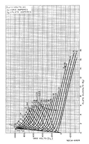
Figure 31. Constant-Current Curves for 5671 Power Triode
