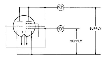
Figure 10. Two-Lamp Triode-Pentode Aging Circuit
