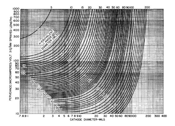
Figure 12. Universal Plane-Parallel Diode Design Curves
