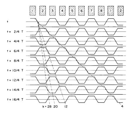
Figure 8. Plot Showing π-Mode Anode Potential Wave at Several Instants in an 8-Resonator Magnetron
