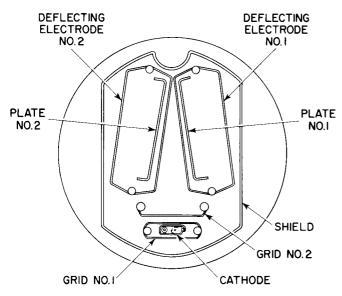
Figure 9. Cross Section of 7360 Beam-Deflection Tube
