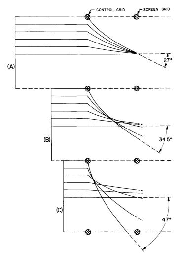
Figure 13. Calculated Beam Shapes: (A) a/b = 1.00; (B) a/b = 0.50; (C) a/b = 0.33
