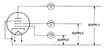
Figure 4. Pentode Aging Circuit
