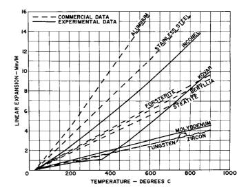
Figure 2. Thermal Expansion of Ceramics and Metals
