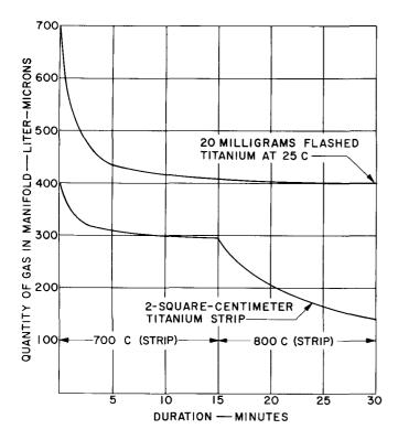
Figure 7. Absorption of a Mixture of 50 Per Cent Oxygen and 50 Per Cent Carbon Monixide by Titanium
