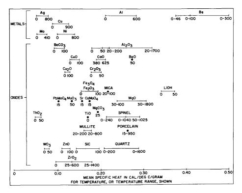
Figure 12. Specific Heats of Ceramics and Metals
