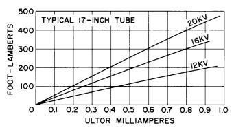
Figure 18. Brightness of a Typical Picture Tube as a Function of Ultor Current for Several Values of Ultor Voltage
