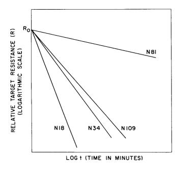
Figure 1. Graph of Target Resistance Plotted Against Elapsed Time for Different Alloys (R<sub>O</sub> is the target resistance at t = 1 minute; resistance units are arbitrary)
