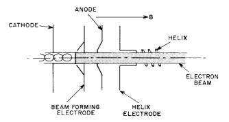
Figure 25. Schematic Diagram of a Parallel-Flow Electron Gun
