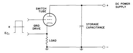
Figure 11. Simplified Circuit of a Triode Tube Used as a Switch in a Hard-Tube Modulator
