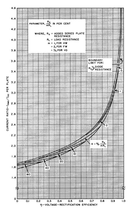
Figure 34. Current Ratio (rms steady-state current to dc-current per plate) vs. Voltage Rectification Efficiency for Rectifiers with High-Input-Capacitance Filter
