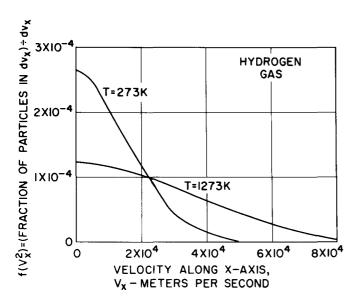
Figure 12. Velocity Distribution (Hydrogen gas)
