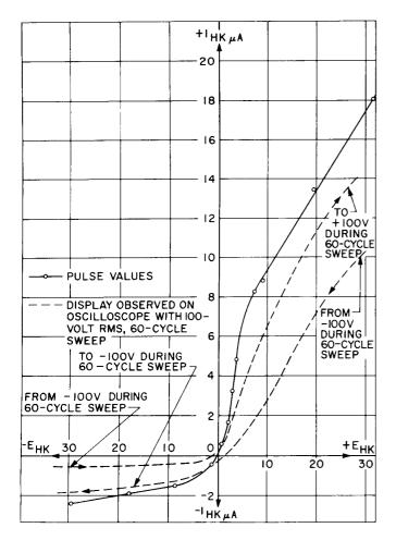
Figure 16. Heater-Cathode Leakage Characteristics Measured by Different Methods on the Same Tube to Illustrate the Effects of Polarization
