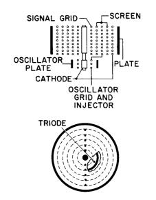
Figure 10. Electrode Arrangement of the Triode-Heptode Type 6J8-G
