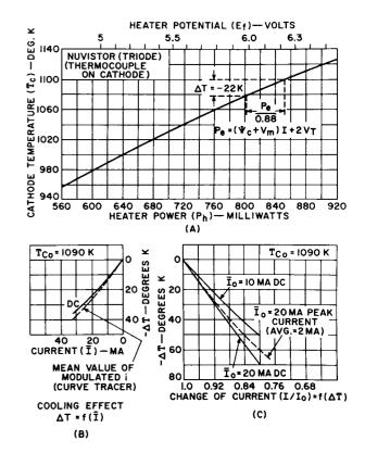
Figure 18. Cathode Temperature ( $T_c$ ) and Cooling Effects (- $\Delta T$ ) Caused by Electron Emission: (A) cathode temperature of a triode as a function of heater power (I=0); (B) cooling effect -  $\Delta T$  as function of average current; (C) current change  $\bar{I}/\bar{I}_0$  as function of temperature change
