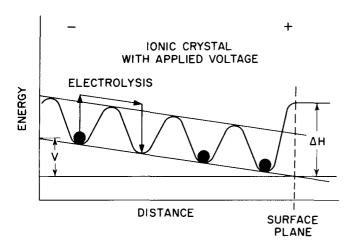
Figure 4. The Periodic Electric Field with a Voltage
