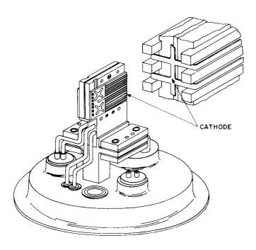
Figure 8. Hairpin-Type, Self-Supported, Directly-Heated Cathode Used in RCA-8D21
