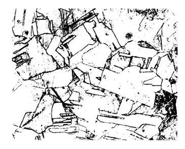
Figure 2. Grain Structure of Nickel (200 X)
