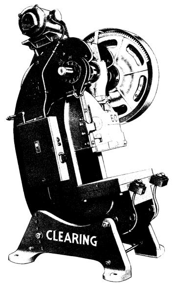
Figure 1. Open Back Inclinable Press
