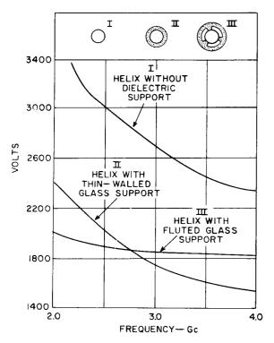
Figure 12. Effect of the Dielectric Loading on Helix Dispersion Resulting from Different Types of Support Structures
