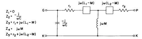
Figure 7. Equivalent Circuit for Figure 6 With Tickler Winding Connected in Wrong Polarity
