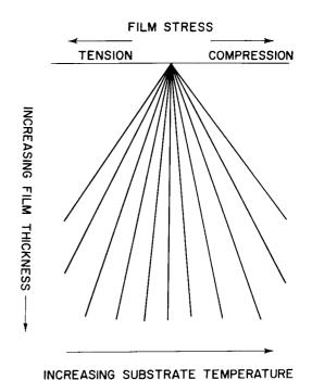
Figure 13. Film Stress for a Typical Semiconductor Evaporated on Glass Substrate
