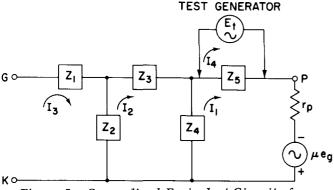
Figure 5. Generalized Equivalent Circuit of an Oscillator Using an Electron Tube to Produce Negative Resistance
