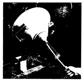
Figure 1. Application of Graphite Internal Conductive
