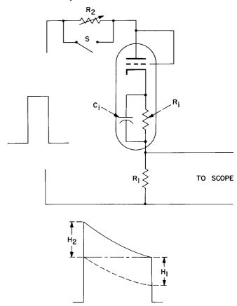
Figure 1. Effect of Cathode-Interface Layer on Plate Current
