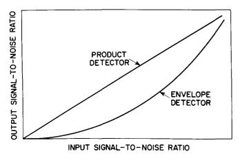
Figure 6. Comparison of Noise Response Characteristics of Product Detectors With Those of Envelope Detectors Showing the Poorer Signal-to-Noise Ratio in the Output With the Envelope Detector
