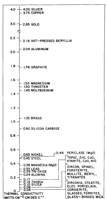
Figure 11. Thermal Conductivities of Ceramics and Metals
