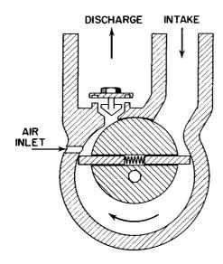
Figure 7. Cross-Section of Gas Ballast Pump
