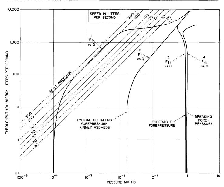
Figure 15. Q-P Curves (Q= gas through put in micronliters/sec.;  $P_1$ = inlet pressure in mm. Hg;  $P_f$ =fore presure;  $P_{ff}$ = tolerable fore pressure — causes 10% increase in  $P_1$ ;  $P_{fb}$ = breaking fore pressure — causes tenfold increase in  $P_1$ )
