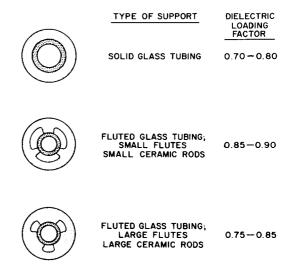
Figure 11. Range of Dielectric Loading Factor for Three Types of Helix Support Structures
