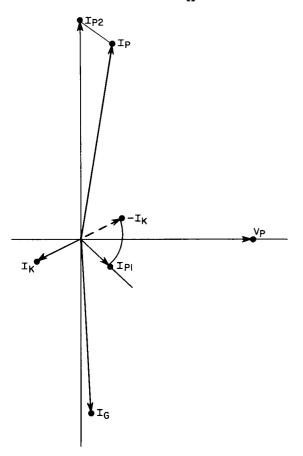
Figure 9. Triode Currents with Voltage to Plate
