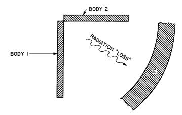
Figure 17. Cross Section of a "Right-Angled" Surface
