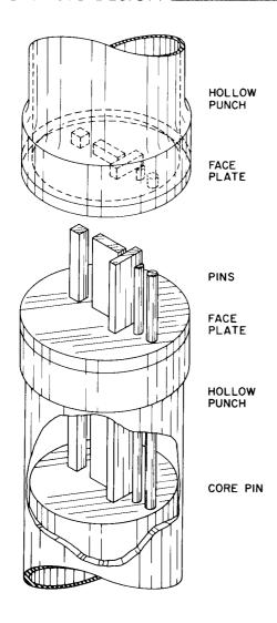
Figure 8. Typical Die For Pressing Tube Spacer
