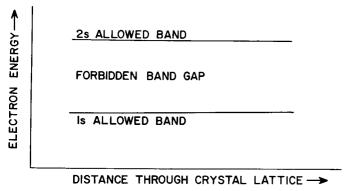
Figure 2. Simplified Band Structure
