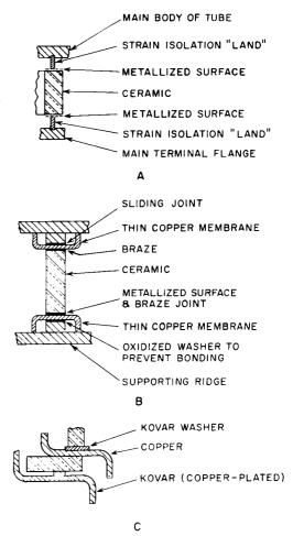
Figure 35. Examples of Metallized and Brazed Ceramic-to-Metal Seals
