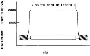
Figure 5. Temperature-Distribution Curves: (A) filament without end-loss correction; (B) filament with end-loss correction
