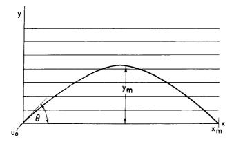
Figure 41. Electron Injection into a Uniform Field
