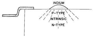
Figure 6. P-N Junction Photocell
