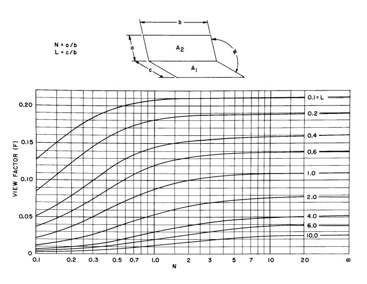
Figure 13. View Factor for Direct Radiation Between Adjacent Rectangles ( $\emptyset = 120^{\circ}$ )
