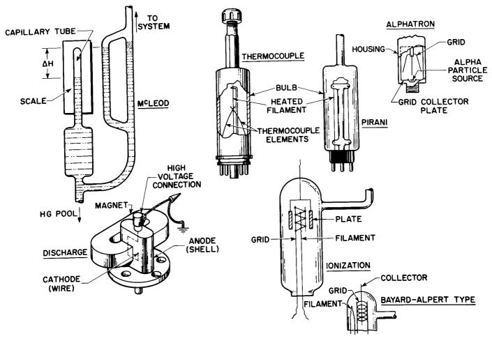
Figure 23. Types of Vacuum Gauges
