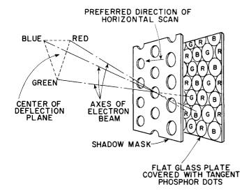
Figure 11. Diagram of Shadow-Mask System
