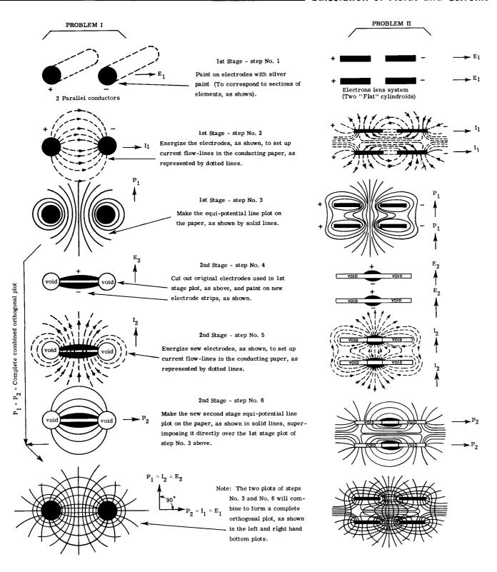
Figure 37. Illustrations of "Two-Stage" Plotting Method
