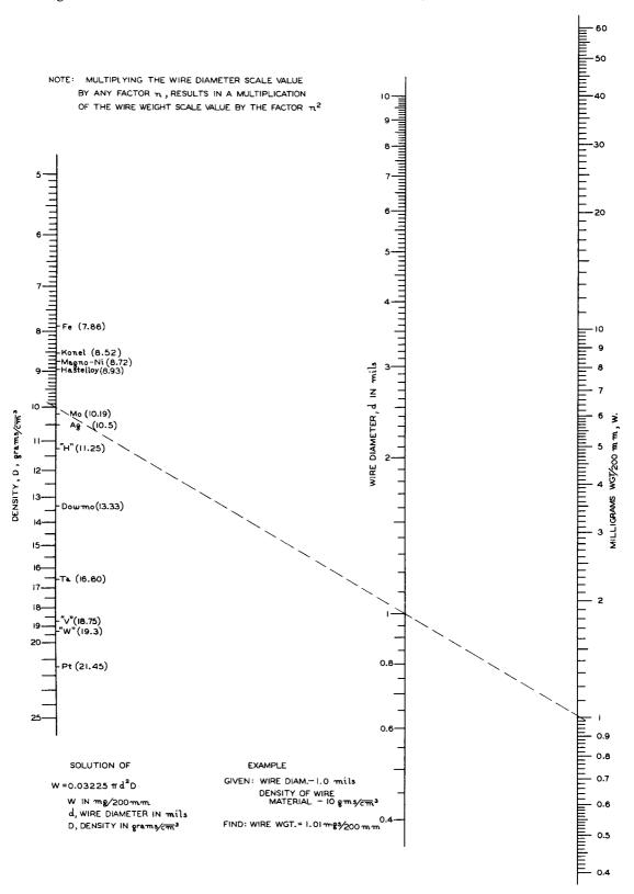
Figure 2. Round Wire: Weight, Diameter, and Density
