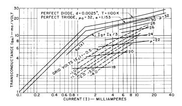
Figure 16. Theoretical and Measured Transconductances  $(g_{mk})$  of a Triode  $(d_1 = 0.00255 \text{ inch}, d_2 = 0.00665 \text{ inch}, \ \bar{\mu}_0 = 32, A = 0.185 \text{ cm}^2)$
