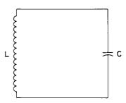
Figure 1. Simple LC Oscillator Circuit
