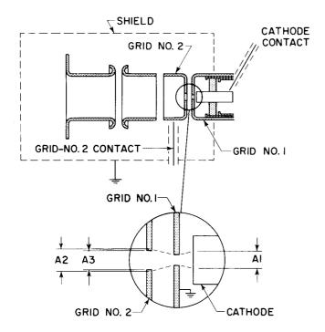
Figure 5. Capacitance in Picture Tube Electron Gun
