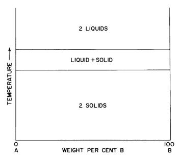
Figure 9. Phase Diagram of Two Mutually Insoluble Elements
