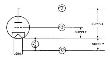
Figure 12. Triode Aging Circuit Showing Heater-Cathode Aging
