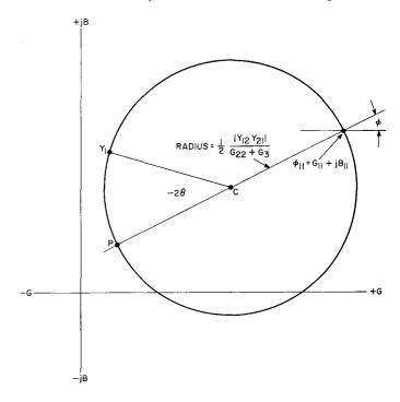
Figure 4. Locus of Input Admittance Equation
