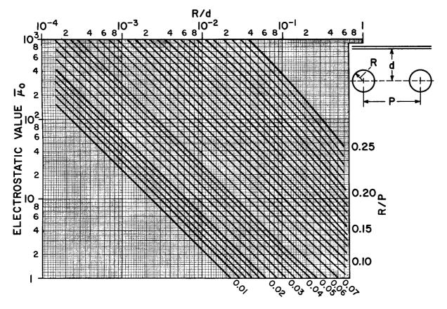
Figure 33. Amplification Factor of Triodes
