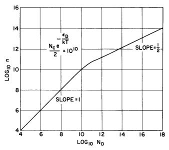
Figure 11. The Density of Electrons n in the Conduction Band of a Solid as a Function of the Donor Density  $N_D$  When  $N_c e^{\epsilon} D/kT = 2 \times 10^{10}$
