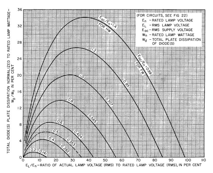
Figure 23. Total Anode Dissipation in Half-Wave and Full-Wave Rectifier Circuits with a Tungsten Lamp Load
