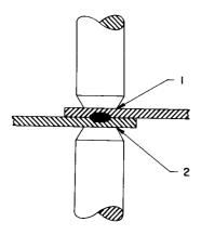
Figure 1. Typical Spot-Welding Operation
