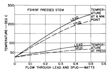
Figure 29. FS1419F Pressed Stem Heat-Flow Characteristics
