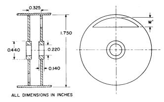
Figure 22. Cross-Sectional Drawings of a Folded-Waveguide Slow-Wave Structure Designed for S-Band Operation at 1 Kilowatt of Peak Power over a 20 Per Cent Bandwidth
