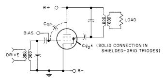
Figure 18. Grid-Driven Tetrode Amplifier
