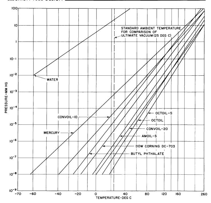
Fig. 18. Pressure-Temperature Characteristics of Pump Fluids
