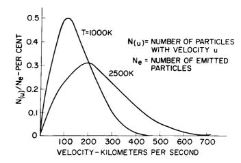
Figure 3. Form of the Normally-Directed Maxwellian Velocity Distribution
