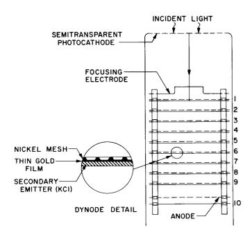
Figure 6. Transmission Type of Multiplier
