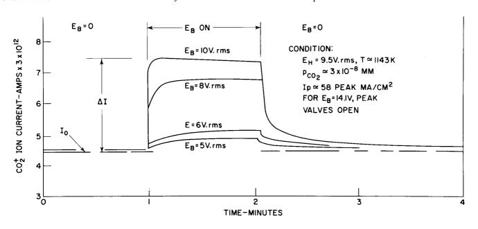
Figure 31. Carbon-Dioxide Evolution of a Ba0 Cathode as a Function of Time and Anode Voltage
