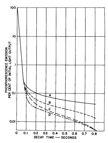
Figure 10. Phosphorescence Emission as a Function of Decay Time for Various Excitation Current Densities. Excitation current density: curve A, 0.04  $\mu$ A/cm²; curve B, 0.25  $\mu$ A/cm²; curve C, 0.56  $\mu$ A/cm²; curve D, 1.5  $\mu$ A/cm²; (after Leverenz)
