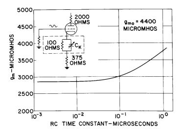
Figure 6. Curve Illustrating the Effect of Cathode Impedances of Different Time Constants on Circuit Response to a 10 Kc Signal (the design  $g_m$  (or  $g_{m0}$ ) is 4400 micromhos;  $R_b$  is 120 ohms in all cases)
