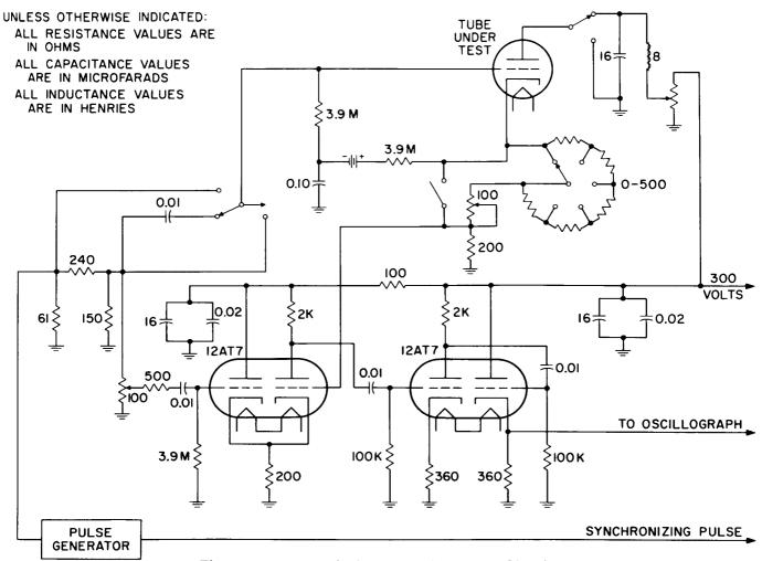
Figure 15. Hannig Cathode-Impedance Test Circuit
