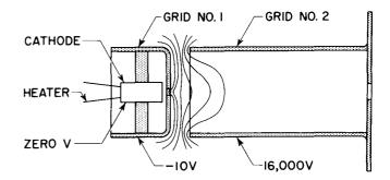
Figure 1. Magnetic-Focus, Triode-Type Gun
