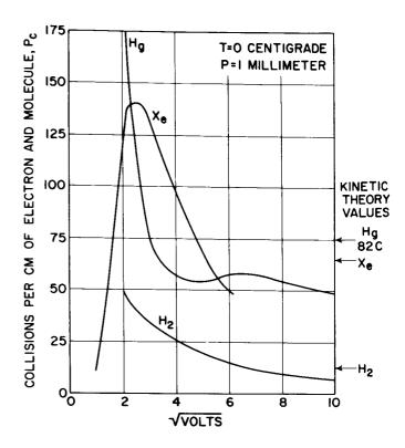
Figure 5. Probability of Collision
