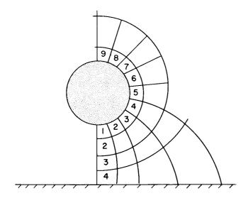
Figure 40. Field Sketching Using Curvilinear Squares
