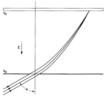
Figure 4. Beam Focusing in Refraction Case
