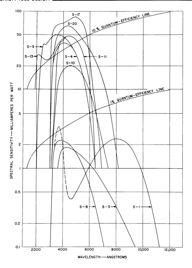
Figure 1. Spectral Sensitivity Characteristics of Photocathodes in Phototubes
