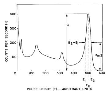
Figure 10. Pulse-height Spectrum of  $Cs^{137}$  as Obtained from a Scintillation Counter Using NaI(Tl)Crystal and a Single-Channel Pulse-Height Analyzer. By Definition Pulse-Height Resolution is  $E_2$ - $E_1$ / $E_0$
