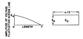
Figure 11. Voltage Along a Resonant Quarter-Wave Circuit
