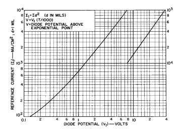
Figure 32. Normalized Diode Characteristic
