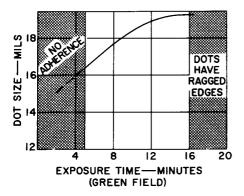
Figure 7. Effect of Exposure Time on Dot Size
