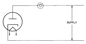
Figure 2. Diode Aging Circuit
