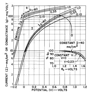
Figure 11. Diode Current and Conductance I, g = f(V) for Different Work Functions ( $\psi_c$ ) and Emission Currents ( $I_s$ ) for d = 2 Millinches, T = 900 K (Inset shows conductance change  $g/g_{1.1}$  for  $\psi_c = 1.1$  to  $\psi_c = 1.6$ .)
