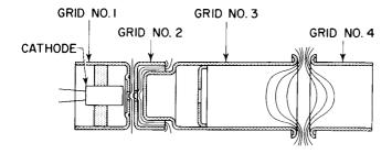
Figure 9. High-Voltage, Electrostatic-Acceleration-Type Focusing Gun
