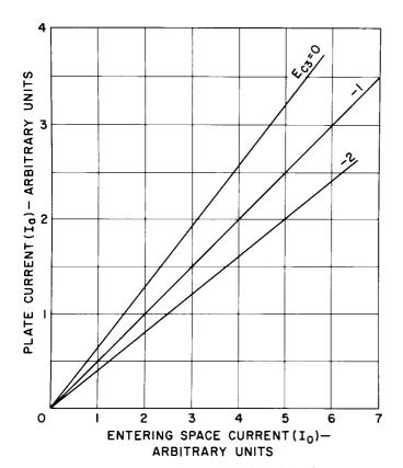
Figure 15. Idealized Curve of the Plate Current vs. the Entering Space Current (Through the Screen-Grid, Grid No. 2) in a Multigrid Tube in which the Grid No. 3 is Negative: (it is assumed that space-charge in the region between the grid No. 2 and grid No. 3 can be neglected and that the ratio of  $I_a/I_0$  is changed only as the electron paths vary with changes in  $E_{g3}$ )
