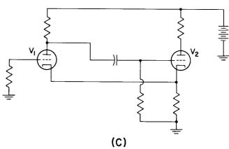
Figure 28. Common Multivibrator Circuits: (A) Platecoupled multivibrator, (B) Biased multivibrator, (C) Cathode-coupled multivibrator
