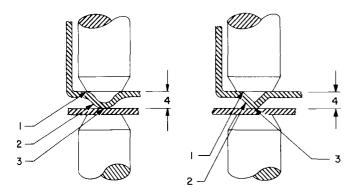
Figure 2. Typical Projection-Welding Operation
