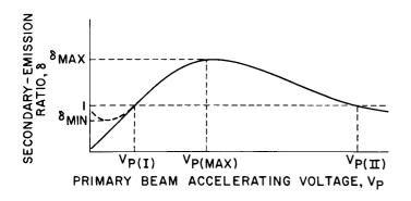
Figure 6. Idealized Secondary-Emission Curve
