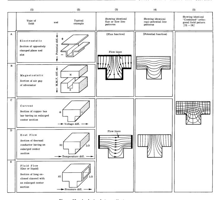
Figure 35. Analogies between Various Types of Fields
