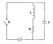
Figure 5. Simplified Equivalent of a Horizontal Deflection Circuit. The Power Tube is Essentially Switch S. Deflection Coils Are Simulated by the LRC Combination
