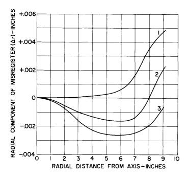
Figure 23. Radial Misregister Characteristic of 70<sup>o</sup> Shadow-Mask Tube
