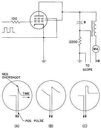
Figure 4. Blackout Test-Circuit and Oscilloscope Displays (A and B, poor tubes; C, good tube)
