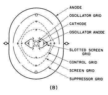
Figure 12. Beam-Type Converter Tubes: (A) crosssectional view of the 6K8 converter tube; (B) crosssectional view of the four-beam octode
