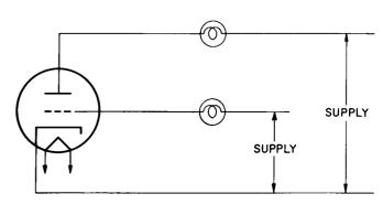
Figure 7. Two-Lamp Triode Aging Circuit
