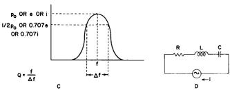
Figure 5. (A) Shunt Circuit; (B) Series Circuit; (C) Universal Resonance Curve; (D) Resonant Circuit to Relate Q and Bandwidth
