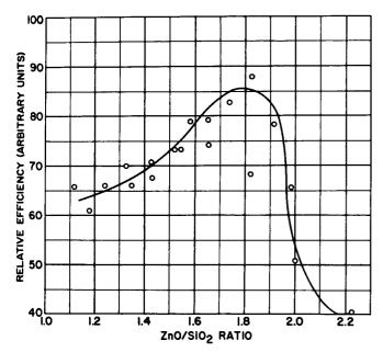
Figure 2. The Effect of the ZnO: SiO<sub>2</sub> Ratio on the Luminescent Efficiency of Willemite (after M. R. Royce)
