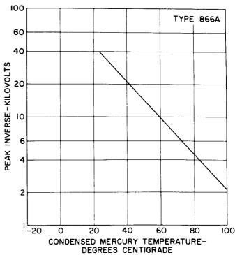
Figure 30. Arcback vs. Temperature
