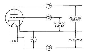
Figure 13. Triode Aging Circuit Showing AC Heater-Cathode Aging
