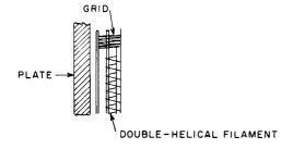
Figure 21. Triode Configuration Using Double-Helical Filament
