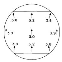
MISREGISTER (IN MILS) DUE TO A HORIZONTAL TRANSVERSE FIELD OF 0.22 GAUSS - TUBE FACING
