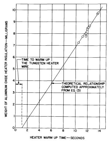
Figure 8. Calculated and Measured Dependence of Warm-Up Time on the Weight of Heater Insulation for a Series of Type 6AU6 Miniature Tubes Drawing Exactly 0.300 Ampere Heater Current
