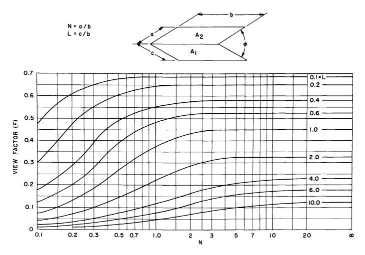
Figure 11. View Factor for Direct Radiation Between Adjacent Rectangles (\$\psi\$ = 60°)
