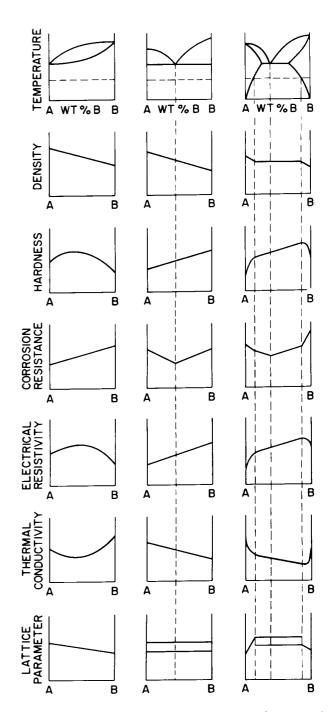
Figure 12. Relationship Between Physical Properties and the Phase Diagram
