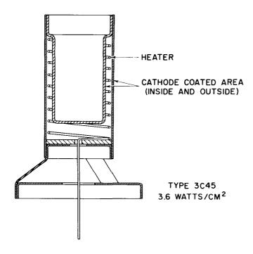
Figure 15. Indirectly Heated Cathode Structure of Type 3C45
