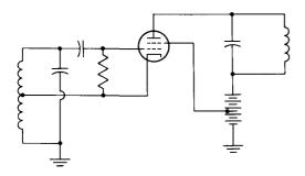
Figure 18. Electron-Coupled Oscillator Circuit Using Tetrode
