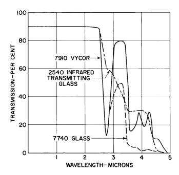
Figure 7. Infrared Transmission of Some Glasses
