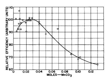
Figure 4. The Dependence of Luminescent Efficiency upon Activator Concentration in Zinc Silicate:
