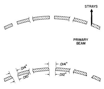
Figure 37. Advantages of Tapered Apertures in Reducing Stray Electrons
