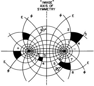
E --- ELECTROSTATIC EQUIPOTENTIAL LINES
