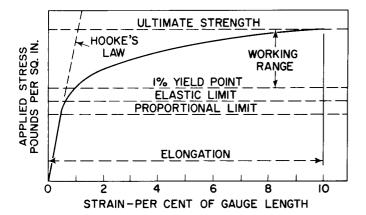
Figure 6. Example of a Tensile Test Curve
