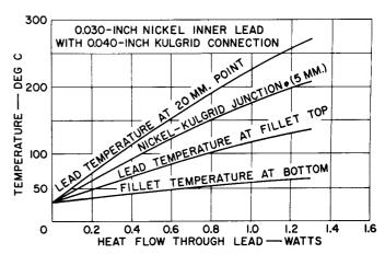
Figure 27. Stem Heat-Flow Characteristics for 1-1/4-Inch Button with 0.030-Inch Nickel Inner Leads, 0.040-Inch Kulgrid Leads Welded to the Nickel at a Point 5 Millimeters Above the Fillet
