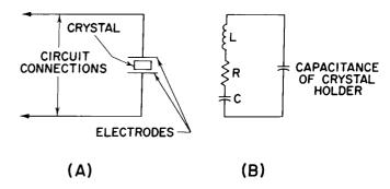
Figure 19. (A) Crystal and holder, (B) Equivalent circuit
