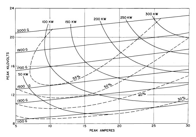
Figure 13. Performance Chart of a Typical Pulse Magnetron (Type 2J32) (frequency, 2800 Mc; pulse duration, 1 µsec; prr, 1000 pps; pulling figure, 12 Mc)
