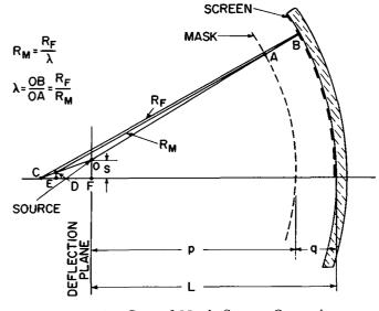
Figure 18. Curved Mask-Screen Geometry
