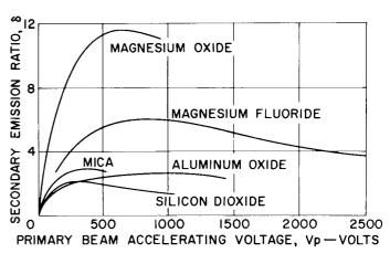
Figure 7. Secondary-Emission Characteristics, Typical Storage-Tube Dielectrics
