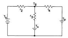
Figure 22. Simplified Heat Transfer Circuit of a Triode
