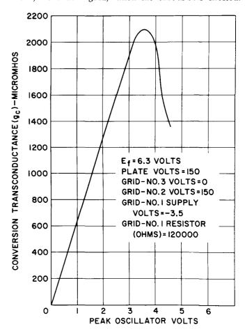
Figure 2. Operation Characteristic of the 6C8G (Pentode Unit) with Separate Oscillator Excitation
