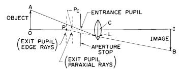
Figure 14. Occurrence of Distortion with Aperture in Front of Lens
