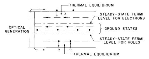
Figure 5. Model Showing Both Shallow Trapping States and Ground States
