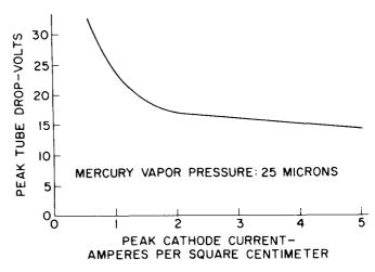
Figure 28. Sparking Limit Curve
