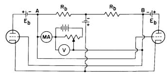
Figure 14. Basic Circuit for Kallirotron Oscillator
