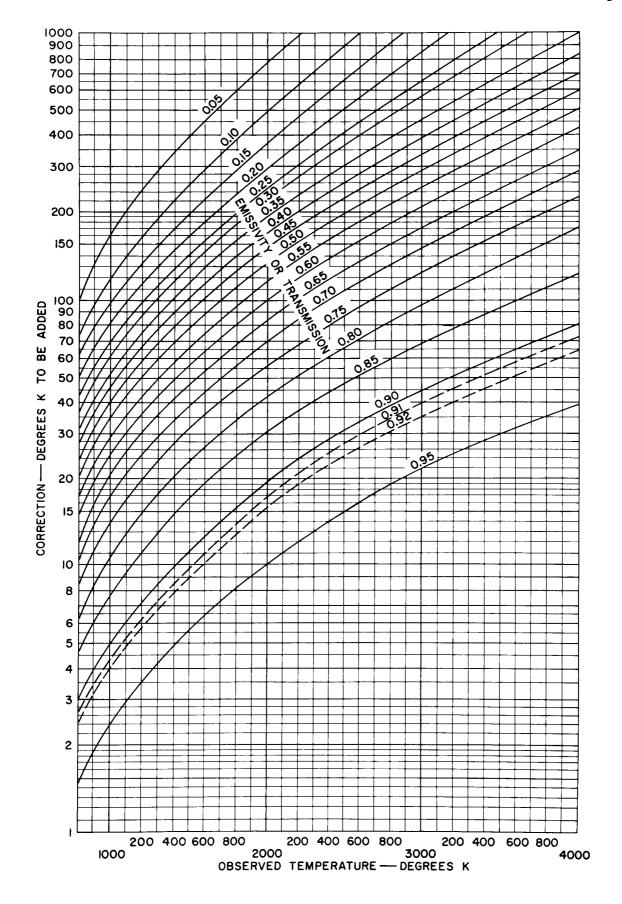
Figure 7. Corrections to Brightness Temperature Determinations by Optical Pyrometer for Transmission of Bulb and Emissivity at 0.665 Microns
