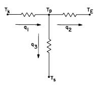
Figure 33. Simplified Heat Transfer Circuit for the Determination of the Average Plate Temperature
