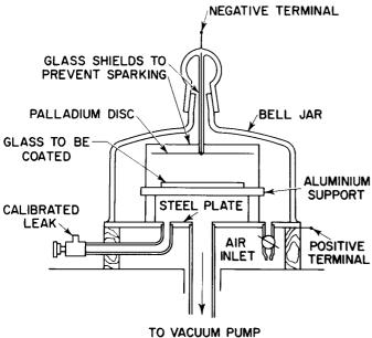
Figure 27. Typical Sputtering Apparatus
