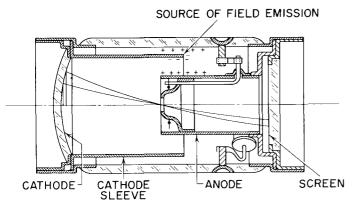
Figure 4. IC6-2 Developmental Version of Type 6929 Image-Converter Tube
