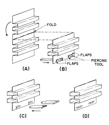
Figure 27. Riveting: (A) formed strip; (B) piercing folded strip; (C) curling and flattening flaps; (D) rivet completed
