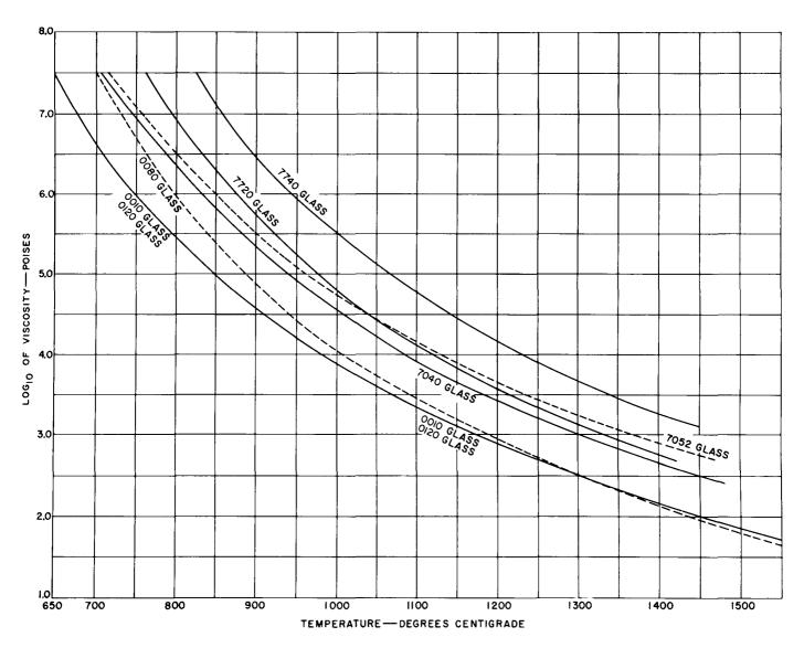
Figure 2. Viscosity vs. Temperature Curves of Representative Glasses
