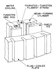
Figure 25. Triode Units Used in 6949 Shielded-Grid Beam Triode
