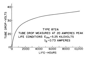
Figure 26. Tube Drop vs. Life
