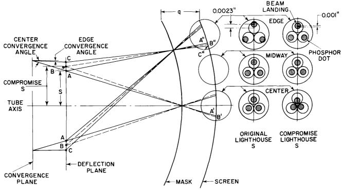
Figure 25. Effect of Dynamic Convergence on Register
