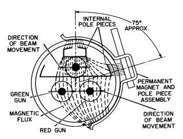
Figure 30. Schematic of Lateral Converging Pole Pieces
