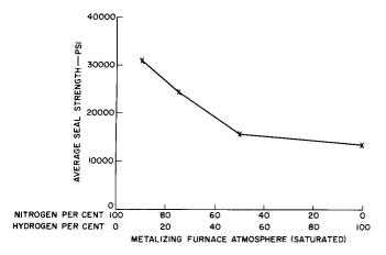
Figure 9. The Effect of Metalizing Furnace
