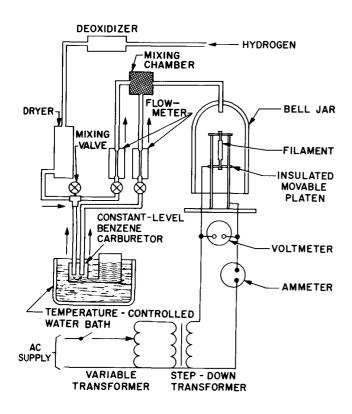
Figure 2. Typical Equipment for Carburizing Thoriated-Tungsten Filaments
