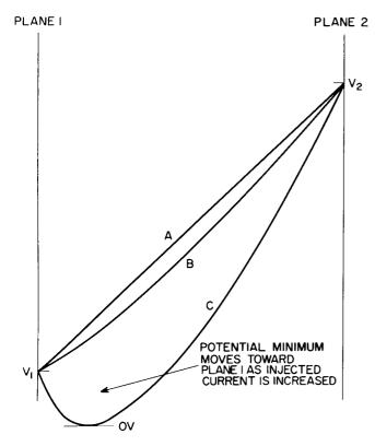
Figure 1. Typical Accelerating Potential Distributions
