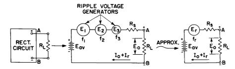
Figure 15. Equivalent Circuit for Rectifier with Resistance Load
