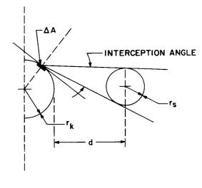
Figure 8. View Factor for Long, Opposed Parallel Rods
