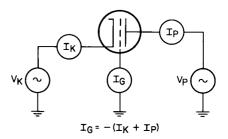
Figure 7. Grounded-Grid Triode
