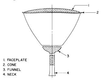
Figure 19. Glass-Metal Bulb Assembly
