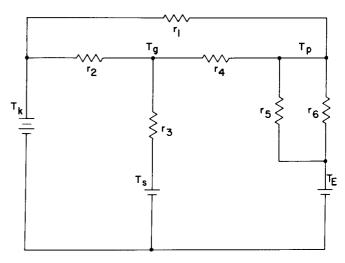
Figure 21. Heat Transfer Circuit of a Triode
