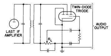
Figure 2. Diode Detector and Triode Amplifier for Amplitude-Modulation Radio Receiver
