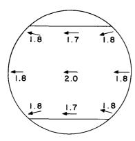
MISREGISTER (IN MILS) DUE TO A VERTICAL FIELD OF 0.54 GAUSS
