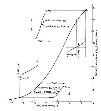
Figure 16. Transconductance as a function of Grid Bias
