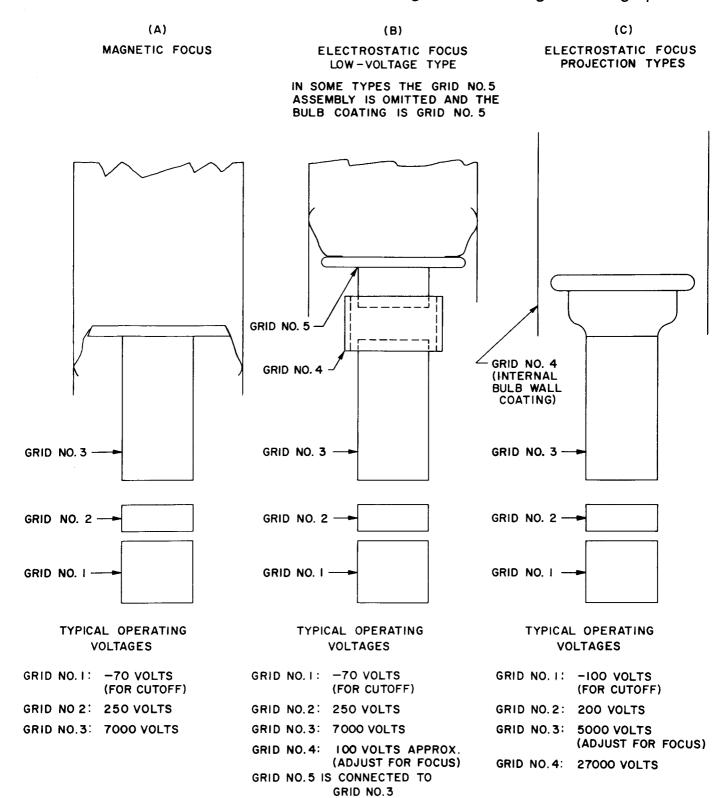
Figure 1. Typical Guns for Magnetic-Deflection Tubes
