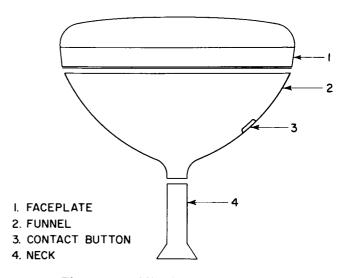
Figure 20. All-Glass Bulb Assembly
