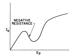
Figure 10. Curve Showing Negative Slope in Plate Current Characteristic
