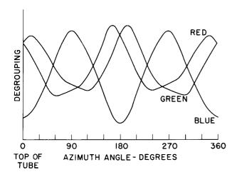
Figure 26. Azimuthal Variation of Dynamic Degrouping
