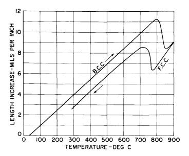
Figure 3. Thermal Expansion Curve of 5 Per Cent Manganese-Iron
