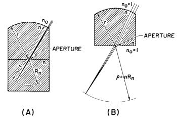
Figure 11. Curvature of Image Field, (A) Image in second medium, (B) A second (plane) boundary at the aperture permits the image to be formed in the first medium of index 1
