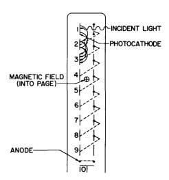
Figure 5. Electromagnetically Focused Multiplier
