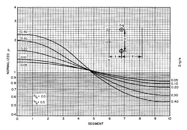
Figure 27. Mu Variation along Cathode 2r/a as a Parameter (Scholz, et al data)
