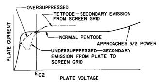
Figure 2. Pentode Plate Characteristic Curve Illustrating the Effects of Several Design Factors on Plate Resistance.
