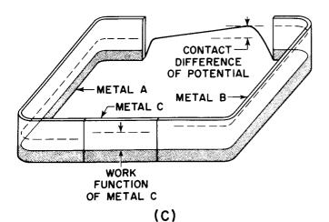
Figure 2. Illustration of the Concept of Contact Potential Between Two Metals: (A) case of two approaching metals separated by two different gaps; (B) case of two approaching metals where one gap has closed but other gap remains; (C) case of two approaching metals where one gap has been closed by a third metal, but other gap remains
