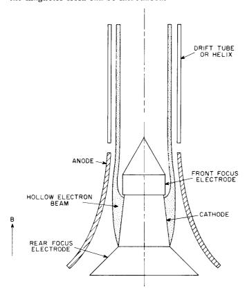
Figure 28. Cross Section of a Magnetron-Injection Electron Gun
