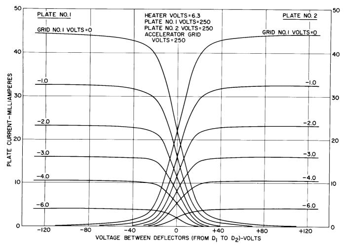
Figure 8. Average Transfer Characteristics of the 6AR8
