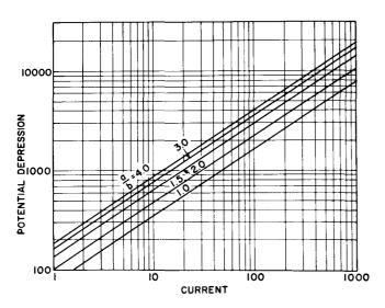
Figure 55. Design Chart Used to Determine the Space-Charge Depression of an Electron Beam
