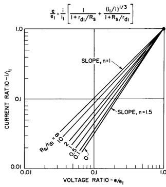
Figure 6. Log-Log Plot of Eq. (6c) for Different Values of  $R_{\rm S}/r_{\rm dl}$
