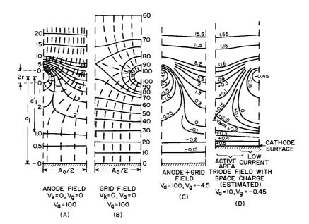
Figure 12. Unit Potential Fields and Composite Potential Field of a Triode: (A) unit anode-field  $V_k=0$ ,  $V_g=0$ ,  $V_a=1$  volt (100 per cent); (B) unit grid-field  $V_k=0$ ,  $V_a=0$ ,  $V_g=1$  volt (100 per cent); (C) composite electrostatic field for  $V_a=100$ ,  $V_g=-4.5$ ; (D) composite field with space charge (estimated) for  $V_a=10$ ,  $V_g=-0.45$
