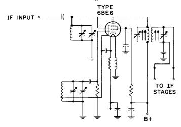
Figure 4. Typical Self-Excited Converter Circuit for 6BE6
