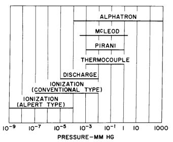
Figure 22. Ranges of Vacuum Gauges
