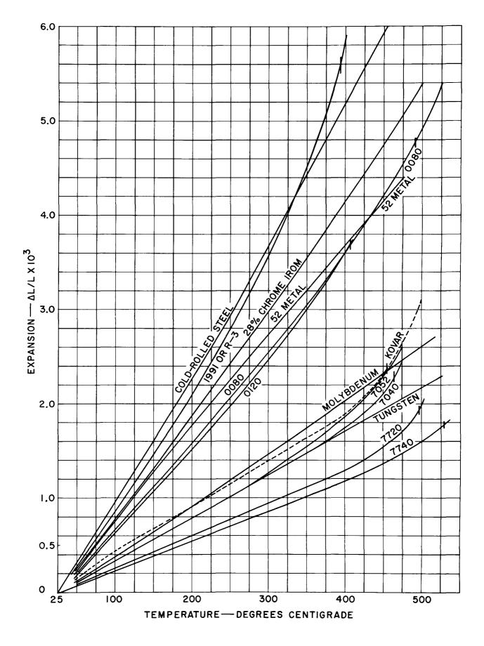
Figure 1. Thermal Expansion of Representative Glasses
