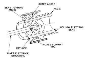
Figure 26. A Hollow-Beam Type of Parallel-Flow Electron Gun
