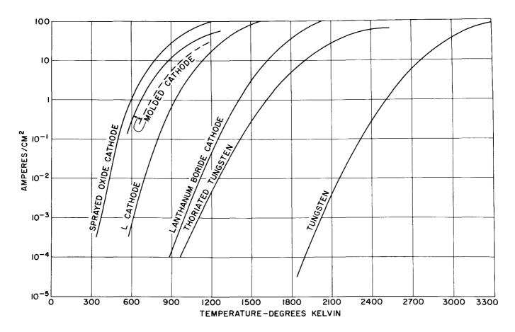
Figure 9. Pulsed-Emission Levels of Cathode Systems $^{28}$
