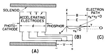
Figure 6. Magnetically Focused Image Converter: (A) schematic arrangement of electrodes, (B) magnetic and electric field and paths of electrons with and without a vertical velocity component, (C) electron paths as seen from the screen
