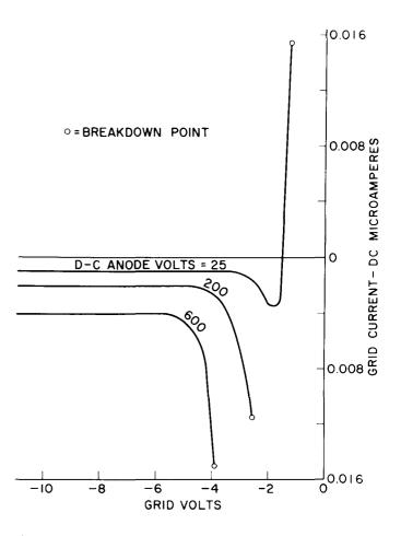
Figure 37. Grid Characteristic at Several Anode Voltages Prior to Conduction
