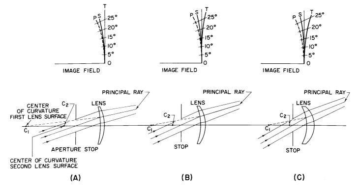
Figure 13. Flattened Image Field Using a Meniscus Lens with Properly Located Aperture Stop
