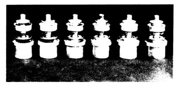
Figure 4. Effect of Chromate Tarnish Protection on Silver-Plated Tubes
