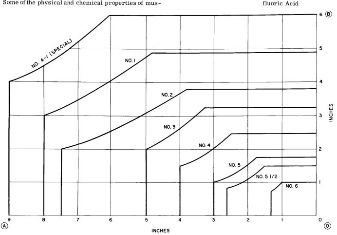
Figure 1. A.S.T.M. Chart for Grading Material Muscovite Block and Film Mica
