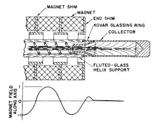
Figure 57. Cross Section of a Magnetically-Shielded Collector Assembly
