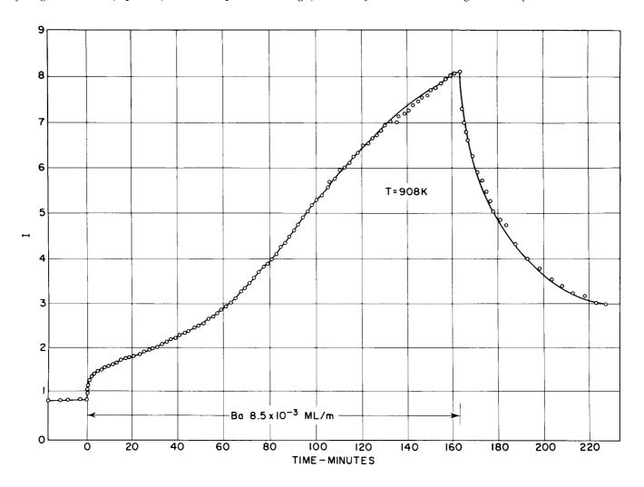
Figure 28. The Current Response of a Diode when Ba is Deposited on the Oxide Cathode. (The deposition rate is  $8.5 \times 10^{-3}$  monolayers per minute, computed on the assumption that the cathode is a smooth Ba0 crystal face.)
