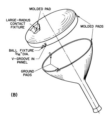
Figure 38. System Used for Referencing: (A) Panel on Screening Lighthouse; (B) Panel on Funnel
