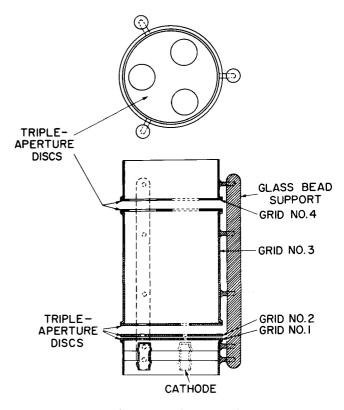
Figure 31. Schematic of Triple-Aperture Gun
