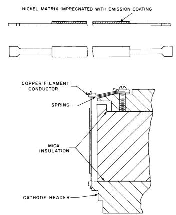
Figure 9. Cantilever-Type Spring-Tension Mounting System
