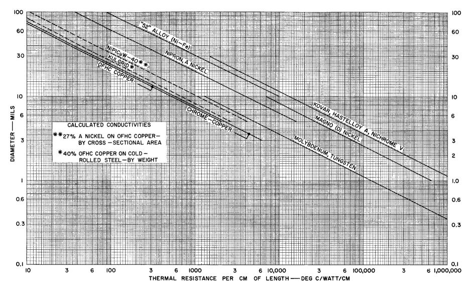
Figure 15. Thermal Resistance of Round Wires (300 C)
