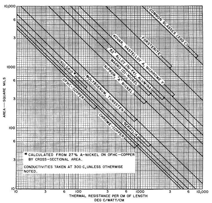
Figure 16. Thermal Resistance of Some Tube Materials
