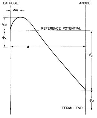
Figure 10. Potential Cross Section of a Thermionic Diode
