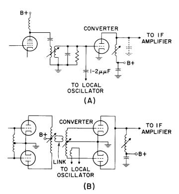
Figure 7. Converter Circuits: (A) triode; (B) balanced twin triode
