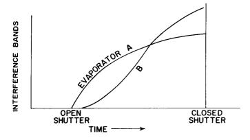
Figure 24. Band Sequence vs. Time for the Evaporation of One Type of Composition-Graded Photolayer
