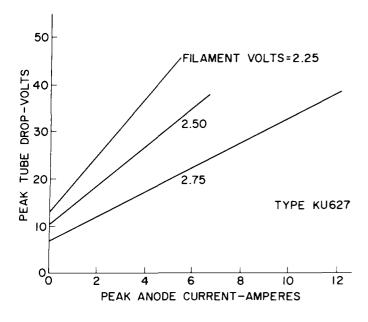
Figure 25. Tube Drop vs. Filament Voltage
