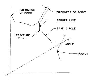
Figure 9. Improper Contour of Mica Points
