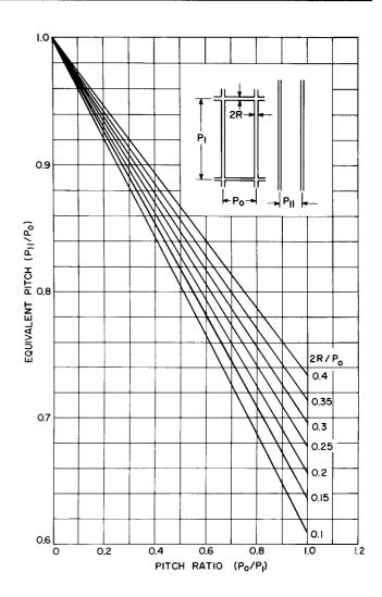
Figure 35. Equivalent Parallel-Wire Pitch  $(P_{11})$  of True-Mesh Grids
