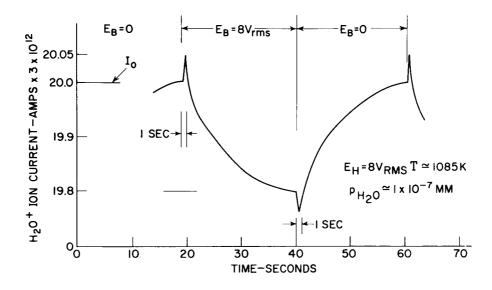
Figure 32. Water Evolution of a Ba0 Cathode as a Function of Time and Anode Voltage
