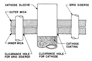
Figure 10. Cross Section of Double Mica Construction.
