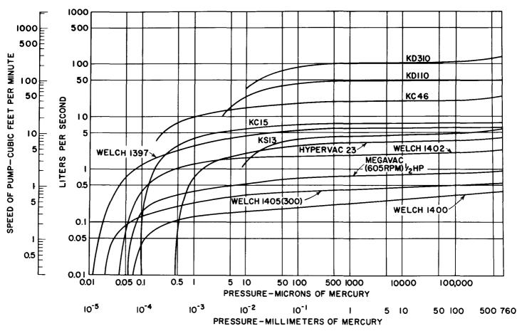
Figure 6. Pumping Speeds of Rotary Oil-Sealed Pumps
