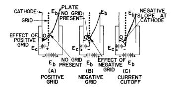
Figure 8. Effect of Grid Voltage on Voltage Distribution
