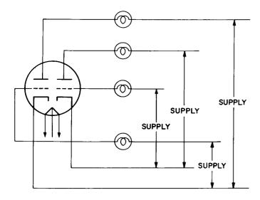
Figure 5. Twin-Triode Aging Circuit
