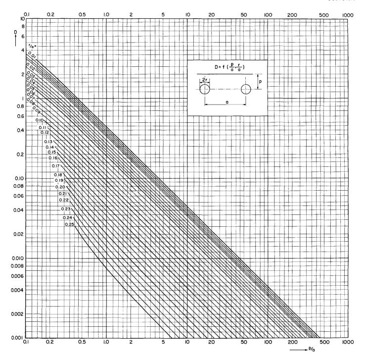
Figure 13. Design Data for Cylindrical Diodes
