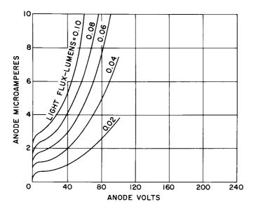
Figure 8. Anode Characteristics of a Gas Phototube (type 5583)
