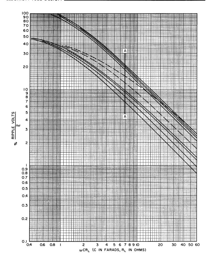
Figure 29. RMS Ripple Voltage for Capacitor-Input-Filtered Load Circuits
