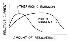
Figure 3. Effect of Resilvering on Infrared Sensitivity and Thermionic Emission
