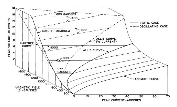
Figure 12. Three-Dimensional Plot of Current vs. Voltage vs. Magnetic Field for a Magnetron
