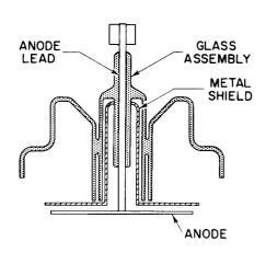
Figure 31. Reentrant Anode Lead Structure
