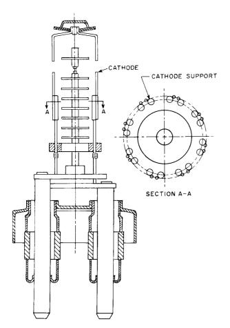
Figure 7. Directly-Heated, Cage-Type, Self-Supported, Thoriated-Tungsten Cathode Used in RCA-6166
