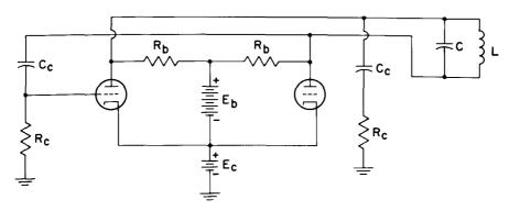
Figure 16. Practical Form of the Kallirotron Oscillator
