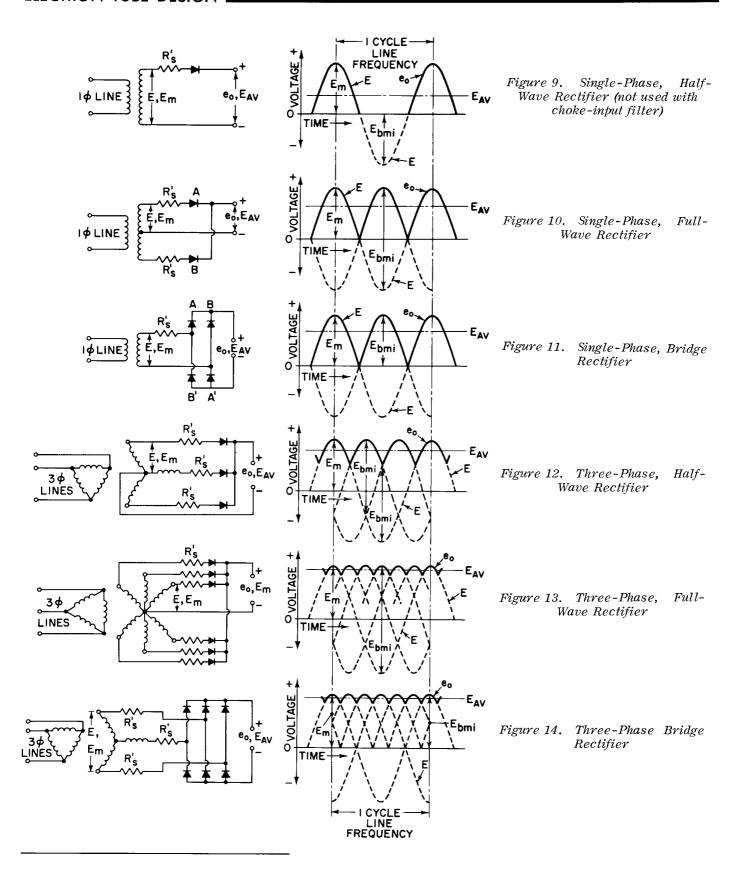
In Figs. 9 to 14 the voltage curves hold for both resistance load and choke-input-filtered load. The heavy solid curve  $(e_0)$  is the voltage at the rectifier output terminals. The voltage consists of a dc component  $E_{Av}$  (dot-dash line) and a superimposed ripple voltage. E and  $E_m$  are the RMS and peak secondary voltages, respectively.  $E_{bmi}$  is the peak inverse voltage across a diode.
