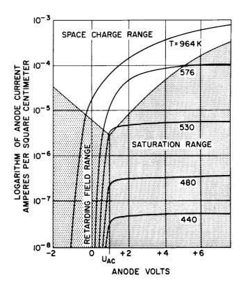
Figure 4. A Typical Family of Contact-Potential Curves with Cathode Temperature as a Parameter. Ref. 1, Vol. II, p. 28.)
