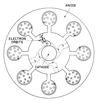
Figure 4. Space Charge in Oscillating Magnetron
