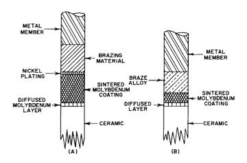
Figure 5. The Sintered-Metal Process: (A) before brazing; (B) after brazing
