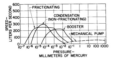
Figure 13. Speed Variations of Oil Diffusion Pumps
