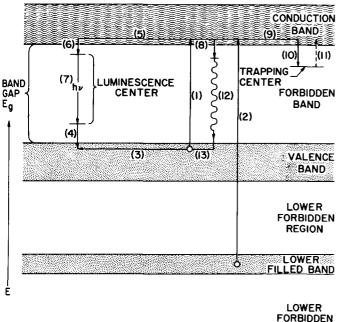
Figure 1. Plot of Electron Energy E in a Phosphor as a Function of Distance Along a Crystal Axis X with
