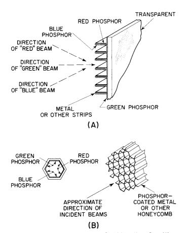
Figure 10. Complex Structures for Direction-Sensitive Screens
