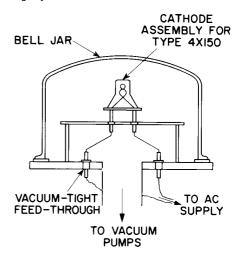
Figure 28. Vacuum Firing (cathode sintering by heating)
