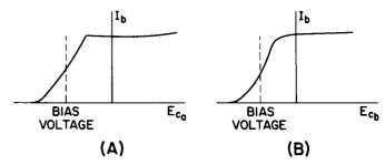
Figure 15. Transfer Characteristics for a Phase-Variation Detector Tube with Two Control Grids: (A) curve of plate current vs. voltage on grid a; (B) curve of plate current vs. voltage on grid b.
