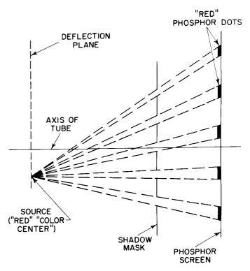
Figure 12. Shadow-Mask Principle of Operation
