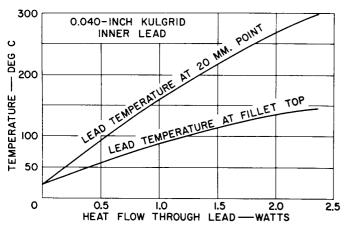
Figure 28. Stem Heat-Flow Characteristics for 1-1/4-Inch Button with 0.040-Inch Kulgrid Inner Leads
