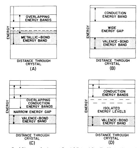
Figure 3. Energy Band Diagrams for Several Crystal Types (after Shockley): (A) Metal, (B) Insulator, (C) Intrinsic Semiconductor, (D) Impurity Semiconductor
