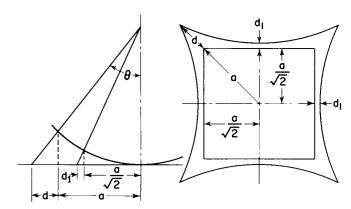
Figure 21. Comparison of Flat and Ideal Spherical Picture-Tube Faces
