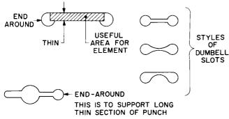
EMBOSSED POSITIONING ELEMENT SLOT WITH THIN HOLDING SECTION
