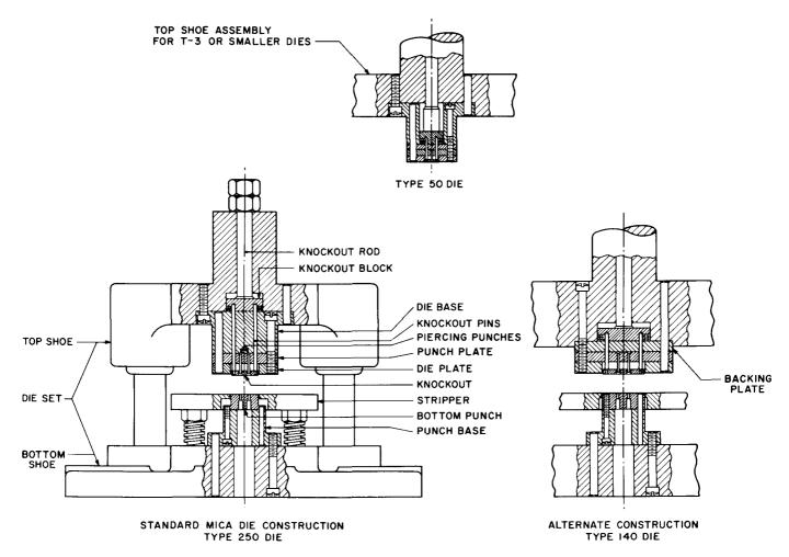
Figure 2. Typical Mica Die Construction.
