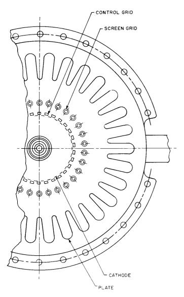
Figure 29. Unit Tetrode Systems Used in "Resnatron" Tube
