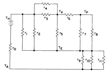
Figure 19. Heat Transfer Circuit of a Diode
