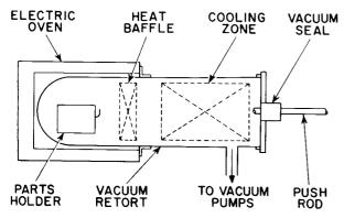
Figure 30. Vacuum Firing (electric oven)
