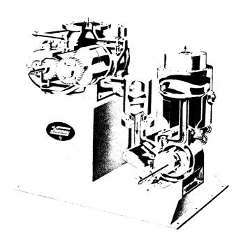
Figure 8. Mechanical Booster Pump
