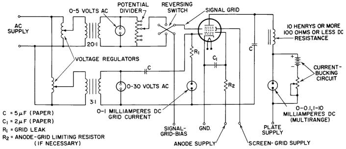
Figure 5. Circuit Arrangement for Measuring Conversion Transconductance
