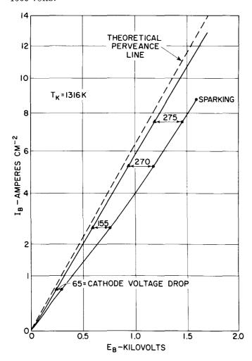
Figure 21. The Effect of Cathode Resistance on a Diode Characteristic (after Eisenstein)
