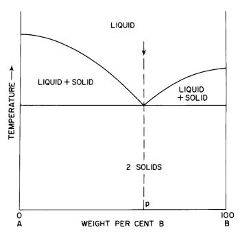
Figure 10. Phase Diagram Showing Mutual Solubility in the Liquid, But Not in the Solid Phase
