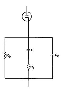
Figure 20. The Small-Signal Equivalent Circuit of a Diode with a Given Direct Current
