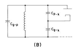
Figure 25. (A) Resonant-line oscillator; (B) Equivalent circuit of a resonant-line oscillator
