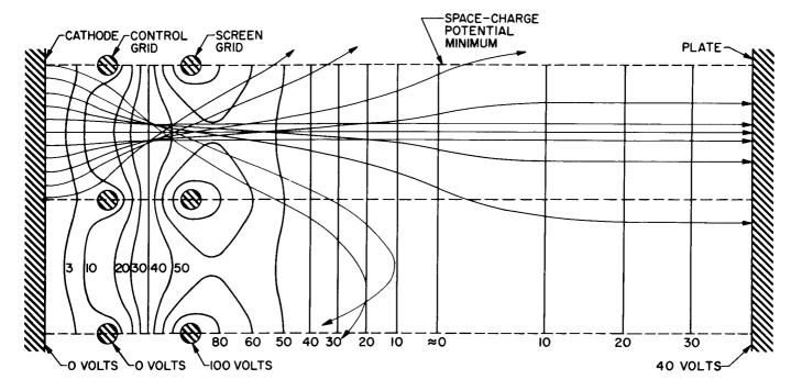
Figure 1. Field Shape and Electron Trajectories in a Typical Tube Operated with the Control Grid at Cathode Potential and the Plate
