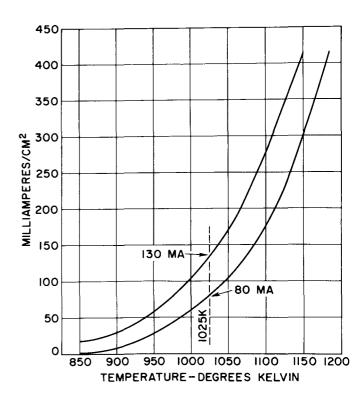
Figure 8. Permissible Direct-Current Density (ma/cm²) for Long Life Performance for Average Oxide-Coated Cathodes
