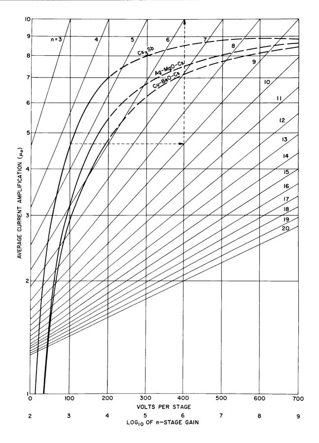
Figure 2. Average Current Amplification per Stage as a Function of Voltage per Stage
