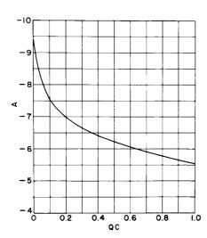
Figure 6. The Initial-Loss Parameter A as a Function of the Space-Charge Parameter QC
