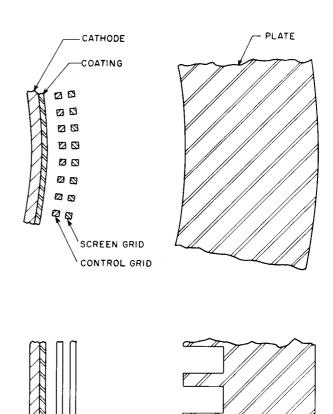
Figure 22. Tetrode Configuration Using Array of Control-Grid and Screen-Grid Elements around Continuous Cathode Surface
