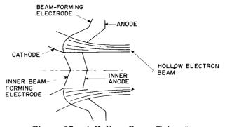
Figure 27. A Hollow-Beam Type of Convergent-Flow Electron Gun
