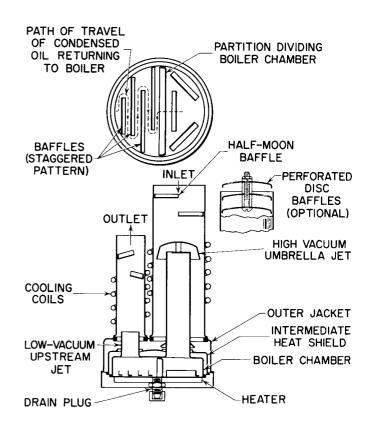
Figure 12. Operation of a Typical High-Vacuum Vapor
