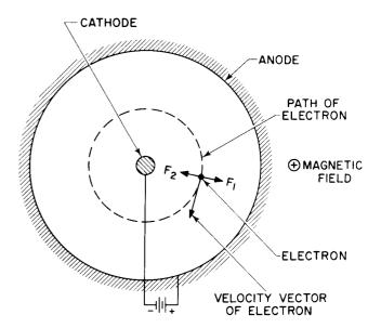
F<sub>1</sub> = FORCE DUE TO ELECTRIC FIELD F<sub>2</sub> = FORCE DUE TO MAGNETIC FIELD
