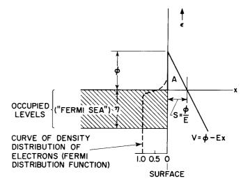
Figure 13. Energy-Level Diagram of a Metal with an Intense Electric Field at the Surface so that Field Emission Occurs
