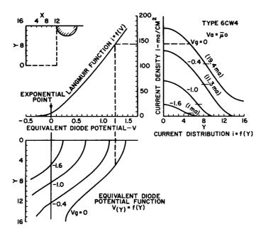
Figure 26. Potential and Current Distribution for Four Grid Potentials ( $V_g$ ) of a Nuvistor Triode at  $V_a = \overline{\mu}_0$
