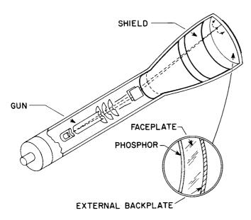
Figure 1. Oscillograph-Type Electrostatic Storage
