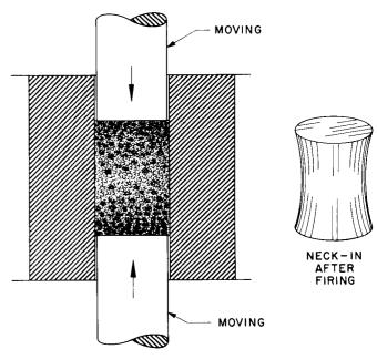
Figure 7. Shrinkage of Long Cylinder Pressed From Both Ends
