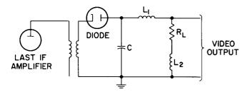
Figure 3. Series Diode Detector Stage for Video Detection in Television Receiver
