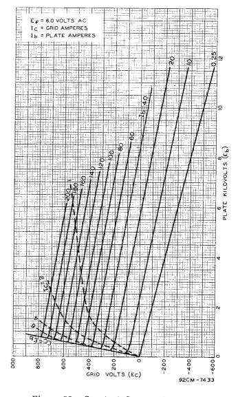
Figure 33. Constant-Current Curves for 5831 Beam Triode
