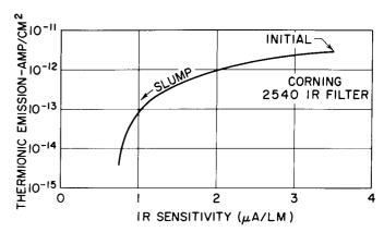
Figure 2. Relation between Infrared Sensitivity and Thermionic Emission as Cathode Sensitivity Slumps
