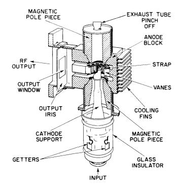
Figure 6. Cutaway View of RCA-6521 Magnetron
