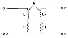
Figure 6. Circuit for Oscillator Using Tickler Feedback Coil
