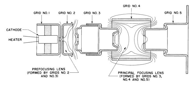
Figure 6. Electrostatic-Focus, Straight-Type Gun
