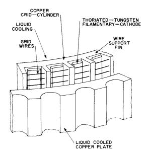
Figure 26. Unit Triode Systems Used in High-Mu Tubes for uhf Service
