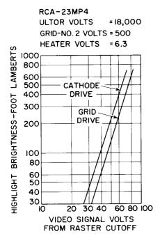
Figure 16. Transfer Characteristics of RCA-23MP4
