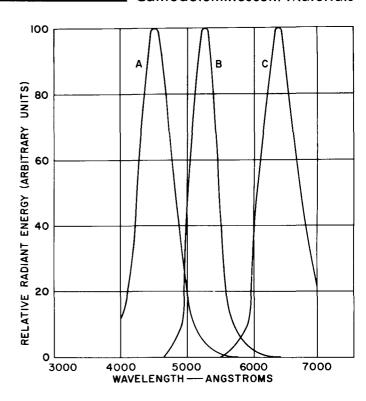
Figure 6. Relative Radiant Energy as a Function of Wavelength for RCA Phosphors (A) 33-Z-265; (B) 33-W-2A, (C) 33-Z-639D. Excitation voltage =8 kilovolts; current density =1.5 \mu A/CM^2 for defocused spot; ordinates for curves A, B, and C are independent
