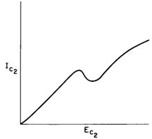
Figure 12. Negative Slope in Screen-Current Characteristic
