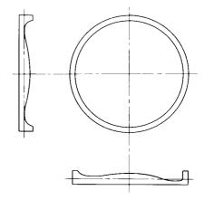
Figure 27. Contour of Degrouping Lens
