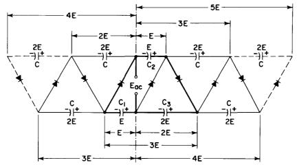
Figure 43. Half-Wave Voltage-Multiplying Rectifier
