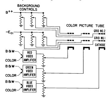
Figure 42. Individual-Video-Gain-Control System
