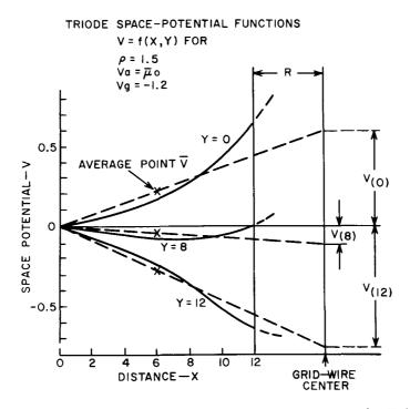
Figure 25. Electrostatic Space-Potential Functions of a Triode
