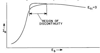
Figure 9. Horizontal Output Beam Power Pentode
