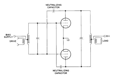
Figure 15. Push-Pull Triode Amplifier Circuit
