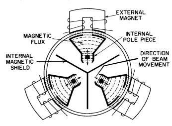
Figure 29. Schematic of Radial-Converging Pole Pieces
