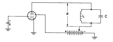
Figure 11. Circuit Diagram of Dynatron Oscillator
