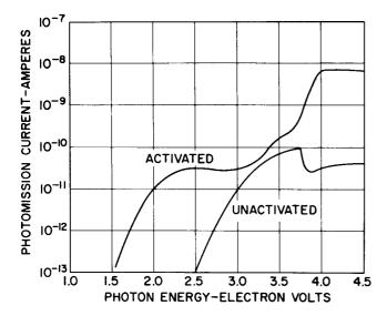
Figure 15. The Photoemission Current vs. Photon Energy for Activated and Unactivated Ba0
