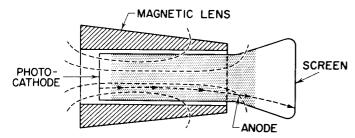
Figure 7. Image Tube with Special Short Magnetic Lens
