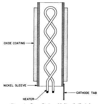
Figure 1. Cross Section of Indirectly Heated Oxide-Coated Cathode
