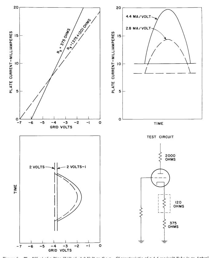
Figure 5. The Effect of a Bias Shift of -0.3 Volt on the  $g_m$  Characteristic of a 4.4 ma/volt Tube in an Actual Circuit (this effect was produced by physically placing a 120-ohm resistor in the cathode circuit)
