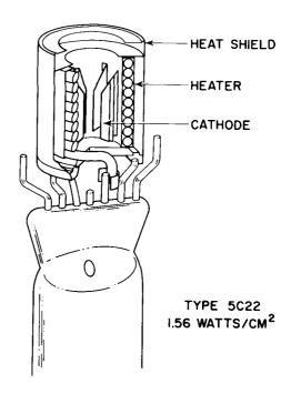
Figure 16. Indirectly Heated Cathode Structure of Type 5C22
