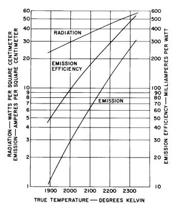
Figure 9. Variation of Emission, Emission Efficiency, and Radiation of Thoriated Tungsten as a Function of Temperature
