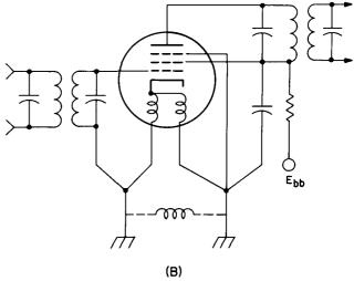
Figure 1. Use of Double Cathode Leads in IF
