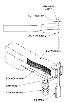
Figure 10. Pantograph-Type Mounting System
