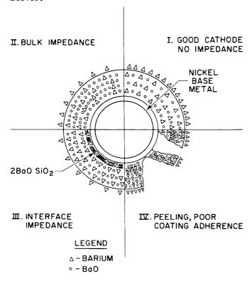
Figure 3. Cathode-Condition Diagram
