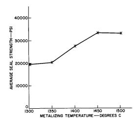
Figure 8. The Effect of Metalizing Temperature on Seal Strength
