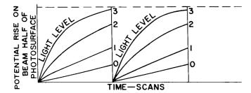
Figure 17. Potential of Beam Side of Photo Surface vs. Time
