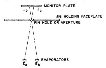
Figure 23. Pin-Hole Evaporation Camera (PHEC)
