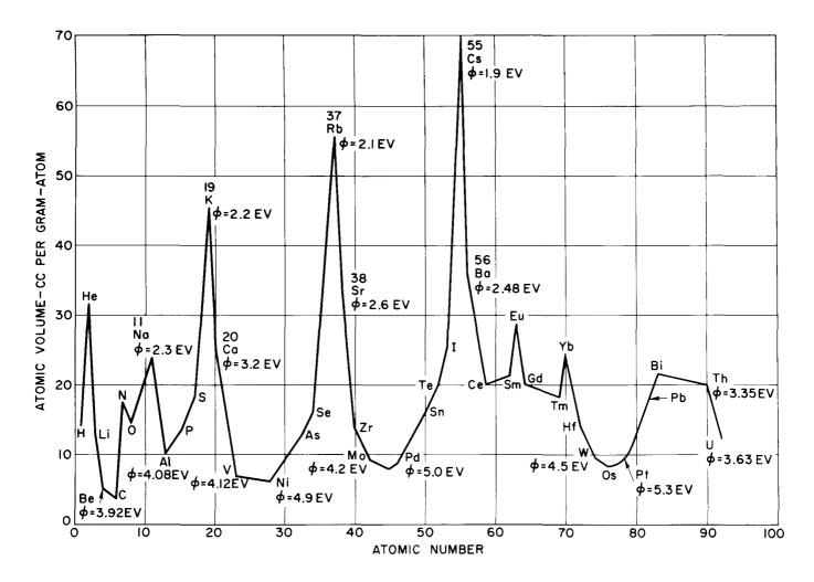
Figure 1. Atomic Number Versus Atomic Volume for Elements with Various Work Functions (Ø)
