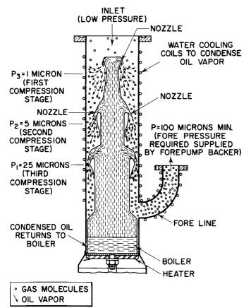
Figure 10. MCF Type Oil Pump
