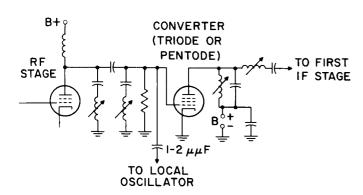
Figure 8. Pentode Converter Circuit
