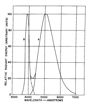
Figure 7. Spectral Emission Curves for Zn): Zn (33-Z--613) Showing the Emission Change When Current Density Is Varied at an Excitation Voltage of 8 Kilovolts: curve A, 1.5 μA/cm<sup>2</sup>; curve B, 100 uA/cm<sup>2</sup>
