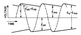
Figure 39. Full-Wave Voltage-Doubler Rectifier and Voltage Waveshapes
