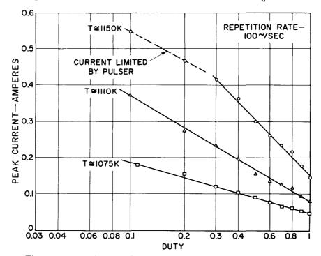
Figure 27. Peak Pulse Current vs. Duty for an Oxide Cathode
