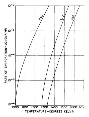
Figure 13. Rate of Evaporation of Alkaline-Earth Oxides 50
