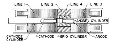
Figure 27. Sketch of Reentrant Oscillator
