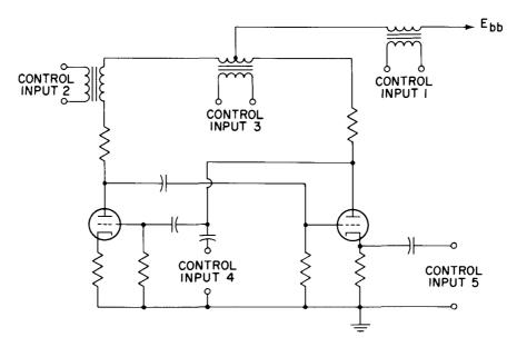
Figure 32. Five Methods of Synchronizing a Multivibrator
