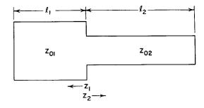
Figure 10. Resonant Circuit with Different Characteristic Impedances
