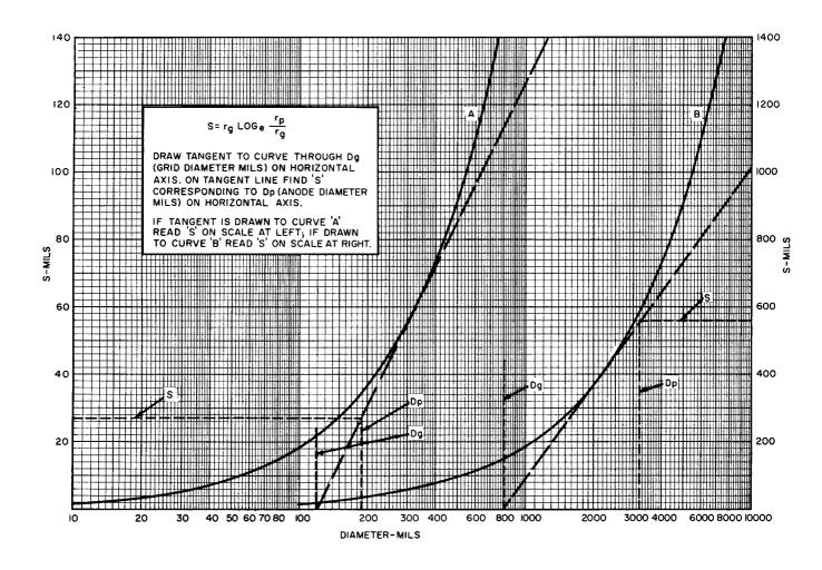
Figure 16. Amplification Factor Nomogram (Vodges & Elder Formula)
