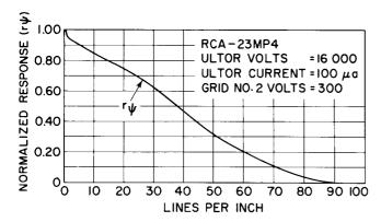
Figure 13. Sine Wave Response of RCA-23MP4
