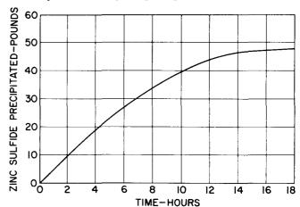
Figure 1. Rate of Precipitation of Zinc Sulfide
