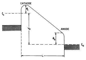
Figure 6. Potential Distribution in a Diode (no space charge)
