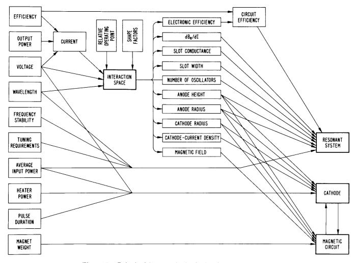
Figure 7. Principal Factors in Analysis of Magnetron Design
