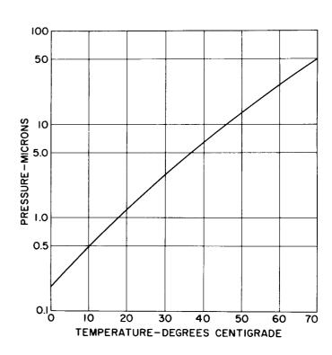
Figure 23. Vapor Pressure of Mercury
