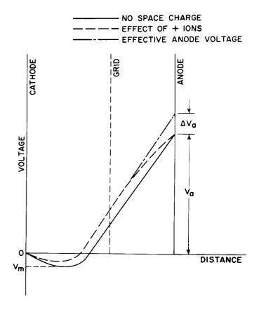
Figure 34. Axial Voltage Distribution in Thyratron Before Conduction
