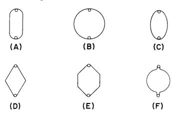
Figure 20. Common Wound-Grid Shapes: (A) flat; (B) round; (C) elliptical; (D) diamond; (E) hexagon; (F) formed round
