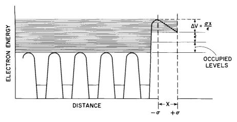
Figure 12. Energy-Level Diagram Showing Reduction of the Work Function of a Metal by Building a Dipole
