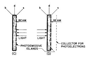
Figure 1. Camera Tube Targets: (A) Image Orthicon or Isocon; (B) Vidicons; (C) Iconoscope; (D) Orthicon (b = backplate electrode; d = dielectric; s = storage surface)
