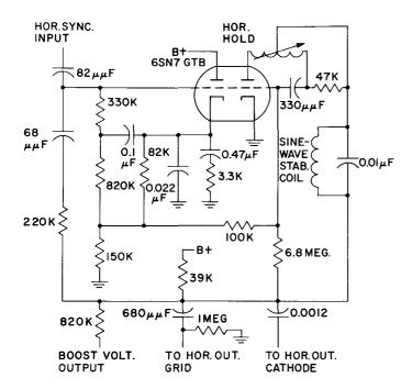
Figure 3. Compensation Used in Synchro-Guide Circuit
