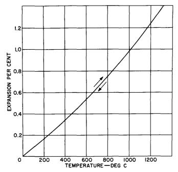
Figure 15. Expansion of Cubic (Stabilized) Zirconia as a Function of Temperature
