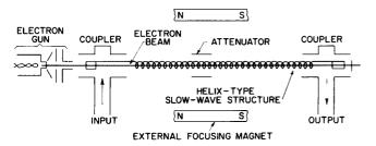
Figure 2. Basic Elements of a Traveling-Wave Tube
