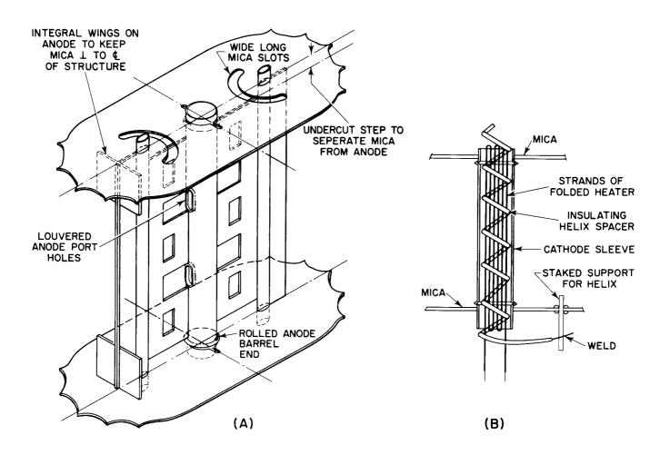
Figure 46. Constructional Details of Damper Diode (6DE4 and 6AU4-GTA): (A) plate and mica assembly, (B) cutaway cathode showing position of helix-insulating spacer and heater
