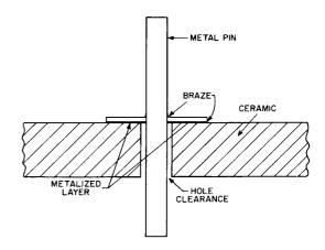
Figure 15. A Typical Pin Seal Design
