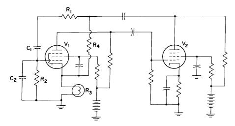
Figure 23. Practical Form of RC-Oscillator Circuit
