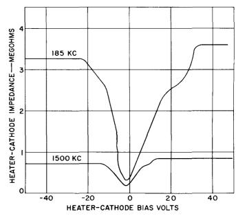
Figure 15. Typical Frequency Effects on Heater-Cathode Impedance
