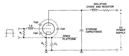
Figure 13. Equivalent Circuit for Hard-Tube Modulator
