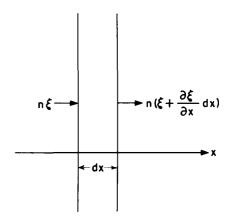
Figure 19. Charge Displacement in an Electron Plasma
