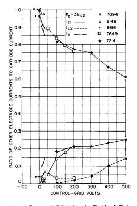
Figure 17. Current Division in Typical Tetrodes
