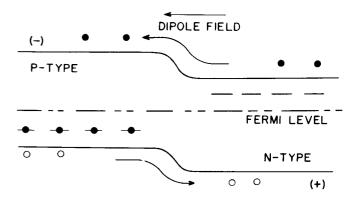
Figure 7. P-N Junction Band Diagram
