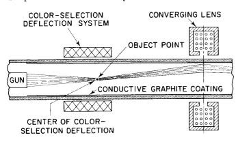
Figure 6. Single-Beam Arrangement for use With Direction-Sensitive Screen (gun end of tube)
