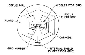
Figure 7. Schematic Cross-Section of the 6AR8
