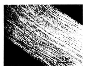
Figure 6. Typical Fibrous Structure of Tungsten Before Recrystallization (The structure of molybdenum is similar)
