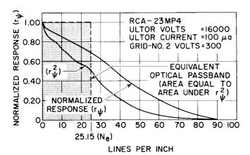
Figure 14. Equivalent Optical Passband of RCA-23MP4
