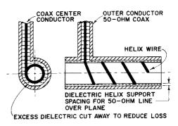
Figure 52. Cross Section of a Coupled-Helix Coupler
