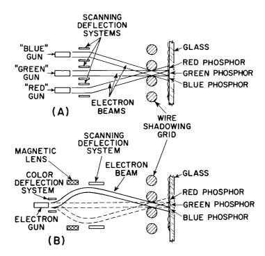
Figure 13. Early Proposal for Line-Structure Shadow-Mask Tubes
