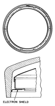
Figure 36. Electron-Masking Shield
