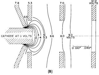
Figure 29. A Typical Low-Noise Electron Gun:
