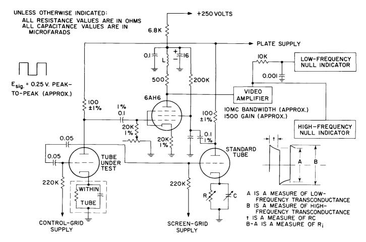
Figure 14. Shipley-Method Test Circuit
