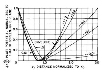
Figure 2. Potential Distribution Curves, Type B
