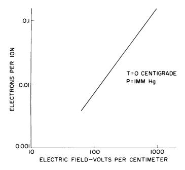
Figure 7. Secondary Ion Emission
