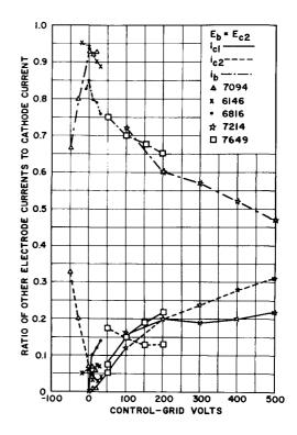
Figure 15. Current Division in Typical Tetrodes
