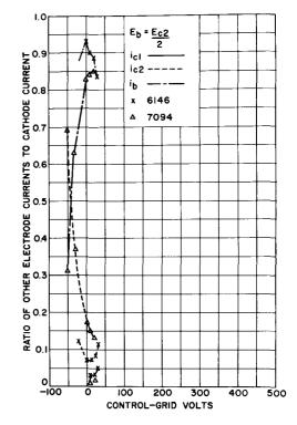
Figure 14. Current Division in Typical Tetrodes
