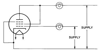
Figure 8. Two-Lamp Pentode Aging Circuit
