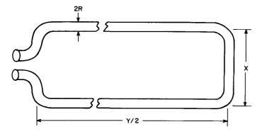
Figure 14. Rectangular Loopformed from Round Wire
