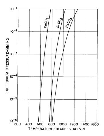
Figure 16. Equilibrium Pressures of the Alkaline-Earth Carbonates
