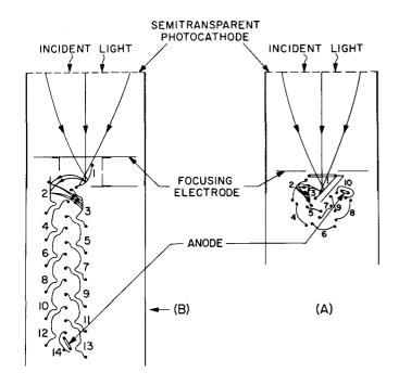
Figure 4. Electrostatically Focused Multipliers: (A) circular multiplier structure used in RCA 6655; (B) in-line multiplier structure used in RCA 6810A
