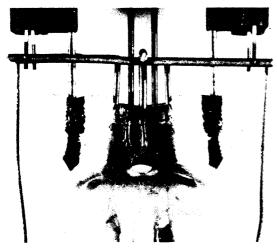
Figure 4. Electrolyzed Stem of Heavy-Duty Rectifier Tube
