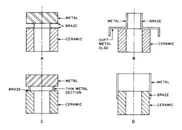
Figure 14. Various Types of Flexible Seals
