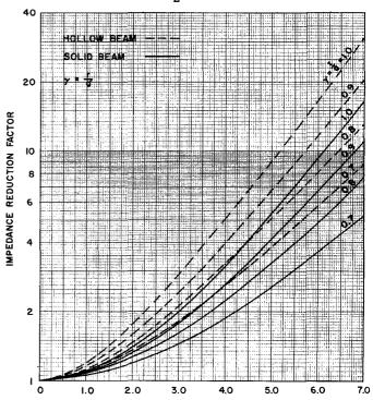
Figure 16. Family of Curves Relating the Impedance-Reduction Factor to  $^{\gamma}$  a for Several Hollow and Solid Beams with Different Radii. This factor is used to modify the impedance on the axis for solid or hollow electron beams.
