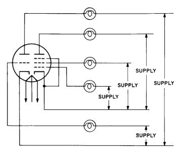
Figure 6. Triode-Pentode Aging Circuit
