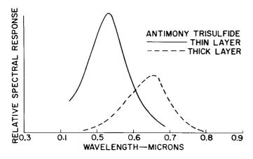
Figure 12. Variation of Spectral Response with Film Thickness
