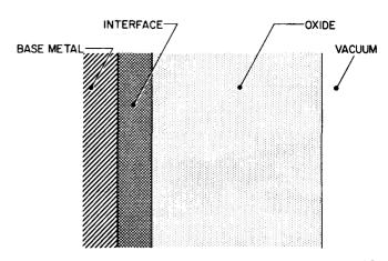
Figure 5. Diagram of Oxide Cathodc with Interface  $^{12}$
