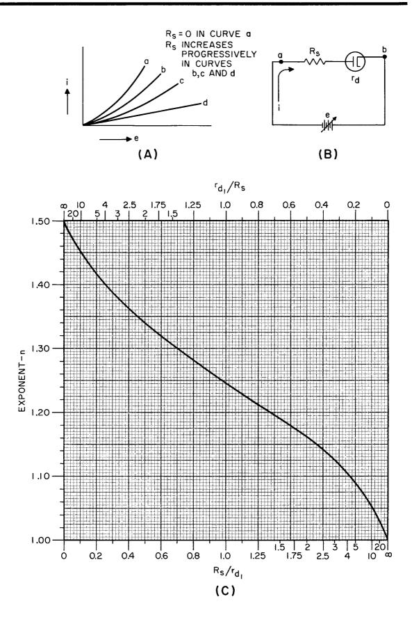
Figure 7. Effect on Diode of Adding Series Resistance  $R_s$ : (A) qualitative relation between current and voltage as  $R_s$  is increased, (B) circuit defining equivalent resistance R at terminals (a, b), (C) value of exponent n as function of  $R_s/r_{d\,1}$  or  $r_{d\,1}/R_s$
