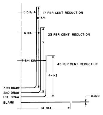
Figure 7. Analysis of Redrawing Operations
