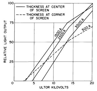
Figure 25. Effect of Aluminum Thickness on Light Output
