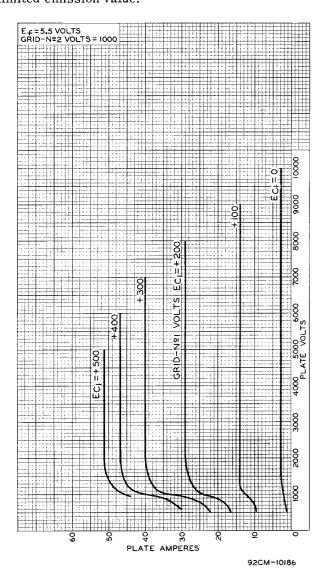
Figure 30. Typical Plate Characteristics for 7214 Beam Power Tube
