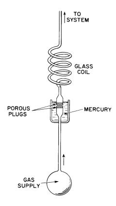
Figure 21. Porous Plug Valve
