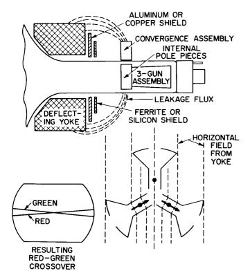
Figure 41. Red-Green Crossover Pattern Caused by Unshielded Pole Pieces
