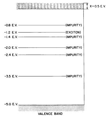
Figure 4. Energy-Level Structure of Oxide Cathode 10
