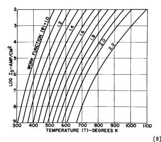
Figure 1. Saturated Emission Current  $I_S$  as a Function of Emitter Temperature and Work Function [Eq. (3a)]:
