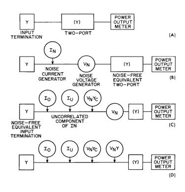
Figure 11. Equivalent Noise Generators
