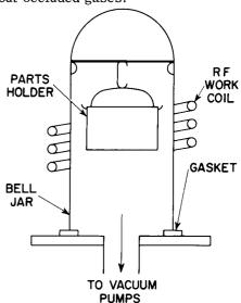
Figure 29. Vacuum Firing (rf induction heating)
