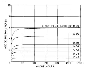
Figure 7. Anode Characteristics of a Vacuum Phototube (type 934)
