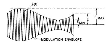
Figure 1. Amplitude-Modulated Carrier
