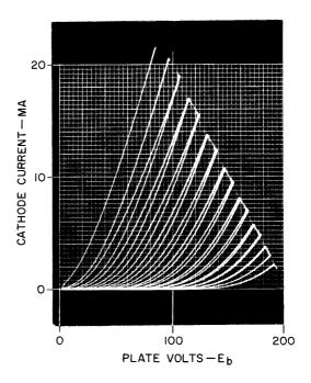
Figure 39. Double-Exposure Photograph Illustrating Change of (V, I) Characteristic of a Close-Spaced Triode (Nuvistor) Caused by a Change of Cathode Temperature  $\Delta T = -200~\rm K$ . The lower temperature shifts the first zero-bias line to lower currents, corresponding to the third bias line ( $\Delta E_c = -0.4~\rm v$ ) of the higher-temperature characteristic.
