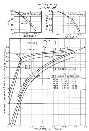
Figure 9. Diode Current I and Conductance g for d=2.5 Milliinches,  $\psi_C=1.6$  as Functions of V and T. (Insets show change of current (I/I<sub>1100</sub>) and conductance (g/g<sub>1100</sub>) from initial values I<sub>1100</sub>, g<sub>1100</sub> obtained with fixed electrode potentials at T=1100 K when T is reduced to 900 K.)
