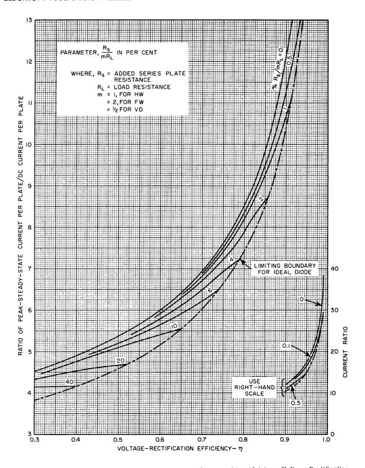
Figure 33. Current Ratio (peak steady-state current to dc-current per plate) vs. Voltage-Rectification Efficiency for Rectifiers with High-Input-Capacitance Filter, Parameter  $R_{\rm S}/mR_{\rm L}$
