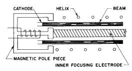
Figure 45. Cross Section of the Electron-Gun and Helix Regions of a Typical Harris-Flow-Focused Traveling-Wave Tube
