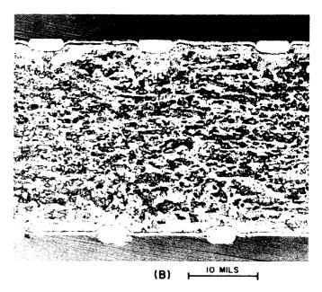
Figure 23. Longitudinal Sections of Grid Side Rods at Lateral Wire Connections: (A) lathe-wound grid; (B) welded grid
