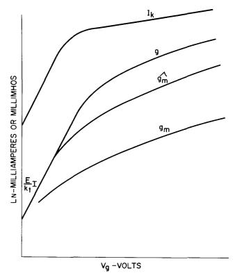
Figure 20. Typical Plot g,  $\widehat{gm}$ , gm, and  $I_K$  vs.  $V_g$
