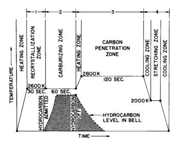
Figure 7. Typical Cycle for Carburizing
