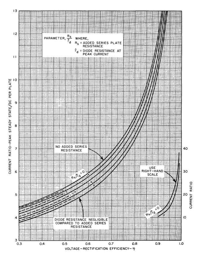
Figure 32. Current Ratio (peak steady-state current to dc-current per plate) vs. Voltage-Rectification Efficiency for Rectifiers with High-Input-Capacitance Filter, Parameter  $R_{\rm S}/\hat{r}_{\rm d}$
