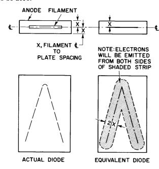
Figure 2. Effective Cathode Area of a Filament-Type Diode
