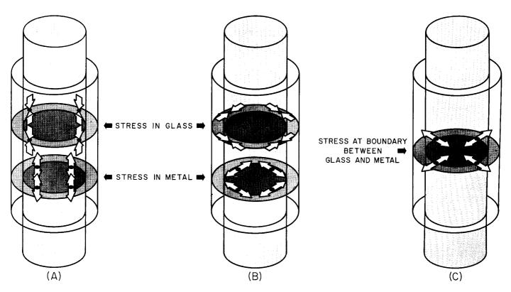
Figure 29. Stresses at Room Temperature in a Lead Seal Due to Differential Contraction of Metal Lead Wire and Glass Stem (coefficient of thermal expansion of metal higher than that of glass): (A) longitudinal stresses; (B) tangential stresses; (C) radial stresses
