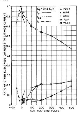
Figure 16. Current Division in Typical Tetrodes
