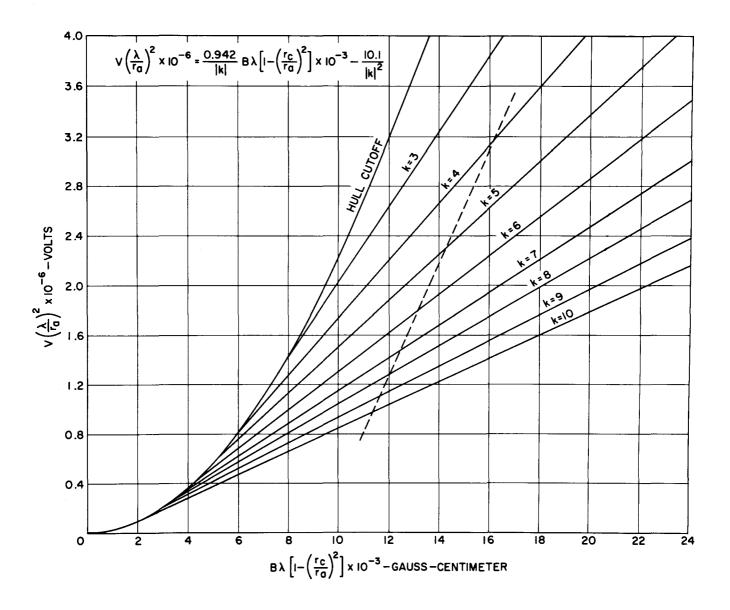
Figure 15. Universal (Generalized) Hartree Diagram
