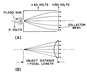
Figure 8. Simplified Collimating System (A) and its Optical Analog (B)
