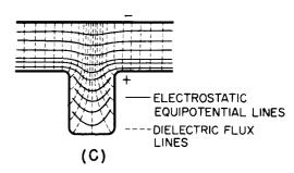
Figure 34. Typical Field Patterns: (A) Electrostatic field between oppositely charged corner and plane; (B) Electrostatic field at a charged corner (all other charges assumed at "infinite" distance away); (C) Electrostatic field between oppositely charged slot and plane
