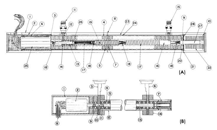
Figure 35. Cross-Sectional Drawings Showing the Arrangement of a PPM Stack in a Helix-Type Traveling-Wave Tube: (A) Tube using helical couplers; (B) Tube using waveguide couplers
