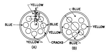
Figure 5. Strain Patterns and Cracks in Button Stems (colors are those obtained with first-order red-tint plates, standard RCA orientation); (A) Radial tension pattern (radial tension type crack. Letters show standard polarimeter measuring — points per Standardizing Notice 34-37-12A); (B) Radial compression pattern (Tangential tension type crack, often called a radial compression crack)
