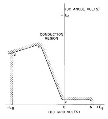
Figure 32. Thyratron Control Characteristic
