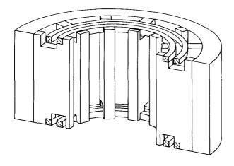
Figure 16. Double-Ring Strapped-Anode Block (Section)
