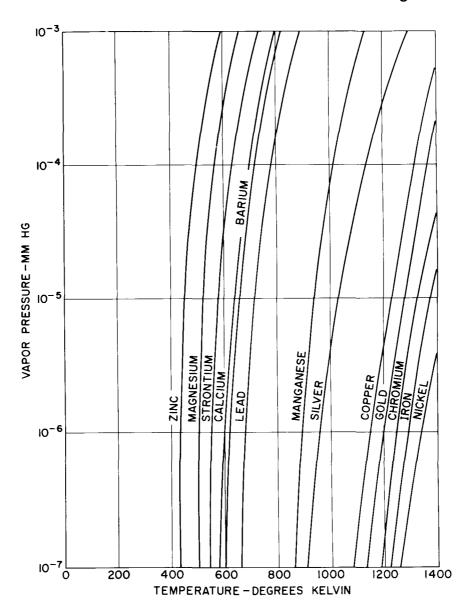
Figure 15. Vapor-Pressure Curves for Some Elements 52
