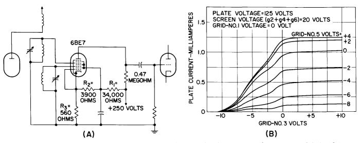
Figure 18. The  $\phi$ -Detector Tube 6BE7: (A) a typical circuit for the 6BE7 as a frequency-modulation detector using inductive coupling between the two quadrature grids: (B) typical transfer characteristics of the 6BE7
