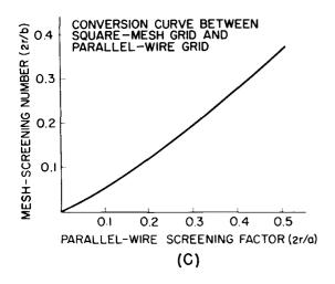
Figure 17. Relations between Helical and Mesh Grids:
