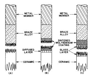
Figure 6. Failure Points in Ceramic-to-Metal Seals
