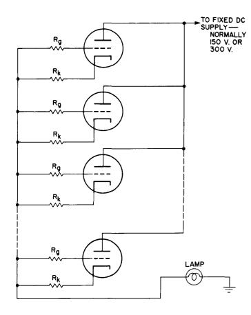
Figure 16. Ten-Tube Stabilization Circuit Showing Cathode Bias Resistors
