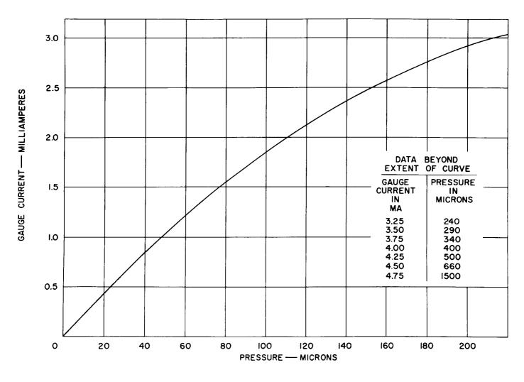
Figure 1. Pirani Gauge Calibration Curve for Dry Air (RCA 1947).
