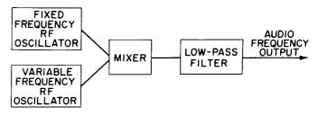
Figure 22. Block Diagram of Beat-Frequency Oscillator in Audio Frequency Range
