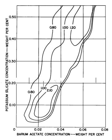
Figure 2. Contour Diagram of Adherence as a Function of Silicate and Acetate Concentration
