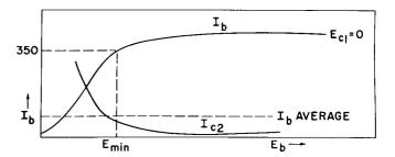
Figure 8. Zero-Bias Characteristics of the Horizontal-Output Beam Power Pentode. Energy which Is Dissipated in the Plate of the Tube Is  $I_b$  Average x  $E_{min}$
