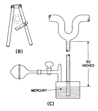
Figure 26. Vacuum Valves: (A) bellows; (B) pinch; (C) mercury
