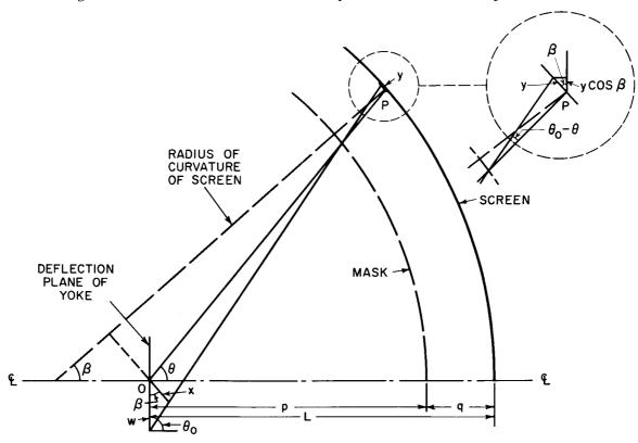
Figure 19. Geometry of Trio Distortions (plane containing tube axis)
