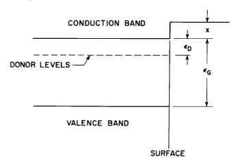
Figure 10. Conventional Energy-Level Diagram for a Solid
