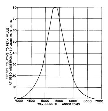
Figure 8. The Spectral Emission Curve of ZnCdS:Cu (Z-601)
