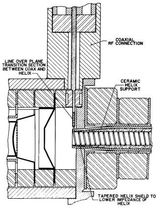
Figure 47. Cross-Sectional Diagram Showing the Direct-Coupling Method of Coupling RF Energy to the Helix
