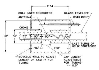
Figure 48. Cross Section of the Cavity Coupler Used in the RCA-6861 Traveling-Wave Tube
