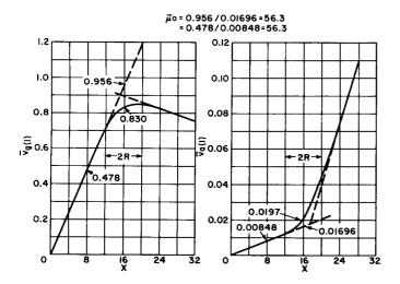
Figure 22. Mean Potentials  $\overline{v}_{g(1)}$  and  $\overline{v}_{a(1)}$  (From Table V) as Functions of x
