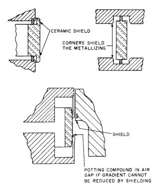
Figure 37. Shields Used for Corona Suppression
