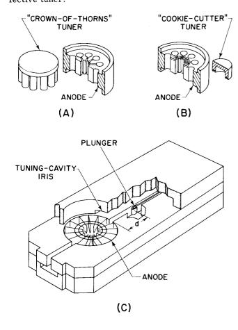
Figure 20. Magnetron Tuning: (A) Crown-of-thorns inductive tuning element and anode; (B) Cookie-cutter capacitive tuning element and strapped anode; (C) Single-cavity tunable magnetron
