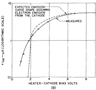
Figure 19. Typical  $^{+1}HK$  Heater-Cathode Leakage Characteristics Obtained by Pulse Measurements on Heaters That Were Unipotential During Measurement ( $E_f = 5.5 \text{ volts}$ )
