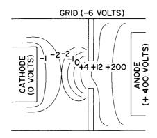
Figure 33. Equipotential Lines in Thyratron Before Conduction
