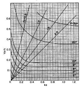
Figure 10. Family of Curves Showing the Phase Velocity of the Helix  $v_{\rm p}/c$  as a Function of ka for Several Values of the Helix Pitch Angle  $\psi$ . Lines of Constant  $\gamma_a$  are Included for Reference.
