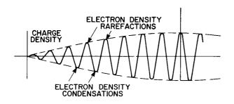
Figure 10. Model Depicting Build-Up of Space-Charge Waves
