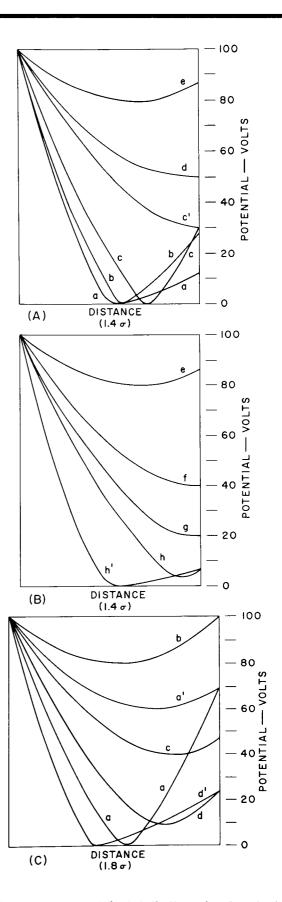
Figure 4. Potential Distributions for Constant Injected Current: (A) sequence of increasing plate voltages — 1.4 $\sigma$ ; (B) sequence of decreasing plate voltages — 1.4 $\sigma$ ; (C) distributions with spacing of 1.8 $\sigma$
