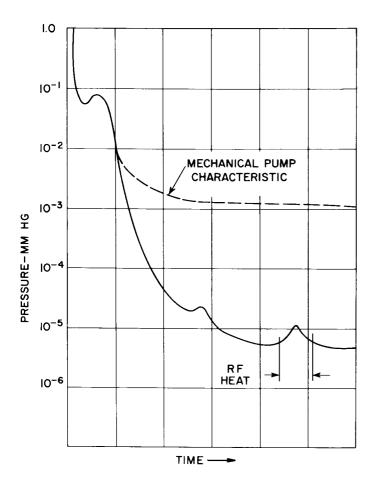
Figure 17. Representative Time-Pressure Curve
