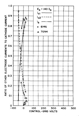
Figure 13. Current Division in Typical Tetrodes
