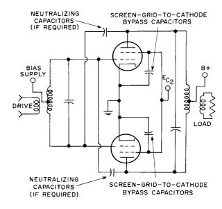
Figure 19. Push-Pull Grid-Driven Tetrode Amplifier
