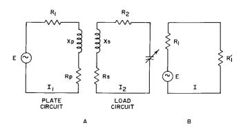
Figure 6. (A) Efficiency of Coupled Circuits; (B) Maximum Power Transfer Circuit
