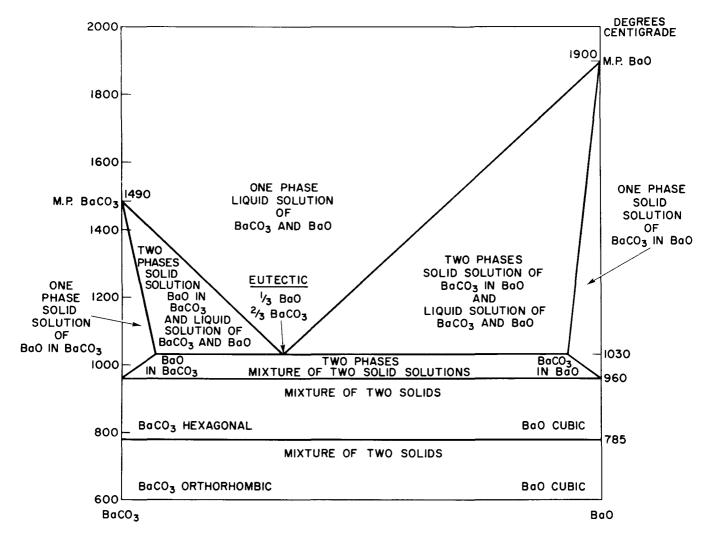
Figure 10. Phase Diagram for Barium Carbonate-Barium Oxide
