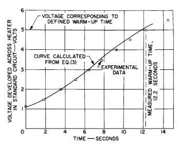
Figure 7. Calculated and Measured Warm-Up Time Characteristics of a 6AU6 Type Miniature in the Standard Heater Warm-Up Circuit
