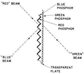
Figure 8. Direction-Sensitive Screen Having Prismatic Surface Elements
