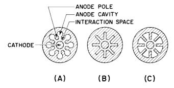
Figure 2. Typical Unstrapped Resonant Systems for Traveling-Wave Magnetron Oscillators: (A) With hole-and-slot-type side resonators, (B) With slot-type side resonators
