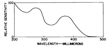
Figure 4. Photosensitivity of PVA-Ammonium Dichromate Film
