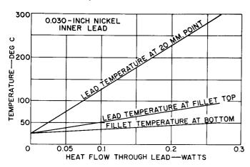
Figure 24. Stem Heat-Flow Characteristics for 1-1/4-Inch Button with Nickel Inner Leads
