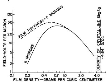
Figure 14. Electric Field Required to Support a Dark Current of 0.07 Microamperes per Cubic Centimeter Plotted Against Density of the Photolayer
