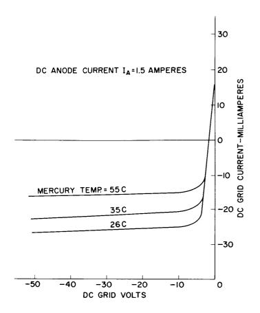
Figure 40. Grid Characteristic at Several Pressures
