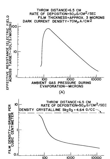
Figure 9. Effects of Pressure: (A) Effective resistance vs. gas pressure during evaporation (B) Film density vs. gas pressure during evaporation
