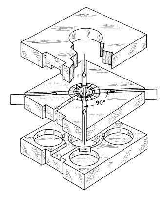
Figure 23. Magnetron with Four Tuning Cavities
