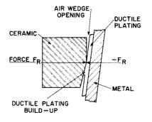
Figure 1. Radial Compression Seal
