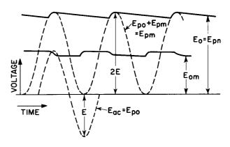
Figure 40. Half-Wave Voltage-Doubler Rectifier and Voltage Waveshapes
