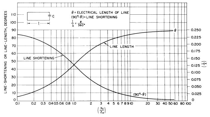
Figure 26. Curves for Computation of Transmission-Line Length
