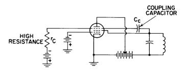
Figure 13. Circuit for Transitron, A Negative-Transconductance Oscillator
