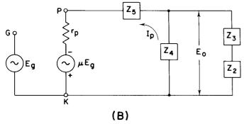
Figure 9. (A) Feedback amplifier, (B) Equivalent circuit with feedback tap omitted
