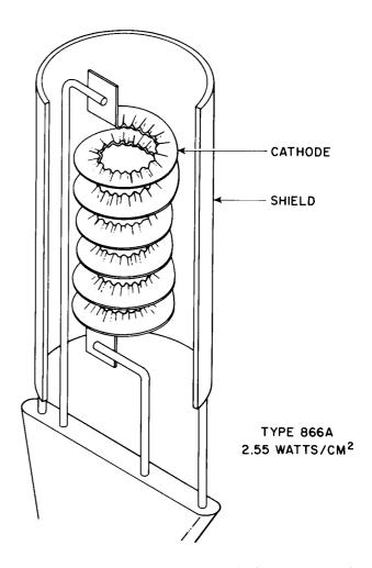
Figure 18. Directly Heated Cathode Structure of Type 866A
