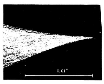
Figure 3. Typical "Pinch Off" Showing Thin Edge at End of Separation
