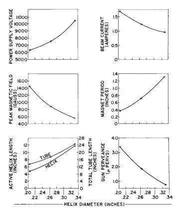
Figure A1. Design Parameters as Functions of Helix Diamater
