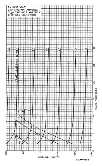
Figure 32. Constant-Current Curves for 6952 Beam Power Tube
