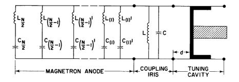
Figure 21. Equivalent Circuit for a Single-Cavity Tunable Magnetron
