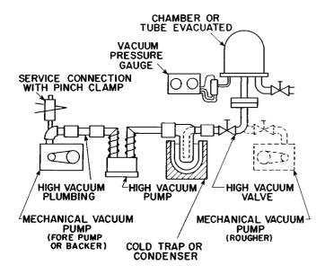
Figure 2. Vacuum System Schematic Diagram
