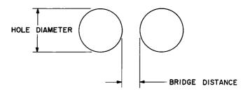
Figure 4. Bridge Between Two Round Holes
