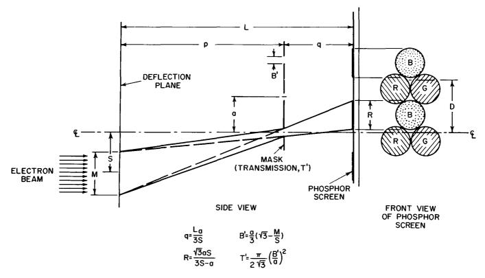
Figure 16. Shadow-Mask Design Parameters
