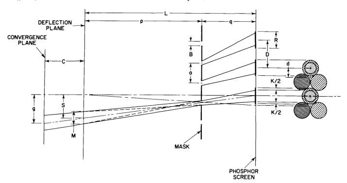
Figure 47. Tube Geometry
