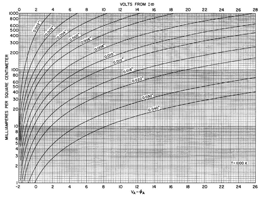
Figure 11. Plot of J vs. V with d as a Parameter
