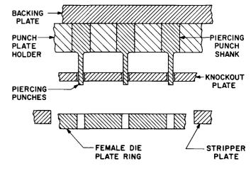
Figure 3. Cross Section of a Compound Die
