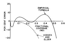
Figure 20. Correction Factors for Determination of Amplification Factor
