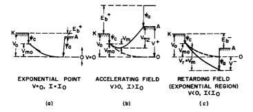
Figure 3. Effective Diode Potential  $V^{\pm}$ : (A) reference condition V=0, exponential point dv/dx=0,  $I=I_0$ ; (B) accelerating fields V>0, dv/dx positive,  $I>I_0$ ; (C) retarding fields V<0, dv/dx negative,  $I<I_0$
