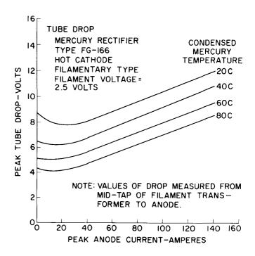
Figure 24. Tube Drop vs. Condensed Mercury Temperature
