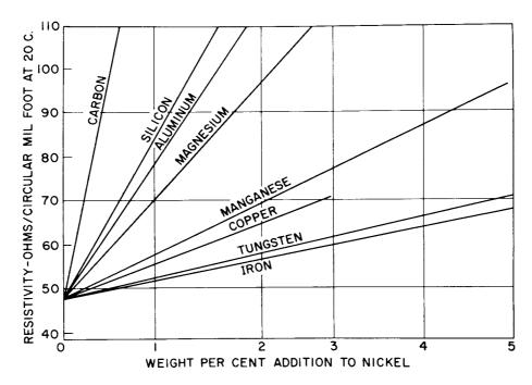
Figure 3. Effects of Various Additives on the Resistivity of Nickel (aluminum and tungsten by C. W. Horsting; all others by E. M. Wise and R. H. Schaefer<sup>6</sup>)
