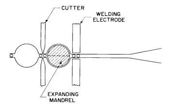
Figure 21. The Welded-Grid Process
