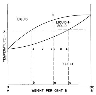
Figure 8. Phase Diagram of Two Mutually Soluble Elements
