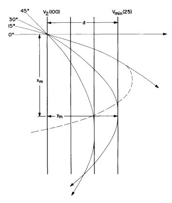
Figure 9. Electron Trajectories in Linear Retarding Field
