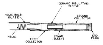
Figure 56. Cross Section of a Two-Stage Collector Assembly
