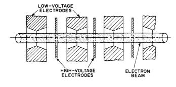
Figure 44. Electrostatically-Focused Folded-Waveguide Slow-Wave Structure: (A) Comparison of the ideal and actual shape of the focusing field; (B) Cross section of the structure
