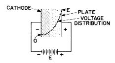
Figure 7. Effect of Voltage on Electron Distribution
