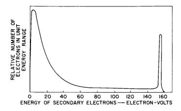
Figure 5. Velocity Distribution of Secondary Electrons
