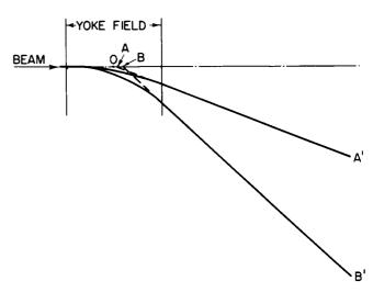
Figure 22. Forward Motion of Deflection Center With Increasing Deflection Angle
