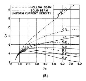
Figure 14. Effect of Beam Size and  $\gamma_a$  on Beam Impedance: (A) Showing that the amplitude of the axial component of the electric field on the axis of the helix (E<sub>Z</sub>) varies as a function of  $\gamma_a$ ; (B) CN as a function of  $\gamma_a$  for several solid and hollow beams of different radii. CN is very nearly proportional to gain; thus, the curves show the variation of gain with frequency.
