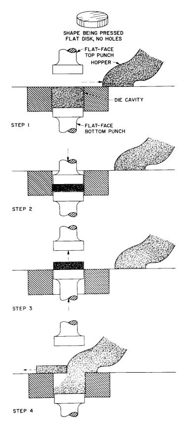
Figure 2. Steps in Pressing a Flat Disk
