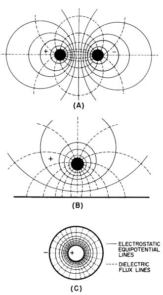
Figure 33. Fundamental Field Patterns: (A) Electrostatic field pattern between two oppositely charged parallel cylinders; (B) Electrostatic field pattern between oppositely charged plane and cylinder; (C) Electrostatic field pattern between oppositely charged concentric cylinders
