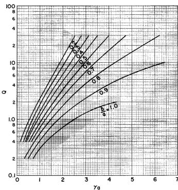
Figure 5. Family of Curves Showing the Passive-Mode Parameter Q as a Function of  $\gamma_a$  for Different Ratios of the Radius of the Electron Beam to the Radius of the Slow-Wave Circuit (b/a): (A) For a solid beam; (B) For a hollow beam
