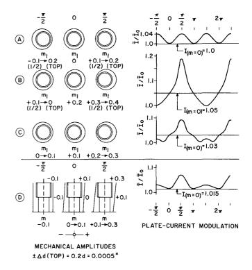
Figure 20. Vibration-Induced Current Modulation  $\bar{l}/\bar{l}_0$  in a Nuvistor Triode; Relative Vibration Amplitude  $m_{1max} = \pm \ 0.1$  at half length of grid, =  $\pm \ 0.2$  at top of grid: (A) coaxial structure; (B) uniform eccentricity ( $m_1$  zero = 0.2); (C) uniform eccentricity ( $m_1$  zero = 0.1); (D) tilted eccentricity
