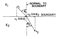
Figure 6. Electron Refraction
