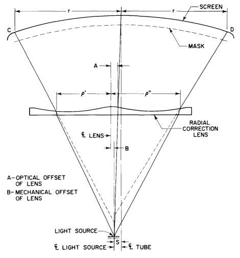
Figure 24. Diagram of "Crowding" Reduction by Use of Lens Offset
