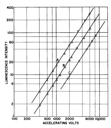
Figure 12. Variation of Cathodoluminescence with Electron Accelerating Potential for a Zn<sub>2</sub>Si0<sub>4</sub>--Mn Phosphor Excitation current density: curve A, 5 µA/cm<sup>2</sup>; curve B, 100 µA/cm<sup>2</sup>; curve C, 550 µA/cm<sup>2</sup>
