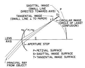
Figure 12. Convergent Refracting Surface Afflicted with Positive Astigmatism (An object off the axis but in the plane of the paper is imaged by rays in the plane of the paper at a shorter distance from the lens than by rays in the plane containing the principal ray but perpendicular to the plane of the paper.)
