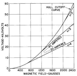
Figure 11. Hartree Diagram for an 8-Resonator Magnetron
