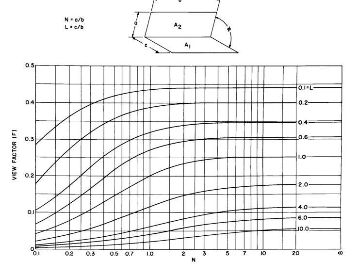
Figure 12. View Factor for Direct Radiation Between Adjacent Rectangles (Ø = 90°)
