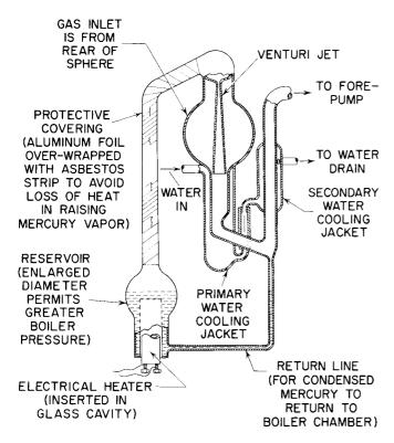
Figure 21. Glass Mercury Pump
