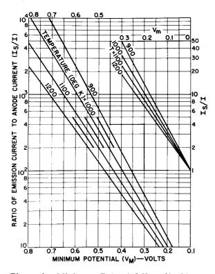
Figure 8. Minimum Potential  $V_m = f(I_S/I)$
