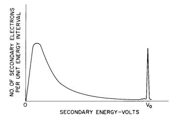
Figure 17. Typical Energy Distribution Curve of Secondary Electrons
