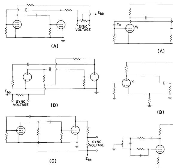
Figure 33. Circuits for Synchronizing to Submultiples of the Control Frequency; (A) Circuit favoring odd value of n; (B) Circuit favoring even value of n; (C) Circuit favoring any value of n
