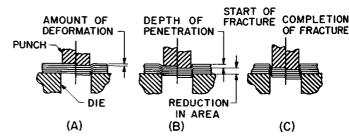
Figure 2. The Shearing of Metal: (A) plastic deformation, (B) reduction in area, (C) fracture
