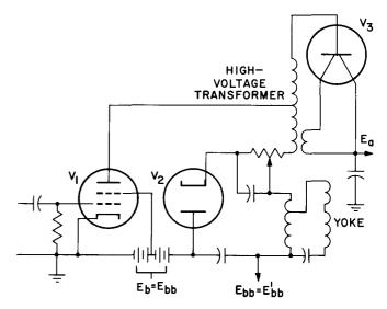
Figure 7. Simplified Horizontal-Deflection Circuit. V<sub>1</sub> Is the Horizontal Output Beam Power Pentode. V<sub>2</sub> Is the Damper Diode. V<sub>3</sub> Is the High-Voltage Rectifier which Rectifies the High-Voltage Pulses from the High End of the High-Voltage Turns and Supplies the Kinescope with its Anode Voltage. E'bb is the Boosted Voltage Developed which Is Higher than the Supply Voltage Ebb
