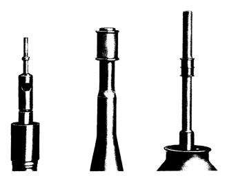
Figure 25. Typical Magnetron Cathodes
