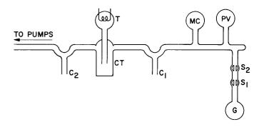
Figure 4. Apparatus for determining Getter Efficiency (G-gas bottle; S<sub>1</sub>, S<sub>2</sub>—stopcocks; PVsystem reservoir; MC-McCleod gauge; C<sub>1</sub>, C<sub>2</sub> cutoffs; CT-cold trap; T-tube containing test getter)
