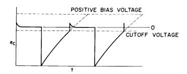
Figure 31. Grid-Voltage Waveform for Circuit in Figure 28B
