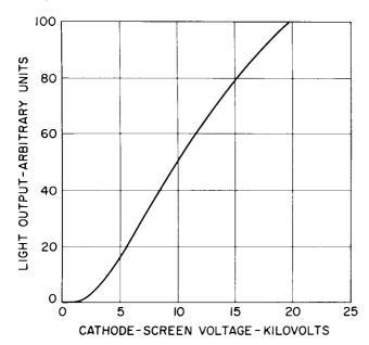
Figure 1. Light Output-vs-Voltage Characteristics of P-20 Screen
