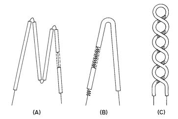
Figure 9. Heater Types Used in Electron Tubes: (A) folded heater; (B) folded single-helical (hairpin) heater; (C) double-helical heater
