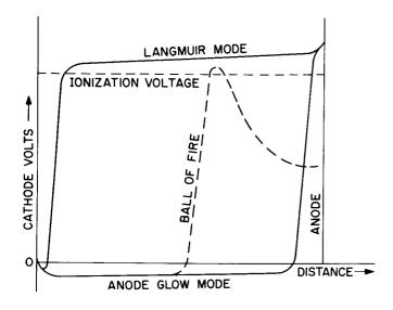
Figure 11. Voltage vs. Distance
