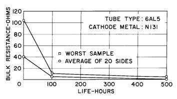
Figure 9. Variation of Cathode Bulk Resistance with Life
