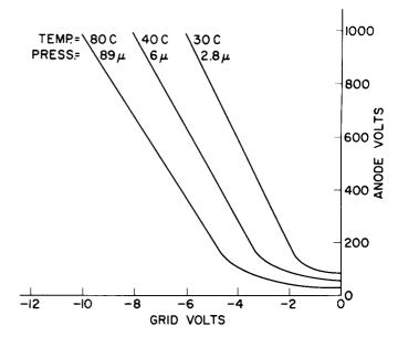
Figure 35. Control Characteristic of Thyratron at Different Pressures
