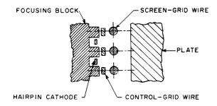
Figure 28. Beam Tetrode Configuration Used in 8D21
