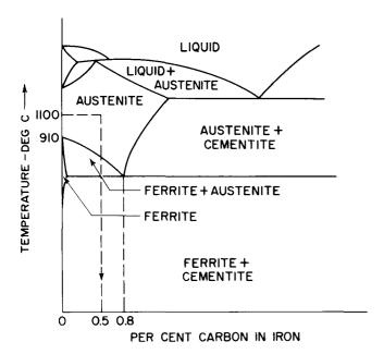
Figure 13. The Iron-Rich Corner of the Iron-Carbon Phase Diagram
