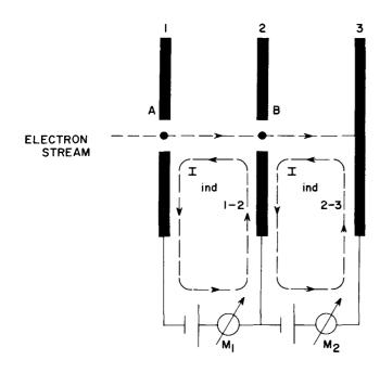
Figure 12. Electron-Induced Currents in a Three-Electrode System
