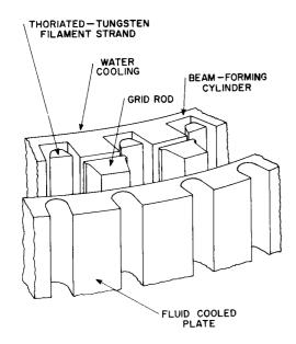
Figure 24. Unit Triode Systems Used in 5831 Beam Triode
