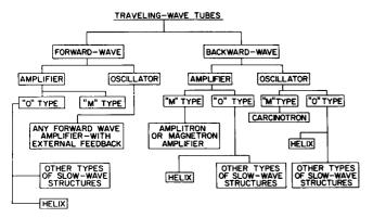
Figure 1. The Various Types of Traveling-Wave Tubes are Divided into Two Basic Classes:
