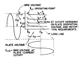
Figure 2. Constant-Current Curves for Typical Amplifier Load Condition
