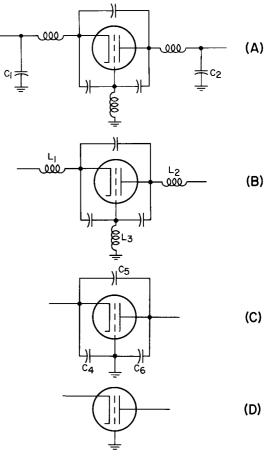
Figure 13. Correction for Lead Inductances and Capacitances
