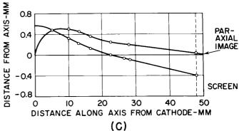
Figure 10. Potential Plot and Electron Paths of Monovoltage Image Tube: (A) developmental type C73413A image tube, (B) axial potential distribution, (C) calculated electron paths, using Gans' method
