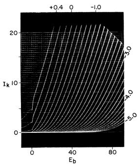
Figure 38. Double-Exposure Photograph of (V, I) Characteristics of a Nuvistor Triode Obtained by Interlacing Grid-Bias Lines
