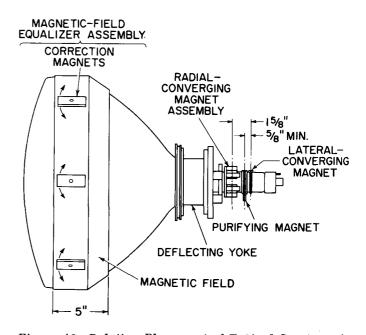
Figure 40. Relative Placement of Typical Components on 21CYP22
