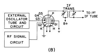
Figure 9. Use of the 6L7: (A) Relative Position of Electrodes; (B) Connection as a Mixer
