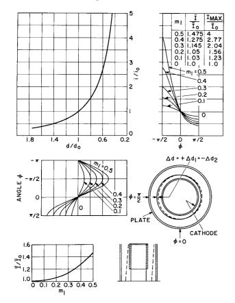
Figure 19. Graphic Evaluation of Current Change (i/i<sub>0</sub>) Caused by a Sinusoidal Variation of Spacing (d/d<sub>0</sub>) Due to Eccentric Electrodes. (Inset, left bottom: Increase of average current  $(\bar{l}/\bar{l}_0)$  as function of cathode grid eccentricity  $m_1$ .)
