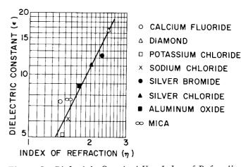
Figure 5. Dielectric Constant Vs. Index of Refraction
