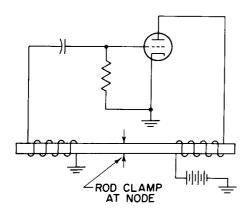
Figure 21. Typical Circuit of Magnetostriction Oscillator
