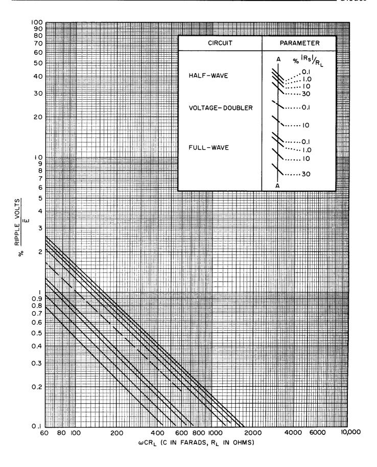
Figure 29. RMS Ripple Voltage for Capacitor-Input-Filtered Load Circuits
