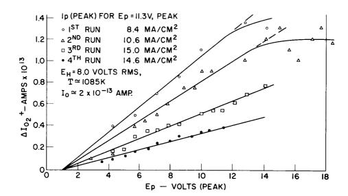
Figure 30. Oxygen Evolution from a Ba0 Cathode as a Function of Diode Voltage and Cathode Activity (The state of cathode activity for each run is noted in the table)
