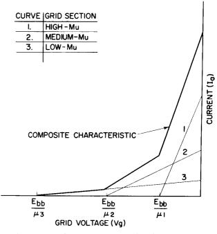
Figure 22. Composite Transfer Characteristic for Variable Mu Tube
