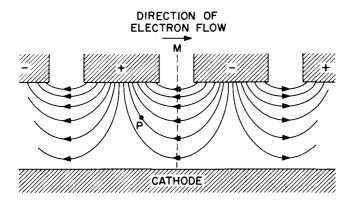
Figure 5. Phase-Focusing Effect in a Traveling-Wave Magnetron
