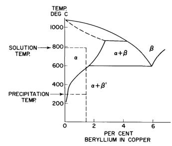
Figure 14. Beryllium Copper, an Example of Precipitation Hardening
