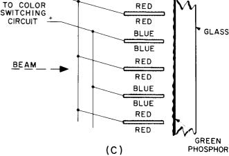
Figure 1. Color Selection by Beam Deflection Between Elementary Electrodes
