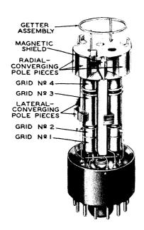
Figure 39. Three-Bead Gun Assembly
