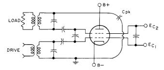
Figure 17. Cathode-Driven Tetrode Amplifier
