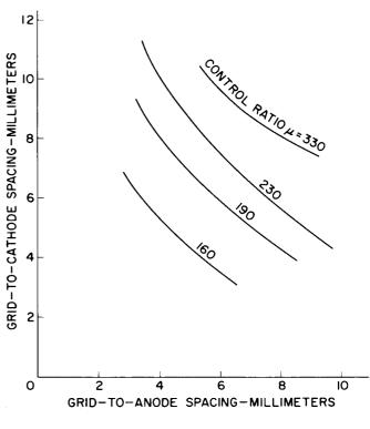
Figure 41. Control Ratio vs. Spacing
