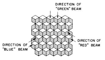
Figure 9. Direction-Sensitive Screen Having Pyramidal Surface Elements
