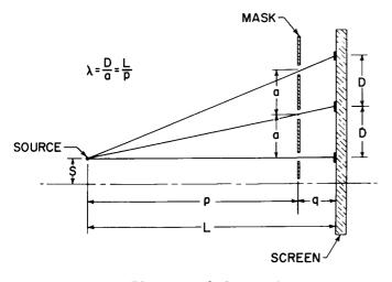
Figure 15. Planar Mask-Screen Geometry
