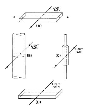
Figure 4. Examples of One-Dimensional Stress-Retardation Relation Which Can Be Determined in the Polariscope: (A) glass piece with a uniform one-dimensional stress, (B) butt seal of glass tubing, (C) bead sealed to wire, (D) tempered flat glass piece
