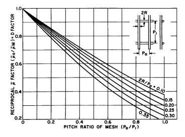
Figure 36. D Factor of Mesh Grids (See text)
