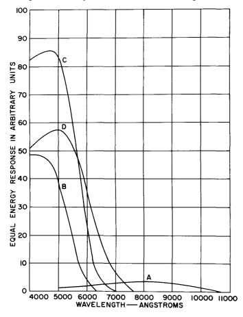
Figure 2. Spectral Sensitivity Characteristics of Various Photoemissive Materials Used as Cathodes in Phototubes: curve A, Ag-O-Cs; curve B, Sb-Cs; curve C, Sb-Cs-(0)
