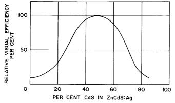
Figure 15. Relative Efficiency of a Phosphor
