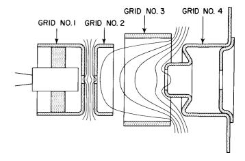
Figure 8. Low-Voltage, Electrostatic-Acceleration-Type Focusing Gun
