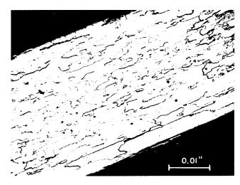
Figure 7. Tungsten Wire Heated From Recrystallization Temperature to 2600 K in 20 Seconds
