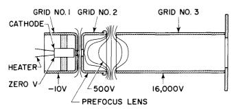
Figure 2. Magnetic-Focus, Tetrode-Type Gun
