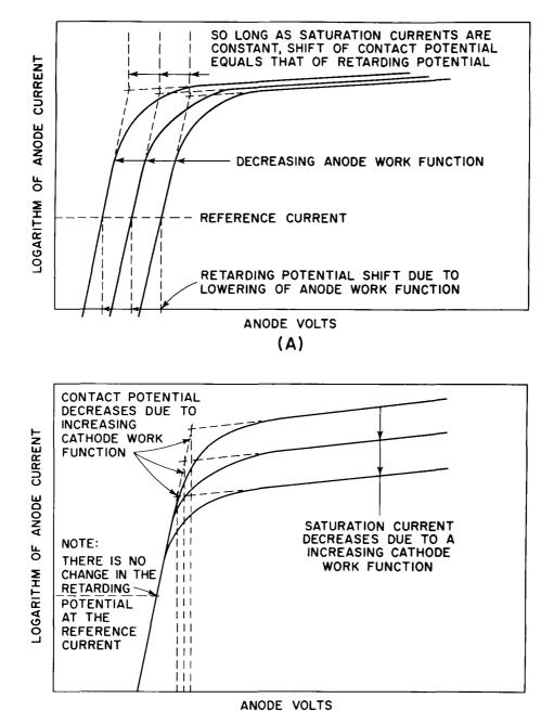
Figure 5. Effects of Work-Function Shifts: (A) illustrating the shift in the retarding potential at some reference current due to grid-work-function shifts; (B) illustrating the shift in the saturation currents due to cathodework-function shifts
