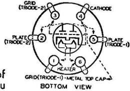
The 79 is a heater-cathode type of tube combining in one bulb two high- $\mu$  triodes designed for Class B operation. It is intended for use in the audio-output stage of radio receivers with 6.3-volt
