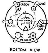
The 43 is a power-amplifier pentode of the heater-cathode type for use in the output stage of radio receivers, especially those of the "d-c power line" type and the "universal (a.c.-d.c.)" type. In such
