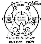
The 6C6 is a triple-grid tube of the heater-cathode type recommended for service as a biased detector in radio receivers designed for its characteristics, especially those of the mobile type employ-
