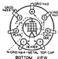
The 2A7 is a multi-electrode type of vacuum tube designed to perform simultaneously the functions of a mixer (first detector) tube and of an oscillator tube in superheterodyne circuits. Through the use
