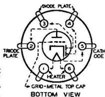
receivers designed for its characteristics. For diode-detector considerations, refer to page 19.
