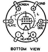
The 42 is a heater-cathode type of power-amplifier pentode for use in the audio-output stage of a-c receivers. It is capable of giving large power output with a relatively small input-signal voltage. Because of the heater-cathode construction, a uniformly low hum-level is attainable in power amplifier design.
