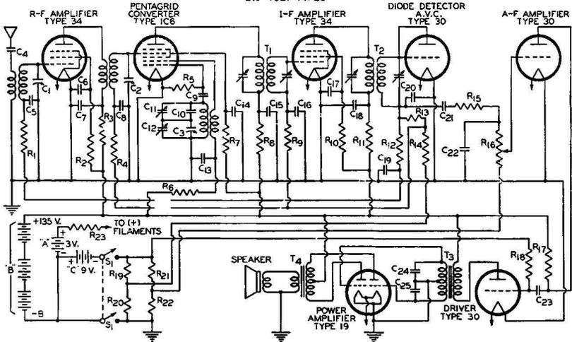
C<sub>1</sub>, C<sub>2</sub>, C<sub>3</sub> = GANGED VARIABLE CONDENSERS
