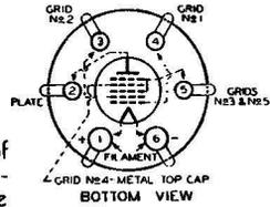
The 1A6 is a multi-electrode type of vacuum tube designed to perform simultaneously the function of a mixer tube and of an oscillator tube in superheterodyne circuits. Through its use, the inde-
