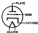
When the grid of a tube is made positive or negative with respect to the cathode, the plate current correspondingly increases or decreases. The grid is located much nearer the cathode than the plate so that a small voltage change on the grid will have the same effect on the plate current as a larger voltage change on the plate. A grid requires very little power, serving merely as a valve to control the plate current.
