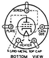
The 35 is a super-control screen grid amplifier tube of the heater-cathode type recommended as an r-f amplifier and an i-f amplifier in a-c receivers. The 35 is very effective in reducing cross-modulation
