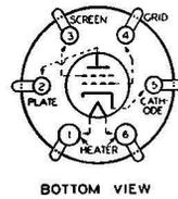
The 48 is a power-amplifier tetrode which has pentode characteristics when operated at the recommended screen and plate voltage. It is for use in the audio-output stage of receivers designed to operate from 115-volt d-c power lines. The 48 is exceptional in its ability to deliver power at the low plate and screen voltage obtainable in such service.
