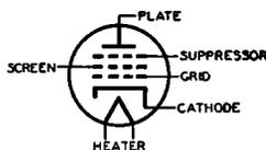
with its own base terminal. With this arrangement, it is possible to obtain special control features by variation of the voltage applied to the suppressor. Typical tubes of this type are the 57 and 58.
