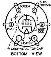
The 78 is a triple-grid super-control amplifier tube recommended for service in the radio-frequency and intermediate-frequency stages of radio receivers designed for its characteristics. The ability of
