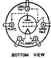
The 46 is a double-grid power-amplifier tube recommended especially for service in Class B amplifier circuits of suitable design. A pair of 46's in a Class B output stage is capable of supplying an exceptionally large amount of virtually undistorted power; while a single 46, operated in the driver stage as a Class A amplifier, can deliver sufficient power to drive the pair of 46's in the output stage.
