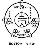
The 56 is a three-electrode tube of the heater-cathode type recommended for use as detector, amplifier, or oscillator in a-c receivers designed for it. This tube is characterized by its high mutual conduc-
