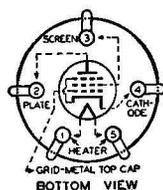
The 39/44 is a heater-cathode tube of the remote cut-off type suitable for use primarily as a radio-frequency amplifier, intermediate-frequency amplifier, and mixer in receivers designed for its characteristics. The 39/44 is effective in reducing cross-modulation and modulation-distortion over the usual range of signal voltages without the use of antenna potentiometers or auxiliary volume-control switches. An explanation of the Super-Control feature is given on page 11.
