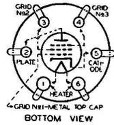
ternal connections for each grid, makes possible its application as (1) a Class A power-Amplifier Triode, (2) a Class A Power-Output Pentode, and (3) a Class B power-Output Triode.
