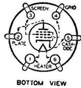
The 2A5 is a heater-cathode type of power-amplifier pentode for use in the audio-output stage of a-c receivers. It is capable of giving large power output with a relatively small input-signal voltage. Because of the heater-cathode construction, a uniformly low hum-level is attainable in power-amplifier design.
