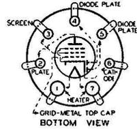
The 2B7 is a heater type of tube consisting of two diodes and a pentode in a single bulb. It is recommended for service as a combined detector, amplifier (radio-frequency, intermediate-frequency or
