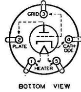
conductance and its comparatively high amplification factor. The 76 is useful in resistance-coupled audio-frequency amplifiers.
