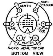
cant among its electrical features are the extended mutual conductance operating range and the adaptability of electrode combinations to various circuit applications. The ability of this tube to handle usual signal voltages without cross-modulation and modulation-distortion makes it adaptable to the r-f and i-f stages of receivers employing automatic volume-control. The 58 is constructed with an internal shield connected to the cathode within the tube.
