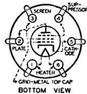
audio-frequency output voltage with relatively small input voltage. Other applications of the 77 include its use as a low-signal-input screen-grid amplifier tube and as an automatic-volume-control tube.
