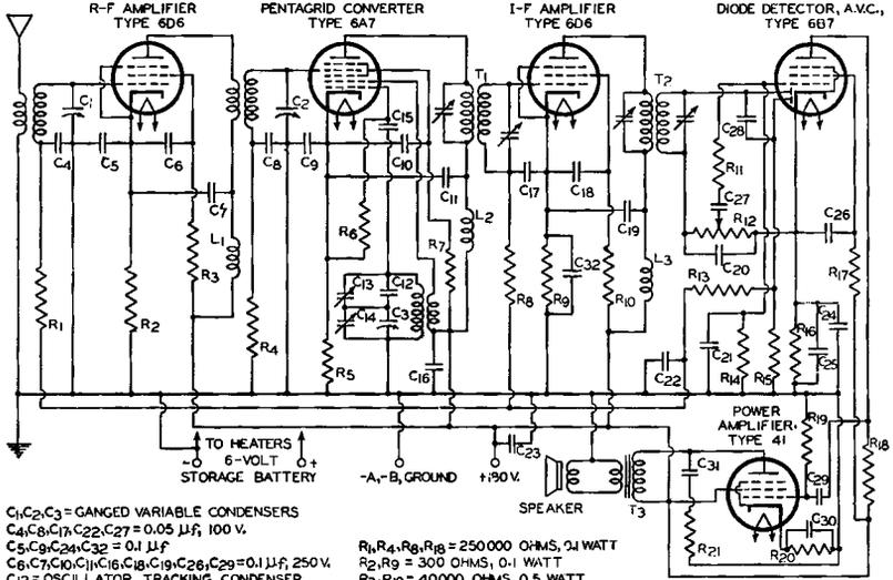
C<sub>1</sub>, C<sub>2</sub>, C<sub>3</sub> = GANGED VARIABLE CONDENSERS
