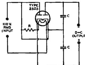
R=HEATER VOLTAGE REDUCING RESISTOR
