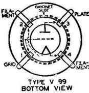
The base pins of the X99 fit the standard four-contact socket; the V99 fits only the small shell socket with bayonet slot. The sockets should be installed so that the tubes will operate in a vertical position. Cushioning of the sockets in the detector stage may be desirable if microphonic disturbances are encountered.
