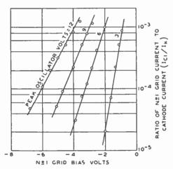
Fig. 15—Signal-grid (grid No. 1) current in a typical mixer with a 20-megacycle oscillator voltage applied to grid No. 3.  $E_{ct} = -10$  volts.  $E_{ct}$  and t = 100 volts,  $E_b = 250$  volts.
