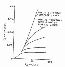
Fig. 15—Single-valued diode characteristics.
