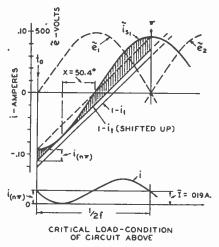
Fig. 23—Graphic solution for the critical load condition with negligible series resistance.
