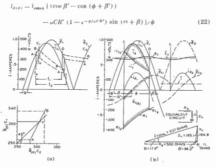
Fig. 32-Graphic solution of final operating conditions for circuit in Fig. 13.
