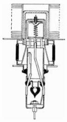
Fig. 1—Cross section of the H-2614 pulse triode.
