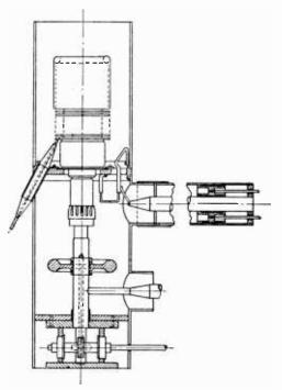
Fig. 4—Cross section of the "half-wave" oscillator circuit.
