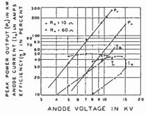
Fig. 5 — Typical pulse operating data at 600 Mc.
