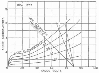
Fig. 6. Anode characteristics of 1P37.
