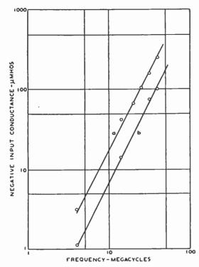
Fig. 11—Signal-grid (grid No. 4) conductance of a typical mixer designed for inner-grid injection of oscillator. Lines are drawn with slope of 2. Curve  $\alpha$  taken with  $E_{c1} = 0$ ,  $E_{c4} = -3$  volts. Curve b taken with  $E_{c1} = -6$ ,  $E_{c4} = -6$  volts.
