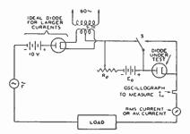
Fig. 10 — Circuit for measuring equivalent diode resistance values.
