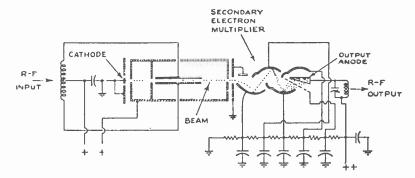
Fig. 10—Cross-sectional view of an early beam-deflection amplifier with 3-stage multipler.
