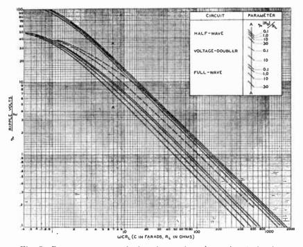
Fig. 7-Root-mean-square ripple voltage of condenser-input circuits.
