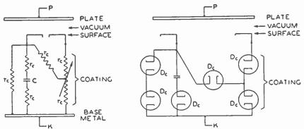
Fig. 17 — Circuit network representing the coating impedance in high-vacuum diodes.
