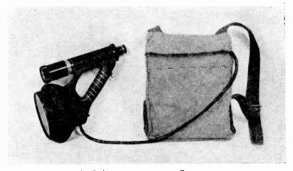
Fig. 9-Laboratory prototype Snooperscope.
