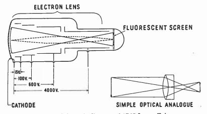
Fig. 4-Schematic diagram of 1P25 Image Tube.
