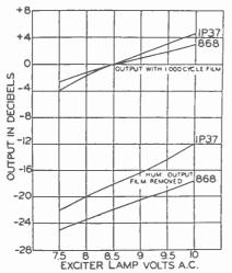
Fig. 2. Relative signal-to-hum response.
