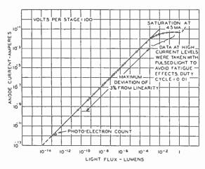
Fig. 5—Linearity characteristics of R C A photo-multipliers.
