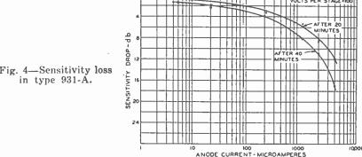
Fig. 4—Sensitivity loss
