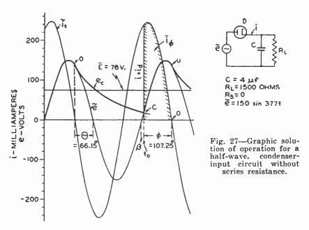
current  $\tilde{\imath}_s$  are constructed on the assumption that the diode is short-circuited. The steady-state condenser voltage  $\tilde{e}_c$  coincides with  $\tilde{e}$  because  $R_8=0$ .
