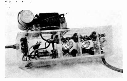
Fig. 23-16-kilovolt voltage quadrupler power supply.
