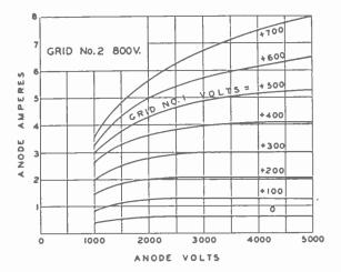
Fig. 8—Anode characteristics for each unit.
