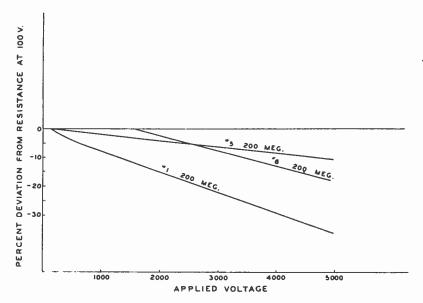
Fig. 16—Voltage characteristics of resistors.
