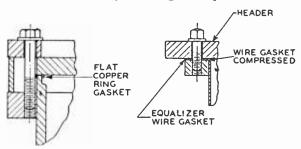
Fig. 2—Details of the copper-gasket vacuum seals.
