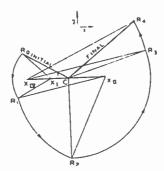
Fig. 7—The graphical construction for the transverse field of Fig. 6. The radius vector representing the initial circular motion is  $CR_{\circ}$ , its magnitude being drawn proportional to the actual radius in centimeters, determined by
