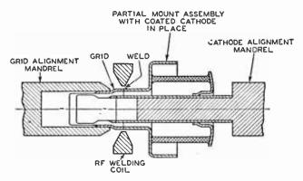
Fig. 3—Arrangement of parts for rf-welding the grid to Kovar support; cross-sectional view.
