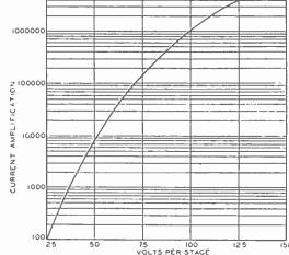
Fig. 2—Average amplification of type 931-A.
