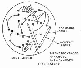
Fig. 1 — Schematic arrangement of type 931-A.
