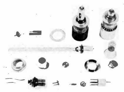
Fig. 2—Individual parts, subassemblies, and a completely assembled H-2614.
