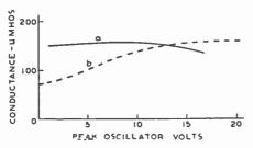
Fig. 17—Signal-grid (grid No. 1) conductance of typical mixer designed for outer-grid injection of oscillator. Frequency, 31.5 megacycles, signal-grid bias,  $E_{ci} = -3$  volts. Curve a corresponds to fixed No. 3 grid bias,  $E_{ci} = -8$  volts. Curve b corresponds to bias through a 50,000-ohm grid leak.
