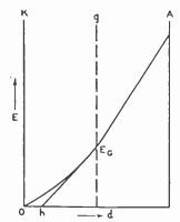
Fig. 9—Apparent location h of the cathode as seen from the grid.
