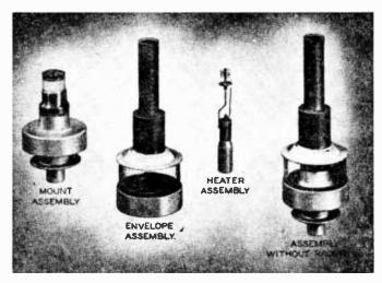
Fig. 4—Three main components and final assembly.
