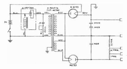
Fig. 19-Voltage doubler power supply (Type S-2).
