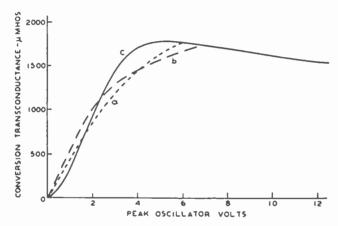
Fig. 5—Conversion transconductance of a typical variable-μ, radio-frequency pentode. Oscillator and signal voltages both applied to grid No. 1. a, fixed-bias operation; b, cathode resistor used to obtain bias; c, bias obtained by means of a high-resistance grid leak.
