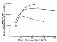
Fig. 9—Conversion transconductance of a typical mixer designed for inner-grid injection of oscillator. Signal-grid bias = -3 volts. a, fixed-bias operation of oscillator grid; b, oscillator-grid bias obtained through high-resistance grid leak; c, oscillator-grid bias obtained through a 50,000 ohm grid leak.
