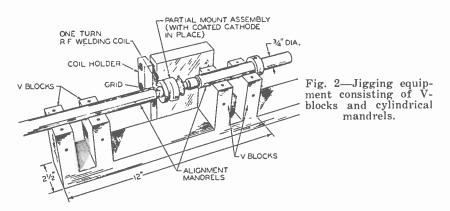
Radio-Frequency Induction Welding
