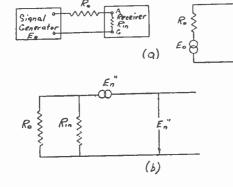
Fig. 7 — Receiver input circuit showing noise and signal voltages. 4KT method of noise-factor measurement.
