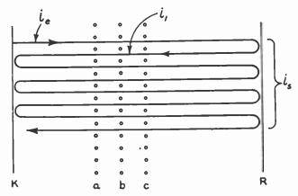
Fig. 2—Schematic electron paths in a triple-grid reflex oscillator, showing the effective current  $i_1$  and the built-up space current  $i_2$  due to multiple transits, between cathode K and reflector R.
