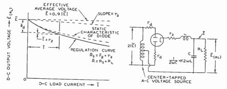
Fig. 26—Regulation characteristic of a full-wave, choke-circuit with high-vacuum diode.
