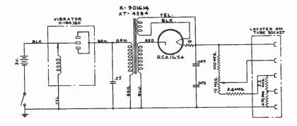
Fig. 13-Basic circuit of vibrator power supply.
