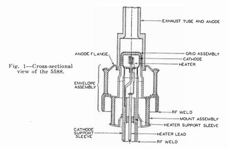
low-inductance cylinders. These members serve the further function of either providing or preventing thermal isolation of the various electrodes.
