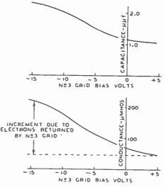
Fig. 16—Signal-grid (grid No. 1) admittance of typical mixer designed for outer-grid injection of oscillator. Data taken at 31.5 megacycles with no oscillator voltage applied.  $E_{c1} = -3$  volts,  $E_{c2}$  and  $\epsilon = 100$  volts,  $E_b = 250$  volts.
