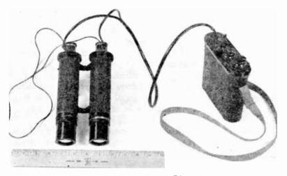
Fig. 10-Infrared In-line Binocular.
