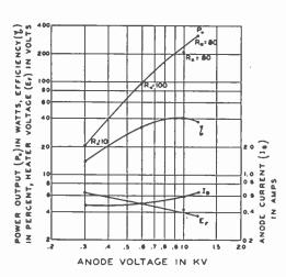
Fig. 6—Typical continuous-wave performance at 600 Mc.
