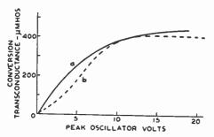
Fig. 14—Conversion transconductance of a typical mixer designed for outer-grid injection of oscillator. Signal-grid bias,  $E_{cl} = -3$  volts. Curve a corresponds to fixed No. 3 grid bias,  $E_{c2} = -8$  volts. Curve b corresponds to bias obtained through a 50,000-ohm grid leak.
