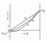
Fig. 2—Potential distribution in a diode, showing the effect of initial velocity of electron emission.
