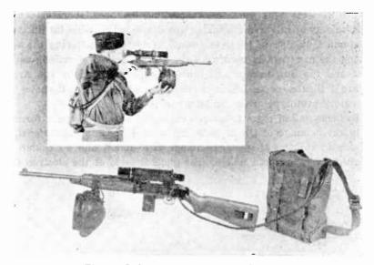
Fig. 2-Laboratory prototype sniperscope.
