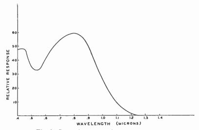
Fig. 6—Spectral response of 1P25 Image Tube.
