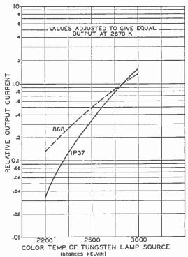
Fig. 5. Relative output of 868 and 1P37 as function of light source color temperature.
