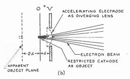
Fig. 9—Two methods of limiting beam current: (a) shows a narrow accelerating aperture; while (b) shows the use of a narrow emitting area on the cathode.
