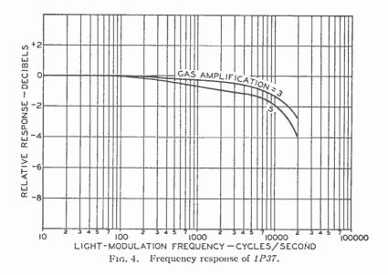
868 and therefore the frequency response of the 1P37 is slightly better. The frequency response for 2 different gas amplification factors is shown in Fig. 4. These curves were obtained using a glow lamp modulated light source,<sup>3</sup> the data being corroborated by measurements with standard frequency sound track.
