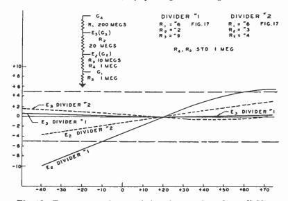
Fig. 18—Temperature characteristics of composite voltage divider.
