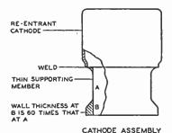
Fig. 7—Cathode assembly, cutaway view.
