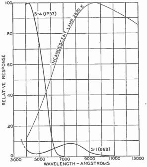
Fig. 2. Spectral response of S-1 and S-4 phototubes.
