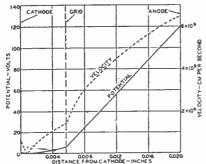
Fig. 1—Potentials and velocities in a parallel-plane triode.
