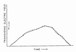
compasses and a protractor one may quickly find the final phase and magnitude of the circular motion acquired by an electron subjected to a time-varying electric field consisting of many linear sections. (See Figures 5 and 7.) The same construction gives information about the path of the electron while the field is acting. By supplementing the construction with a simple formula the complete paths may be plotted if required.
