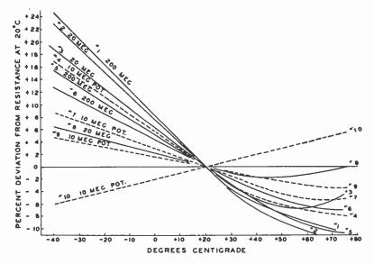
Fig. 17—Temperature characteristics of high-valued resistors.
