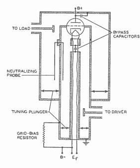
Fig. 14—Diagrammatic sketch of 1000-Mc amplifier of the foldedback type.
