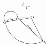
Fig. 5—The graphical construction giving the circular motion produced by the transverse field of Fig. 3. The radius vector  $CR_2$  indicates the phase and magnitude of the motion at the instant the electric field ceases to act.
