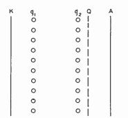
Fig. 8—Determination of amplification factor and inter-electrode capacitance in multigrid structures by use of the Q plane.
