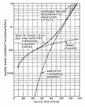
Fig. 6 — Dark current in photo-multiplier tubes.
