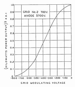
Fig. 11— Modulation characteristics.
