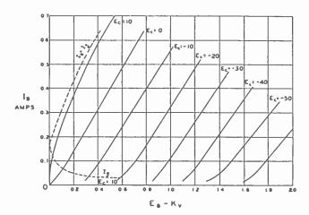
Fig. 3-Low-voltage plate characteristics of the H-2614.
