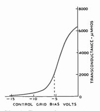
Fig. 4—Transconductance characteristic of a typical variable-μ, radio-frequency pentode.
