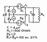
Fig. 28—Graphic solution of operation for a full-wave, condenser-input circuit without series resistance.
