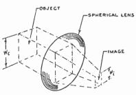
Fig. 11—Representation of electron optics using a spherical lens system to focus both width and thickness of a rectangular electron beam.
