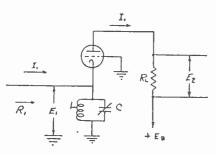
Fig. 1—Single stage grounded-grid amplifier.
