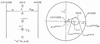
Fig. 3—Cross section of a triode in normal co-ordinates.
