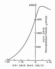
Fig. 8 — Signal-grid-(grid No. 4) to-plate transconductance versus oscillator-grid (grid No. 1) voltage curve of a typical mixer designed for inner-grid injection. Signal-grid bias = —3 volts.
