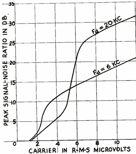
Fig. 1—Peak signal-to-noise ratio characteristics for frequency-modulation systems using maximum frequency deviations,  $F_d$ , of 20 and 6 kilocycles, respectively. The audio band width was 5 kilocycles. The noise was internal receiver noise and the signal-to-noise ratios were measured on an oscilloscope.
