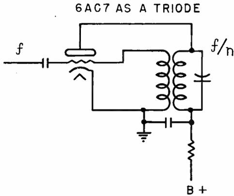
Fig. 10—Locked-In Oscillator Frequency Divider
