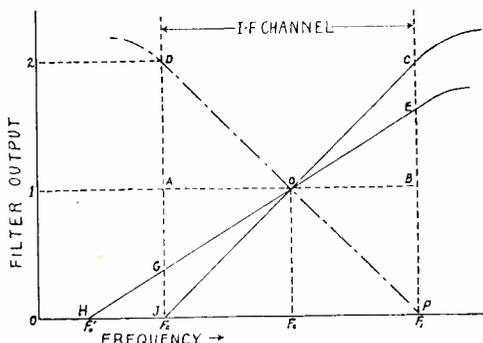
Fig. 2—Ideal sloping filter characteristics.
