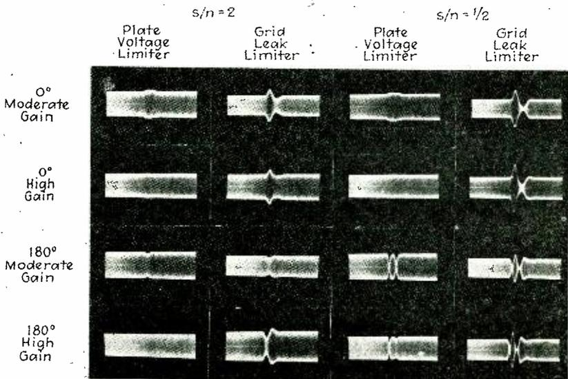
Fig. 4—Oscillograms demonstrating the relative effectiveness of plate voltage and grid leak limiters.
