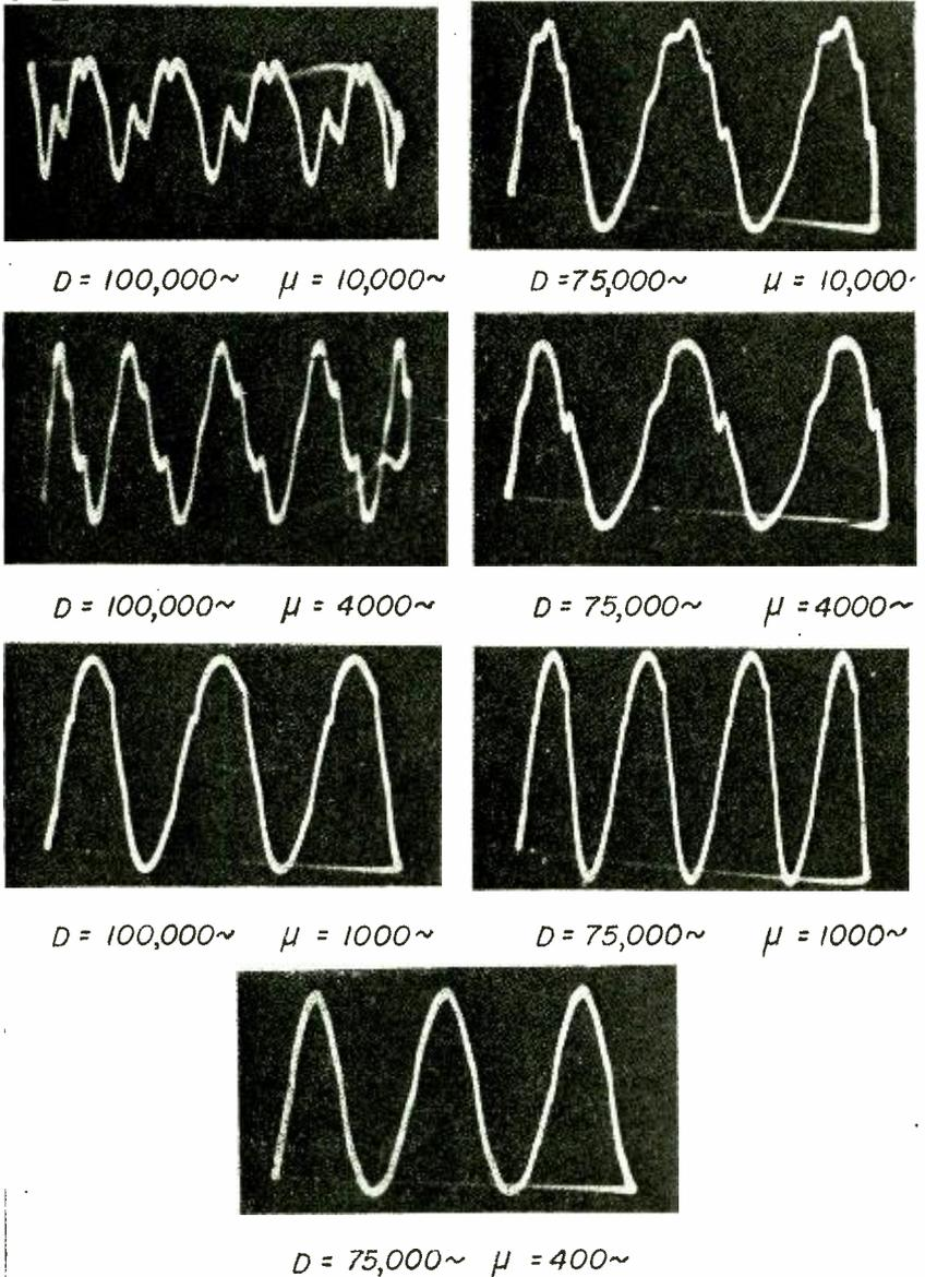
Fig. 23—Oscillograms showing distortion.
