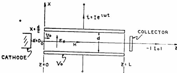
Fig. 1—Schematic diagram of beam and electrode arrangement.
