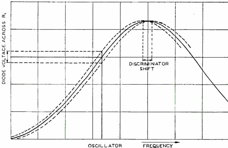
Fig. 3—Graphical representation of the modulated discriminator FM action.
