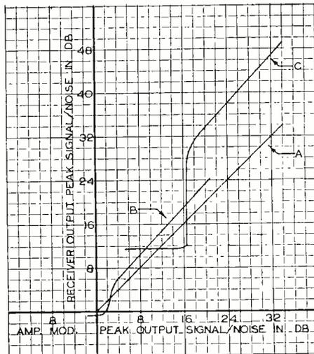
Fig. 15—Measured peak signal-noise ratio characteristics of impulse noise. Curve A = amplitude modulation receiver. Curve B = frequency modulation receiver with deviation ratio of unity. Curve C = frequency modulation receiver with deviation ratio of four.
