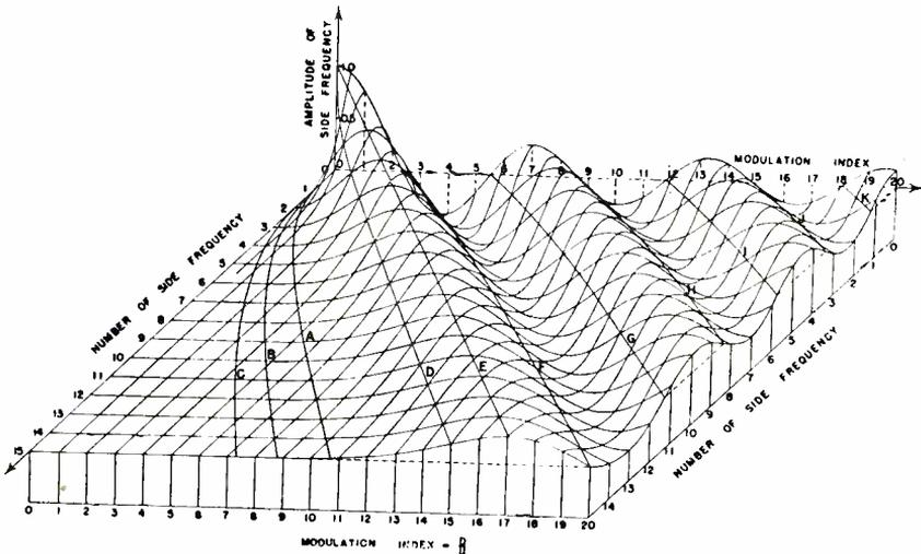
Fig. 4—Side-frequency amplitudes.
