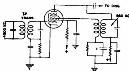
Fig. 13—Tuned-feedback coil.
