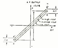
Fig. 22—Effect on the output of a balanced detector when amplitude modulation causes a detuning of the secondary. This is referred to as an unbalanced a-m component.
