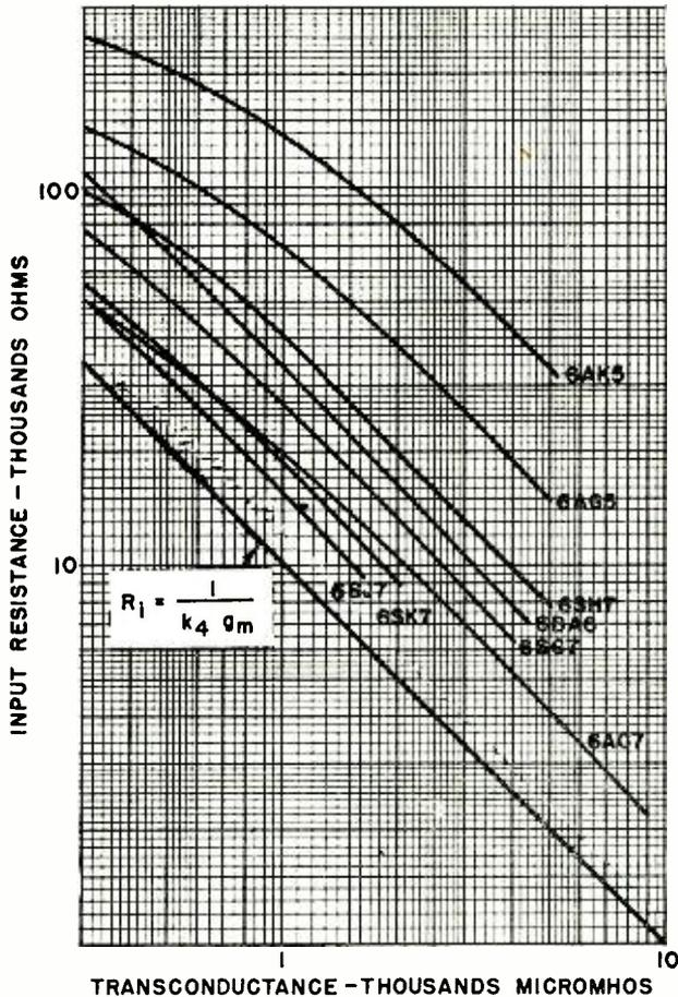
Fig. 6—Input resistance with variable transconductance at 50 megacycles.
