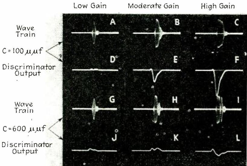
Fig. 2—Oscillograms of noise wave train and output of discriminator showing detuning due to grid current at higher amplitudes.
