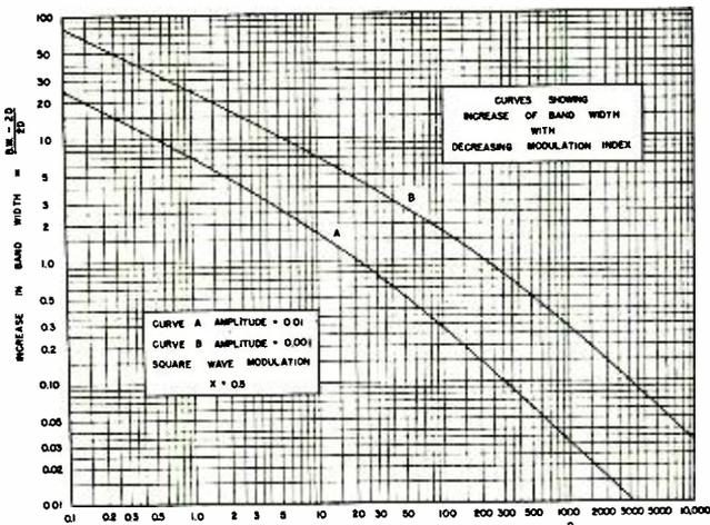
Fig. 11—Variation of bandwidth with modulation index.
