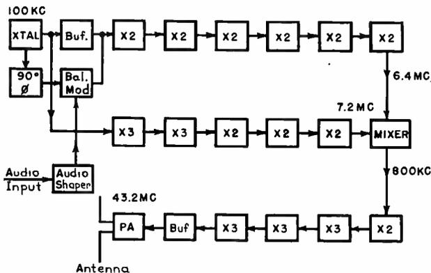
Fig. 2—Block Diagram of Armstrong Type FM Transmitter.
