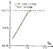
Fig. 17—The fraction of the total rectified voltage which must be stabilized to reduce the residual balanced amplitude modulation is a function of  $S/P$ . For values of  $S/P$  greater than about unity, the a-m in the output increases if less than the full rectified voltage is stabilized.
