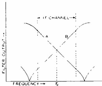
Fig. 3—Characteristics of the conversion filters used to convert frequency modulation into amplitude modulation for detection.
