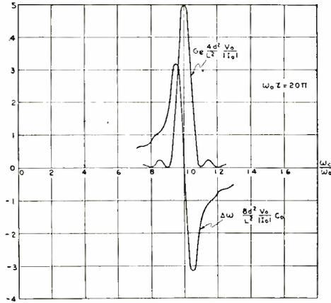
Fig. 5(a)—Theoretical frequency shift and electronic loading as a function of magnetic field strength.
