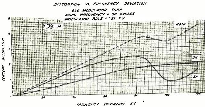
$E_g$  curve. This can be corrected, if desired, by some types of regenerative audio circuits, which tend to increase non-linearity in the modulator tube  $R_p$  curve, or by the use of an additional modulator to supply 2nd harmonic variations in  $R_p$  to produce additional curvature.
