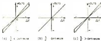
Fig. 24—On either side of the optimum value of  $S/P$  for which the balanced component of a-m is zero, there is a reversal in the phase of the a-m in the output. Since, for a given transformer, the value of  $S/P$  changes with coupling, the figure shows that for a loose coupling the output is 180 degrees out of phase with the input a-m, while the two are in phase for close coupling.
