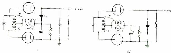
Fig. 25—Either one or two diode load condensers may be used in the ratio-detector load circuit. To obtain the same effective diode load capacitance in (b) as in (a),  $C_3$  must be equal to the sum of  $C_1$  and  $C_2$ .
