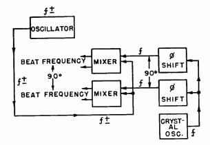
Fig. 6-Fundamental Frequency Control Circuit
