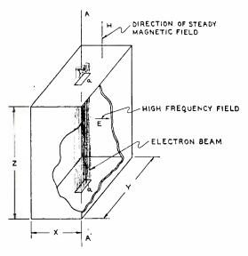
Fig. 11—Schematic diagram showing beam in rectangular resonant cavity.
