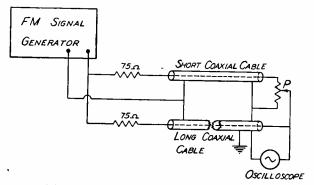
Fig. 8—Circuit for studying interference.
