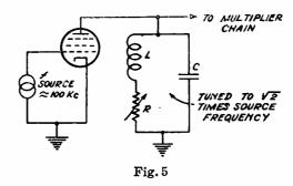
equal in magnitude to the reactance of the circuit capacitance, for all values of R from zero to infinity. Hence, no amplitude modulation is present, regardless of the extent or amount of phase modulation. Appendix I contains a development of the equations of phase vs. R, and also a proof of the constancy of plate-load impedance as R is varied.
