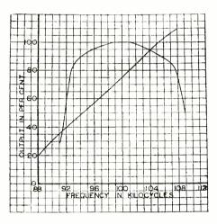
Fig. 8—Band-pass characteristic of receiver intermediate-frequency amplifier, and characteristic of sloping filter.
