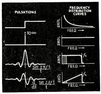
Fig. 8—Various types of pulsations and the corresponding curves of relative amplitude vs. frequency.
