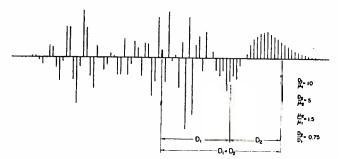
Fig. 6-Spectrum for complex modulation.
