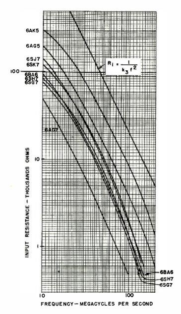
Fig. 1—Input resistance vs. frequency with plate by-passed and tubes operated under conditions given in Table 1.
