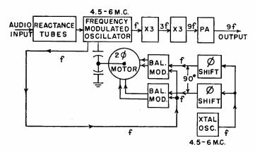
Fig. 7-Preliminary Frequency Control FM Exciter
