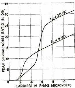
Fig. 1—Peak signal-to-noise ratio characteristics for frequency-modulation systems using maximum frequency deviations,  $F_d$ , of 20 and 6 kilocycles, respectively. The audio band width was 5 kilocycles. The noise was internal receiver noise and the signal-to-noise ratios were measured on an oscilloscope.
