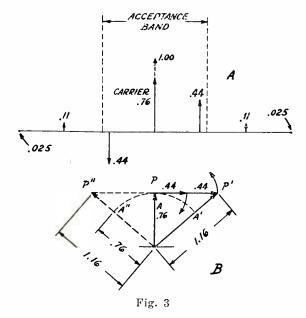
Under these conditions it can be seen that the resultant instantaneous scalar magnitude of the carrier will vary between .76 and 1.16. In other words, amplitude modulation at twice the modulating frequency has resulted from deletion of all but the first side bands. This amplitude modulation contains no components at the 10,000-cycle frequency, is chiefly second harmonic, and contains small amounts of other even harmonics.
