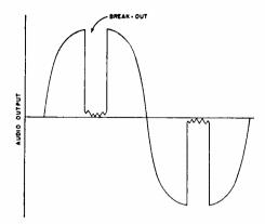
Fig. 7-Breakout characteristic.
