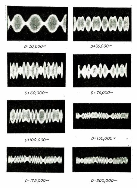
Fig. 9—Oscillograms of carrier envelopes.
