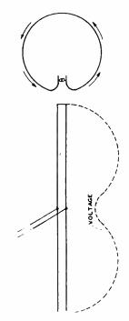
Fig. 4—The slot functions as a transmission line when fed with power.
