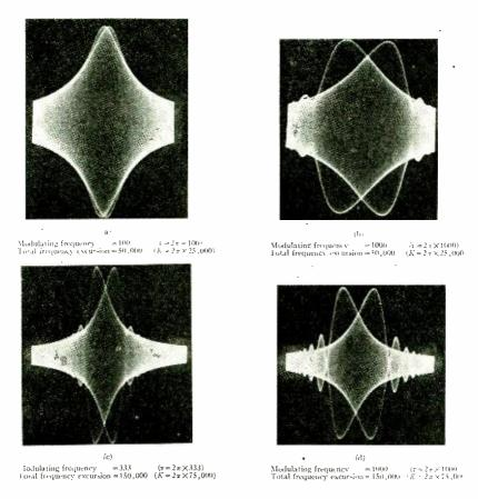
Fig. 2—Experimental amplitude—instantaneous-input-frequency and phase-shift—instantaneous-input-frequency response of a tuned amplifier to a frequency-modulated wave.
