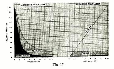
program modulation, depending upon the character of the sound source. The NBC field test confirmed these conclusions. Therefore, in presetting transmitter gain controls, using low-frequency tone modulation, a 2.5 db correction should be made for program modulation.
