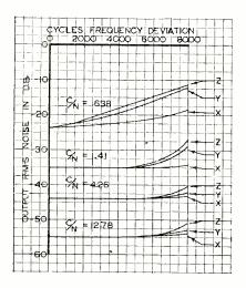
Fig. 13—Variation of frequency modulation receiver output noise as frequency modulation is applied. 1600-cycle low-pass filter in audio output. Modulation frequency: for curve  $X\!=\!6000$  cycles,  $Y\!=\!3000$  cycles, and  $Z\!=\!2000$  cycles.  $C/N\!=\!$  peak carrier-noise ratio in the output of intermediate-frequency channel.
