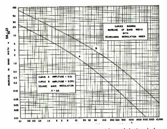
Fig. 11-Variation of bandwidth with modulation index.
