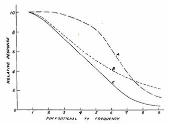
Fig. 4-Frequency-response curves of wide-range frequency discriminator.
