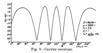
Another interesting difference is that the two voltages come almost, but not quite, into phase at 30 degrees. This peak is therefore slightly lower than the others. The difference is caused by the fact that the sine of an angle is not linear, but departs from a straight line for larger angles. The maximum angle through which the one vector of Figure 2 rotates with respect to the other is given by
