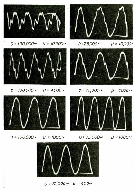
Fig. 23—Oscillograms showing distortion.
