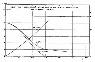
Fig. 8—Admittance modulation factor and phase shift versus modulation transit angle for  $\theta = \pi$ .
