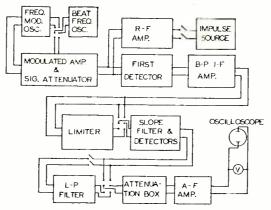
Fig. 7-Block diagram of experimental setup.
