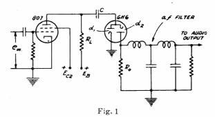
increase the average value of current flowing through  $R_o$ . Conversely, a decrease in repetition rate decreases the average current through  $R_o$ , and the average potential across  $R_o$  is thus a perfectly linear function of the repetition rate or frequency of the input signal.
