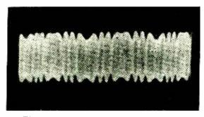
Fig. 10—Oscillogram of carrier envelope.
