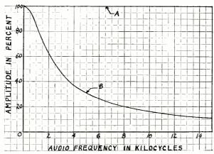
Fig. 4—Amplitude-modulation audio noise spectrums.
