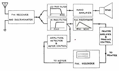
Fig. 7—Receiver block diagram for multiplex operation of aural and facsimile.
