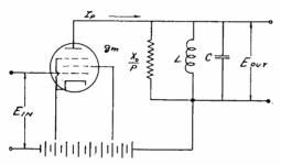
Fig. 3-Simplified schematic of a tuned amplifier.
