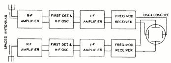
Fig. 4—Block diagram of receiver arrangement used in determining the phase relation between the detected outputs from receivers connected to spaced antennas.
