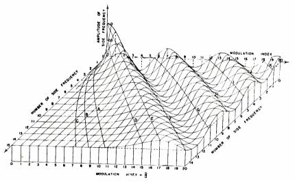
Fig. 4-Side-frequency amplitudes.
