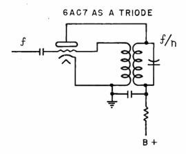
Fig. 10-Locked-In Oscillator Frequency Divider
