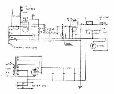
Fig. 13-Schematic of the push-pull FM calibrator.
