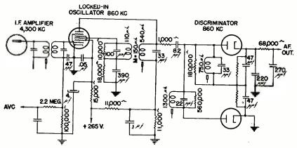
Fig. 16-Locked-in oscillator and discriminator.
