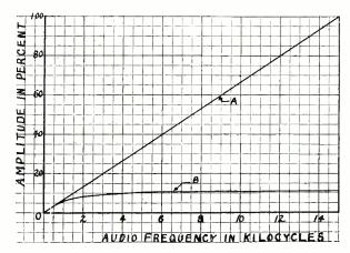
Fig. 5—Frequency-modulation audio noise spectrums. Curve A = no de-emphasis used.
