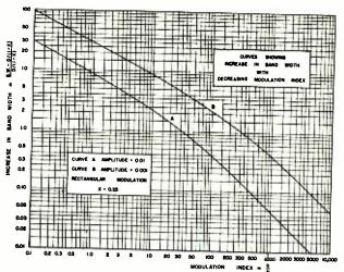
Fig. 12-Variation of bandwidth with modulation index.
