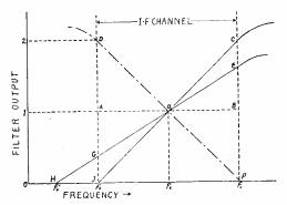
Fig. 2—Ideal sloping filter characteristics.
