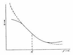
Fig. 11-Matching the discriminator to the oscillator.
