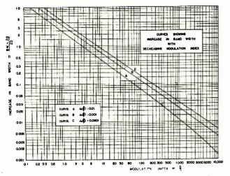
Fig. 5-Variation of bandwidth with modulation index.
