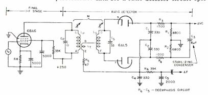
Fig. 8—A ratio-detector circuit using a balanced phase shift transformer feeding a 6AL5 double diode. The closely coupled tertiary winding  $L_{r}$  is wound over the  $B^{+}$  end of the primary to provide impedance matching and improved sensitivity.
