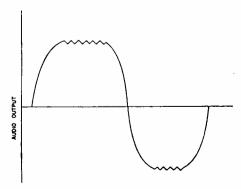
Fig. 8-Breakout characteristic.
