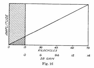
The maximum height of this F-M triangle, corresponding to voltage, is only one-fifth of the height of an FM-15 triangle or the A-M rectangle. Such being the case, the FM-75 advantage over FM-15 is 5 to 1, or 14 db, and over AM it is 1.73 x 5 or 18.75 db.
