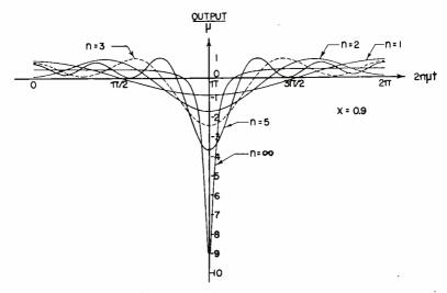
Fig. 12—Effect of low-pass filter.
