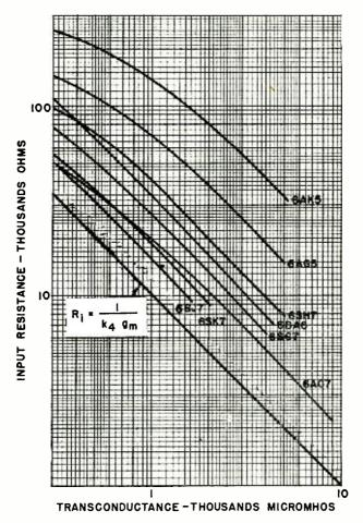
Fig. 6-Input resistance with variable transconductance at 50 megacycles.
