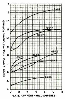
Fig. 7-Input capacitance variation with plate current.
