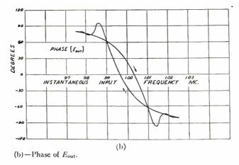
Fig. 5—Calculated amplitude—instantaneous-input-frequency and phase-shift—instantaneous-input-frequency response of a tuned amplifier to a frequency-modulated wave.
