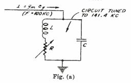
(1) To demonstrate the constancy of tuned impedance as R is varied.  $\omega_s = 2\pi \times \text{input frequency (100 kc)}$
