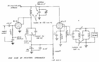
Fig. 8-Phase modulator circuit.
