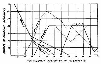
Fig. 1—Spurious responses caused by harmonic combinations of signal and oscillator versus intermediate frequency.
