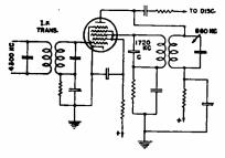
Fig. 2-The locked-in oscillator.
