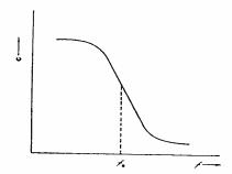
Fig. 9-Input capacitance of discriminator.
