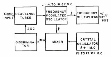
Fig. 4-Reactance Tube FM Exciter.
