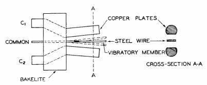
Fig. 6-One form of push-pull FM transducer.
