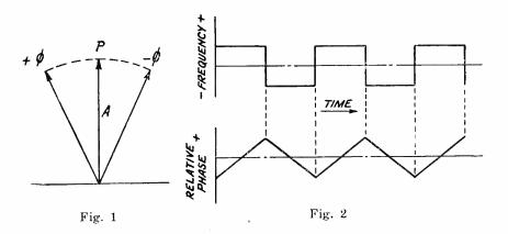
is progressively retarded. The square wave will be instantly recognized as the first derivative of the triangular wave below. This is another simplified means of illustrating the fact that frequency modulation is a function of the first derivative or rate of change of any existing phase modulation.
