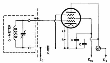
Fig. 2-Circuit for input impedance measurements.
