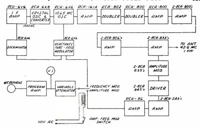
FM-FIELD TEST TRANSMITTER WZXWG
