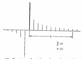
Fig. 18-Spectrum for triangular pulse modulation.
