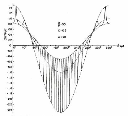
Fig. 19—Common-channel interference, interfering signal detuned.
