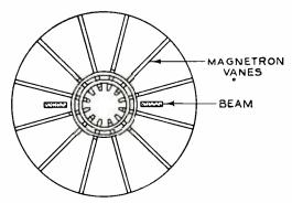
Fig. 7—Cross-sectional view of multivane magnetron with auxiliary beams.
