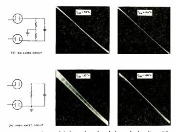
Fig. 26—A comparison of balanced and unbalanced circuits with respect to their effectiveness in rejecting low-frequency amplitude modulation.
