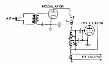
Fig. 1-Circuit diagram of frequency modulated master oscillator.
