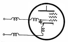
Fig. 3a-Series resonance in tube input circuit.
