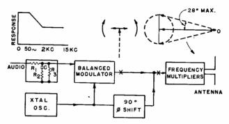
Fig. 1—Operation of Phase-Shift Modulator, Armstrong Type FM Transmitter.
