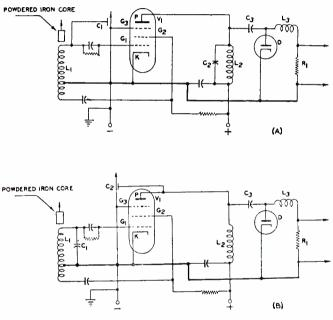
Fig. 1—(A) Modulated oscillator FM circuit.
