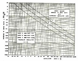
Fig. 17-Variation of bandwidth with modulation index.
