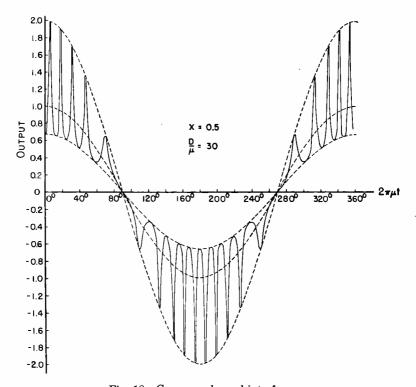
Fig. 18—Common-channel interference.
