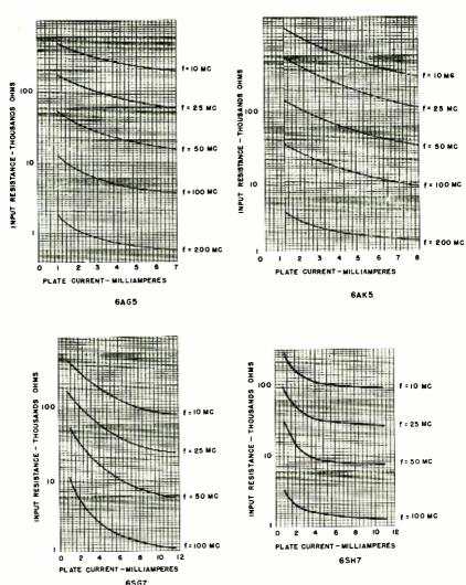
Fig. 4-Input resistance variation with plate current.
