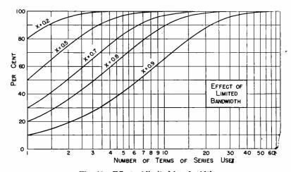
Fig. 13 - Effect of limited band width.
