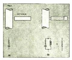
Fig. 2—By properly mounting antenna elements on the supporting pole impedances may be controlled and zero reactances obtained.
