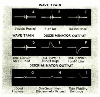
Fig. 1—Oscillograms of noise wave train and output of discriminator for various conditions of tuning.
