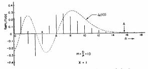
Fig. 16—Spectrum for triangular modulation.
