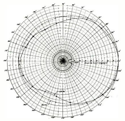
Fig. 8-Plot of the horizontal radiation, at frequencies of 86 and 110 mc.
