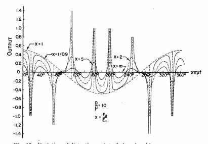
Fig. 15—Variation of distortion as interfering signal becomes stronger.
