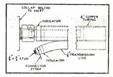
Fig. 6-Details of one radiator element.
