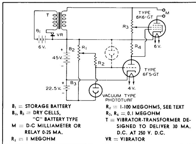
Fig. 6—Battery-operated circuit for relay or measurement operations.
