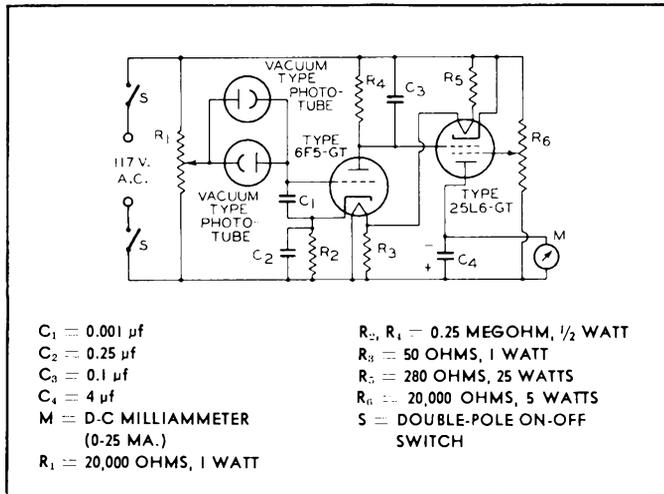
Fig. 10—Circuit for measurement of light-intensity ratios.
