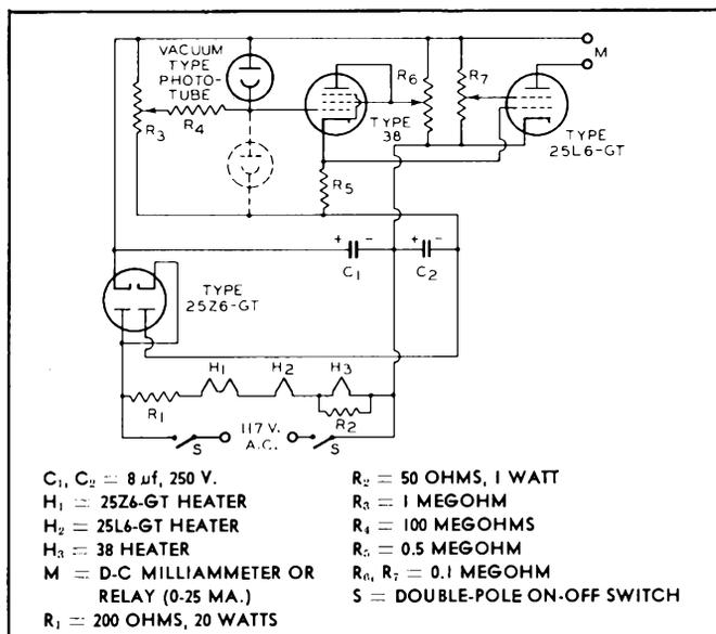
Fig. 5—Fast-acting circuit for relay or measurement operations.
