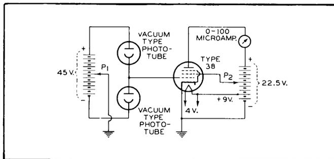
Fig. 7—Sensitive circuit for matching measurements.
