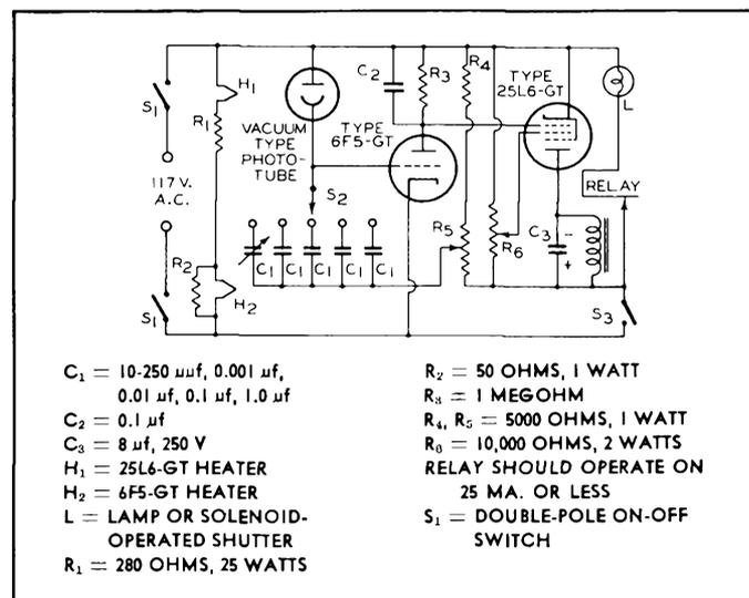
*Fig. 12—Photographic-exposure control circuit.*
