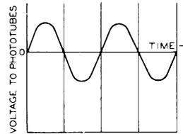
Fig. 11a—Equal illuminations on phototubes.
