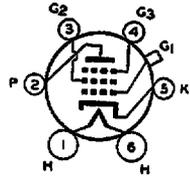
istics. The ability of this tube to handle the usual signal voltages without cross-modulation and modulation-distortion makes it adaptable to the r-f and i-f stages of receivers employing automatic volume control. The 6D6 is constructed with an internal shield connected to the cathode within the tube.
