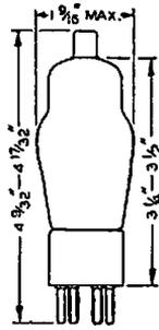
The 89 is a triple-grid power-amplifier tube of the heater-cathode type recommended for use in receivers with 6.3-volt heater supply. The triple-grid construction of this tube,
