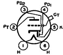
The 75 is a heater type of tube consisting of two diodes and a high-mu triode in a single bulb. It is for use as a combined detector, amplifier, and automatic-volume-control tube in a-c receivers designed for its characteristics. For diode-detector considerations, refer to page 26.
