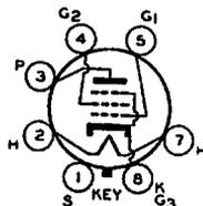
The 25A6 is a power-amplifier pentode of the All-Metal type for use in the output stage of radio receivers, especially those of the "d-c power line" or "universal" type. In such applications, the 25A6 is capable of handling relatively large audio power.
