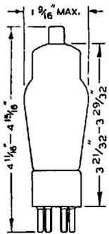
The 58 is a triple-grid super-control amplifier tube recommended especially for service in the radio-frequency and intermediate-frequency stages of a-c receivers designed for its
