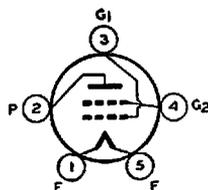
The 49 is a double-grid power-amplifier tube designed for use in battery-operated receivers employing 2-volt tubes. In such service, it may be used either as a Class B output tube or, by a change in socket connections, as a Class A driver tube.
