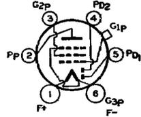
The 1F6 is a duplex-diode pentode consisting of two diodes and a pentode in a single bulb. It is recommended for service as a combined detector, amplifier (radio-frequency, intermediate-frequency or audio-frequency), and automatic-volume-control tube in battery-operated receivers. For diode-detector considerations, refer to page 26.
