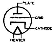
The grid, plate, and cathode of a triode form an electrostatic system, each electrode acting as one plate of a small condenser. The capacitances are those existing between grid and plate, plate and cathode, and grid and cathode. These
