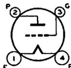
The 30 is a detector and amplifier tube of the three-electrode type for battery-operated radio receivers where economy of filament-current drain is important.
