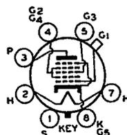
The 6L7 is a multi-electrode vacuum tube of the All-Metal type designed with two separate control grids shielded from each other. This design permits each control grid to
