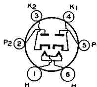
suited for "transformerless" receivers of either the "universal (a.c.-d.c.)" type or the "a-c operated" type. In "universal" receivers, the 25Z5 may be used as a half-wave rectifier, while in the "a-c operated" type, it may be used as a voltage doubler to provide about twice the d-c output voltage obtainable from the half-wave arrangement. This two-fold application is made possible by the use of a separate base pin for each of the two cathodes. For voltage-doubler considerations, see page 25.
