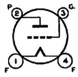
The 31 is a power-amplifier tube of the three-electrode type for battery-operated radio receivers where economy of filament-current drain is important.
