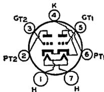
The 53 is a heater-cathode type of tube combining in one bulb two high- $\mu$  triodes designed for Class B operation. It is intended primarily for use in the output stage of a-c
