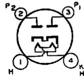
The 83-v is a high-vacuum, full-wave rectifier tube of the heater-cathode type. It is intended for use in suitable rectifying devices designed to supply d-c power to receivers having large d-c requirements. The excellent voltage regulation characteristic of the 83-v is due to the close spacing of the cathode and plate.
