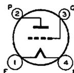
The 10 is a three-electrode, high-vacuum tube suitable for use as an audio-frequency amplifier in equipment designed for its characteristics.
