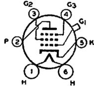
The 6C6 is a triple-grid tube of the heater-cathode type recommended for service as a biased detector in radio receivers designed for its characteristics. This tube is capable of delivering a large audio-frequency output voltage with relatively small input voltage. Significant among its electrical features are its sharp plate current "cut-off" with respect to grid voltage. The 6C6 is constructed with an internal shield connected to the cathode within the tube.
