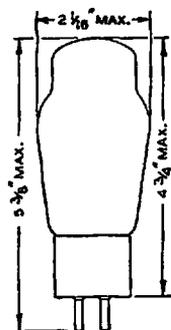
The 83 is a heavy-duty, full-wave, mercury-vapor rectifier tube of the hot-cathode type. It is intended for use in suitable rectifying devices designed to supply d-c power of
