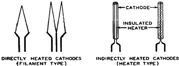
Directly heated filament-cathodes require comparatively little heating power. For that reason, they are used in almost all the tube types designed for battery operation because it is, of course, desirable to impose as small a drain as possible on the batteries. Examples of the battery-operated filament types are the 30, 31, 32, 33, and 34. A-c operated types having directly heated filament-cathodes are the 2A3 and 45.
