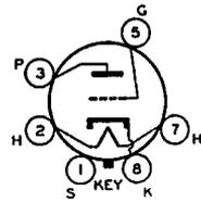
The 6C5 is a three-electrode tube of the metal type recommended for use as a detector, amplifier, or oscillator. This tube has a high trans-conductance together with a comparatively high amplification factor.
