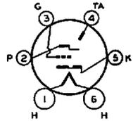
The 6E5 is a high-vacuum, heater-cathode type of tube designed to indicate visually, by means of a fluorescent target, the effects of a change in the controlling voltage.
