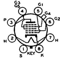
The 6A8 is a multi-electrode vacuum tube of the metal type designed to perform simultaneously the functions of a mixer (first detector) tube and of an oscillator tube in super-heterodyne circuits. Through the use of this type, the independent control of each function is made possible within a single tube. For general discussion of pentagrid types, refer to **FREQUENCY CONVERSION**, page 31.
