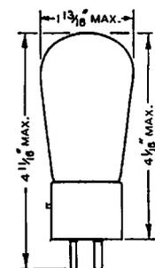
which the direct-current requirements are subject to considerable variation. The excellent voltage-regulation characteristic of the 82 is due to its low and practically constant tube voltage drop (only about 15 volts) for any current drain up to the full emission of the filament (see page 8).
