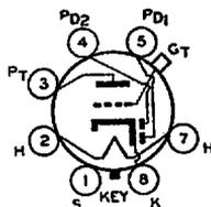
The 6R7 is an All-Metal tube consisting of two diodes and a triode in a single envelope. It is for use as a combined detector, amplifier, and automatic-volume-control tube in
