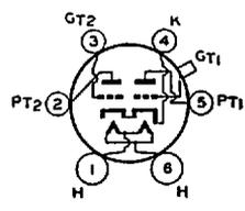
The 79 is a heater-cathode type of tube combining in one bulb two high- $\mu$  triodes designed for Class B operation. It is intended for use in the audio-output stage of radio receivers with 6.3-volt heater supply. The triode units have separate external terminals for all electrodes except the cathode and heater so that circuits employing the 79 are similar to those of Class B amplifiers utilizing individual tubes in the output stage.
