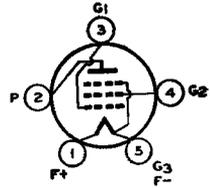
The 1F4 is a power-amplifier pentode for use in the output stage of battery-operated receivers. This tube has low filament and plate-current requirements, high power sensitivity,
