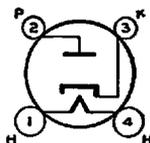
The 12Z3 is a half-wave, high-vacuum rectifier of the heater-cathode type for use in suitable circuits designed to supply d-c power from an a-c power line. It is intended for use in "transformerless" receivers of the "universal" (a.c.-d.c.) type. The adaptability of the 12Z3 to such receivers is facilitated by the heater design which permits of convenient series operation with other tube types.
