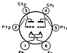
The 19 combines in one bulb two high- $\mu$  triodes designed for Class B operation. It is intended for use in the output stage of battery-operated receivers and is capable of supplying approximately 2 watts of audio power. The triode units have separate external terminals for all electrodes except the filaments, so that circuit design is similar to that of Class B amplifiers utilizing individual tubes in the output stage.
