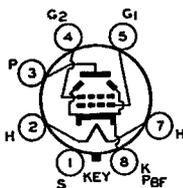
The 6L6 is a power-amplifier tube of the All-Metal type for use in the output stage of radio receivers, especially those designed to have ample reserve of power-delivering ability.
