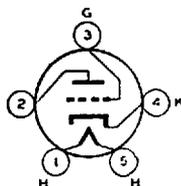
The 56 is a three-electrode tube of the heater-cathode type recommended for use as detector, amplifier, or oscillator in a-c receivers designed for it. This tube is characterized by its high mutual conductance, and its comparatively high amplification factor. The 56 is useful in resistance-coupled audio-frequency amplifiers.
