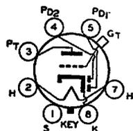
The 6Q7 is an All-Metal tube consisting of two diodes and a high-mu triode in one envelope. It is for use as a combined detector, amplifier, and automatic-volume-control tube in
