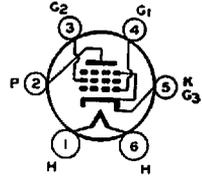
The 42 is a heater-cathode type of power-amplifier pentode for use in the audio-output stage of receivers. It is capable of giving large power output with a relatively small input-signal
