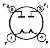
The 80 is a full-wave rectifying tube intended for use in d-c power-supply devices which operate from the a-c supply line.
