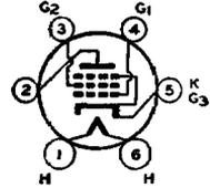
The 2A5 is a heater-cathode type of power-amplifier pentode for use in the audio-output stage of a-c receivers. It is capable of giving large power output with a relatively small input-signal voltage. Because of the heater-cathode construction, a uniformly low hum-level is attainable in power-amplifier design.
