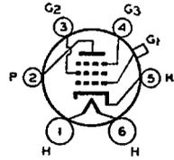
The 77 is a triple-grid tube recommended especially for service as a biased detector in radio receivers designed for its characteristics. In such service, this tube is capable of delivering
