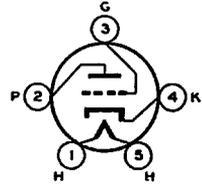
The 76 is a three-electrode tube of the heater-cathode type recommended for use as detector, amplifier, or oscillator with either a-c or d-c heater supply. This tube is characterized by its high mutual conductance and its comparatively high amplification factor. The 76 is useful in resistance-coupled audio-frequency amplifiers.
