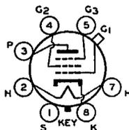
The 6K7 is a triple-grid super-control amplifier tube of the All-Metal type recommended for service in the radio-frequency and intermediate-frequency stages of radio receivers designed for its characteristics. The ability of this tube to handle unusual signal voltages without cross-modulation and modulation-distortion makes it adaptable to the r-f and i-f stages of receivers employing automatic volume control.
