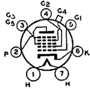
The 2A7 is a multi-electrode type of vacuum tube designed to perform simultaneously the functions of a mixer (first detector) tube and of an oscillator tube in superheterodyne circuits. Through the use of this type, the independent control of each function is made possible within a single tube. The 2A7 is intended especially for use in a-c receivers having a 2.5-volt heater supply. For general discussion of pentagrid types, see FREQUENCY CONVERSION, page 31.
