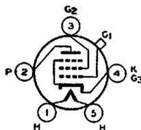
The 39/44 is a heater-cathode tube of the remote cut-off type suitable for use primarily as a radio-frequency amplifier, intermediate-frequency amplifier, and mixer in receivers
