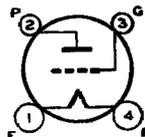
The 2A3 is a three-electrode, high-vacuum type of power amplifier tube for use in the power-output stage of a-c operated receivers. The exceptionally large power-handling ability of the 2A3 is the result of its design features. Among these are its extremely high transconductance and its large effective cathode area.
