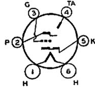
The 6G5 is a high-vacuum, heater-cathode type of tube designed to indicate visually, by means of a fluorescent target, the effects of change in the controlling voltage.
