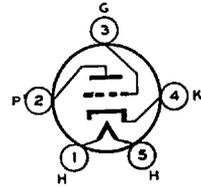
The 27 is a three-electrode general purpose tube of the heater-cathode type for use as an amplifier and detector in a-c receivers.
