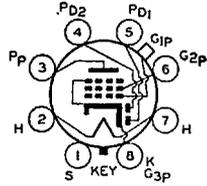
The 6B8 is an All-Metal type of tube consisting of *two diodes* and a *pentode* in a single envelope. It is recommended for service as combined detector, amplifier (radio-frequency, intermediate-frequency or audio-frequency), and automatic-volume-control tube in radio receivers. For diode-detector considerations, refer to page 26.
