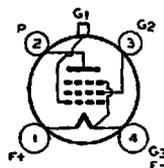
The 34 is a super-control pentode recommended for use primarily as a radio-frequency amplifier and intermediate-frequency amplifier in battery-operated receivers where economy of
