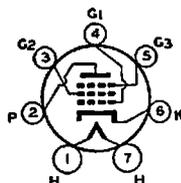
The 59 is a triple-grid power-amplifier tube of the heater-cathode type for use in the output stage of a-c operated receivers. The triple-grid construction of this tube, with
