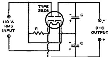
R=HEATER VOLTAGE-REDUCING RESISTOR
