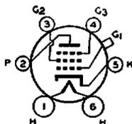
The ability of this tube to handle usual signal voltages without cross-modulation and modulation-distortion makes it adaptable to the r-f and i-f stages of receivers employing automatic volume-control. The internal shield around the plate of the 78 is connected to the cathode within the tube.
