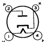
The 1-v is a half-wave, high-vacuum rectifier tube employing a heater cathode. It is intended for use in radio equipment of either the "universal" or the automobile type designed for its characteristics. The low voltage drop of this tube makes it uniquely adapted to such service. The 1-v is interchangeable with type 1.
