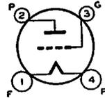
The 26 is an amplifier tube containing a filament designed for operation on alternating current. This tube is for use as an r-f or a-f amplifier in equipment designed for
