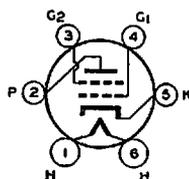
The 48 is a power-amplifier tetrode which has pentode characteristics when operated at the recommended screen and plate voltage. It is for use in the audio-output stage of
