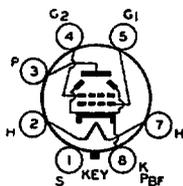
The 25L6 is a power-amplifier tube of the All-Metal type for use in the output stage of "transformerless" (a.c.-d.c.) radio receivers, especially those designed to have ample reserve of power-delivering ability. The new tube provides high power output at the relatively low plate and screen voltages available for transformerless receivers. The high power output is obtained with high power sensitivity and high efficiency.
