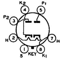
The 6H6 is a heater-cathode type of All-Metal tube combining two diodes in one shell. Each diode has its own separate cathode and corresponding base pin. This arrangement offers flexibility in the design of circuits employing the 6H6 for detection, for low-voltage low-current rectification, or for automatic volume control. For diode-detector considerations, refer to page 26.
