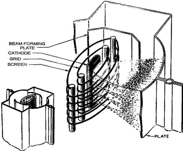
INTERNAL STRUCTURE OF BEAM POWER TUBE
