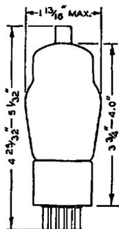
The 35 is a super-control screen grid amplifier tube of the heater-cathode type recommended as an r-f amplifier and an i-f amplifier in a-c receivers. The 35 is very effective
