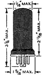
The 6F6 is a heater-cathode power-amplifier pentode of the All-Metal type for use in the audio-output stage of a-c receivers. It is capable of giving large power output with a relatively small input voltage. Because of the heater-cathode construction, a uniformly low hum-level is attainable in power-amplifier design.
