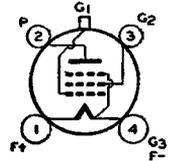
The 1A4 is a super-control pentode of the filament type. It is useful as a radio-frequency amplifier or intermediate-frequency amplifier in battery-operated receivers. The 1A4, although similar in application to type 34, is constructed in a smaller bulb and, because of its less remote cut-off characteristic, requires less B-battery power.
