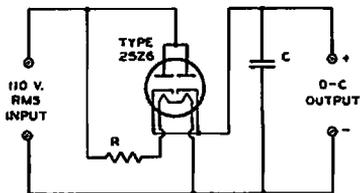
R=HEATER VOLTAGE-DROPPING RESISTOR
