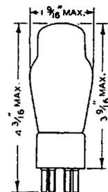
The 41 is a power-amplifier pentode of the heater-cathode type for use in the audio-output stage of radio receivers with 6.3-volt heater supply. The tube is capable of giving
