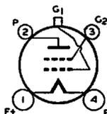
The 32 is a screen-grid tube recommended primarily for use as a radio-frequency amplifier in battery-operated radio receivers where economy of filament-current drain is important.
