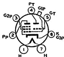
The 6F7 is a heater type of tube combining in one bulb a triode and an r-f pentode of the remote cut-off type. Since these two units are independent of each other except for the common cathode, the 6F7 may be adapted to circuit design in several ways.
