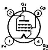
The 1B4 is a pentode of the filament type. It is recommended for use primarily as a radio-frequency amplifier or detector in battery-operated receivers. The 1B4 is similar
