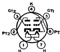
The 6A6 is a heater-cathode type of tube combining in one bulb two high- $\mu$  triodes designed for Class B operation. The triode units have separate external terminals for all
