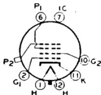
light brightness of the projected picture is about 15 foot-lamberts when the 5TP4 is operated at 27 kilovolts. Utilizes electrostatic focusing and magnetic deflection. Has solid deflection angle of 50° approx. Maximum bulb diameter is 5-1/8 inches; maximum overall length, 12-1/8 inches. Outline 37, OUTLINES SECTION. Provided with small-shell duodecal 7-pin base and a recessed small cavity cap.
