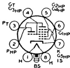
ductance, 525 μmhos; plate ma., 1.8; grids-No.2-and-No.4 ma., 3.0. Typical operation of triode unit: plate supply volts, 250 (300 max) applied through a 20000-ohm dropping resistor bypassed by a 0.1-μf capacitor; grid resistor, 50000 ohms; plate ma., 5.0; total cathode ma. (both units), 10.2.
