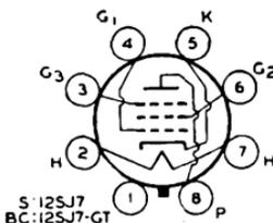
Metal type 12SJ7 and glass-octal type 12SJ7-GT used as rf amplifiers and biased detectors in ac/dc radio receivers. Outlines 3 and 19, respectively, OUTLINES SECTION.
