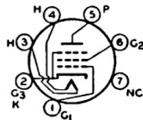
may be mounted in any position. For heater and cathode considerations, refer to miniature type 6AQ5. Within its maximum ratings, type 6AR5 is equivalent in performance to glass-octal type 6K6-GT. Refer to type 6K6-GT for characteristic curves.
