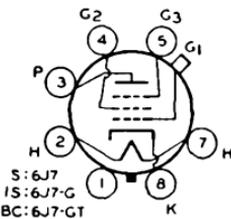
SECTION. All types require octal socket and may be mounted in any position. For typical operation as resistance-coupled amplifiers, refer to Charts 11 and 14, RESISTANCE-COUPLED AMPLIFIER SECTION. For heater and cathode considerations, refer to type 6AT6.
