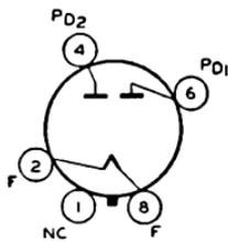
but horizontal mounting is permissible if pins 1 and 4 are in vertical plane. The coated filament is designed to operate from the ac line through a step-down transformer. The voltage at the filament terminals should be 5.0 volts under operating conditions at an average line voltage of 117 volts. It is especially important that this tube, like other power-handling tubes, should be adequately ventilated.
