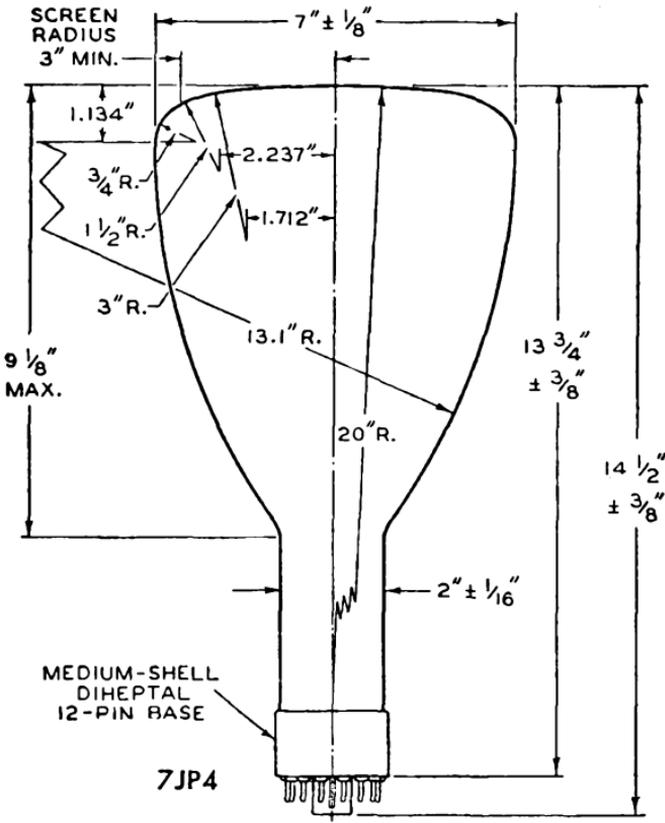
Center line of bulb will not deviate more than  $2^\circ$  in any direction from the perpendicular erected at the center of bottom of the base.
