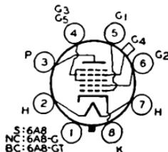
SECTION. All require octal socket. For general discussion of pentagrid types, see Frequency Conversion in ELECTRON TUBE APPLICATIONS SECTION. For heater and cathode considerations, refer to type 6AT6.
