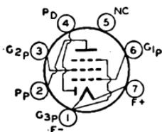
Miniature type used in light-weight, compact, portable, battery-operated receivers as combined detector and af voltage amplifier. Diode unit is located at negative end of filament
