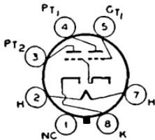
Glass octal type used as class A<sub>1</sub> power amplifier. One triode, the driver, is directly connected within the tube to the second, or output, triode. Heater volts (ac/dc), 25; amperes, 0.3. Characteristics as class A<sub>1</sub> amplifier—input triode: plate volts, 100 (180 max); grid volts, 0; peak af grid volts, 29.7; plate ma., 5.8. Output triode: plate volts, 180 max; plate ma., 46; load resistance, 4000 ohms; output watts, 3.8. This is a DISCONTINUED type listed for reference only.
