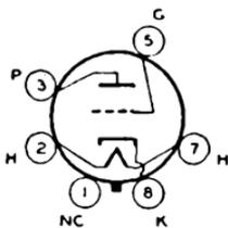
Glass octal type used in single-ended or push-pull audio-frequency power amplifiers of the direct-coupled type in which a driver tube develops positive grid bias for the 6AC5-GT output stage. Outline 17, OUTLINES SECTION. Tube requires octal socket. Heater volts (ac/dc), 6.3; amperes, 0.4. Maximum ratings: plate volts, 250 *max*; peak plate ma. (per tube), 110 *max*; average plate dissipation, 10 *max* watts. This type is used principally for renewal purposes.
