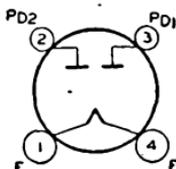
Glass type used in power supply of radio equipment having large dc requirements. Outline 34, OUTLINES SECTION. Tube requires four-contact socket. Vertical mounting is preferred
