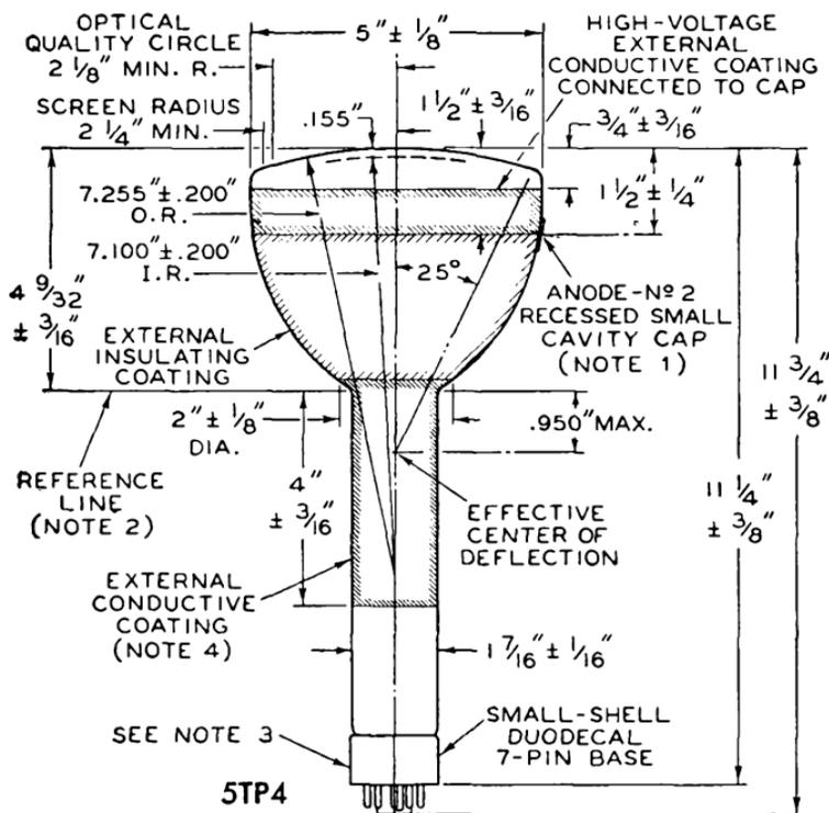
NOTE 1: The plane through the tube axis and vacant pin position No.3 may vary from the plane through the tube axis and anode-No.2 terminal by an angular tolerance (measured about the tube axis) of 10°. Anode-No.2 terminal is on same side as vacant pin position No.3.
