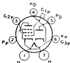
Glass type used as combined half-wave rectifier and power amplifier. Outline 27, OUTLINES SECTION. Tube requires small seven-contact (0.75-inch, pin-circle diameter) socket. Heater volts (ac/dc), 12.6; amperes, 0.3. Typical operation of pentode unit as class A<sub>1</sub> amplifier: plate volts and grid-No.2 volts, 135 *max*; grid-No.1 volts, -13.5; load resistance, 13500
