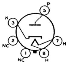
given by Outline 17, OUTLINES SECTION, but the 6W4-GT has a short intermediate-shell octal 6-pin base. Tube requires octal socket and may be mounted in any position. It is especially important that this tube, like other power-handling tubes, should be adequately ventilated.
