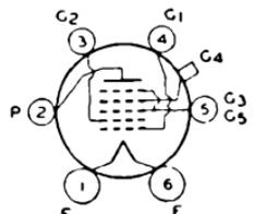
Glass type used in battery-operated receivers. Similar electrically to type 1C7-G except for interelectrode capacitances. Outline 27, OUTLINES SECTION. Tube requires six-contact socket. Filament volts (dc), 2.0; amperes, 0.12. For general discussion of pentagrid types, refer to Frequency Conversion in ELECTRON TUBE APPLICATIONS SECTION. This type is used principally for renewal purposes.
