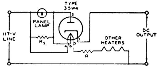
DRQP ACROSS R AND ALL HEATERS (WITH PANEL LAMP) SHOULD EQUAL 117 VOLTS AT 0.15 AMPERE.  $R_s$  = SHUNTING RESISTOR REQUIRED WHEN DC OUTPUT CURRENT EXCEEDS 60 MILLIAMPERES
