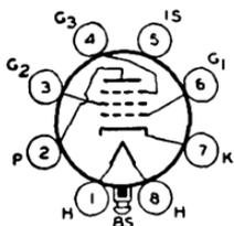
Glass lock-in type used as rf amplifier in high-frequency and wide-band applications. Outline 12, OUTLINES SECTION. Tube requires lock-in socket. Heater volts (ac/dc), 6.3; amperes, 0.15. Maximum ratings and characteristics as class A<sub>1</sub> amplifier: plate and grid-No.2 volts, 250 (300 max); plate dissipation, 2 max watts; grid-No.2 dissipation, 0.7 max watt; bias resistor, 250 ohms; grid No.3 and internal shield
