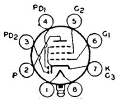
Glass lock-in type used as combined detector, amplifier, and avc tube. Outline 12, OUTLINES SECTION. Tube requires lock-in socket. Heater volts (ac/dc), 6.3; amperes, 0.3. Typical operation and maximum ratings of pentode unit as class A<sub>1</sub> amplifier: plate volts, 250 *max*; grid-No.2 volts, 100 *max*; plate dissipation, 2 *max* watts; grid-No.2 dissipation, 0.3
