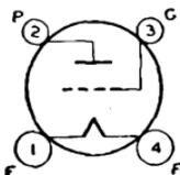
Glass type used in output stage of battery-operated receivers. Outline 25, OUTLINES SECTION. Tube requires four-contact socket. Filament volts (dc), 2.0; amperes, 0.13. Typical operation as class A<sub>1</sub> amplifier: plate volts, 180 *max*; grid volts, -30; plate ma., 12.3; plate resistance, 3600 ohms; amplification factor, 3.8; transconductance, 1050  $\mu$ mhos; load resistance, 5700 ohms; output watts, 0.375. This type is used principally for renewal purposes.
