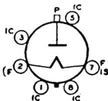
produced in the scanning system for the kinescope. When used as an rf rectifier, one 1B3-GT in a half-wave circuit is capable of delivering a maximum dc output voltage of about 20000 volts. In a voltage-doubler circuit, two tubes will give about 40000 volts; and in a voltage-tripler circuit, three 1B3-GT's will deliver 60000 volts approximately.
