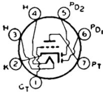
Miniature type used in compact radio equipment as combined detector, amplifier, and avc tube. The triode unit is particularly useful as a driver for impedance- or transformer-coupled
