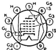
dimensions of type 6BA7 are given by Outline 11, OUTLINES SECTION. Tube requires noval nine-contact socket and may be mounted in any position. Its characteristics are similar to those of metal type 6SB7-Y. For heater and cathode considerations, refer to type 6AT6.
