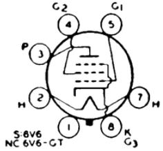
lines 6 and 17, respectively, OUTLINES SECTION. Tubes require octal socket and may be mounted in any position. The 6V6 and 6V6-GT are equivalent in performance to type 6AQ5. Refer to type 6AQ5 for heater and cathode considerations, application information, and characteristic curves.
