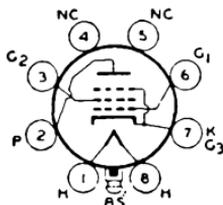
Glass lock-in type used in output stage of ac/dc receivers. Outline 15, OUTLINES SECTION. Tube requires lock-in socket. Heater volts (ac/dc), 50; amperes, 0.15. For ratings and data, refer to glass-octal type 50L6-GT.
