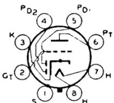
socket and may be mounted in any position. Heater volts (ac/dc), 6.3; amperes, 0.15. Direct interelectrode capacitances of triode unit (shell connected to cathode): grid to plate, 1.1  $\mu\mu\text{f}$ ; grid to cathode, 2.4  $\mu\mu\text{f}$ ; plate to cathode, 2.8  $\mu\mu\text{f}$ . For diode operation curves, refer to type 6SQ7.
