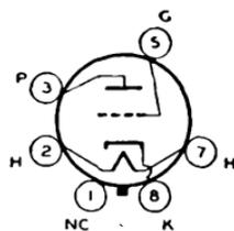
As a class A<sub>1</sub> amplifier, the 6L5-G may be operated in resistance-coupled circuits as shown in Chart 15, RESISTANCE-COUPLED AMPLIFIER SECTION. This type is used principally for renewal purposes.
