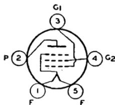
operation is permissible if pins 1 and 5 are in vertical plane. Filament volts (ac/dc), 2.5; amperes, 1.75.
