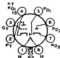
Glass lock-in type used as combined detector, amplifier, and avc tube in circuits which require diodes with separate cathodes. Outline 15, OUTLINES SECTION. Tube requires lock-in socket. Heater volts (ac/dc), 6.3; amperes, 0.3. Ratings and characteristics of triode unit as class A<sub>1</sub> amplifier: plate volts, 250 (300 max); grid volts, -1; amplification factor, 100; plate resistance, 67000 ohms; transconductance, 1500 μmhos; plate ma., 1.9.
