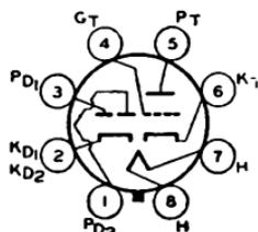
octal socket. Heater volts (ac/dc), 6.3; amperes, 0.3. Ratings and characteristics of triode unit as class A<sub>1</sub> amplifier: plate volts, 250 max; grid volts, -2; amplification factor, 70; plate resistance (approx.), 44000 ohms; transconductance, 1600 μmhos; plate ma., 2.3.
