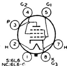
These types provide high power output, sensitivity, and high efficiency. Power output at all levels has low third and negligible higher-order harmonics. For discussion of beam power amplifier considerations, refer to ELECTRONS, ELECTRODES, AND ELECTRON TUBES SECTION.
