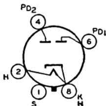
Metal type used in power supply of radio equipment having moderate dc requirements. Outline 6, OUTLINES SECTION. Tube requires octal socket and may be mounted in any position. Heater volts (ac), 5.0; amperes, 2.0. Maximum ratings: peak inverse plate volts, 1400 max; peak plate ma. per plate, 375 max. Typical operation as full-wave rectifier with capacitor-input filter: ac plate-to-plate supply
