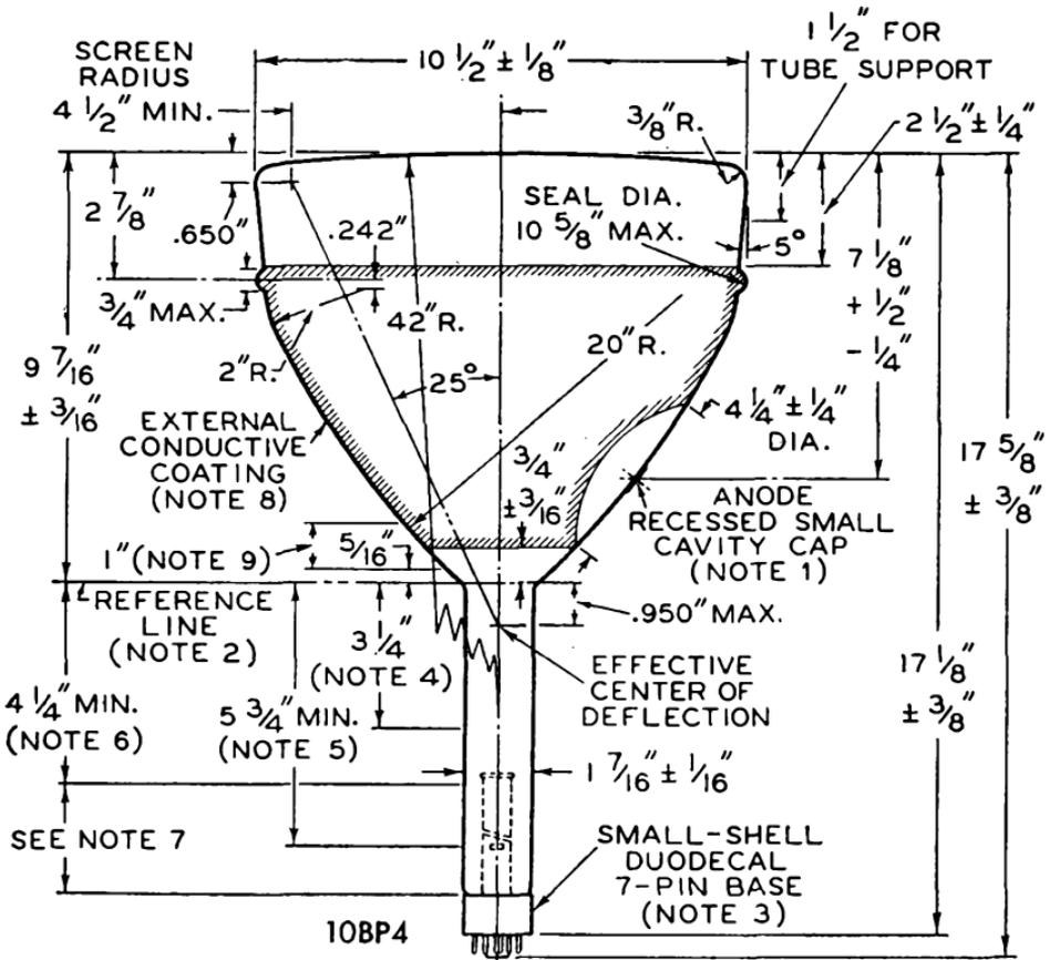
NOTE 1: The plane through the tube axis and vacant pin position No.3 may vary from the plane through the tube axis and anode terminal by an angular tolerance (measured about the tube axis) of 10°. Anode terminal is on same side as vacant pin position No.3.
