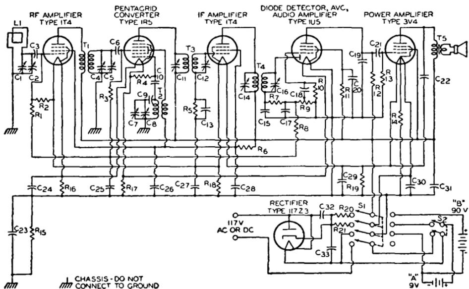
C<sub>1</sub> C<sub>4</sub> C<sub>8</sub> = Ganged tuning capacitors, 20-450  $\mu$ f
