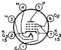
Miniature type used in compact radio equipment as an rf or if amplifier up to 400 megacycles. Outline 10, OUTLINES SECTION. Tube requires miniature seven-contact socket and may be mounted in any position. The two cathode leads facilitate isolation of the input and output circuits thus helping to minimize degeneration. For heater and cathode considerations, refer to type 6AT6.
