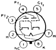
Glass octal type used as class A<sub>1</sub> power amplifier. Outline 28, **OUTLINES SECTION.** Heater volts (ac/dc), 6.3; amperes, 0.8. For electrical characteristics, refer to type 6B5. Type 6N6-G is used principally for renewal purposes.
