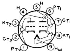
vices. Outline 11, OUTLINES SECTION. Tube requires noval nine-contact socket and may be mounted in any position. Its characteristics are similar to glass-octal type 6SN7-GT. Each triode unit is independent of the other except for the common heater. For typical operation as a resistance-coupled amplifier, refer to Chart 10, RESISTANCE-COUPLED AMPLIFIER SECTION.
