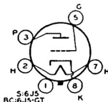
high amplification factor. Outlines 3 and 19, respectively, OUTLINES SECTION. Tubes require octal socket and may be mounted in any position. For heater and cathode considerations, refer to type 6AT6. For typical operation as a resistance-coupled amplifier, refer to Chart 13, RESISTANCE COUPLED AMPLIFIER SECTION.
