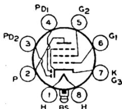
grid-No.1 volts, -1 (0 min); plate resistance (approx.), 1.0 megohm; transconductance, 3400 μmhos; plate ma., 6.2; grid-No.2 ma., 1.6, grid-No.1 volts for transconductance of 2 μmhos, -20. Refer to type 6SQ7 for diode operation curves.
