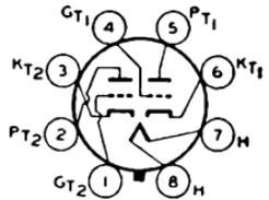
any position. Except for the common heater, each triode unit is independent of the other. For typical operation as phase inverter or resistance-coupled amplifier, refer to Chart 7, RESISTANCE-COUPLED AMPLIFIER SECTION. For heater and cathode considerations, refer to type 6AT6.
