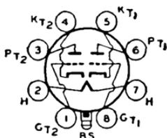
Glass lock-in type used as amplifier or oscillator in radio equipment. Except for overall length of 2-9/32 inches and seated height of 1 1/4 inches, the dimensions of type 7F8 are given by Outline 12, OUTLINES SECTION. Tube requires lock-in socket. Heater volts (ac/dc), 6.3; amperes, 0.3. Typical operation and maximum ratings as class A<sub>1</sub> amplifier (per unit): plate
