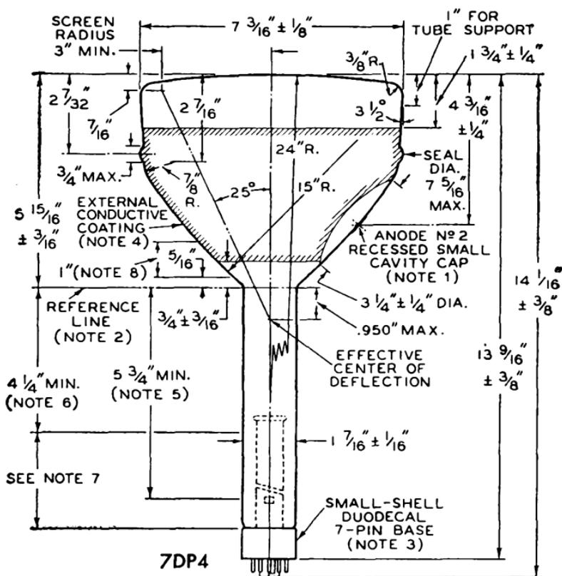
NOTE 1: The plane through the tube axis and vacant pin position No.3 may vary from the plane through the tube axis and anode-No.2 terminal by an angular tolerance (measured about the tube axis) of 10°. Anode-No.2 terminal is on same side as vacant pin position No.3.
