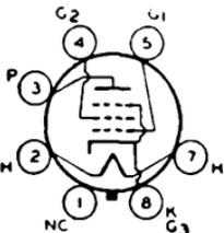
Glass octal type used in output stage of radio receivers. It is capable of delivering moderate power output with relatively small input voltage. Tube may be used singly or in push-pull.
