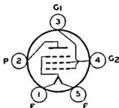
Glass type used in output stage of automobile receivers. Outline 29, OUTLINES SECTION. Tube requires five-contact socket. Filament volts (ac/dc), 6.3; amperes, 0.3. Typical operation: plate and grid-No. 2 volts, 180 max; grid-No. 1 volts, -12; plate ma., 22; grid-No. 2 ma., 3.9; plate resistance, 45500 ohms approx.; transconductance, 2200 μmhos; load resistance, 8000 ohms; cathode-bias resistor, 465 ohms; output watts, 1.4. This type is used principally for renewal purposes.
