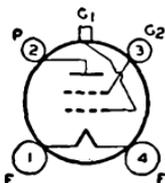
Glass type used as *rf* amplifier or biased detector in battery-operated receivers. Outline 32, OUTLINES SECTION. Tube requires four-contact socket. Filament volts (dc), 2.0; amperes, 0.06. Typical operation as class A<sub>1</sub> amplifier: plate volts, 180 *max*; grid-No.2 ma., 0.4 *max*; plate resistance, greater than 1 megohm; plate ma., 1.7; transconductance, 650  $\mu$ mhos. This type is used principally for renewal purposes.
