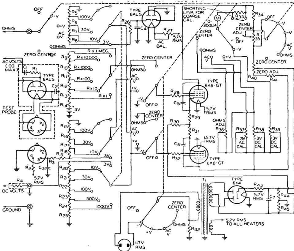
C<sub>1</sub> C<sub>3</sub> = 0.05 μf, oil-filled, 600 v.
