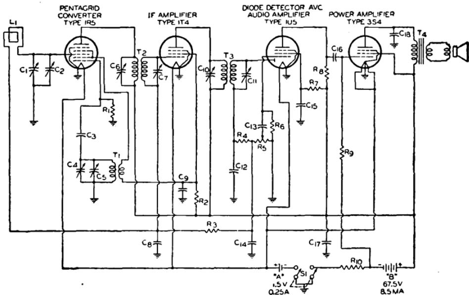
C<sub>1</sub> C<sub>4</sub> = Ganged tuning capacitors: C<sub>1</sub>, 10-274  $\mu\text{f}$ ; C<sub>4</sub>, 7.5-122.5  $\mu\text{f}$
