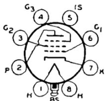
Glass lock-in type used as rf amplifier in ac/dc receivers or in mobile equipment where low heater-current drain is important. Outline 12, OUTLINES SECTION. Tube requires lock-in socket. Heater volts (ac/dc), 6.3; amperes, 0.15. Maximum ratings and characteristics as class A<sub>1</sub> amplifier: plate and grid-No.2 volts, 250 (300 max); plate dissipation, 2 max watts; grid-No.2 dissipation, 0.75 max watt;
