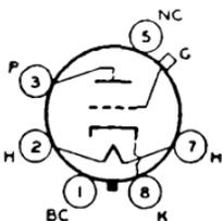
Glass octal type used as voltage amplifier in radio equipment. Outline 18, OUTLINES SECTION. Tube requires octal socket. Heater volts (ac/dc), 6.3; amperes, 0.3. Characteristics as class A<sub>1</sub> amplifier: plate volts, 250 max; grid volts, -3; amplification factor, 70; plate resistance, 50000 ohms; transconductance, 1400 μmhos; plate ma., 1.1. This type is used principally for renewal purposes.
