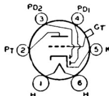
resistance, 20000 ohms; output watts, 0.35. For typical operation as a resistance-coupled amplifier, refer to Chart 22, RESISTANCE-COUPLED AMPLIFIER SECTION. This type is used principally for renewal purposes.
