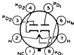
between pins 2 and 7), 2. Maximum ratings as rectifier or doubler: peak inverse plate volts, 700 *max*; peak plate ma. per plate, 400 *max*; dc output ma. per plate with panel lamp, 65 *max*; peak heater-cathode volts, 350 *max*; panel lamp section volts (pins 6 and 7), 2.5 *max*. This is a DISCONTINUED type listed for reference only.
