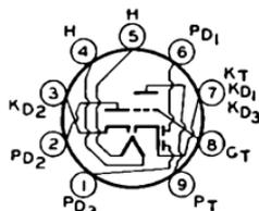
requires noval nine-contact socket and may be mounted in any position. Heater volts (ac/dc), 18.9; amperes, 0.15. Except for heater rating, this type is identical with miniature type 6T8.
