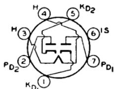
Miniature, high-perveance type used as detector in FM and television circuits. It is especially useful as a ratio detector in ac/dc FM receivers. Outline 8, OUTLINES SECTION.
