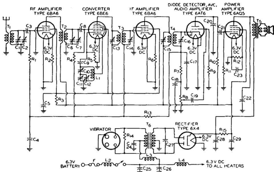
C<sub>1</sub> C<sub>7</sub> C<sub>11</sub> = Ganged tuning capacitors, 365  $\mu\text{mf}$
