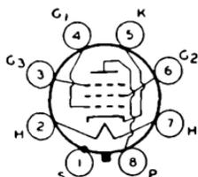
Metal type used in rf and if stages of picture amplifier of television receivers particularly those employing automatic-gain control. Outline 3, OUTLINES SECTION. Tube requires octal socket. Heater volts (ac/dc), 6.3; amperes, 0.45. Maximum ratings as class A<sub>1</sub> amplifier: plate and grid-No. 2 supply volts, 300 *max*; grid-No. 2 volts, 200 *max*; plate dissipation, 3.75 *max* watts; grid-No. 2 dissipation, 0.7 *max*
