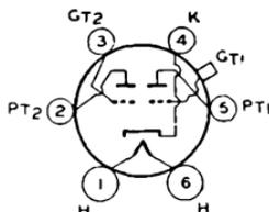
(plate-to-plate), 14000 ohms; output watts (approx.), 8; peak plate ma. per plate, 90 *max*; average plate dissipation, 11.5 watts *max*. For typical operation as a resistance-coupled amplifier, refer to Chart 24, RESISTANCE-COUPLED AMPLIFIER SECTION. This type is used principally for renewal purposes.
