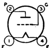
Glass type used in output stage of radio receivers. Outline 34, OUTLINES SECTION. Tube requires four-contact socket. Except for filament rating (6.3 volts ac/dc; 1.0 ampere) and slightly lower power output, type 6A3 is identical electrically with type 2A3. This type is used principally for renewal purposes.
