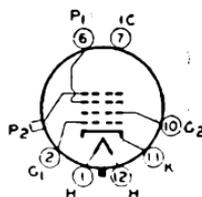
deflection to provide a picture of about 4 by 5-1/2 inches. Has solid deflection angle of 50° approx. Maximum bulb diameter is 7-5/16 inches; maximum overall length, 14-7/16 inches. Outline 38, OUTLINES SECTION. Tube has small-shell duodecal 7-pin base and recessed small cavity cap.
