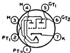
SECTION. Tube requires miniature seven-contact socket and may be mounted in any position. For direct interelectrode capacitances, ratings, and typical operation as a class A<sub>1</sub> amplifier, and curves, refer to type 6J6.
