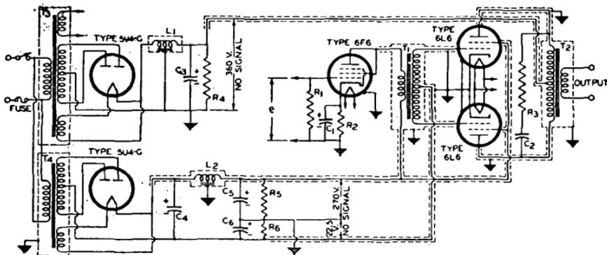
C<sub>1</sub> C<sub>2</sub> = 25 μf, electrolytic, 25 v.
