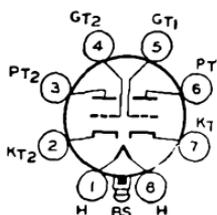
Glass lock-in type used as voltage amplifier or phase inverter in radio equipment. Outline 12, OUTLINES SECTION. Tube requires lock-in socket. Heater volts (ac/dc), 6.3; amperes, 0.3. Ratings and characteristics as class A<sub>1</sub> amplifier (each section): plate volts, 250 (300 max); cathode resistor, 1100 ohms; plate ma., 9; transconductance, 2100 μmhos; amplification factor, 16; plate resistance, 7600 ohms.
