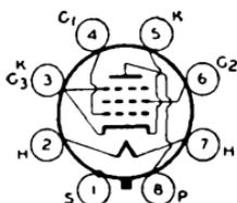
Metal type used as rf amplifier in ac/dc receivers involving high-frequency, wide-band applications and as limiter tube in FM equipment. Outline 3, OUTLINES SECTION. Heater volts (ac/dc), 12.6; amperes, 0.15. Except for heater rating, this type is identical with metal type 6SH7.
