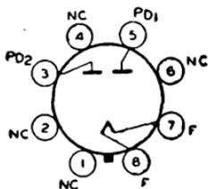
Glass octal type used in power supply of radio equipment having moderate dc requirements. Outline 28, OUTLINES SECTION. Tube requires octal socket. Vertical tube mounting is preferred, but horizontal mounting is permissible if pins 2 and 7 are in horizontal plane. Filament volts (ac), 5.0; amperes, 2.0. For maximum ratings, typical operation, and curves, refer to type 5Y3-GT.
