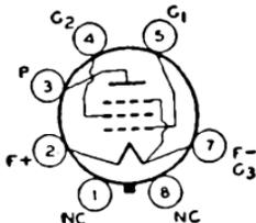
Glass octal type used in output stage of battery-operated receivers. Outline 17, OUTLINES SECTION. Tube requires octal socket and may be mounted in any position. For filament considerations, refer to 1U4.
