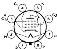
Metal type used as rf amplifier in ac/dc receivers involving high-frequency, wide-band applications. Outline 3, OUTLINES SECTION. Heater volts (ac/dc), 12.6; amperes, 0.15. Except for heater rating, this type is identical with metal type 6SG7.
