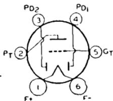
Glass type used as combined detector, amplifier, and avc tube in battery-operated receivers. Outline 25, OUTLINES SECTION. Tube requires six-contact socket. Filament volts (dc), 2.0; amperes, 0.06. Typical operation as class A<sub>1</sub> amplifier: plate volts, 135 *max*; grid volts, -3; plate ma., 0.8; plate resistance 35000, ohms; amplification factor, 20; transconductance, 575  $\mu$ mhos. This type is used principally for renewal purposes.
