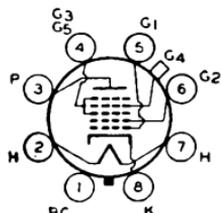
Glass octal type used as converter in ac/dc receivers. Outline 18, OUTLINES SECTION. Heater volts (ac/dc), 12.6; amperes, 0.15. Except for heater rating, this type is identical with glass-octal type 6A8-GT.
