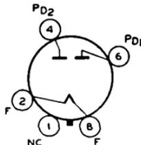
is permissible if pins 2 and 8 are in horizontal plane. It is especially important that this tube, like other power-handling tubes, should be adequately ventilated.
