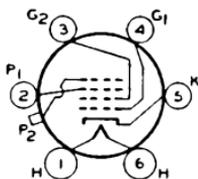
Directly viewed picture tube used in television receivers. Features white fluorescent screen having medium persistence and high efficiency. It utilizes electrostatic focus and magnetic deflection to provide a picture about 7 $\frac{3}{8}$  by 9 $\frac{3}{8}$  inches. Maximum diameter is 12-3/16 inches; maximum overall length is 25-3/8 inches. Tube requires six-contact socket. For
