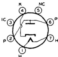
Miniature type used in power supply of small, portable, ac/dc/battery receivers where small size and low heat dissipation are important. Outline 10, OUTLINES SECTION. Tube requires miniature seven-contact socket and may be mounted in any position.
