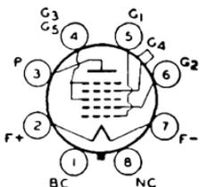
Glass octal type used in superheterodyne circuits having battery power supply. Outline 18, OUTLINES SECTION. Filament volts (dc), 1.4; amperes, 0.1. This is a DISCONTINUED type listed for reference only. The 1B7-GT may be replaced by the 1A7-GT if circuit adjustment is made for lower filament current of type 1A7-GT.
