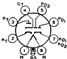
Glass lock-in type used as FM detector and audio amplifier in circuits which require diode and triode units with separate cathodes. Outline 12, OUTLINES SECTION. Tube requires lock-in socket. Heater volts (ac/dc), 6.3; amperes, 0.3. For ratings and typical operation, refer to glass-octal type 6AQ7-GT.
