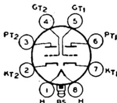
Glass lock-in type used as phase inverter or resistance-coupled amplifier. Outline 12, OUTLINES SECTION. Tube requires lock-in socket. Heater volts (ac/dc), 6.3; amperes, 0.3. For maximum ratings, typical operation as class A<sub>1</sub> amplifier, and curves, refer to glass-octal type 6SL7-GT.
