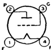
1700  $\mu$ mhos; load resistance, 4800 ohms; undistorted output watts, 0.79. This type is used principally for renewal purposes.
