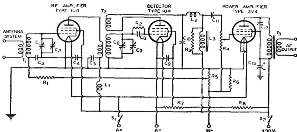
$C_1$   $C_6$  = Midget tuning capacitors, 140  $\mu\text{f}$
