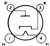
Heater volts (ac/dc), 12.6; amperes, 0.3. Maximum ratings as half-wave rectifier: peak inverse plate volts, 700 *max*; peak plate ma., 330 *max*; dc output ma., 55 *max*; peak heater-cathode volts, 350 *max*. With typical operating ac plate voltages of 117, 150, and 235 volts RMS, the minimum total effective plate-supply impedance required is 0, 30, and 75 ohms, respectively.
