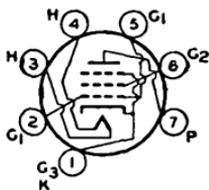
Miniature type used as output amplifier primarily in automobile and in ac-operated receivers. Outline 13, OUTLINES SECTION. Tube requires miniature seven-contact socket and may be mounted in any position. For heater and cathode considerations, refer to type 6AQ5. For curves, refer to type 35B5.
