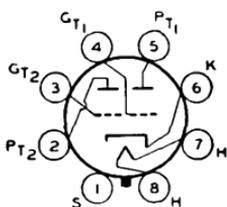
Metal type used as phase inverter or voltage amplifier in radio equipment. Except for common cathode, each triode is independent of the other. Outline 3, OUTLINES SECTION.
