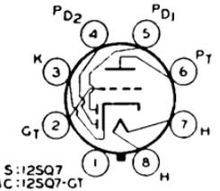
Heater volts (ac/dc), 12.6; amperes, 0.15. Except for heater rating, type 12SQ7 is identical with metal type 6SQ7, and type 12SQ7-GT is identical with glass-octal type 6SQ7-GT.
