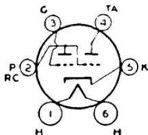
Glass type used to indicate visually by means of a fluorescent target the effects of a change in a controlling voltage. It is used as a convenient means of indicating accurate radio-receiver tuning. Outline 23, OUTLINES SECTION. Tube requires six-contact socket. For heater and cathode considerations, refer to type 6AT6. Heater volts (ac/dc), 6.3; amperes, 0.15. Ratings: plate-supply volts, 180 *max*; target volts 180 *max*, 125 *min*.
