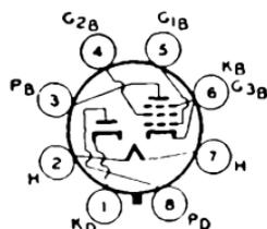
Glass octal type used as combined half-wave rectifier and output amplifier in ac/dc receivers. Outline 21, OUTLINES SECTION. Tube requires octal socket. Heater volts (ac/dc), 70; amperes, 0.15. Maximum ratings of rectifier unit: peak inverse plate volts, 350; peak plate ma., 420; dc output ma., 70; peak heater-cathode volts, 175; minimum total effective
