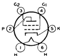
Glass type used in audio output stage of radio receivers designed to operate from dc powerlines. Outline 34, OUTLINES SECTION Heater volts (dc), 30; amperes, 0.4. Typical operation as class A<sub>1</sub> amplifier: plate volts, 125 *max*; grid-No.2 volts, 100 *max*; grid-No.1 volts, -20; plate ma., 56; grid-No.2 ma., 9.5; transconductance, 3900  $\mu$ mhos; load resistance, 1500 ohms; output watts, 2.5. This is a DISCONTINUED type listed for reference only.
