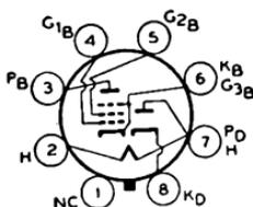
any position. Heater volts (ac/dc), 117; amperes, 0.09. When the amplifier unit is operated at maximum rated conditions, the grid circuit should have a dc resistance not higher than 0.25 megohm for fixed bias; for higher values, cathode bias is required. With cathode bias, the grid circuit may have a dc resistance as high as, but not higher than, 1.0 megohm.
