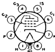
0.8 max watt; grid No.3 connected to cathode at socket; cathode-bias resistor, 160 min ohms; plate resistance, 0.3 megohm; transconductance, 5800 μmhos; plate ma., 10; grid-No.2 ma., 3.9; grid-No.1 volts for plate current of 10 μa., -16. The application of this type is similar to that of miniature type 6AU6.
