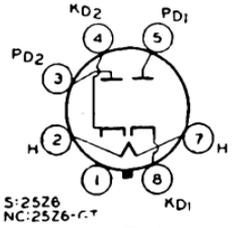
doubler type. Outlines 6 and 17, respectively, OUTLINES SECTION. Tubes require octal socket and may be mounted in any position.
