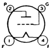
Glass type used in output stage of af amplifiers employing transformer input coupling. Outline 36, OUTLINES SECTION. Tube requires four-contact socket and should be mounted in vertical position with base down. Filament volts (ac/dc), 7.5; amperes, 1.25. Characteristics as class A<sub>1</sub> amplifier: plate volts, 450 *max*; grid volts, -84; cathode resistor, 1530 ohms; plate ma., 55; plate resistance, 1800 ohms; amplification factor, 3.8; transconductance, 2100  $\mu$ mhos;
