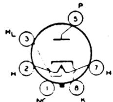
octal socket and may be mounted in any position. For installation and application considerations, refer to miniature type 35W4.
