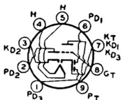
Miniature type used as combined audio amplifier, AM detector, and FM detector in AM/FM radio receivers. Diode unit No.1 is used for AM detection, and diode units No.2 and No.3
