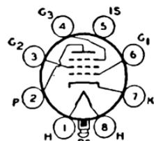
Glass lock-in type used in video amplifiers of television receivers and in other applications requiring high transconductance. Outline 12, OUTLINES SECTION. Tube requires lock-in socket. Heater volts (ac/dc), 6.3; amperes, 0.45. Typical operation and maximum ratings as class A<sub>1</sub> amplifier: plate volts, 250 (300 *max*); grid-No.2 volts, 100 *max*; plate dissipation, 1.5
