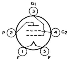
amplification factor, 5.6; transconductance, 2350  $\mu$ mbos; load resistance for maximum undistorted power output, 6400 ohms; undistorted output watts, 1.25.
