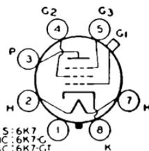
LINES SECTION. These tubes require octal socket and may be mounted in any position. For voltage supplies and application, refer to type 6SK7. For heater and cathode considerations, refer to type 6AT6.
