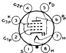
Metal type used as combined rf or if amplifier and detector or avc tube in ac/dc radio receivers. Outline 3, OUTLINES SECTION. Heater volts (ac/dc), 12.6; amperes, 0.15. Except for heater rating, this type is identical with metal type 6SF7.
