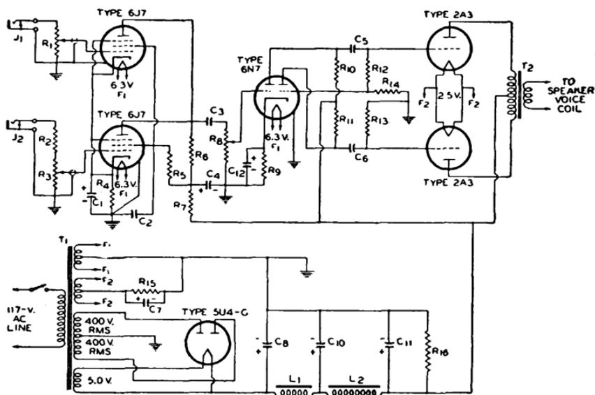
$C_1 = 10 \mu\text{f}$ , electrolytic, 25v.
