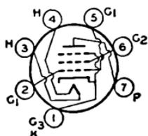
Miniature type used in output stage of compact, ac/dc radio receivers. Because of its high power sensitivity and high efficiency at plate and screen voltages available in ac/dc receivers, the 50C5 is capable of providing a relatively high power output. Outline
