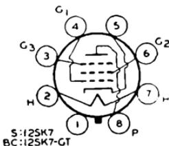
Metal type 12SK7 and glass-octal type 12SK7-GT used as rf and if amplifiers in ac/dc radio receivers. Outlines 3 and 19, respectively, OUTLINES SECTION. Heater volts (ac/dc), 12.6; amperes, 0.15. Except for heater rating, type 12SK7 is identical with metal type 6SK7, and type 12SK7-GT is identical with glass-octal type 6SK7-GT.
