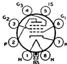
resistor, 68 ohms; plate ma., 28; grid-No.2 ma., 7; plate resistance ,30000 ohms; transconductance, 9590  $\mu$ mhos.
