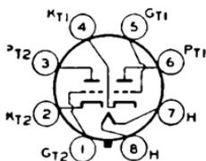
Glass octal tube used as audio amplifier in radio equipment. Outline 14, OUTLINES SECTION. Tube requires octal socket. Heater volts (ac/dc), 12.6; amperes, 0.15. Typical operation as class A<sub>1</sub> amplifier: plate volts, 180 *max*; grid volts, -6.5; amplification factor, 16; transconductance, 1900  $\mu$ mhos; plate resistance, 8400 ohms; plate ma., 7.6; grid-bias volts for plate current of 10  $\mu$ a, -16.
