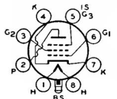
Glass lock-in type used as rf or if amplifier in radio receivers. Outline 15, OUTLINES SECTION. Tube requires lock-in socket. Heater volts (ac/dc), 6.3; amperes, 0.45. This type is the same as type 7V7 except for socket connections.
