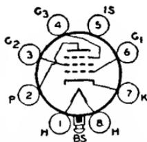
ma., 1.7; plate resistance, 0.75 megohm; transconductance, 1750  $\mu$ mhos; transconductance at bias of -40 volts, 10  $\mu$ mhos. The application of this type is similar to that of metal types 6SK7 and 6SS7.
