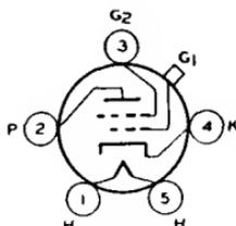
Glass type used as rf or if amplifier in ac receivers. Outline 41, OUTLINES SECTION. Tube requires five-contact socket. Heater volts (ac/dc), 2.5; amperes, 1.75. Characteristics as class A<sub>1</sub> amplifier: plate volts, 250 (275 *max*); grid-No.2 volts, 90 *max*; grid-No.1 volts, -3 *min*; plate ma., 6.5; grid-No.2 ma., 2.5; transconductance, 1050  $\mu$ mhos; transconductance at
