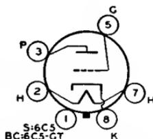
plate volts, 300 *max*; plate dissipation, 2.5 *max* watts; grid volts, 0 *min*. Typical operation: plate volts, 250; grid volts, -8 (grid-circuit resistance should not exceed 1.0 megohm); amplification factor, 20; plate resistance, 10000 ohms; transconductance, 2000  $\mu$ mhos; plate ma., 8. For typical operation as a resistance-coupled amplifier, refer to Chart 11, RESISTANCE-COUPLED AMPLIFIER SECTION. Type 6C5-GT is used principally for renewal purposes.
