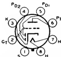
Metal type used as combined detector, amplifier, and AVC tube in radio receivers. Except for heater-current rating and interelectrode capacitances, this type is essentially the same electrically as type 6AT6. Outline 3, OUTLINES SECTION. Tube requires octal socket and may be mounted in any position. Heater volts (ac/dc), 6.3; amperes, 0.15. Direct interelectrode capacitances of triode unit (shell connected to cathode):
