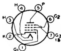
Tube requires miniature seven-contact socket and may be mounted in any position. For heater and cathode considerations, refer to type 6AV6.
