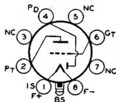
Glass lock-in type used as combined detector and amplifier in battery-operated receivers. Outline 15, OUTLINES SECTION. Tube requires lock-in socket. Filament volts (dc), 1.4; amperes, 0.05. For electrical characteristics, refer to glass-octal type 1H5-GT.
