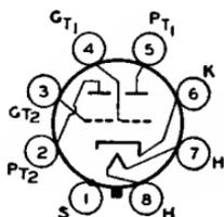
Metal type used as phase inverter or voltage amplifier in ac/dc radio equipment. Outline 3, OUTLINES SECTION. Heater volts (ac/dc), 12.6; amperes, 0.15. Except for heater rating, this type is identical with metal type 6SC7.
