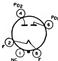
but horizontal mounting is permissible if pins 1 and 4 are in vertical plane. The coated filament is designed to operate from the ac line through a step-down transformer. The voltage at the filament terminals should be 5.0 volts under operating conditions at an average line voltage of 117 volts. It is especially important that this tube, like other power-handling tubes, be adequately ventilated. For discussion of Rating Chart and Operation Characteristics, refer to type 6AX5-GT.
