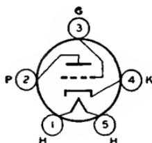
Glass type used as detector or class A<sub>1</sub> amplifier in radio receivers. Outline 34, OUTLINES SECTION. Heater volts (ac/dc), 3; amperes, 1.25. Characteristics: plate volts, 180; grid volts, -9; amplification factor, 12.5; plate resistance, 8900 ohms; transconductance, 1400  $\mu$ mhos; plate ma., 5.8. This is a DISCONTINUED type listed for reference only.
