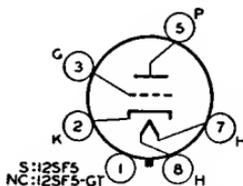
Metal type 12SF5 and glass-octal type 12SF5-GT used in resistance-coupled amplifier circuits of ac/dc radio equipment. Outlines 3 and 23, respectively, OUTLINES SECTION. Type 12SF5-GT may be supplied with pin No. omitted. Heater volts (ac/dc), 12.6; amperes, 0.15. Except for heater rating, type 12SF5 is identical with metal type 6SF5, and type
