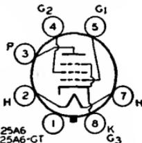
volts, 160; grid-No.2 volts, 135; plate dissipation, 5.3 watts; grid-No.2 input, 1.9 watts. Type 25A6 is used principally for renewal purposes. Type 25A6-GT is a DISCONTINUED type listed for reference only.
