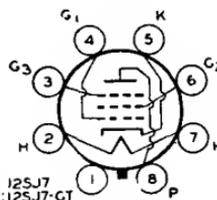
Heater volts (ac/dc), 12.6; amperes, 0.15. Except for heater rating, type 12SJ7 is identical with metal type 6SJ7, and type 12SJ7-GT is identical with glass-octal type 6SJ7-GT. Type 12SJ7-GT is a DISCONTINUED type listed for reference only.
