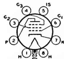
maz watt; grid No.1 volts, -3; grid No.3 connected to cathode at socket; plate resistance, greater than 1 megohm; transconductance, 1575  $\mu$ mhos; plate ma., 2.2; grid-No.2 ma., 0.7. Within the limits of its maximum ratings, this type is similar in performance to metal types 6SJ7 and 12SJ7.
