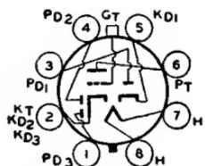
Glass octal type used as audio amplifier, AM detector, and FM detector in AM/FM receivers. Diode unit No.2 is used for AM detection, and diode units No.1 and No.3 are used for FM detection. The grid of the high-mu triode is brought out to a top cap. Outline 28-OUTLINES SECTION. Tube requires octal socket and may be mounted in any position. For
