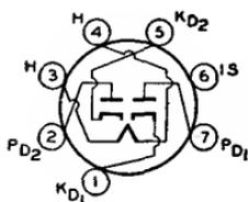
Miniature, high-perveance type used as detector in FM and television circuits. It is especially useful as a ratio detector in ac/dc FM receivers. Outline 9, OUTLINES SECTION. Heater volts (ac/dc), 12.6; amperes, 0.15. Except for heater rating, this type is identical with miniature type 6AL5.
