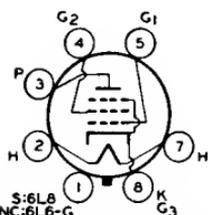
Metal type 6L6 and glass-octal type 6L6-G are used in output stage of radio receivers and amplifiers, especially those designed to have ample reserve of power-delivering ability.
