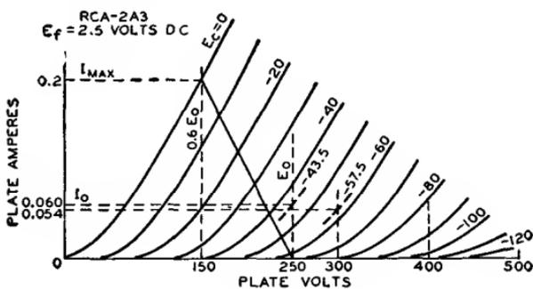
The method for calculating maximum power output for **triodes in push-pull class A operation** is as follows: Erect a vertical line at  $0.6E_0$  (see Fig. 22), intersecting the  $E_c=0$  curve at the point  $I_{max}$ . Then,  $I_{max}$  is determined from the curve for use in the formula
