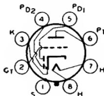
Metal type used as combined detector, amplifier, and AVC tube. Within maximum ratings this type is electrically identical to type 6BF6 except for interelectrode capacitances and heater current. Outline 3, OUTLINES SECTION. Tube requires octal socket and may be mounted in any position. Heater volts (ac/dc), 6.3; amperes, 0.15. Maximum ratings of triode
