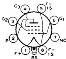
Glass lock-in type used as rf or if amplifier in battery-operated receivers. Outline 15, OUTLINES SECTION. Tube requires lock-in socket. Filament volts (dc), 1.4; amperes, 0.05. Typical operation as class A<sub>1</sub> amplifier: plate and grid-No.2 (screen) volts, 90 (110 max); grid-No.1 volts, 0; plate ma., 1.6; grid-No.2 ma., 0.35; plate resistance (approx.), 1.1 megohms; transconductance, 800 μmhos.
