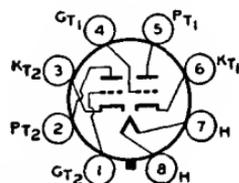
multivibrators, or resistance-coupled amplifiers in radio equipment. Outline 22, OUTLINES SECTION. Tubes require octal socket and may be mounted in any position. Except for the common heater, each triode unit is independent of the other. For typical operation as phase inverter or resistance-coupled amplifier, refer to Chart 13, RESISTANCE-COUPLED AMPLIFIER SECTION. For heater and cathode considerations, refer to type 6AQ5.
