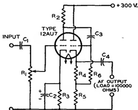
$C_1$   $C_3=0.1 \mu\text{f}$ , paper, 400 v.
