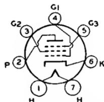
plate resistance, 2300 ohms; amplification factor, 6; transconductance, 2600; load resistance for maximum undistorted power output, 5000 ohms; undistorted output watts, 1.25. For typical operation as class A<sub>1</sub> amplifier (pentode connection; grid No.3 tied to cathode at socket), refer to type 6F6 with plate voltage of 250 volts. Type 59 is a DISCONTINUED type listed for reference only.
