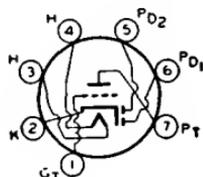
Miniature type used in compact radio equipment as combined detector, amplifier, and avc tube. The triode unit is particularly useful as a driver for impedance- or transformer-coupled
