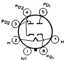
Glass octal type used as half-wave rectifier or voltage doubler in ac/dc receivers. This type is used particularly in "transformerless" receivers of either the ac/dc type or the voltage-doubler type. Outline 23, OUTLINES SECTION. This type may be supplied with pin No.1 omitted. Tube requires octal socket. Heater volts (ac/dc), 50; amperes, 0.15. Except for heater rating, this type is electrically identical with type 25Z6-GT.
