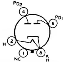
position. The heater is designed to operate from the ac line through a step-down transformer. The voltage at the heater terminals should be 5.0 volts under operating conditions at an average line voltage of 117 volts. It is especially important that this tube, like other power-handling tubes, be adequately ventilated.
