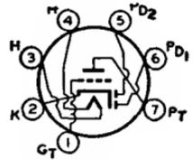
Heater volts (ac/dc), 12.6; amperes, 0.15. Except for heater rating, this type is identical with miniature type 6AV6.
