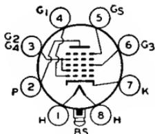
Glass lock-in type used as converter in superheterodyne circuits. Outline 15, OUTLINES SECTION. Tube requires lock-in socket. Heater volts (ac/dc), 6.3; amperes, 0.3. For maximum ratings, typical operation in converter service, and curves, refer to metal type 6SA7.
