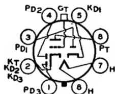
Glass octal type used as audio amplifier, AM detector, and FM detector in AM/FM receivers. Outline 28, OUTLINES SECTION. Heater volts (ac/dc), 12.6; amperes, 0.15. Except for heater rating, this type is identical with glass octal type 6S8-GT. Type 12S8-GT is a DISCONTINUED type listed for reference only.
