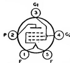
250 max; cathode-bias resistor, 450 ohms; plate ma., 31; grid-No.2 ma., 6; plate resistance, 60000 ohms; transconductance, 2500  $\mu$ mhos; load resistance, 7000 ohms; power output, 2.7 watts. This type is used principally for renewal purposes.
