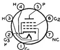
Miniature type used as output tube primarily in automobile receivers and ac-operated receivers. Outline 16, OUTLINES SECTION. Tube requires miniature seven-contact socket and may be mounted in any position. For heater and cathode considerations, refer to miniature type 6AQ5. Within its maximum ratings, type 6AR5 is equivalent in performance to glass-octal type 6K6-GT. Refer to type 6K6-GT for characteristic curves. Type 6AR5 is used principally for renewal purposes.
