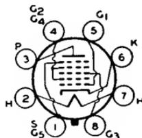
Metal type 12SA7 and glass-octal type 12SA7-GT used as converter in ac/dc receivers. Outlines 3 and 23, respectively, OUTLINES SECTION. Heater volts (ac/dc), 12.6; amperes, 0.15. Except for heater ratings, type 12SA7 is identical with metal type 6SA7, and type 12SA7-GT is identical with glass-octal type 6SA7-GT.
