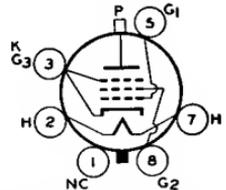
line 44, **OUTLINES SECTION**. Tube requires octal socket. Vertical tube mounting is preferred but horizontal operation is permissible if pins No.2 and 7 are in vertical plane.
