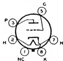
volts (ac/dc), 6.3; amperes, 0.4. Maximum ratings: plate volts, 250 *max*; peak plate ma. (per tube), 110 *max*; average plate dissipation, 10 *max* watts. This type is used principally for renewal purposes.
