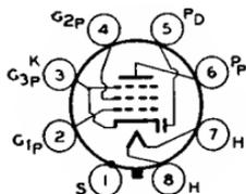
Metal type used as combined rf or if amplifier and detector or avc tube in ac/dc radio receivers. Outline 3, OUTLINES SECTION. Heater volts (ac/dc), 12.6; amperes, 0.15. Except for heater rating, this type is identical with metal type 6SF7.
