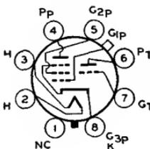
Glass octal type used as an amplifier. Outline 35, OUTLINES SECTION. Heater volts (ac/dc), 6.3; amperes, 0.3. Except for interelectrode capacitances, this type is identical electrically with type 6F7. Type 6P7-G is a DISCONTINUED type listed for reference only.
