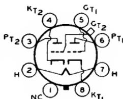
amperes, 0.3. Maximum ratings for each triode unit as class A<sub>1</sub> amplifier: plate volts, 250 *max*; grid volts, 0 *min*; plate dissipation, 1.0 *max* watt. Typical operation: plate volts, 250; grid volts, -4.5; plate ma., 3.2; plate resistance, 22500 ohms; amplification factor, 36; transconductance, 1600  $\mu$ mhos. For typical operation as a resistance-coupled amplifier, refer to Chart 12, RESISTANCE-COUPLED AMPLIFIER SECTION. This type is used principally for renewal purposes.
