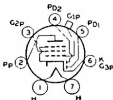
Glass type used as combined detector, avc tube, and amplifier. Outline 36, OUTLINES SECTION. Tube requires small seven-contact (0.75-inch, pin-circle diameter) socket. Except for its heater rating (2.5 volts ac/dc; 0.8 ampere) and its interelectrode capacitances, the 2B7 has electrical characteristics identical with type 6B8-G. Type 2B7 is a DISCONTINUED type listed for reference only.
