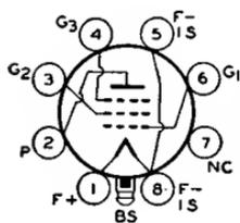
Lock-in type used as rf or if amplifier in battery-operated receivers. Outline 15, OUTLINES SECTION. Tube requires lock-in socket. Filament volts (dc), 1.4; amperes, 0.05. Typical operation and maximum ratings as class A<sub>1</sub> amplifier: plate volts, 90 (110 max); grid-No.2 volts, 45 (110 max); grid-No.1 volts, 0; plate resistance (approx.), greater than 1 megohm; transconductance, 800 μmhos; plate ma., 1.7; grid-No.2 ma., 0.4; grid-No.1 voltage for transconductance of 10 μmhos, -10 volts.
