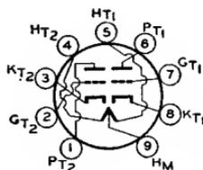
vices. Outline 14, **OUTLINES SECTION**. Tube requires noval nine-contact socket and may be mounted in any position. Its characteristics are similar to glass-octal type 6SN7-GT. Each triode unit is independent of the other except for the common heater. For typical operation as a resistance-coupled amplifier, refer to Chart 10, **RESISTANCE-COUPLED AMPLIFIER SECTION**.
