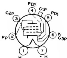
general, its electrical characteristics are similar to those of the 6B7, but the two types are usually not directly interchangeable. These are DISCONTINUED types listed for reference only.
