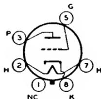
Glass octal type used as detector, amplifier, or oscillator in radio receivers. Outline 33, OUTLINES SECTION. Heater volts (ac/dc), 6.3; amperes, 0.15. Typical operation and characteristics: plate volts, 250 *max*; grid volts, -9; plate ma., 8; plate resistance, 9000 ohms; amplification factor, 17; transconductance, 1900  $\mu$ mhos; grid-bias volts for cathode-current cutoff, -20. This is a DISCONTINUED type listed for reference only.
