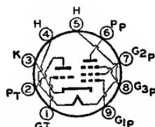
SECTION. Except for interelectrode capacitances and basing arrangement, this type is identical with miniature type 6X8. The basing arrangement of the 6AT8 is particularly suitable for connection to the coils of certain designs of turret tuners.
