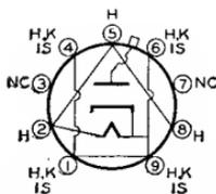
Miniature type used as rectifier of high-voltage pulses produced in the scanning systems of color television receivers. Outline 19, OUTLINES SECTION. Tube requires noval nine-
