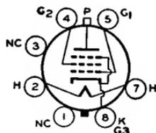
except seated height is 3 to 3-5/16 inches and over-all height is 3 7/8 max inches. Tube requires octal socket and may be mounted in any position. This type may be supplied with pin No.1 omitted.
