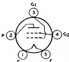
plification factor, 5.6; transconductance, 2350  $\mu$ mhos; load resistance for maximum undistorted power output, 6400 ohms; undistorted output watts, 1.25. This is a DISCONTINUED type listed for reference only.
