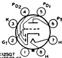
Metal type 12SQ7 and glass-octal type 12SQ7-GT used as combined detector, amplifier, and avc tube in ac/dc radio receivers. Outlines 3 and 25, respectively, OUTLINES SECTION.
