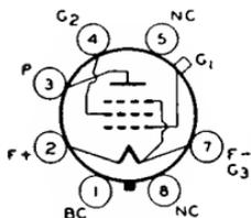
Glass octal type used as rf or if amplifier in battery-operated receivers. Outline 24, OUTLINES SECTION. Tube requires octal socket and may be mounted in any position. When used
