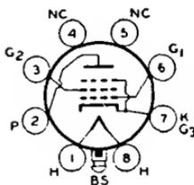
Glass lock-in type used in output stage of ac/dc receivers. Outline 20, OUTLINES SECTION. Tube requires lock-in socket. Heater volts (ac/dc), 35; amperes, 0.15. For ratings, and curves, refer to glass-octal type 35L6-GT. Type 35A5 is used principally for renewal purposes.
