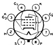
up to 18 megacycles per second (approx.). Two separate cathode terminals enable the input and output circuits to be effectively isolated from each other. Outline 3, OUTLINES SECTION. Tube requires octal socket and may be mounted in any position. For heater and cathode considerations, refer to type 6AV6.
