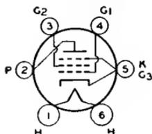
Glass type used in output stage of ac-operated receivers. Outline 38, OUTLINES SECTION. Tube requires six-contact socket. Except for its heater rating (2.5 volts ac/dc; 1.75 amperes), the 2A5 has electrical characteristics identical with type 6F6. Type 2A5 is a DISCONTINUED type listed for reference only.
