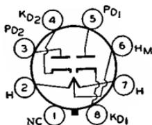
Glass octal type used as half-wave rectifier or voltage doubler in ac/dc receivers. This type is used particularly in "transformerless" receivers of either the ac/dc type or the voltage-doubler type. The heater is provided with a tap for operation of a panel lamp. Outline 23, OUTLINES SECTION. Tube requires octal socket. For maximum ratings and typical operation as
