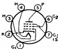
features very high transconductance combined with low interelectrode capacitance values, and is provided with separate base pins for grid No.3 and the cathode to permit the use of an unbypassed cathode resistor to minimize the effects of regeneration. Outline 13, OUTLINES SECTION. Tube requires miniature seven-contact socket and may be mounted in any position. For heater and cathode considerations, refer to type 6AV6.
