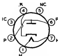
ma. 390 max; dc output ma., 65 max; peak heater-cathode volts, 175 max. Typical operation with capacitor-input filter: ac plate volts (rms), 117; minimum total effective plate-supply impedance, 15 ohms; dc output ma., 65. This is a DISCONTINUED type listed for reference only.
