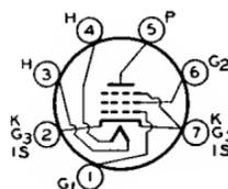
Miniature type used in compact radio equipment as an rf or if amplifier up to 400 megacycles per second. Outline 13, OUTLINES SECTION. Tube requires miniature seven-contact socket and may be mounted in any position. The two cathode leads facilitate isolation of the input and output circuits thus helping to minimize degeneration. For heater and cathode considerations, refer to type 6AV6.
