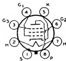
ical operation: plate and grid-No.2 supply volts, 300; grid-No.3 volts, 0; grid-No.2 series resistor, 30000 ohms; grid-No.1 volts, -3; plate resistance (approx.), 0.7 megohm; transconductance, 5000  $\mu$ mhos; grid-No.1 volts for transconductance of 50  $\mu$ mhos, -15; plate ma., 12.5; grid-No.2 ma., 3.2. This type is used principally for renewal purposes.
