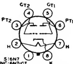
as a class B amplifier. Outlines 6 and 23, respectively, OUTLINES SECTION. Tubes require octal socket and may be mounted in any position. For typical operation as a resistance-coupled amplifier, refer to Chart 6, RESISTANCE-COUPLED AMPLIFIER SECTION. For class B amplifier considerations, refer to ELECTRON TUBE APPLICATIONS SECTION. Type 6N7 is used principally for renewal purposes.
