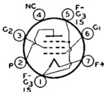
Miniature type used in lightweight, compact, portable, battery-operated receivers as rf or af amplifier. Because of internal shielding feature, an external bulb shield is not needed,
