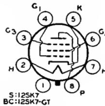
(ac/dc), 12.6; amperes, 0.15. Except for heater rating, type 12SK7 is identical with metal type 6SK7, and type 12SK7-GT is identical with glass-octal type 6SK7-GT. Type 12SK7-GT is used principally for renewal purposes.
