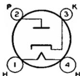
Glass type used in ac/dc or automobile receivers. Outline 31 or 34, OUTLINES SECTION. Tube requires four-contact socket. For heater considerations, refer to type 6AT6. Heater volts (ac/dc), 6.3; amperes, 0.3. Maximum ratings as half-wave rectifier: peak in verse plate volts, 1000; peak plate ma., 270; peak heater-cathode volts, 500; dc output ma., 45. This type is used principally for renewal purposes.
