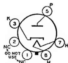
29, OUTLINES SECTION. Tube requires octal socket and may be mounted in any position. This type may be supplied with pin No.1 omitted. It is especially important that this tube, like other power-handling tubes, be adequately ventilated. For curve of average plate characteristics, see page 61.
