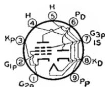
used as an audio detector, video detector, or dc restorer. Outline 14, **OUTLINES SECTION**. Tube requires miniature nine-contact socket and may be mounted in any position. For curve of average plate characteristics of pentode unit, see type 6AN8.
