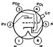
Glass type used in ac-operated receivers chiefly as a combined detector, amplifier, and avc tube. Outline 36, OUTLINES SECTION. Tube requires six-contact socket. Except for its heater rating (2.5 volts ac/dc; 0.8 ampere), and within its 250-volt maximum plate rating, the 2A6 has electrical characteristics identical with type 6SQ7. Type 2A6 is a DISCONTINUED type listed for reference only.
