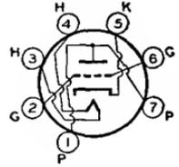
miniature seven-contact socket and may be mounted in any position.
