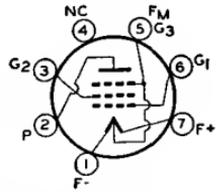
filament mid-tap so that tubes may be used either with a 1.4-volt battery supply or in series with other miniature tubes having 0.050-ampere filaments.
