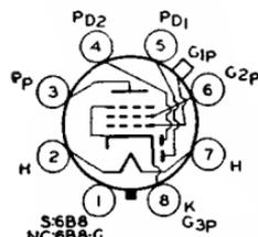
Heater volts (ac/dc), 6.3; amperes, 0.3. Maximum ratings of pentode unit as class A<sub>1</sub> amplifier: plate volts, 300 *max*; grid-No.2 (screen) volts, 125 *max*; grid-No.2 supply volts, 300 *max*; grid-No.1 volts, 0 *min*; plate dissipation, 3.0 *max* watts (6B8), 2.25 *max* watts (6B8-G); grid-No.2 input, 0.3 *max* watt. For typical operation as a resistance-coupled amplifier, refer to Chart 5, RESISTANCE-COUPLED AMPLIFIER SECTION.
