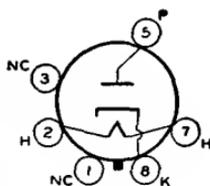
plate volts, 350 *max*; peak plate ma., 540 *max*; peak heater-cathode volts, 175 *max*. Typical operation with capacitor-input filter: ac plate supply volts (rms), 117; minimum total effective plate-supply impedance, 30 ohms; dc output ma., 90. This is a DISCONTINUED type listed for reference only.
