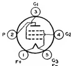
load resistance, 6000 ohms; output watts, 1.4. This is a **DISCONTINUED** type listed for reference only.
