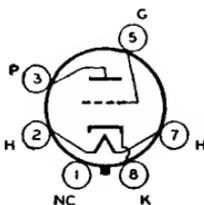
Glass octal type used as detector, amplifier, or oscillator in radio receivers. Outline 23, OUTLINES SECTION. This type may be supplied with pin No.1 omitted. Tube requires octal socket. Heater volts (ac/dc), 6.3; amperes, 0.3. Except for interelectrode capacitances, this type is identical electrically with type 76. Type 6P5-GT is a DISCONTINUED type listed for reference only.
