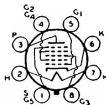
version in ELECTRON TUBE APPLICATIONS SECTION. Outline 3, OUTLINES SECTION. Tube requires octal socket and may be mounted in any position. For heater and cathode considerations, refer to type 6AV6. Type 6SB7-Y is used principally for renewal purposes.
