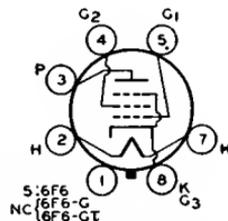
Outlines 6, 37, and 27, respectively, **OUTLINES SECTION**. Type 6F6-GT may be supplied with pin No.1 omitted. Tubes require octal socket and may be mounted in any position. It is especially important that these tubes, like other power-handling tubes, be adequately ventilated. Type 6F6-G is used principally for renewal purposes.
