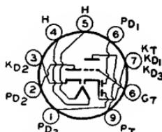
are used for FM detection. Outline 14, OUTLINES SECTION. Tube requires noval nine-contact socket and may be mounted in any position. For typical operation as a resistance-coupled amplifier, refer to Chart 7, RESISTANCE-COUPLED AMPLIFIER SECTION. For heater and cathode considerations, refer to type 6AQ5.
