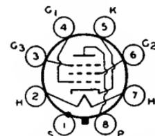
Metal type used in rf or if stages of radio receivers particularly those employing AVC. Outline 3, OUTLINES SECTION. Tube requires octal socket and may be mounted in any position. For heater and cathode considerations, refer to type 6AV6. Heater volts (ac/dc), 6.3; amperes, 0.15. Typical operation and maximum ratings as class A<sub>1</sub> amplifiers: plate volts, 250 (300 *max*), grid-No.2 supply volts, 300 *max*;
