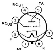
Glass octal type used to indicate visually, by means of two shadows on the fluorescent target, the effects of changes in the controlling voltages. It is a twin-indicator type and is used as a convenient means of indicating accurate radio-receiver tuning. Outline 12, OUTLINES SECTION. This type may be supplied with pin No.1 omitted. Tube requires octal socket.
