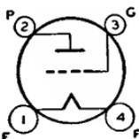
Glass type used as resistance-coupled or impedance-coupled amplifier in battery-operated receivers. Outline 38, OUTLINES SECTION. Filament volts (dc), 5; amperes, 0.25. Characteristics as class A<sub>1</sub> amplifier: plate-supply volts, 180; load resistance, 250000 ohms; grid volts, -3; plate ma., 0.2; plate resistance, 150000 ohms; amplification factor, 30; transconductance, 200  $\mu$ mhos. This is a DISCONTINUED type listed for reference only.
