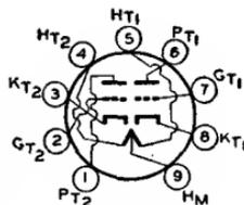
contact socket and may be mounted in any position. Each triode unit is independent of the other except for the common heater.
