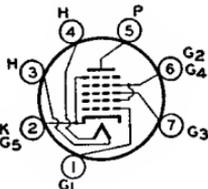
TION. Tube requires miniature seven-contact socket and may be mounted in any position.
