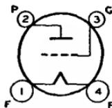
ma., 55; plate resistance, 1800 ohms; amplification factor, 3.8; transconductance, 2100  $\mu$ mhos; load resistance, 4350 ohms; output watts, 4.6. Resistance in grid-coupling circuit should not exceed 10000 ohms. This is a DISCONTINUED type listed for reference only.
