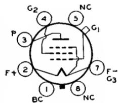
volts on grid-No.1, 10 μmhos; plate ma., 2.3; grid-No.2 ma., 0.7. This is a DISCONTINUED type listed for reference only.
