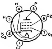
providing a relatively high power output. Outline 16, OUTLINES SECTION. Tube requires miniature seven-contact socket and may be mounted in any position. Within its maximum ratings, type 50B5 is equivalent in performance to glass-octal type 50L6-GT and miniature type 50C5. Refer to type 50C5 for maximum ratings, typical operation, maximum circuit values, installation, application information, and curves.
