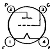
5000 ohms; transconductance, 1600  $\mu$ mhos; load resistance, 10200 ohms; undistorted output watts, 1.6. This is a **DISCONTINUED** type listed for reference only. Replace by transmitting type 10-Y.
