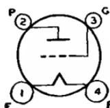
Glass type used in output stage of radio receivers. Outline 38, OUTLINES SECTION. Filament volts (ac/dc), 5.0; amperes, 1.25. Characteristics: plate volts, 250; grid volts, -60; plate ma., 30; amplification factor, 3; plate resistance, 1750 ohms; transconductance, 1700  $\mu$ mhos; load resistance, 5000 ohms; output watts, 1.8. This is a DISCONTINUED type listed for reference only.
