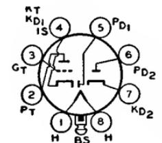
Glass lock-in type used as combined detector, amplifier, and avc tube in circuits which require diodes with separate cathodes. Outline 20, OUTLINES SECTION. Tube requires lock-in socket. Heater volts (ac/dc), 6.3; amperes, 0.3. Ratings and characteristics of triode unit as class A<sub>1</sub> amplifier: plate volts, 250 (300 *max*); grid volts, -1; amplification factor, 100; plate resistance, 67000 ohms; transconductance, 1500  $\mu$ mhos; plate ma., 1.9.
