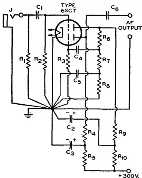
$C_1$   $C_4$   $C_6=0.05 \mu\text{f}$ , paper, 600 v.
