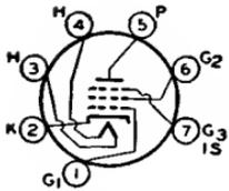
requires miniature seven-contact socket and may be mounted in any position. For heater and cathode considerations, refer to type 6AV6.
