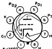
Metal type 12SR7 and glass-octal types 12SR7-GT used as combined detector, amplifier, and avc tube in ac/dc radio receivers. Outlines 3 and 23, respectively, OUTLINES SECTION. Heater volts (ac/dc), 12.6; amperes, 0.15. Except for heater rating, type 12SR7 is identical with type 6SR7, and type 12SR7-GT is electrically identical with type 6SR7 except for interelectrode capacitances. The 12SR7-GT
