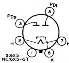
used principally for renewal purposes. Type 6X5-GT may be supplied with pin No.1 omitted. Both types require octal socket. Type 6X5 should be mounted in vertical position, but horizontal operation is permissible if pins 3 and 5 are in horizontal plane. Type 6X5-GT may be operated in any position. For maximum ratings, typical operation data, and curves, refer to type 6X4. Type 6X5 is used principally for renewal purposes.
