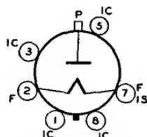
scanning systems. When used as an rf rectifier, one 1B3-GT in a half-wave circuit is capable of delivering a maximum dc output voltage of about 15000 volts. In a voltage-doubler circuit, two tubes will give about 30000 volts; and in a voltage-tripler circuit, three 1B3-GT's will deliver 45000 volts approximately. For curve of average plate characteristics, see page 61.
