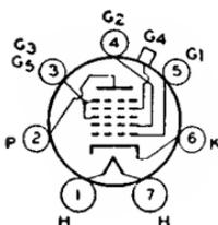
Glass type used in ac-operated receivers. Outline 36, OUTLINES SECTION. Tube requires small seven-contact (0.75-inch, pin-circle diameter) socket. Except for its heater rating (2.5 volts ac/dc; 0.8 ampere) and its interelectrode capacitances, the 2A7 has electrical characteristics identical with type 6A8. Complete shielding of this tube is generally necessary. Type 2A7 is a DISCONTINUED type listed for reference only.
