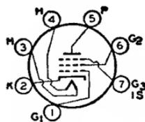
LINEs SECTION. Tube requires seven-contact miniature socket and may be mounted in any position.
