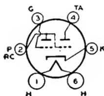
Glass type used to indicate visually by means of a fluorescent target the effects of a change in a controlling voltage. It is used as a convenient means of indicating accurate radio receiver tuning. Outline 31 or 34, OUTLINES SECTION. Tube requires six-contact socket. Except for its heater rating (2.5 volts ac/dc; 0.8 ampere), the 2E5 has electrical characteristics identical with type 6E5. Type 2E5 is a DISCONTINUED type listed for reference only.
