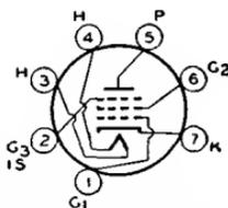
OUTLINES SECTION. Tube requires miniature seven-contact socket and may be mounted in any position. For a discussion of limiters, refer to ELECTRON TUBE APPLICATIONS SECTION. For typical operation as resistance-coupled amplifier, refer to Chart 8, RESISTANCE-COUPLED AMPLIFIER SECTION. For heater and cathode considerations, refer to type 6AV6.
