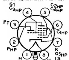
Glass lock-in type used as combined triode oscillator and heptode mixer in radio receivers. Outline 15, OUTLINES SECTION. Tube requires lock-in socket. Heater volts (ac/dc), 6.3; amperes, 0.3. Typical operation of heptode unit: plate volts, 250 (300 *max*); grids-No.2-and-No.4 volts, 100; grid-No.1 volts, -2; plate resistance, 1.25 megohms; conversion transconductance,
