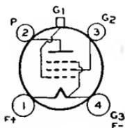
Glass type used as rf or if amplifier in battery-operated radio receivers, particularly those employing avc. Outline 41, OUTLINES SECTION. Tube requires four-contact socket. Filament volts (dc), 2.0; amperes, 0.06. Characteristics as class A<sub>1</sub> amplifier: plate volts, 180 *max*; grid-No.2 volts, 67.5 *max*; grid-No.1 volts, -3 *min*; plate ma., 2.8; grid-No.2 ma., 1.0; plate
