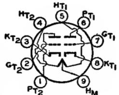
noval nine-contact socket and may be mounted in any position. Each triode unit is independent of the other except for the common heater.
