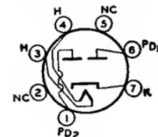
socket and may be mounted in any position. Outline 16, OUTLINES SECTION. It is especially important that this tube, like other power-handling tubes, be adequately ventilated. For discussion of Rating Chart and Operation Characteristics, refer to type 6AX5-GT.
