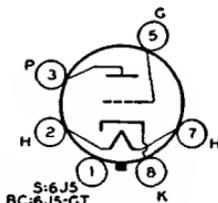
high amplification factor. Outlines 3 and 25, respectively, OUTLINES SECTION. Tubes require octal socket and may be mounted in any position. For heater and cathode considerations, refer to type 6AV6. For typical operation as resistance-coupled amplifiers, refer to Chart 13, RESISTANCE-COUPLED AMPLIFIER SECTION.
