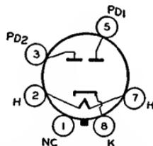
Glass octal type used in power supply of radio equipment having moderate dc requirements. The heater of this tube can be operated from the same transformer winding that sup-
