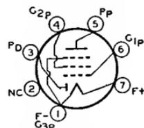
Miniature type used in lightweight, compact, portable, battery-operated receivers as combined detector and af voltage amplifier. Outline 13, OUTLINES SECTION. Filament volts (dc), 1.4; amperes, 0.05. Tube requires miniature seven-contact socket and may be mounted in any position. For electrical characteristics, curves, and application, refer to type 1U5.
