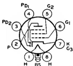
Glass lock-in type used as combined detector, amplifier, and avc tube. Outline 15, OUTLINES SECTION. Tube requires lock-in socket. Heater volts (ac/dc), 6.3; amperes, 0.3. Typical operation and ratings of pentode unit as class A<sub>1</sub> amplifier: plate volts, 250 *max*; grid-No.2 volts, 100; plate dissipation, 2 *max* watts; grid-No.2 input, 0.25 *max* watt; grid-No.1
