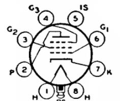
Glass lock-in type used as rf or if amplifier in radio receivers. Outline 15, OUTLINES SECTION. Tube requires lock-in socket. Heater volts (ac/dc), 6.3; amperes, 0.45. Typical operation and maximum ratings as class A<sub>1</sub> amplifier: plate volts and grid-No.2 supply volts, 300 *max*; grid-No.2 series resistor, 40000 ohms; plate dissipation, 4 *max* watts; grid-No.2 input,
