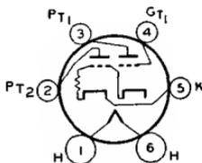
ma., 8. Output triode: plate volts, 300 max; plate ma., 45; plate resistance, 24000 ohms; load resistance, 7000 ohms; output watts, 4. This is a DISCONTINUED type listed for reference only.
