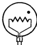
Constant-current regulating devices (half-tubes) used in radio receivers. Bases fit the standard mogul screw socket and tubes may be mounted in any position. Tubes operate at high bulb temperature. They must be surrounded by a protective metal ventilating stack. Operating conditions: voltage range, 40 to 60 volts; ambient temperature, 150°F; operating current for the 876, 1.7 amperes; for the 886, 2.05 amperes. These are DISCONTINUED types listed for reference only.
