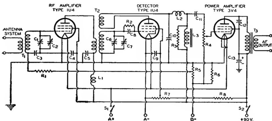
**C<sub>1</sub> C<sub>6</sub>**=Ganged band-setting capacitors, 140  $\mu\text{f}$ , maximum per section
