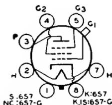
Metal type 6S7 and glass-octal type 6S7-G used in rf and if stages of automobile receivers employing avc. Outlines 5 and 35, respectively, OUTLINES SECTION. Type 6S7 is used principally for renewal purposes. Type 6S7-G is a DISCONTINUED type listed for reference only. Tubes require octal socket and may be mounted in any position. Heater volts, 6.3; amperes, 0.15. Typical operation and maximum
