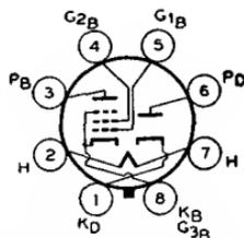
90; grid-No.1 volts, -7; plate ma., 27; grid-No.2 ma., 2; plate resistance, 17000 ohms; transconductance, 4800 μmhos; load resistance, 2600 ohms; maximum-signal output watts, 1.0. This is a **DISCONTINUED** type listed for reference only.
