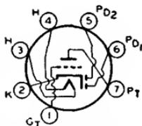
**OUTLINES SECTION.** Tube requires miniature seven-contact socket and may be mounted in any position. For typical operation as resistance-coupled amplifier, refer to Chart 7, **RESISTANCE-COUPLED AMPLIFIER SECTION.** For heater considerations, refer to type 6AV6.
