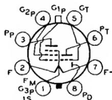
amplification factor, 65; plate resistance, 0.2 megohm; transconductance, 325  $\mu\text{hos}$ ; plate ma., 0.2. (Typical operation of pentode unit as class A<sub>1</sub> amplifier: plate volt, 90 (110 max); grid-No.2 volts, 90 (110 max); grid-No.1 volts, 0; plates resistance, 0.8 megohm; transconductance, 750  $\mu\text{hos}$ ; plate ma. 1.5; grid-No. 2 ma., 0.5. This is a DISCONTINUED type listed for reference only.
