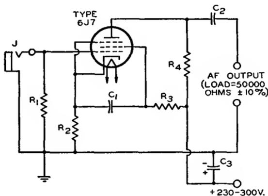
$C_1=0.25 \mu\text{f}$ , paper, oil-filled, 600 v.
