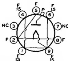
Outline 19, OUTLINES SECTION. Tubes require noval nine-contact socket and may be mounted in any position. Plate connection is cap at top of bulb. Pins 3 and 7 may be used as tie points for filament dropping resistor and high-voltage filter resistor, or may be connected to the filament. These pins should not be connected to low-potential circuits. For other filament and high-voltage considerations, refer to type 1B3-GT. For curve of average plate characteristics, see page 61.
