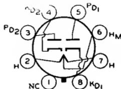
Glass octal type used as half-wave rectifier or voltage doubler in ac/dc receivers. Outline 33, OUTLINES SECTION. The heater is provided with a tap for operation of a panel lamp. Without panel lamp, heater volts (ac/dc) of entire heater (pins 2 and 7), 50; amperes, 0.15. With panel lamp, heater volts (ac/dc) of panel-lamp section (pins 6 and 7) with 0.15 ampere
