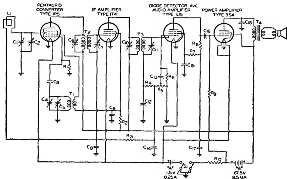
**C<sub>1</sub> C<sub>4</sub>** = Ganged tuning capacitors: C<sub>1</sub>, 10-274 μf; C<sub>4</sub>, 7.5-122.5 μf
