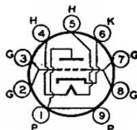
SECTION. Tube requires miniature nine-contact socket and may be mounted in any position.
