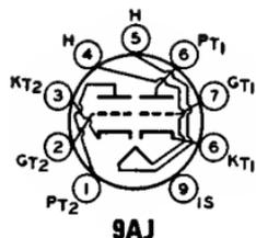
Miniature type used as a cascode amplifier in vhf color and black-and-white television tuners and in push-pull cathode-drive rf amplifiers. Outlines section, 6B; requires miniature 9-contact socket. For typical operation as a resistance-coupled amplifier, refer to Resistance-Coupled Amplifier section. Type 5BK7A is identical with type 6BK7B except for heater ratings.
