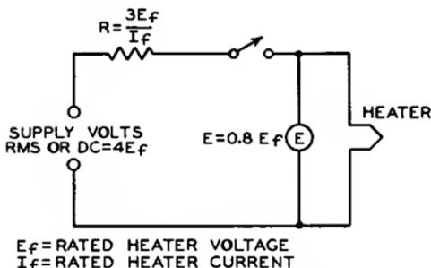
Fig. 124—Test circuit for measuring heater warm-up time.
