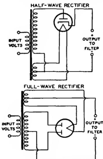
Fig. 18—Half-wave and full-wave rectifier circuits.
