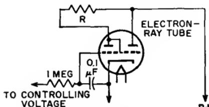
Fig. 110—Indicating circuit using an electron-ray tube.
