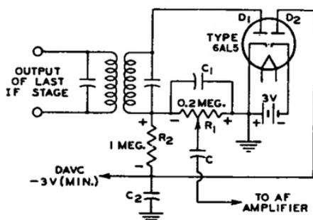
Fig. 62—Delayed avc (davc) circuit.
