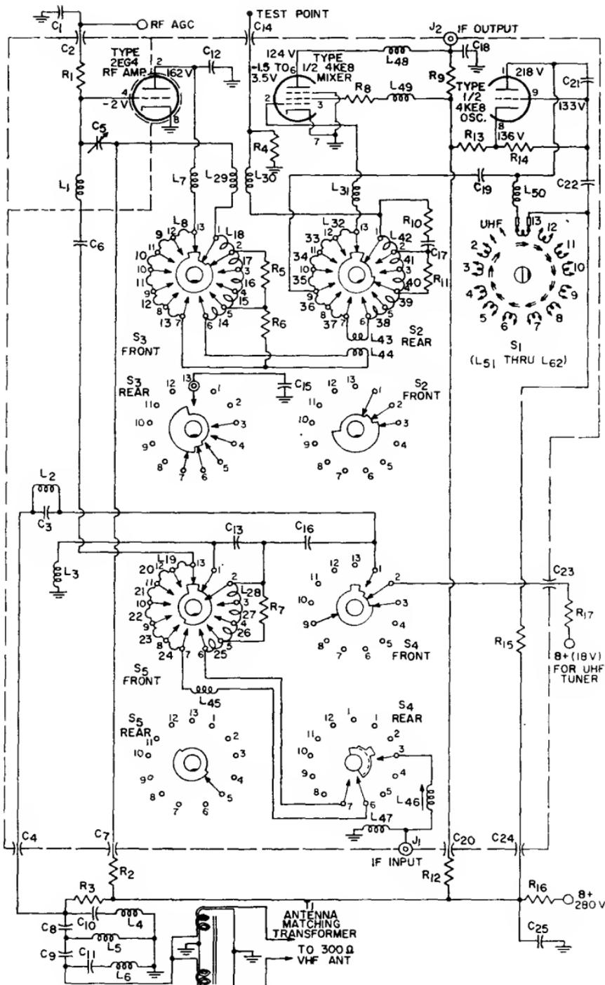
**Note:** Switches S<sub>1</sub> through S<sub>5</sub> are ganged together on the same shaft and are shown in channel 13 position.
