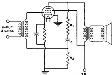
Fig. 48—Power-output stage using constant voltage inverse feedback.
