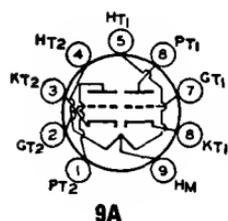
Miniature type used as phase inverter or resistance-coupled amplifier in high-quality, high-fidelity audio amplifiers. Outlines section, 6B; requires miniature 9-contact socket. This type is identical with miniature type 12AX7A except that it has a controlled equivalent noise and hum characteristic. For operation as resistance-coupled amplifier, refer to Resistance-Coupled Amplifier section.
