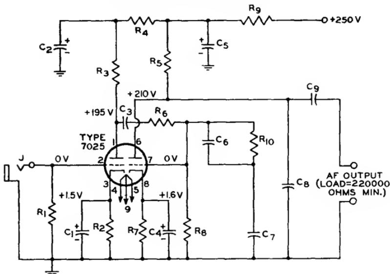
Sensitivity=3 millivolts rms input for output of 0.55 volt at frequency of 1000 Hz.
