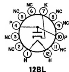
Duodecar type used as damper tube in horizontal-deflection circuits of black-and-white television receivers. **Outlines section, 8C;** requires duodecar 12-contact socket. Socket terminals 5, 6, 8, and 9 should not be used as tie points. This tube, like other power-handling tubes, should be adequately ventilated. **Heater:** volts (ac/dc), 6.3; amperes, 1.2.
