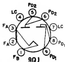
Novar types used in power supplies of radio equipment and television receivers having high dc requirements. Outlines section, 31C; requires novar 9-contact socket. Vertical operation is preferred, but tubes may be operated in horizontal position if pins 2 and 7 are in vertical plane. It is especially important that these tubes, like other power-handling tubes, be adequately ventilated. Filament: volts (ac), 5; amperes, 3.
