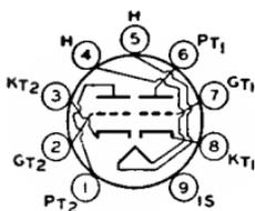
Miniature type used as combined rf-amplifier and mixer-oscillator tube in FM tuners. Unit No.1 is used as an oscillator-mixer, and unit No.2 is used as an rf amplifier. Outlines section, 6B; requires miniature 9-contact socket and may be mounted in any position.
