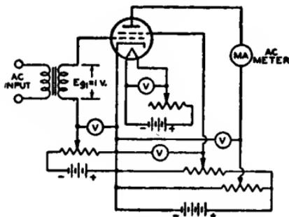
Fig. 132—Fundamental circuit of a dynamic transconductance tester.
