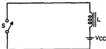
Fig. 85—Simplest form of deflection circuit.
