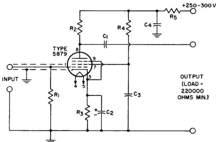
Sensitivity=3 millivolts rms input for output of 220 millivolts.
