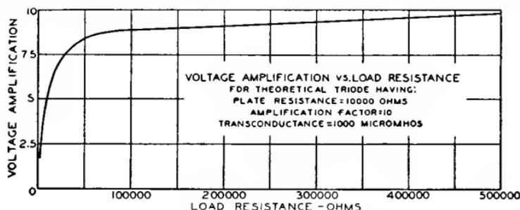
Fig. 36—Gain curve for triode amplifier circuit.
