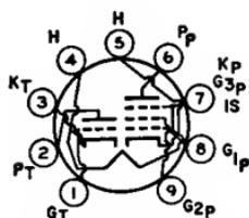
Miniature type used in color and black-and-white television receiver applications. The triode unit is used as a sync-separator, sync-amplifier, keyed-agc, or noise-suppressor tube. The pentode unit is used as a video-output tube. Outlines section, 6E: requires miniature 9-contact socket.
