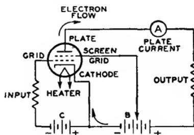
Fig. 7—Basic tetrode circuit.
