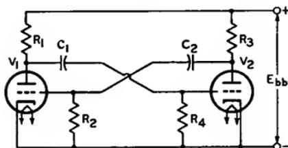
Fig. 100—Basic multivibrator circuit of the free-running type.
