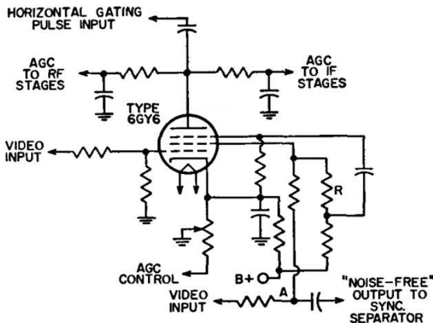
Fig. 84—Typical noise-cancellation circuit.
