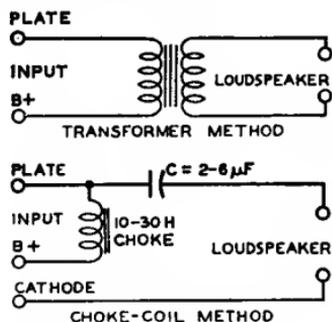
Fig. 123—Typical output-coupling devices.
