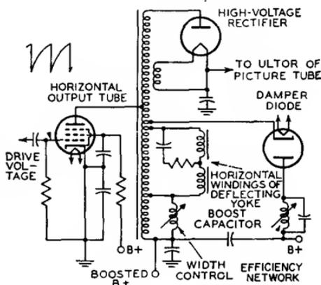
Fig. 89—Typical horizontal-deflection and high-voltage circuit.
