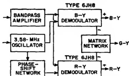
Fig. 98—Block diagram of demodulator circuit used to apply signals directly to color picture tube.
