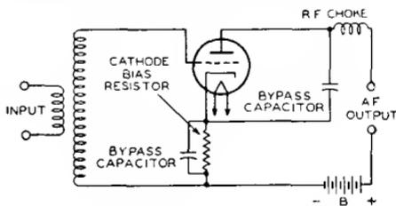
Fig. 26—Grid-bias detector circuit.
