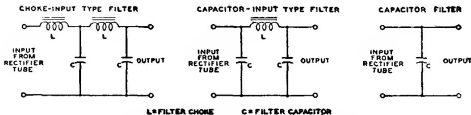
Fig. 121—Typical smoothing filters for rectifier tubes.
