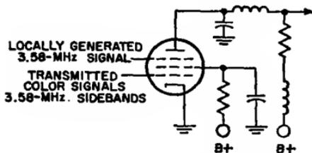
Fig. 97—Low-level color demodulator.
