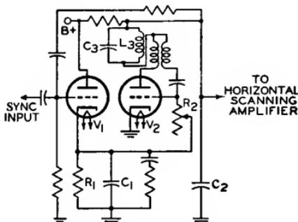
Fig. 101—Simplified synchroguide circuit.
