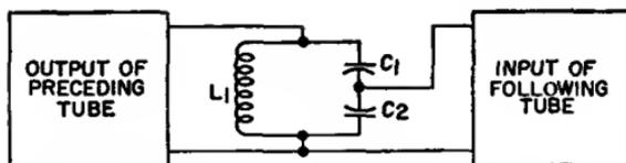
Fig. 71—Single-tuned coupling network using capacitive division.
