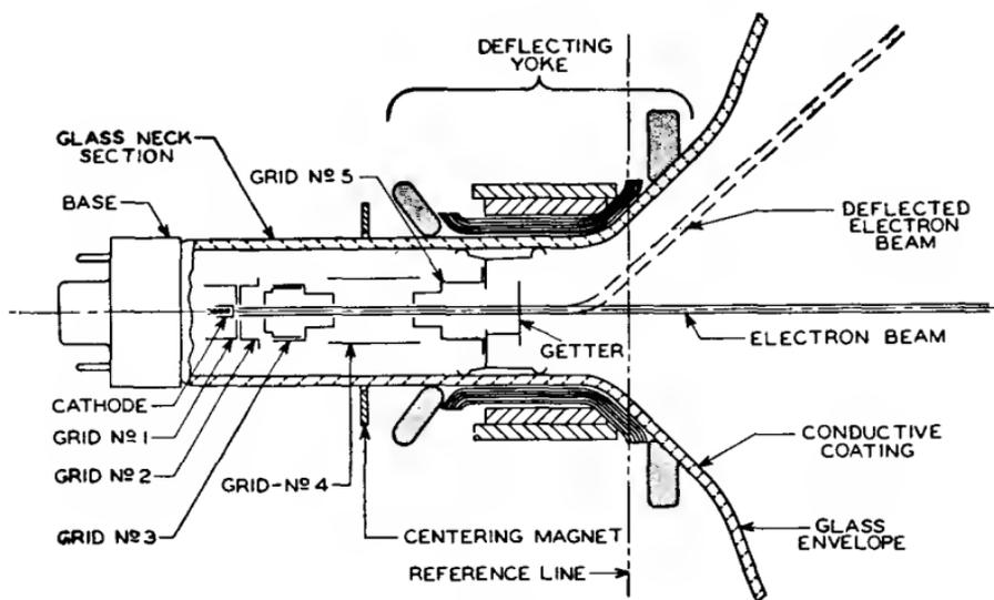
Fig. 10—Structure of television-picture-tube electron gun
