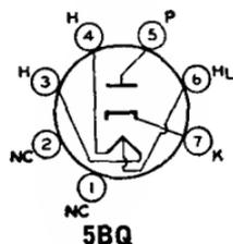
Miniature type used in power supply of ac/dc radio receivers. The heater is provided with a tap for operation of a panel lamp. For typical circuit, refer to type 35W4. Outlines section, 5D; requires 7-contact socket.
