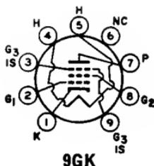
Miniature type used in the output stage of audio amplifying equipment and also in the video output stage of color and black-and-white television receivers. Outlines section, 6G; requires miniature 9-contact socket. Types 10GK6 and 16GK6 are identical with type 6GK6 except for heater ratings.
