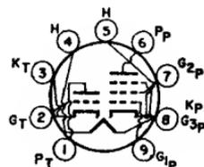
Miniature type used as combined oscillator and mixer. Outlines section, 6B; requires miniature 9-contact socket. Heater: volts (ac/dc), 18.9; amperes, 0.15; maximum heater-cathode volts, ±200 peak, 100 average.
