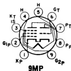
Miniature type with frame-grid pentode unit used as combined oscillator and mixer tubes in vhf color and black-and-white television receivers. **Outlines section, 6B**; requires miniature 9-contact socket. Type 7HG8/PCF86 is identical with type 6HG8/ECF86 except for slightly higher current and dissipation ratings and for heater ratings.
