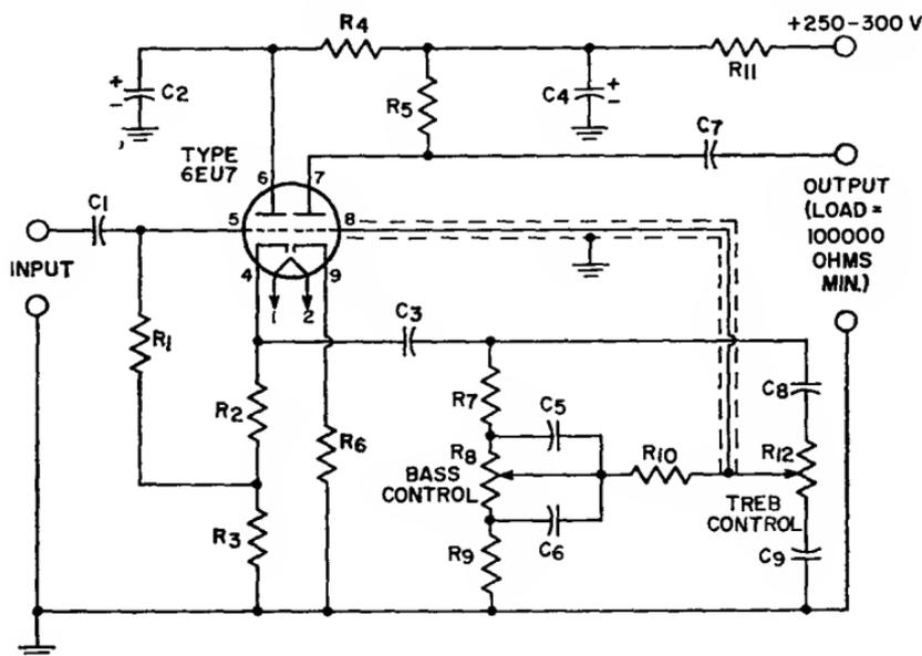
Sensitivity=0.5 volt rms input for output of 1.25 volts with controls set for flat response.
