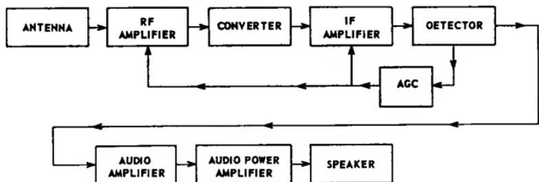
Fig. 14—Simplified block diagram for a broadcast-band receiver.
