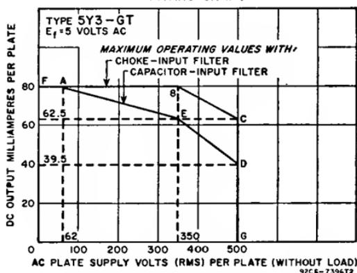
\* Higher values of capacitance than indicated may be used but the effective plate supply impedance may have to be increased to prevent exceeding the maximum rating for hot-switching transient plate current.
