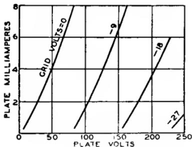
Fig. 12—Family of plate-characteristics curves.
