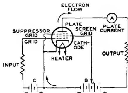
Fig. 8—Basic pentode circuit.
