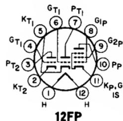
Duodecar type used in color and black-and-white television receiver applications. The triode units are used for general-purpose applications, and the pentode unit is used for horizontal-deflection service. **Outlines section, 8B;** requires duodecar 12-contact socket. **Heater:** volts (ac/dc), 6.3; amperes, 0.8; maximum heater-cathode volts,  $\pm 200$  peak, 100 average.
