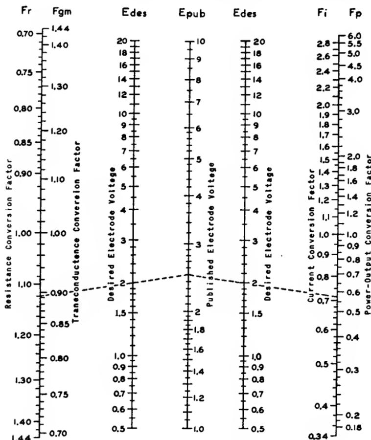
Fig. 44—Nomograph of tube conversion factors.
