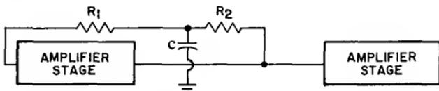
Fig. 55—Negative-feedback frequency-compensation network.
