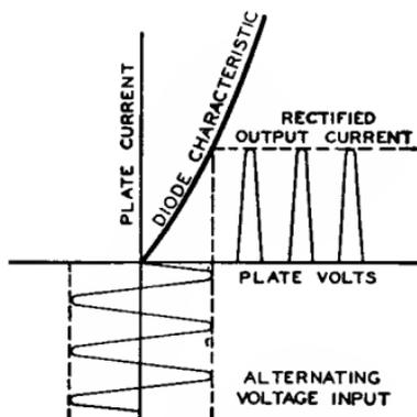
Fig. 4—Current characteristics of rectifier circuit.
