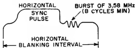
Fig. 96—Waveform for synchronizing signal.
