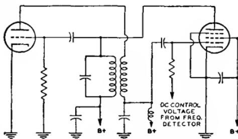
Fig. 104—Automatic-frequency-control (afc) circuit.
