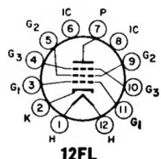
Duodecar type used as horizontal-deflection amplifier in television receivers. **Outlines section, 15C**; requires duodecar 12-contact socket.
