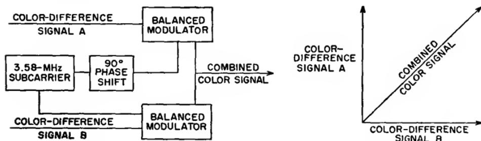
Fig. 94—Formation of combined color signal for transmission.
