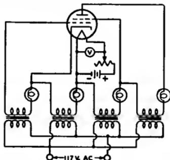
Fig. 129—Fundamental circuit of a short-circuit tester.
