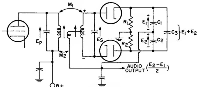
Fig. 33—Ratio-detector circuit.
