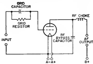
Fig. 27—Detector circuit using grid-resistor-and-capacitor bias.
