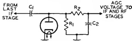
Fig. 63—Automatic-gain control (agc) circuit.
