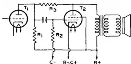
Fig. 50—Resistance-coupled stages using feedback resistor.
