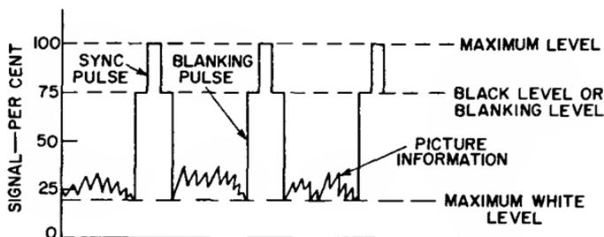
Fig. 79—Detected video signal.
