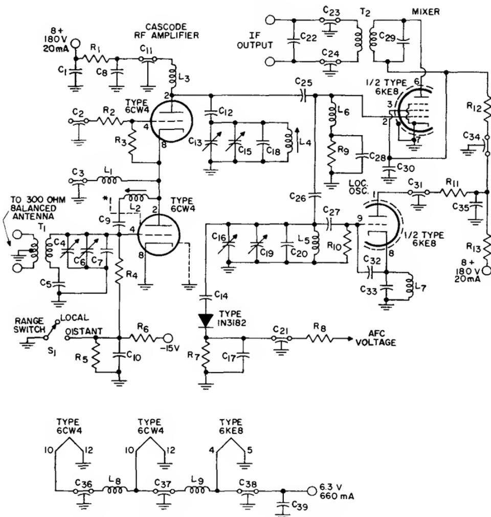
\* A metal shield should be provided between grid and plate terminals on the 6CW4 socket.
