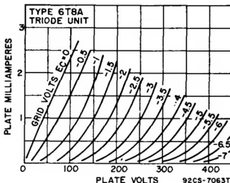
**Triode Unit as Class A<sub>1</sub> Amplifier**
