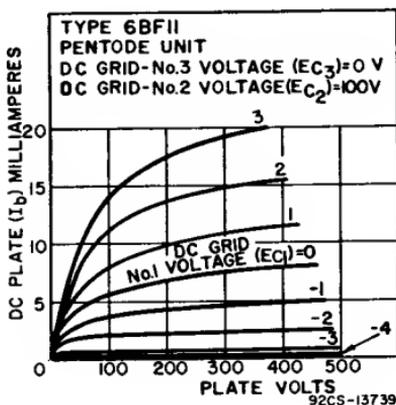
**Pentode Unit as Class A<sub>1</sub> Amplifier****CHARACTERISTICS**
