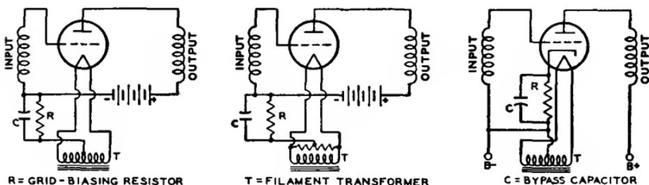
Fig. 113—Typical grid-voltage supply circuits.
