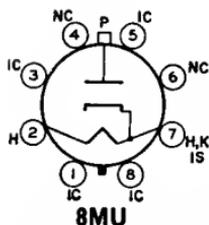
and X-ray safety considerations, refer to type 1G3GT/1B3GT. Heater: volts (ac/dc), 3.15; amperes, 0.48; operational warm-up time, 4 seconds.
