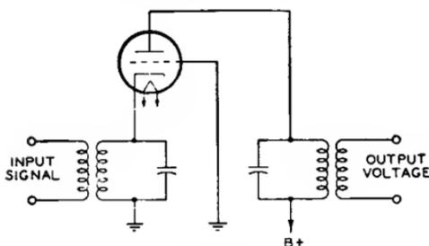
Fig. 47—Cathode-drive circuit.
