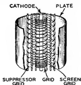
Fig. 37—Structure of remote-cutoff grid.
