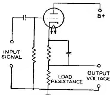
Fig. 52—Cathode-follower circuit modified for increased bias.
