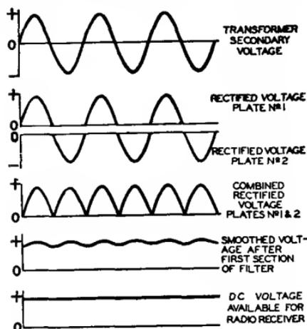
Fig. 17—Voltage waveforms of full-wave rectifier circuit.
