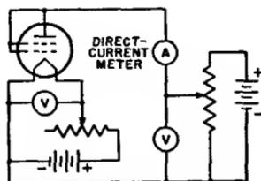
Fig. 130—Fundamental circuit of an emission tester
