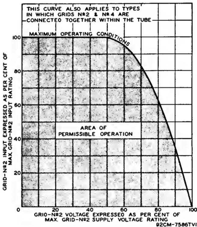
Fig. 128—Grid-No. 2 input rating curve.
