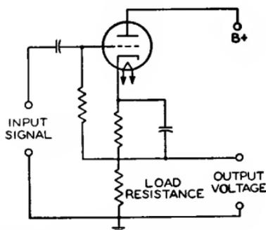
Fig. 53—Cathode-follower circuit modified for reduced bias.
