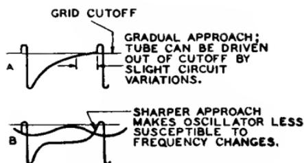
Fig. 103—Waveforms showing effect of tuned circuit L<sub>3</sub>C<sub>3</sub> in Fig. 101.
