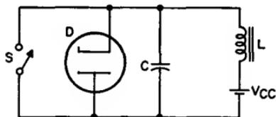
Fig. 88—Incorporation of damper diode.
