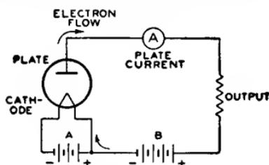
Fig. 3—Basic diode circuit.
