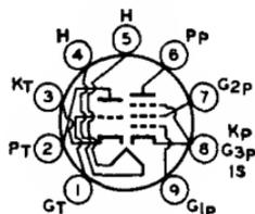
Miniature type used as if-amplifier and af voltage-amplifier tube in radio receivers. Outlines section, 6B; requires miniature 9-contact socket.
