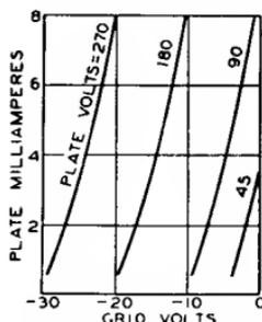
Fig. 13—Family of transfer-characteristics curves.
