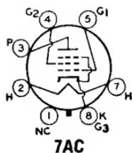
Glass octal type used in the output stages of radio receivers and high-fidelity audio amplifiers. Outlines section, 29M; requires octal socket. For typical operation as push-pull class A<sub>1</sub>, class AB<sub>1</sub> (within maximum ratings), and class AB<sub>2</sub> amplifier, and for curves of average plate characteristics, refer to type 6L6GC. Heater: volts (ac/dc), 6.3; amperes, 0.9; maximum heater-cathode volts, ±200 peak.
