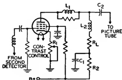
Fig. 76—Typical video amplifier stage.
