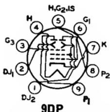
Miniature type used in color-demodulator and burst-gate circuits in color television receivers. This type has two plates and two deflecting electrodes; the control grid varies beam deflection. Outlines section, 6E; requires miniature 9-contact socket. Pin 5 should be connected to cathode at socket. The 6JH8 should be so located in the equipment that it is not subjected to stray magnetic fields.
