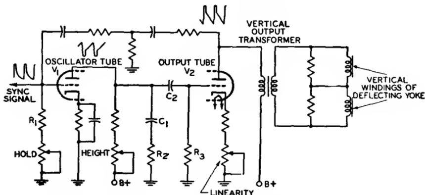
Fig. 90—Simplified combined vertical-oscillator-and-output stage.
