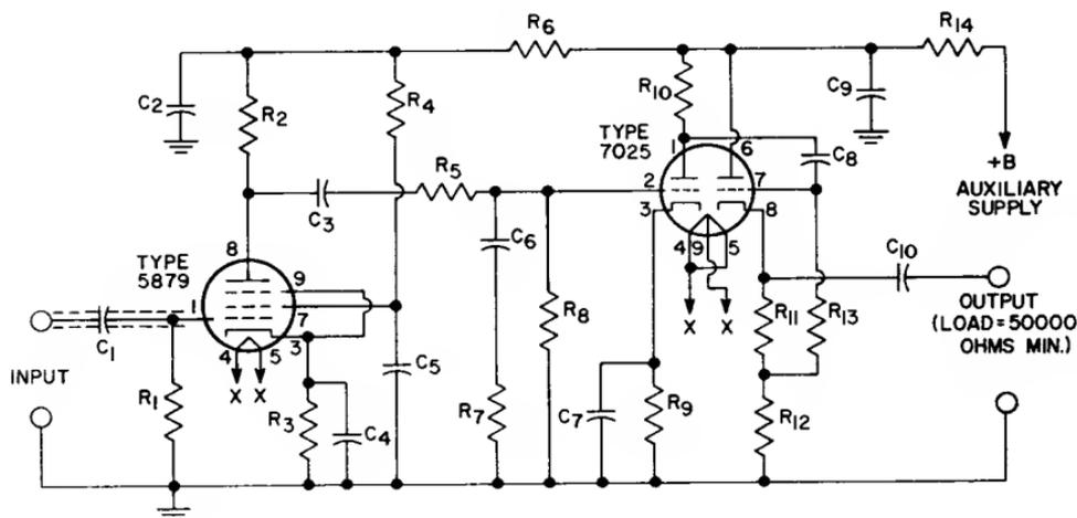
Sensitivity=3 millivolts rms input for output of 0.55 volt at frequency of 1000 Hz.
