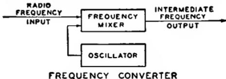
Fig. 106—Block diagram of simple frequency-converter circuit.
