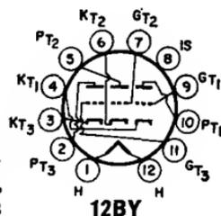
Duodecar type used as combined agc, sync, and noise-inverter tube in television receivers. Outlines section, 8A; requires duodecar 12-contact socket. Heater: volts
