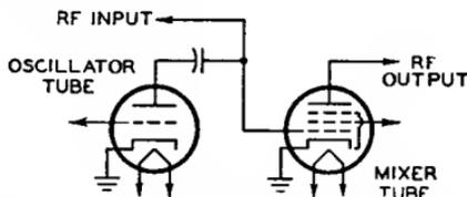
Fig. 108—Typical television mixer-oscillator circuit.
