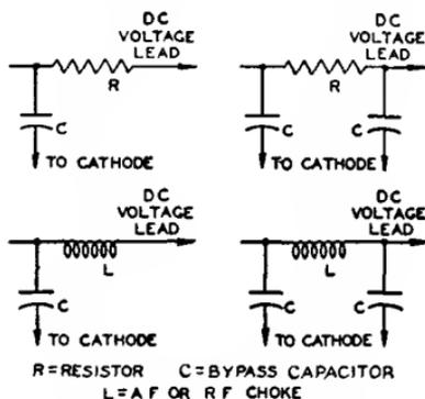
Fig. 120—Typical filter circuits.
