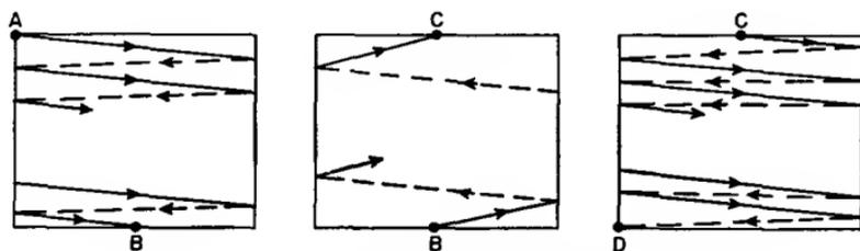
Fig. 78—The odd-line interlaced scanning procedure.
