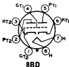
Glass type used as combined vertical-deflection-oscillator and vertical-deflection-amplifier tube in color and black-and-white television receivers. Outlines section, 13B; requires octal socket. Heater: volts (ac/dc), 6.3; amperes, 1.05; maximum heater-cathode volts,  $\pm 200$  peak, 100 average.
