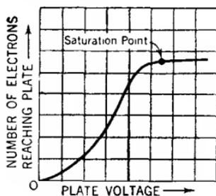
Fig. 5—Current characteristic of diode tube.
