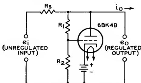
Fig. 92—High-voltage regulator circuit for color television.
