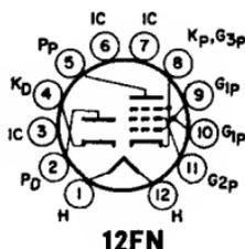
Beam Power Unit as Class A<sub>1</sub> Amplifier
