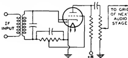
Fig. 25—Diode-biased detector circuit.
