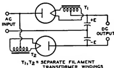
Fig. 19—Full-wave voltage-doubler circuit.
