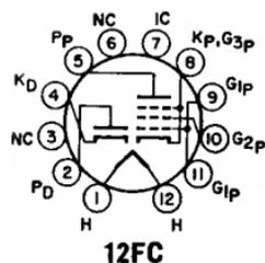
Duodecar type used in television receiver applications. The diode unit is used for damper service and the beam power unit for horizontal-deflection amplifier service. Outlines section, 15A; requires duodecar 12-contact socket. Heater: volts (ac/dc), 33.6; amperes, 0.45; warm-up time, 11 seconds; maximum heater-cathode volts,  $\pm 200$  peak, 100 average.
