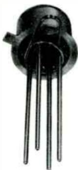
Fig. 138—Illustration shows shorting spring for RCA MOS field-effect transistors that do not contain the integral gate protection. (Spring should not be removed until after the device is soldered into circuit).
