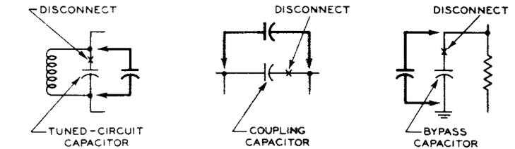
Fig. 3—Faulty capacitors can be detected by the substitution method: Disconnect one or both ends of the suspected capacitor. Temporarily connect a good capacitor in the circuit. If the new capacitor remedies the trouble, it may be assumed that the original capacitor is defective. See text for additional details.
