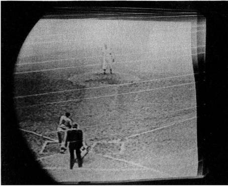
Fig. 4. Example of 60 cycle horizontal pulling, accompanied by light and dark areas, caused by heater-cathode leakage in the r.f., i.f., or video amplifiers. Here and in Fig. 6 picture is moved to left in order to show that edge of raster is straight without variation in width of raster (no change in amplitude of horizontal deflection). Picture pulling is result of 60 cycle variation in horizontal sync phasing.
