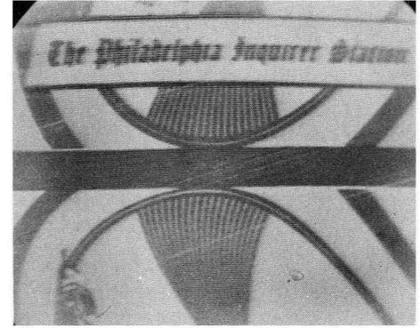
Fig. 7. Horizontal pulling caused by poor low frequency response in r.f. and i.f. amplifiers, reducing amplitude of sync signals with respect to higher frequency picture signals. The horizontal wedge, which represents low frequency signals, is faint compared with vertical wedge representing high frequency signals. Fault is poor alignment. Picture carrier is too low on the slope of the over-all response curve.
