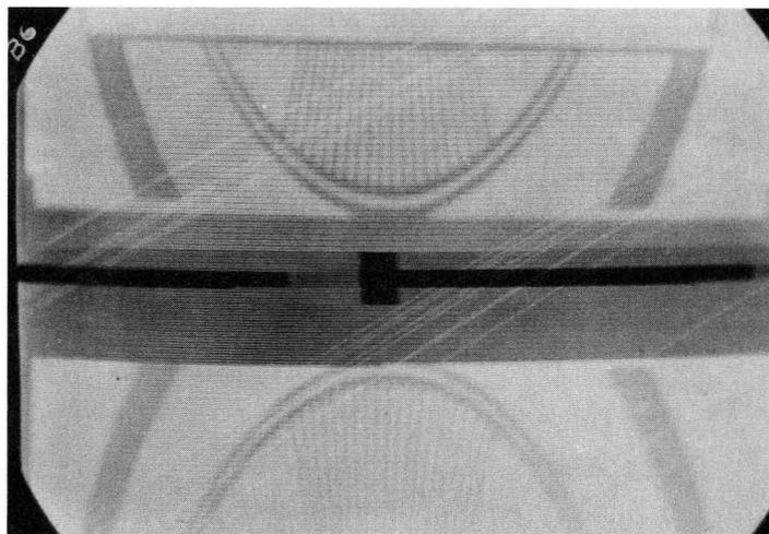
Fig. 3—Vertical blanking and sync, showing only a portion of the total width of these signals. The blanking should be slightly darker than the darkest picture elements, and sync should be definitely darker than the blanking. Refer to detailed views in Figs. 4, 5, and 6.
