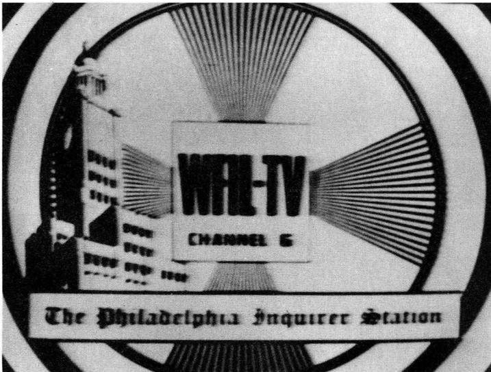
Fig. 2—This shows normal conditions. There is a slight trailing light-grey smear on the right-hand side of the lettering, and after the lines in horizontal wedge.
