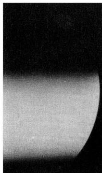
Fig. 5. Same trouble as in Fig. 3, except that the heater-cathode leakage is 400 ohms instead of 1000 ohms; note that the 60-cycle hum bars are more pronounced.
