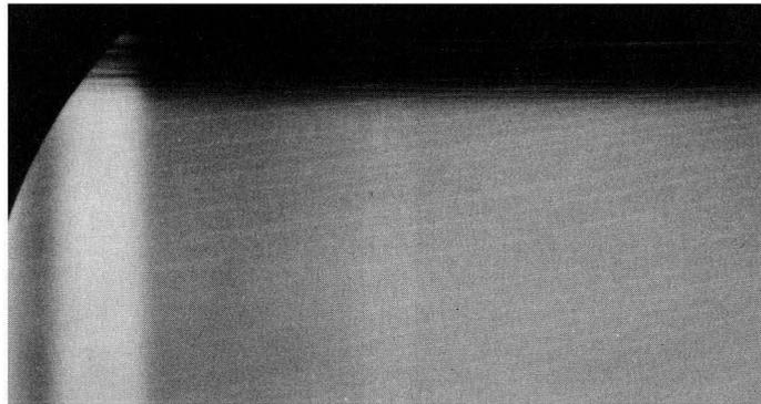
Fig. 13—Same trouble as Fig. 11, but greater intensity. This effect may be minimized by adjusting the horizontal drive control, checking lead dress and shielding, and, in extreme cases, by replacing the horizontal output tube.
