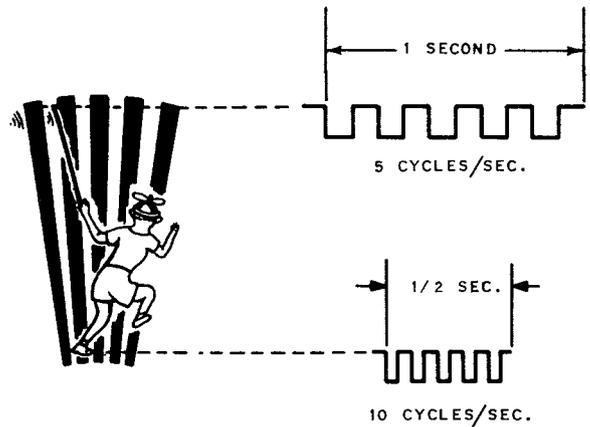
Figure 2. Analogy to vertical wedge in test pattern.
