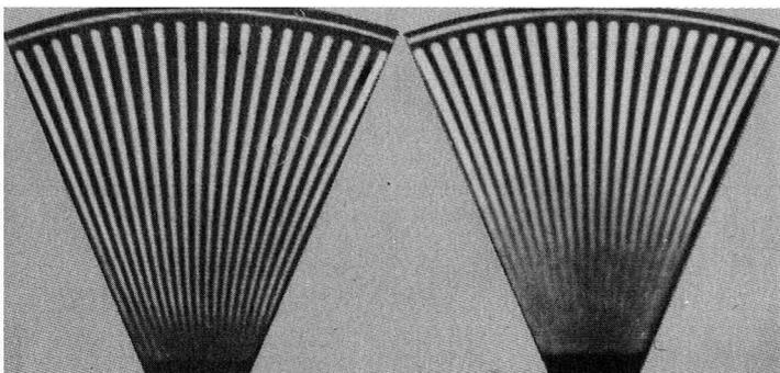
**Fig. 12—Vertical wedge at left shows normal conditions** in video amplifier. Wedge at right is with the 120-microhenry peaking coil in the 1st-video amplifier open. This condition reduces definition in the vertical wedge and makes the wedge and lettering fuzzy.
