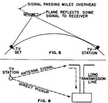
Because the antenna signal is delayed traveling down the transmission line, the direct signal picked up in the rf or 1st detector circuits appear ahead, or on the left-hand side of the antenna-signal picture.
