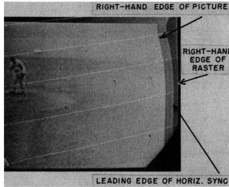
upper portion) thereby indicating a variation in horizontal sync phasing. Edge of raster is substantially straight, indicating pulling is not present in raster itself.
