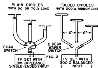
tion, is to use three separate antennas with reflectors, and three separate transmission lines running to a selector switch near the receiver, as shown in Figure 2.
