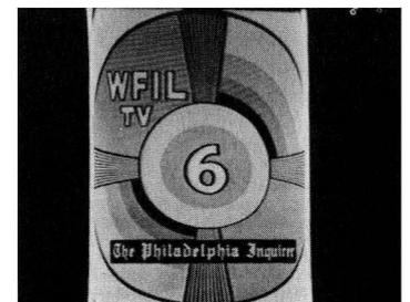
Fig. 11. Fold-over at left and right sides of raster produced by changing the grid resistor of the horizontal output tube from 1.0 megohm to 60,000 ohms. Circuit shown in Fig. 1.
