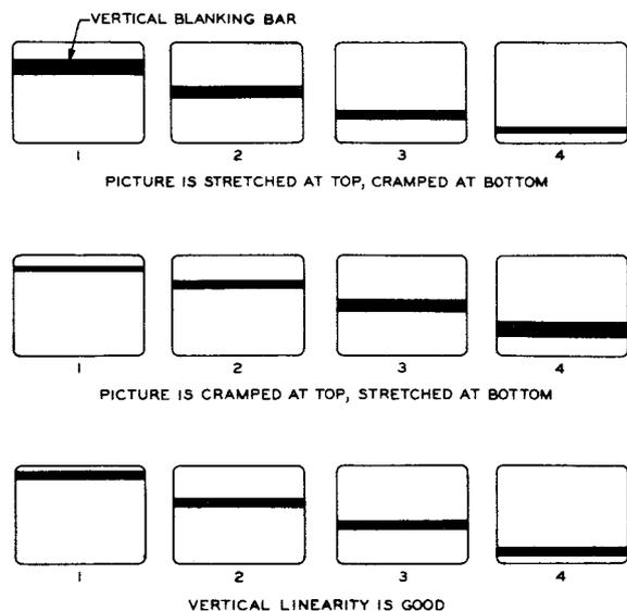
Figure 3. Checking Vertical Linearity with Vertical Blocking Bar.
