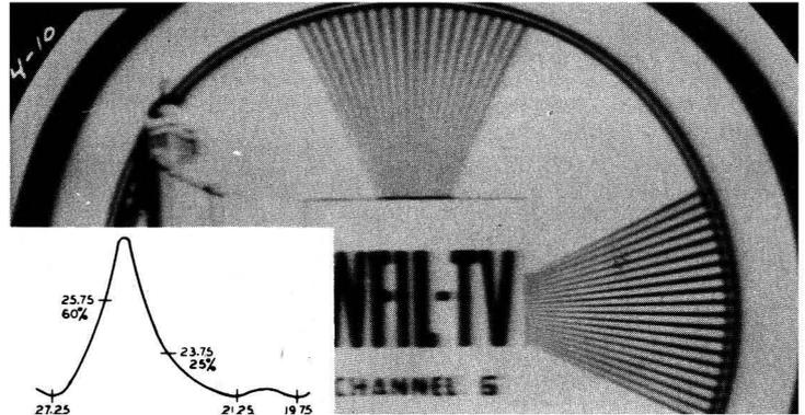
Fig. 8—Similar to Fig. 7, but vertical wedge is much weaker due to position of carrier, and narrower bandwidth.
