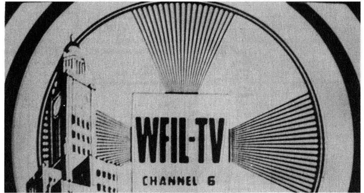
**Fig. 7—Excessive high-frequency response.** 1st- or 2nd-video plate load of 3300 ohms dropped to 1000 ohms. Reduces low-frequency response, exaggerating highs. Note trailing reversal, white followed by a fine dark line, after lettering.
