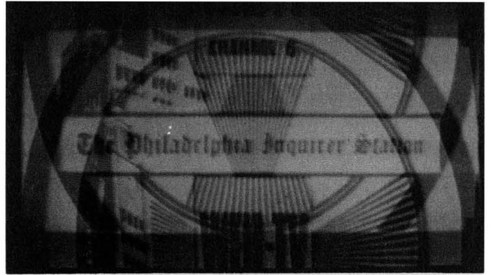
Fig. 4—The presence of two superimposed half-pictures indicates that the electron beam in the kinescope is being deflected from top to bottom in 1/120th second, or that the frequency or blocking rate of the vertical oscillator is 120 instead of 60 cycles per second. This condition was produced by a short circuit across the 1.5-megohm resistor in the oscillator grid circuit and by adjusting the hold control for a stationary picture.
