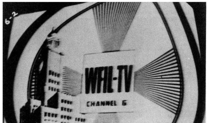
A PM speaker field near the top right-hand side of the flare of the kinescope pulled this picture out of shape. Reversing the magnet would squeeze the picture.
