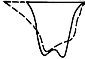
Fig. 2. Generator amplitude tilt detected by comparison. Solid curve represents tuner output when the generator used is known to have a flat characteristic. Dotted curve represents the response of the same tuner when a generator having tilted output is used.
