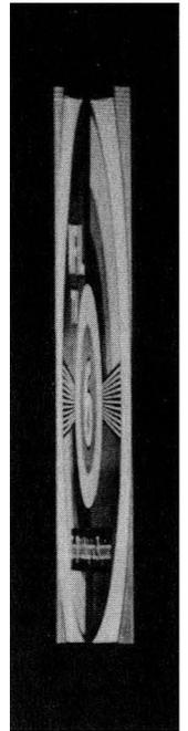
Fig. 7. Extremely narrow picture bars produced by a shorted 0.018- $\mu\text{f}$  capacitor in the damper circuit of Fig. 1.
