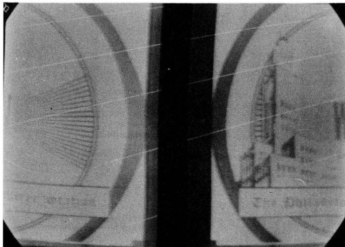
Fig. 7—Photograph of horizontal blanking and sync signals.
