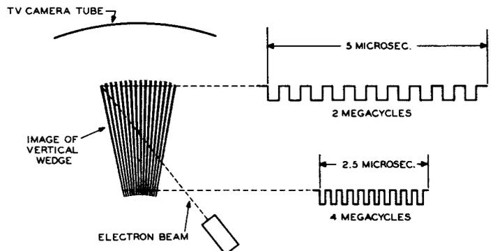
Figure 3. Vertical wedge is used in providing square-wave video signals of a wide frequency range.
