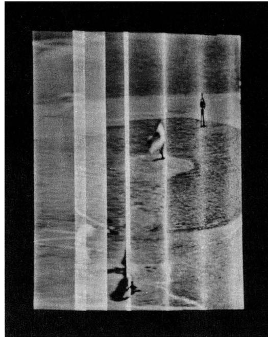
Fig. 6. Fold-over and bright vertical bars produced by an open 0.018- $\mu\text{f}$  capacitor in the damper circuit of Fig. 1.
