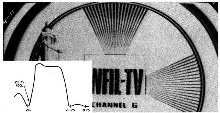
Fig. 9—Poor low-frequency response, evidenced by weak horizontal wedge. This was caused by tuning adjacent-channel sound trap close to picture carrier. Similar to Fig. 1.
