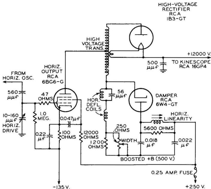
Fig. 1. "Direct" horizontal-deflection circuit used in RCA model T164 and many other recent models. Note that the horizontal-deflection coils are connected in series with the plate winding of the high-voltage transformer, which is an air-core type. In earlier models, the horizontal-deflection coils are connected to a secondary winding on an iron-core, high-voltage transformer. This RCA direct-deflection type of circuit has higher power efficiency than earlier circuits.
