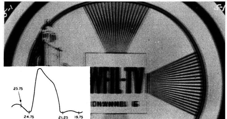
Fig. 10—Poor response in general, caused by tuning adjacent-channel sound trap lower than picture carrier. Note leading smear on left-hand side of lettering.
