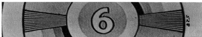
Fig. 5. Effect on width of picture produced by adjustment of width coil in model 630TS type of horizontal-deflection circuit.
