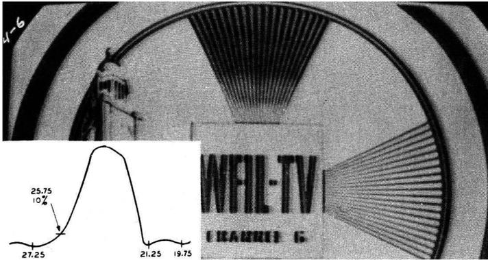
Fig. 4—Picture carrier at 10%. Poor low-frequency response, evidenced by the fact that horizontal wedge is lighter than vertical wedge. Poor sync, blanking, and signal-noise ratio.
