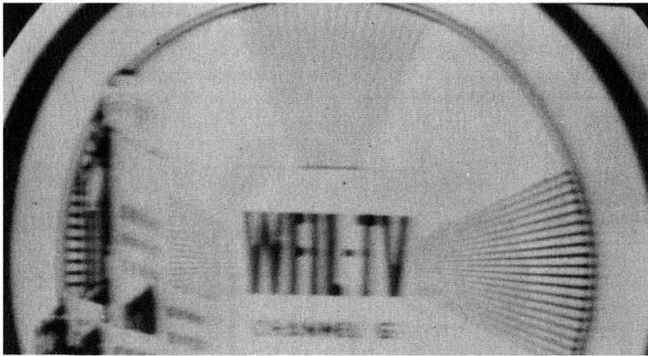
**Fig. 6—Poor high-frequency response.** 1st-video plate filter capacitor (10 uf) open, effectively increasing plate load resistor from 3300 to 10,100 ohms (3300 plus 6800). General smearing of wedges except center lines in horizontal wedge.
