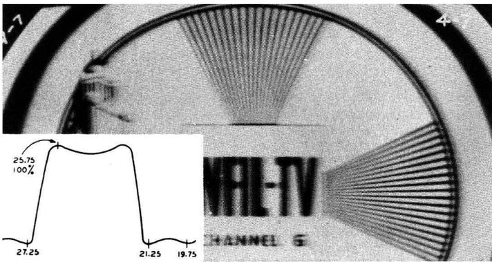
Fig. 5—Picture carrier at 100%. Excessive low-frequency response, evidenced by the fact that horizontal wedge is darker than vertical wedge. Considerable smear after lettering.
