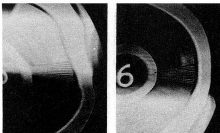
Fig. 2. One cycle of change in brightness (60-cycle hum bars) and one cycle of horizontal pulling, between top and bottom of picture, indicates heater-cathode leakage in the rf, if, or video amplifiers. The trouble in this example was caused by a defective tube in the picture-if amplifier. The 60-cycle leakage current flows through the cathode resistor and modulates the TV signal. The position of the hum symptoms is shifted, as shown above at left and right by reversing the power-cord plug.
