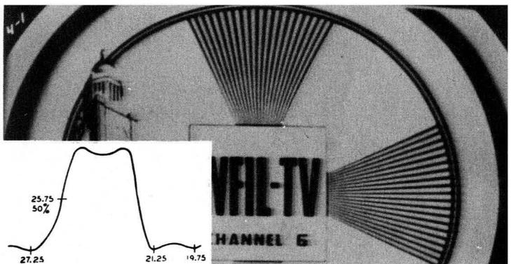
Fig. 2—Normal response with normal alignment, carrier at 50%
