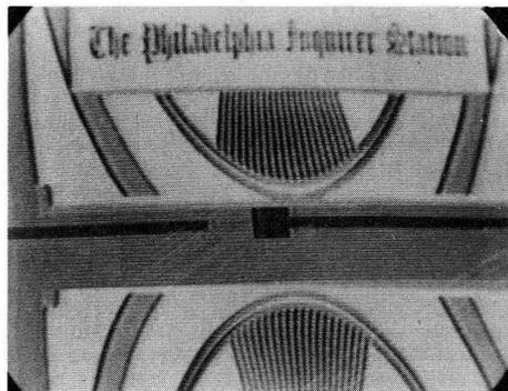
Fig. 14. Instance where sync amplitude is reduced to approximately same level as the darkest picture signals. Trouble is caused by poor r.f.-i.f. alignment, the picture carrier is too low on the slope of the response curve. Also refer to Fig. 7 (Part 1).
