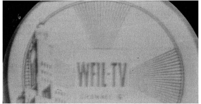
Fig. 12—Normal expansion in picture size when brightness control is turned up. Turning up the brightness increases the kinescope beam current so that the voltage drop across the 1-megohm high-voltage filter resistor is increased and the accelerating voltage decreased. As a result of the decreased accelerating voltage, the beam is more easily deflected and the picture becomes larger.
