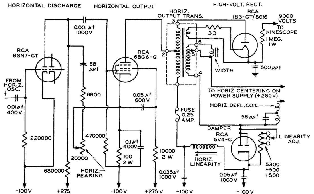
Fig. 1—Horizontal-deflection and high-voltage circuit used in producing the troubles shown in accompanying photographs. The input signal for this circuit is obtained from the horizontal oscillator which operates at 15,750 cycles per second.
