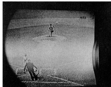
Fig. 6. In addition to 60-cycle change in picture brightness, heater-cathode leakage in the rf, if, or video amplifiers may also produce 60-cycle horizontal pulling in the picture. Both effects are evident in this example, which was produced by heater-cathode leakage in a tube in the picture-if amplifier (Refer to Fig. 7 and the note at the end of the caption for Fig. 9.)
