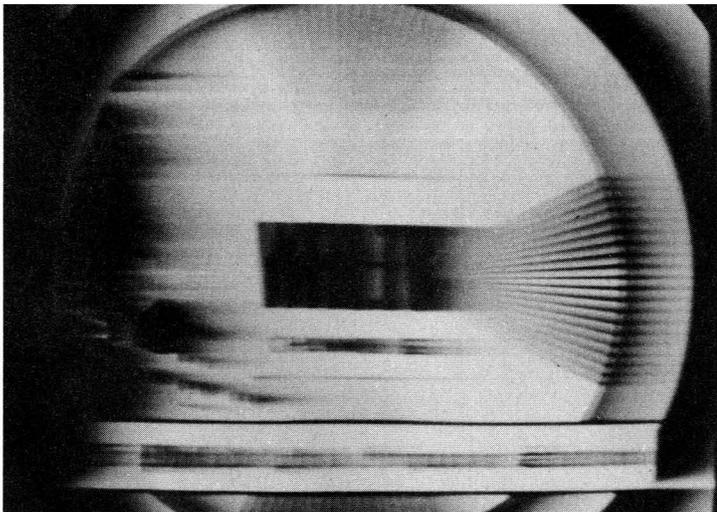
Fig. 4—Excessive low-frequency response and phase shift. 2nd-detector load resistor increased from 3900 to 100,000 ohms. Note smearing of lettering and horizontal wedge, and almost complete wiping out of vertical wedge.
