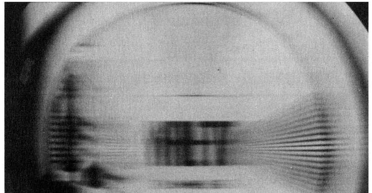
**Fig. 11—Loss of highs, and low-frequency phase shift** produced by open coupling capacitor (0.05 uf) to the kinescope grid. Note that vertical wedge is practically wiped out. Note smear after lettering and after horizontal wedge.
