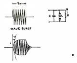
Fig. 9-Response of a tuned circuit to a pulse of frequency modulation.
