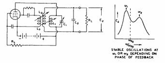
Fig. 4—Oscillator circuit for all values of K, and stable characteristic when  $K >> K_c$ .
