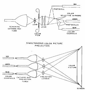
Fig. 1—Block diagram of the simultaneous all-electronic color television system. (Each of the color channels, shown at the right of the upper figure, have the same operating standards as the current black-and-white system. At the receiving end, shown at the left of the lower figure, each color channel is associated with its separate cathode-ray projection tube.)
