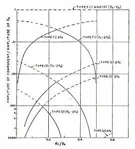
Fig. 5—Frequency components resulting from width modulation of a pulse carrier wave by a sine wave. Type (1) = dissymmetrical modulation Type (2) = symmetrical modulation  $f_c =$  pulse frequency  $f_0 =$  modulating frequency
