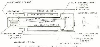
Fig. 8-Line diagram of the image orthicon.
