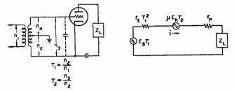
Fig. 8—Tapped cathode-input amplifier and equivalent network.
