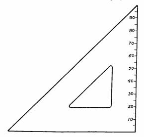
Fig. 15—Calibrated triangle<sup>8</sup> for reading contributions of harmonics from synthesis charts.
