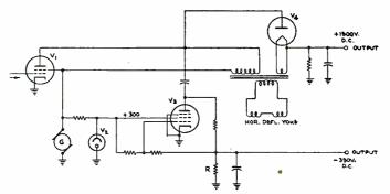
Fig. 4-High Voltage Power Supply and Regulator
