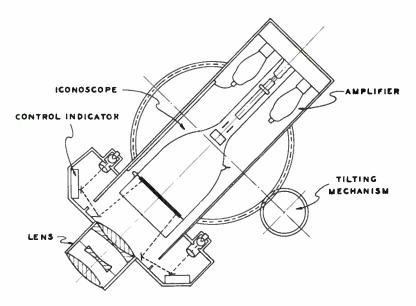
Fig. 2-Iconoscope camera for the Flying Torpedo.
