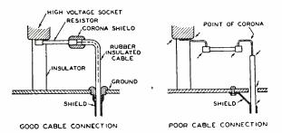
Fig. 10-Corona shielding of cable connections.
