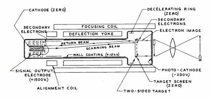
Fig. 2-Cross-sectional diagram of the image orthicon.
