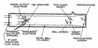
Fig. 3--Cross-sectional diagram of the Mimo tube.
