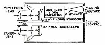
Fig. 7-Combination duplicate-lens and kinescope view finder.
