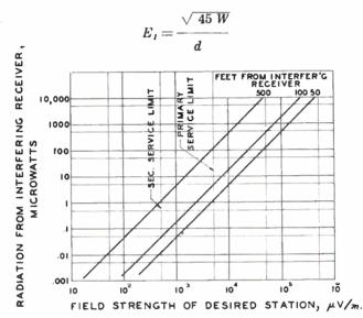
Fig. 8—Permissible radiation from television receiver to give an interference level of -20 decibels. A half-wave dipole is assumed on the receiver causing the interference.
