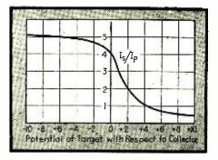
Fig. 5-Secondary emission characteristic of photosensitized silver.
