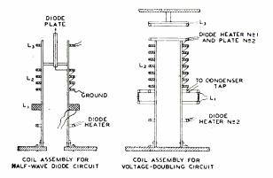
Fig. 9-Typical high-frequency transformer assemblies.
