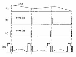
Fig. 4—Width-modulated duplex wave forms. (A) audio modulation M(t)
