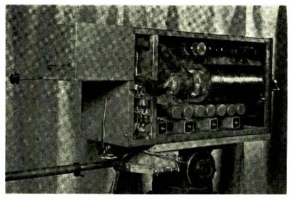
Fig. 4-Experimental Color Camera, Right Side.
