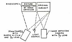
Fig. 9-Setup for comparing the sensitivities of image orthicon and photographic film.
