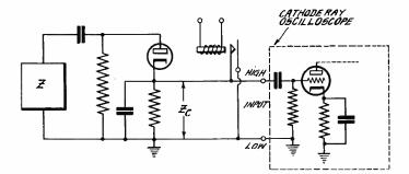
Fig. 1—Diode rectifier, "Vibroswitch," and cathode ray oscilloscope circuit arrangement.
