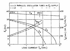
Fig. 15-Regulation characteristics of the 30-kilovolt supply.
