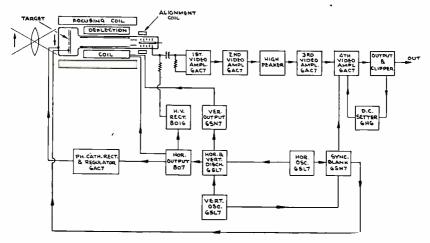
Fig. 2-Camera Block Diagram.
