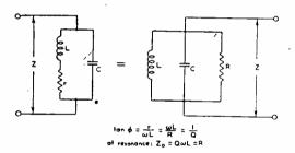
Fig. 1—Power factor and impedance of tuned circuits.
