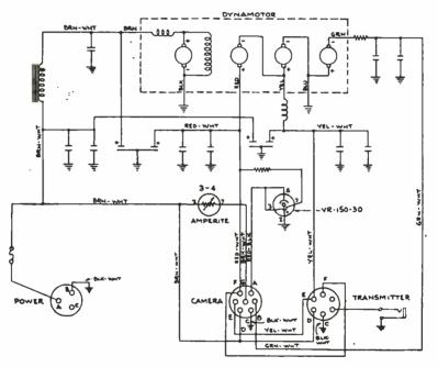
Fig. 13-Mimo power supply diagram.
