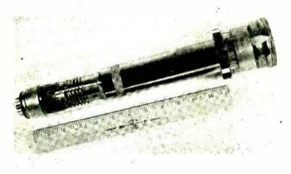
Fig. 7-The image orthicon-a sensitive television pick-up tube.
