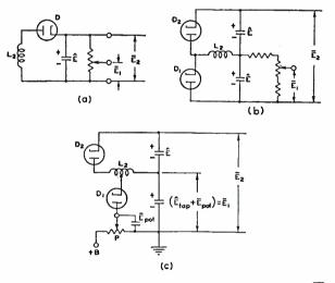
Fig. 5-Rectifier circuits for kinescope supply voltages  $\overline{E_1}$  and  $\overline{E_2}$ .
