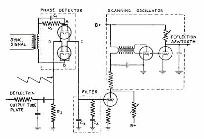
Fig. 10-Four-diode automatic frequency- and phase-controlled circuit.
