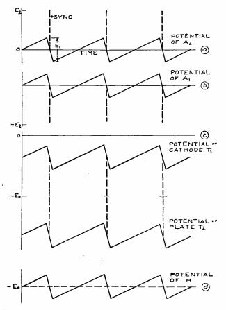
Fig. 6-Composite signals for possible equilibrium position.
