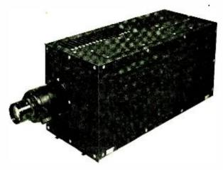
Fig. 7-External View of Camera Assembly with Lens
