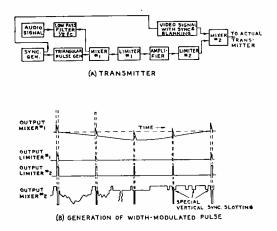
Fig. 6-Width-modulated duplex-system transmitter.
