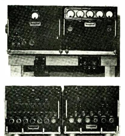
Fig. 13—The video transmitter and linear power amplifier. (These are shown at the top, mounted together as a unit on a special shock mounting. The remote control box and modulation indicator unit are shown mounted below the transmitter. The lower two units are the transmitter and power amplifier power supplies.)
