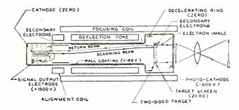
Fig. 2-Diagram of the image orthicon.
