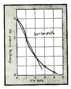
Fig. 6-Charging current characteristic of an Iconoscope mosaic.
