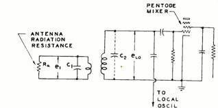
Fig. 9—Typical pentode mixer with double-tuned input circuit. The required local oscillator voltage is indicated as  $e_{Lo}$ , whereas the resulting antenna voltage is shown as  $e_1$ .
