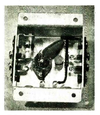
Fig. 7-Internal view of radio-frequency amplifier.
