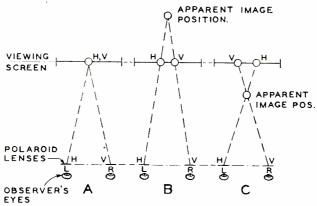
Fig. 13-The Geometry of Stereo Viewing.
