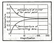
Fig. 4—Manner in which the semi-apertures of the mirror and correcting lens vary with magnification.
