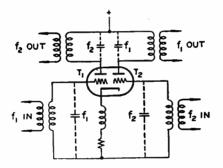
Fig. 10-Bidirectional-amplifier circuit.
