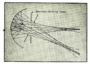
Fig. 2-Spherical mirror with an aperture at its center of curvature.
