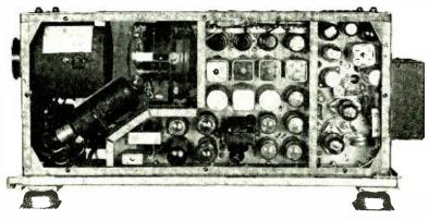
Fig. 2-Camera transmitter-tube side.
