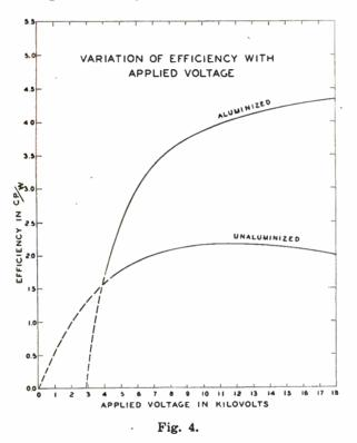
trolled by the aluminum thickness is primarily dictated by such considerations as operating voltage and ion spot elimination. As seen from Figure 4, the increase in efficiency above the cross-over voltage is quite considerable; for luminescent screens with poor secondary emission characteristics, the gain may be considerably greater than that shown on the figure.
