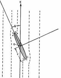
Fig. 2—A platelike particle is viewed edge on in an electric field. The field component parallel to the surface induces charges on the particle and the field component perpendicular to the surface acts upon these induced charges to produce a torque which tends to rotate the particle so as to place its long axis parallel to the electric field.
