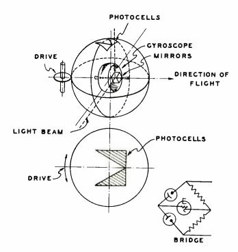
Fig. 4--Control mechanism of the Flying Torpedo.
