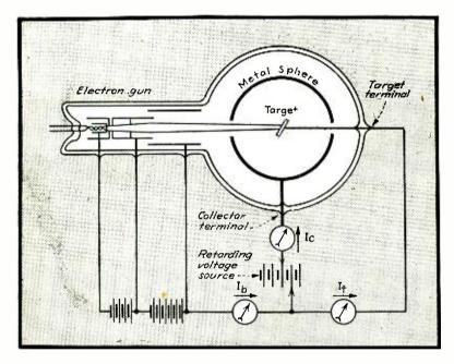
Fig. 1—Essential features of special cathode-ray tube developed for studying electron bombardment of target surfaces.
