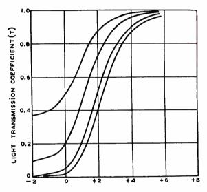
Fig. 3—Theoretical curves of light transmission as a function of time t for a suspension of particles of infinite shape factor, under a constant orienting field. The constant  $c = E^2(\epsilon/\mu)$ . At ct = 0 all particles lie at 45 degrees to the field.
