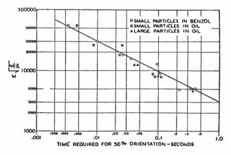
Fig. 5—Time required for light transmission to rise to half of its final value as a function of the parameter  $E \sqrt{e/\mu}$ . This curve checks the square-law response to field strength, the effect of dielectric constant and viscosity, and the independence of particle size upon rate of orientation.
