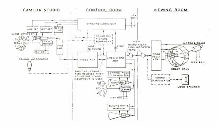
Fig. 2-Block Diagram of Color Television System.
