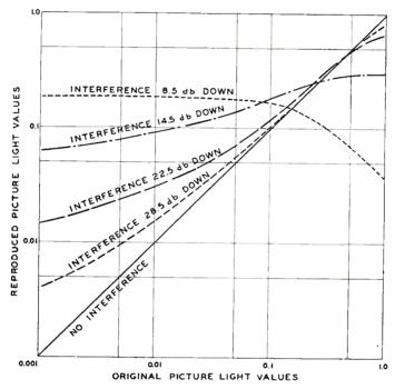
Fig. 5—Effect of c-w interference on television picture contrast using a direct current restorer which follows the average of the synchronizing pulse. Kinescope gamma = 2, transmitter gamma = ½, and vestigial side-band operation using U. S. standards.
