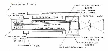
Fig. 3—Image orthicon (schematic).
