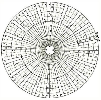
Fig. 11—Chart for square-wave synthesis.Scale0.05-microsecond intervals10.25 Mc30.75 Mc51.25 Mc71.75 Mc
