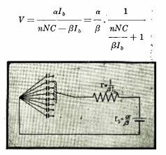
Fig. 7---Equivalent circuit of a dark mosaic undergoing scanning.
