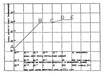
Fig. 5-Signal versus light characteristic.
