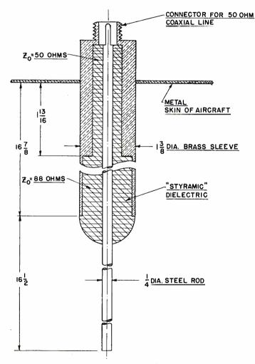
Fig. 15-Transmitting antenna.
