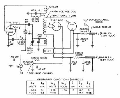
Fig. 8—Circuit and operating conditions of the 10-kilovolt supply for kinescopes.
