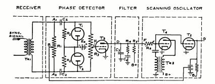
Fig. 5-Automatic frequency- and phase-controlled circuit.
