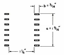
Fig. 6-Dimensions of high-voltage coil for 10 to 15 kilovolts.
