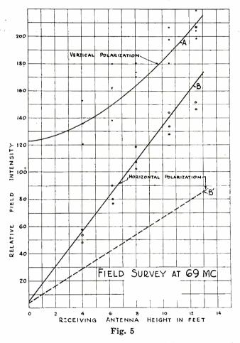
of theoretical calculations<sup>3</sup>, in which a ground dielectric constant of 15 and a transmitter height of 43 feet were assumed. With a transmitter antenna height of 5 feet, the response to horizontally polarized waves relative to vertically polarized waves would be approximately in the ratio of Curve B' to Curve A.
