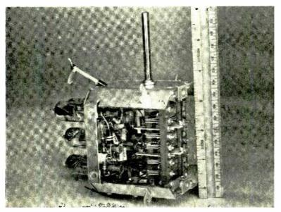
Fig. 16-Block I receiver tuning unit-top cover removed.
