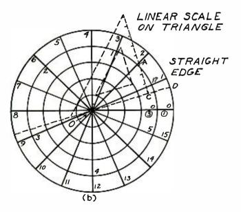
Fig. 14 (a) Basic principle of construction of synthesis charts. (b) Use of synthesis charts.
