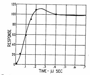
Fig. 8—Exact response to a unit function of a 2-stage compensated resistance-capacitance amplifier where  $K = \sqrt{2}$  and  $f_0 = 3$  megacycles. Points shown were obtained by synthesis from theoretical amplitude and delay characteristics in Figure 7.
