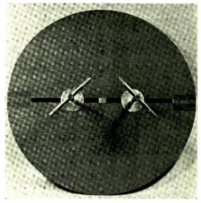
Fig. 16-Two dipoles as Mimo-plane antenna.
