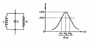
Fig. 16-Impedance characteristic of band-pass filter.
