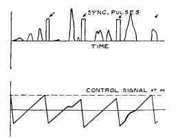
Fig. 9-Synchronizing signal and control signal when noise is present.
