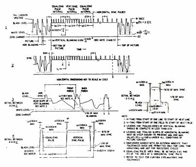
Fig. 1-Television synchronizing wave form.
