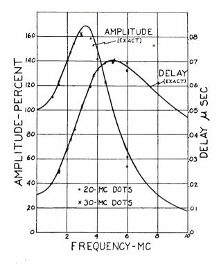
Fig. 9—Theoretical amplitude and delay characteristics of a 2-stage compensated resistance-capacitance amplifier in which K = 1.1 and  $f_0 = 4$  megacycles. Amplitude and delay characteristics determined by chart analysis of Figure 10 are shown by data points.
