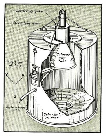
Fig. 11—Method of mounting optical components of a projection television system to give rigidity while permitting adjustments when required.
