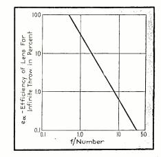
Fig. 7—Variation of lens efficiency with its f/number
