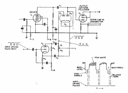
Fig. 9-Keyed black-level clamp circuit.
