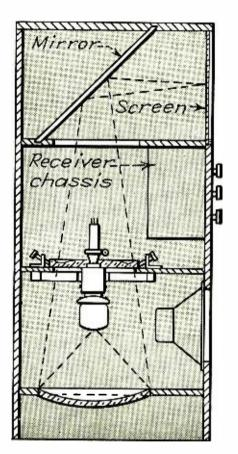
Arrangement of optical system for a home television receiver employing reflective optical principles. This design gives a large-screen picture with a console cabinet no deeper than that of an ordinary home radio receiver.
