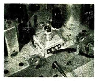
Fig. 6-Radio-frequency amplifier on RCA television-receiver chassis.
