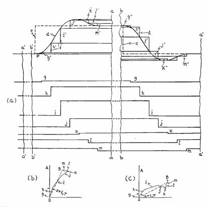
Fig. 1—(a) Approximation of a square-wave response d by a stepped wave f. (b) Vector addition of components of frequency  $f_n$  in waves g, h, i, etc. (c) Vector addition of components of frequency  $2f_n$  in waves g, h, i, etc.
