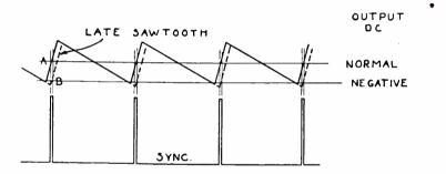
Fig. 11-Equilibrium and off-equilibrium conditions for four-diode circuit.
