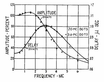
Fig. 7—Curves show exact amplitude and delay characteristics of a 2-stage compensated resistance-capacitance amplifier in which  $K = \sqrt{2}$ ,  $f_0 = 3$  megacycles. Amplitude and delay characteristics determined by chart analysis of Figure 8 are shown by data points.
