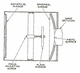
Fig. 9-Construction of the Reflective Optical System
