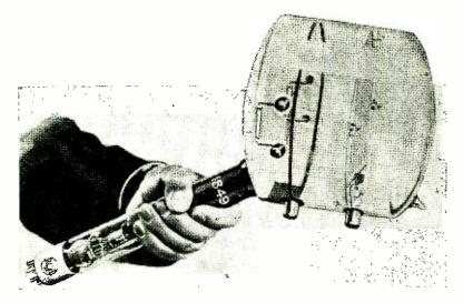
The Iconoscope—a television pickup tube.
