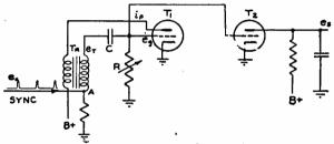
Fig. 1-Conventional triggered scanning oscillator.
