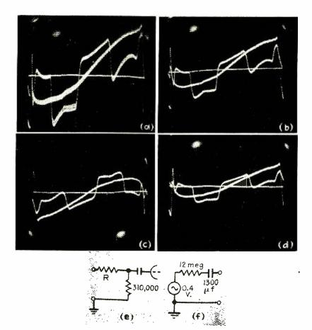
Fig. 11—Internal impedance measurements on an Iconoscope having a beam current of 0.1 µa and a 180-cycle square-wave output signal. Impedance values R in Iconoscope circuit (c) for the four oscillograms are as follows:
