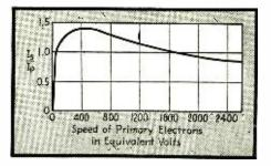
Fig. 2—Ratio of secondary electrons to primary electrons as plotted against speed of primary electrons when using a pure nickel target in the tube of Fig. 1.
