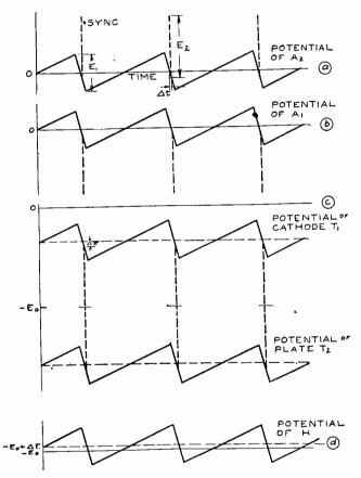
Fig. 7-Phase of saw-tooth delayed from equilibrium position of Fig. 6.
