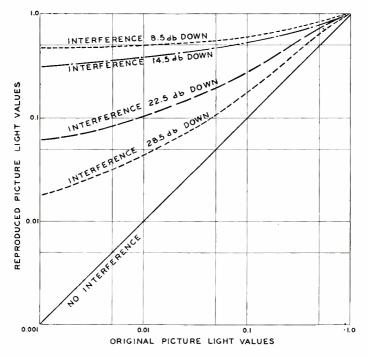
Fig. 6—Effect of c-w interference on television picture contrast using a peak-operated direct current restorer and no limiter. Kinescope gamma = 2, transmitter gamma  $= \frac{1}{2}$ , vestigial side-band operation using U. S. standards.
