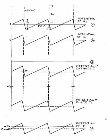
Fig. 8-Phase of saw-tooth advanced from equilibrium position of Fig. 6.
