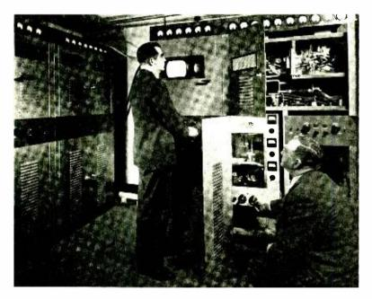
Fig. 3-288-megacycle television transmitter.
