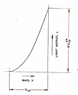
Fig. 3—Characteristic of an assumed power-law kinescope following the equation  $L = K (V_{ee} + V)^{\gamma_R}$
