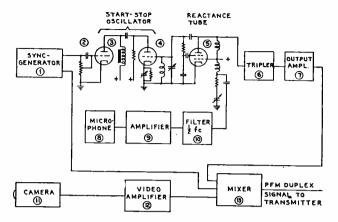
Fig. 10-Transmitter for pulsed frequency modulation.
