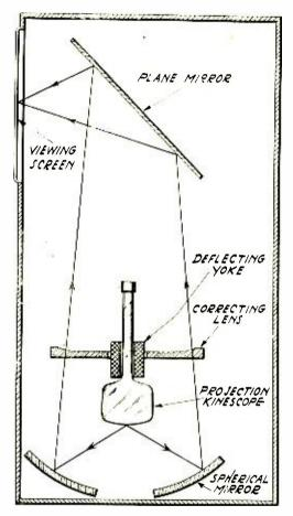
Fig. 11—Cross-sectional sketch of reflective optical system used in television receivers to produce an enlarged image by projection.
