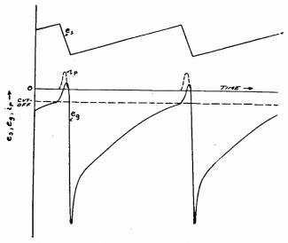
Fig. 2-Operation of the scanning oscillator.
