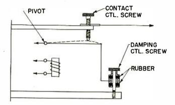
Fig. 2-Mechanical schematic diagram of the "Vibroswitch."
