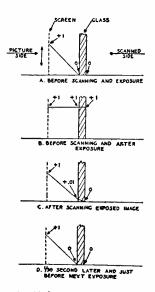
Fig. 4-Target potentials during a typical scanning cycle.
