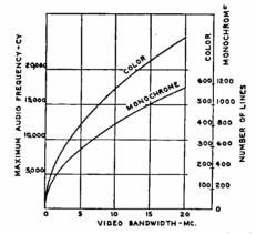
Fig. 3—Maximum audio frequency versus video bandwidth and number of lines.
