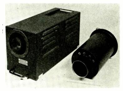
Fig. 3-The BC-1212 iconoscope camera and the Mimo camera.
