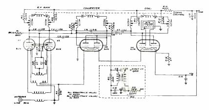
Fig. 17-Block I receiver tuning unit-schematic diagram.
