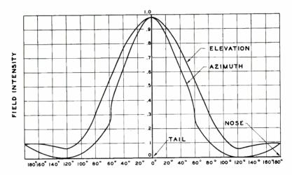
Fig. 15-Radiation patterns of the "Roc" dipole at 310 megacycles.
