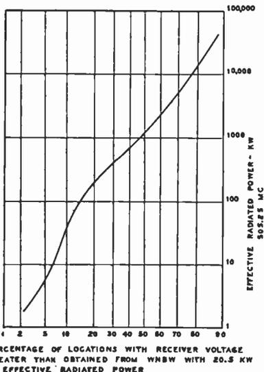
Fig. 18—A statistical analysis of the voltages on receiver terminals in home locations, expressed in terms of power requirements at 505.25 megacycles in order that a given percentage of locations shall have as great a signal as obtained from WNBW with 20.5 kilowatts of effective radiated power.
