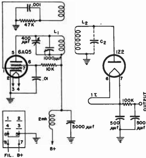
Fig. 1—Circuit of 4-kilovolt supply.
