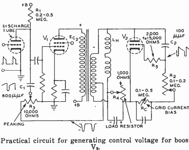
Fig. 17—Practical circuit for generating control voltage for booster triode,  $V_2$ .
