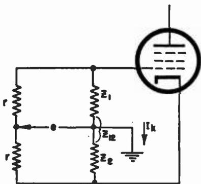
Fig. 2—Grid-cathode fed tube with longitudinal induced voltage.
