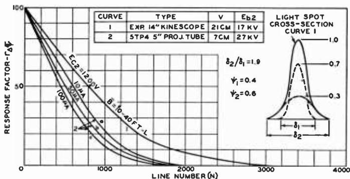
Fig. 42—Aperture flux response of two kinescopes.
