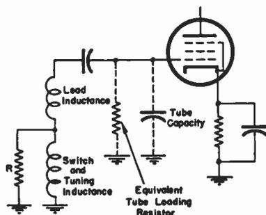
Fig. 7—High-frequency equivalent circuit of the mixer input.
