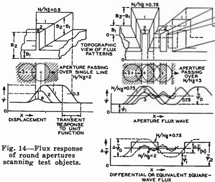
Fig. 14—Flux response of round apertures scanning test objects.
