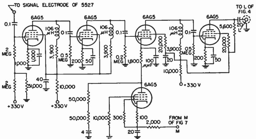
Fig. 3—Video preamplifier circuit.
