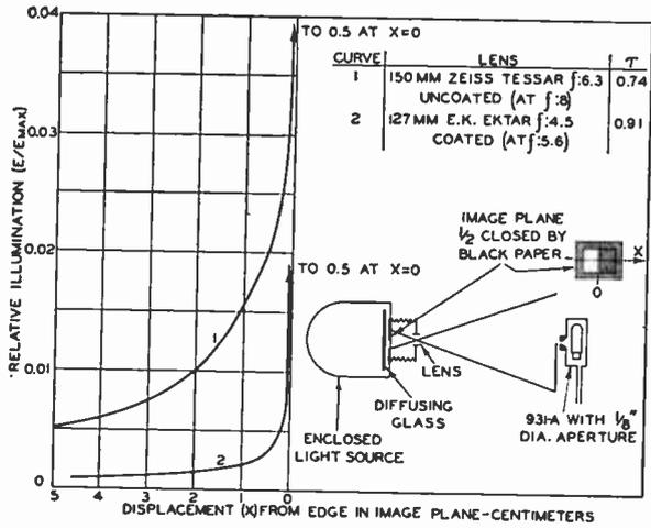
Fig. 48—Transition curves for coated and uncoated lens.
