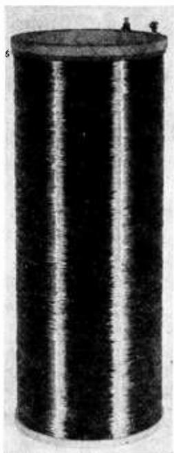
Fig. 7—Focus field coil for the image orthicon.
