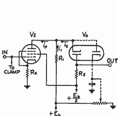
Fig. 20 — Schematic diagram of linear clipper.
