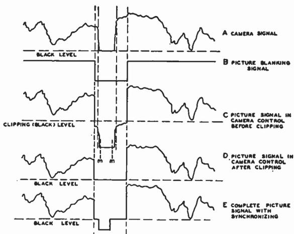
and is applicable only in cases where there are pulse intervals present in the amplifier signal during which the switching operation can take place. Since a television picture signal (having blanking pulses to suppress the scanning beam during the retrace periods) is of this type, the clamp circuit may be used successfully.
