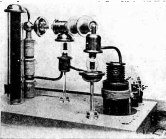
Fig. 3—Side view of 90-kilovolt tripler.
