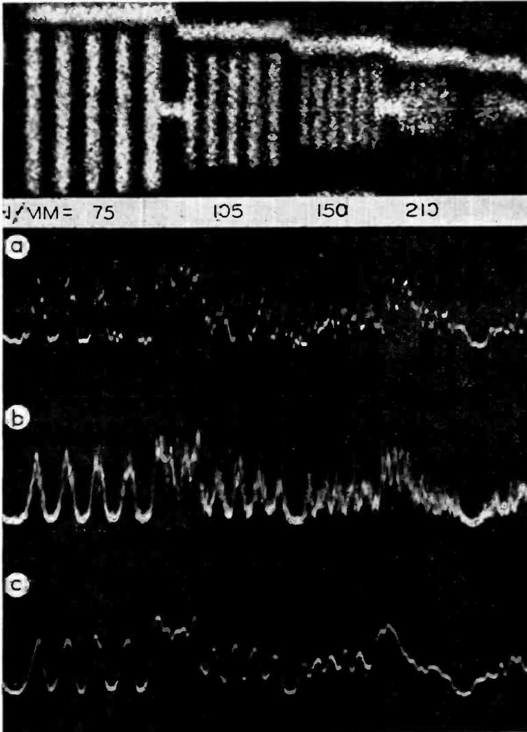
Fig. 78—Kinescope image and microphotometer traces showing limiting resolution of microfilm. a. Single line cross section. b. Six line cross sections superimposed. c. Single line cross section traced with larger scanning beam not resolving individual grains.
