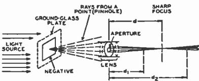
Fig. 21—Aperture effect on shape of point-imaging beam in out-of-focus imaging.
