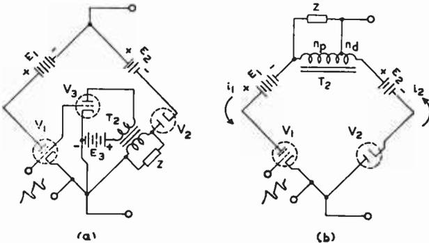
Fig. 12—Diode switch circuits with negative resistance ( $-R$ ).
