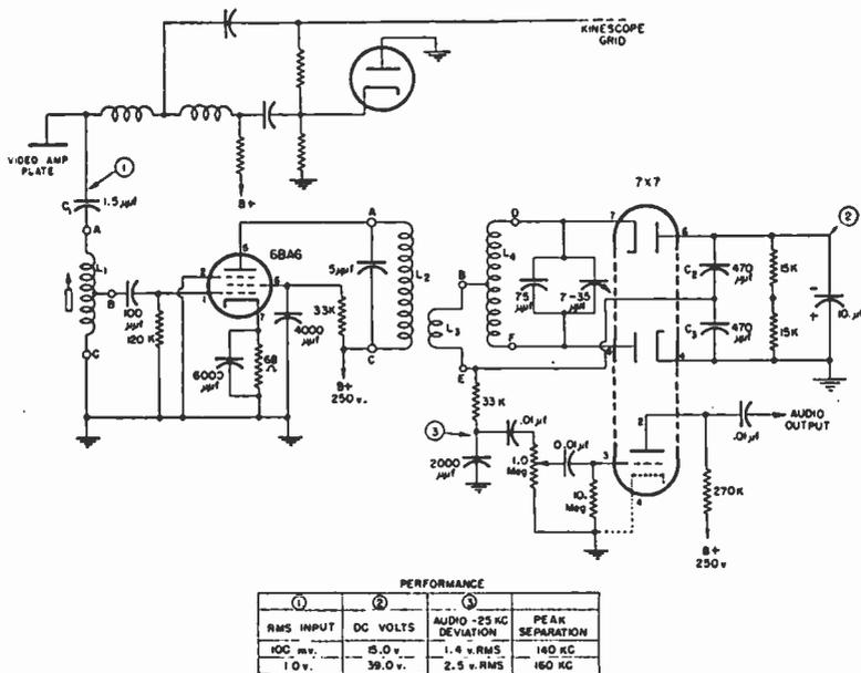
Fig. 7—Circuit diagram of 4.5-megacycle amplifier and detector.
