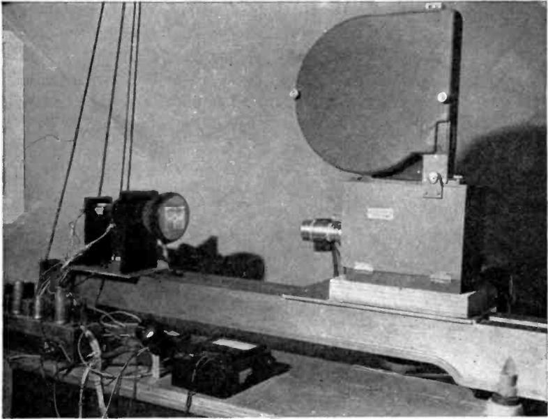
Fig. 3—The Eastman Kodak television recording camera.
