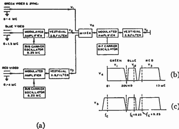
Fig. 1 — Simultaneous color transmitter of the subcarrier type.
