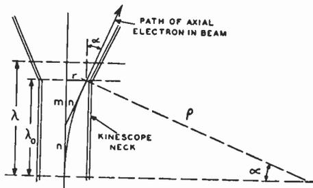
Fig. 22—Path of electron beam through transverse deflection-coil field of kinescope. ( $m = n \cos \alpha$ ;  $n = r / \sin \alpha$ ;  $\lambda_o = m + n = r (1 + \cos \alpha) / \sin \alpha$ ).
