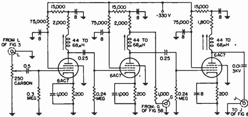
Fig. 4—Circuit of video line amplifier.
