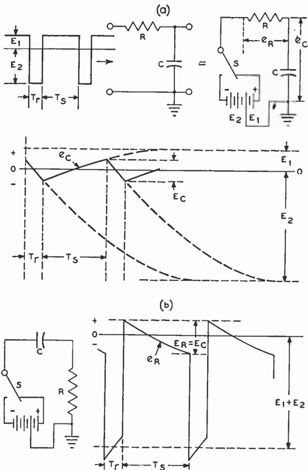
Fig. 16—Generation of control voltage for booster triode,  $V_s$ .
