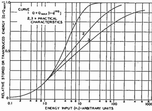
Fig. 45—Transfer characteristics with diminishing returns.
