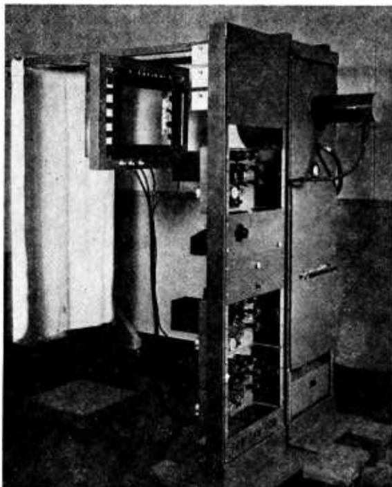
Fig. 16—The live-pickup scanner.
