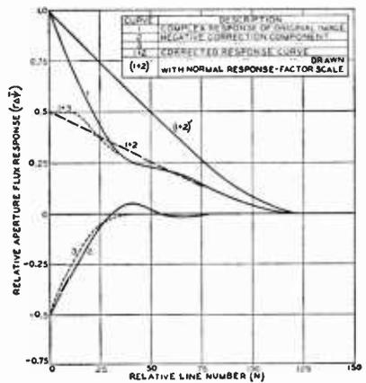
Fig. 93—Aperture response correction by "negative" response characteristics.
