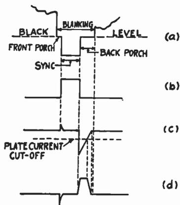
Fig. 18 — Derivation of keying pulses for back-porch clamping.
