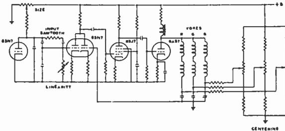
Fig. 7—Vertical-deflection circuit.
