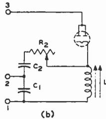
Circuit (b) combines  $C_2$  and  $C_3$ , but is restricted by capacitive tap to higher Q-values and more critical operating conditions (Class B) than circuit (a). Ratio  $C_2/C_1$  adjusts stepdown.
