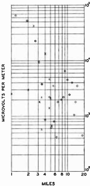
Fig. 20—A comparison of field intensity data with voltage on receiver terminals. The circles are the measured field intensities along the northnorthwest radial. The crosses are the apparent field intensity obtained from the receiver terminal voltages at home locations divided by the effective height of a dipole antenna.
