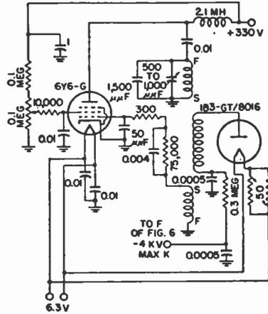
Fig. 9—R-f operated high-voltage supply for the 7GP4.
