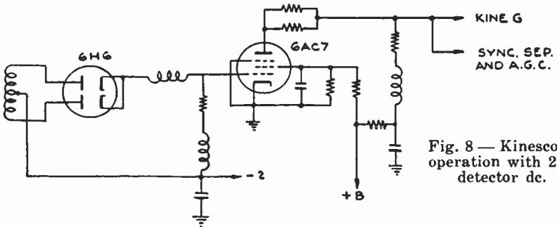
Fig. 8 — Kinescope operation with 2nd detector dc.
