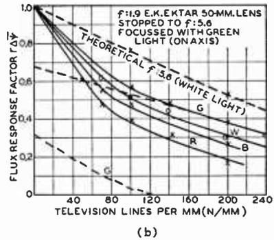
Fig. 58—Flux response characteristic of miniature-camera lenses illustrating chromatic aberration.
