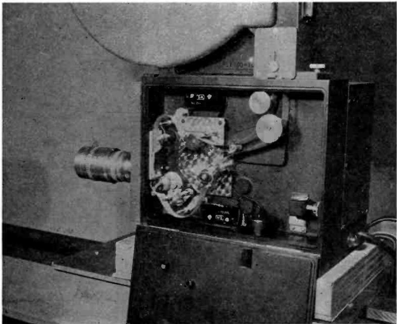
Fig. 4—Eastman Kodak camera interior showing film threading.
