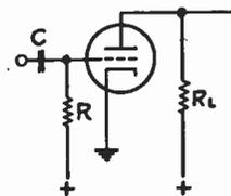
Fig. 19 — Schematic diagram of differentiating circuit.
