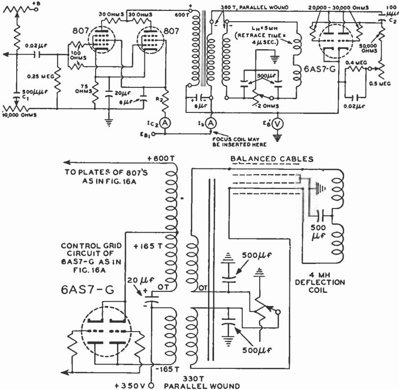
Fig. 20—Practical circuits with power feedback for balanced and unbalanced deflection-coil connections with 6AS7-G triode.
