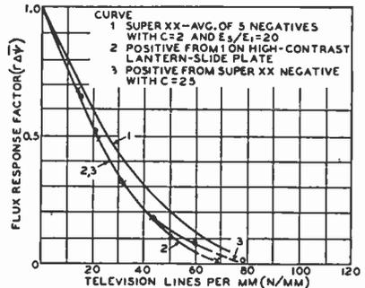
Fig. 80 — Aperture response of Super XX film before and after transfer on fine-grain positive film.
