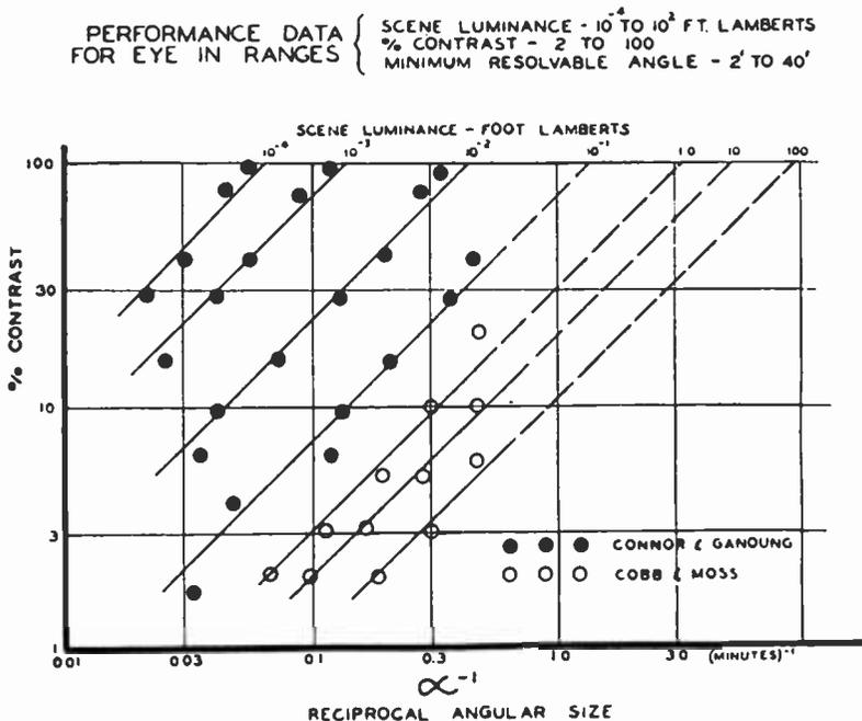
Fig. 7—The solid lines with 45-degree slope are approximations to the experimental data by ideal performance curves.
