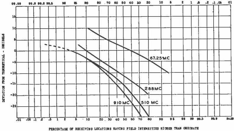
Fig. 16—An analysis of the data shown in Figures 11 to 14. (A curve for a given frequency relates the measured field intensities at that frequency to the theoretical curve for the same frequency.)
