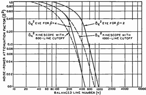
Fig. 10—Noise attenuation due to filter effect of eye or kinescope.
