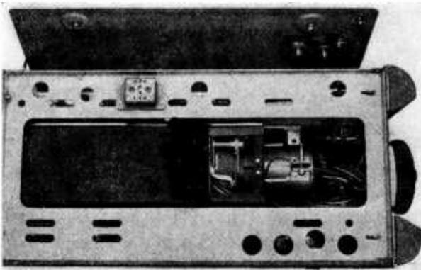
Fig. 6—Top view of camera, showing coil assembly.
