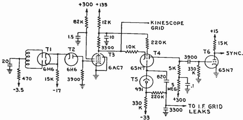
Fig. 5—Combined AGC and sync separator.
