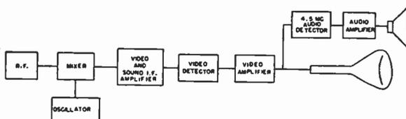
Fig. 2—Intercarrier receiver.
