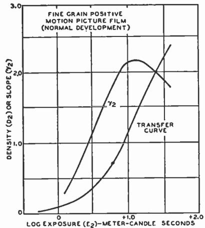
Fig. 73 — Transfer characteristics of motion picture film.
