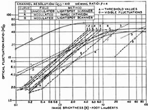
Fig. 90 — Development of characteristic curves of the optical signal-to-fluctuation ratio  $|R|_o$  for threshold grain visibility at various brightness levels.
