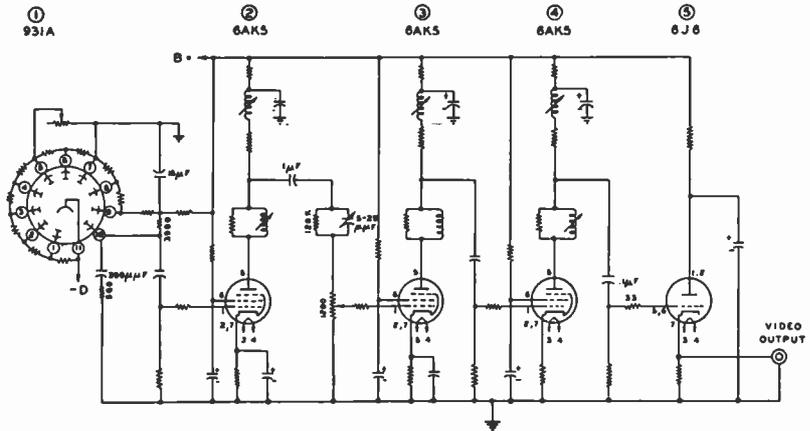
Fig. 9—The circuit diagram of the equalizing amplifier.
