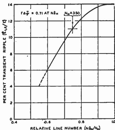
Fig. 38—Aperture size ( $1/N\delta_H$ ) of frequency channels as a function of transient ripple.
