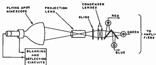
Fig. 1—Diagram of the color-slide scanner.
