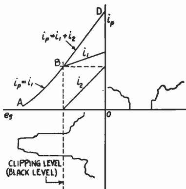
Fig. 21 — Characteristic curve of linear clipper.
