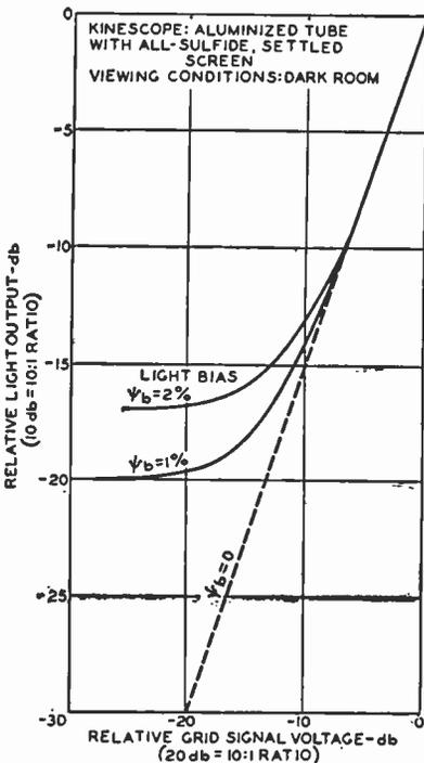
Fig. 87—Dynamic transfer characteristics of kinescope.
