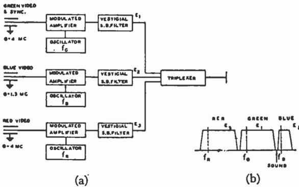
Fig. 2—Simultaneous color transmitter of the three-carrier type.
