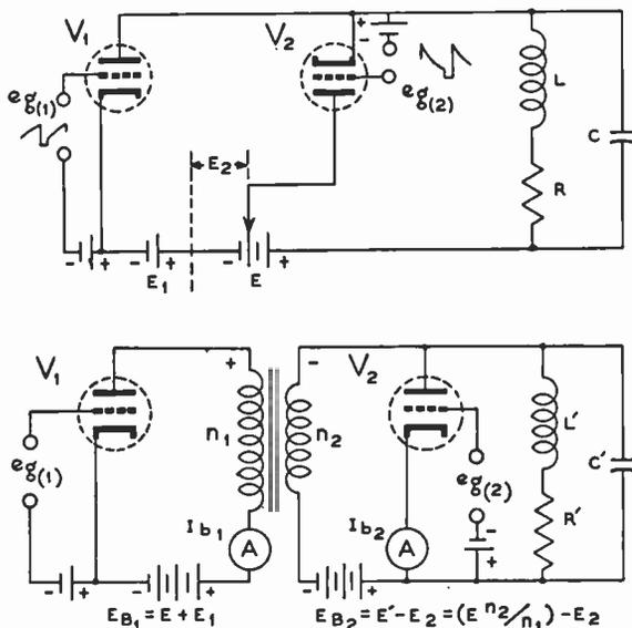
Fig. 8—Practical circuits with two controlled electron tubes.
