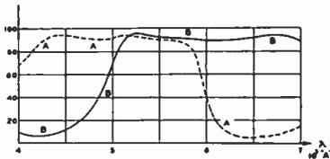
Fig. 4—Spectral characteristic of two dichroic mirrors.
