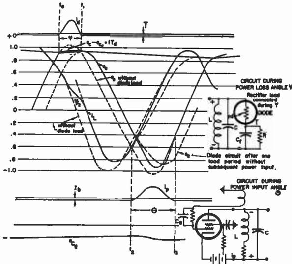
Fig. 18—Oscillator-rectifier circuit power relations.
