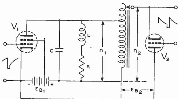
Fig. 18—Circuit with parallel connection for power feedback.
