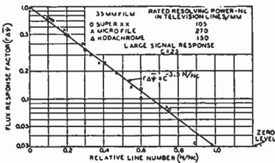
Fig. 79—General aperture response characteristics of photographic film for large signals.
