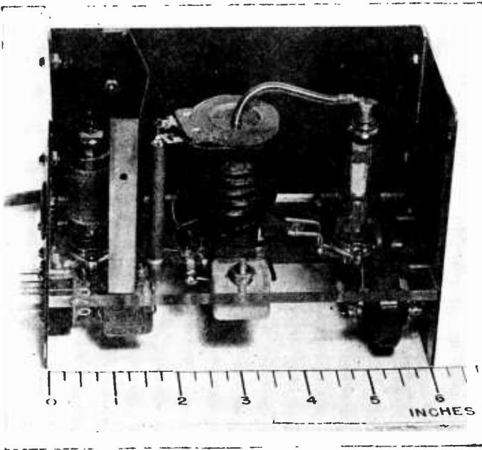
Fig. 22—Side view of 4-kilovolt supply.
