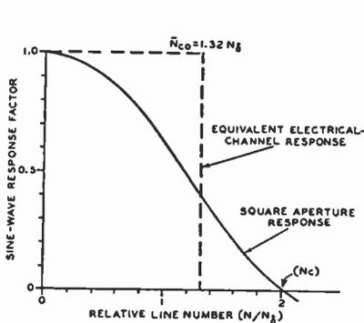
Fig. 77—Sine-wave response characteristics with equal filter effect on the RMS value of random fluctuations.
