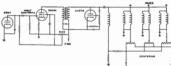
Fig. 6—Horizontal-deflection circuit.
