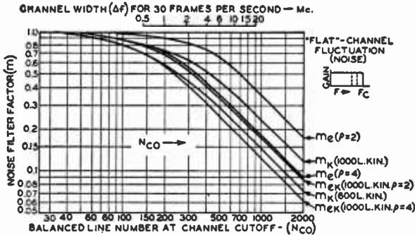
Fig. 11a—Effect of channel width on fluctuation filter factors for a flat channel.
