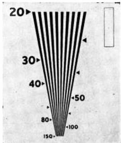
Fig. 22—Wedge test pattern and pinhole apertures in sharp focus.
