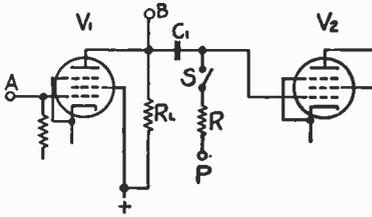
Fig. 16—Simplified schematic diagram of clamp circuit.
