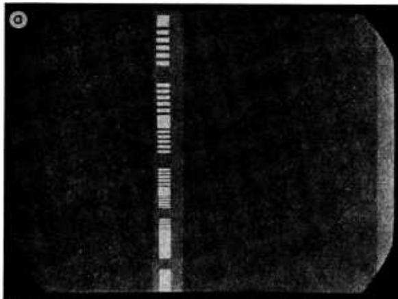
Fig. 29 — Kinescope images of "vertical" aperture-response samples.
