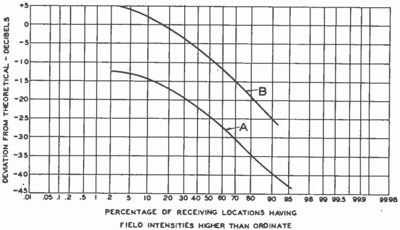
Fig. 16—An analysis of the data shown in Figures 8 to 15. Curve A relates the measured field intensities at 505.25 megacycles to the theoretical curve for the same frequency. Curve B relates the measured field intensities at 505.25 megacycles to the theoretical curve at 67.25 megacycles.
