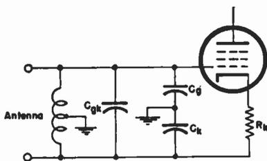
Fig. 3—Distributed capacities of grid-cathode fed tube.
