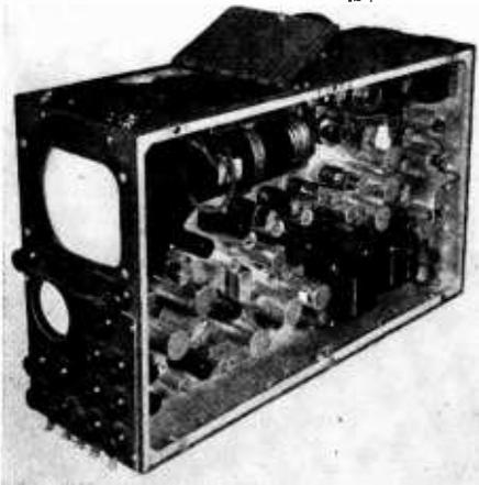
Fig. 10—Field-camera control.
