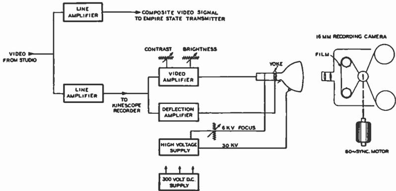
Fig. 5—Kinescope photographic monitor block diagram.
