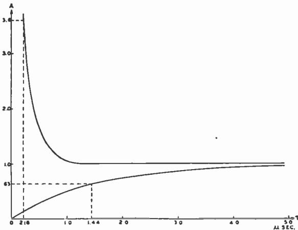
Fig. 8— Unit-function responses of the flying - spot scanner.
