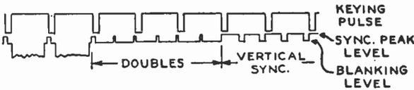
Fig. 11—Absence of blanking level during vertical sync and keying pulse.
