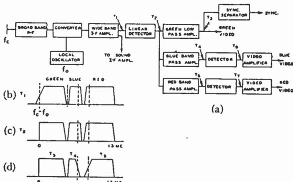
Fig. 3 — Simultaneous color receiver for subcarrier reception.
