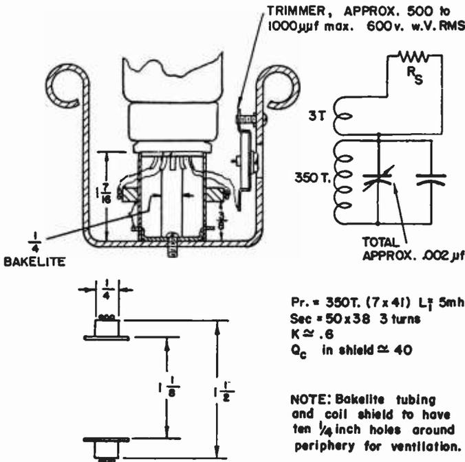
Fig. 14—Typical filament transformer assembly.
