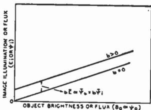
Fig. 49(a) — Transfer characteristics and "flare" light-bias of a lens.
