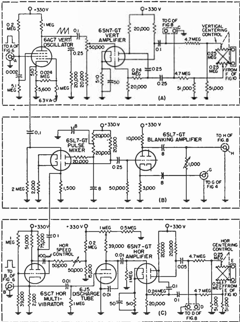
Fig. 5—(Top) Vertical oscillator and scanning circuit for the 5527. (Middle) Mixing and blanking circuits. (Bottom) Horizontal multivibrator and scanning circuit for 5527.
