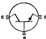
Silicon n-p-n type used in a wide variety of aerospace, military, and industrial applications requiring a high degree of reliability. The high current-handling capability of this type and its fast switching speed
