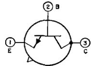
small-signal beta, very low capacitance, and large gain-bandwidth product. JEDEC No. TO-46 package; outline 18, Outlines Section. This type is electrically identical with type 2N2896.
