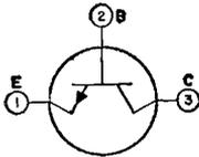
Germanium n-p-n type used in low-noise small-signal audio-frequency amplifier applications. It is used in input stages of audio-frequency amplifiers operating from extremely small input signals, such
