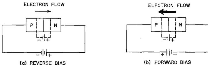
Figure 7. Electron current flow in biased p-n junctions.
