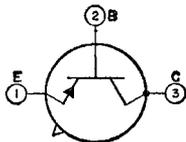
Germanium p-n-p type used in high-speed saturated switching applications in industrial data-processing equipment. JEDEC No. TO-18 package; outline 12, Outlines Section.
