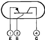
Germanium p-n-p type used in large-signal audio-frequency amplifier applications. It is used in single-ended or double-ended output stages, in high-gain class A driver stages of radio receivers and
