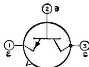
JEDEC No. TO-5 package; outline 6, Outlines Section. For curve of typical transfer characteristics, refer to type 2N1893.
