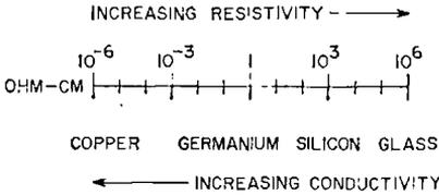
Figure 1. Resistivity of typical conductor, semiconductors, and insulator.
