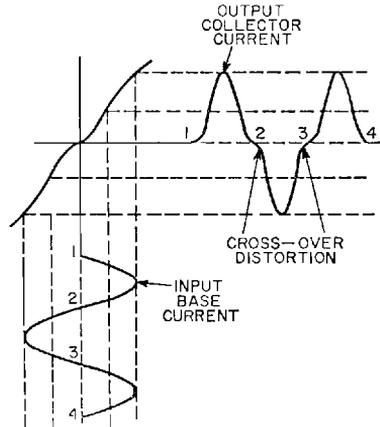
Figure 44. Waveforms showing cause of cross-over distortion.
