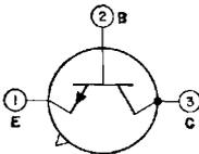
Germanium n-p-n type used for low-power radio-frequency amplifier applications in the vhf range in industrial and military equipment. JEDEC No. TO-18 package; outline 12, Outlines Section.
