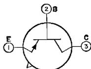
Germanium p-n-p type used in medium-speed switching applications in data-processing equipment. JEDEC No. TO-5 package; outline 6, Outlines Section. This type is identical with type 2N404 except for
