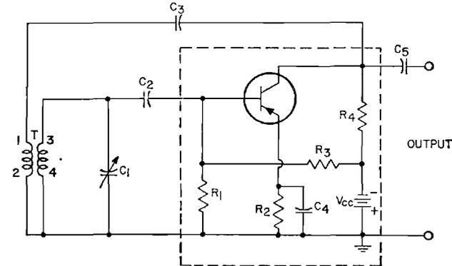
Figure 64. Tuned-base oscillator.
