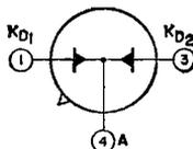
ambient temperature range = -65 to 85°C. Package is similar to JEDEC No. TO-33 (outline 13, Outlines Section) except that lead No. 2 is omitted. This is a discontinued type listed for reference only.
