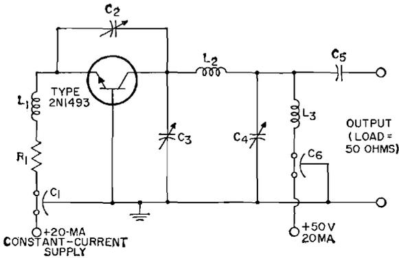
$C_1, C_5 = 1000$  pf, feed-through, ceramic
