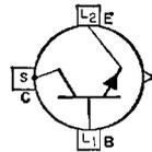
and relay control circuits; in oscillator, regulator, and pulse-amplifier circuits; and as a class A or class B push-pull audio and servo amplifier. It features low saturation resistance, high current and power dissipation, high beta at high current, and excellent high-temperature performance. This type is stud-mounted to provide positive heat-sink contact and has a cold-weld seal. JEDEC No. TO-36 package; outline 14, Outlines Section. This type is electrically identical with type 2N1488.
