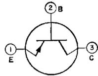
audio-amplifier and driver stages. It features a high small-signal forward current-transfer ratio, excellent linearity over the entire range of collector current, high cutoff frequency, low saturation currents, and uniform gain characteristics over the entire audio-frequency spectrum. JEDEC No. TO-1 package; outline 4, Outlines Section.
