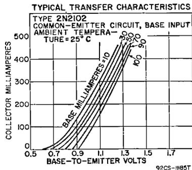
Figure 25. Transfer-characteristic curves.
