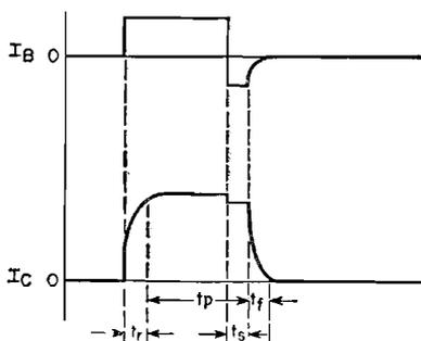
Figure 75. Current waveforms obtained in switching circuit.
