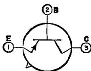
Germanium p-n-p bidirectional type used in medium-speed switching circuits in data-processing equipment. This type is designed so that the emitter can also function as a collector and the collector can
