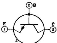
Germanium n-p-n type used in medium-speed switching applications in data-processing equipment. JEDEC No. TO-5 package; outline 6, Outlines Section. This type is identical with type 2N1302 except
