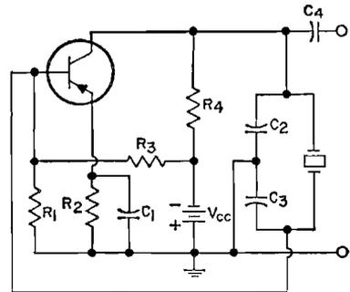
Figure 69. Pierce-type transistor crystal oscillator.
