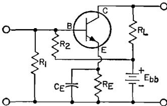
Figure 33. Bias network using emitter stabilizing resistor.
