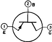
Germanium p-n-p type used in radio-frequency amplifier applications in battery-operated AM portable radio receivers. In an unneutralized rf amplifier circuit, this type can provide a power gain of 25.6 db
