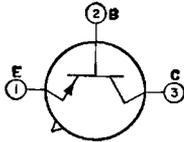
Germanium p-n-p type used in high-speed switching applications in data-processing equipment. JEDEC No. TO-5 package; outline 6, Outlines Section. Maximum ratings for this type are the same as for type
