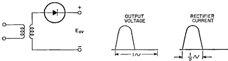
Figure 86. Single-phase half-wave circuit.
