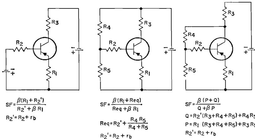
Figure 38. Circuit-stability-factor equations for three typical circuit configurations.
