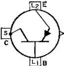
Germanium p-n-p type used in a wide variety of switching and amplifier applications in industrial and military equipment requiring transistors having high voltage, current, and dissipation values. It is used in
