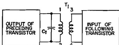
Figure 53. Single-tuned coupling network using inductive coupling.
