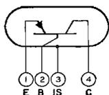
Germanium p-n-p type used as an amplifier in AM broadcast-band battery-operated portable radio receivers and short-wave receivers. JEDEC No. TO-7 package; outline 7, Outlines Section.
