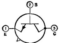
as low base and collector cutoff currents, low saturation voltages at high values of collector current, and exceptional stability of characteristics. JEDEC No. TO-52 package; outline 20, Outlines Section.
