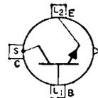
noid and relay control circuits; in oscillator, regulator, and pulse-amplifier circuits; and as a class A or class B push-pull audio and servo amplifier. It features low saturation resistance, high current and power dissipation, high beta at high current, and excellent high-temperature performance. JEDEC No. TO-36 package; outline 14, Outlines Section.
