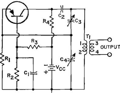
Figure 66. Transistor Colpitts oscillator.
