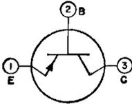
Germanium p-n-p type used in converter (mixer-oscillator) applications in battery-operated portable radio receivers. In a common-emitter circuit, this type is capable of providing a useful conversion power
