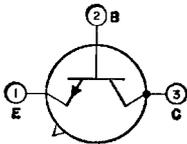
Silicon n-p-n type used in a wide variety of small-signal and medium-power applications in industrial and military equipment. It can be used in rf service as an amplifier, mixer, oscillator, and converter;
