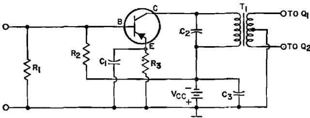
Figure 42. Driver stage for push-pull output circuit.
