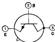
Silicon n-p-n type used in a wide variety of small-signal and medium-power applications in industrial and military equipment. It can be used in rf service as an amplifier, mixer, oscillator and converter; in af service in small-signal and power applications. It features low output capacitance and exceptionally low noise and leakage characteristics.
