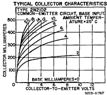
Figure 24. Collector-characteristic curves.
