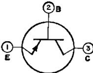
Germanium p-n-p type used in class A audio-frequency driver-amplifier applications in battery-operated portable radio receivers. JEDEC No. TO-1 package; outline 4, Outlines Section.
