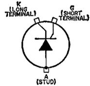
of 200 volts and a forward-current capability of 16 amperes (average value) or 25 amperes (rms value). This type is designed to meet stringent military environmental and mechanical specifications. The special high-strength copper-alloy stud can withstand an installing torque up to 50 inch-pounds. JEDEC No. TO-48 package; outline 19, Outlines Section. This type is identical with type 2N681 except for the following items:
