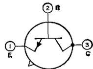
circuits. It is designed to assure freedom from second breakdown and features low leakage current and wide beta range. JEDEC No. TO-5 package; outline 6, Outlines Section.
