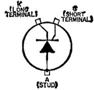
of 500 volts and a forward-current capability of 16 amperes (average value) or 25 amperes (rms value). This type is designed to meet stringent military environmental and mechanical specifications. The special high-strength copper-alloy stud can withstand an installing torque up to 50 inch-pounds. JEDEC No. TO-48 package; outline 19, Outlines Section. This type is identical with type 2N681 except for the following items:
