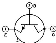
noid and relay control circuits; in oscillator, regulator, and pulse-amplifier circuits; and as a class A or class B push-pull audio and servo amplifier. It features low saturation resistance, high current and power dissipation, high beta at high current, and excellent high-temperature performance. JEDEC No. TO-5 package; outline 6, Outlines Section. This type is identical with type 2N1482 except for the following items:
