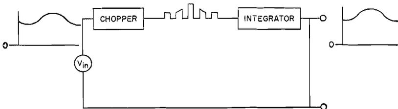
Figure 60. Block diagram showing action of "chopper" circuit.
