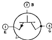
This type features high collector-to-emitter voltage ratings, fast rise time, and high power dissipation. JEDEC No. TO-5 package; outline 6, Outlines Section.
