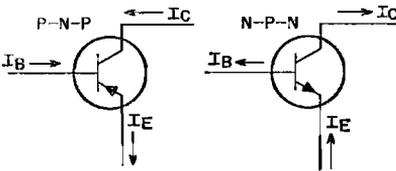
Figure 47. Electron-current flow in p-n-p and n-p-n transistors.
