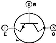
Silicon n-p-n type used in very-high-speed switching and high-frequency applications in equipment which requires high reliability and high packaging densities. JEDEC No. TO-18 package; outline 12, Outlines Section.
