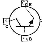
noid and relay control circuits; in oscillator, regulator, and pulse-amplifier circuits; and as a class A or class B push-pull audio and servo amplifier. It features low saturation resistance, high current and power dissipation, high beta at high current, and excellent high-temperature performance. JEDEC No. TO-36 package; outline 14, Outlines Section. This type is identical with type 2N2016 except for the following:
