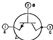
This type can also be used in switching service in circuits requiring transistors having high voltage, current, and dissipation values. JEDEC No. TO-39 package; outline 32, Outlines Section. This type is identical with type 2N1493 except for the following items:
