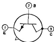
Silicon n-p-n type used in a wide variety of small-signal and high-speed switching applications. JEDEC No. TO-18 package; outline 12, Outlines Section. For curves of typical collector and transfer characteristics, refer to type 2N718A.
