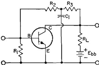
Figure 34. Bias network using split voltage-divider network.
