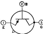
Silicon n-p-n type used in very-high-speed applications in equipments which require high reliability and high packaging densities. JEDEC No. TO-46 package; outline 18, Outlines Section.
