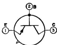
Germanium p-n-p type used in medium-speed switching applications in data-processing equipment. JEDEC No. TO-5 package; outline 6, Outlines Section. This type is identical with type 2N1303 except
