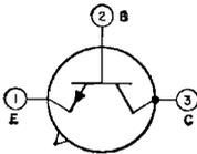
Silicon n-p-n type used in a wide variety of large-signal high-power vhf applications in military and industrial communications equipment. It is intended primarily for use in AM, FM, and CW circuits at fre-
