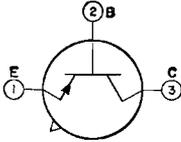
Germanium p-n-p type used in high-speed switching applications in data-processing equipment. JEDEC No. TO-5 package; outline 6, Outlines Section. This type is identical with type 2N1853 except for the
