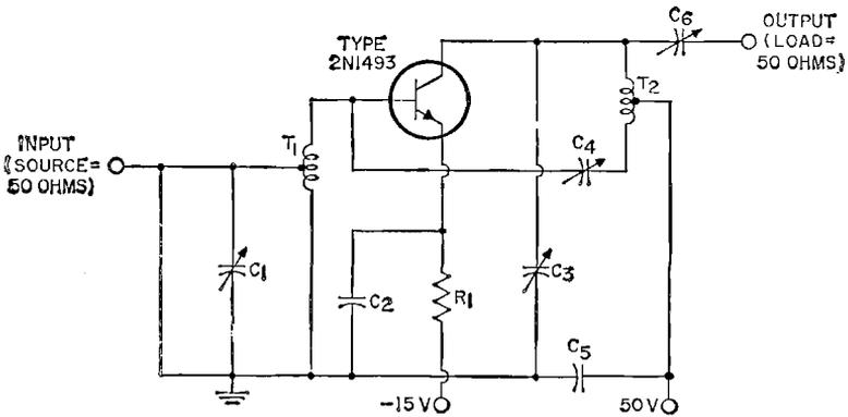
$C_1, C_3, C_4, C_5 = 3-20$  pf,
