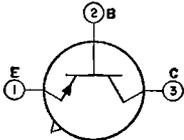
Germanium n-p-n bidirectional type used in medium-speed switching circuits in data-processing equipment. This type is designed so that the emitter can also function as a collector and the collector can
