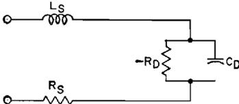
Figure 109. Equivalent circuit for a tunnel diode biased in the negative-resistance region.
