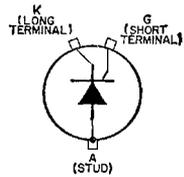
copper alloy stud can withstand an installing torque up to 50 inch-pounds. JEDEC No. TO-48 package; outline 19, Outlines Section.
