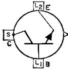
Silicon n-p-n type used in a wide variety of switching and amplifier applications in industrial equipment. It is used in power-switching, dc-to-dc converter, inverter, chopper, and relay-control
