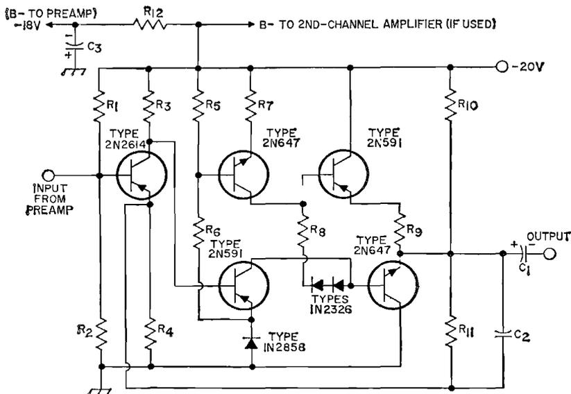
$C_1 = 250 \mu\text{f}$ , miniature electrolytic, 15 v.
