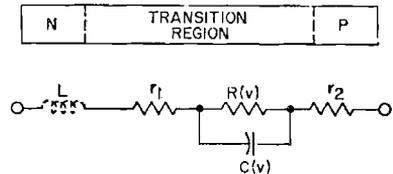
Figure 108. Equivalent circuit for a tunnel diode.
