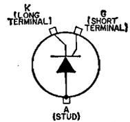
of 50 volts and a forward-current capability of 16 amperes (average value) or 25 amperes (rms value). This type is designed to meet stringent military environmental and mechanical specifications. The special high-strength copper-alloy stud can withstand an installing torque up to 50 inch-pounds. JEDEC No. TO-48 package; outline 19, Outlines Section. This type is identical with type 2N681 except for the following items:
