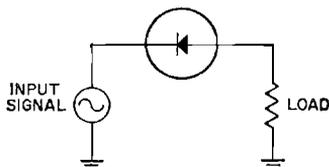
Figure 11. Simple diode rectifying circuit.
