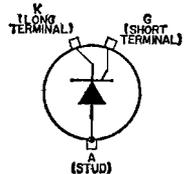
of 250 volts and a forward-current capability of 10 amperes (average value) or 16 amperes (rms value). This type is designed to meet stringent military environmental and mechanical specifications. The special high-strength copper-alloy stud can withstand an installing torque up to 50 inch-pounds. JEDEC No. TO-48 package; outline 19, Outlines Section. This type is identical with type 2N1842A except for the following items:
