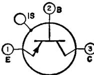
Germanium p-n-p type used in rf and if amplifier circuits; oscillator, mixer, and converter circuits; and low-level video-amplifier circuits in industrial and military equipment. It is used in the design of rf circuits
