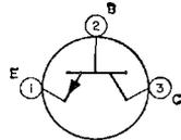
quencies up to 150 megacycles. It features high power output and high voltage ratings. This type is 100 per cent tested to assure freedom from second breakdown in class A operation at maximum ratings. It uses a special stud-mounted package which is electrically isolated from all electrodes and designed to provide excellent performance at high frequencies. Outline 35, Outlines Section.
