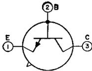
Germanium n-p-n types used in medium-speed switching applications in data-processing equipment. JEDEC No. TO-5 package; outline 6, Outlines Section.
