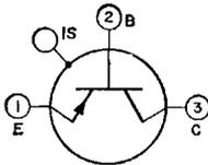
Germanium p-n-p type used in rf and if amplifier circuits; oscillator, mixer, and converter circuits; and low-level video-amplifier circuits in industrial and military equipment. It is used in the design of rf circuits
