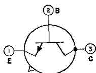
Silicon n-p-n type used in very-high-speed switching applications in equipment requiring high reliability and high packaging densities. JEDEC No. TO-18 package; outline 12, Outlines Section.
