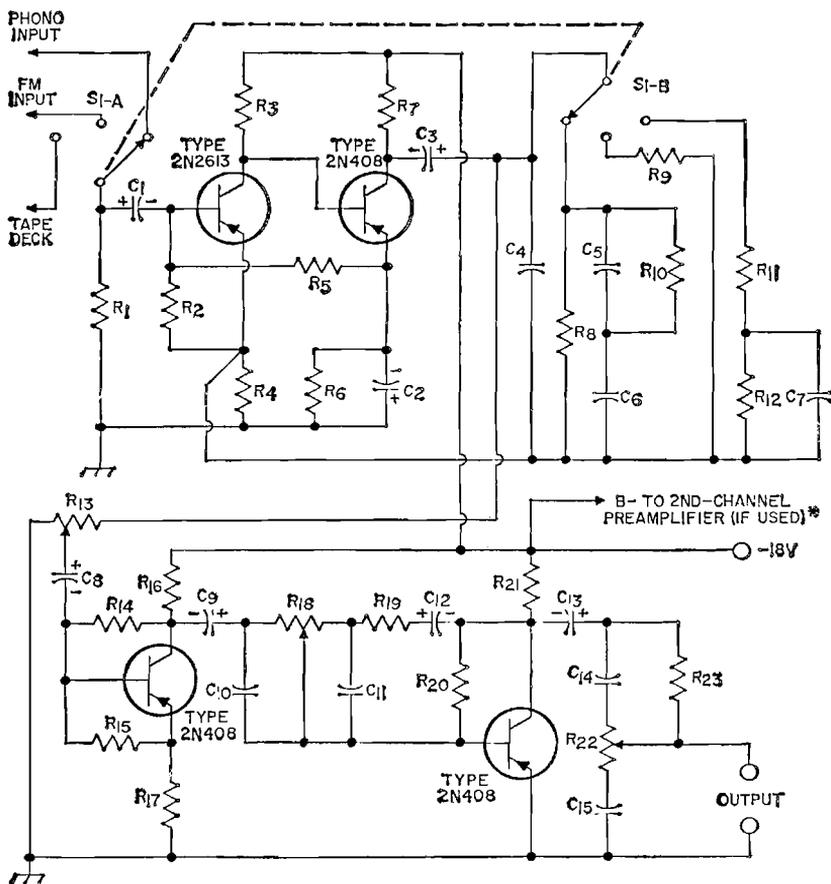
$C_1$  = 25  $\mu\text{f}$ , miniature electrolytic, 3 v.
