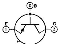
Germanium p-n-p type used in medium-speed switching applications in data-processing equipment. JEDEC No. TO-5 package; outline 6, Outlines Section. This type is identical with type 2N1303 except
