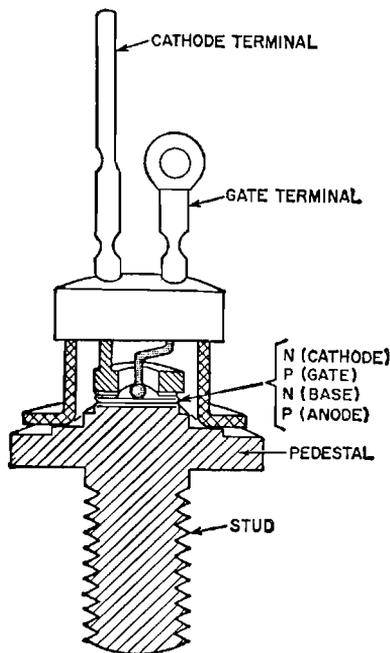
Figure 94. Construction details of typical silicon controlled rectifier.
