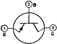
Germanium p-n-p type used in converter (mixer-oscillator) applications in AM automobile radio receivers. In an unneutralized circuit, this type can provide a useful conversion power gain of 37 db at 1.5
