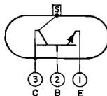
used in power switching, dc-to-dc converter, inverter, chopper, and relay actuating circuits; in voltage- and current-regulator circuits; and in dc and servo amplifier circuits. This type has an offset pedestal, stud-mount arrangement which provides positive heat-sink contact. Outline 28, Outlines Section. This type is electrically identical with type 2N1486 except for the following items:
