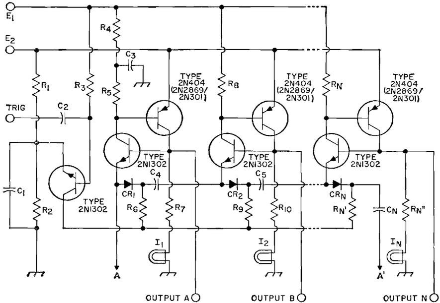
$C_1 = 100 \mu\text{f}$ , electrolytic, 6 v.
