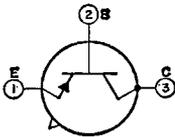
Germanium p-n-p type used in high-speed saturated switching applications in industrial data-processing equipment. JEDEC No. TO-18 package; outline 12, Outlines Section. This type is identical with type
