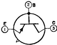
Germanium p-n-p type used in medium-speed switching applications in data-processing equipment. JEDEC No. TO-5 package; outline 6, Outlines Section. This type is identical with type 2N395 except for
