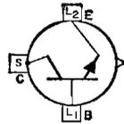
and relay control circuits; in oscillator, regulator, and pulse-amplifier circuits; and as a class A or class B push-pull audio and servo amplifier. It features low saturation resistance, high current and power dissipation, high beta at high current, and excellent high-temperature performance. This type is stud-mounted to provide positive heat-sink contact and has a cold-weld seal. JEDEC No. TO-36 package; outline 14, Outlines Section. This type is electrically identical with type 2N1487.
