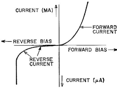
Figure 8. Voltage-current characteristic for a p-n junction.
