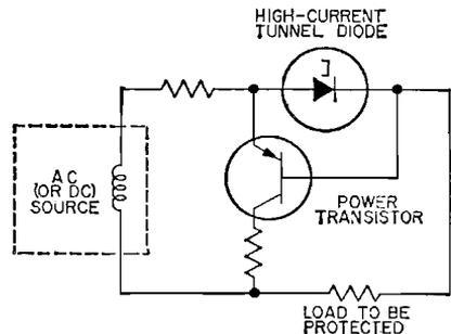
Figure 113. Overload sensor circuit using tunnel diode.
