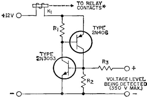
$K_1$  = dc relay; 12-volt, 71-ohm coil; Potter-Brumfield Type PR11DY, or equivalent.
