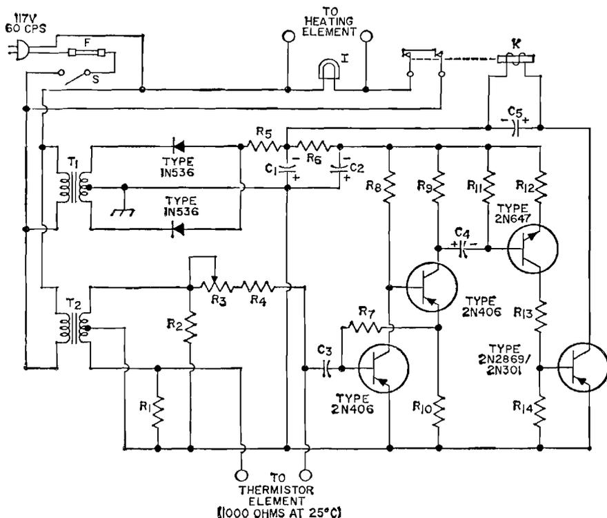
$C_1, C_3 = 1000 \mu\text{f}$ , electrolytic, 25 v.
