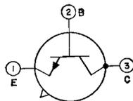
in af service for small- and large-signal driver and power applications. It features low saturation voltage, high sustaining voltage, high dissipation, high pulse beta, low output capacitance, and exceptionally low noise and leakage characteristics. JEDEC No. TO-5 package; outline 6, Outlines Section. For curves of transfer characteristics, refer to type 2N2102.
