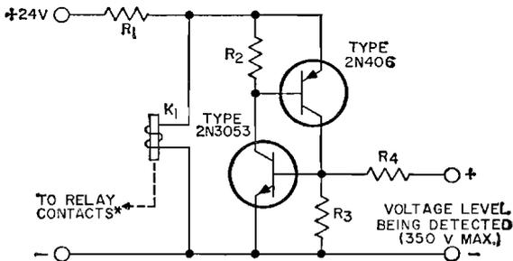
$K_1$  = dc relay; 12-volt, 71-ohm coil; Potter-Brumfield Type PR11DY, or equivalent.
