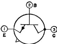
Silicon n-p-n type used in a wide variety of medium-power switching and amplifier applications in industrial and military equipment. It is used in power switching, dc-to-dc converter, inverter, chopper, sole-
