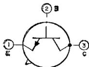
Silicon n-p-n type used in a wide variety of small-signal and medium-power applications in industrial equipment. This type features low noise and leakage characteristics, high pulse beta, high switching
