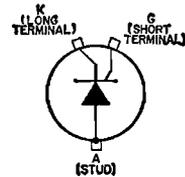
of 250 volts and a forward-current capability of 16 amperes (average value) or 25 amperes (rms value). This type is designed to meet stringent military environmental and mechanical specifications. The special high-strength copper-alloy stud can withstand an installing torque up to 50 inch-pounds. JEDEC No. TO-48 package; outline 19, Outlines Section. This type is identical with type 2N681 except for the following items:
