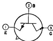
noid and relay control circuits; in oscillator, regulator, and pulse-amplifier circuits; and as a class A or class B push-pull audio and servo amplifier. It features low saturation resistance, high current and power dissipation, high beta at high current, and excellent high-temperature performance. JEDEC No. TO-5 package; outline 6, Outlines Section.
