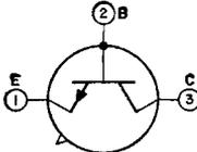
Germanium n-p-n type used in medium-speed switching applications in data-processing equipment. These transistors are n-p-n complements of the p-n-p types 2N404 and 2N404A. JEDEC No. TO-5 package;
