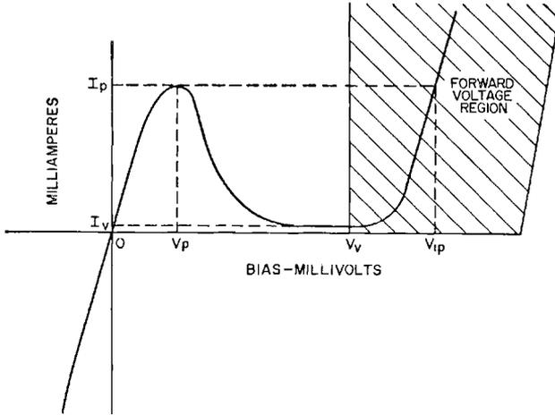
Figure 107. Typical current-voltage characteristic of a tunnel diode.
