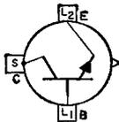
and relay control circuits; in oscillator, regulator, and pulse-amplifier circuits; and as a class A or class B push-pull audio and servo amplifier. It features low saturation resistance, high current and power dissipation, high beta at high current, and excellent high-temperature performance. This type is stud-mounted to provide positive heat-sink contact and has a cold-weld seal. JEDEC No. TO-36 package; outline 14, Outlines Section. This type is electrically identical with type 2N1490.
