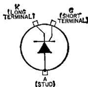
of 500 volts and a forward-current capability of 10 amperes (average value) or 16 amperes (rms value). This type is designed to meet stringent military environmental and mechanical specifications. The special high-strength copper-alloy stud can withstand an installing torque up to 50 inch-pounds. JEDEC No. TO-48 package; outline 19, Outlines Section. This type is identical with type 2N1842A except for the following items:
