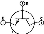
Germanium n-p-n type used in medium-speed switching applications in data-processing equipment. JEDEC No. TO-5 package; outline 6, Outlines Section.
