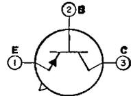
also function as an emitter. It is especially useful in bidirectional switching, core-driver, and ac-signal relay circuits. JEDEC No. TO-5 package; outline 6, Outlines Section.
