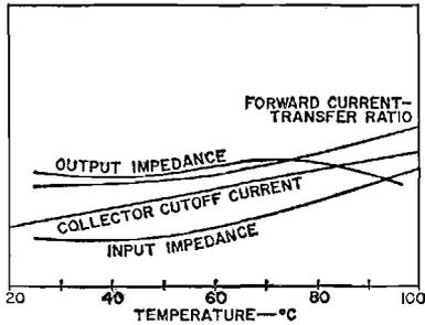
Figure 120. Variation of transistor characteristics with temperature.
