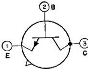
Silicon n-p-n type used in core-driving and line-driving applications requiring exceptionally fast switching speeds at high currents. JEDEC No. TO-5 package; outline 6, Outlines Section.
