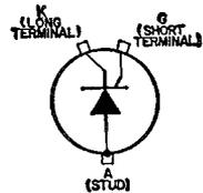
of 50 volts and a forward-current capability of 10 amperes (average value) or 16 amperes (rms value). This type is designed to meet stringent military environmental and mechanical specifications. The special high-strength copper-alloy stud can withstand an installing torque up to 50 inch-pounds. JEDEC No. TO-48 package; outline 19, Outlines Section. This type is identical with type 2N1842A except for the following items:
