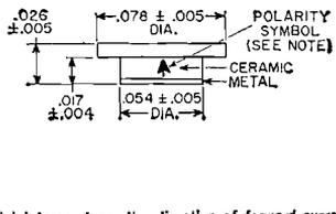
Note: Arrow shows the direction of forward current flow as indicated by dc ammeter.
