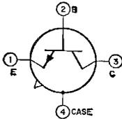
Silicon n-p-n type used in a wide variety of uhf applications in industrial and military equipment. It is used primarily in low-noise amplifier, oscillator, and converter circuits. When operated in the common-
