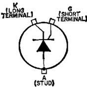
Diffused-junction n-p-n-p type used in a wide variety of power-control and power switching applications in industrial and military equipment. This type has a maximum peak forward blocking voltage
