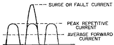
Figure 83. Representation of rectifier currents.
