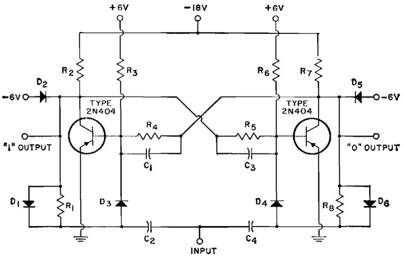
C<sub>1</sub> C<sub>3</sub> = 180 pF, mica, 24 v.
