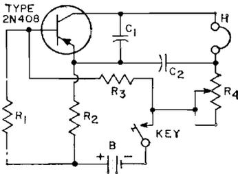
B - 1.5-4.5 v. (One to three series-connected RCA VS036 dry cells may be used, depending upon the volume level desired.)
