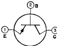
Germanium p-n-p type used in audio-frequency driver-amplifier applications in consumer and industrial equipment. This type features exceptionally high gain under typical operating conditions for driver
