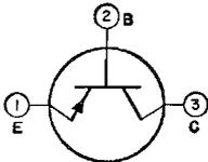
Germanium p-n-p low-noise type used in low-level preamplifier or input stages of audio-frequency amplifiers. JEDEC No. TO-1 package; outline 4, Outlines Section. This type is electrically identical with
