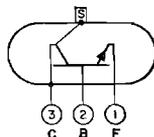
used in power-switching, dc-to-dc converter, inverter, chopper, and relay actuating circuits; in voltage- and current-regulator circuits; and in dc and servo amplifier circuits. This type has an offset pedestal, stud-mount arrangement which provides positive heat-sink contact. Outline 28, Outlines Section. This type is identical with type 2N1486 except for the following items:
