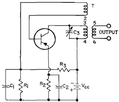
Figure 65. Tuned-collector oscillator.
