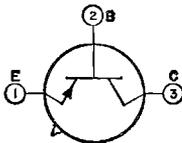
Germanium p-n-p types used for direct high-voltage control of "on-off" devices such as neon indicators, relays, incandescent-lamp indicators, and indicating counters of electronic computers. JEDEC No. TO-5
