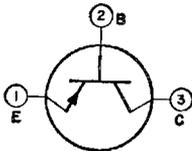
Germanium p-n-p type used primarily in converter and mixer-oscillator applications in AM battery-operated portable radio receivers and automobile radio receivers operating from either a 6-volt or a 12-volt supply. JEDEC No. TO-1 package; outline 4, Outlines Section. This type is electrically identical with type 2N140.
