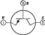
Germanium n-p-n type used in large-signal audio-frequency amplifier applications. It is designed especially for use with its p-n-p counterpart, RCA-2N217, in class B complementary-symmetry power-
