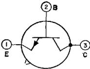
Silicon n-p-n type used in a wide variety of small-signal and medium-power switching applications in industrial and military equipment. It features high collector-to-emitter sustaining voltage, low leakage characteristics, high switching speeds, and a high dc forward current-transfer ratio.
