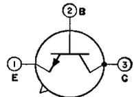
oscillator, voltage- and current-regulator circuits; and in dc and servo amplifier circuits. JEDEC No. TO-5 package; outline 6, Outlines Section.
