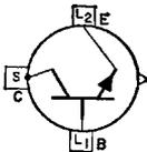
Silicon n-p-n type used in a wide variety of switching and amplifier applications in industrial equipment. It is used in power-switching, dc-to-dc converter, inverter, chopper, and relay-control circuits; in
