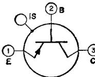
Germanium p-n-p type used in rf- and if-amplifier circuits; oscillator, mixer, and converter circuits; and low-level video-amplifier circuits in industrial and military equipment. It is used in the design
