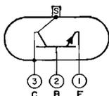
Silicon n-p-n type used in a wide variety of switching and amplifier applications in industrial equipment. It is used in power-switching, dc-to-dc converter, inverter, chopper, and relay-control circuits; in
