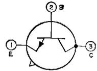
small-signal beta, very low capacitance, and large gain-bandwidth product. JEDEC No. TO-18 package; outline 12, Outlines Section.
