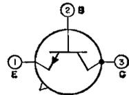
A amplifier circuits. This type features high output power, high collector-to-emitter voltage ratings, high gain-bandwidth product, high power gain, and high power dissipation. JEDEC No. TO-5 package; outline 6, Outlines Section.
