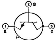
small-signal beta, very low capacitance, and large gain-bandwidth product. JEDEC No. TO-46 package; outline 18, Outlines Section. This type is electrically identical with type 2N2897.
