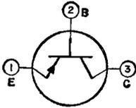
Germanium p-n-p type used in 262.5-kilocycle or 455-kilocycle intermediate-frequency amplifier applications in AM automobile radio receivers. In an unneutralized circuit, this type is capable of providing
