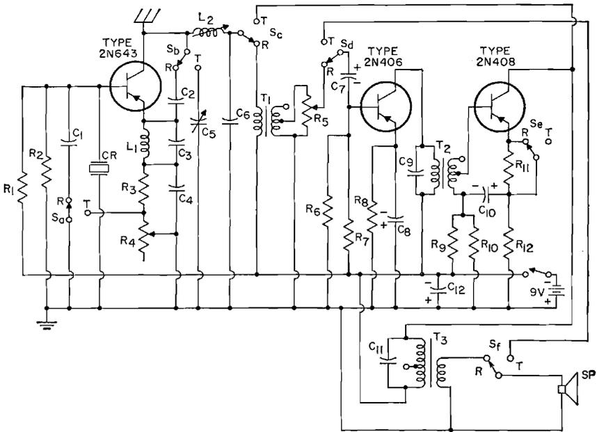
$C_1 C_8 C_9 = 0.001 \mu\text{f}$ , ceramic disc
