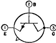
Silicon n-p-n type used in a wide variety of intermediate-power switching and amplifier applications in industrial and military equipment. It is used in power switching, dc-to-dc converter, inverter, chop-
