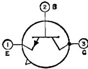
Silicon n-p-n type used in a wide variety of small-signal and high-speed switching applications. JEDEC No. TO-18 package; outline 12, Outlines Section.
