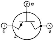
Silicon n-p-n type used in a wide variety of small-signal and low-to-medium power applications in military and industrial equipment. It features extremely low leakage characteristics, high pulse beta, high
