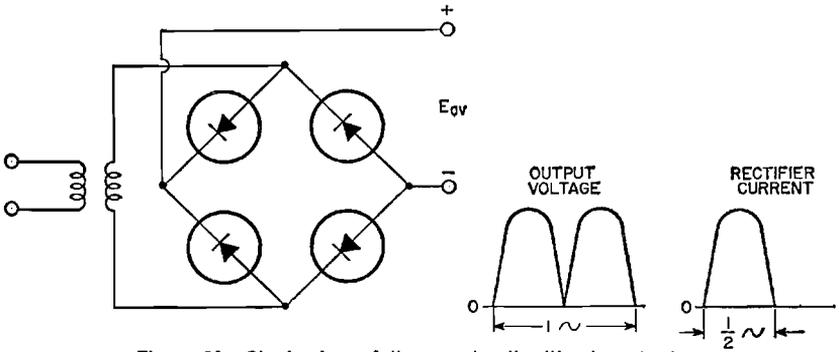
Figure 88. Single-phase full-wave circuit without center-tap.
