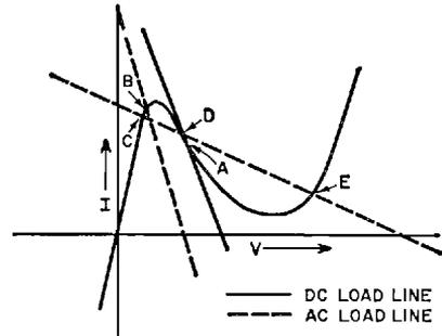
Figure 110. Typical load lines for tunnel-diode circuits.
