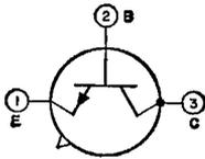
Silicon n-p-n type used in a wide variety of high-frequency and vhf applications in industrial and military equipment. It is used in large-signal power-amplifier, video-amplifier, oscillator, and mixer circuits over a wide temperature range. This type can also be used in switching service in circuits requiring transistors having high voltage, current, and dissipation values. JEDEC No. TO-39 package; outline 32, Outlines Section.
