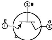
Germanium p-n-p type used in high-speed saturation switching applications in industrial data-processing equipment. JEDEC No. TO-18 package; outline 12, Outlines Section.
