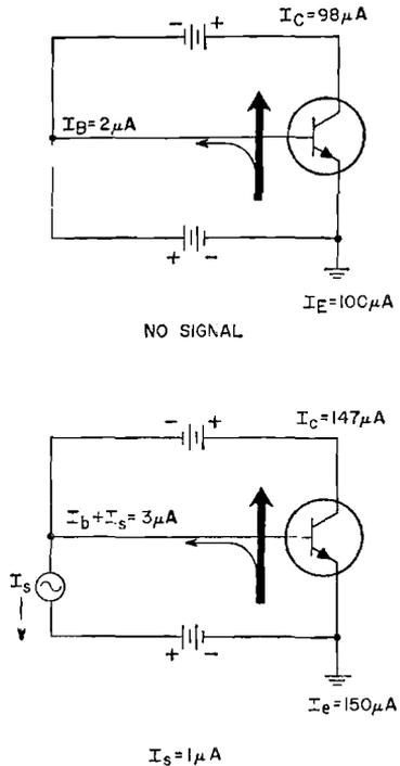
Figure 26. Electrode currents under no-signal and signal conditions.
