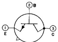
Silicon n-p-n type used in high-speed logic-switching and very-high-frequency amplifier applications. JEDEC No. TO-18 package; outline 12, Outlines Section.
