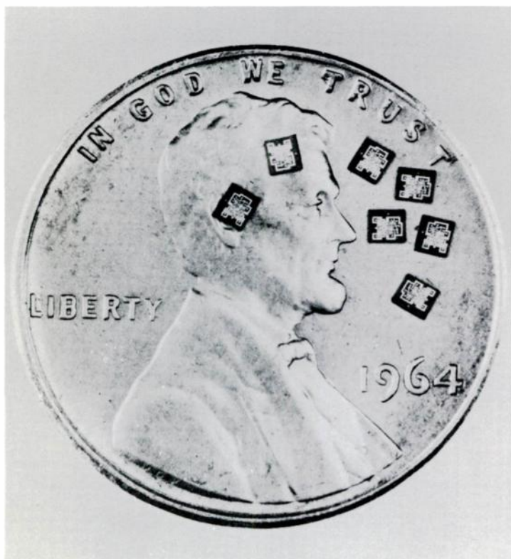
Fig. 1-7. Seven complete IC chips on a penny.
