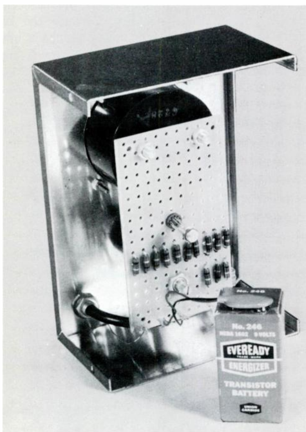
Fig. 8-2. Inside view of the electronic voltmeter.
