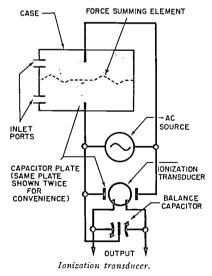
**ionization transducer** – A transducer in which displacement of the force-summing member is sensed by the induced changes in differential ion conductivity.
