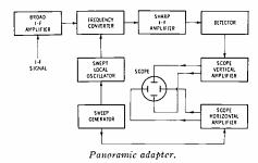
**panoramic** adapter – An attachment used with a search receiver to provide, on an oscilloscope screen, a visual presentation of the band of frequencies extending above and below the center frequency to which the search receiver is tuned.
