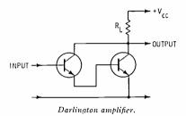
Darlington pair—See Darlington Amplifier. D'Arsonval current—A high-frequency, lowvoltage current of comparatively high amperage. **D'Arsonval galvanometer**—A dc galvanometer consisting of a narrow rectangular coil suspended between the poles of a permanent magnet.
