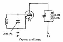
frequency of oscillation is controlled by a piezoelectric crystal.
