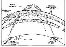
Refraction (of radio waves).
