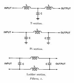
filter-1. A selective network of resistors, inductors, or capacitors which offers comparatively little opposition to certain frequencies or to direct current, while blocking or attenuating other frequencies. *See also* wave filter. 2. A device or program that separates data, signals, or materials in accordance with specified criteria. 3. Also called extractor or mask. A machine word that specifies which parts of another machine word are to be operated on.
