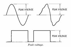
peak voltmeter—A voltmeter that reads peak values of an alternating voltage.
