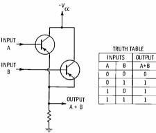
OR gate (using transistors).
