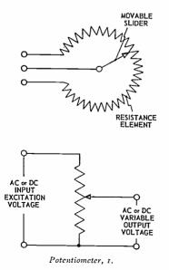
**potentiometer circuit**—A network arranged so that, when two or more electromotive forces (or potential differences) are present in as many branches, the response of a suitable detecting device in any branch can be made zero by adjusting the electrical constants of the network.
