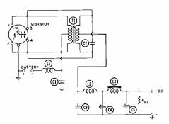
Synchronous-vibrator power supply.
