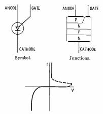
Anode characteristic. Complementary silicon controlled rectifier.
