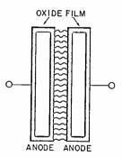
Nonpolarized electrolytic capacitor.
