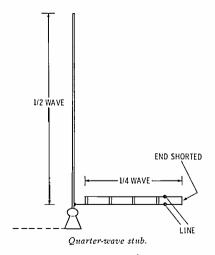
quarter-wave support -A quarter-wave metallic stub, used in place of dielectric insulators between the inner and outer conductors of a coaxial transmission line.
