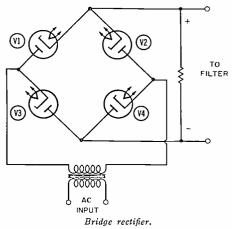
bridge circuit so that dc voltage is obtained from one pair of opposite junctions when an alternating voltage is applied to the other pair of junctions.
