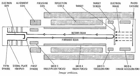
image and focuses it on one side of a separate storage target. The opposite side of the target is then scanned by low-velocity electrons to produce the output.
