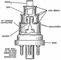
Cutaway view of lighthouse tube.
