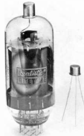
Transistors vs Tube (size comparison)
