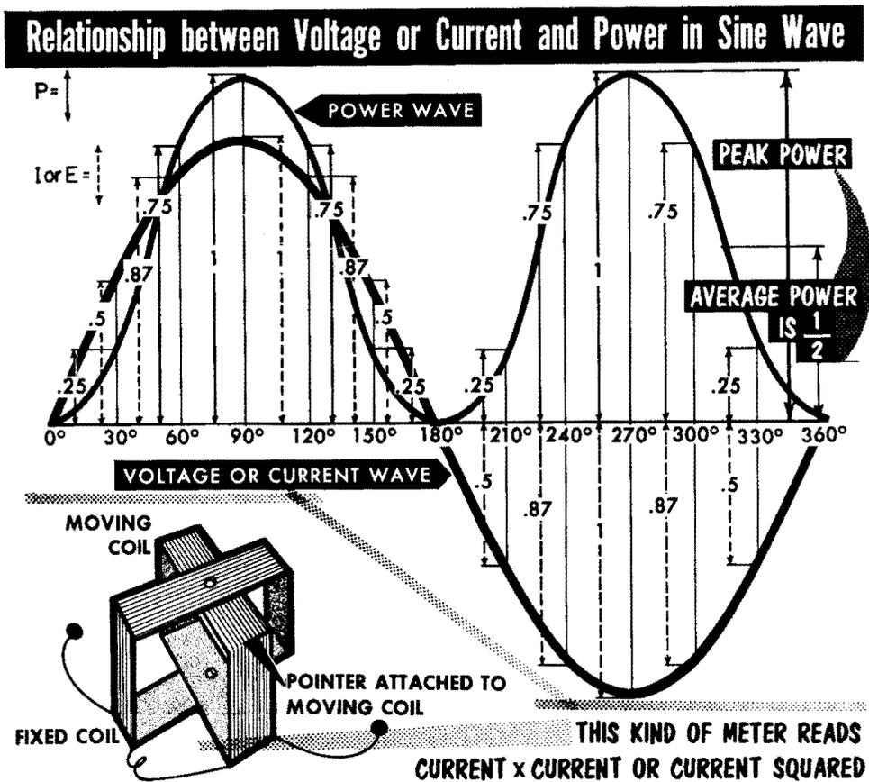
The power-equivalent reading of any a-c waveform could be read on a meter where both the field and the current in the moving coil come from the circuit being measured. This is called a *dynamometer* movement. Torque at every instant is proportional to power. So, the reading will be the average *power* represented by the current or voltage. If it is marked with square-root readings, or the steady current or voltage that would give the same reading, this meter will read true *rms* of any waveform.
