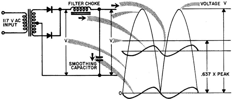
THE OUTPUT OF A CHOKE FILTER
