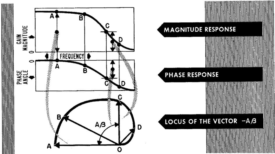
The loop gain  $A\beta$  is the important thing to consider. We can draw a series of lines from a starting point called O (for Origin). Each line represents both the magnitude and the phase angle of  $A\beta$  for a different frequency. Joining the outer ends of these lines produces a curve that represents all possible positions for the tip of the  $A\beta$  vector and shows how  $A\beta$  varies in phase and magnitude due to frequency changes. This curve is called a Nyquist diagram.
