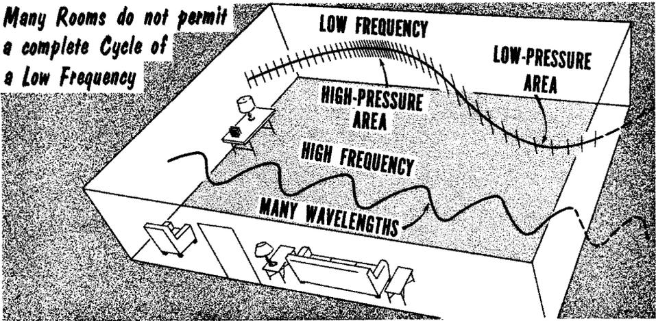
As a result of the tremendous differences in wavelength, the low frequencies may not even have one complete wave in an average-sized room at the same instant, whereas a high-frequency sound will have many complete waves in the room traveling in a number of directions at the same time.
