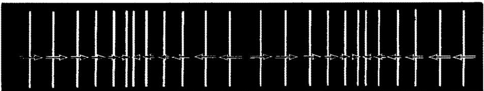
At low frequencies (long wavelengths), large volumes of air are compressed and expanded, requiring large air movement.
