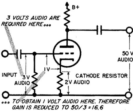
**THE CATHODE RESISTOR PROVIDES NEGATIVE FEEDBACK**
