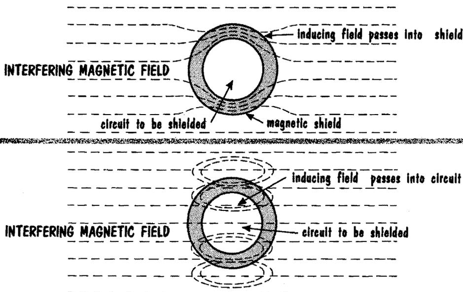
AT HIGHER FREQUENCIES, FIELD CHANGES TOO FAST FOR SHIELD TO WORK. SHIELD PRODUCES DELAYED REACTIONARY FIELD, WHICH DOES NOT ELIMINATE INDUCTION ANY MORE.
