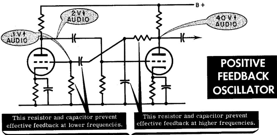
These four components control oscillation frequency because there is maximum transfer at a given frequency.
