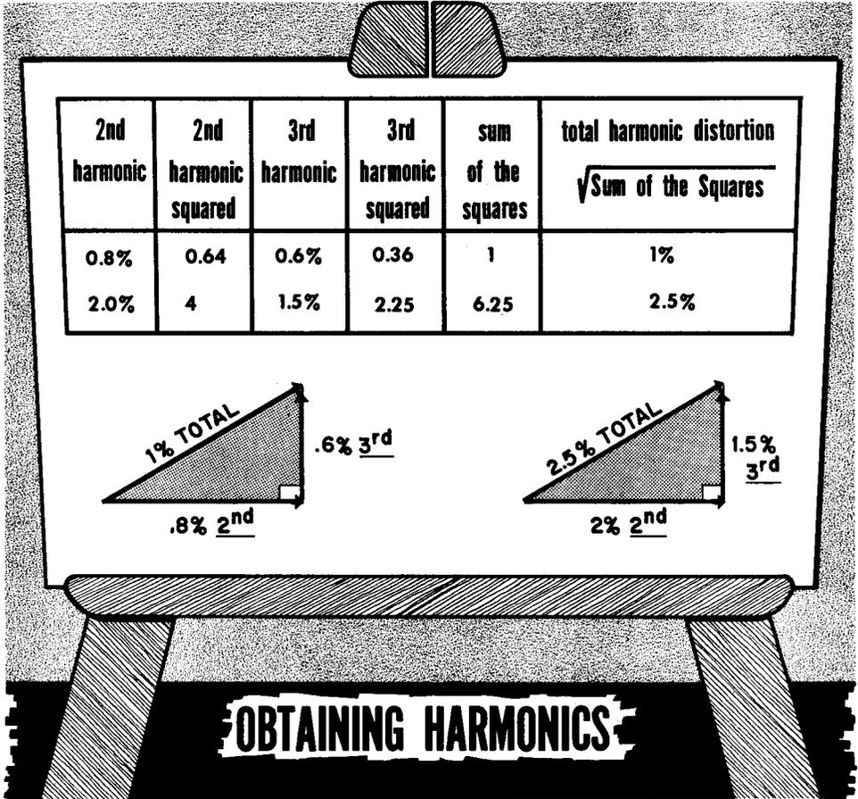
It is important that, to obtain the total harmonic distortion, one must obtain the square root of the sum of squares of the individual harmonics. The method of combining harmonics is the same regardless of which components are combined. The different components could be second and fifth or any other combination, or a combination of more than just two individual components.
