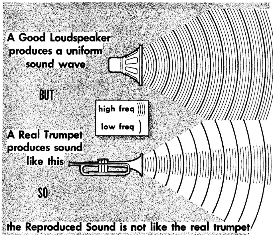
For example, a trumpet gives out sound that is very rich in overtones. The lower (fundamental) notes of the trumpet go out in all directions, whereas the high-frequency sound is almost squirted in the direction in which the trumpet is pointed. This kind of sound production and the way in which the sound bounces around before reaching our ears have become part of our experience in listening to trumpets.
