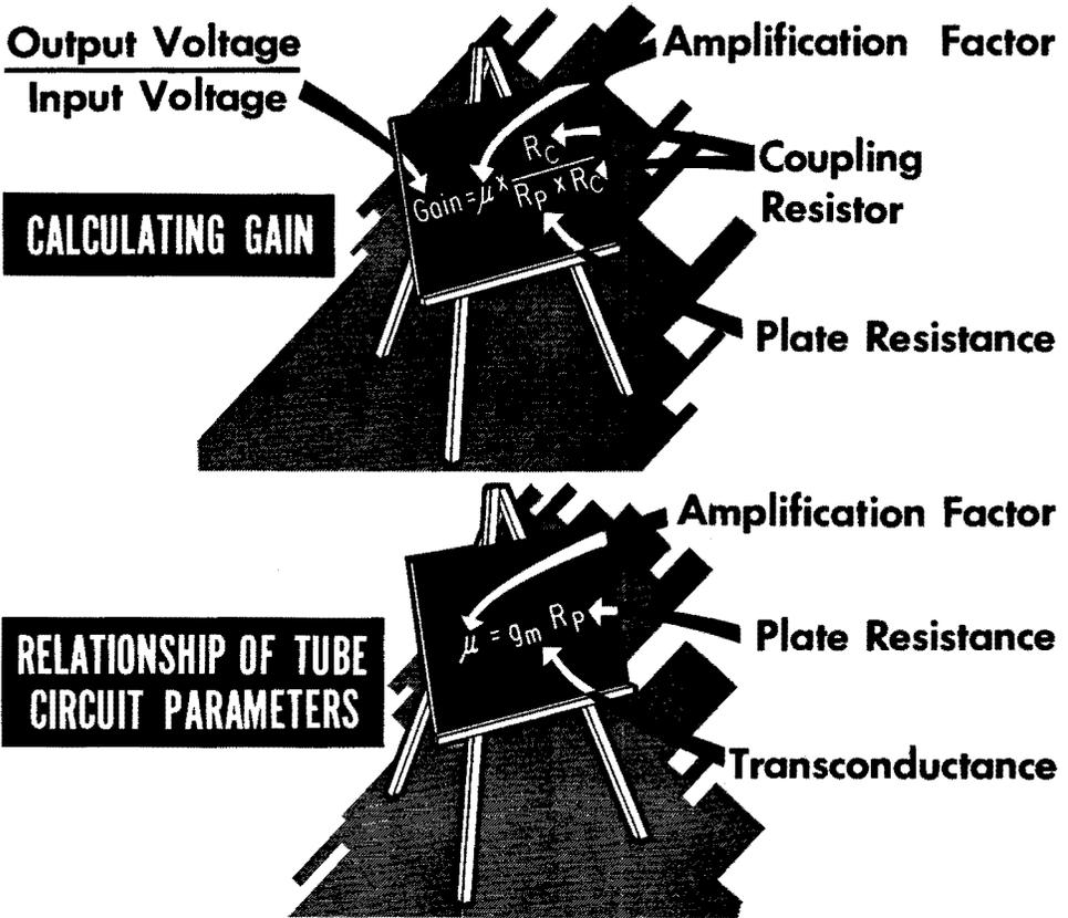
If there is no coupling resistor present (this was the case when we first examined the circuit), the voltage remains constant, and the current fluctuates. The plate current fluctuation for each volt of grid fluctuation is the transconductance of the tube. The relationship between these two conditions (which have no practical use, but help no end in figuring out the operation of practical tube circuits) is determined only by the parameter that we have called plate resistance.
