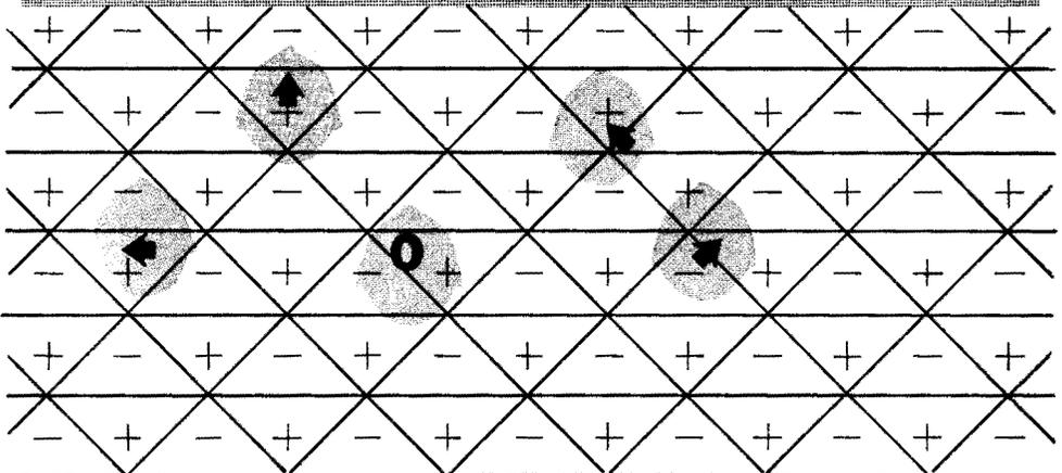
The arrows indicate the direction from which sound seems to come; the circle shows a position at which all sense of direction is lost.
