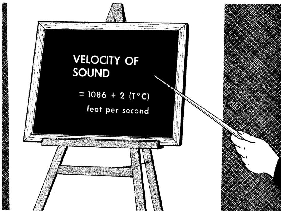
At  $20^{\circ}$  C (normal room temperature), sound travels at  $1086 + (2 \times 20) = 1126$  feet per second.
