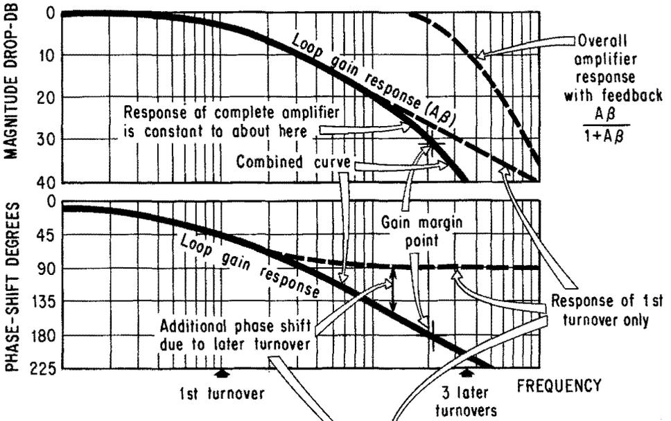
**CURVES OF  $A\beta$  TO SHOW HOW LARGE AMOUNTS OF FEEDBACK ARE OBTAINED WITH SEVERAL STAGES**
