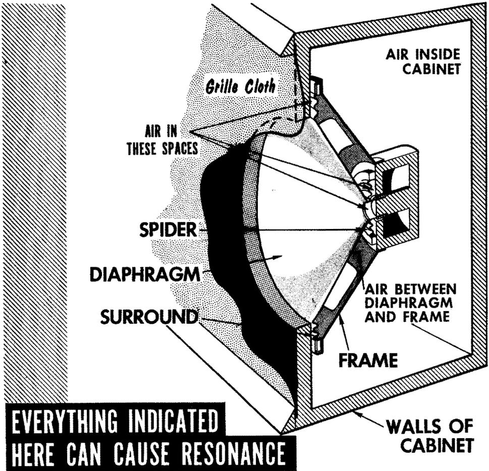
In loudspeaker design, every effort is made to minimize resonance effects, but there are still plenty left. The best that can be done in a good design is to spread the resonances so they all have as little effect as possible. Some manufacturers, from time to time, make the claim of having produced the perfect loudspeaker, with no "tone" of its own. So far, none of these claims has been true, and future claimants should be checked very carefully.
