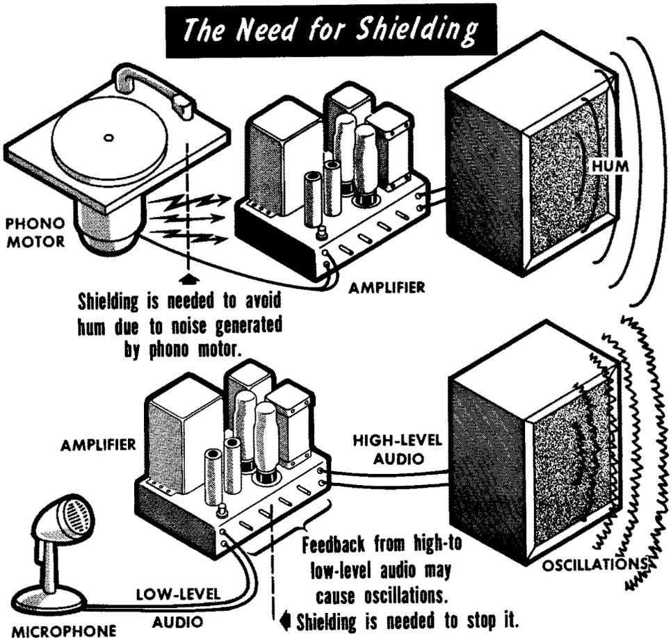
All kinds of power components and circuits radiate at power frequencies (mostly 60 and 120 cycles). If this radiation is induced into a low-level audio circuit, hum will result. The second kind of induction is that of high-level circuit, if the two are in close proximity to each other. (This interference is known as *crosstalk*.) If the *same* audio at high level is induced in low-level circuit, it is the same as undesired feedback, which can cause instability or oscillation.
