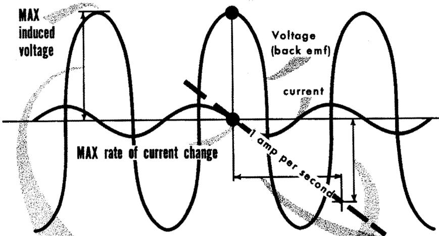
When the current changes at 1 amp per second, the Voltage Induced is a measure of the Inductance in henries
