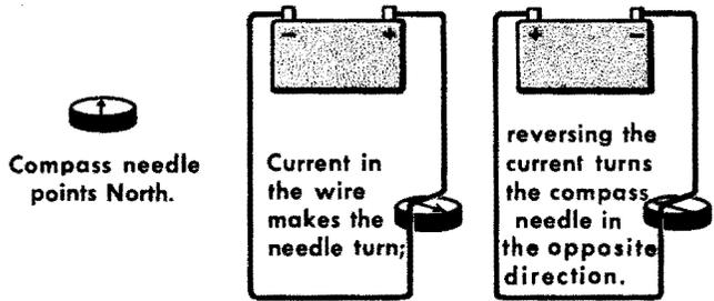
If you suspend a magnet or a compass needle over a wire connected to a battery, the needle will swing to one side. If you reverse the current in the wire, the magnet (or needle) will swing in the opposite direction.
