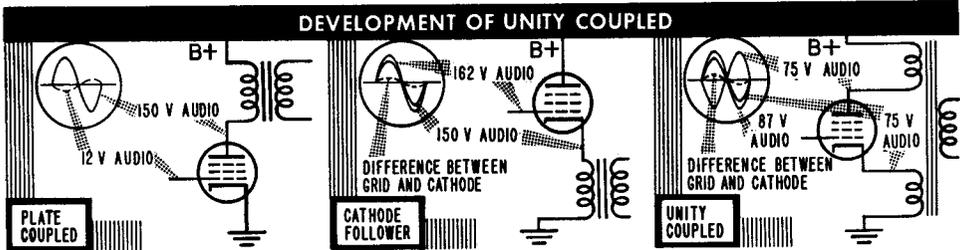
Until feedback came along, the choice for output tubes was between triodes and pentodes. Pentode operation is much more efficient in terms of audio power output for the power input, but it is far more critical of being operated with exactly the right load resistance value than when the same tubes are triode connected.
