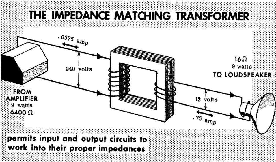
Suppose 9 watts are to be transferred. The formula for power is  $W = EI$ , where  $W$  is power in watts,  $E$  is voltage in volts, and  $I$  is current in amperes. (Remember that the relation between voltage and current in a resistance is  $E = IR$ , where  $R$  is the resistance in ohms.)
