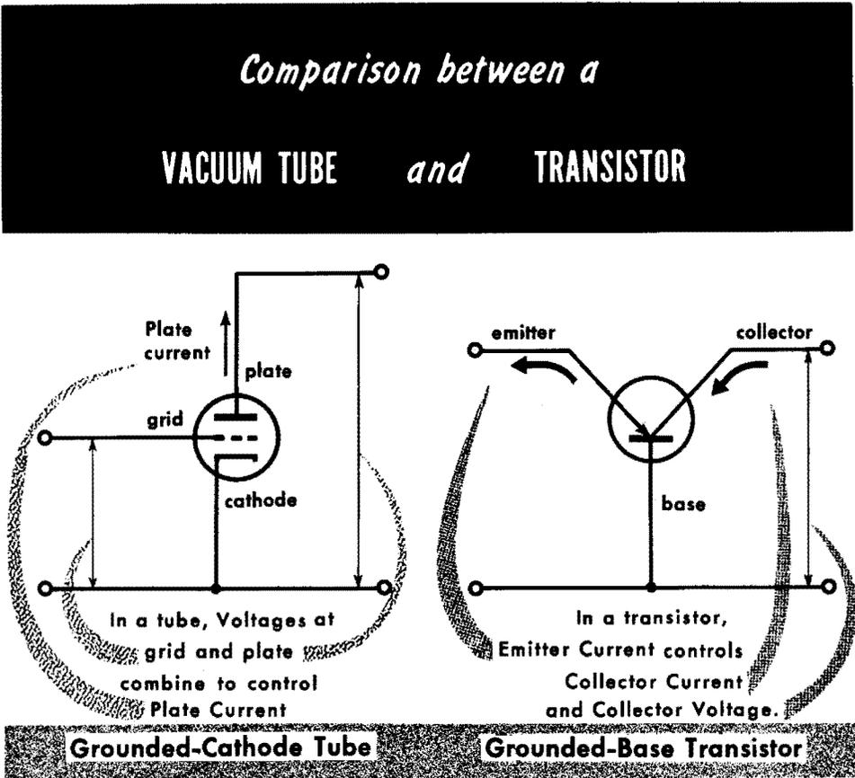
To understand what all this means, we need to know something about a transistor. It is essentially a piece of special alloy, using germanium or silicon as a base, with very small amounts (a few parts in a million, very accurately controlled) of an "impurity" added. Two electrodes are connected to this carefully blended base. They may be point contact "whiskers" or a "grown junction," formed by a process called electrolytic deposition.
