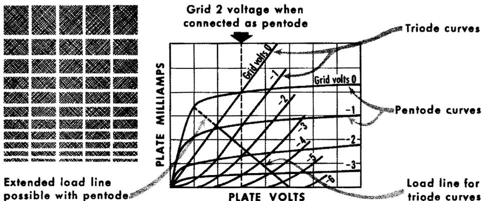
Using the best possible load resistance with triode-connected tubes, the voltage fluctuation between  $B+$  and plate reaches little more than half the  $B+$  supply voltage. Changing the method of connection to pentode alters the curve so that the zero grid-voltage curve is pushed out into a "knee." This extends, very considerably, both the voltage and current fluctuation available in the plate circuit. This, in turn, triples or quadruples the power that any pair of tubes will give.
