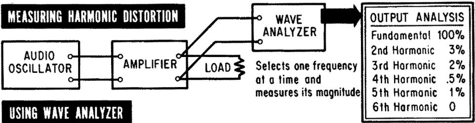
The use of the wave analyzer is rather a long-winded method, so a simple distortion measuring set is usually used to give the answer quite quickly. This method uses another kind of frequency-selective filter to eliminate the fundamental. Two positions are provided on the switch: one for measuring the amount of fundamental and the other for measuring the total amount of audio after the fundamental has been removed. This gives a quick and ready means of measuring the total distortion.
