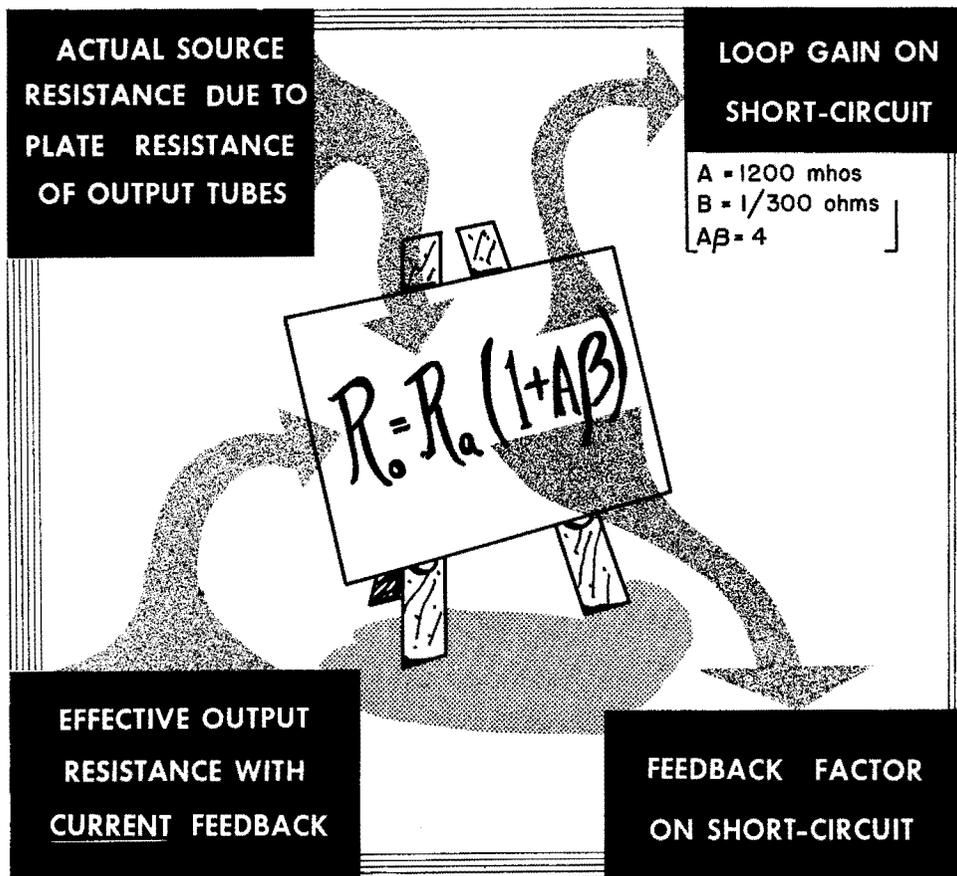
At normal loaded condition, the reduction in gain due to feedback is 2. (Without feedback, 2 millivolts produces the same output as 4 millivolts does with feedback.) Disconnecting the load entirely results in no feedback. Thus, for *current* feedback, the *effective* output source resistance is the actual source resistance multiplied by the feedback factor when the amplifier output is short-circuited.
