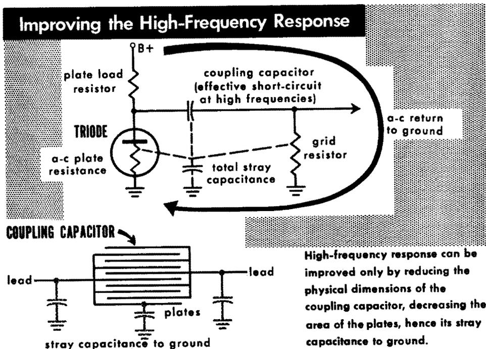
For high-frequency signals, the coupling capacitor is effectively a short circuit—no audio voltages appear across it, and both sides of the capacitor are at the same audio voltage at any instant. This means that we now have three effective resistance paths to ground from the plate of the tube: through the plate resistance of the tube, through the coupling resistor, and through the following stage's grid resistor.
