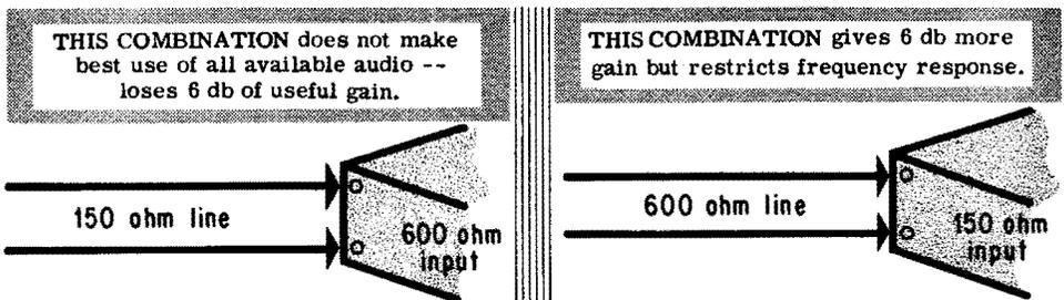
There is nothing particularly magical about one particular line impedance. The use of any middle-value impedance (150, 250, 500, or 600 ohms) merely minimizes the defects of either high or low impedances. It is, of course, good to use a consistent impedance in any particular system. Using a 150-ohm impedance and connecting it to a transformer designed for a 600-ohm impedance at the amplifier (or vice versa) will not make the best use of the available audio.
