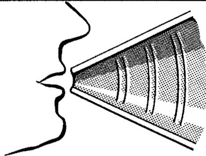
Using a *horn* is a way to improve this situation. The method by which a horn improves acoustic efficiency can be illustrated by two devices: a speaking tube and a megaphone. In a speaking tube, sound is propagated without the wave being allowed to expand. For this reason, the intensity does not fall off according to the inverse-square law, but reaches the other end of the tube almost undiminished.
