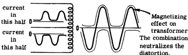
When audio signal is fed into output stage, current in one primary rises, while current in the other falls. On next half-wave, opposite primary currents rise and fall.
