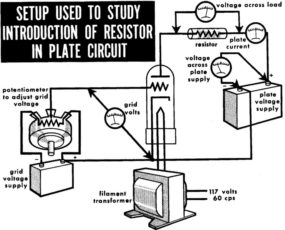
We can make the fluctuating plate current produce a voltage fluctuation by passing it through a resistor. The higher the value of the resistor, the greater the voltage drop that a given current will cause, and hence the greater the *voltage fluctuation* a given *current fluctuation* will produce.
