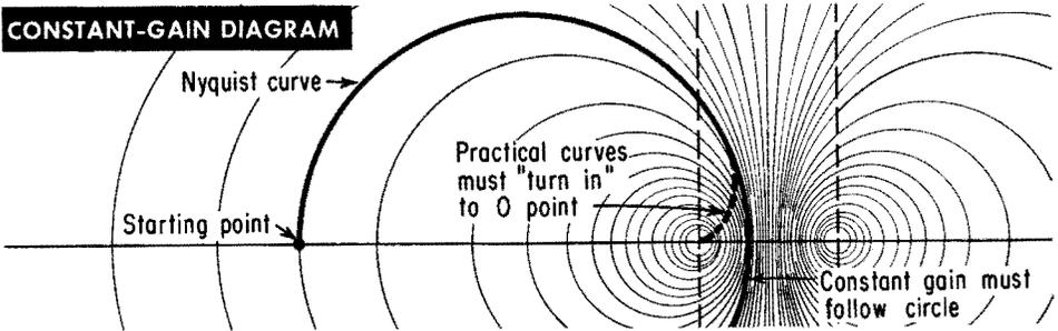
The locus vector curve itself is called a *Nyquist diagram*. If the curve representing the locus of  $A\beta$  follows one of the circles which represents a constant ratio of distances from  $O$  and  $1$ , the gain of the amplifier with feedback would be *constant*, although there would be *phase change* in both  $A\beta$  and  $(1 + A\beta)$ , as well as a transition from positive to negative value of  $A\beta$ .
