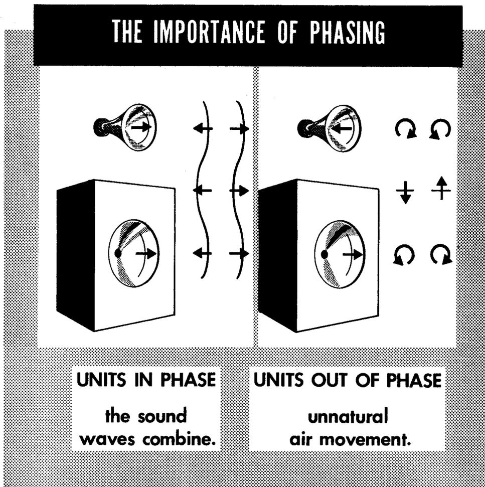
When the units work correctly (in phase), the combined sound wave builds up into the same kind as would be produced by one big loudspeaker unit. When they are out of phase, however, the motion of the air particles is cross-ways. This makes quite an unnatural kind of sound, and the realism of the reproduction is destroyed. For this reason care should be taken to connect the units so that they are in phase.
