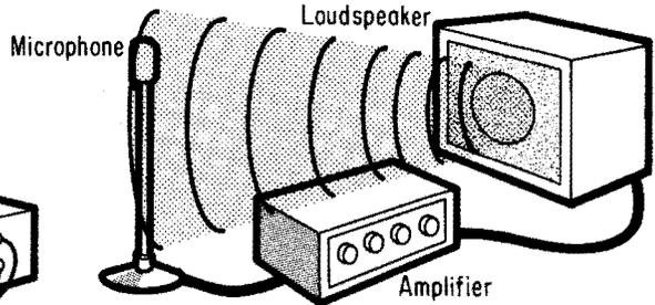
THE FEEDBACK CAN BE BY MEANS OF SOUND WAVES FROM A LOUDSPEAKER CONNECTED TO THE OUTPUT TO A MICROPHONE CONNECTED TO THE INPUT.
