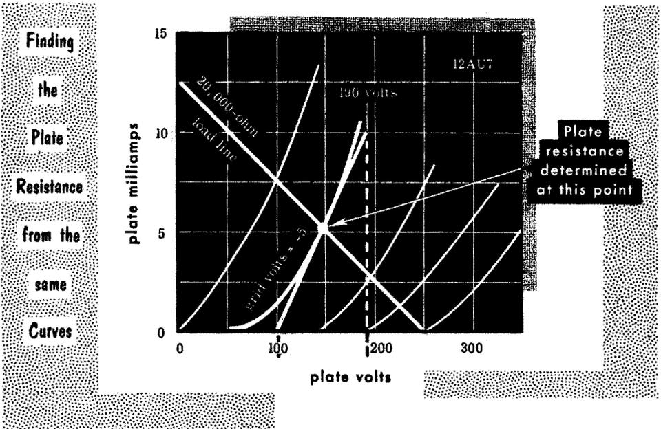
By laying a straight-edge (ruler) along the curve at the point where the two lines cross, its slope *at this particular point* can be found. Extending the line drawn as tangent to the curve down to the zero current line and up to the 10-milliampere line, the corresponding voltages may be read off and the plate resistance calculated.
