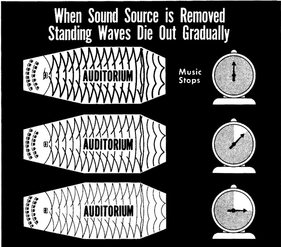
This dying away occurs in a fraction of a second in an ordinary living room. Most of us are so used to the brief presence of these patterns that we do not normally notice it. In a large hall or auditorium, however, or in a stadium with walls all around it, the time required for sound to die away can be quite noticeable.
