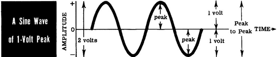
A pure frequency has a waveform called a *sine wave*, and is called a *sinusoidal wave*. If the wave fluctuates between  $+1$  volt and  $-1$  volt from 0 as the starting point, the total change, called the *peak-to-peak* voltage, is 2 volts. The “swing” each way from the central starting point is called the *peak* voltage, in this case 1 volt.
