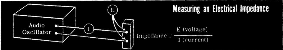
In a microphone, the voltage source is internal or *inside* the component, so that we cannot measure it separately. But we can measure the open-circuit voltage and then measure current when we short-circuit the microphone, so that there is no voltage. The relationship between this voltage and current is the impedance of the microphone.
