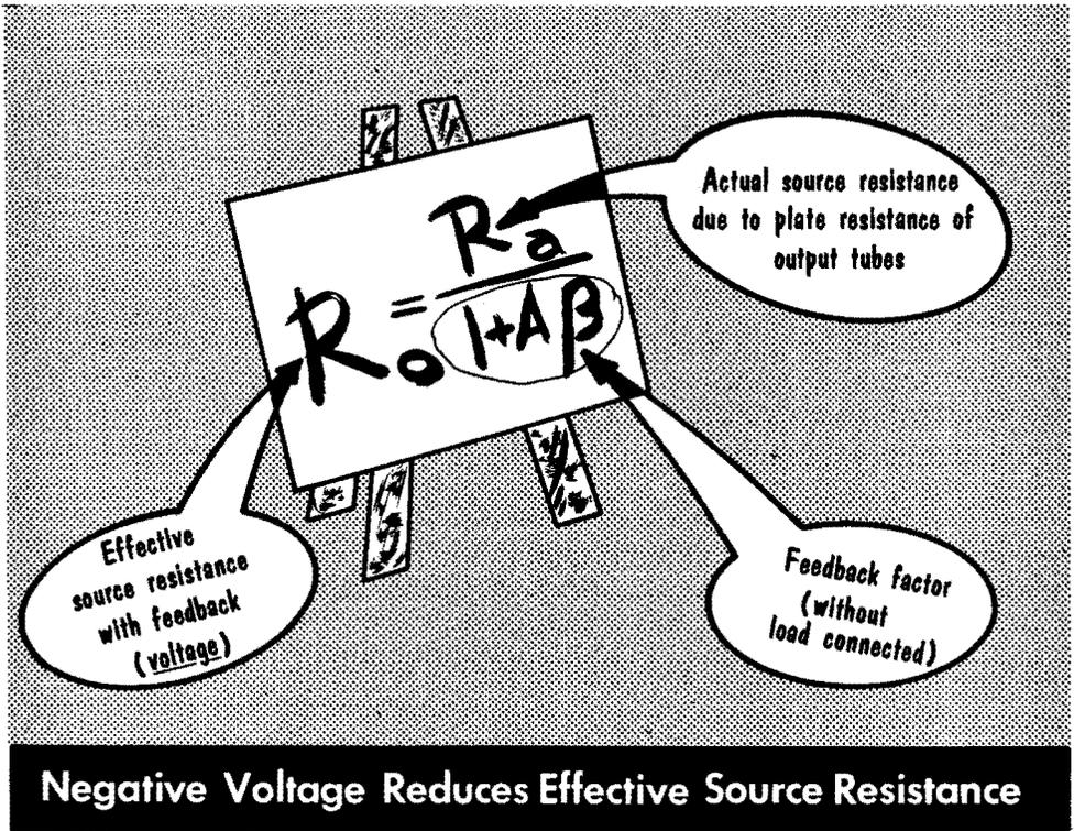
We could use the formula instead of the numbers and come out with the same answer — that the internal resistance with voltage feedback is divided by the same factor that the gain is reduced by. An important point to notice (not stated in many textbooks on the subject) is that we must use the gain *without the load connected* in this formula.
