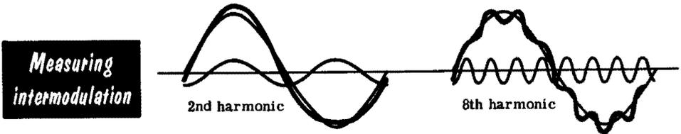
Both harmonics are same magnitude, but the higher numbered one has much bigger effect on the shape of the combined waveform.
