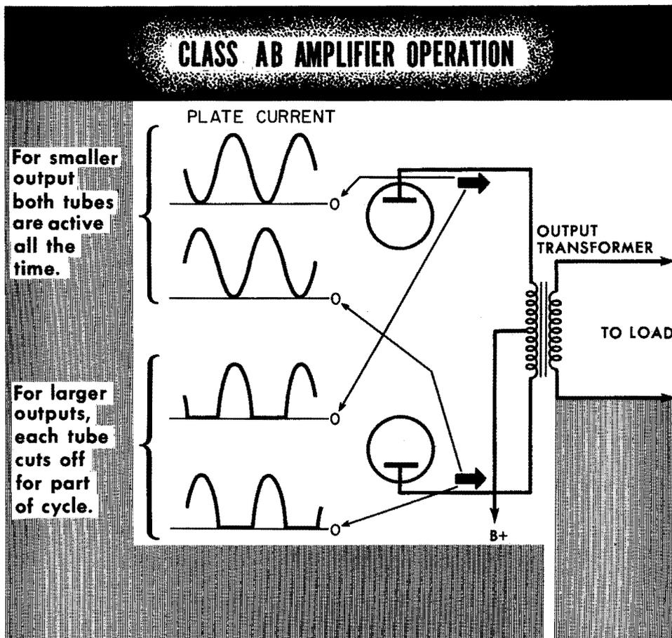
For this reason a popular method (called class-AB) consists of splitting the difference. For small outputs, up to about half maximum power, both tubes are conducting current all of the time. When full output is needed, each tube goes beyond the zero plate current for part of the cycle, but for not a complete half-waveform. This design results in an amplifier that is less critical in operation and can be used without critical selection of output tubes and adjustment of bias.
