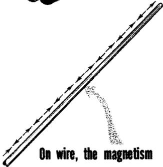
On wire, the magnetism is in alternate directions along the wire.
