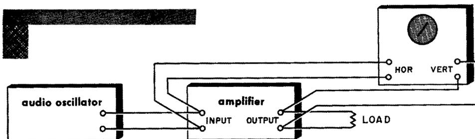
SCOPE TRACE IS A STRAIGHT SLOPING LINE IF OUTPUT IS ALWAYS A PROPORTIONATELY AMPLIFIED VERSION OF THE INPUT
