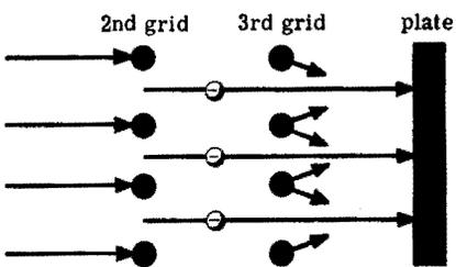
With third grid at same voltage as cathode, secondary electrons are always sent back to plate.
