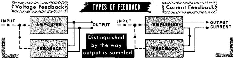
There are several ways in which feedback may be distinguished. For example, either the output *voltage* or the output *current* can be used as a basis for the output “sampling.” The chief difference as far as the operation of the amplifier is concerned is in the effect on the amplifier’s effective output impedance.
