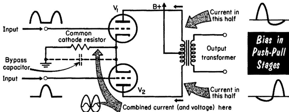
Self bias using a resistor in the cathode circuit is found in push-pull stages as well as in "single-ended" stages. When the push-pull stage is operated class AB, the plate currents in the tubes change appreciably during different parts of the waveform. These currents are added in the common cathode resistor, not subtracted as in the output transformer primary. This results in a double-frequency current in the cathode resistor, because of the asymmetrical current waveforms in the tubes.
