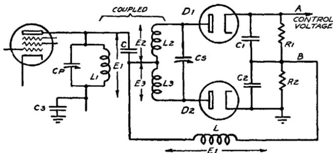
Fig. 27. The basic discriminator circuit. Note that the transformer has a center-tapped secondary  $L_2$  and  $L_3$  instead of the two tuned circuits heretofore discussed
