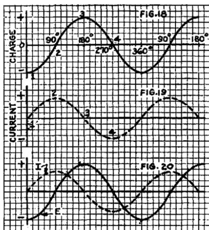
The charge on C in Fig. 17 follows the sine-wave variation of the voltage, see Fig. 18: the positive and negative peaks of charge occur at the same instant as the voltage peaks. The current in Fig. 17 follows a sine-wave variation, but its zero values occur when the charge goes through its peak values as shown Fig. 19. In Fig. 20 both voltage and current waves are plotted on the same axis, showing that the current I leads the voltage E by one-quarter cycle, or  $90^\circ$
