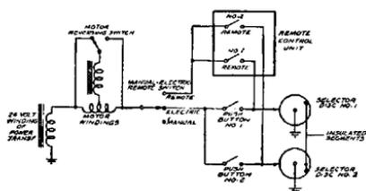
provide remote control operation. A separate remote control box, which contains a set of push buttons identically similar to those mounted on the receiver, is connected to the receiver through a cable of appropriate length.
