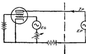
Fig. 62. If  $E_g$  lags  $E_p$  by  $90^\circ$ , then the tube circuit to the left of the dotted line appears to the a-c generator  $E_p$  as a variable inductance
