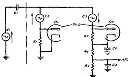
As to the signal voltages active in the circuit, the voltage which is effective in causing rectified current to flow through R1 is  $E1 + E2$  and the voltage which is effective in causing rectified current to flow through R2 is  $E1 + E3$ .
