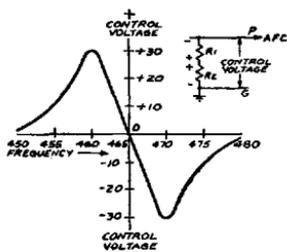
Fig. 26. This S-shaped curve represents the combined voltage across R1 and R2 and is obtained by combining for each frequency the separate voltages across R1 and R2, Fig. 25. Note that at 465 kc the control voltage is zero, due to the cancelling of the voltages across R1 and R2 shown in the inset, Fig. 26B
