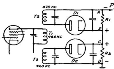
Fig. 23. This discriminator circuit has two staggered tuned circuits, one peaked above and one below the i-f peak by the same amount. The diode circuits are arranged so that the rectified voltages across R1 and R2 oppose each other
