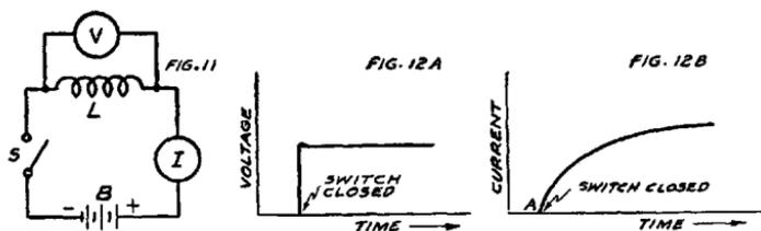
Fig. 11. The ammeter  $I$  indicates the current flowing in the series circuit, consisting of a coil, battery, and switch, while the voltmeter  $V$  shows the voltage across the coil  $L$ . When the switch  $S$  is closed, the voltage rises at once to its maximum value, Fig. 12A, but the current rises slowly to its maximum value, Fig. 12B, and thus lags behind the voltage
