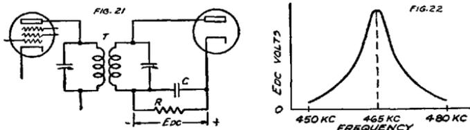
Figs. 21, 22. In the simple tuned rectifier circuit of Fig. 21, the d-c voltage  $E_{dc}$  developed across the diode load  $R$  is greatest at the resonant frequency of the tuned circuit, in this case 465 kc. The curve of Fig. 22 shows how  $E_{dc}$  falls off on both sides of the resonant frequency
