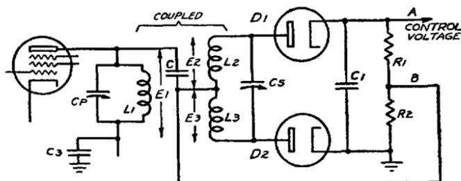
Fig. 45. This form of discriminator circuit is similar in operation to that shown in Fig. 31. The omission of the by-pass condenser at the junction of R1 and R2 makes it possible to eliminate an i-f choke for coupling the voltage E1 into the diode circuit
