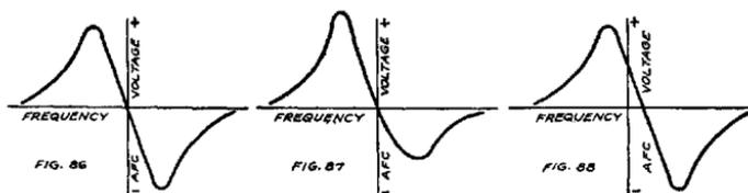
Figs. 86, 87, and 88. In Fig. 86 is shown the discriminator output characteristic when the circuit is correctly aligned. When the primary trimmer is misaligned, the characteristic of Fig. 87 results and when the secondary trimmer is misaligned that of Fig. 88 is produced. Note that misalignment of the primary results in a change of shape in the curve whereas an incorrect adjustment of the secondary trimmer results in zero control voltage being produced at a frequency different from the i-f peak
