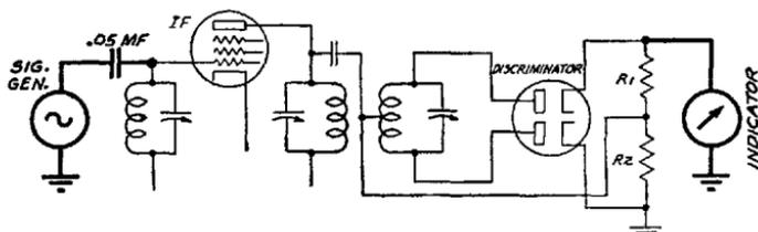
Fig. 89. The signal generator and the output indicator connections used during AFC alignment are shown in heavy lines
