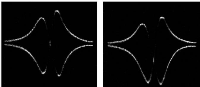
Figs. 92 and 93. The oscillogram of Fig. 92, left, is the type of pattern obtained when the discriminator trimmers are correctly adjusted. The effect of an incorrect adjustment of the secondary trimmer is shown in Fig. 93
