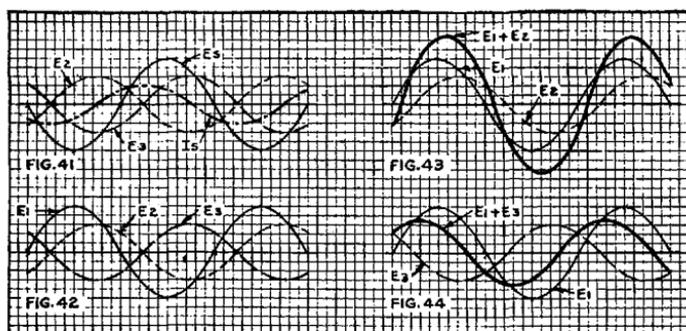
Figs. 41 to 44. The phase relations existing in the discriminator circuit of Fig. 31 for the case where the input signal is lower than the resonant frequency of the secondary tuned circuit, i.e., lower than the i-f peak
