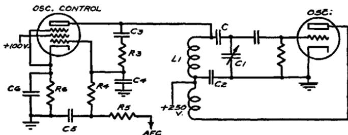
Fig. 65. A basic oscillator control tube circuit, showing how it is connected to the oscillator circuit.  $R_3$  and  $C_4$  supply the lagging grid voltage, while  $C_3$  keeps the d-c voltage from the grid of the control tube
