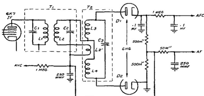
Fig. 54. The triple-tuned discriminator circuit that is used in several Sears-Robuck receivers. This is a modification of the basic discriminator circuit and it should be noted that the three windings are enclosed in two separate shields, as indicated by the dotted lines
