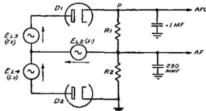
noted by reference to the breakdown diagram shown in Fig. 55. This is a simplified version of Fig. 54, and the various voltages involved in Fig. 54 are identified. Once again you see that the voltage across the secondary tuned circuit L2-L2'-C2,
