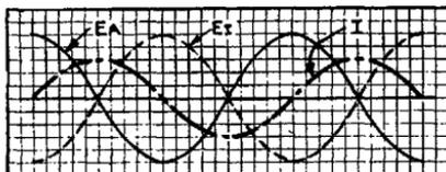
in the case of the d-c circuit, the current does not reach its final peak value until after the applied voltage, and in fact, lags one quarter cycle or  $90^\circ$  behind the applied voltage. Thus the current  $I$  is shown as lagging  $90^\circ$  behind  $E_a$  in Fig. 13.
