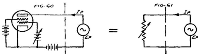
Fig. 60. By varying the grid bias, the tube circuit to the left of the dotted line can be made to appear to the a-c generator  $E_p$  as a variable resistance. Fig. 61 shows the tube circuit represented as a variable resistance
