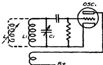
in order to show how the control tube is tied in with a conventional oscillator circuit. In general, the basic arrangement shown in Fig. 65 is generally used, although there are some slight modifications in the different receivers, which represent the individual ideas of various set designers. While the resemblance between Figs. 65 and 63 is not great at first glance,
