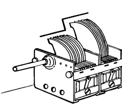
① Ganged capacitors with sections of differing sizes
