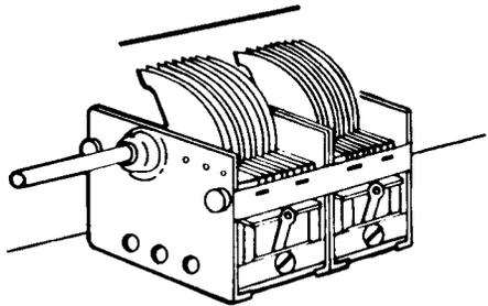
② Ganged capacitors with identical sections
