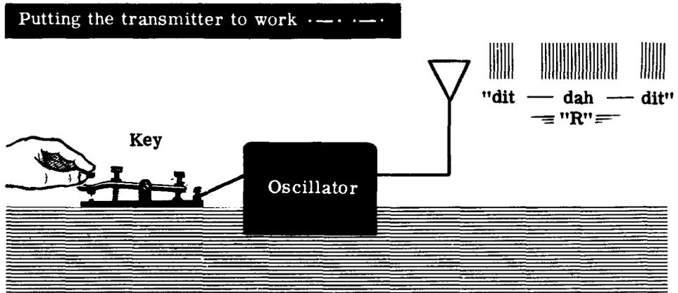
A signal of this type contains intelligence since a message can be obtained from it. The radio would produce a sound somewhat like "dit-dah-dit" which a radio operator understands as the letter "R."
