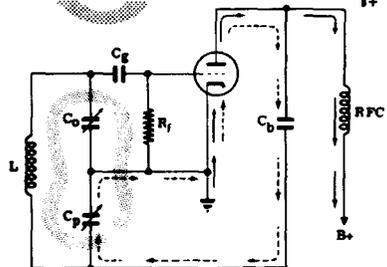
**TPTG OSCILLATOR**—uses the grid-plate capacitance of a triode to feed back pulses to a tuned circuit connected to the grid. It oscillates only when the two tuned circuits are set to or near the same frequency.
