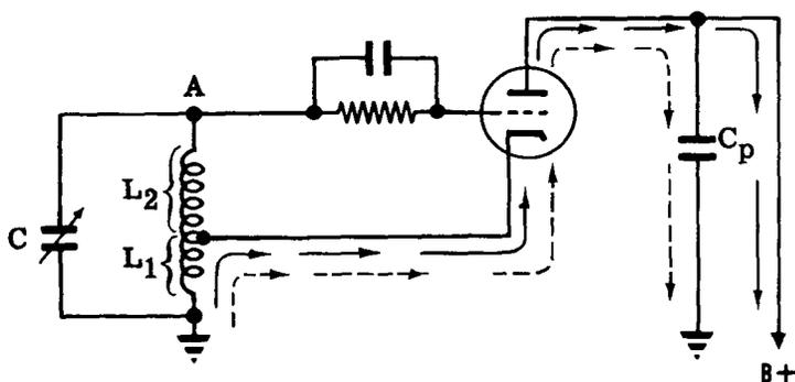
... Showing DC current path and RF feedback path
