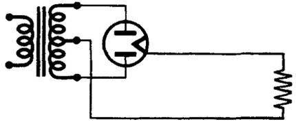
FULL-WAVE RECTIFIER TUBE - A vacuum tube consisting of two specially designed diodes and a common cathode in the same glass envelope. Both direct and indirectly heated cathodes are used depending on the requirements of the rectifier circuit.
