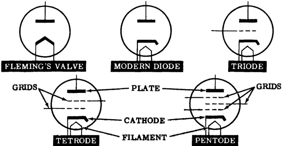
Tubes have developed in a logical sequence. . .
