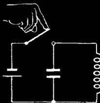
Extra voltage being applied to LC circuit.
