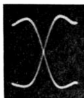
FIG. 6-5. A typical discriminator characteristic such as is obtained when the visual method of alignment is used.
