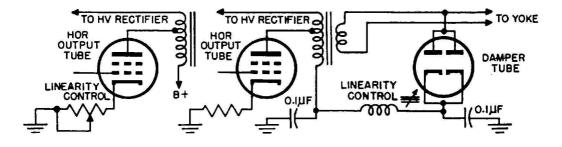
Fig. 6-8. Typical linearity control circuits.
