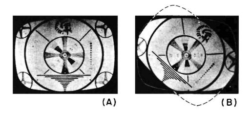
Fig. 4-1. (A) Test pattern properly aligned with mask. (B) Test pattern tilted, due to misalignment of deflection yoke.
