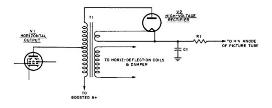
Fig. 2-9. Typical high-voltage power supply circuit.
