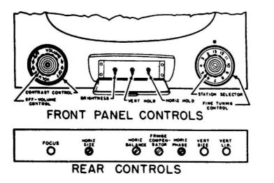
Fig. 1-8. Typical control location diagram. Courtesy: Emerson
