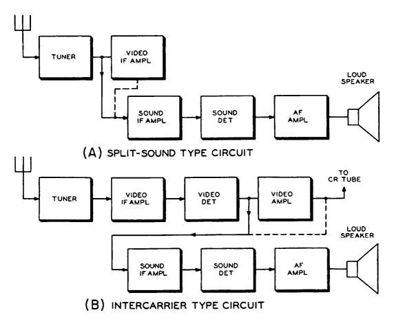
Fig. 10-1. Complete sound signal paths for (A) split-sound type and (B) intercarrier type TV receivers.
