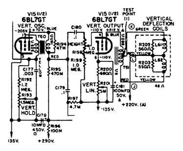
Fig. 6-11. One circuit arrangement for controlling height of the picture. Courtesy: Sylvania
