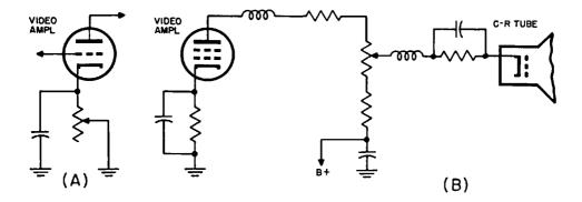
Fig. 6-2. Two commonly-used methods of contrast control. (A) By variation of cathode resistance, and (B) by a plate circuit potentiometer connection.
