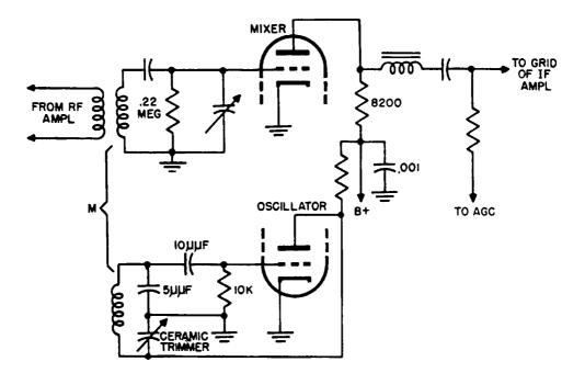
Fig. 2-3. Typical dual-triode mixer-oscillator circuit.
