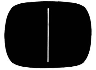
Fig. 9-4. Pattern when there is no horizontal sweep but with high voltage still present.
