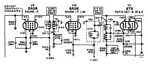
Fig. 1-7. Portion of a TV schematic, showing how the pin numbers of the tubes are indicated on the symbols of the tubes. Courtesy: Sylvania
