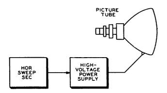
Fig. 9-1. If screen is dark and low voltage is normal (sound reception is satisfactory), the trouble area reduces to that shown by this block diagram.
