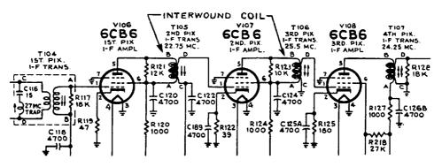
Fig. 1-3. How interwound, or bifilar, windings of a transformer are indicated on a schematic diagram.
