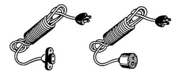
Fig. 3-2. Two types of linecord interlock jumpers required for TV troubleshooting.
