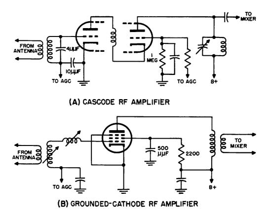
Fig. 2-4. Typical r-f amplifiers used in TV receivers.
