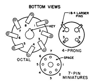
Fig. 1-6. Some of the commonly used types of tube sockets, showing the physical arrrangement of the contacts and connecting lugs from a bottom view, and showing how these contacts are numbered for reference to the schematic diagram.
