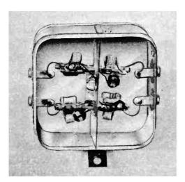
Fig. 9-18. Typical high-pass filter for connection in the antenna lead of a TV receiver to reduce certain kinds of interference.
