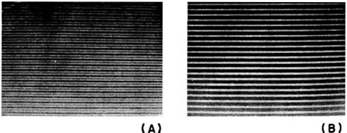
Fig. 9-12. Close examination of the horizontal sweep lines of a TV picture indicates whether there is poor interlace. (A) shows how lines pair when there is partial loss of interlace, while (B) shows how the lines merge when the loss of interlace is complete.
