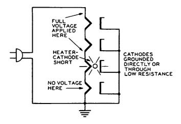
Fig. 8-3. How a heatercathode short circuit can cause some heaters to glow overbrightly and others to be dead. Fig. 8-3. When such is the case, the tubes which have been overloaded should be checked by replacement, to determine whether the overload has caused them damage.
