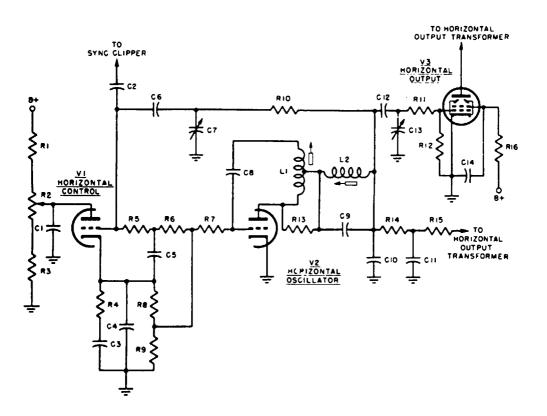
Fig. 2-8. Typical pulse-width horizontal AFC circuit.
