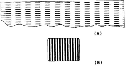
Fig. 5-2. How vertical bars are formed by a video signal considerably higher than the horizontal deflection frequency.
