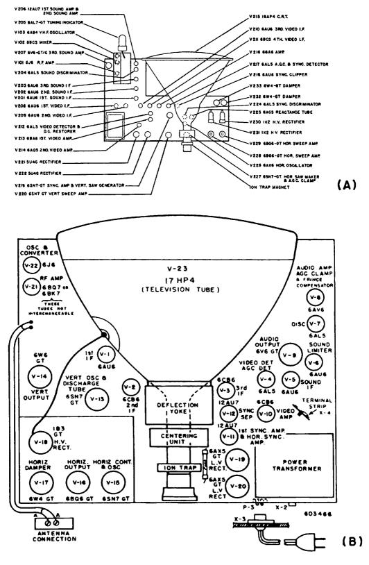
Fig. 7-1. Typical tube layout diagrams.
