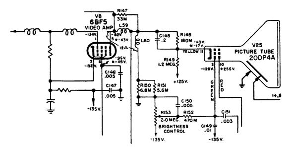
Fig. 6-3, Typical coupling circuit between video amplifier and picture tube, showing location of brightness control.
