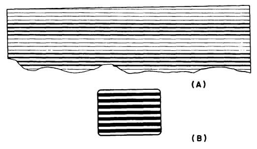
Fig. 5-3. How horizontal bars are formed by a video frequency appreciably lower than the horizontal deflection frequency.
