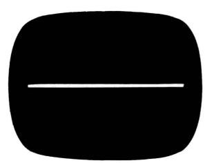
Fig. 9-2. Type of pattern indicating no vertical sweep.
