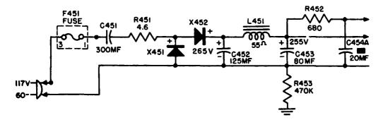
Fig. 2-12. Typical transformerless power supply.
