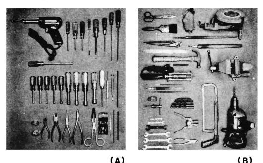
Fig. 3-1. Assortment of hand (A) and bench (B) tools used in TV servicing work. Courtesy: Electrical Merchondising
