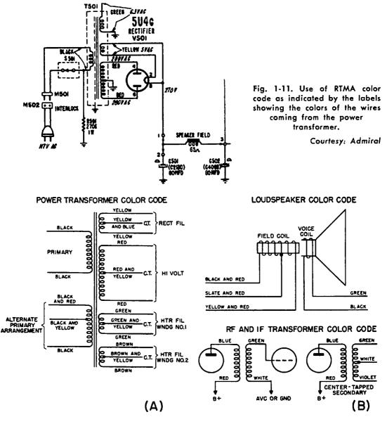
Fig. 1-12. RTMA color codes for wiring of power transformers, i-f transformers, and loudspeakers.
