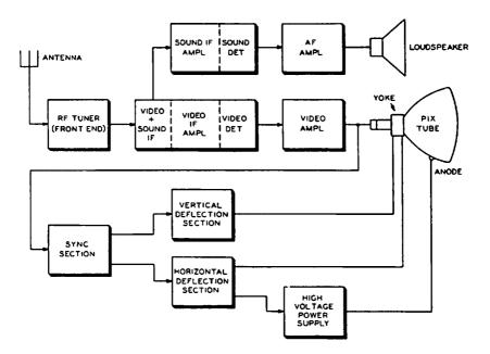
Fig. 2-1. Block diagram of split-sound TV receiver, showing division into sections appropriate for troubleshooting indications.
