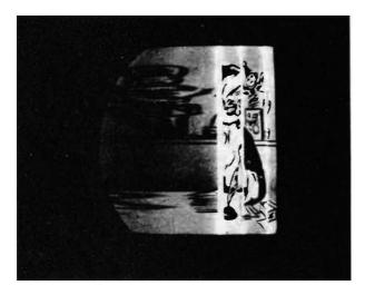
Fig. 9-13. Typical case of picture fold-over resulting from transients in the horizontal sweep section.
