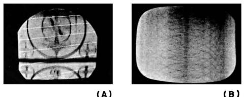
(A) Fig. 9-10. Examples of loss of vertical sync.
