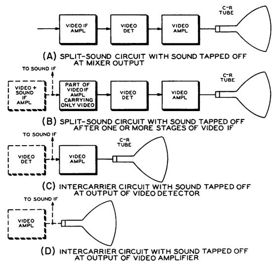
Fig. 9-6. Possible trouble areas for different circuit arrangements when the symptom is raster and sound but no picture.
