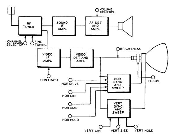
Fig. 6-1. Various controls of a TV receiver and the related sections of the receiver.
