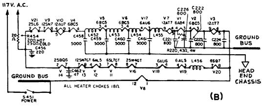
Fig. 8-1. Examples of series-heater circuits used in transformerless TV receivers.
