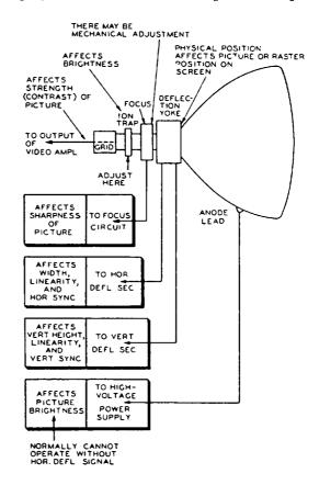
Fig. 2-6. Block diagram showing the source of each indication on the picturetube screen. both the sound and the picture paths, and can affect either or both. If the tap-off point is *before* the video amplifier, then trouble in the video amplifier will affect only the picture.
