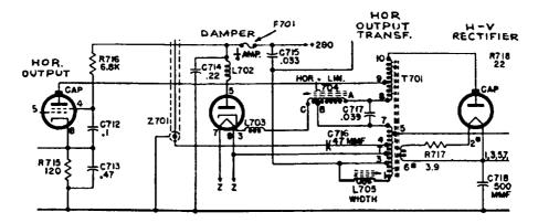
Fig. 6-10. Typical width control circuit.
