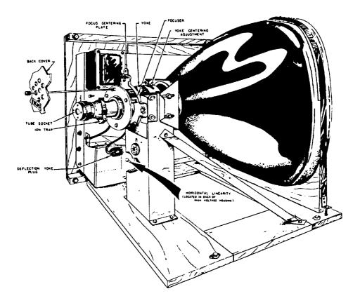
Fig. 6-5. Typical focus adjustment assembly on neck of picture tube.
