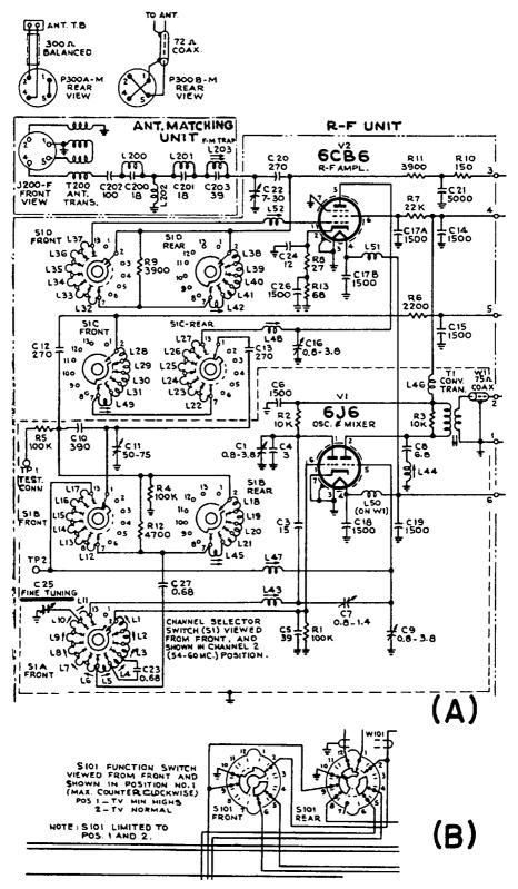
Fig. 1-10. How wafer-type switches and their connections are shown on service schematic diagrams.
