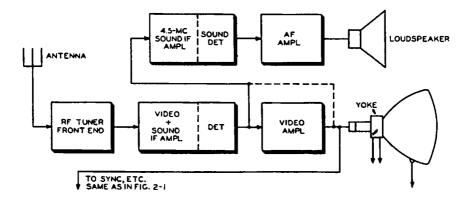
Fig. 2-2. Block diagram of intercarrier type of receiver, with division into troubleshooting sections.
