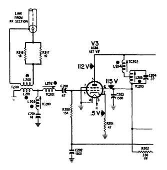
Fig. 1-1. Section of a typical service-type schematic diagram showing particularly how capacitance and resistance values are indicated, and how labels indicate the voltages at strategic points.
