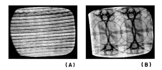
Fig. 9-9. Types of patterns which result from failure of the horizontal sweep to synchronize.
