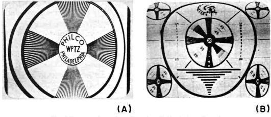
Fig. 6-7. (A) Horizontal nonlinearity. (B) Vertical nonlinearity. (A) Courtesy: Philco (B) Courtesy: G.E.
