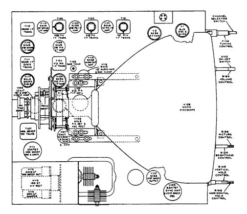
Fig. 1-5. Typical tube location diagram, as provided with the service data for many TV receivers. Note that this diagram includes additional information on the locations of the front controls, adjustments on the yoke, focus, and ion trap magnet.
