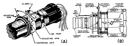
Fig. 6-13. Yoke and other adjustments on the neck of the picture tube. (A) Courtesy: Emerson (B) Courtesy: RCA
