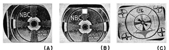
Fig. 6-12. (A) Improper centering, picture to right. (B) Improper centering, picture low. (C) Picture tilted. (A) (B) Courtesy: RCA (C) Courtesy: G.E.
