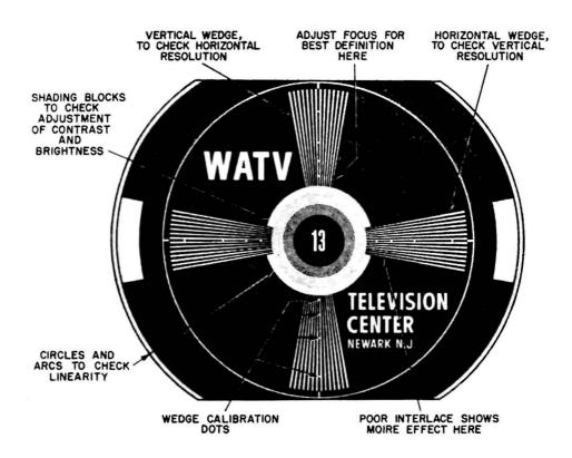
Fig. 5-1. Typical test pattern and the information which it presents.
