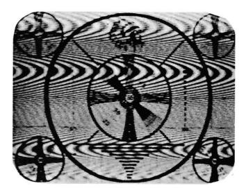
Fig. 9-17. Another type of interference arising from r-f interference.
