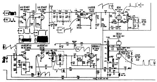
Fig. 1-13. How the waveforms of the voltages at various test points in a receiver circuit are sometimes placed right on a schematic diagram for convenience in oscilloscope testing. Courtesy: Admiral
