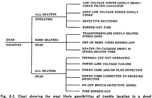
Fig. 8-2. Chart showing the most likely possibilities of trouble location in a dead receiver, and how they may be separated according to whether the heaters are operating.
