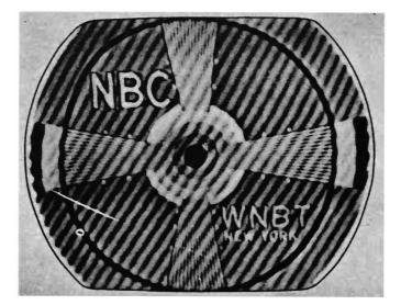
Fig. 9-16. Typical r-f interference pattern. Courtesy: RCA
