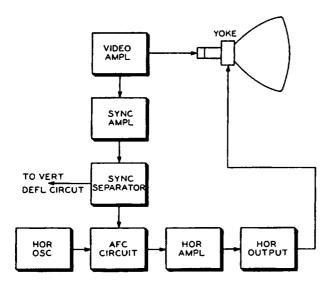
Fig. 2-7. Block diagram showing the horizontal sync section and how it is related to other parts of the circuit.
