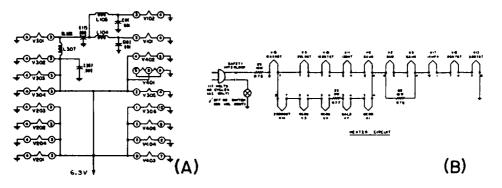
Fig. 1-14. Typical heater circuit diagrams for TV receivers.
