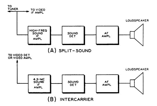
Fig. 10-2. Shows resulting limited sound signal paths after sections which share sound and picture signals have been removed. These are appropriate trouble areas for cases in which the picture is good but the sound reception is not satisfactory.
