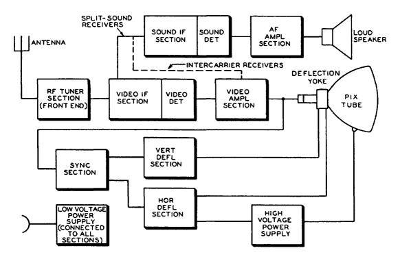
Fig. 2-10. The difference between the division points between the sound and video i-f signals for split-sound and intercarrier type receivers.
