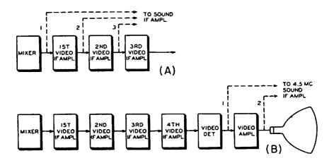
Fig. 2-5. Points at which the sound i-f signal is tapped off in the two main types of receivers: (A) split-sound, and (B) intercarrier. In a given receiver, the tap-off point may be any one of those shown in dotted lines. Where this juncture is found in a serviced receiver is important in determining the source of trouble.
