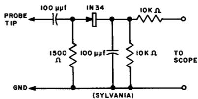
RELATIVELY LOW-IMPEDANCE TYPE; MODERATE SENSITIVITY. SERIES RECTIFIER. SCOPE CABLE ISOLATED.
