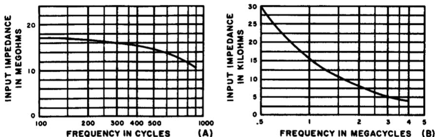
Fig. 5-17. How the input impedance of a typical low-capacitance probe decreases as the frequency increases through the audio-frequency and radio-frequency ranges up to video frequency (4 mc).
