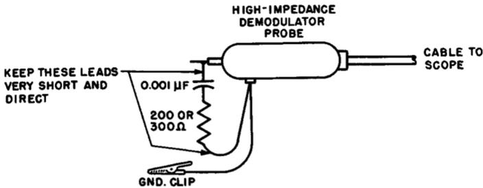
Fig. 7-13. A low-impedance demodulator probe is often required for proper i-f stage-by-stage alignment or signal tracing. In the absence of this type of probe, the technician may make use of a conventional high-impedance general-purpose demodulator probe, in combination with a 200-ohm damping or swamping resistor and blocking capacitor connected across it, to shunt down and flatten the response of the tuned plate-circuit load to which the scope is applied.
