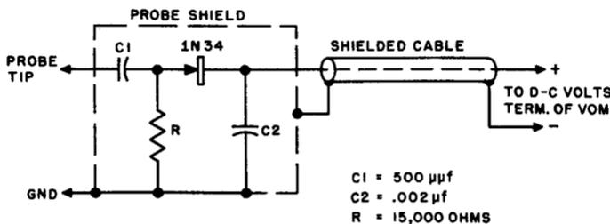
Fig. 6-20. R-F probe which makes possible the use of a service-type vom for indicating the presence, or comparative values, of r-f voltages of almost any waveform.
