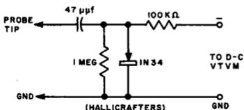
HIGH IMPEDANCE, RELATIVELY HIGH SENSITIVITY, PEAK-INDICATING TYPE. SHUNT RECTIFIER. INTENDED FOR HIGH FREQUENCY APPLICATIONS.
