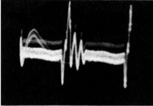
Fig. 2-7. Typical ripple voltage on the output voltage of the high-voltage supply at the second-anode of the picture tube.
