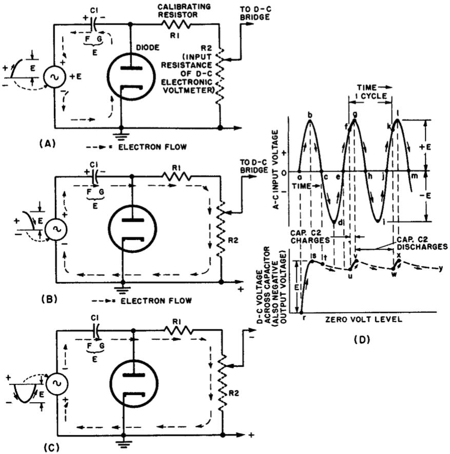
Fig. 6-5. (A), (B), (C) Basic circuit arrangement and action of a tube diode rectifier for a vtvm, during one cycle of the a-c input voltage. (D) If an a-c voltage (lower graph) is applied to the input circuit, a practically smooth d-c voltage (upper graph) that is proportional to the peak value of the a-c voltage, can be made to appear across the output circuit by proper choice of the time constant of the R-C circuit network.
