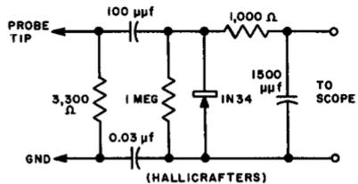
MEDIUM-LOW IMPEDANCE TYPE; MODERATE SENSITIVITY. SHUNT RECTIFIER. SCOPE CABLE ISOLATED.
