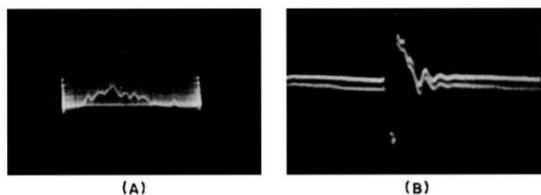
Fig. 7-26. An attempt to obtain signal pickup for a demodulator probe by means of a floating tube shield may be disappointing unless the horizontal- and vertical-sweep circuits of the tv receiver are first disabled. (A) Interference from stray field of horizontal sweep circuit. (B) Interference from stray field of vertical sweep circuit.
