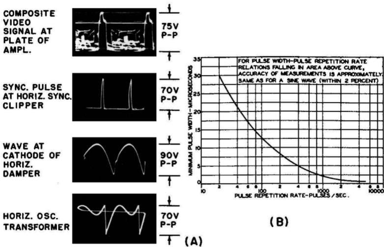
Fig. 6-9. (A) Typical narrow-pulse voltage waveforms of low repetition rate encountered in tv receivers. Use of a p-p vtvm to measure the p-p voltages of such waveforms may result in inaccurate readings. (B) Typical pulse-response capability of a high-quality service-type vtvm. The graph shows the inherent capability of the instrument. (B) Courtesy: RCA
