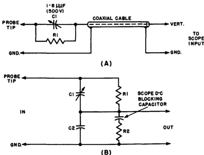
Fig. 5-2. (A) A simple type of low-capacitance probe which causes a-c signal attenuation only. The probe capacitance  $C_1$  and resistance  $R_1$ , and the overall scope (plus cable) input capacitance  $C_2$  and resistance  $R_2$ , form the resistance-capacitance divider circuits shown in (B). The scope d-c blocking capacitor is neglected in this consideration, because its reactance is practically zero at radio frequencies.
