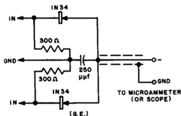
BALANCED-INPUT LOW IMPEDANCE, RELATIVELY LOW SENSITIVITY, PEAK-INDICATING TYPE. BALANCED SHUNT RECTIFIER. MICROAMMETER OR SCOPE INDICATOR. USEFUL FOR CHECKING STANDING-WAVE RATIO ON LINE, IMPEDANCE MATCH, FLATNESS, ETC.
