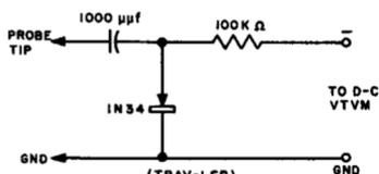
HIGH IMPEDANCE, HIGH SENSITIVITY, PEAK-INDICATING TYPE. SHUNT RECTIFIER. INTENDED FOR HIGH-FREQUENCY APPLICATIONS.
