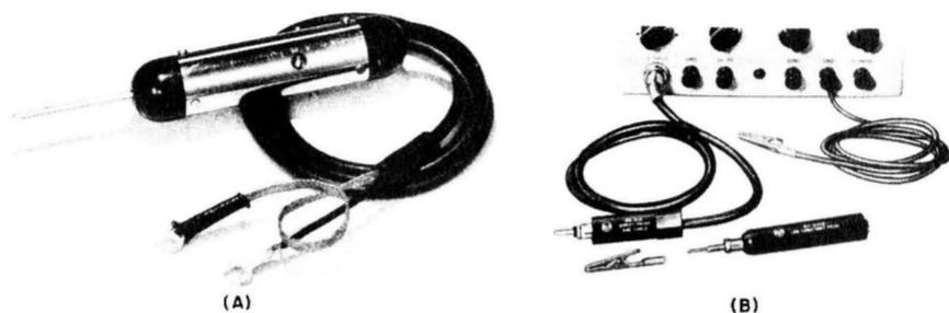
Fig. 5-5. (A) External appearance of a low-capacitance type scope probe provided with its own shielded cable and terminals. (B) A separable type of low-capacitance probe designed to be slipped on to the standard direct probe (with cable) employed for several models of this manufacturer's scopes. (A) *Courtesy: Hickok Elect. Inst. Co.* (B) *Courtesy: RCA*
