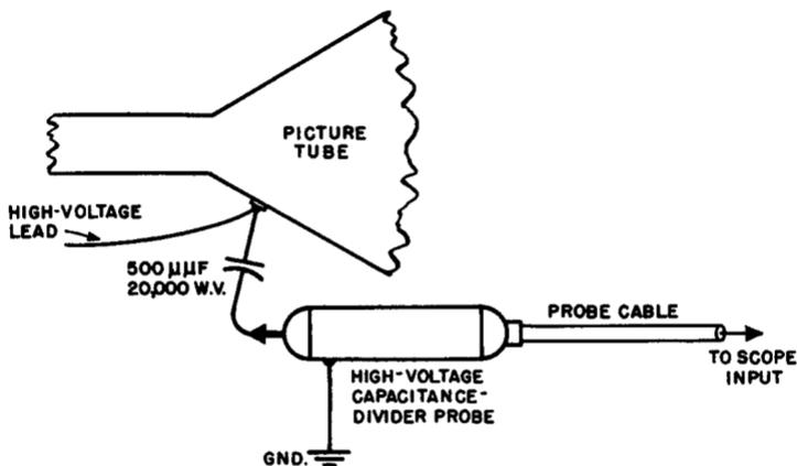
Fig. 2-9. When testing at the second anode of the picture tube for ripple, or for tunable buzz pulses, it is good practice to place a d-c blocking capacitor,  $C$ , in series with the voltage-divider probe, as shown here, for protection in the event that the d-c voltage at this point exceeds the voltage rating of the probe.
