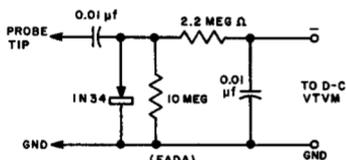
HIGH IMPEDANCE, HIGH SENSITIVITY, PEAK-INDICATING TYPE. SHUNT RECTIFIER. CAN BE USED DOWN TO RELATIVELY LOW FREQUENCIES.
