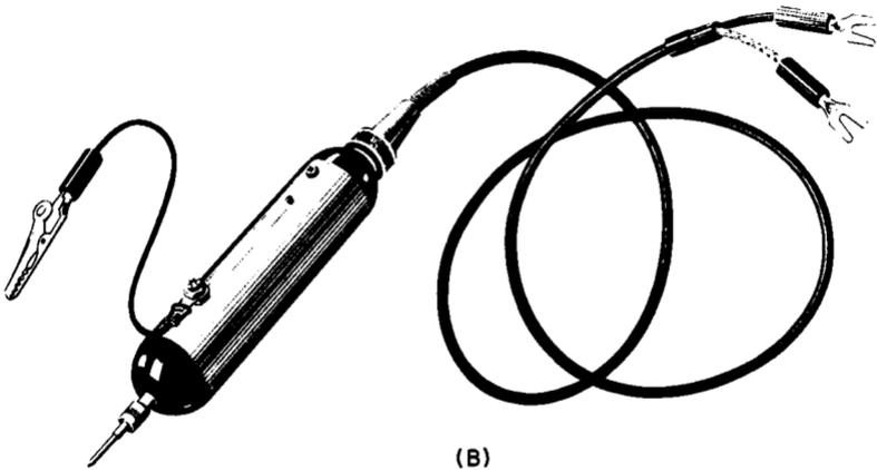
Fig. 7-18. (A) Voltage-doubler type of demodulator probe for obtaining increased output and greater deflection on the scope than is provided by conventional type of demodulator probes. (B) A typical commercial probe of this type. This probe is provided with its own shielded cable for connection to the scope input terminals. (B) Courtesy: Scala Radio Co.
