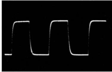
for the observation of sweep-curve response in tv alignment work (in which a 60-cycle sweep is usually employed).
