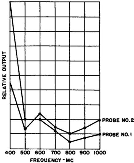
Fig. 6-24. Actual response of two typical commercial r-f crystal-diode rectifying probes at uhf. These probes, which are designed for application in the 30- to 300-mc vhf range, develop sharp peaks and valleys in the response characteristic, due to multiple resonances, and also an appreciable drop in output, when used in the uhf range. The input impedance of such probes is also very low at uhf.
