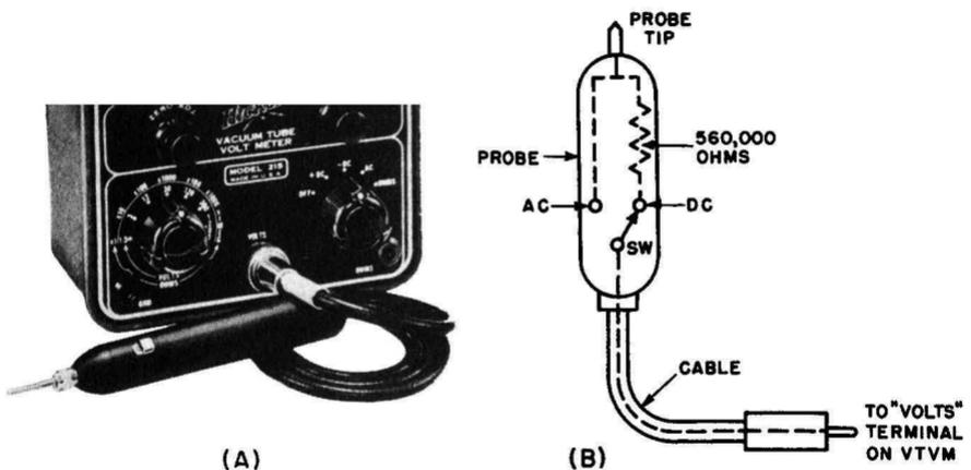
Fig. 4-6. Slide-switch arrangement used on vtvm resistive isolation (d-c) probe to provide d-c and a-c voltage test facilities using one test cable. (B) Switching circuit. (A) Courtesy: Hickok Elect. Instr. Co.
