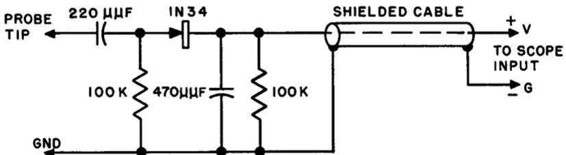
Fig. 7-6. Practical series-type demodulator probe having a relatively high input impedance and provided with a blocking capacitor, a bleeder resistor, and a shunting resistor for hum-voltage reduction.
