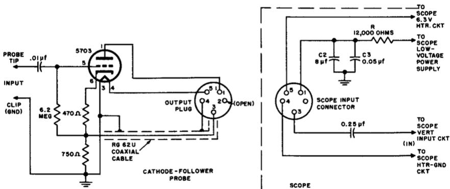
Fig. 5-22. Schematic circuit diagram of 10-LCP cathode-follower type of circuit-isolation probe which features a high input impedance, and comparatively low attenuation factor. Courtesy: Jackson
