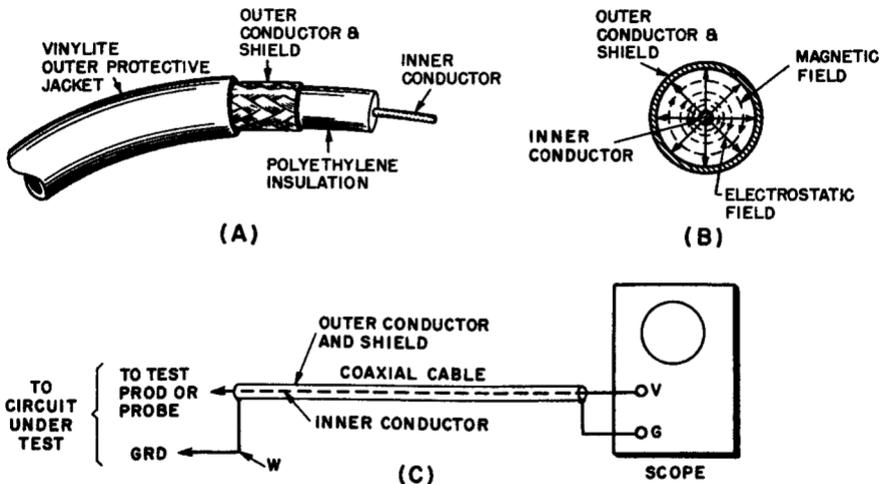
Fig. 3-5. (A) Type of r-f flexible coaxial cable widely employed for test leads. (B) The instantaneous magnetic and electrostatic fields that exist at one point along a coaxial cable due to the current flowing through it at that instant. (C) Method of connecting a coaxial cable to serve as the test leads between a test instrument and a test prod or probe.
