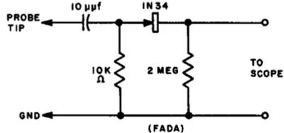
MEDIUM-IMPEDANCE TYPE; MEDIUM SENSITIVITY. SERIES RECTIFIER. SCOPE CABLE UNISOLATED.
