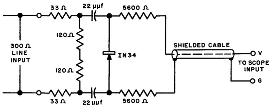
Fig. 7-17. When operating at uhf, the balanced-input demodulator probe network can be tapped down on the load, as shown here, so that the capacitance of the network does not seriously disturb the line termination. *Courtesy: RCA*
