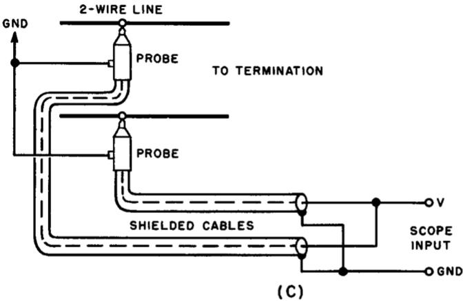
Fig. 7-16. (A) Shop-constructed balanced-input probe arrangement for checking the voltage existing at any point along a 2-wire line. Such probes are useful for impedance-match (standing-wave) testing procedures. (B) Sensitive arrangement employing only one diode and requiring no ground return. (C) Method of using two conventional general-purpose demodulator probes for the purpose, instead of a special balanced-input probe.
