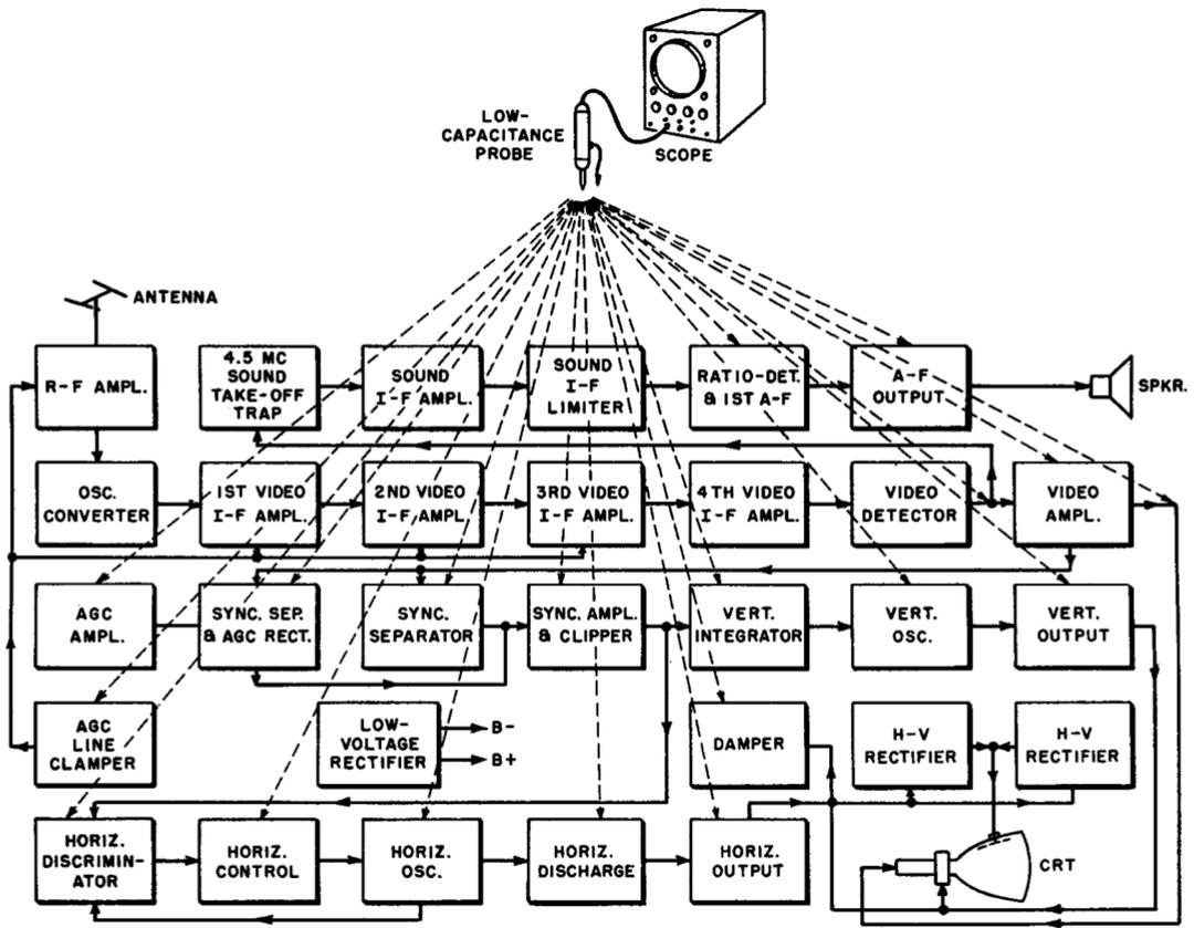
Fig. 5-16. Applications of the low-capacitance probe, used in conjunction with a scope, for waveform checks and p-p voltage measurements in a tv receiver.
