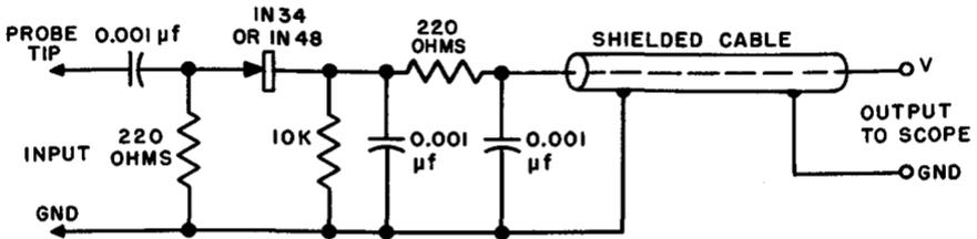
Fig. 7-11. Shop-constructed, low-impedance (traveling detector), series-rectifier type of demodulator probe designed especially for stage-by-stage signal-tracing or alignment work in r-f amplifiers. The output is well filtered by the pi-filter section provided.
