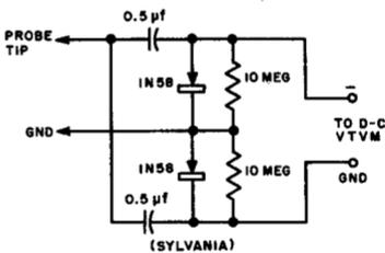
PEAK-TO-PEAK INDICATING PROBE, MEDIUM-HIGH SENSITIVITY. SHUNT RECTIFIERS, VOLTAGE-DOUBLER CIRCUIT. INTENDED FOR P-P MEASUREMENT OF COMPLEX WAVEFORMS.
