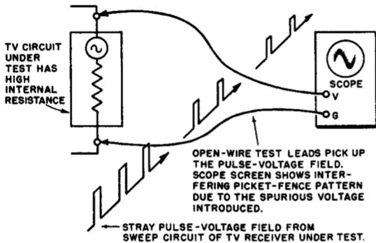
Fig. 3-4. When open-wire test leads are used with a scope, spurious voltages may be induced in the exposed leads, or in an unshielded probe, by strong stray fields present about the equipment under test. If the circuit under test has a high impedance, a corresponding visible interference pattern is likely to appear on the scope screen.
