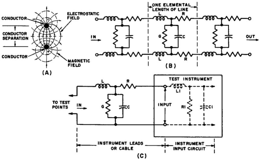
Fig. 3-2. (A) View of the instantaneous magnetic and electrostatic fields about each wire at one point along an open-wire transmission line. (B) As a result of the existence of these fields each elemental length of the line contains series inductance and resistance, and shunt capacitance and leakage. The distributed constants in an open-wire line are shown here. (C) Equivalent circuit, assuming lumped constants.
