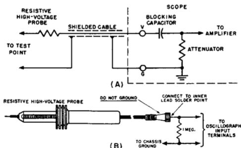
Fig. 1-8. (A) Technicians sometimes make the error of attempting to use a resistive high-voltage probe with an a-c type oscilloscope to observe the ripple in the high-voltage supply. This leads to possible breakdown of the blocking capacitor in the scope input circuit. Use of the alternative circuit arrangement (B), which is often suggested, is also open to several objections which are discussed in the accompanying text.
