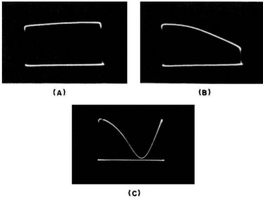
Fig. 7-43. Typical patterns obtained when checking the flatness of the sweep-signal output from sweep generators by means of a demodulator probe and a scope. (A) Reasonably flat output over the swept range. (B) Output slump-off at one end of the swept range. (C) Output with very bad slump-off at mid-sweep region. In all cases, sweep-generator blanking was employed to produce the zero-volt baseline.
