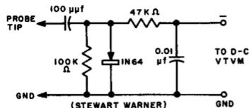
RELATIVELY HIGH IMPEDANCE, MEDIUM-HIGH SENSITIVITY. PEAK-INDICATING TYPE. SHUNT RECTIFIER. INTENDED FOR HIGH-FREQUENCY APPLICATIONS.
