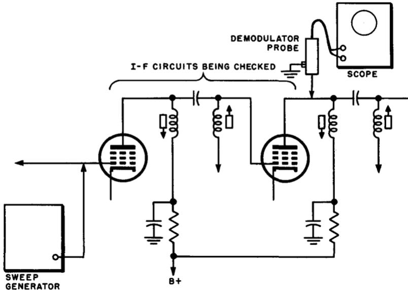
Fig. 7-31. Conventional method of checking the alignment, or testing the response, of a single stage of a video i-f amplifier, using a demodulator probe and scope for visual indication.
