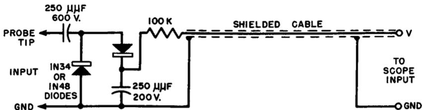
Fig. 7-41. Special shop-constructed voltage-doubler demodulator probe designed to have a high degree of 60-cycle voltage rejection due to the small size of series capacitance employed in it. This type of probe is extremely useful for localizing spurious high-frequency voltages in 60-cycle a-c heater lines.
