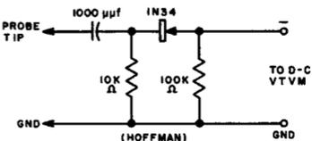
MODERATELY HIGH IMPEDANCE, MEDIUM SENSITIVITY, PEAK-INDICATING TYPE. SERIES RECTIFIER. INTENDED FOR HIGH-FREQUENCY APPLICATIONS.
