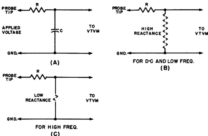
Fig. 4-3. Resistive-isolation probe circuit action which illustrates why the high frequencies are discriminated against when an attempt is made to employ a resistive isolation probe to minimize the loading effect of the cable capacitance upon the circuit under test during high-frequency a-c voltage measurements made with a vtvm.
