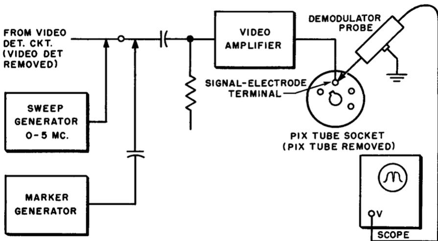
Fig. 7-36. Instrument setup for frequency-response check, or signal tracing, in a video amplifier by means of a sweep signal, if the video detector is not to be included. The demodulator probe used in this work must meet several important requirements (see text).
