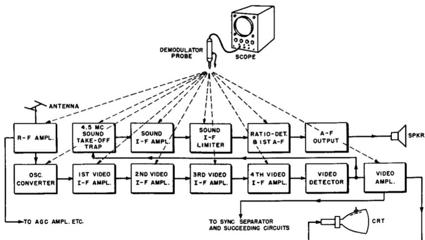
Fig. 7-28. Sections of a tv receiver in which demodulator probes are widely used in visual circuit-alignment and troubleshooting procedures.
