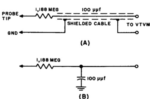
Fig. 1-7. (A) A high-voltage resistive probe with the capacitance of its shielded cable is seen to have the characteristics of a low-pass filter (B). This property of the probe is useful in measuring d-c plate voltage values in the presence of high-voltage short-duration a-c pulses at the plate of the horizontal-output tube of a tv receiver, without damage to the vom or vtvm.
