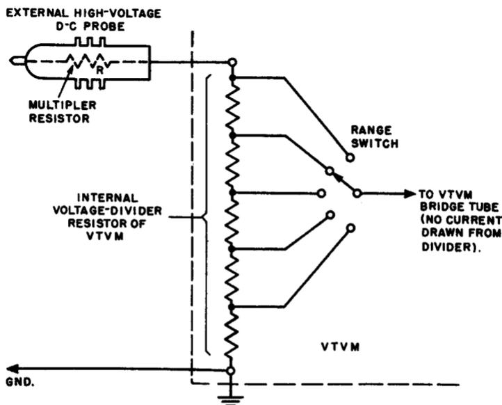
Fig. 1-4. The measuring tube of a vtvm draws no current, and hence the meter in the vtvm really indicates the voltage drop at any selected point along the internal voltage-divisor resistor, instead of measuring the current through the instrument, as does a vom. For convenience, the value of the external multiplier resistor in the the resistive high-voltage probe can be selected to multiply each of the vtvm voltage ranges by a convenient decimal factor, such as 100.
