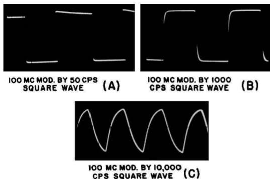
Fig. 7-21. Demodulating ability of a conventional type demodulator probe for modulation of various frequencies. It can be seen that the demodulating ability of the probe decreases as the modulation frequency increases, and distortion of the modulation waveform results. A voltage-doubler type of probe is usually more unfavorable than the conventional type in this respect.
