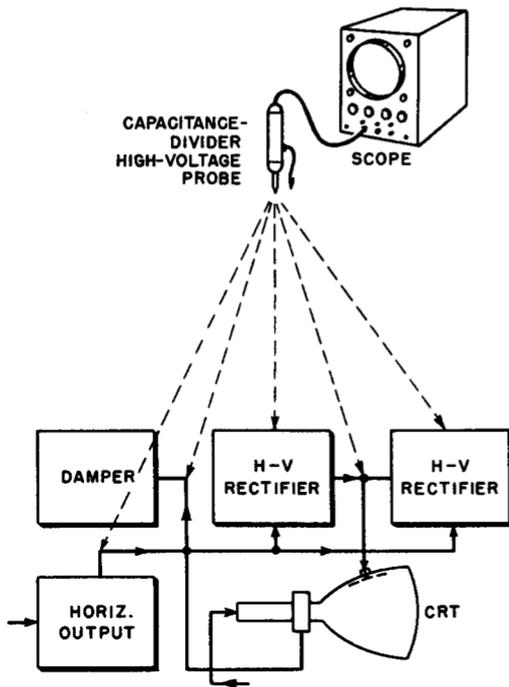
Fig. 2-1. Tv receiver high-voltage 15,750 cps horizontal sweep circuit in which a capacitance-divider type high-voltage probe must be used with a scope for a-c voltage measurement or waveform observation.
