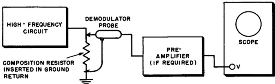
Fig. 7-27. The waveform of modulated high-frequency currents in a tv receiver can be displayed on a scope screen with the aid of a demodulator probe and a small resistor. A pre-amplifier will often be necessary to obtain sufficient deflection on the scope screen when a small resistor is used. A large value of resistance is likely to disturb the circuit action, and will also result in a distorted waveform due to the effect of the input capacitance of the demodulator probe.
