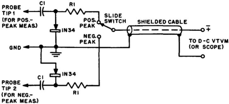
Fig. 6-16. A special peak-indicating probe arranged to provide either positive-peak or negative-peak indication, as desired. This general circuit arrangement, employing suitable values for  $C1$  and  $R1$ , may also be employed with a scope.
