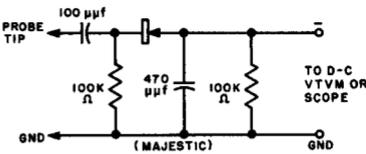
(PEAK-INDICATING OR DEMODULATOR PROBE -- DEPENDING UPON SIGNAL FREQUENCY). RELATIVELY HIGH IMPEDANCE AND SENSITIVITY. SERIES RECTIFIER.
