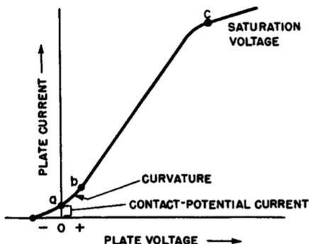
Fig. 6-10. Contact potential and curvature of the lower end of the operating characteristic are shown here for a typical tube diode.
