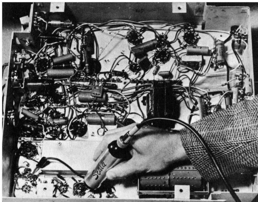
Fig. 7-33. Signal-tracing in a video i-f amplifier with a crystal demodulator probe and scope. Observe that the probe ground-return is clipped to chassis ground (at lower left) as close as possible to the signal take-off point. *Courtesy: Scala Radio Co.*
