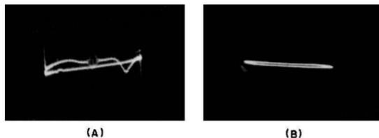
Fig. 7-32. Typical patterns obtained when the demodulator probe detunes an i-f stage and throws it into oscillation. Since the scope deflection becomes so small, an oscillating stage due to probe loading can easily be confused with a weak or a dead stage.
