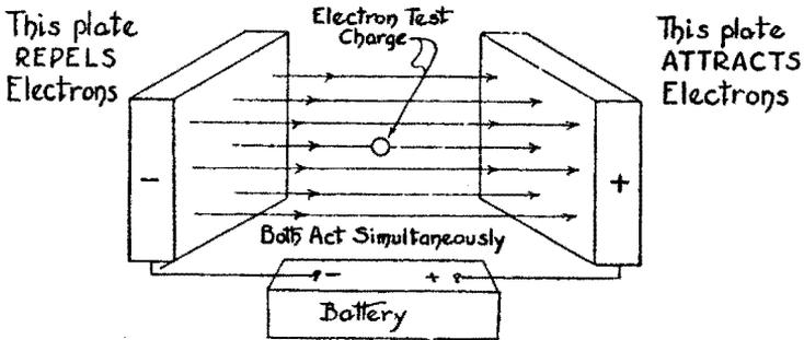
The uniform field is due to the existence of two forces acting on the electron and the fact that the sum of these forces remains the same no matter where the electron may be located between the two fixed charged plates.
