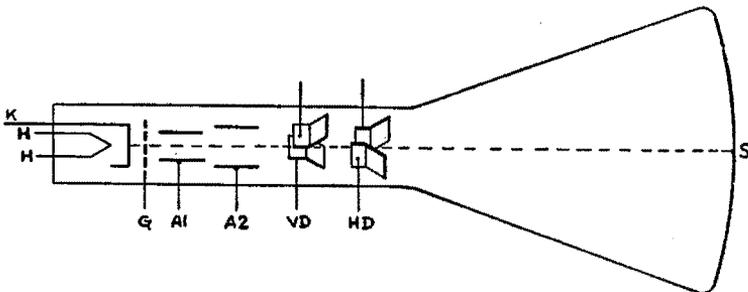
FIG. 15-25. The fundamental elements of a cathode-ray tube.
