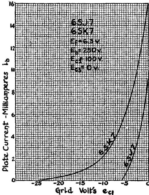
FIG. 15-19. The grid voltage—plate current curve marked 6SJ7 is for a sharp-cutoff pentode and that marked 6SK7 is for a remote-cutoff (variable mu) tube. These show that the 6SK7 can be operated at a grid voltage that is about five times more negative than the other.
