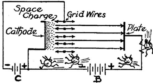
electrons, it must be in a direction which is *away* from the control grid. Thus the arrows which originate at each of the grid wires point away from the grid.
