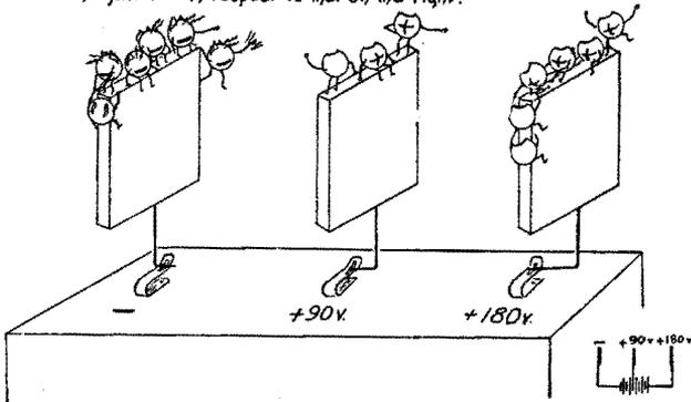
to an intermediate terminal, which happens to be 90-volts plus, then has the deficiency of electrons which would charge that plate 90-volts plus with respect to the negative plate. If the third plate is connected to the plus 180-volt terminal of the voltage source, that terminal has a deficiency of electrons (a preponderance of positive ions) equal to the surplus upon the negative plate, but twice as many positive ions as the plate which is joined to the 90-volt terminal of the voltage source.
