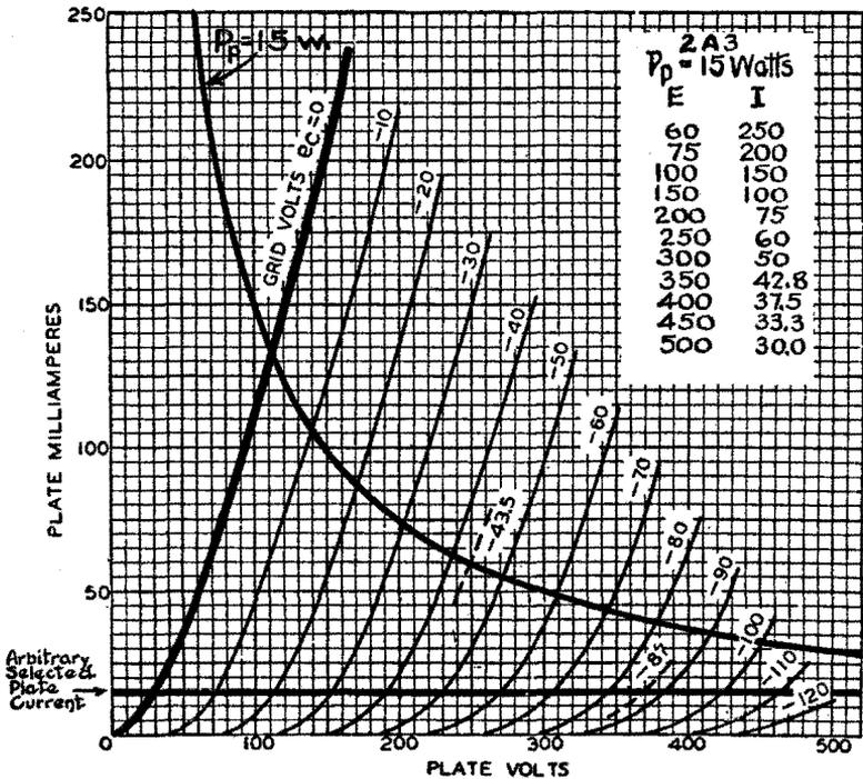
FIG. 14-2. The three boundaries for correct operation of a power tube are the plate-dissipation curve ( $P_p$ ), the  $e_c = 0$  curve of the plate family, and an arbitrarily selected plate-current line, in this case 15 milliamperes.
