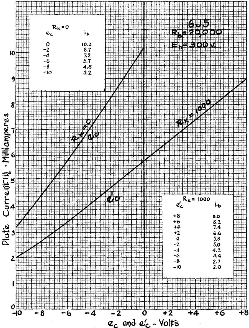
FIG. 13-8. The difference that a cathode resistor makes in the dynamic transfer characteristic of a triode is illustrated by these two curves. The curve marked  $e_c$  was derived when no cathode resistor was included, and the  $e'_c$  curve was derived when 1000 ohms was in the cathode circuit. In both instances a plate load of 20,000 ohms was used.
