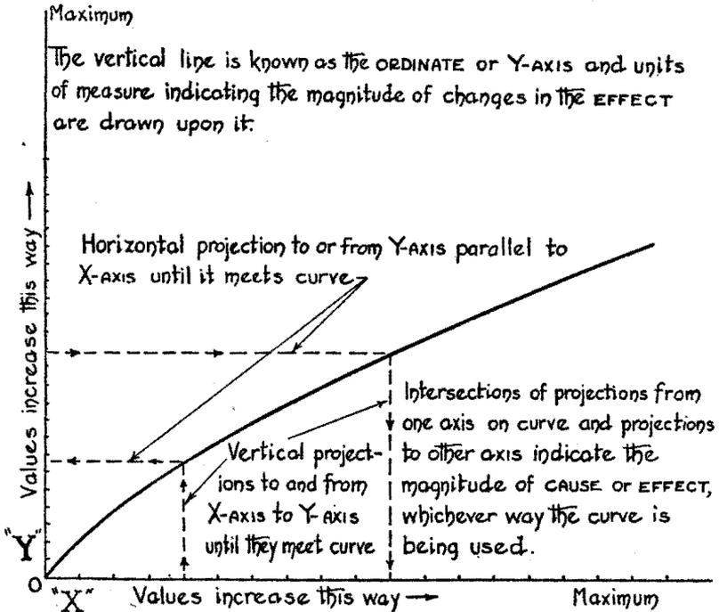
The horizontal line is known as the **ABSCISSA** or **X-AXIS** and units of measure indicating changes in magnitude of the **CAUSE** are shown upon it.
