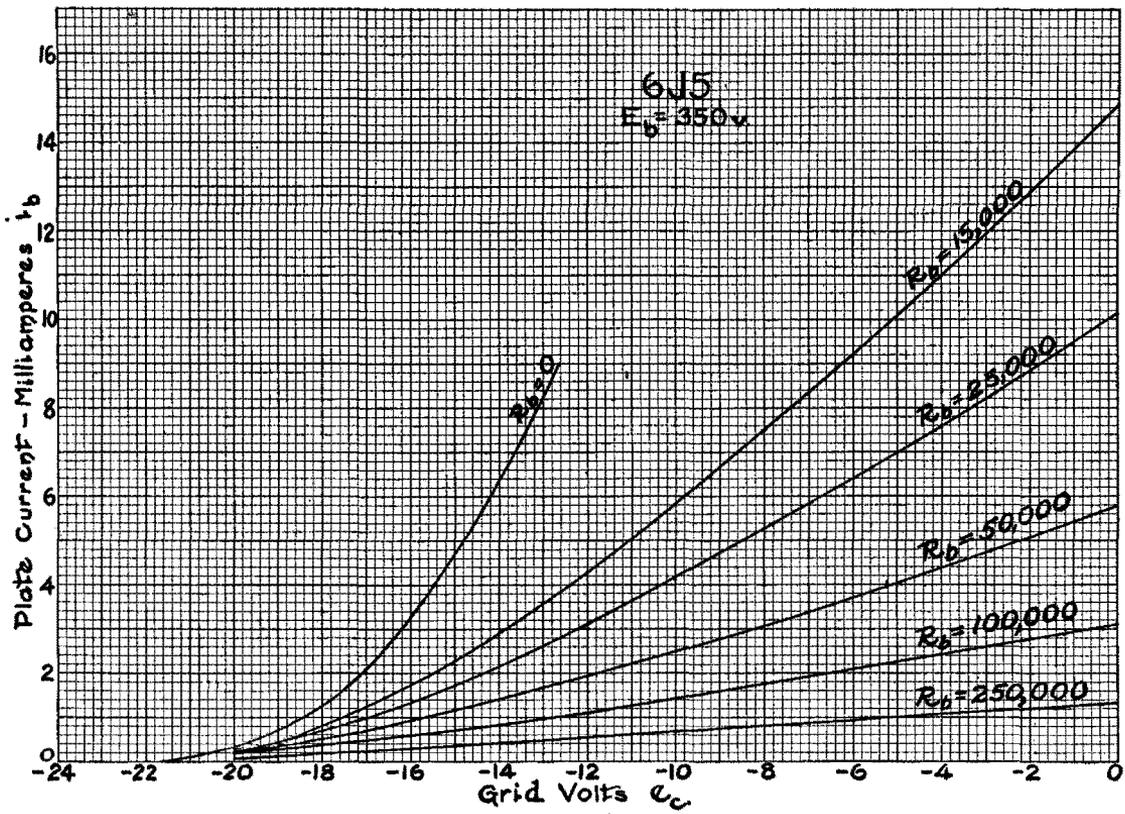
Fig. 9-11. These dynamic transfer characteristic curves correspond to the load lines of Fig. 9-9 for the same operating conditions.
