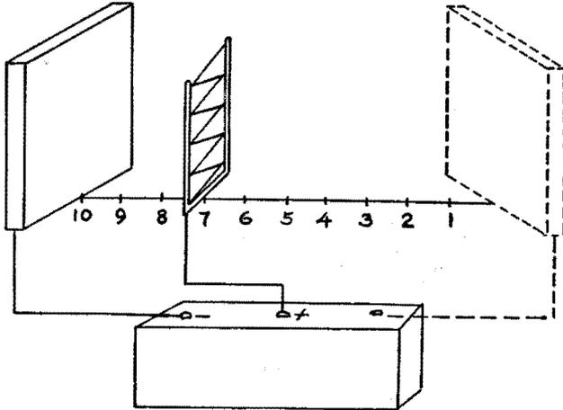
Locating a charged body closer to the test charge requires a much lower voltage to exert a certain constant force upon an electron than another charged body further removed.
