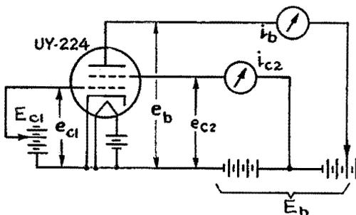
the graph of Fig. 12-6. The tetrode used in this test was the now obsolete filament-type UY-224, because it exhibits certain properties of fundamental interest which later types of tetrodes do not show. Curves for just one control-grid and screen-grid voltage setting are shown in Fig. 12-6 for illustrative purposes: the control-grid voltage  $e_{c1}$  is equal to  $-1.5$  volts and the screen-grid voltage  $e_{c2}$  is equal to  $+75$  volts.
