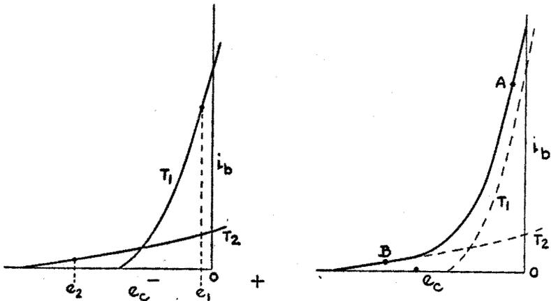
FIGS. 15-17 (left), 15-18 (right). The curves marked  $T_1$  and  $T_2$  are the dynamic transfer characteristics of tubes  $T_1$  and  $T_2$  respectively of Fig. 15-16. The curve on the right is a combination of the two curves on the left and is the characteristic of a variable- $\mu$  amplifier.
