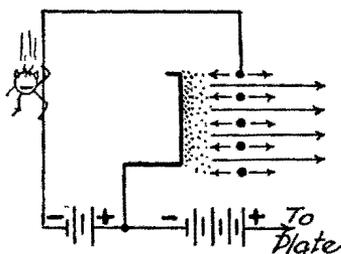
FIG. 7-7. In some instances, electrons do flow in the grid circuit when the grid is negatively charged because the grid bias is insufficient to repel the electrons that are attracted to the plate because of the high plate voltage.
