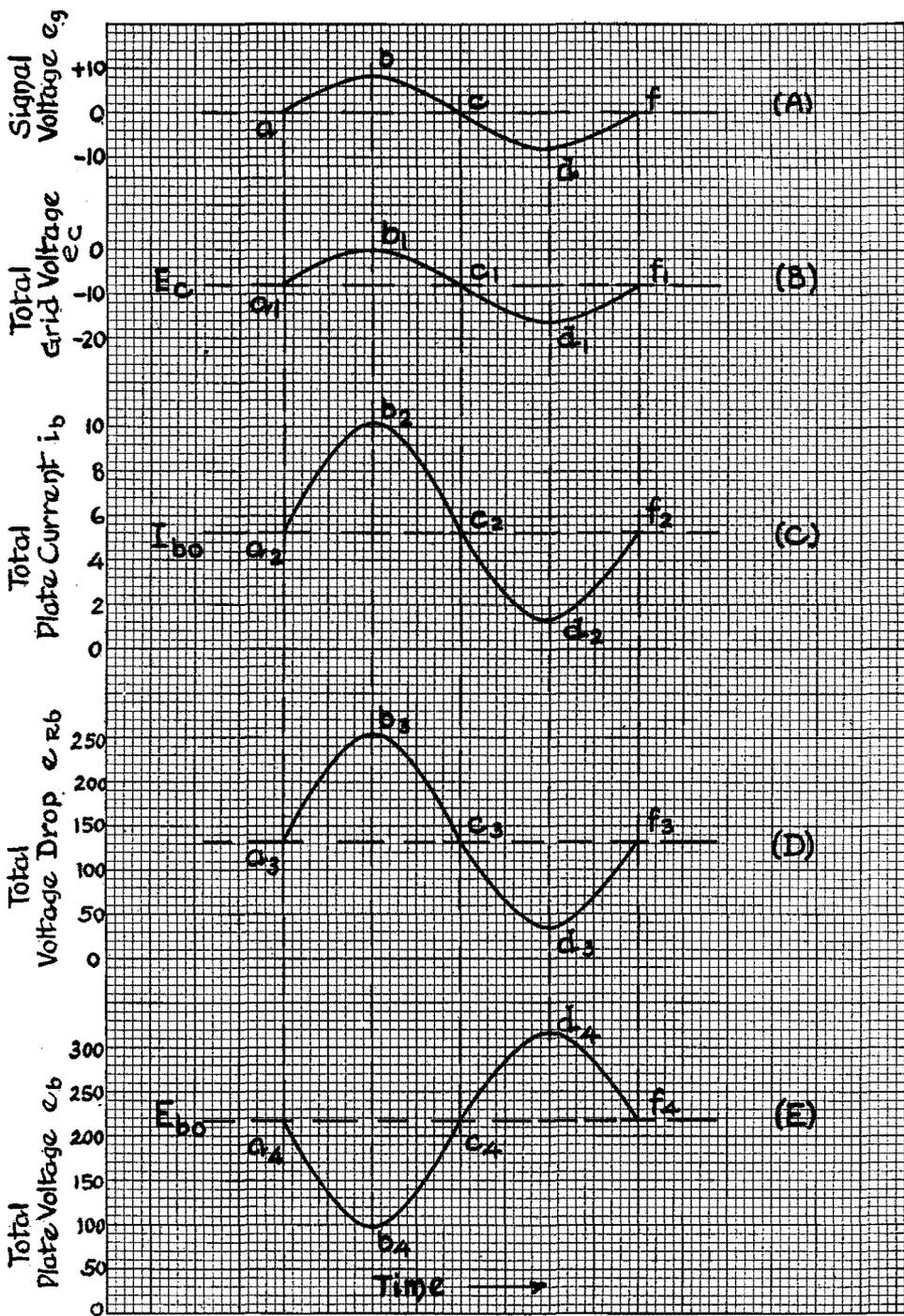
FIG. 11-8. This series of waves shows that the input voltage  $e_g$  is in phase with the plate current  $i_b$  and that  $e_g$  is  $180^\circ$  out of phase with the plate voltage  $e_b$ .
