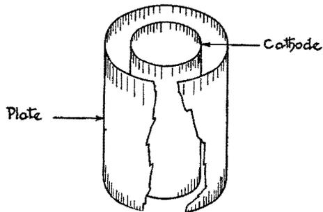
FIG. 6-5. The cylindrical plate surrounds the cathode in the actual diode, as indicated on the right. These two electrodes are supported by wires that are embedded in the glass press at the bottom of the tube.
