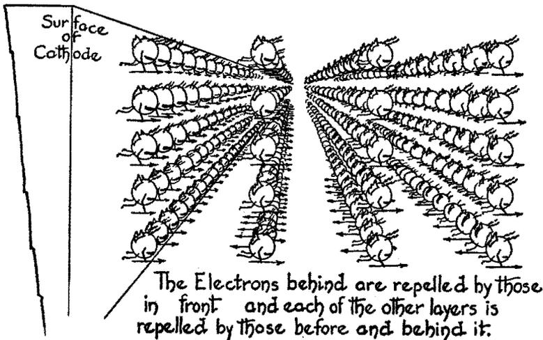
Since the basic law pertaining to charged bodies states that like charges repel one another, the electrons in back of the first group are experiencing a repelling force due to the electrons in front of them and the direction of this force is such as to tend to retard the motion of the electrons in their advance away from the cathode.
