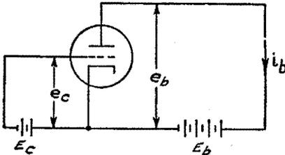
FIG. 8-1. The voltages and current in this triode circuit are designated as follows:  $E_b$  and  $E_c$  are the plate supply and grid bias voltages respectively;  $e_b$ , the voltage effective at the plate;  $e_c$ , the voltage effective at the grid, and  $i_b$ , the plate current.
