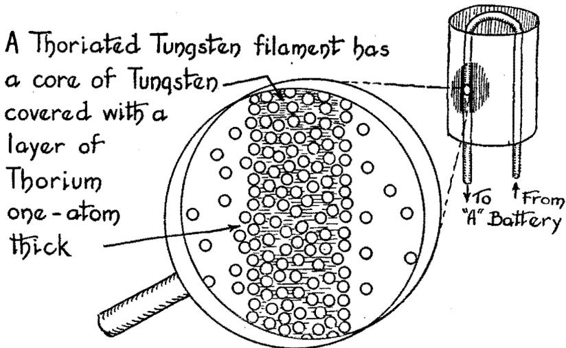
Thoriated-tungsten filaments as electron emitters largely supplanted tungsten filaments in receiving and low-powered transmitting tubes. This type of filament affords the advantage of greater electron emis-
