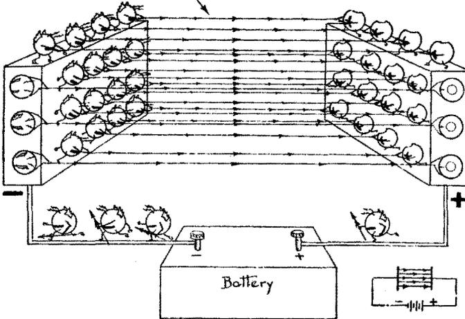
plates are connected to the terminals of this battery, electrons flow from the metal plate connected to the plus terminal and other electrons flow from the negative terminal to the other metal plate, so that these extensions of the voltage source develop an electron distribution, shortage and surplus, exactly equal to that which exists at the terminals of the voltage source. The charges upon these plates are assumed to be uniformly distributed upon the respective surfaces.
