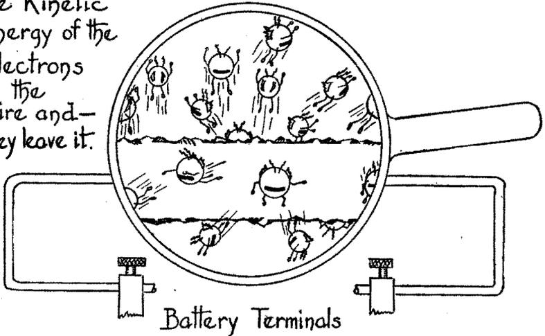
in the substance, and that their motion is accelerated sufficiently so that they are liberated from the substance. This action is called *photoelectric emission*.
