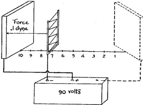
voltage required upon the original plates, which were separated by 10 centimeters in order to create the same change in the force upon the unit charge, is 540 volts. Thus we see that this third electrode is about 3.3 times as effective as the positive plate in controlling the force upon the test charge.
