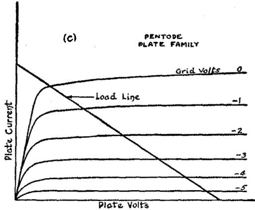
The general plate voltage—plate current characteristic curves with a typical load line on each for the three fundamental types of amplifier tubes; (A) the triode, (B) the tetrode, and (C) the pentode.
