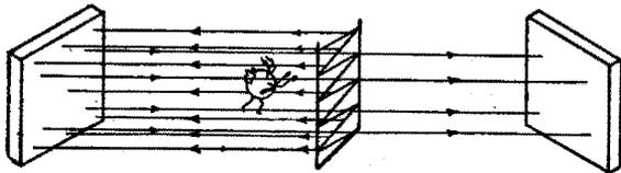
When the field due to the wire mesh is opposite to that of the plate, the progress of the unit charge is hindered.
