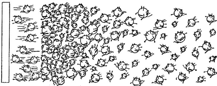
creases. When this increase in density has again reached such a value that the repelling force of the electrostatic field of the space charge is sufficient to overcome the higher average velocity of the electrons emitted at the increased cathode temperature, and is again repelling the emitted electrons, a new state of equilibrium has again been established and *emission saturation* again exists.
