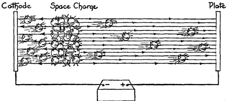
With a certain voltage impressed between the Plate and Cathode and with a certain Cathode temperature, as many Electrons enter the Space Charge from the Cathode as leave it for the Plate
