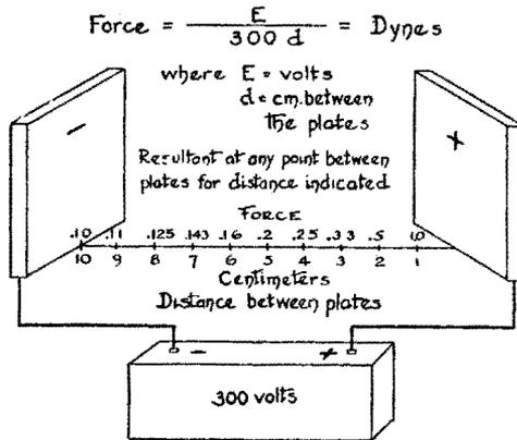
evident that increasing the separation between the plates to 20 centimeters would decrease the force to 0.05 dyne, assuming, of course, that the voltage between the plates remains 300 volts.
