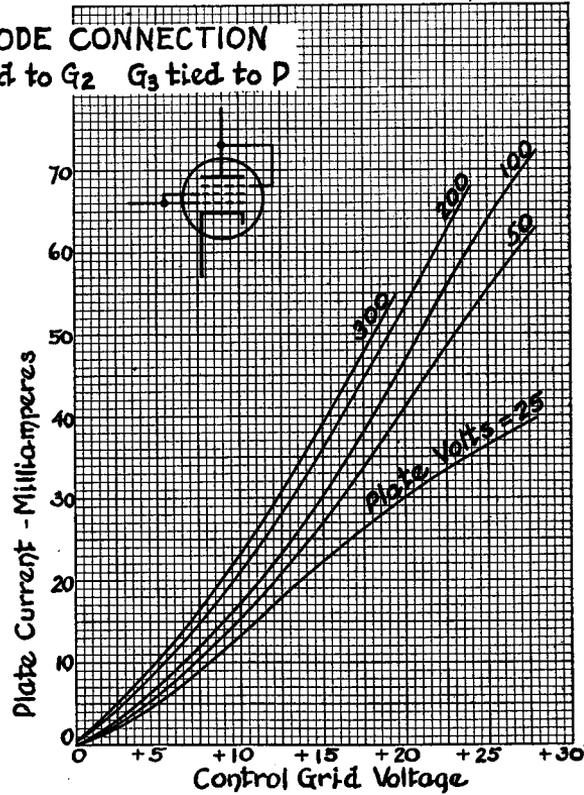
Figs. 12-25 (left), 12-26 (right). The plate and grid families of a 6SJ7 connected as a triode when the control-grid is connected to the screen-grid and the suppressor-grid is connected to the plate.
