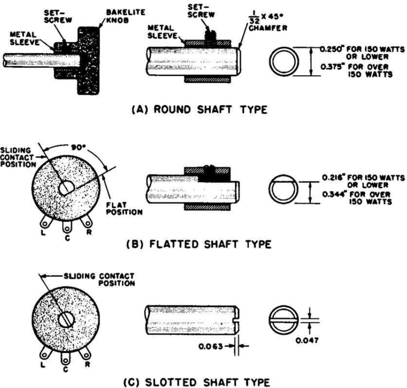
Fig. 2-7. Military standard shaft types. (A) Round. (B) Flatted. (C) Slotted.
