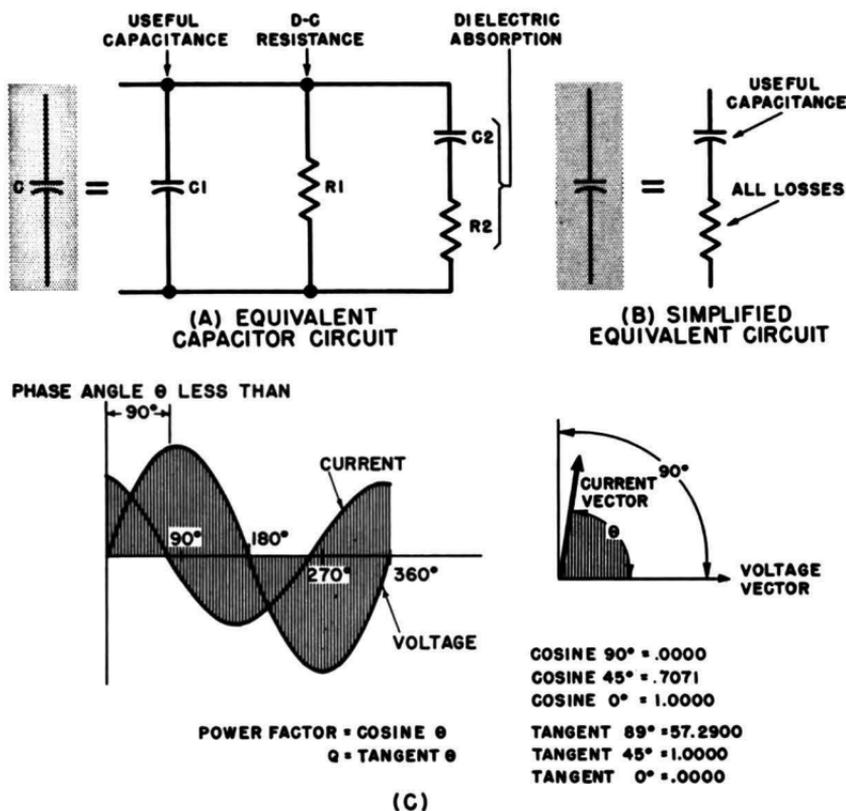
Fig. 3-6. Basic capacitor characteristics. (A) Equivalent circuit. (B) Simplified equivalent circuit. (C) Power factor and  $Q$ .
