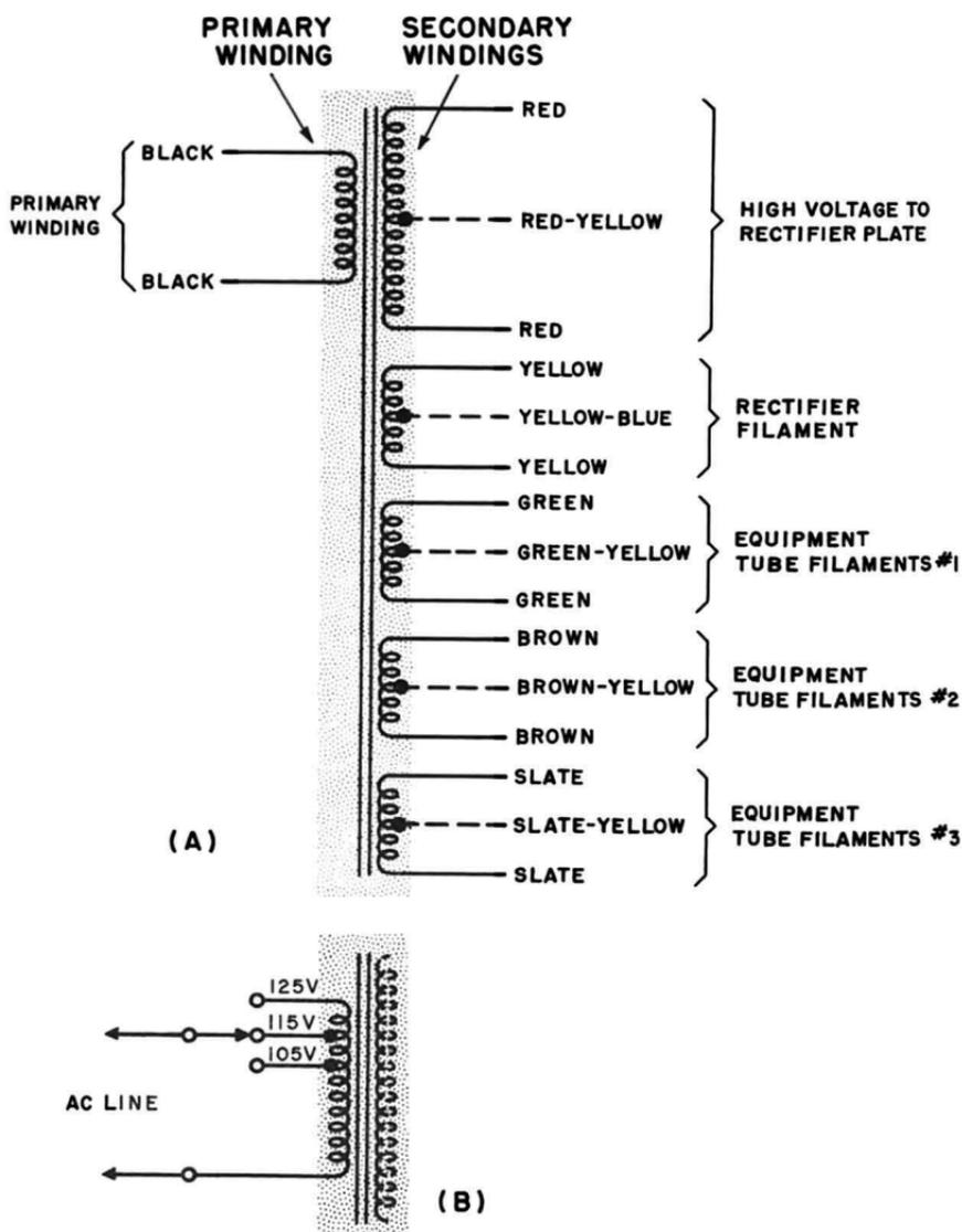
Fig. 6-7. Power transformers. (A) Color code for rectifier plate- and filament-supply transformer. (B) Transformer with tapped primary.
