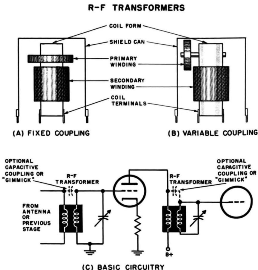
Fig. 6-11. R-f transformers. (A) Fixed coupling. (B) One type of variable coupling. (C) Basic circuits.
