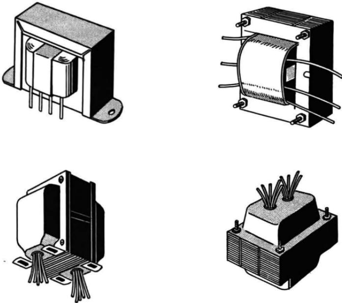
Fig. 6-1. Typical laminated iron-core inductor and transformer shapes. After Chicago Standard Transformer Corp.
