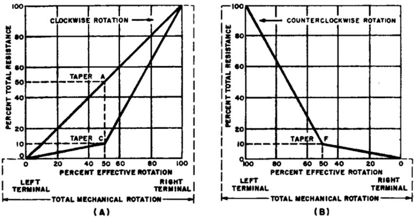
Fig. 2-14. Charts of variable wirewound resistor tapers. (A) Clockwise tapers. (B) Counterclockwise tapers.
