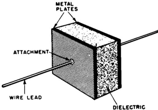
Fig. 3-2. Basic capacitor construction.
