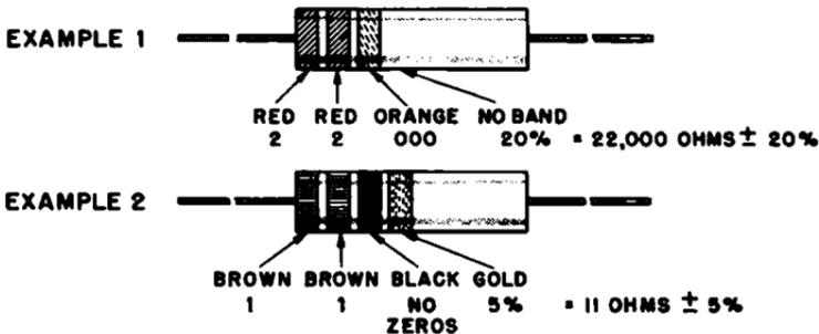
Fig. 2-1. Axial-lead composition resistor color code and examples.
