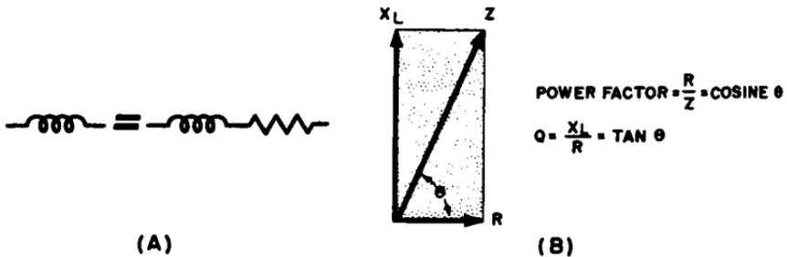
Fig. 5-4. Definition of coil power factor and  $Q$ . (A) Equivalent circuit of inductance and resistance. (B) Impedance diagram.
