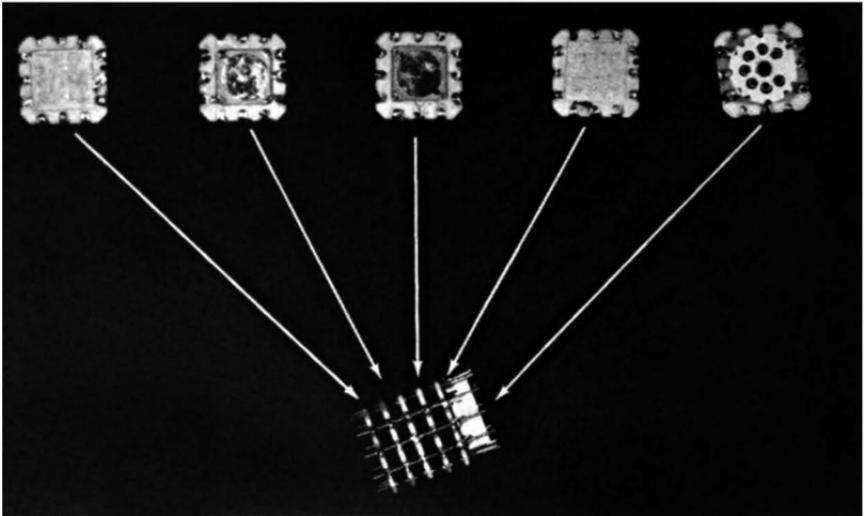
Fig. 6-15. Component parts of a module. Wafers contain tube socket, capacitors and resistors. Courtesy National Bureau of Standards.
