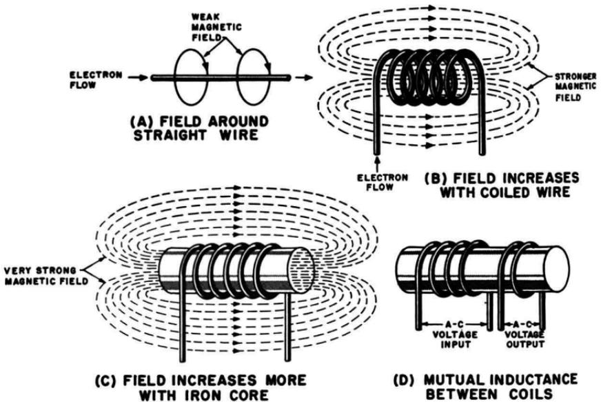
Fig. 5-1. Basic characteristics of magnetic fields. (A) Field around straight wire. (B) Field increases with coiled wire. (C) Field increases more with iron core. (D) Mutual inductance between two coils.
