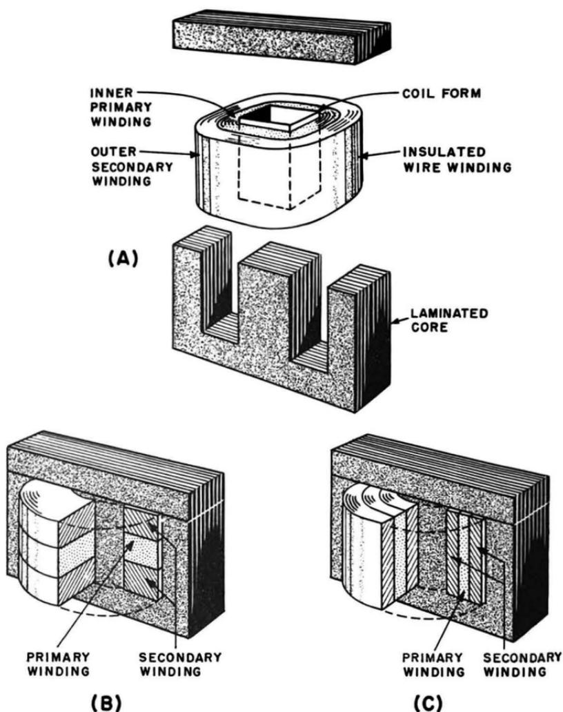
Fig. 6-5. Laminated core windings. (A) Coil on laminated core. (B) Side-by-side sectionalization. (C) Layer-by-layer sectionalization.
