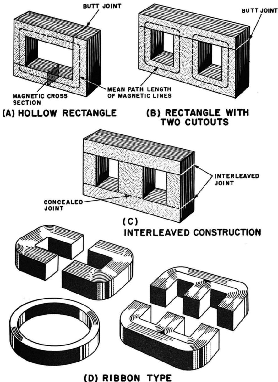
Fig. 6-2. Typical laminated cores. (A) Hollow rectangle. (B) Rectangle with two cutouts. (C) Interleaved construction. (D) Typical ribbon cores. After Arnold Engineering Co.
