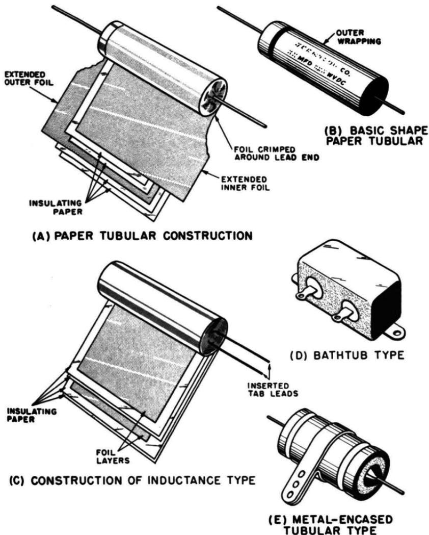
Fig. 4-1. Paper capacitors. (A) Basic construction. (B) Markings. (C) Construction of inductive type. (D) Bathtub type. (E) Metal-encased tubular.
