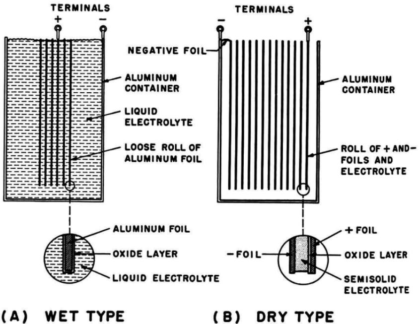
Fig. 4-4. Electrolytic capacitors, simplified construction. (A) Wet type. (B) Dry type.
