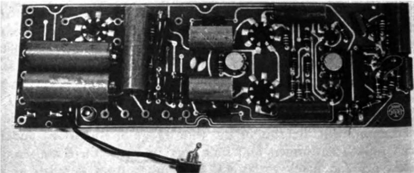
Fig. 6-13. Etched board with assembled components. Courtesy Photocircuits Corp.
