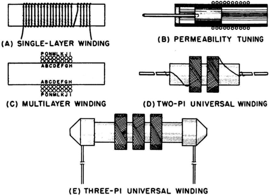
Fig. 6-4. Typical coil windings. (A) Single-layer (solenoid) winding. (B) Permeability tuning. (C) Multilayer winding. (D) Two-pi universal winding. (E) Three-pi universal winding. Courtesy National Co., Inc.
