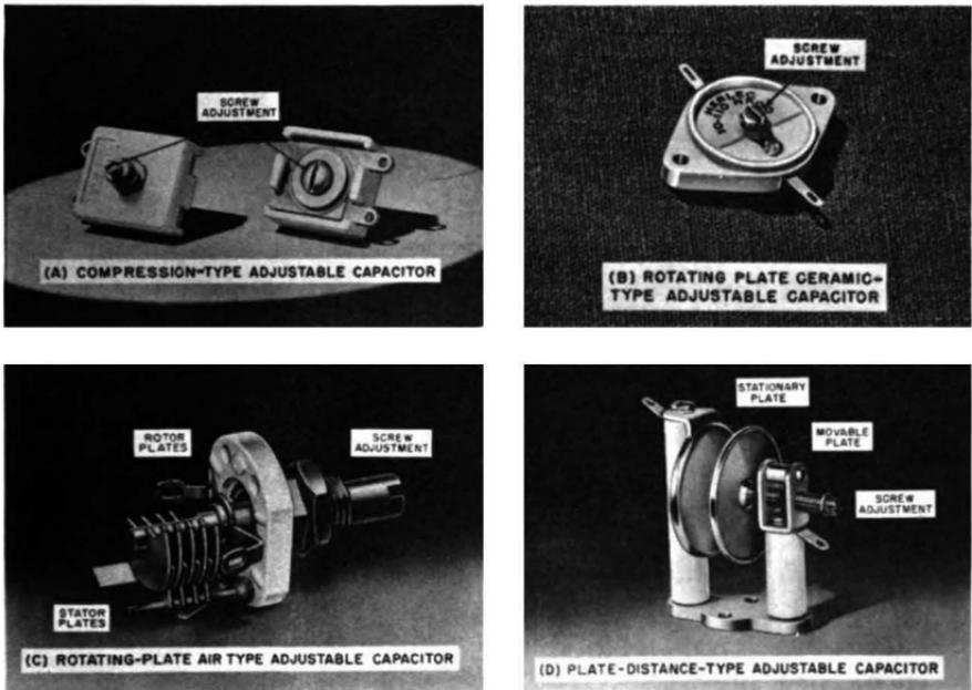
**Fig. 3-4. Adjustable capacitors. (A) Compression type. Courtesy Electro Motive Mfg. Co., Inc. (B) Rotating-plate ceramic type. Courtesy Sprague Electric Co. (C) Rotating-plate air type. (D) Adjustable-plate distance type. Courtesy Hammarlund Mfg. Co., Inc.**
