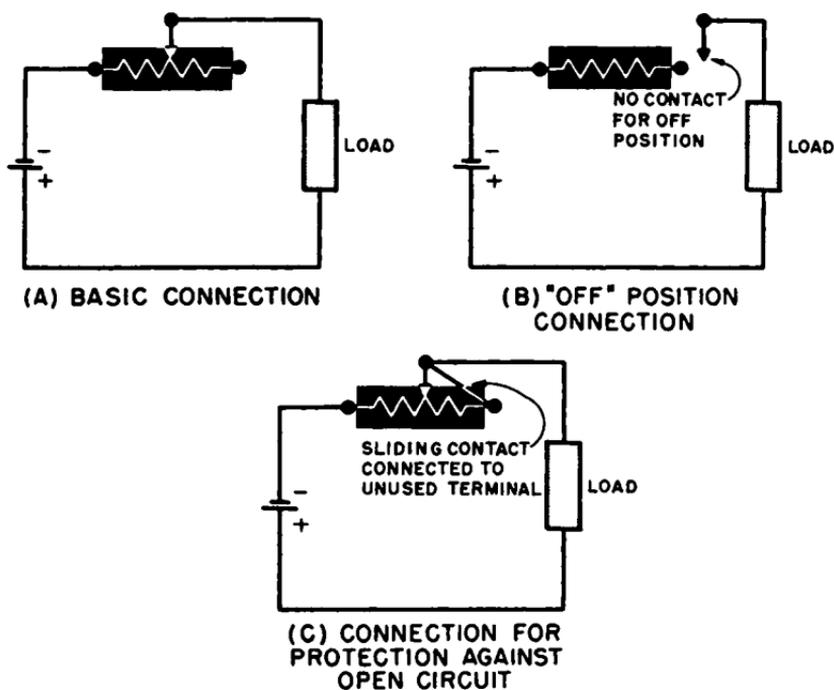
Fig. 2-10. (A) Rheostat connection. (B) Rheostat with "off" position. (C) Connection for unused terminal.
