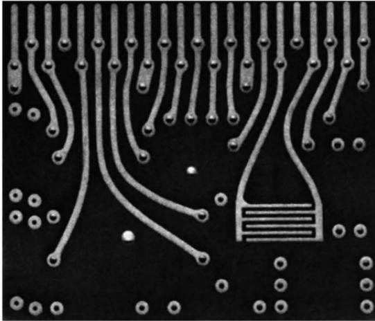
Fig. 6-14. Plug-in circuit with printed capacitor. Courtesy Photocircuits Corp.
