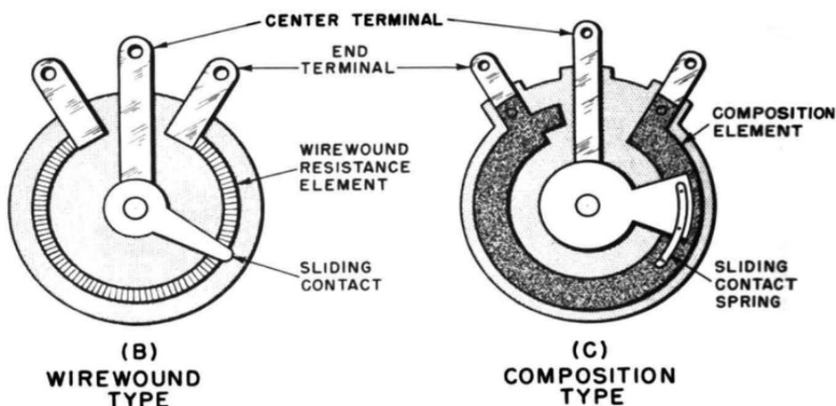
Fig. 1-3. Variable resistors. (A) General appearance. Courtesy Clarostat Mfg. Co., Inc. (B) Simplified construction, wirewound type. (C) Simplified construction, composition type.
