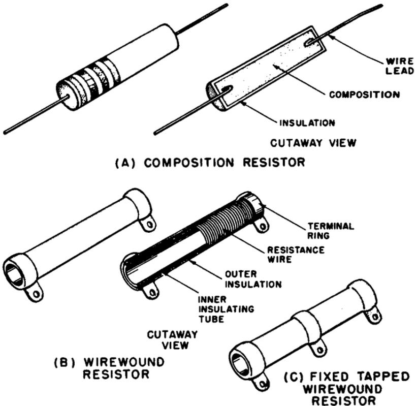
Fig. 1-1. Fixed resistors, appearance and construction. (A) Composition resistor. (B) Wirewound resistor. (C) Tapped wirewound resistor.
