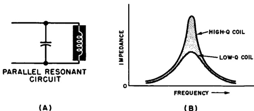
Fig. 5-3. (A) Parallel resonant circuit. (B) Impedance change with frequency.
