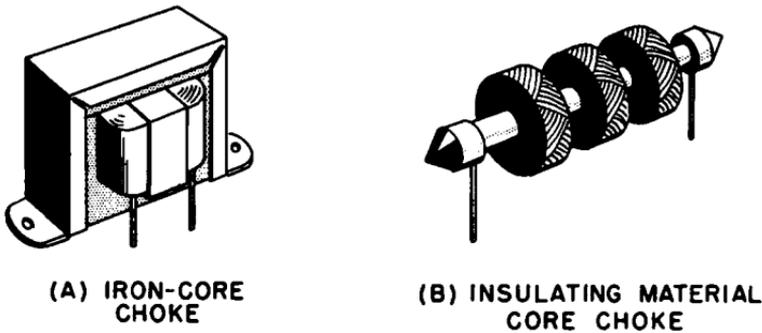
Fig. 5-2. Typical chokes. (A) Iron-core type. Courtesy Standard Transformer Corp.
