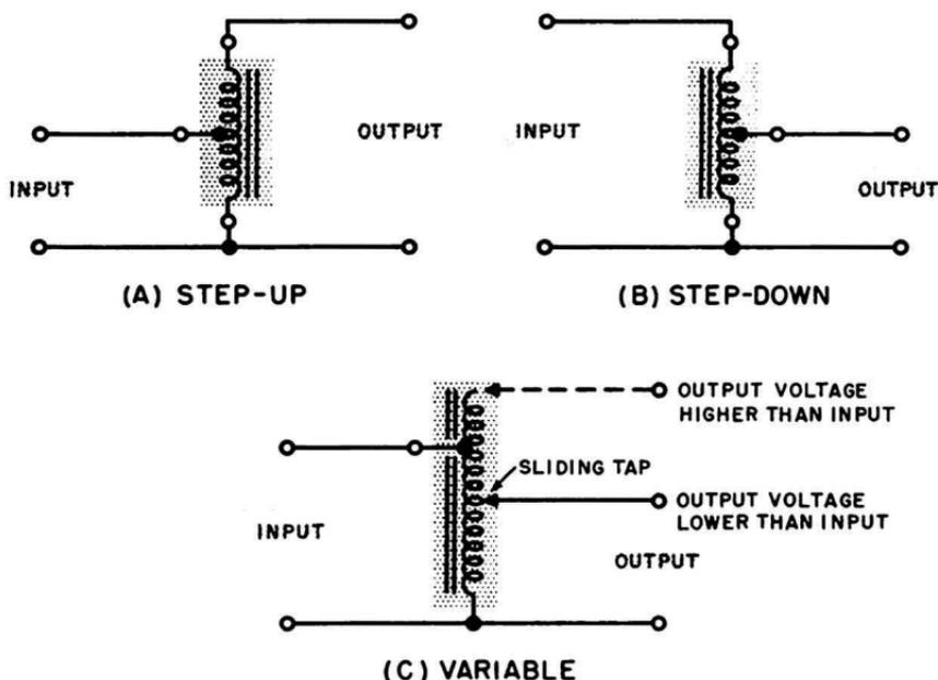
Fig. 6-8. Autotransformers. (A) Step-up. (B) Step-down. (C) Variable.
