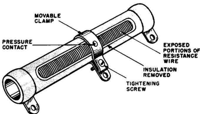
Fig. 1-2. Adjustable resistor.
