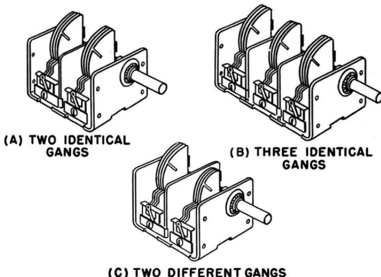
Fig. 4-10. Grounded stator construction. (A) Two identical gangs. (B) Three identical gangs. (C) Two different gangs. After Insuline Corp. of America.
