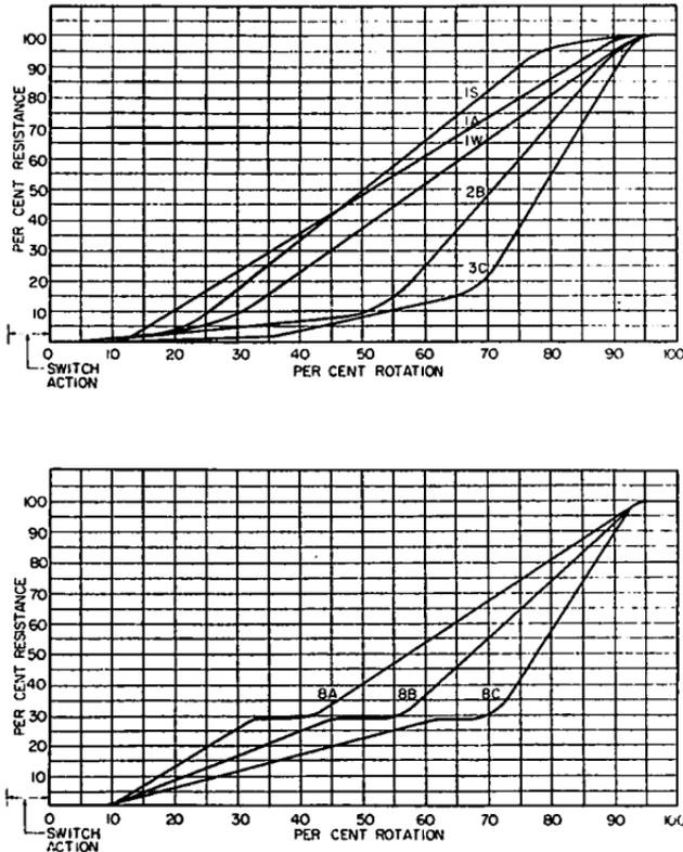
Fig. 2-13. Commercial variable composition resistor taper charts. Courtesy Stackpole Carbon Co.
