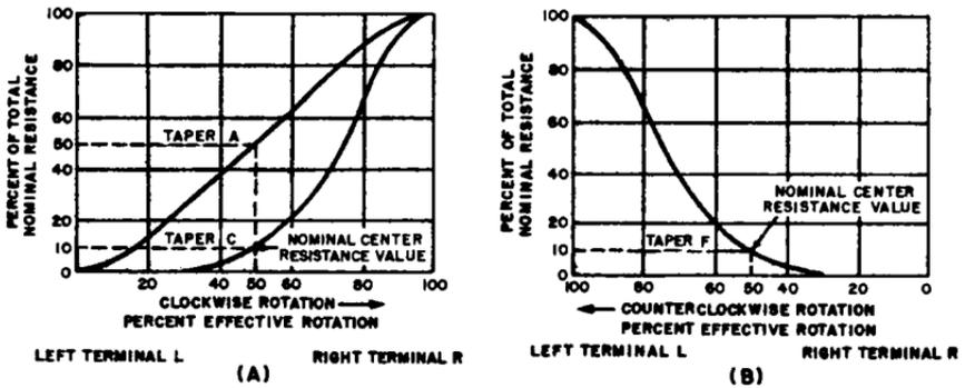
Fig. 2-12. Variable composition resistor tapers. (A) Clockwise tapers A and C. (B) Counterclockwise taper.
