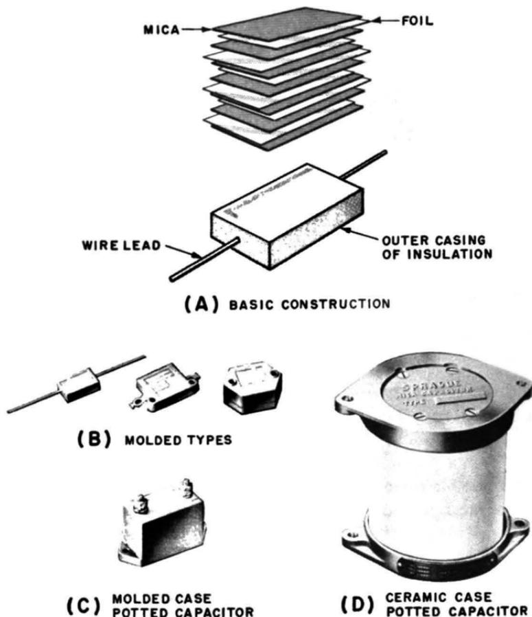
Fig. 4-2. Mica capacitors. (A) Basic construction. (B) Molded types. (C) Molded case potted capacitor. (D) Ceramic case potted capacitor. Courtesy Sprague Electric Co.
