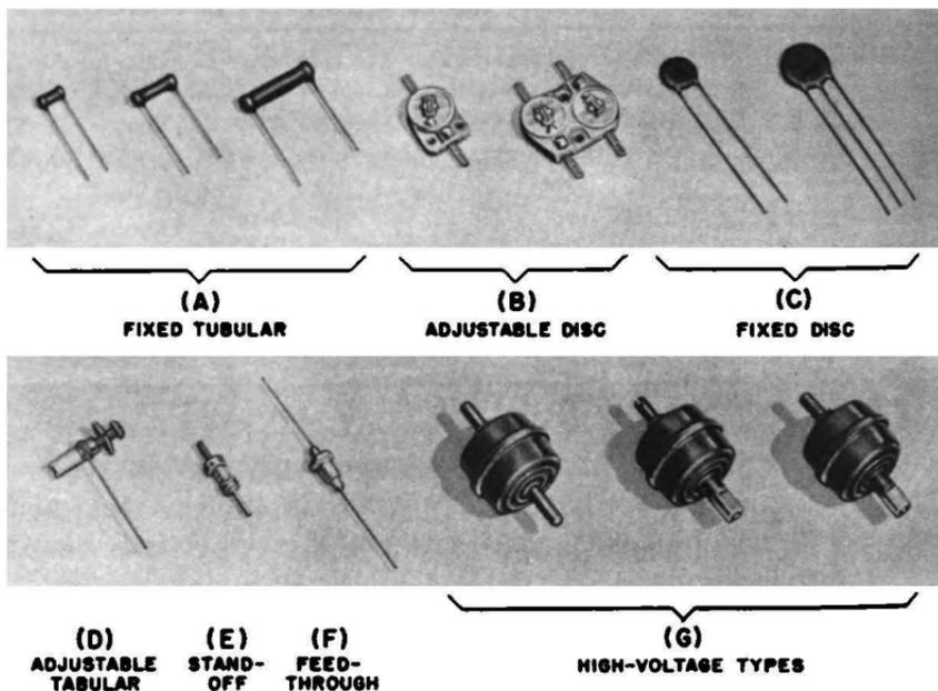
Fig. 4-6. Basic types of ceramic capacitors. (A) Fixed tubular. (B) Adjustable disc. (C) Fixed disc. (D) Adjustable tabular. (E) Stand-off. (F) Feed-through. (G) High Voltage. Courtesy P. R. Mallory & Co., Inc.
