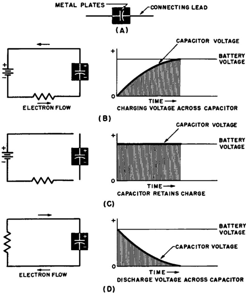
Fig. 3-1. Capacitor characteristics. (A) Basic form. (B) Delay in capacitor charge. (C) Capacitor retains charge. (D) Delay in capacitor discharge.
