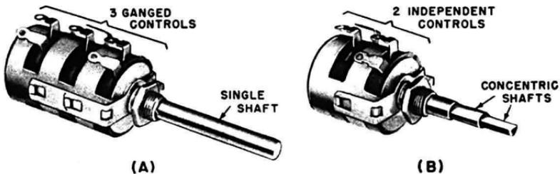
Fig. 2-9. Multiple variable resistor units. (A) Three variables controlled by single shaft. (B) Two independent variables with concentric shafts. Courtesy Clarestat Mfg. Co., Inc.
