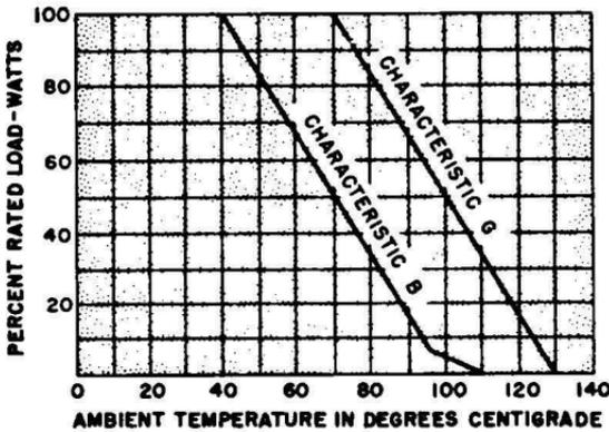
Fig. 1-4. Derating curves for composition resistors. Characteristic B designed for operation below 40° C. Characteristic G designed for operation below 75° C.
