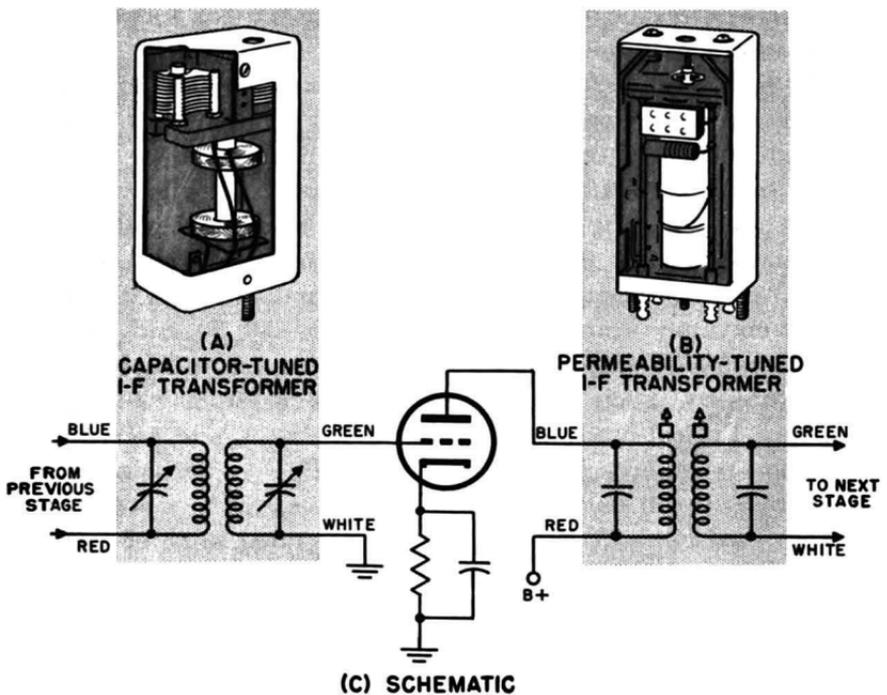
Fig. 6-12. I-f transformers. (A) Capacitor tuned. (B) Permeability tuned. (B) Basic circuits.
