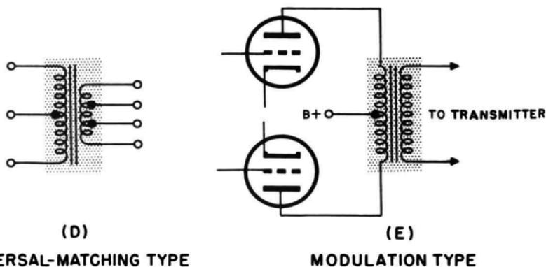
Fig. 6-10. Audio transformers. (A) Input. (B) Interstage. (C) Push-pull interstage and push-pull output. (D) Universal matching. (E) Modulation.
