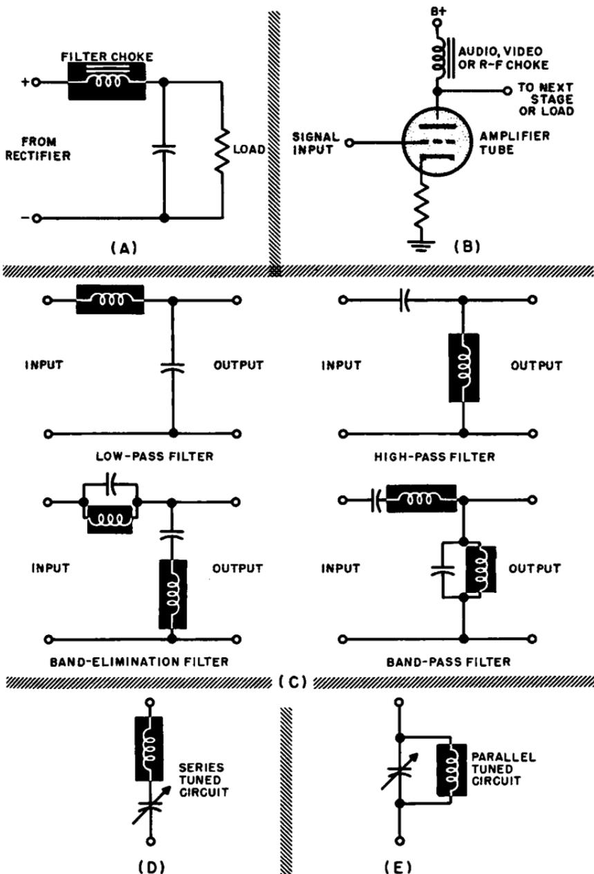
Fig. 6-6. Basic inductor circuits. (A) Filter circuit. (B) Plate-supply choke. (C) Special filter circuits. (D) Series-tuned circuit. (E) Parallel-tuned circuit.
