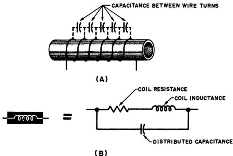
Fig. 5-5. Distributed capacitance effect. (A) Capacitance between turns. (B) Resultant effect of coil resistance and distributed capacitance.
