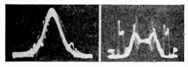
Fig. 295, left, Fig. 295-A, right. On the lower right side of the curve in Fig. 295 may be seen a large peak, which indicates the presence of some undesired frequency that is at zero beat several kilocycles away from the mean frequency. The "ghost" patterns behind the main curve in Fig. 295-A are due to the presence of a harmonic of the frequency modulated i-f. signal in the r-f. amplifier.
