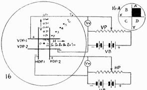
Fig. 16. Applying positive voltages to the plates VDP-1 and HDP-2 by means of the batteries and potentiometers, the beam's spot can be placed ANYWHERE in quadrant A, see Fig. 16-A. The solid spots, 1 to 7, indicate the resultant positions of the beam's spot, when acted upon by the white dots IV to 7V and IH to 7H respectively.
