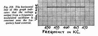
variation in voltage output may exist over the band used, but we shall assume for our discussion that the voltage output is of constant amplitude. The selection of the 450 kc. to 470 kc. band is purely illustrative. We assume that similar conditions prevail over any band width both sides of any periodic or mean frequency. It should be realized that a departure from such linearity of output will distort the final resonance curve.
