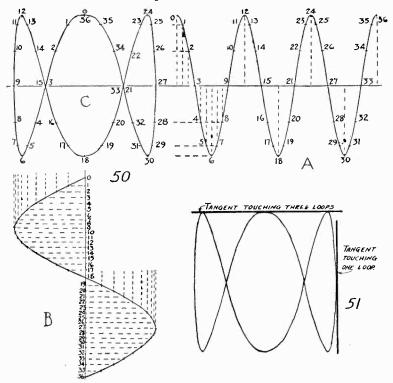
Fig. 50. The sine wave at A is three times the frequency of that at B and is 90° out of phase. Both waves are divided into equal time intervals. The numbers on the resultant image at C indicate the amplitude displacement of each wave at the same instant.
