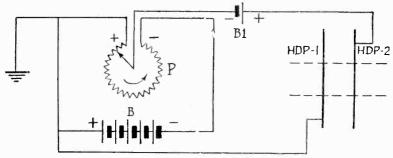
Fig. 29. An electro-mechanical equivalent of the sweep circuit used in several oscillographs. The normal position of the spot is at one side of the screen on the X axis instead of ct the center.
