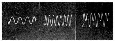
Figs. 160, left, 161, middle, 162, right. The 400-cycle wave of Fig. 160 has an amplitude smaller than its second harmonic, 800 cycles, Fig. 161, and a greater dip can be readily noted in the composite wave of Fig. 162 than those composite waves shown in earlier illustrations.
