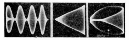
Figs. 393, left, 394, middle, 395, right. The three oscillograms were made with 100 percent. modulation. The pattern of Fig. 395 differs from that of Fig. 394 because of phase shift.
