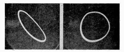
Fig. 95. C, left, D, right. Each pattern indicates a 1-1 ratio. The phase difference in C is about 45° and that in D is about 90°.
