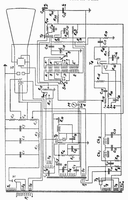
Fig. 279. Schematic diagram of the Egert Model VRO oscillograph.
