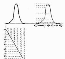
Fig. 53. The sweep frequency is such that one cycle occurs during the time that the oscillator's frequency varies from 455 to 485 kc. The tuned circuit to which this band of frequencies is applied is resonant at 470 kc. The frequency response curve taken across the detector load appears at the right and its image, as seen on the screen is at the left, above the sweep.
