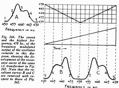
mum peaks have been transposed from the outside to the inside of the curves and the two smaller peaks have been transposed from the inside to the outside of the curves. Curve B in figure 263 is like curve C in figure 264, because the direction of the frequency sweep is the same. A similar situation exists with respect to curve C in figure 263 and curve B in figure 264.
