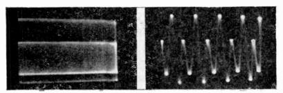
Fig. 241, left, Fig. 242, right. The light and dark streaks of the pattern in Fig. 241 indicate that the unmodulated carrier, which was 90 kc., was distorted. When the sweep frequency was increased, so that only a few cycles of this 90-kc. carrier appeared on the screen, the waveform in Fig. 242 showed the distortion that the solid pattern indicated.
