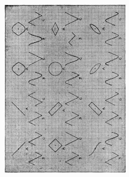
Fig. 49. In each case A is the resultant image that will appear upon the screen when the wave at B is impressed on the vertical deflecting plates and the wave at C on the horizontal plates. These waves are of equal amplitude and have the same frequency.
