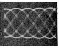
Fig. 69, left, Fig. 70, right. Two examples of patterns that are under-synchronized. The fine lines in Fig. 69 can be seen to follow the usual outline of a sine wave. This can be readily seen in Fig. 70.
