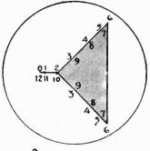
Fig. 386-D. The effect of over modulation of the modulated signal can be seen in the pattern developed. The sweep voltage is in phase with the modulated signal in this instance.
