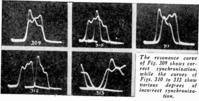
As far as timing frequency (linear sweep) is concerned, the adjustment is correct as indicated by the pattern. The adjustment of the circuit trimmers for symmetrical response is another matter. The same pattern, with the synchronizing voltage control advanced too far, is shown in figure 310. The same pattern, with the linear sweep frequency slightly higher than the frequency of the frequency modulating condenser rotor, is shown in figure 313.
