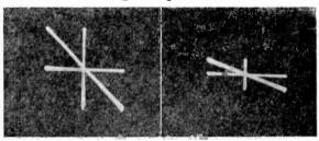
Fig. 93-C, left, Fig. 93-D, right. A phase difference of O° exists between the two voltages. In C equal amplitudes on both axes give the pattern a 45° angle with the horizontal, but when the horizon-
