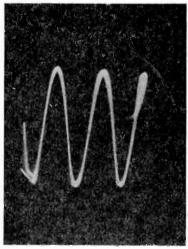
Fig. 83, left, Fig. 84, right. The vertical amplitude in Fig. 83 is correct for observation of the waveshape. The same wave was photographed for Fig. 84, but the vertical deflection plate voltage was increased to such an extent that one peak of the wave is blurred as it touches the rounded portion of the screen.
