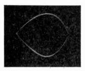
Fig. 73. The image resulting when the sweep frequency is twice the frequency of the wave being observed. Compare Fig. 27. Such a pattern is difficult to stop on the screen, as the points are moving on the fastest portion of the cycle. The top and bottom halves of the wave should coincide.
