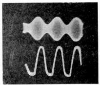
the fact that the i-f. wave envelope is satisfactory and that the rectified signal should be the original sine wave fed into the input of the receiver in the form of a modulated carrier. The distorted diode output is shown as the lower photograph.
