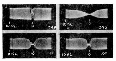
Figs. 349 to 352. These four oscillograms show the effects on the response curve of changing the blocking condenser in a resistance coupled amplifier.
