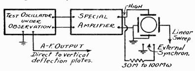
Fig. 224. Circuit used for checking the modulated and unmodulated carrier outputs and the a-f. output of a test oscillator.
