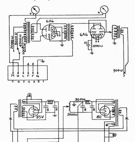
trolled, with a buffer stage and power amplifier. The modulator system employs a class A stage and a class B stage.
