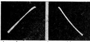
Fig. 95. A, left, B, right. Both patterns show a 1-1 ratio between the frequencies. The phase difference in A is 180° and that in B is 0°.
