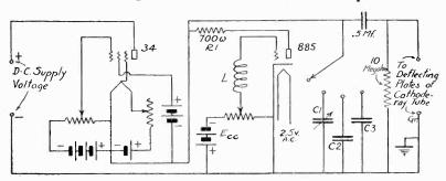
Fig. 38. The type 34 tube replaces the resistor, R, (Fig. 34) as a current limiting device in this relaxation oscillator sweep circuit. The constant current flow tends to charge whatever condenser is in the circuit at a constant rate, making the voltage rise constant thereby supplying a linear output to the deflecting plates.
