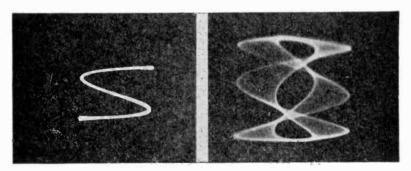
Fig. 97. G, left, H, right. The 3-1 pattern of G was made when the voltages had a phase difference of 180°. In H one of the voltages was modulated.
