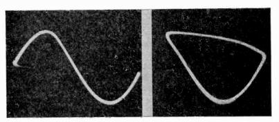
Fig. 79, left, Fig. 80, right. The proper amount of synchronizing voltage was applied to get the single cycle of Fig. 79. When the maximum amount of synchronizing voltage was applied, the distorted figure of Fig. 80 resulted.
