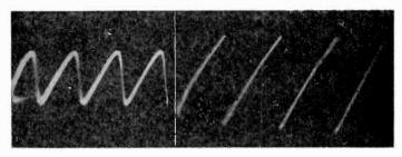
Fig. 35 (left) shows the output waveform of a sweep circuit of a commercial oscillograph with a low tripping voltage, making the charging portion of the wave fairly linear. Fig. 36 (right) shows the same wave with the amplitude control advanced, resulting in a slight departure from the good linearity of the wave of Fig. 35.
