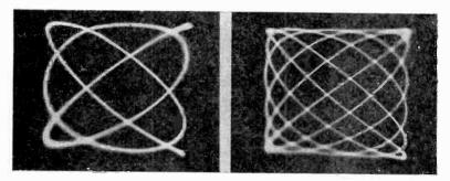
Fig. 104. A, left, B, right. Both patterns were made with a 6-5 ratio. The one shown in A was photographed when the loops were "closed" and that in B when the loops were "open."
