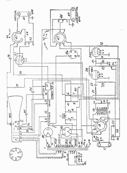
Fig. 62. Above is the schematic diagram of the Clough Brengle Model CRA oscillograph. The tube complement is as follows: Type 906 cathode-ray tube with 3-inch screen; 81 rectifier for the anode of the cathode-ray tube various control voltages; 80 rectifier for supplying the amplifier voltages; 85 tube as the timing axis voltage oscillator; type 2A5 as the timing axis voltage amplifier and a type 57 for amplifying the voltage fed to the vertical deflecting plates.
