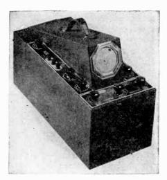
accompanying illustration, are the following: focus, intensity, vertical selector switch (providing a 60-cycle, direct, or through amplifier connection to the vertical plates), internal-external synchronizing switch, locking control, step and vernier sweep-frequency controls, horizontal gain, vertical gain, and horizontal selector switch. The schematic is shown in the accompanying figure.
