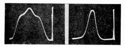
Fig. 276, left, Fig. 277 right. The resonance curve in Fig. 276 is non-symmetrical and that in Fig. 271 is symmetrical. These oscillograms were made using the frequency modulator and sweep described in Fig. 275. The vertical line on the right of each oscillogram indicates the vertical displacement due to change in frequency, but as the sweep was shorted, it is not spread across the screen.
