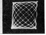
Fig. 111. A, left, B, right. The pattern in A is an 8-3 ratio and that in B is 8-7 ratio.
