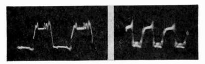
Figs. 374, left, 375, right. The effect of maximum and minimum separation between the secondary contacts is shown in Figs. 374 and 375 respectively. that shown in figure 377. The output voltage also dropped from a normal of about 245 volts to about 150 volts. This is the voltage measured across the 5000-ohm load.
