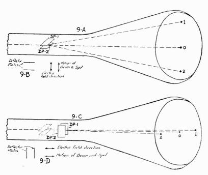
Fig. 9A shows the pair of deflecting plates that cause the electron beam to move vertically and Fig. 9C, the plates that are responsible for the horizontal movement. Figs. 9B and 9D show the direction of the electric fields and the motions of the beam for each of the two pairs of plates.
