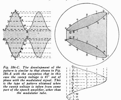
but is sinusoidal, does not interfere with a linear pattern as long as the amplitude variation of the modulated signal occurs at the same rate and is of identical shape and correct phase. Provided the modulation is linear, any complex modulating wave will produce a perfect trapezoid.
