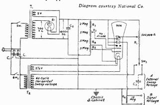
trols are mounted upon the front of the housing and upon the right side. The spot intensity and spot focusing controls are mounted upon the front panel; also the power supply switch. The horizontal and vertical deflection plate connection posts are mounted on the side; also the potentiometer controlling the amplitude of the voltage supplied to the horizontal plates. The unit is equipped with a 60-cycle
