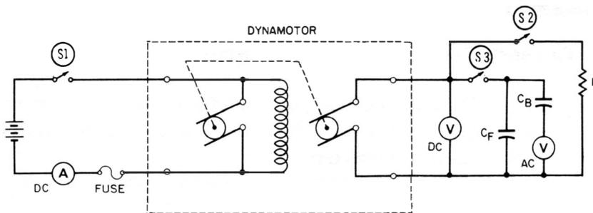
Fig. 76. Test setup for checking a dynamotor.
