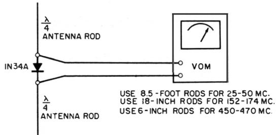
*Evaluation of Results:* This arrangement gives a relative field-strength indication, which must be observed with respect to a reference reading corresponding to the normal field strength.
