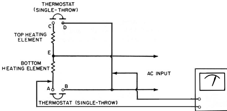
**Fig. 10. Wiring diagram of a two-element water heater.**
