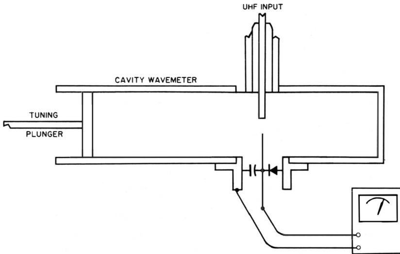
**Fig. 45.** DC voltmeter as an indicator for a cavity wavemeter.
