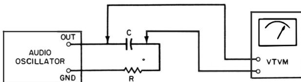
**Fig. 50. Voltage measurement across C is often in error, because of VTVM "ground" capacitance.**
