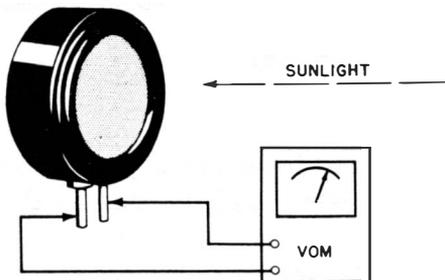
**Fig. 101.** Testing the condition of a photovoltaic cell.
