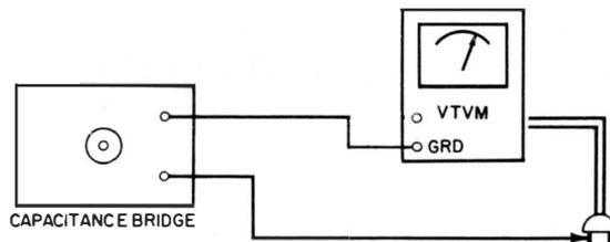
**Fig. 49. Measuring the input capacitance to the ground terminal of a VTVM.**
