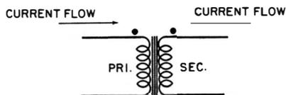
**Fig. 96. Meaning of polarity markings on AC devices.**
