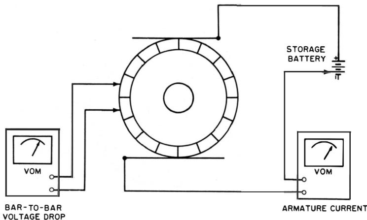
Fig. 28. DC check for shorted turns in an armature coil.
