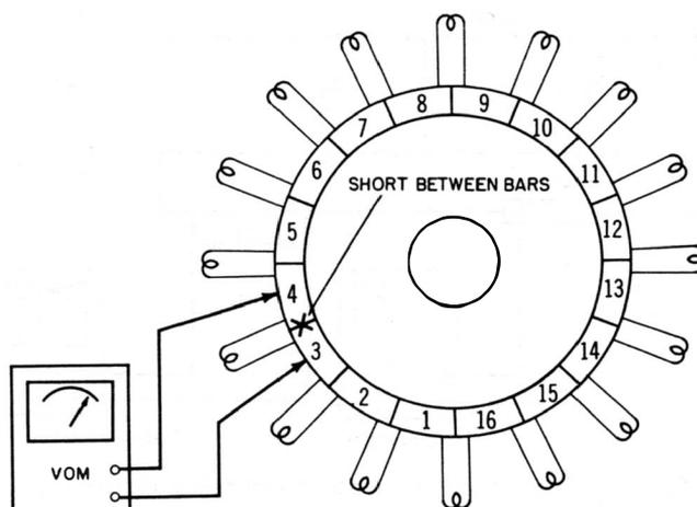
**Fig. 39. Localizing a short between bars.**
