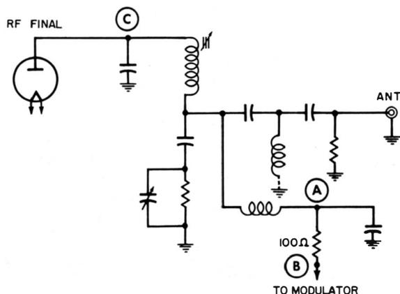
**Fig. 72. Measurements of DC voltages from A to B, and at C indicate power input.**
