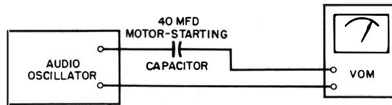
**Fig. 56. Determination of scale factor for the output function of the VOM.**
