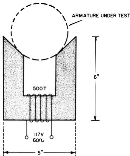
**Fig. 31. Plan of laminated core and winding for growler.**
