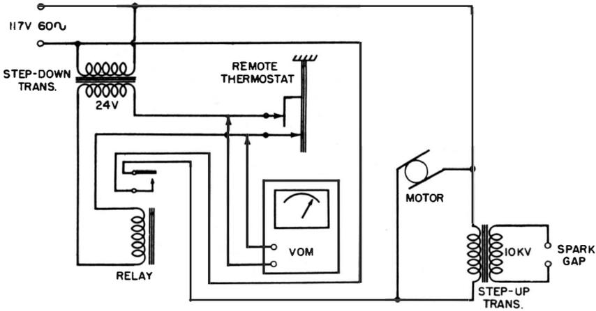
**Fig. 3. Basic configuration of an oil-burner electrical system.**
