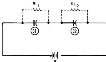
will fail is very great. To insure that such a series connection is valid, check each capacitor at its intended working voltage and get a sensitive test of insulation resistance by feeding the small leakage current into a VTVM, which can be oper-
