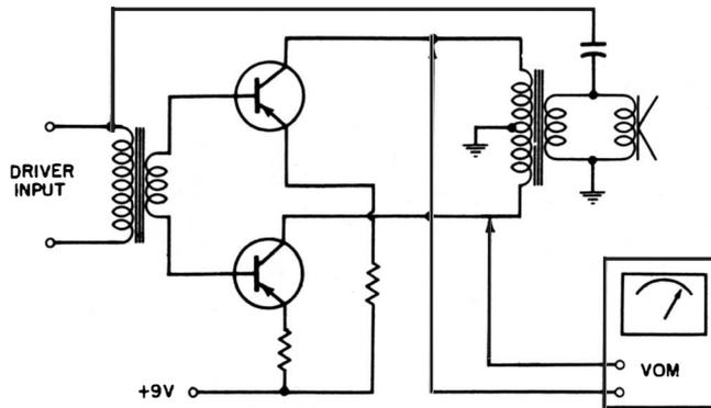
**Fig. 69.** Checking a transistorized audio-output stage for correct balance.
