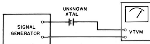
*Evaluation of Results:* The frequency indicated on the generator dial is the same as the resonant frequency of the crystal, within the accuracy of the generator.
