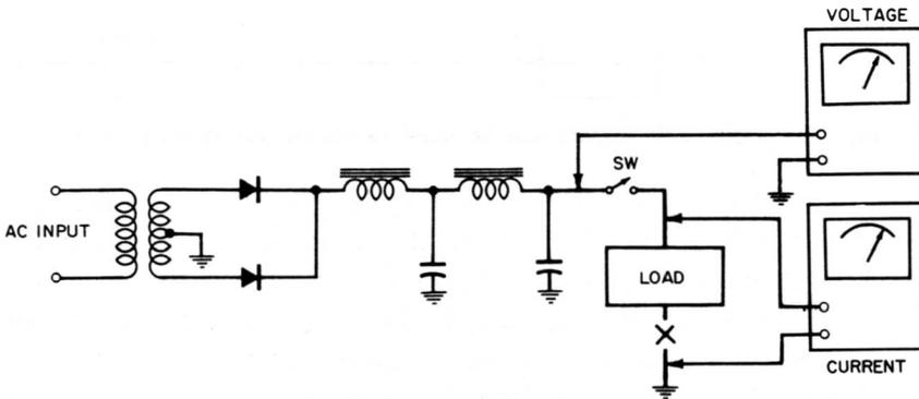
**Fig. 80. Determining the internal resistance of a power supply.**
