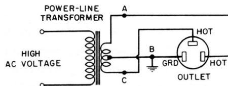
**Fig. 22.** Wiring diagram of a 3-wire, 220-volt supply.
