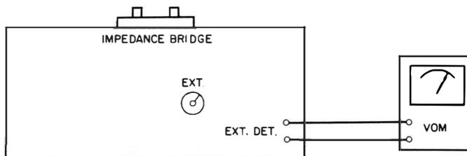
**Fig. 44. Test setup of impedance bridge and VOM.**
