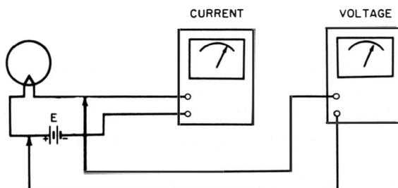
**Fig. 85. Determination of hot-resistance value.**
