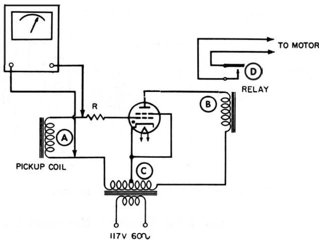
**Fig. 2. Circuit of a thyatron door-opener control.**
