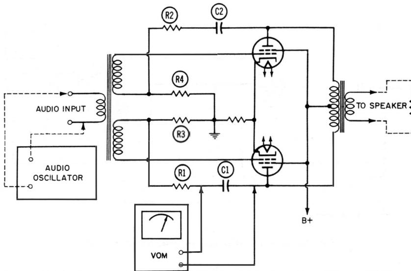
**Fig. 67. Checking the feedback branches in a push-pull output stage.**
