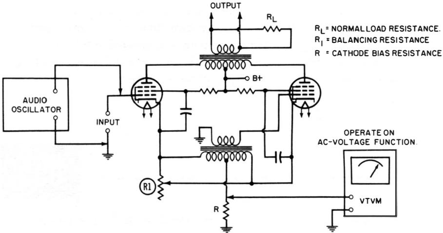
**Fig. 66. Adjusting a cathamplifier for balance.**
