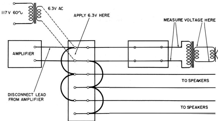
**Fig. 81.** A 60-cycle signal can be used to check out speaker lines.
