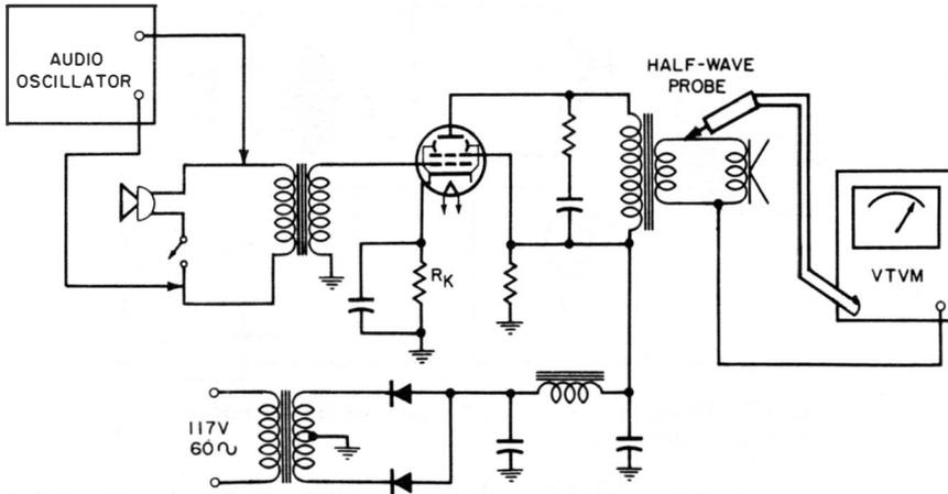
**Fig. 70. Simple one-stage paging amplifier.**
