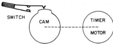
**Fig. 16. Time-control cam and switch.**
