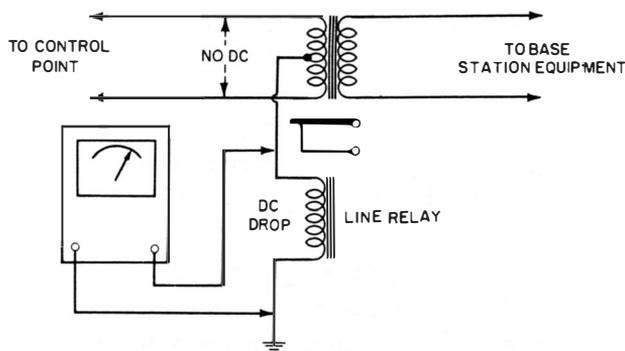
Fig. 75. Control-voltage check at line relay.
