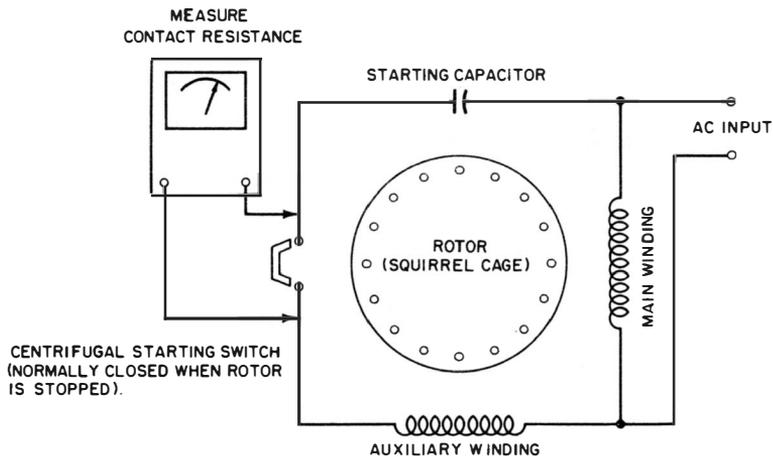
**Fig. 18. Motor will not start when switch contacts do not close.**
