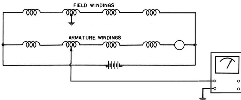
**Fig. 35. False null occurs in this configuration when localizing a ground.**
