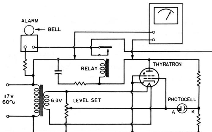
**Fig. 117. Typical hookup for a simple burglar alarm using a photoelectric cell.**
