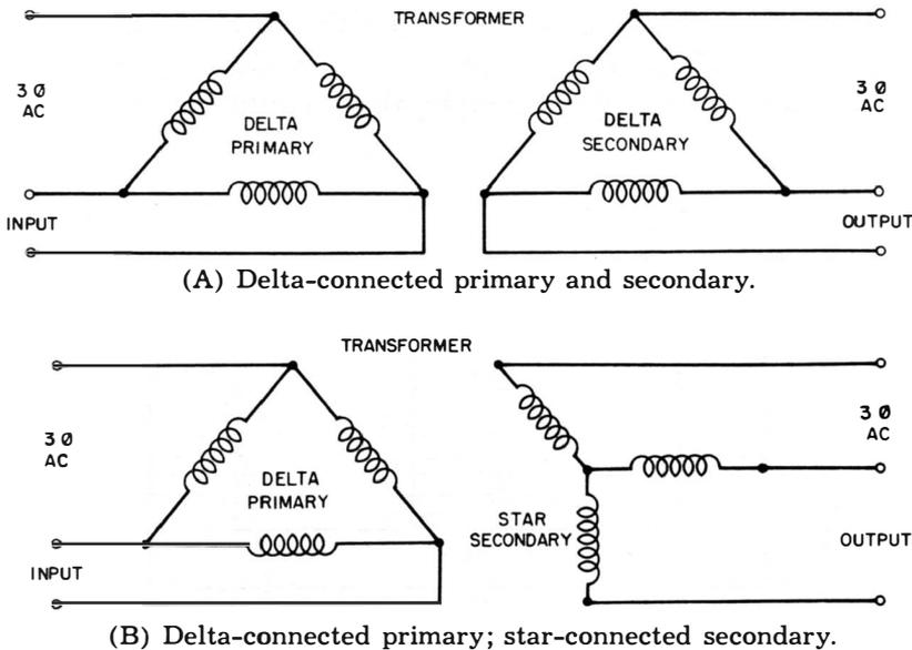
**Fig. 111. Changing primary connections from delta to star lowers the output line voltage to 0.58 of its initial value.**
