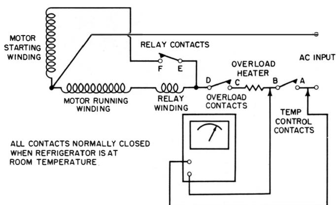
**Fig. 19.** Wiring diagram of a refrigerator motor circuit.
