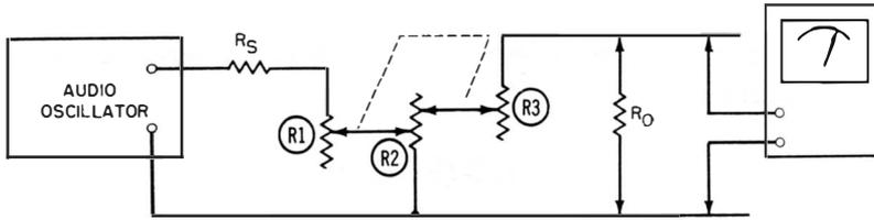
**Fig. 62. Checking a T-pad for reactive response.**
