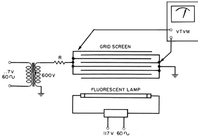
**Fig. 114. Typical hookup for an insect electrocutor.**
