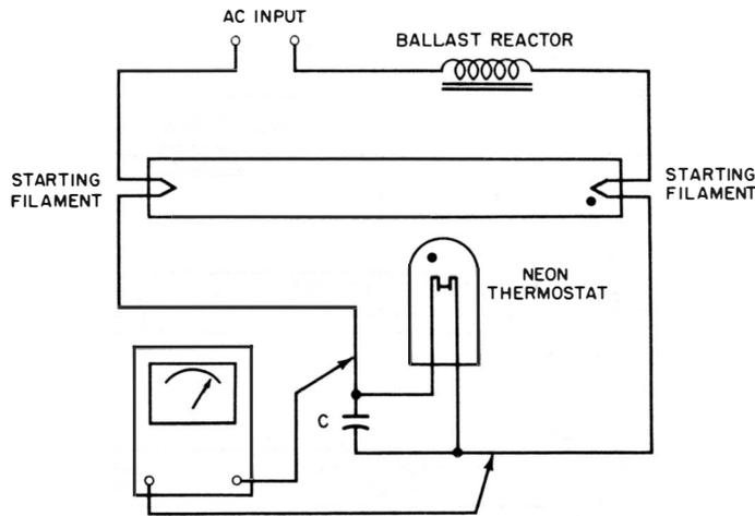
**Fig. 13. Fluorescent lamp will not start if thermostat contacts do not close.**
