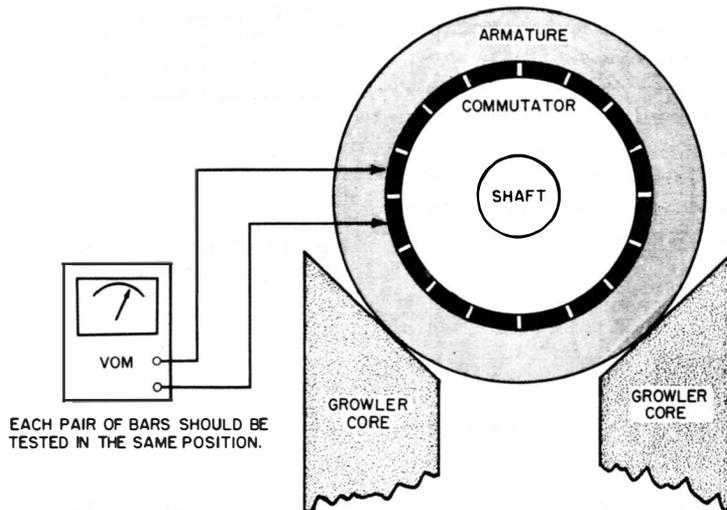
**Fig. 30. Test position for armature.**
