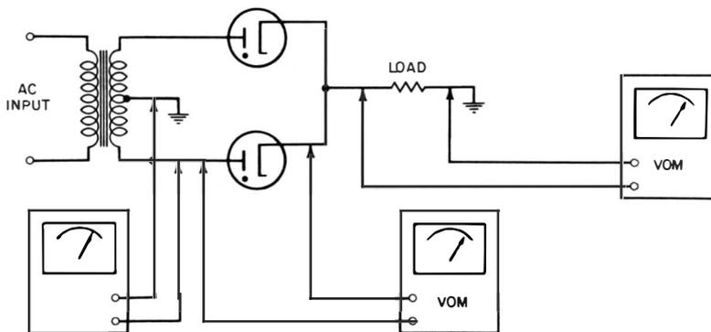
**Fig. 103. Measurement of average DC voltages.**
