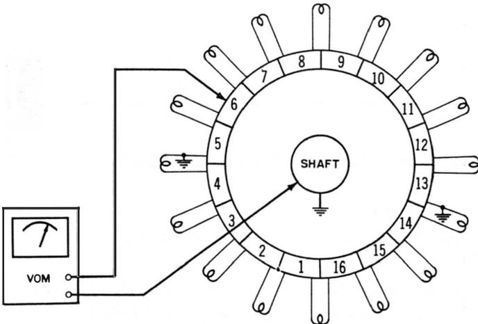
**Fig. 34. Localizing two grounded coils.**
