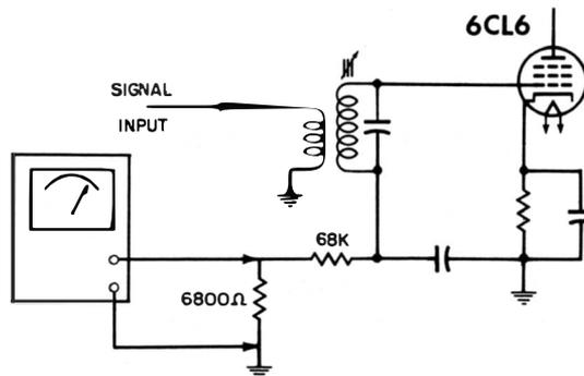
**Fig. 82. Checking grid drive to a transmitter tripler.**
