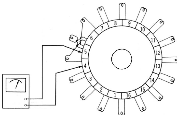
**Fig. 36. Reversed coils on rewound armature.**
