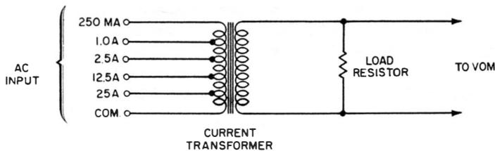
**Fig. 26. Current transformer and load resistor converts VOM to AC ammeter.**
