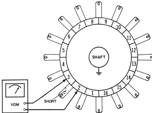
**Fig. 32. Checking for short circuit in a coil.**
