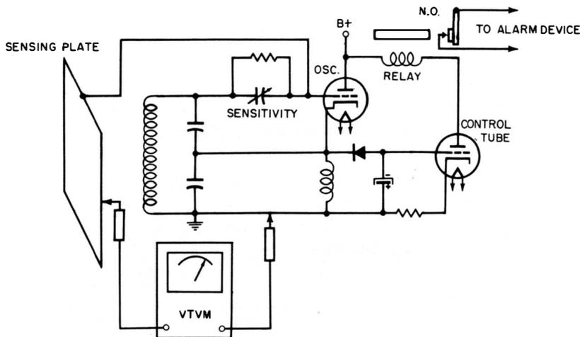
**Fig. 116. Test setup of a proximity-type burglar alarm.**
