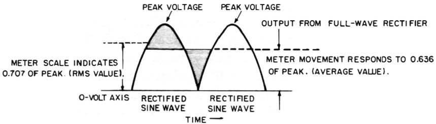
**Fig. 58. If the VOM has a full-wave instrument rectifier, this current waveform flows through the meter movement.**
