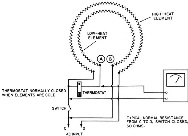
**Fig. 7. Wiring diagram of a two-heat coffee maker.**
