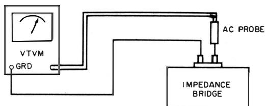
**Fig. 48. Measuring the input capacitance of a VTVM on its AC-voltage function.**
