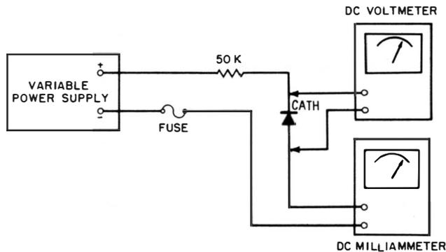
**Fig. 91.** Test setup to measure negative resistance.
