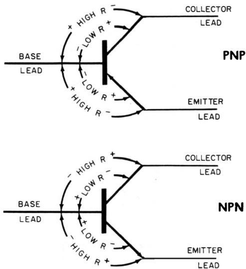
**Fig. 98. Comparative ohmmeter readings for low-power PNP and NPN transistors.**
