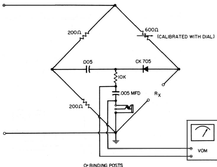
**Fig. 43. Typical antenna Z-meter circuit.**
