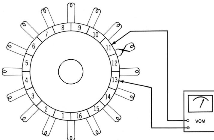
**Fig. 37. Meter indicates reversed coil connections.**
