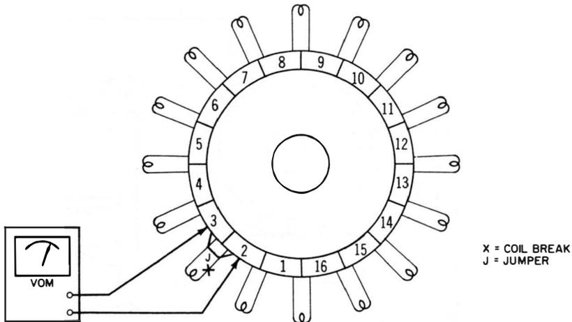
**Fig. 29. Checking for open coil, and temporary repair.**
