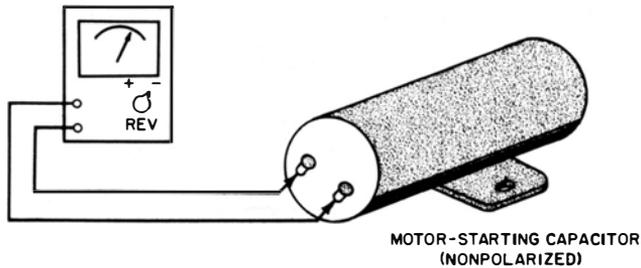
**Fig. 24. Checking a motor-starting capacitor.**
