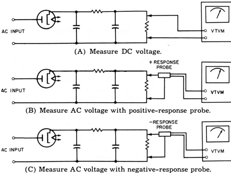
**Fig. 106. Finding the crest and trough values of a pulsating DC voltage.**
