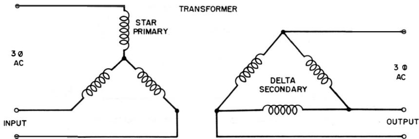
(B) Star-connected primary; delta-connected secondary.
