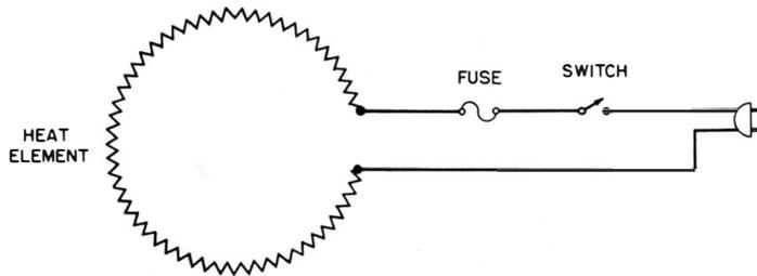
**Fig. 8. Wiring diagram of a simple percolator.**
