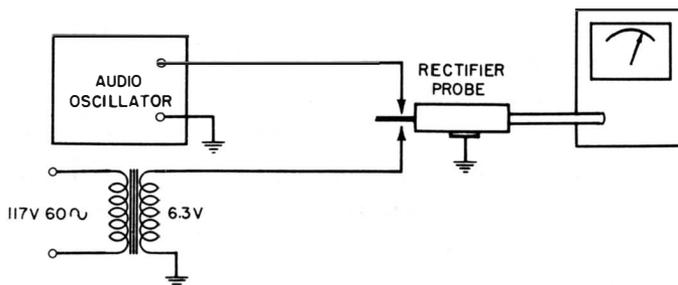
**Fig. 52. Setup used to check the calibration of an audio oscillator at 60 cycles.**
