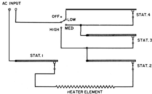
Fig. 4. Wiring diagram of a heating pad.
