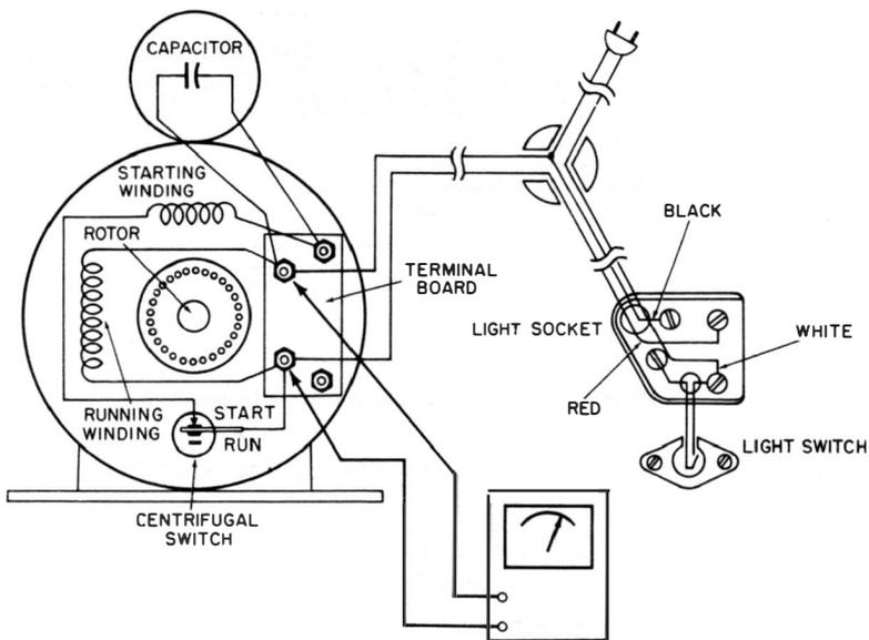
**Fig. 17. Checking applied voltage at refrigerator motor.**
