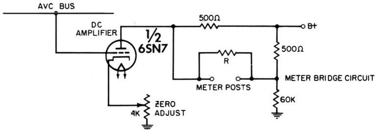
**Fig. 41.** Arrangement for using the VOM as an S meter.
