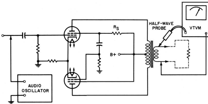
Fig. 68. Circuit of a screen-grid phase splitter.
