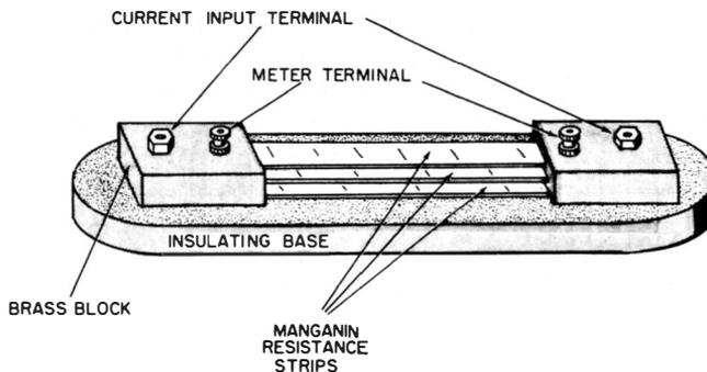
**Fig. 27. Typical current shunt for a voltmeter.**
