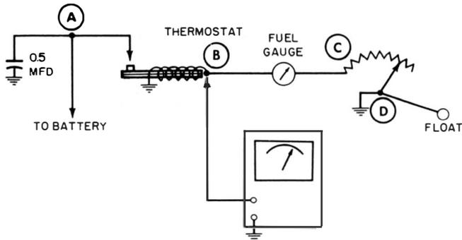
**Fig. 115. Typical fuel-gauge hookup.**
