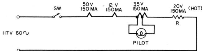
**Fig. 86. Globar resistor must be checked hot.**
