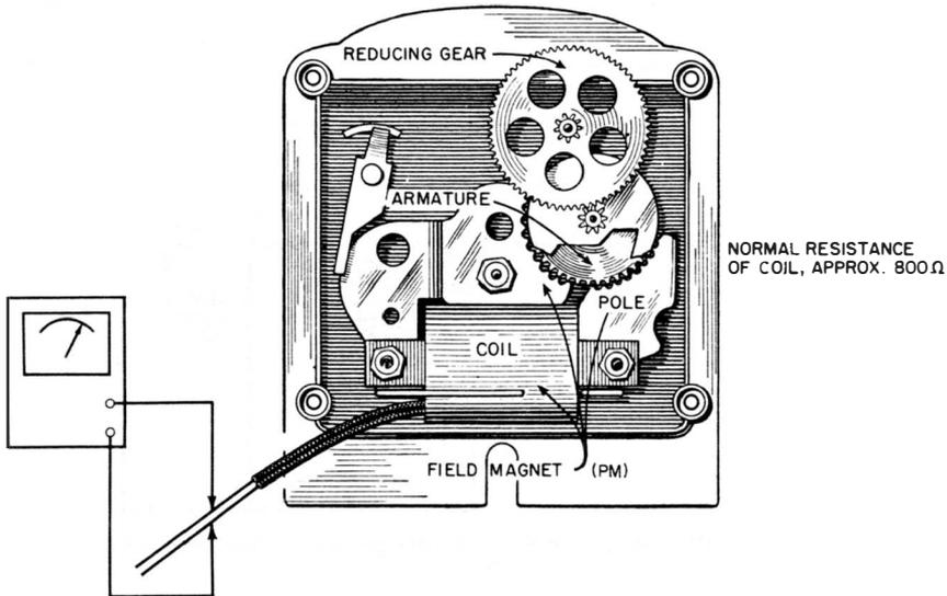
**Fig. 20.** Configuration of a synchronous motor in an electric clock.
