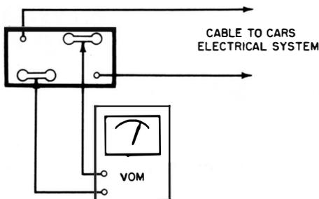
**Fig. 84.** Battery cells can be checked while engine is cranking.
