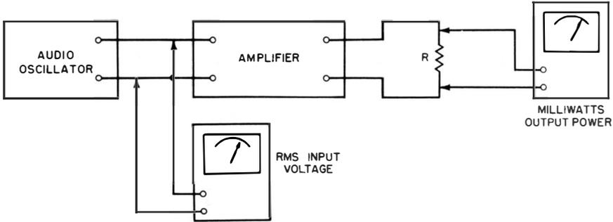
**Fig. 64. Test setup to determine the sensitivity of an amplifier.**
