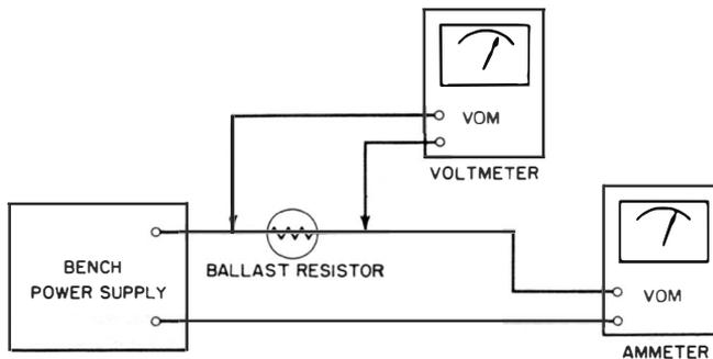
**Fig. 92.** Test setup for checking the characteristic of a ballast resistor.
