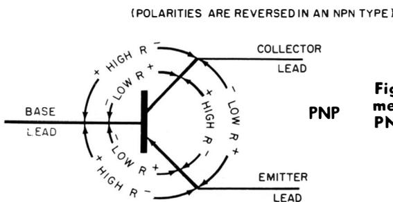
**Fig. 99. Comparative ohmmeter readings for high-power PNP and NPN transistors.**
