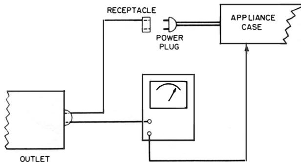
**Fig. 25. Checking an appliance for insulation resistance at line voltage.**
