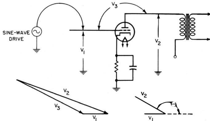
**Fig. 108. Finding the phase angle between two AC voltages.**
