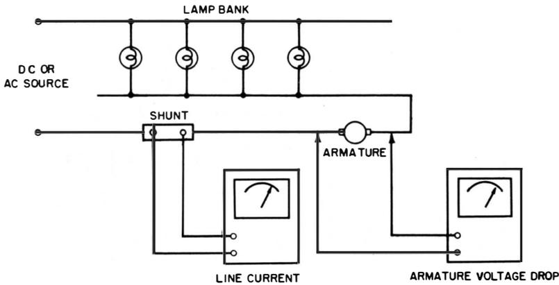
**Fig. 38. Test setup to measure armature resistance.**
