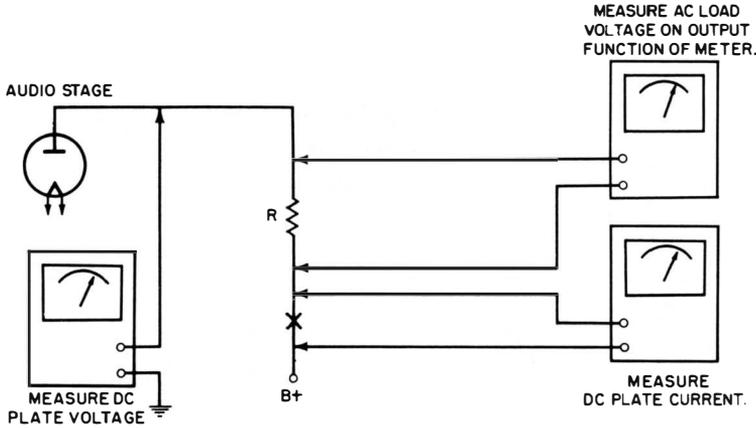
**Fig. 73. Checking plate efficiency of an amplifier.**
