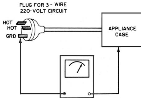
**Fig. 21.** Checking the ground circuit of an appliance.
