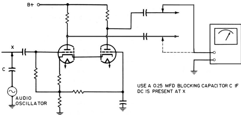
**Fig. 65. Checking a Schmitt phase inverter for balance.**
