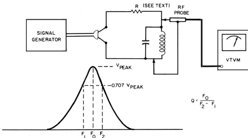
**Fig. 89.** Test setup for measuring the Q of a tuned circuit.
