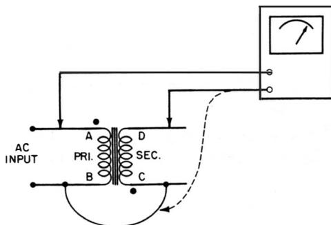
**Fig. 95. Checking polarity markings on AC devices.**
