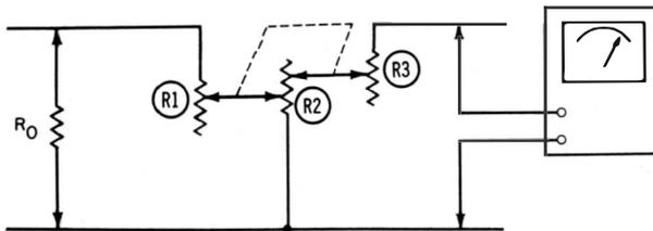
**Fig. 61.** To check the output impedance of a T-pad.
