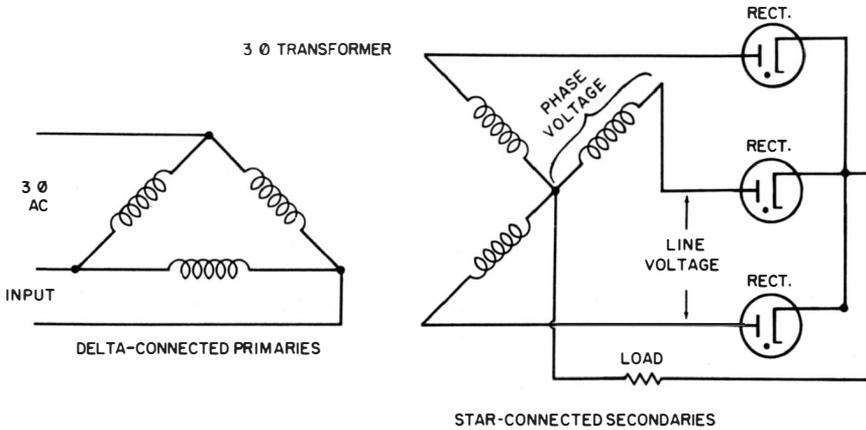
**Fig. 109. Points of phase- and line-voltage measurements.**
