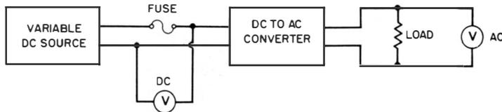
NOTE: THE SAME VOM OR VTVM CAN BE USED FOR BOTH MEASUREMENTS.
