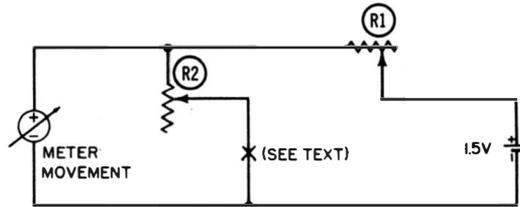
**Fig. 55. Determination of the internal resistance of a meter movement.**
