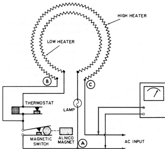
MAGNETIC SWITCH CONTACTS NORMALLY CLOSED AT START OF CYCLE, THEN OPEN AT END OF HIGH-HEAT CYCLE.
