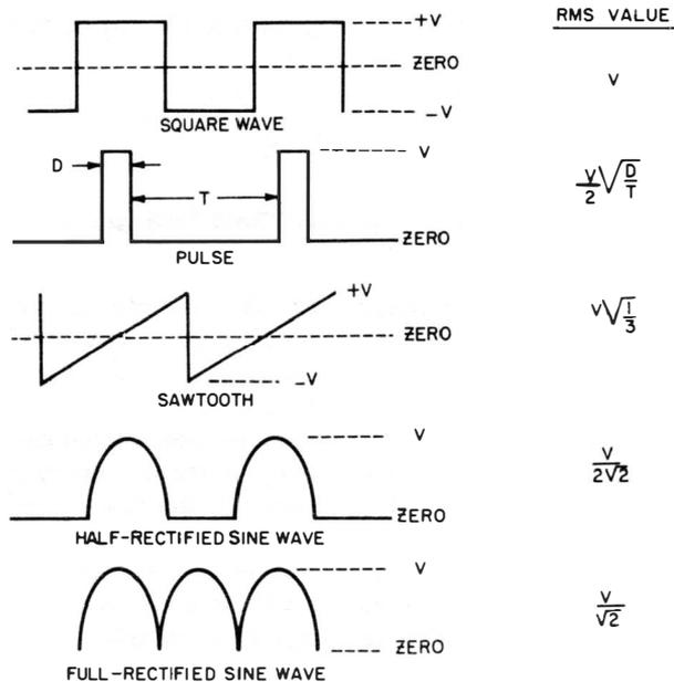
**Fig. 59. RMS values of common waveforms.**
