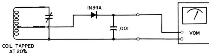
**Fig. 40. RF meter configuration.**
