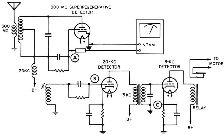
Fig. 1. Typical receiver for a door opener.
