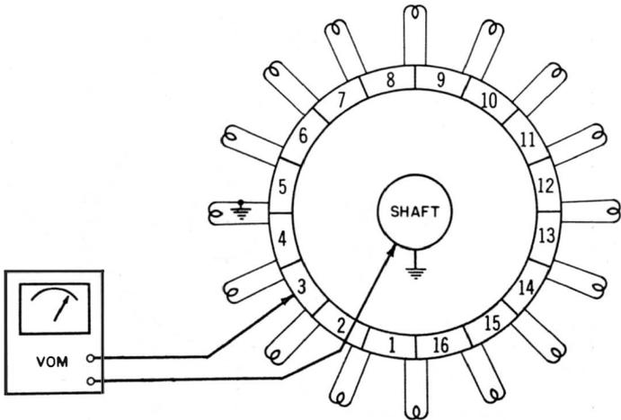
**Fig. 33. Checking for a grounded coil.**
