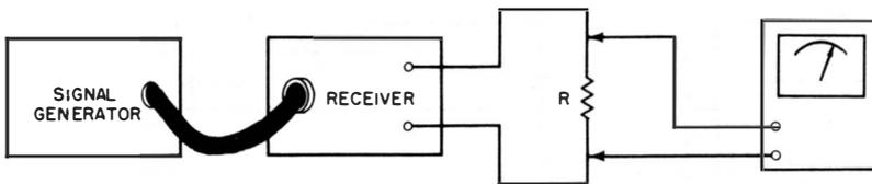
Fig. 74. Measuring the sensitivity of a receiver.
