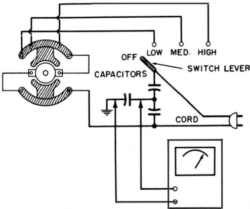
**Fig. 23.** Checking capacitors in an electric mixer.
