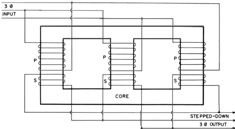
**Fig. 110. Plan of a three-phase transformer.**
