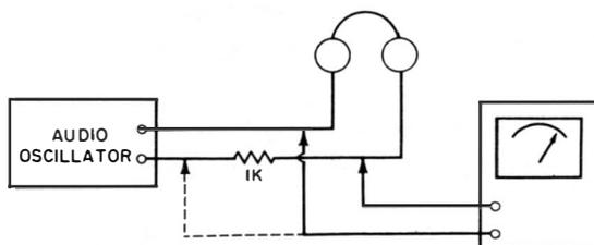
**Fig. 118. Measuring ear-phone impedance.**
