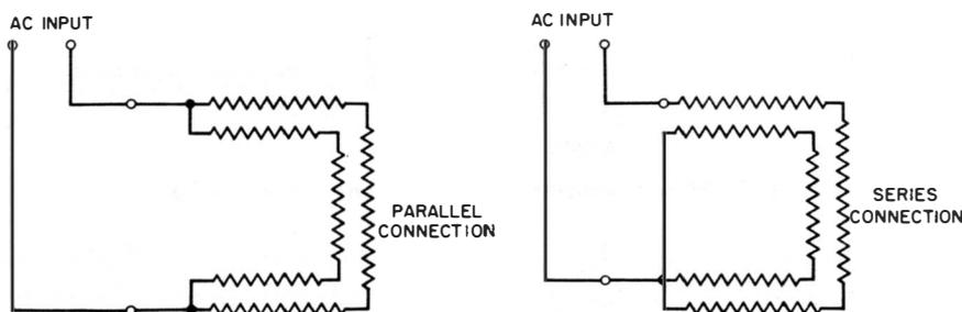
**Fig. 6. Series connection of heater elements develops 25% of heat developed by parallel connection.**
