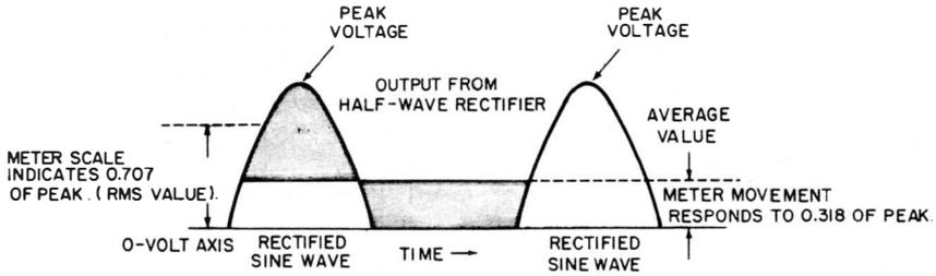
**Fig. 57. An ordinary VOM has this current waveform flowing through the movement of the meter.**
