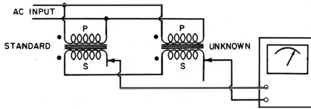
**Fig. 97. Determining consistency of polarity markings.**
