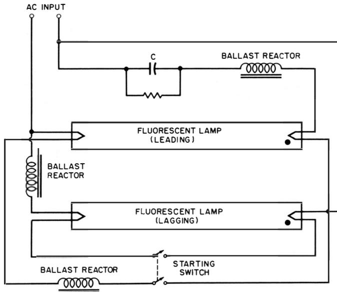
**Fig. 14. A shorted lead capacitor will result in strobe flicker in a dual fluorescent lamp.**
