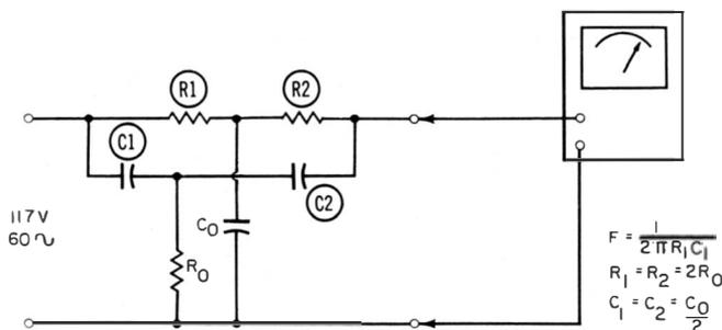
**Fig. 113. Checking line voltage for harmonics.**
