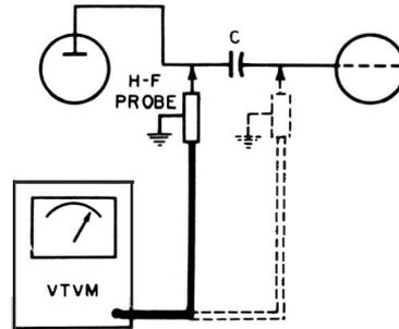
of the capacitor are above AC ground. The ground terminal of the VTVM has appreciable input capacitance (typically 250 mmf) which will often load an above-ground point excessively.
