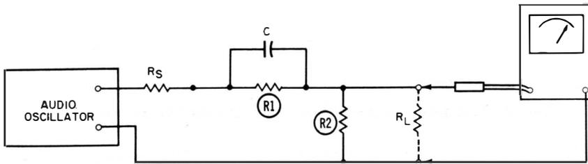
**Fig. 63.** Test setup to check the frequency characteristic of an equalizer.
