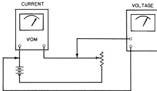
**Fig. 54. Determining the internal resistance of a milliammeter or ammeter.**
