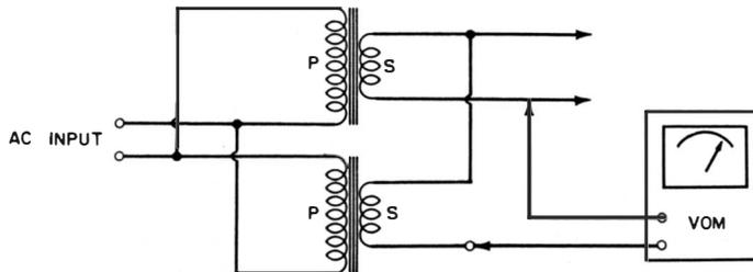
**Fig. 94. Checking transformer phase for safe parallel connection of the windings.**
