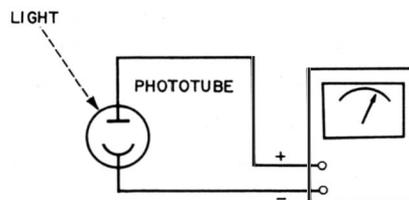
*Evaluation of Results:* A phototube does not convert light energy into electricity, but develops a finite plate resistance when exposed to light. This plate resistance can be measured with an ohmmeter, which, incidentally, applies an accelerating voltage between cathode and anode. Since the applied voltage is comparatively low, the normal plate resistance may not be available in tube data and it may be necessary to make a comparison test against a good tube of the same type.
