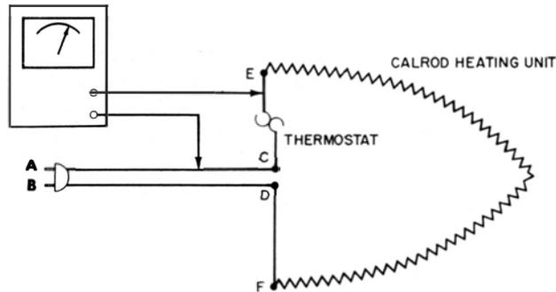
Fig. 11. Wiring diagram of an electric iron.
