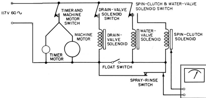
Fig. 15. Wiring diagram of an automatic washer.
