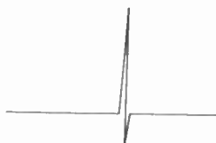
Normal appearance of a pulse voltage on base line.
