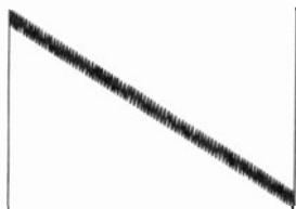
Display at 60-cycle horizontal sweep in scope.
