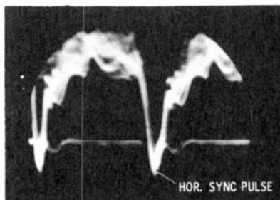
Video signal waveform from a TV station.
