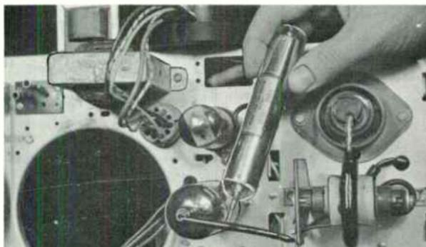
**Checking for presence of horizontal-output voltage.**
