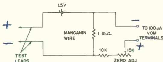
Circuit for a VOM low-ohms probe.
