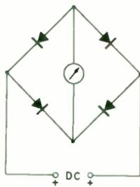
**The basic full-wave bridge rectifier circuit.**
