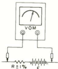
**(A) Measuring battery voltage.**
