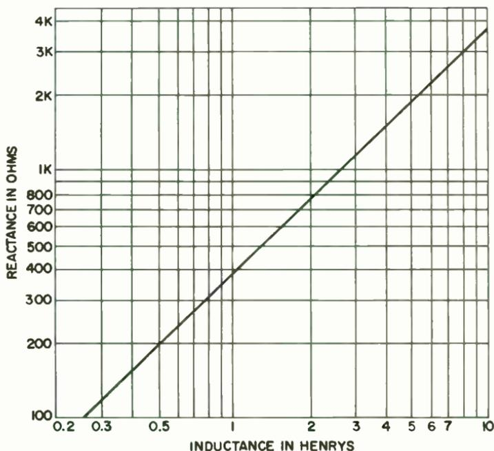
Fig. 7. Reactance of inductors at 60 cycles.
