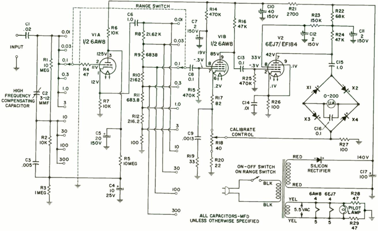
Frequency compensation provides flat response to 1 megacycle. (Courtesy of Heath Co.)
