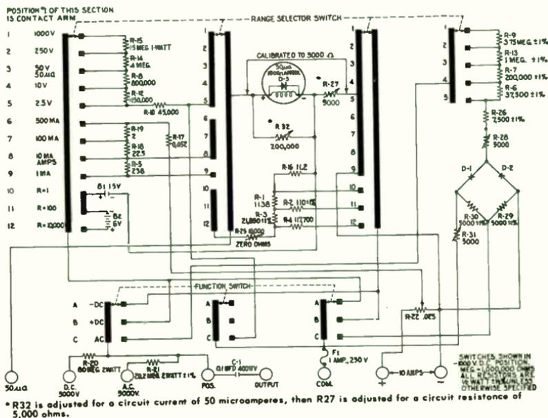
Ohmmeter section of a VOM may be protected by a fuse. (Courtesy of Simpson Electric Co.)
