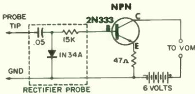
**Construction of a sensitive rectifier probe for checking signal-generator output.**
