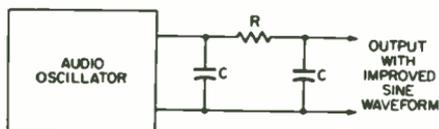
**An R-C low-pass filter for removing harmonics.**
