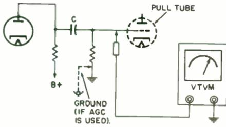
**Test setup for in-circuit test.**
