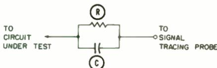
Wide-band voltage divider for signal-tracing probe.
