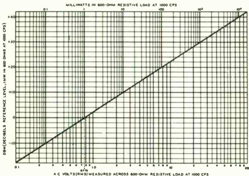
Graph for conversion of rms voltages to dbm values. (Courtesy of Radio Corporation of America.)
