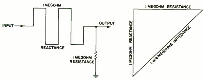
**Fig. 9. Resistance and reactance add at right angles.**
