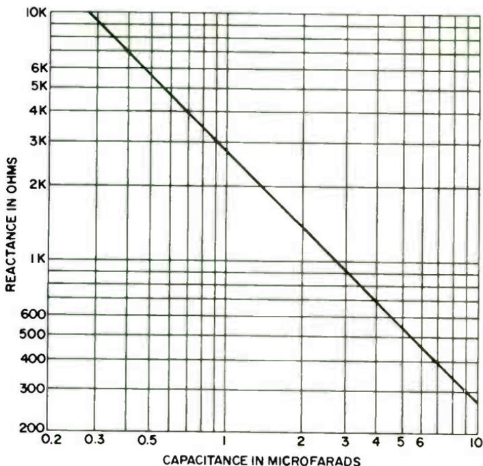
Fig. 6. Reactance of capacitors at 60 cycles.
