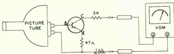
Checking raster brightness at low-brightness levels.
