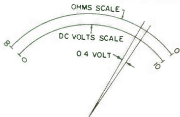
An accuracy of  $\pm 2\%$  corresponds to an interval of 0.4 volt on a 10-volt scale.
