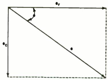
(B) Parallelogram voltage diagram.
