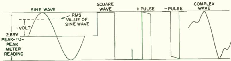
Fig. 3. Typical voltage waveforms.
