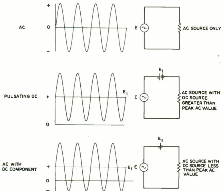
Fig. 5. Three basic classes of current.
