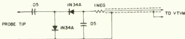
A peak-to-peak signal-tracing probe for a VTVM.
