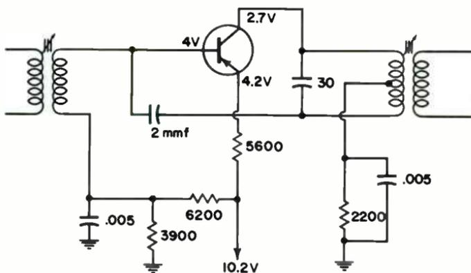
**(B) Leaky transistor can affect DC voltage distribution.**
