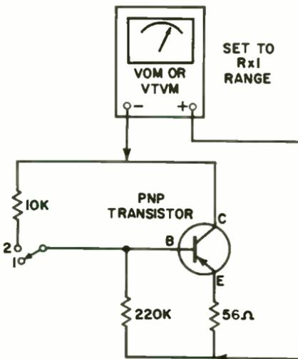
**Ohmmeter test of a transistor.**
