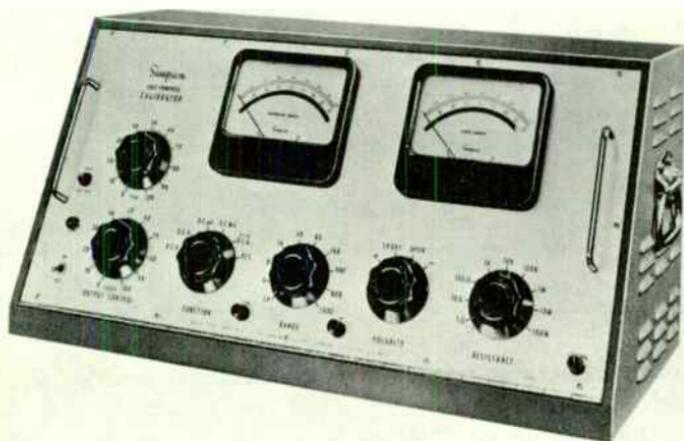
Typical calibrator for VOM's and VTVM's. (Courtesy of Simpson Electric Co.)
