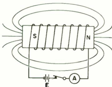
A-3. Expanding or contracting flux lines produce self-induction.
