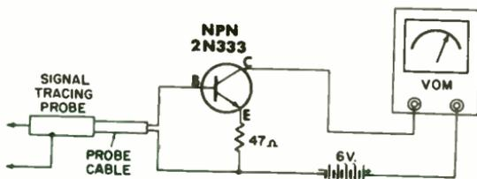
**Transistor probe amplifier.**
