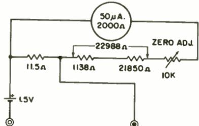
(B) Nominal circuit on R × 1 range includes resistance of test leads (not shown).
