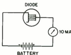
Fig. A-2. Current consists of electrons in motion.
