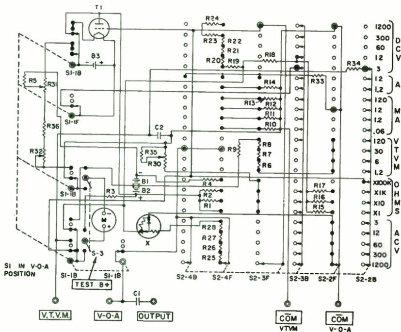
**VOM and VTVM combined in a single instrument. (Courtesy of Triplet Electrical Instr. Co.)**
