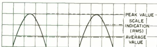
**Output of half-wave rectifier.**
