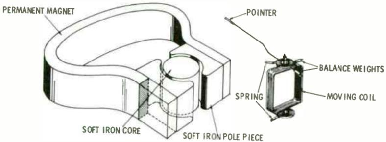
The moving coil may have as many as 2000 turns of wire 0.001 inch in diameter.
