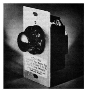
Courtesy International Resistance Company Fig. 6-1. A solid-state power control.
