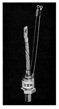
Courtesy International Rectifier Corp. Fig. 1-20. A seventy-ampere SCR.
