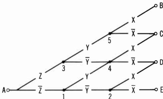
Fig. 8-5. Circuit representing three symmetric functions.
