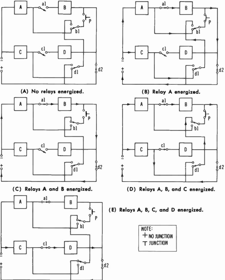
Fig. 3-17. Sequence switching with simple relays.
