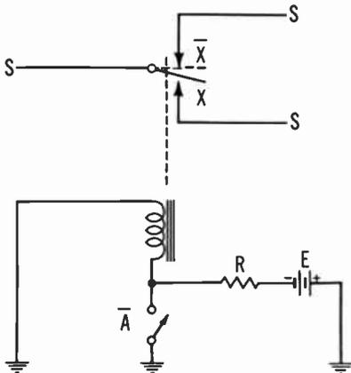
Fig. 8-11. Relay locking circuit.
