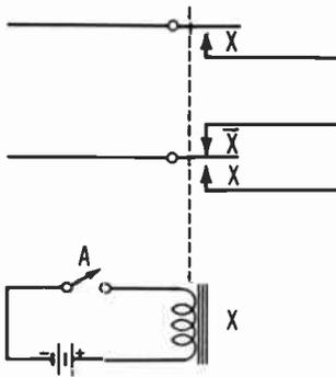
Fig. 8-10. Typical relay control circuit.
