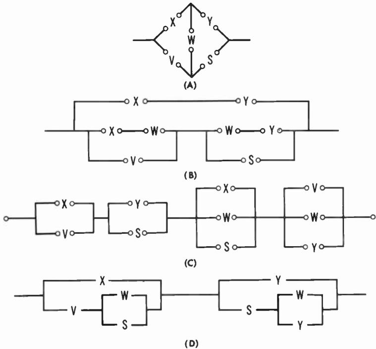
Fig. 8-4. Electrically-equivalent bridge circuits.
