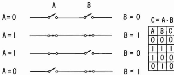
Fig. 2-2. AND circuit using switches.
