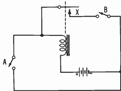
Fig. 8-12. Relay locking-circuit variation.
