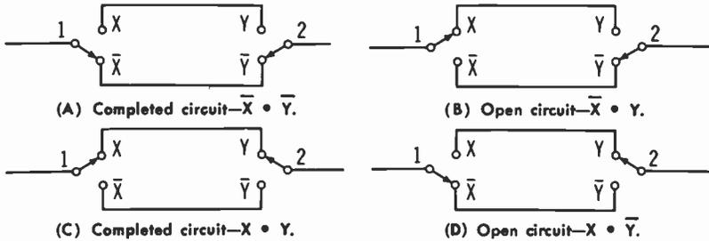
Fig. 3-14. A relay AND circuit.
