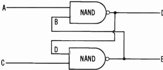
Fig. 6-9. A flip-flop constructed from NAND circuits.
