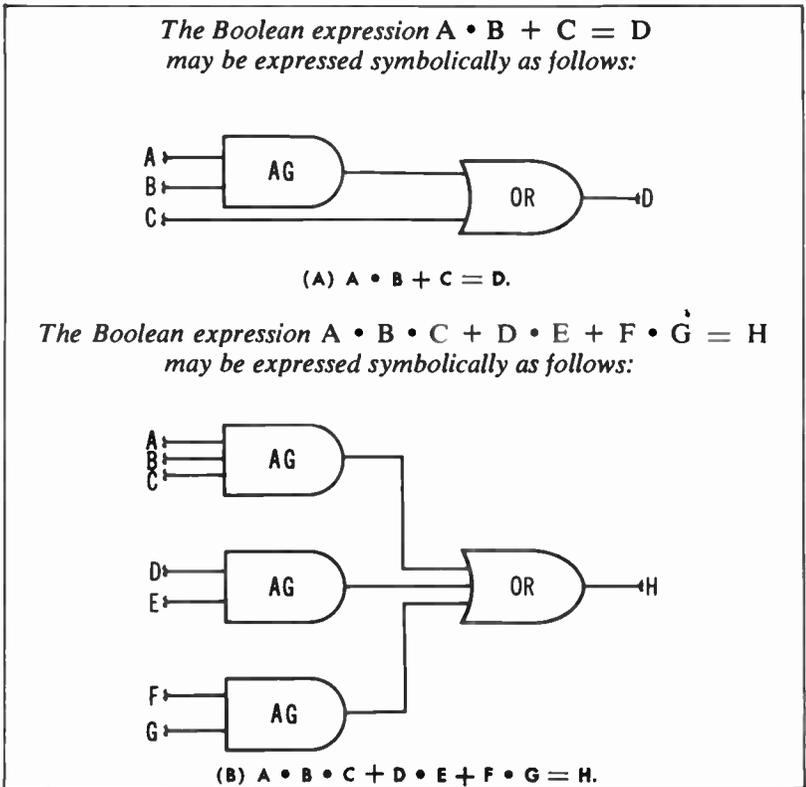
Fig. 4-15. Logical circuit arrangements.
