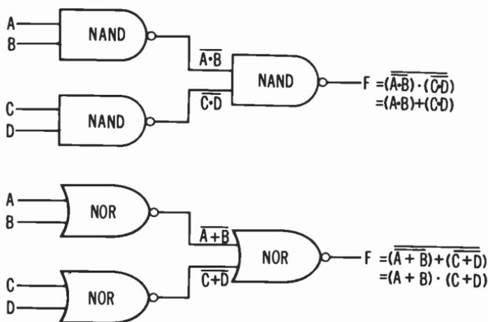
Fig. 4-21. Combinations of NAND and NOR logic.
