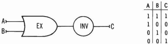
Fig. 7-6. Simplified circuit for logic used in Fig. 7-5.
