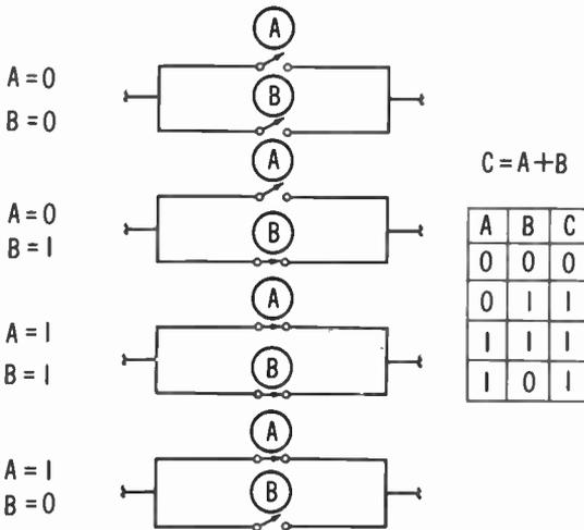
**Fig. 2-1. OR circuit using switches.**
