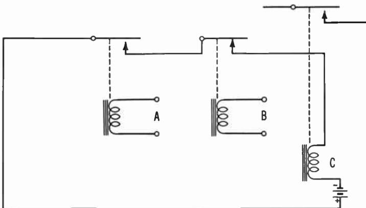
Fig. 8-15. Relay arrangement to obtain  $A \bullet \bar{B}$ .
