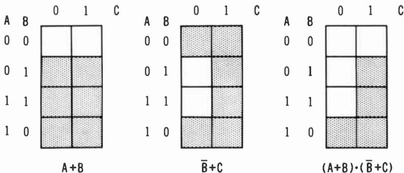
Fig. 6-6. Chart development of function  $X = (A + B) \cdot (\bar{B} + C)$ .
