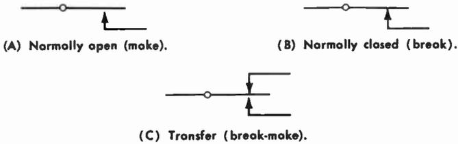
Fig. 8-8. Types of relay contacts.
