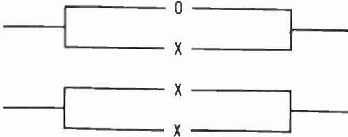
Fig. 3-3. Implementation of  $0 + X$  and  $X + X$  with switches.
