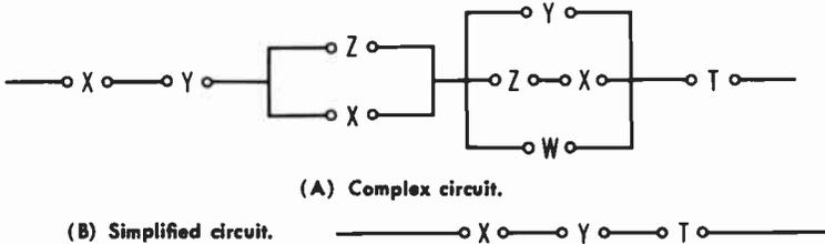
Fig. 3-11. Circuit simplification.
