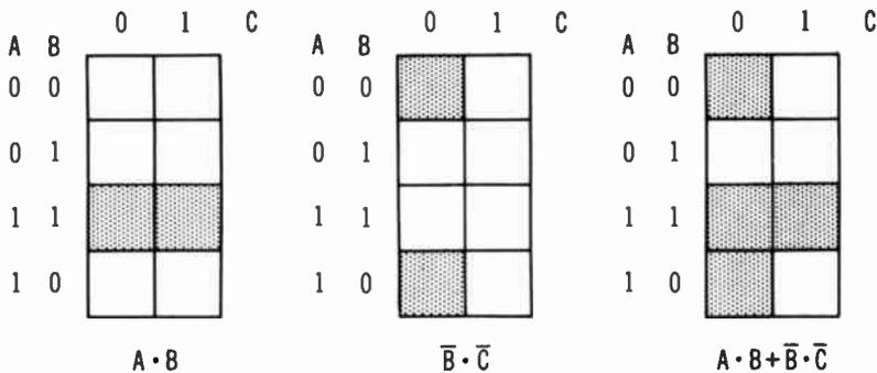
Fig. 6-5. Chart development of function  $X = A \cdot B + \bar{B} \cdot \bar{C}$ .
