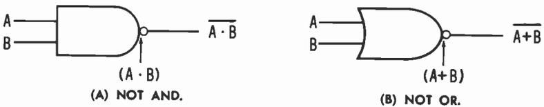
Fig. 4-3. Negation of logical functions.
