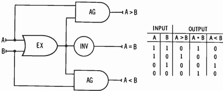
Fig. 7-7. Comparator logic.
