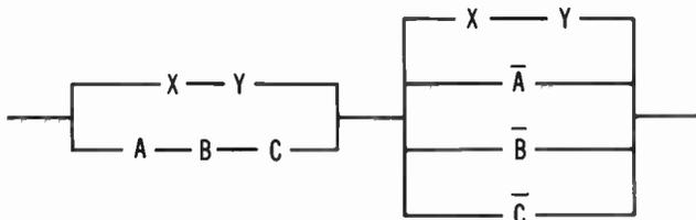
**Fig. 6-3. Example of complex switching circuit.**
