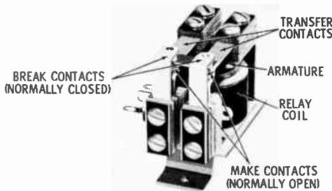
Fig. 8-9. Typical power relay.
