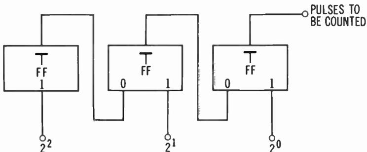
**Fig. 6-10. A three-bit, flip-flop counter.**
