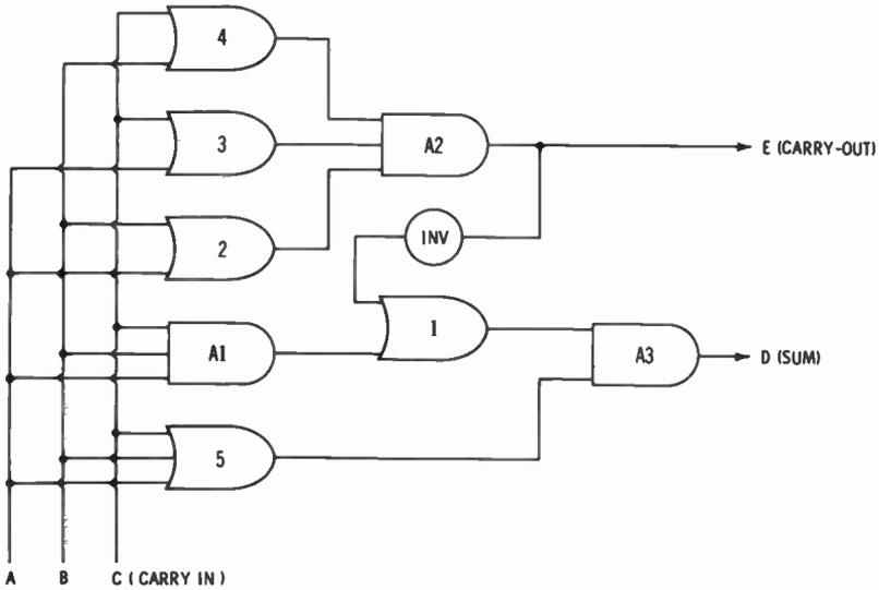
Fig. 4-28. Logical circuit for addition.
