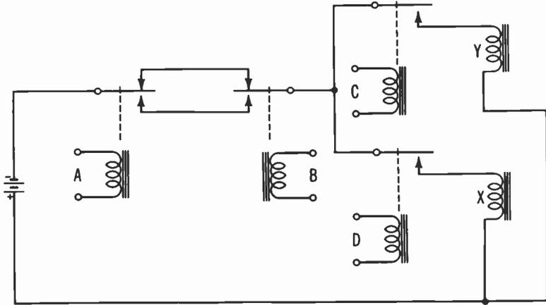
Fig. 8-16. Using relays to implement algebraic expression.
