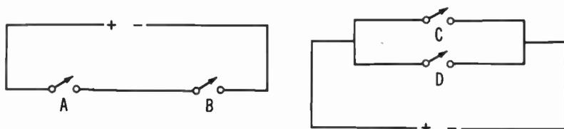
Fig. 3-13. Simple switch circuits.
