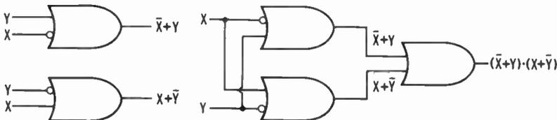
Fig. 4-17. How diagrams are developed from expressions.
