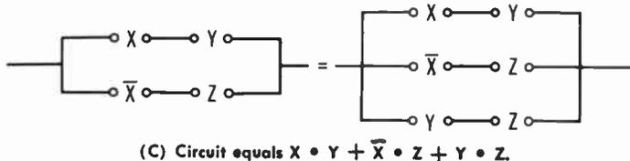
Fig. 3-12. Examples of equivalent logical circuits.
