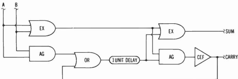
Fig. 4-26. Full-adder logic using exclusive OR.
