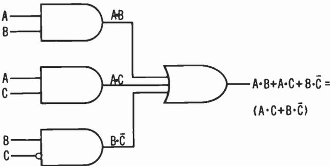
Fig. 4-14. Logical operation circuit.
