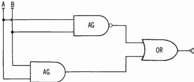
Fig. 7-5. Equalizer circuit logic.
